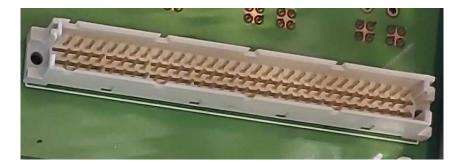
Deceptively similar non-standard connector for interchassis wiring:
