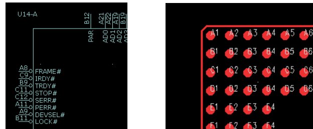
Schematic symbol and pcb decal both have corresponding alphanumeric pin numbers
