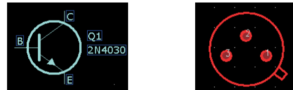
Schematic symbol with alphanumeric pin numbers mapping to pcb decal with numeric pin numbers
