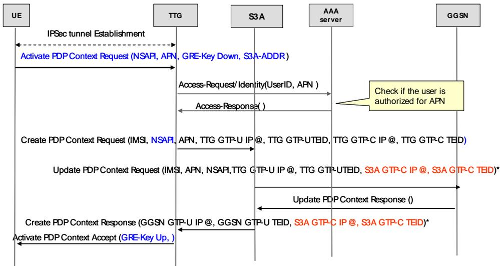
\*Depending on operator's configuration with regards to the user plane path rules, the user plane may go through the S3A . In this case, the S3A sends an Update PDP context request / Create PDP context response with its own TEID and IP addresses for control and user planes.
