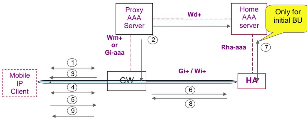
**Figure A.3: Use of MIPv6 with Diameter application**
