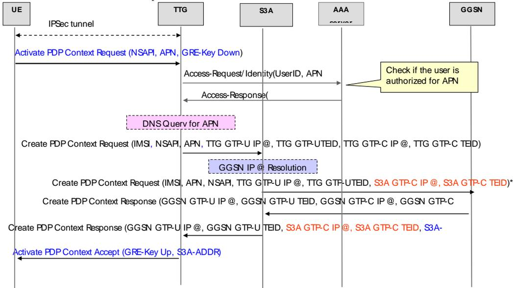
Figure 6.2.11 First PDP context activation on the I-WLAN side
