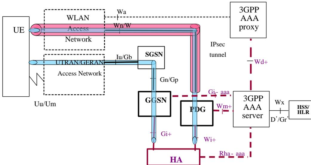
**Figure A.5: Use of MIPv6 or MIPv4 with co-CoA for GPRS-WLAN mobility**
