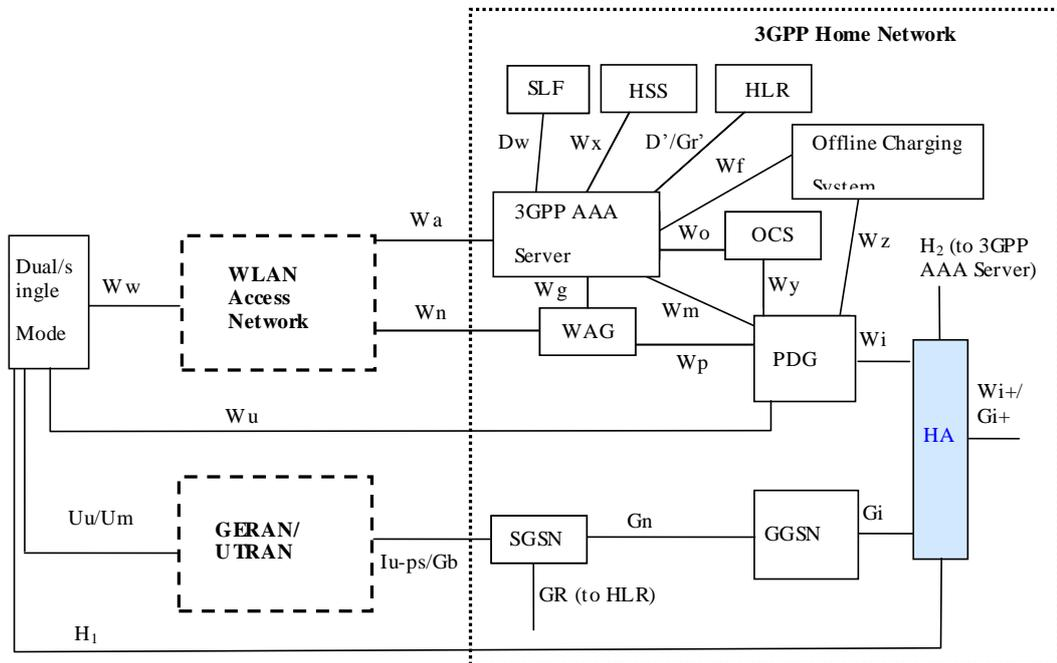
Figure 6.2.16 Alternative Non-Roaming Architecture for I-WLAN Mobility
