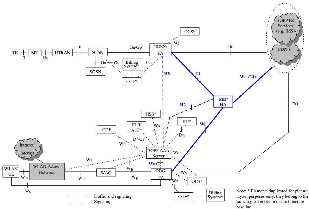
**Figure 6.2.20 Solution for GPRS-IWLAN mobility based on the MIPv4 FA protocol**
