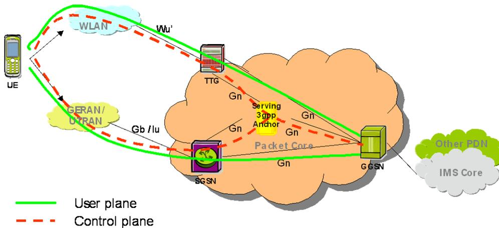
Figure 6.2.9 Handover mechanism for I-WLAN/3GPP Mobility
