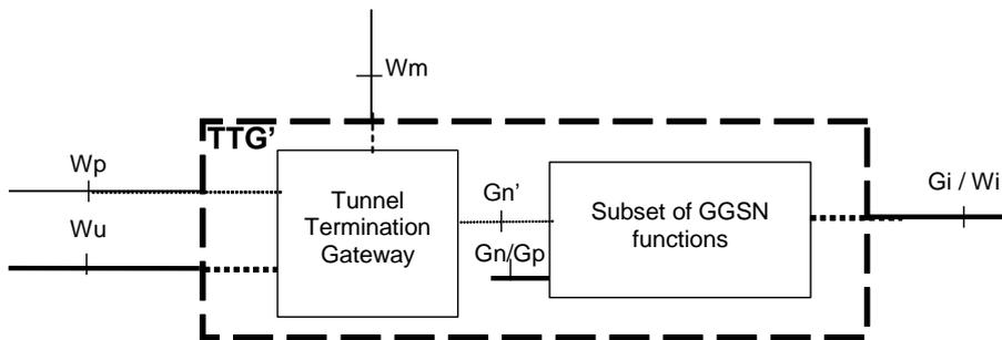
Figure 6.2.4 : TTG' implementation re-using GGSN functionality
