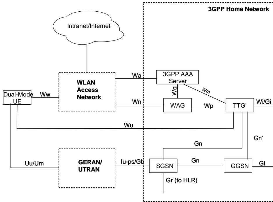
Figure 6.2.1 : Non-Roaming Architecture for I-WLAN Mobility
