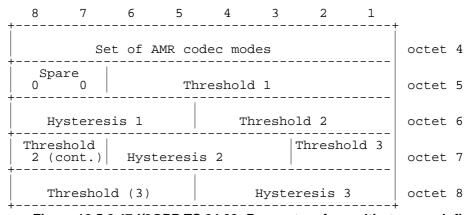
Figure 10.5.2.47d/3GPP TS 04.08: Parameters for multirate speech fiel for the MR version 1 when a set of four modes is chosen
