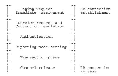
Figure 7.1/3GPP TS 04.08: Components of structured procedures
