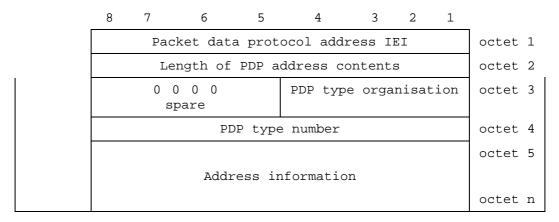
Figure 10.5.137/3GPP TS 04.08: Packet data protocol address information element
