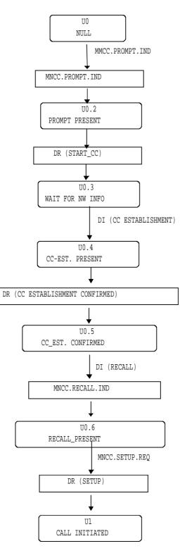
Figure 5.1a.1/3GPP TS 04.08: Overview call control protocol/MS side, extension:
