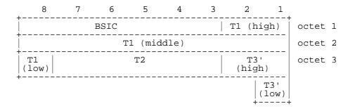
Figure 9.3/3GPP TS 04.08: Frame synchronization information element
