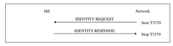
Figure 4.7.8/1 3GPP TS 04.08: Identification procedure
