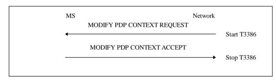
Figure 6.5/3GPP TS 04.08: PDP context modification procedure
