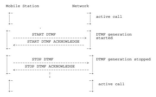
Figure 7.13/3GPP TS 04.08: DTMF protocol control
