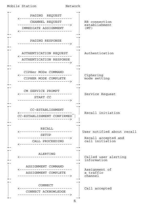
Figure 7.21/3GPP TS 04.08: Network initiated mobile originating call establishment with assignment after A and B party alerting
