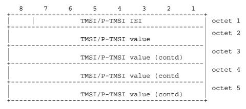
Figure 10.5.70/3GPP TS 04.08: TMSI/P-TMSI information element
