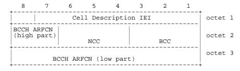
Figure 10.5.20/3GPP TS 04.08: Cell Description information element
