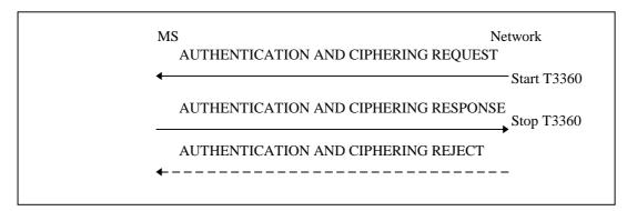
Figure 4.7.7/1 3GPP TS 04.08: Authentication and ciphering procedure
