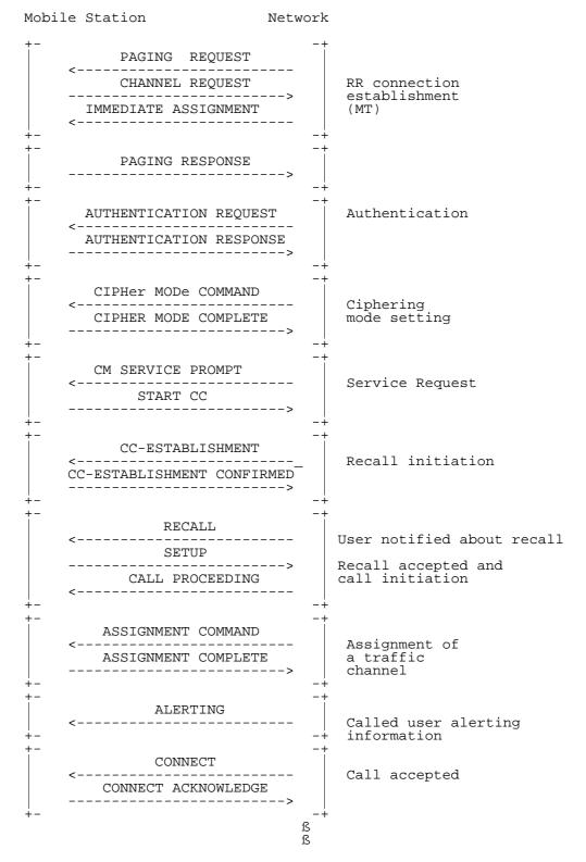
Figure 7.20/3GPP TS 04.08: Network initiated mobile originating call establishment with assignment before B party alerting
