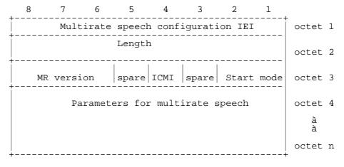
Figure 10.5.2.47/3GPP TS 04.08: MultiRate configuration information element
