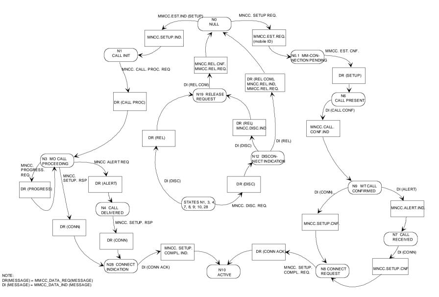
Figure 5.1b/3GPP TS 04.08: Overview call control protocol/Network side
