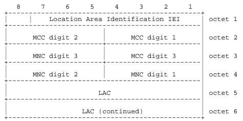
Figure 10.5.3/3GPP TS 04.08: Location Area Identification information element
