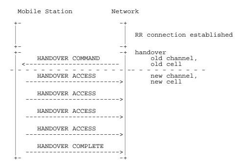
Figure 7.14/3GPP TS 04.08: Handover to a finely synchronized cell, successful case
