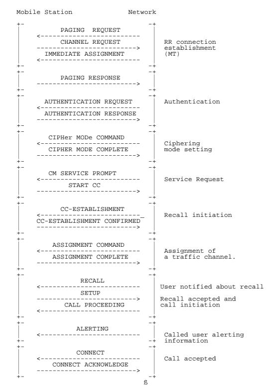
Figure 7.19/3GPP TS 04.08: Network initiated mobile originating call establishment with assignment before A party alerting
