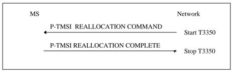
Figure 4.7.6/1 3GPP TS 04.08: P-TMSI reallocation procedure
