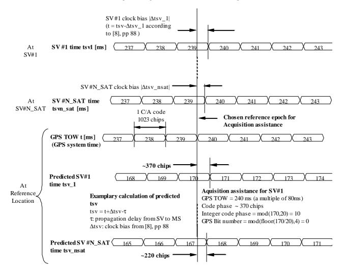
Figure A.2. Exemplary calculations of Acquisition Assistance fields.
