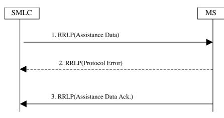
Figure 2.2: Assistance Data Delivery procedure
