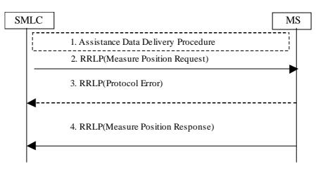
Figure 2.1: Position Measurement procedure
