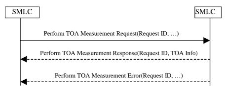
The Perform TOA Measurement Request message includes all the relevant details pertaining to the MS from which to measure signals. The Response message includes the results from one or several LMUs. An error message is returned by the SMLC Server in the case the request cannot be fulfilled (e.g. the LMUs can not measure the MS), or there is another error situation (syntax errors). The Request ID value in the Response, and the possible Error are the same as in the Request.
