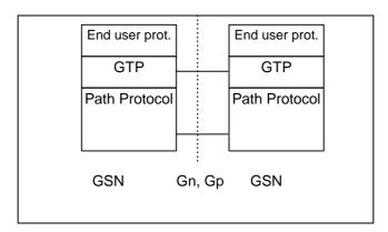
Figure 39: Transmission Plane - Protocol Stack
