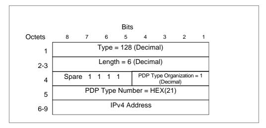
Figure 26: End User Address information element for IPv4
