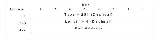
Figure 37: Charging Gateway Address information element
