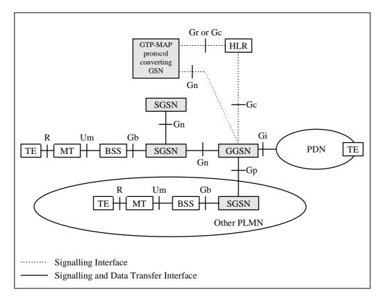
Figure 1: GPRS Logical Architecture with interface name denotations
