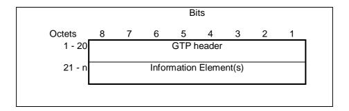
Figure 5: GTP header followed by subsequent Information Elements
