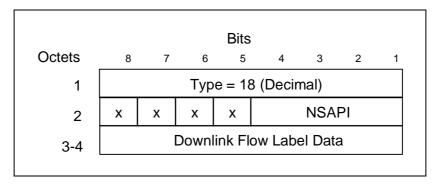
Figure 23: Flow Label Data II information element
