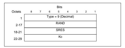
Figure 15: Authentication Triplet information element
