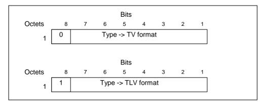
Figure 7: Type field for TV and TLV format
