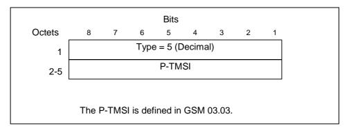
Figure 12: The Packet TMSI information element
