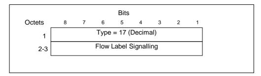
Figure 22: Flow Label Signalling information element
