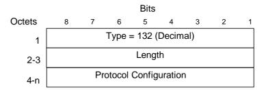
Figure 34: Protocol Configuration Options information element
