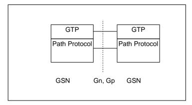
Figure 4: Signalling Plane - Protocol stack
