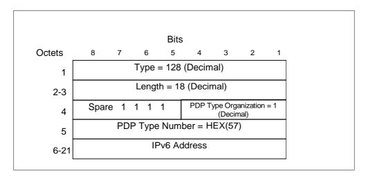
Figure 27: End User Address information element for IPv6
