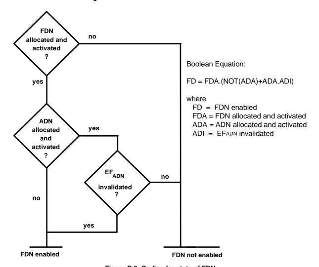
Figure C.6: Coding for state of FDN
