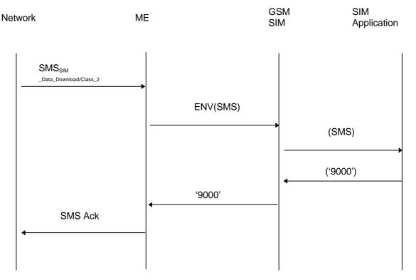
This shows the simple case where an SMS for SIM updating is received from the network, passed to the SIM by the ME and processed immediately by the SIM application. This requires no ME action except to acknowledge the SMS.
