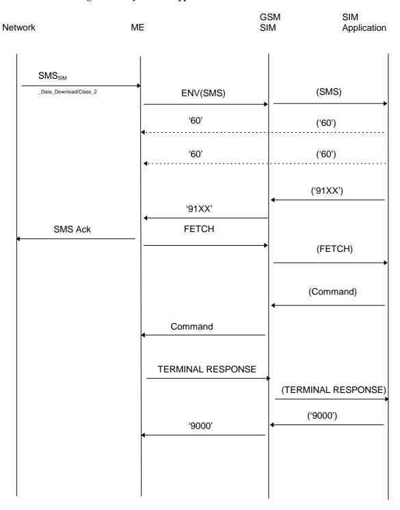
This shows the case where an SMS for SIM updating is received from the network, passed to the SIM by the ME and processed by the SIM application which then generates a command for action by the ME (e.g. PLAYTONE).
