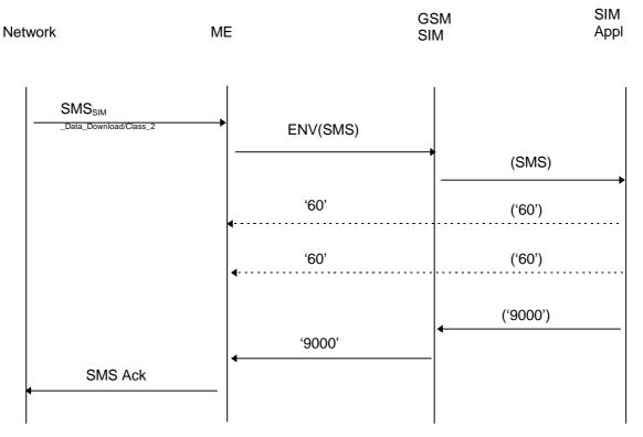
This shows the simple case where an SMS for SIM updating is received from the network, passed to the SIM by the ME and which requires some time to process by the SIM application. The processing time is "not long" and is obtained by the SIM application sending "null procedure bytes" to the ME. Each byte has the effect of restarting the work waiting time so that the ME does not abort the transaction before the SIM application has finished processing the command(s) sent in the SMS.
