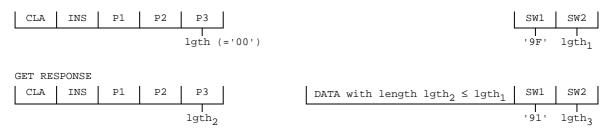
[Possible "normal GSM operation" command/response pairs]
