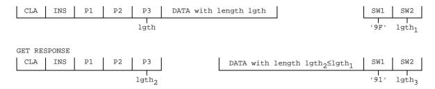
[Possible "normal GSM operation" command/response pairs]
