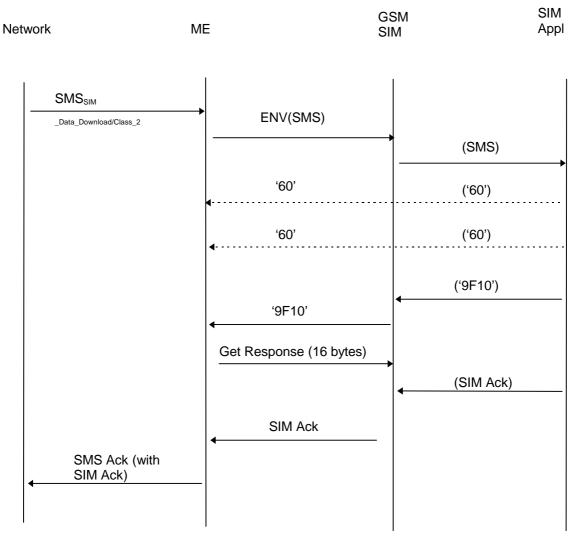
This shows the same case as previously where an SMS for SIM updating is received from the network, passed to the SIM by the ME and which requires some time to process by the SIM application. However in this case the SIM application has SIM acknowledgement data to include in the SMS acknowledgement being returned to the network by the ME.
