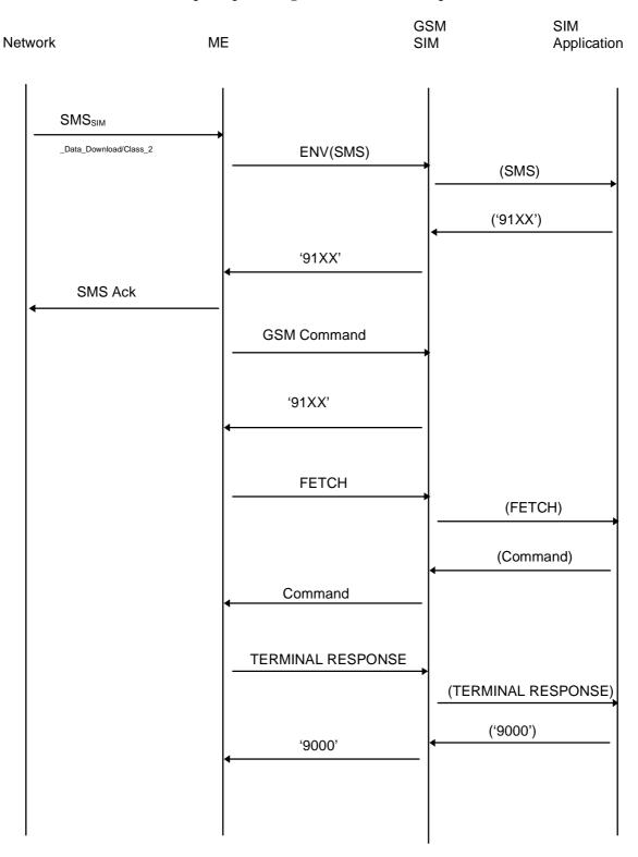
This shows the case where an SMS for SIM updating is received from the network, passed to the SIM by the ME and processed by the SIM application which then generates a command for action by the ME (e.g. PLAYTONE). However a normal GSM command requires processing before the ME can FETCH the command which the SIM is waiting to give it. The response to the normal GSM command is '91XX' in this case to remind the ME of the outstanding SIM application command request.
