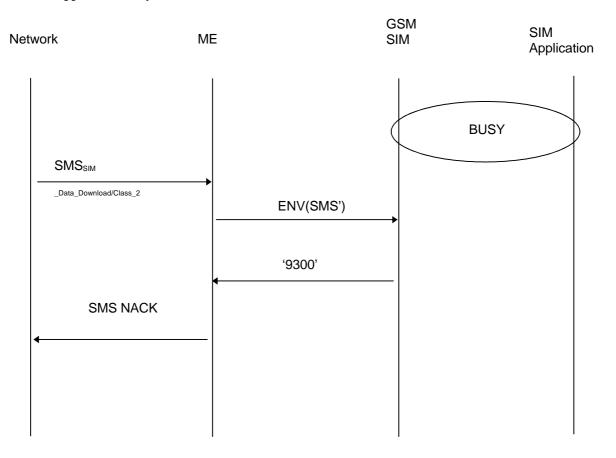
While the SIM application is busy processing a SMS for the SIM application arrives from the network and is sent to the SIM by the ME in the usual manner. The SIM operating system recognizes that the SIM application is busy, and it sends a busy response ('9300') to the ME. The ME then sends negative acknowledgement to the network. The responsibility for a retry rests with the network.
