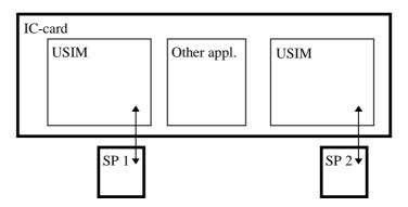
Figure 3 Example of a Multifunction UICC
