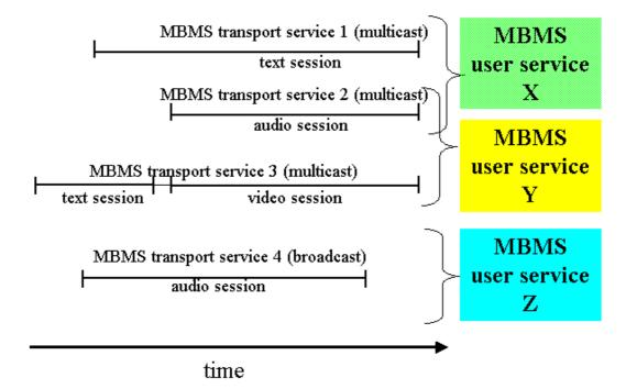
It shall be possible for an MBMS user service to make use of different application independent MBMS transport services at different times or in parallel. The MBMS transport services used may vary for instance in QoS parameters or target broadcast or multicast area.
