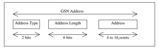
Figure 9: Structure of GSN Address
