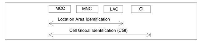
Figure 5: Structure of Cell Global Identification
