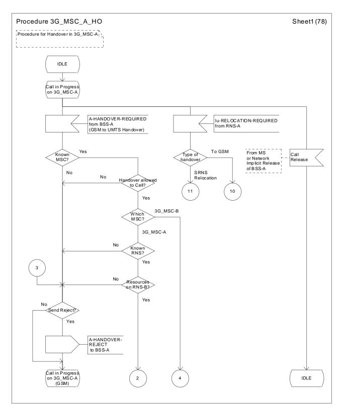
Figure 43 (sheet 1 of 78): Handover control procedure in 3G\_MSC-A
