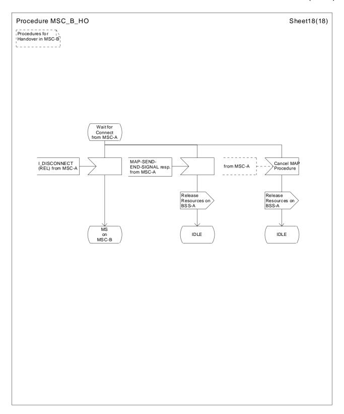
Figure 42 (Sheet 18 of 18): Handover control procedure in MSC-B
