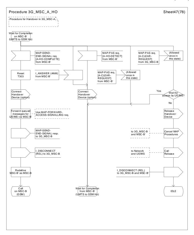
Figure 43 (sheet 47 of 78): Handover control procedure in 3G\_MSC-A
