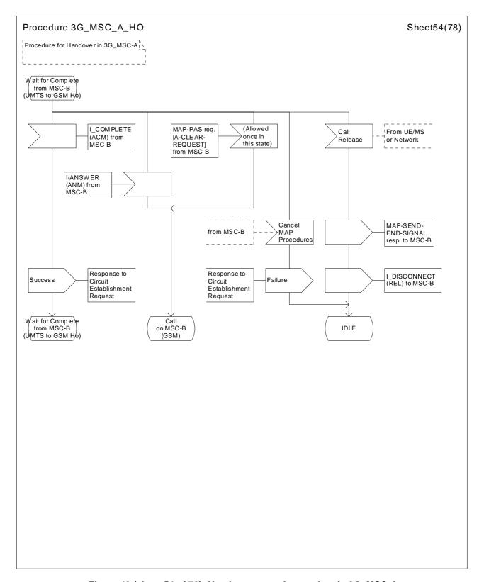
Figure 43 (sheet 54 of 78): Handover control procedure in 3G\_MSC-A
