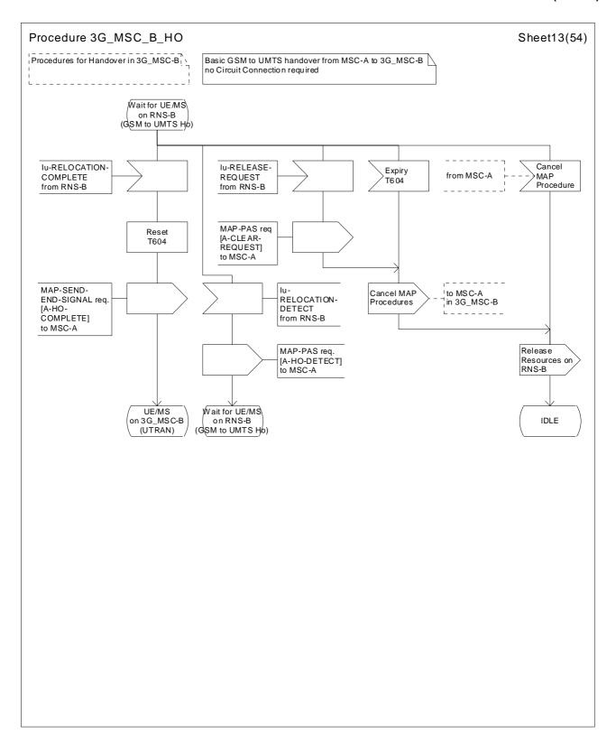
Figure 44 (sheet 13 of 54): Handover control procedure in 3G\_MSC-B
