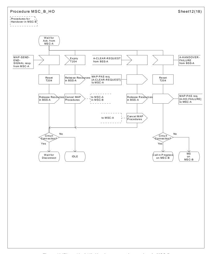
Figure 42 (Sheet 12 of 18): Handover control procedure in MSC-B
