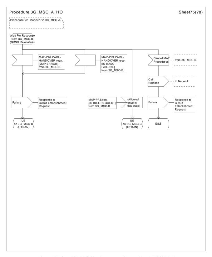
Figure 43 (sheet 75 of 78): Handover control procedure in 3G\_MSC-A
