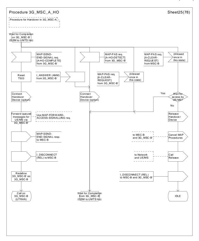
Figure 43 (sheet 25 of 78): Handover control procedure in 3G\_MSC-A
