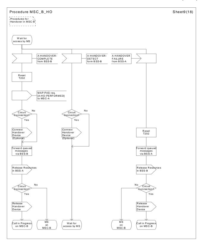
Figure 42 (Sheet 9 of 18): Handover control procedure in MSC-B
