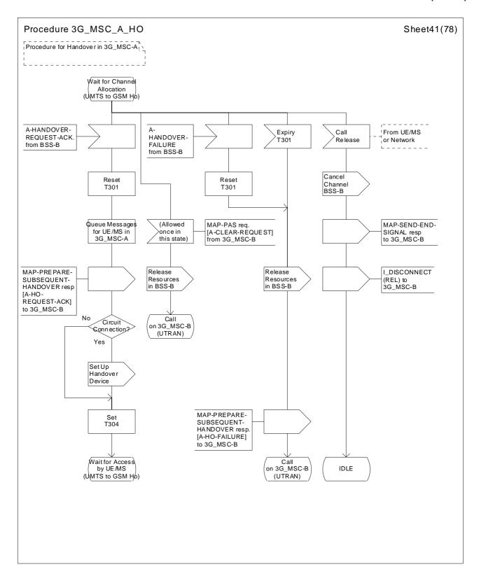
Figure 43 (sheet 41 of 78): Handover control procedure in 3G\_MSC-A
