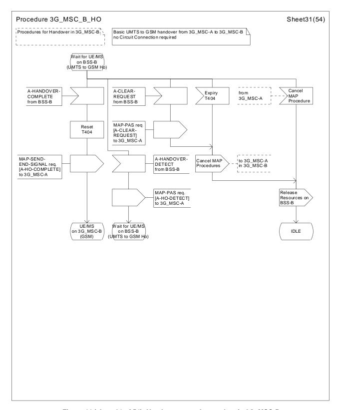
Figure 44 (sheet 31 of 54): Handover control procedure in 3G\_MSC-B
