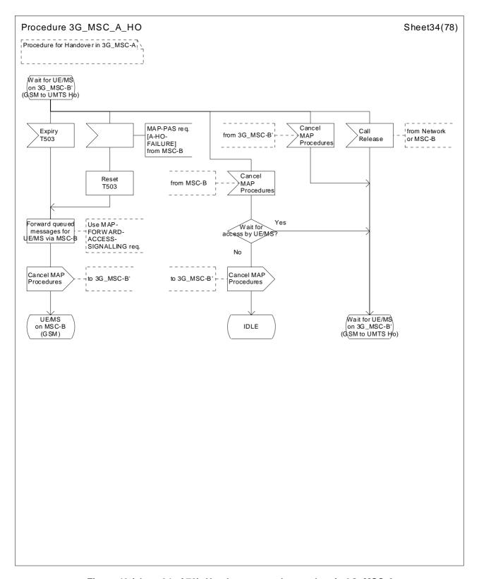
Figure 43 (sheet 34 of 78): Handover control procedure in 3G\_MSC-A
