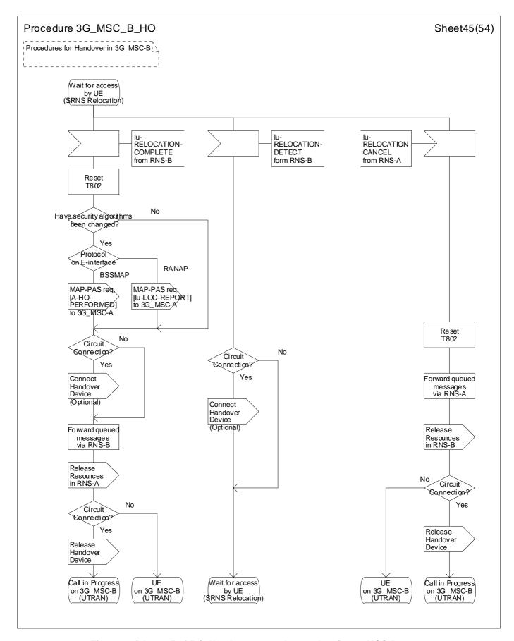
Figure 44 (sheet 45 of 54): Handover control procedure in 3G\_MSC-B
