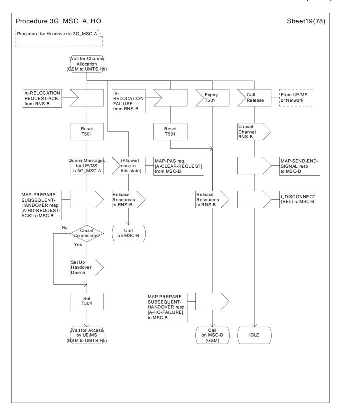
Figure 43 (sheet 19 of 78): Handover control procedure in 3G\_MSC-A
