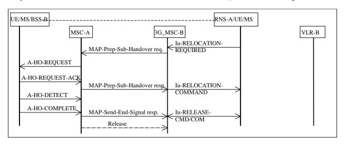
Figure 20: Subsequent UMTS to GSM handover procedure i): successful UMTS to GSM handover from 3G\_MSC-B to MSC-A using a circuit connection
