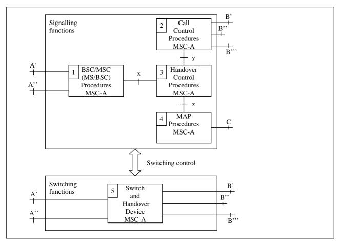
Figure 1: Functional composition of the controlling MSC (MSC-A) for supporting handover
