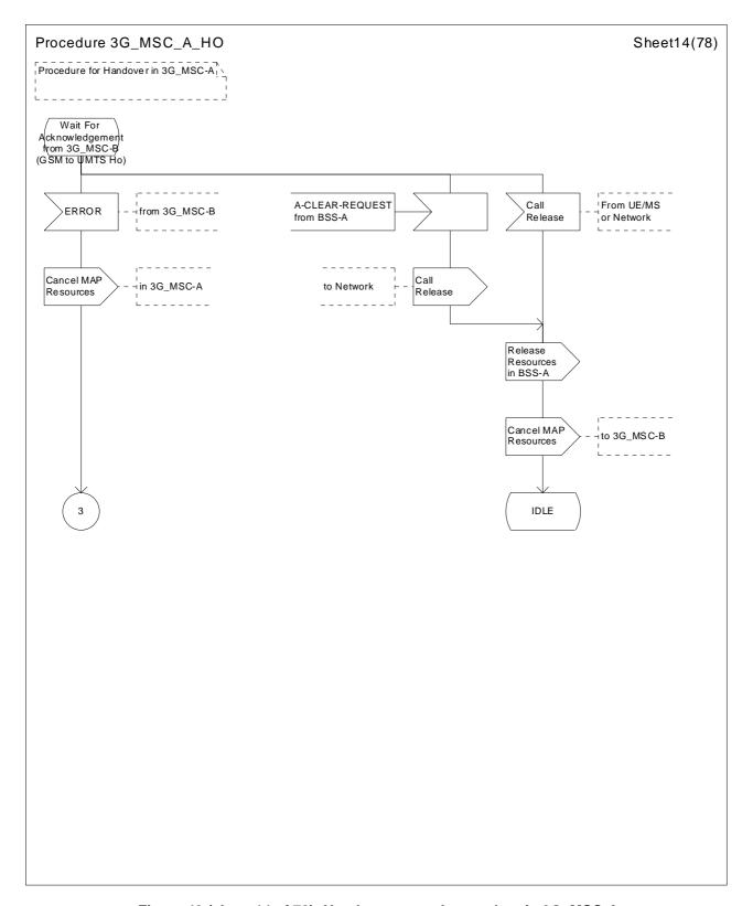
Figure 43 (sheet 14 of 78): Handover control procedure in 3G\_MSC-A
