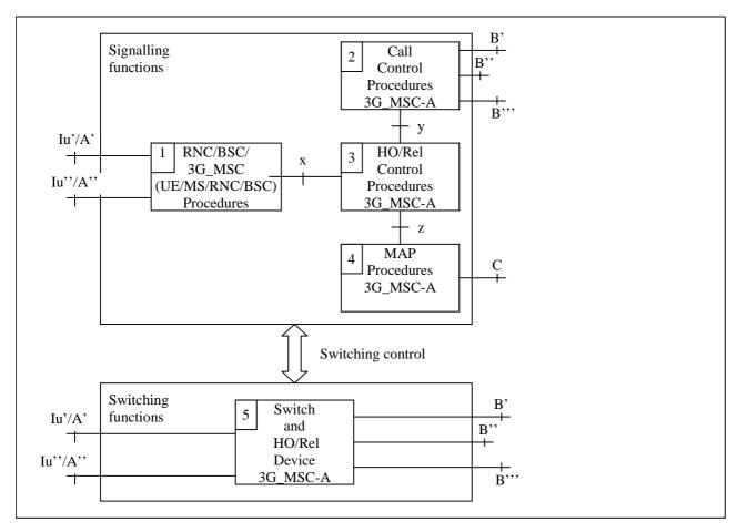
Figure 4: Functional composition of the controlling 3G\_MSC (3G\_MSC-A) for supporting handover/relocation
