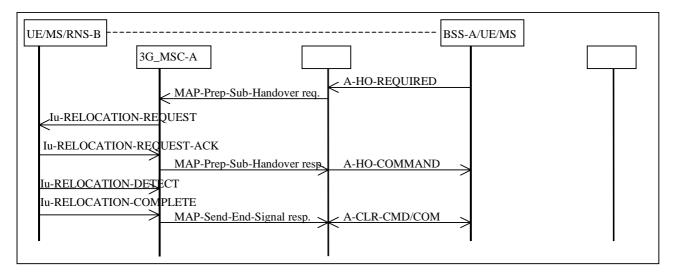
Figure 28: Subsequent GSM to UMTS handover procedure i): Successful handover from MSC-B to 3G\_MSC-A not requiring a circuit connection
