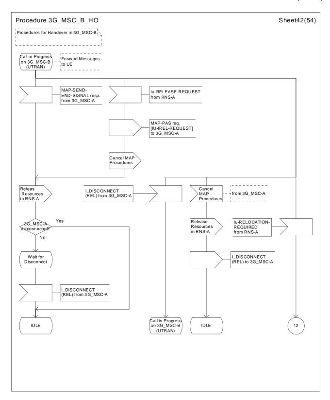
Figure 44 (sheet 42 of 54): Handover control procedure in 3G\_MSC-B
