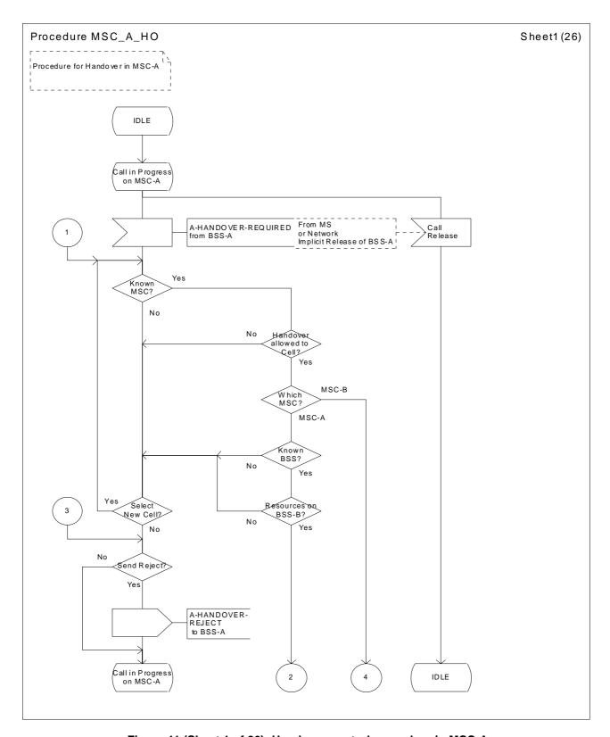
Figure 41 (Sheet 1 of 26): Handover control procedure in MSC-A
