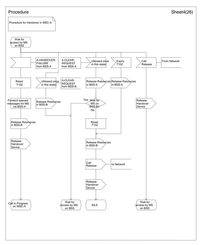
Figure 41 (Sheet 4 of 26): Handover control procedure in MSC-A
