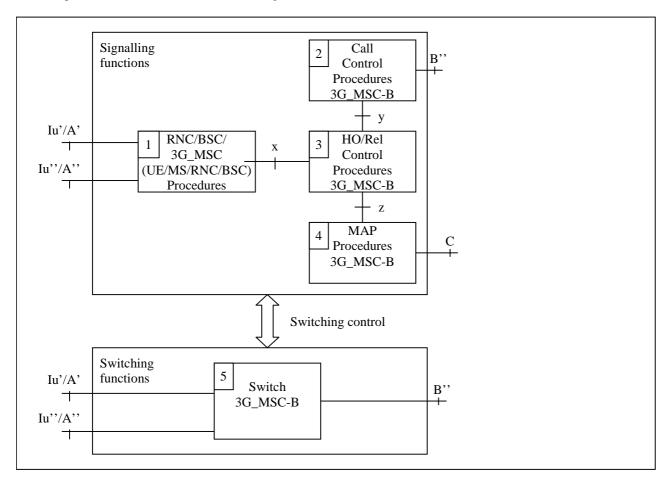
Figure 6: Functional composition of 3G\_MSC-B for supporting handover/relocation
