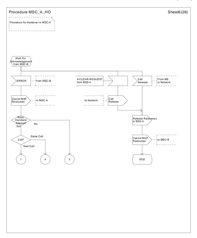
Figure 41 (Sheet 6 of 26): Handover control procedure in MSC-A
