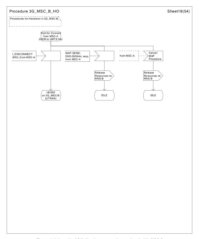
Figure 44 (sheet 18 of 54): Handover control procedure in 3G\_MSC-B
