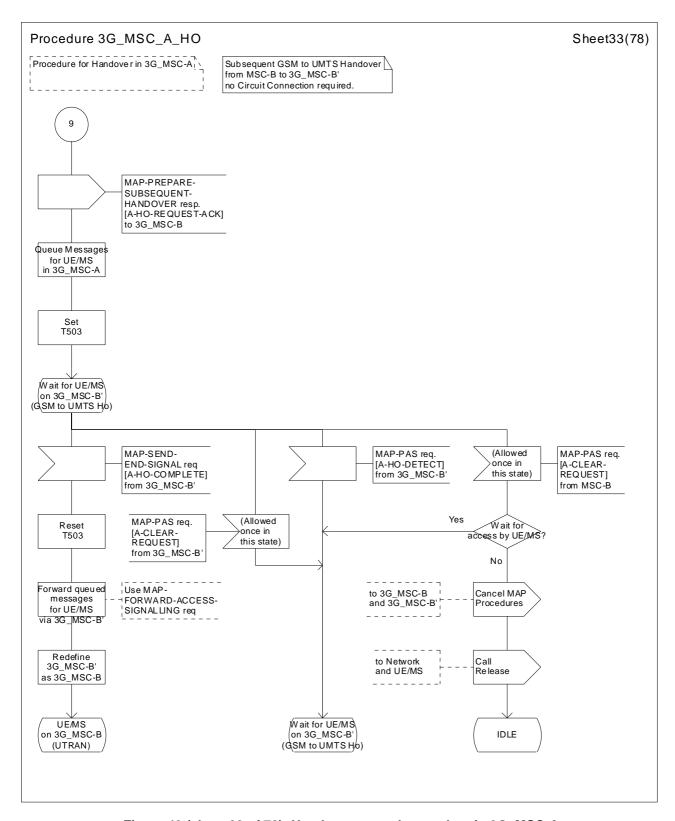
Figure 43 (sheet 33 of 78): Handover control procedure in 3G\_MSC-A
