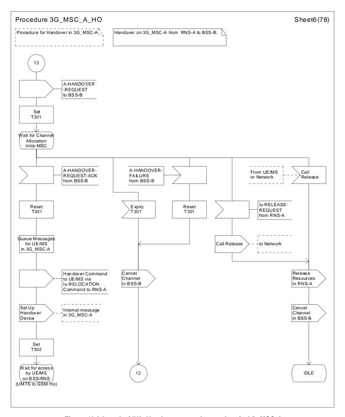
Figure 43 (sheet 6 of 78): Handover control procedure in 3G\_MSC-A
