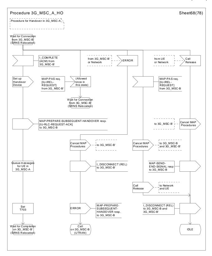
Figure 43 (sheet 68 of 78): Handover control procedure in 3G\_MSC-A
