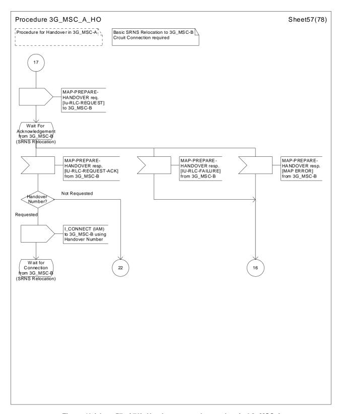
Figure 43 (sheet 57 of 78): Handover control procedure in 3G\_MSC-A
