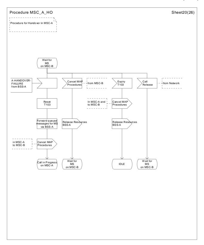
Figure 41 (Sheet 20 of 26): Handover control procedure in MSC-A
