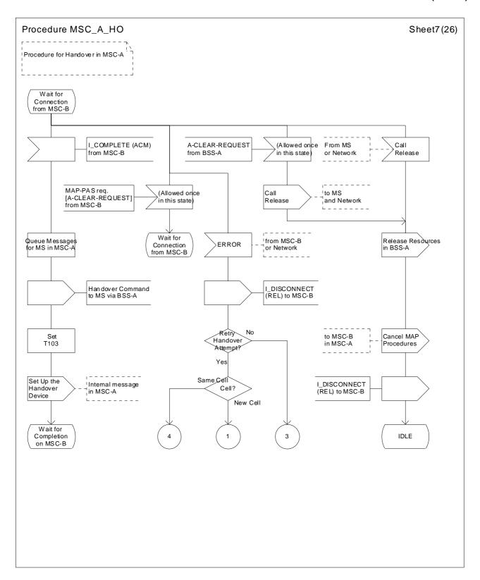
Figure 41 (Sheet 7 of 26): Handover control procedure in MSC-A
