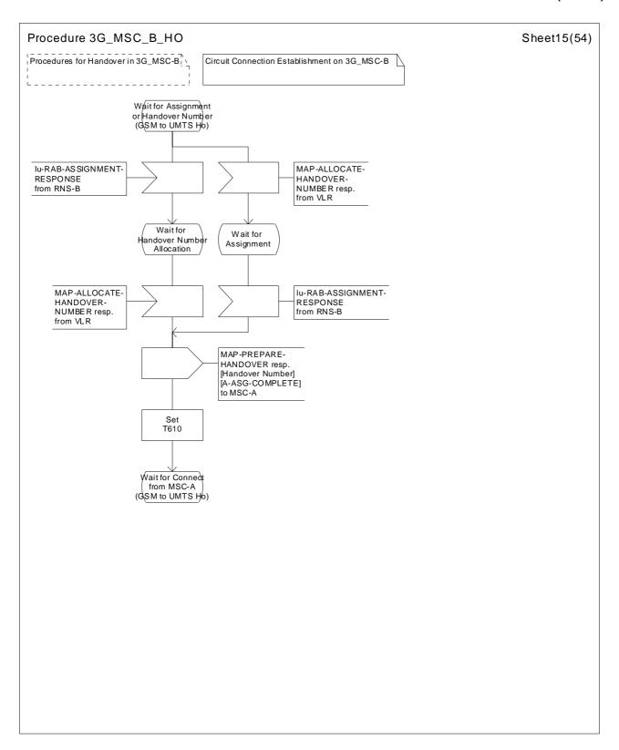
Figure 44 (sheet 15 of 54): Handover control procedure in 3G\_MSC-B
