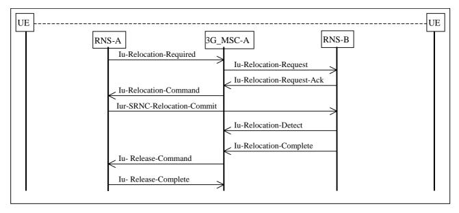
Figure 10 Basic intra-3G MSC SRNS Relocation Procedure
