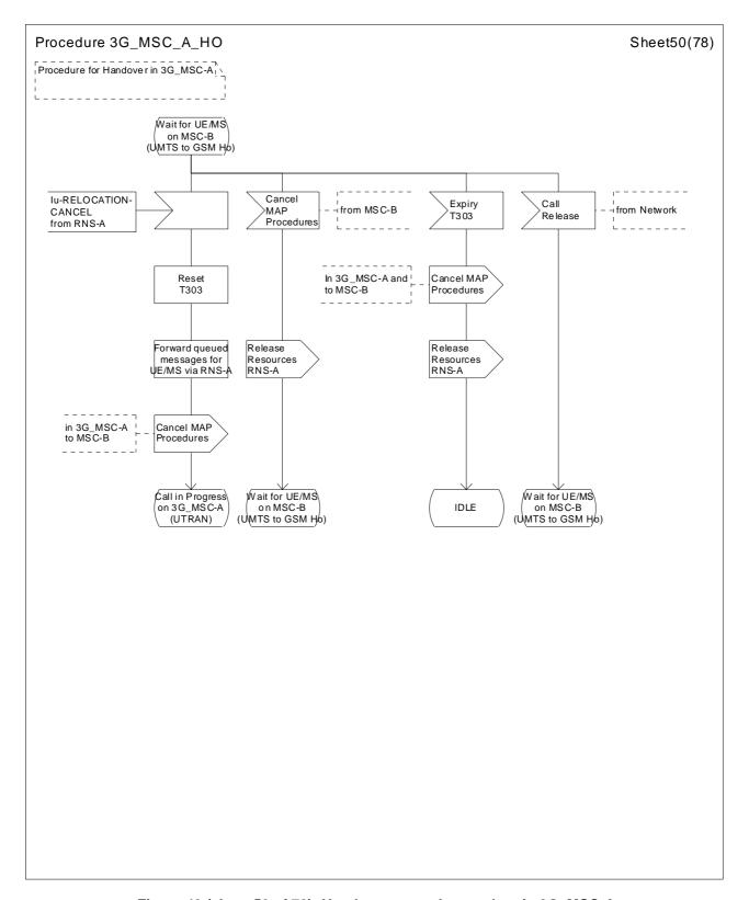
Figure 43 (sheet 50 of 78): Handover control procedure in 3G\_MSC-A
