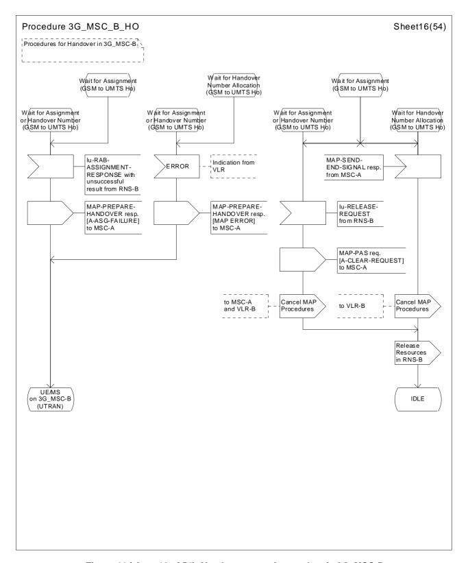
Figure 44 (sheet 16 of 54): Handover control procedure in 3G\_MSC-B
