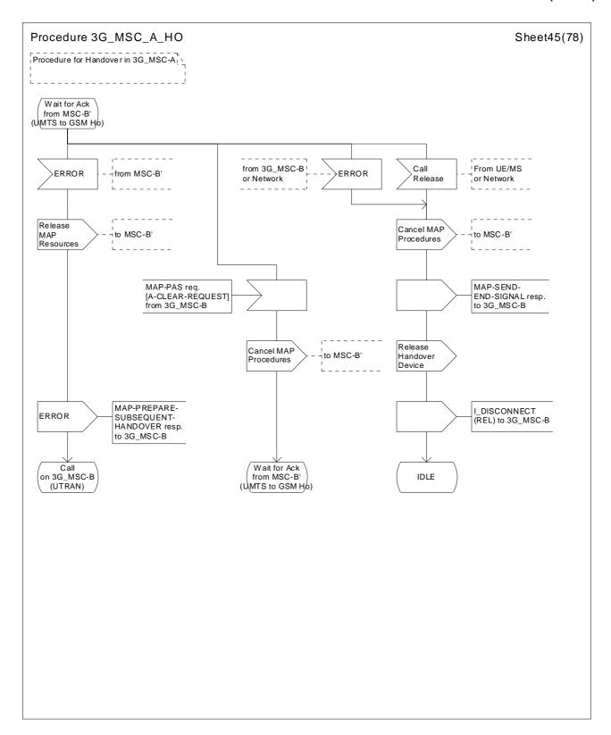
Figure 43 (sheet 45 of 78): Handover control procedure in 3G\_MSC-A
