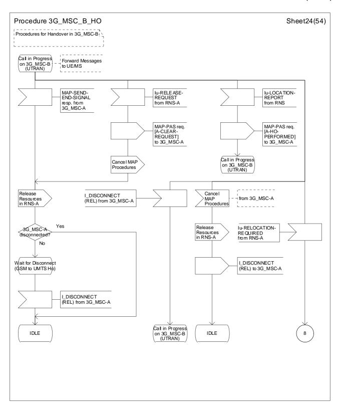
Figure 44 (sheet 24 of 54): Handover control procedure in 3G\_MSC-B
