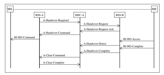
Figure 7: Basic External Intra-MSC Handover Procedure
