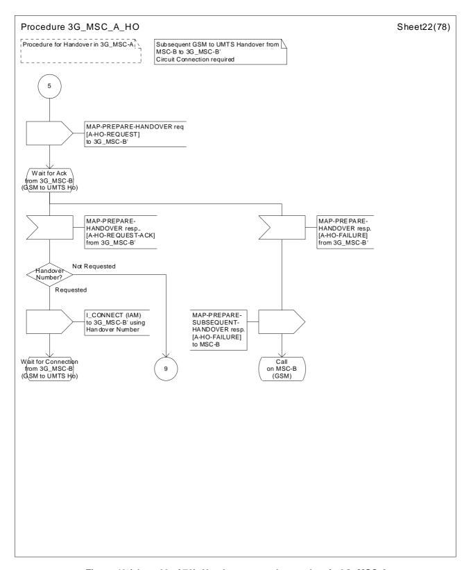
Figure 43 (sheet 22 of 78): Handover control procedure in 3G\_MSC-A
