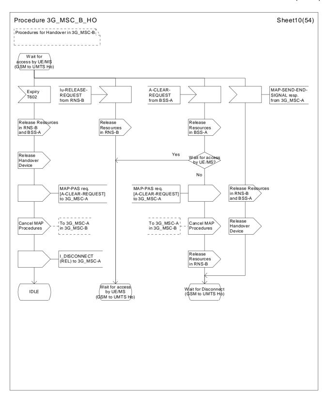
Figure 44 (sheet 10 of 54): Handover control procedure in 3G\_MSC-B
