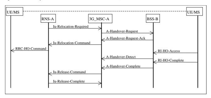
Figure 8: Basic Intra-3G\_MSC Handover from UMTS to GSM Procedure
