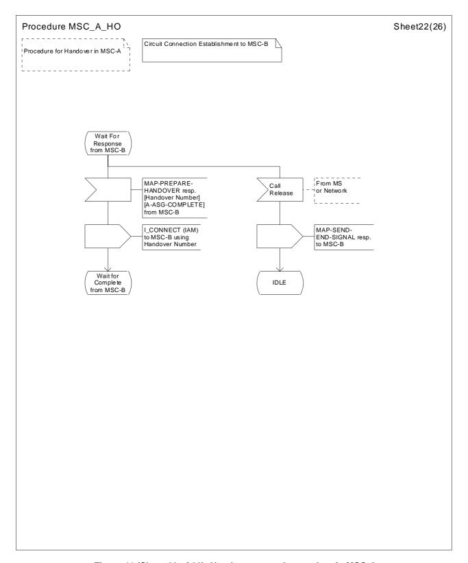
Figure 41 (Sheet 22 of 26): Handover control procedure in MSC-A
