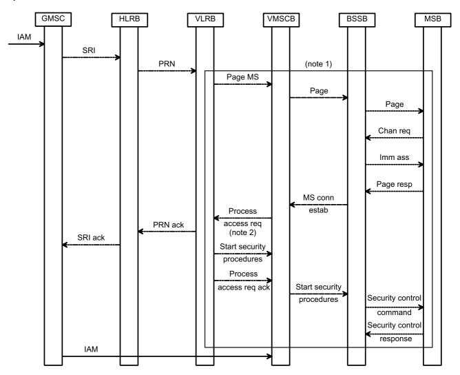
Figure 4: Information flow for retrieval of routeing information for a basic mobile terminated call
