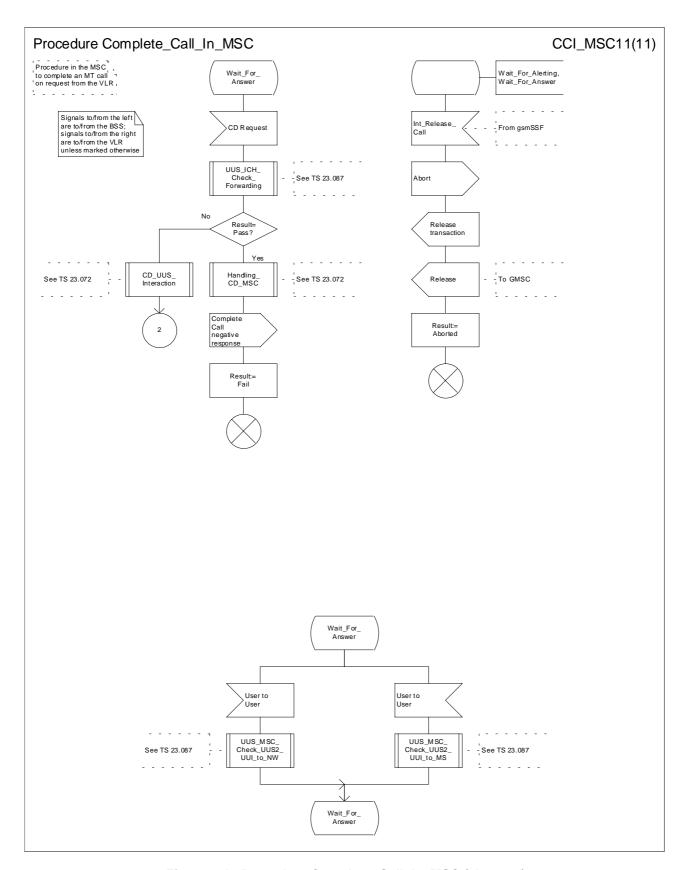
Figure 69k: Procedure Complete\_Call\_In\_MSC (sheet 11)
