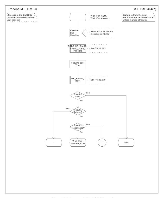
Figure 35d: Process MT\_GMSC (sheet 4)
