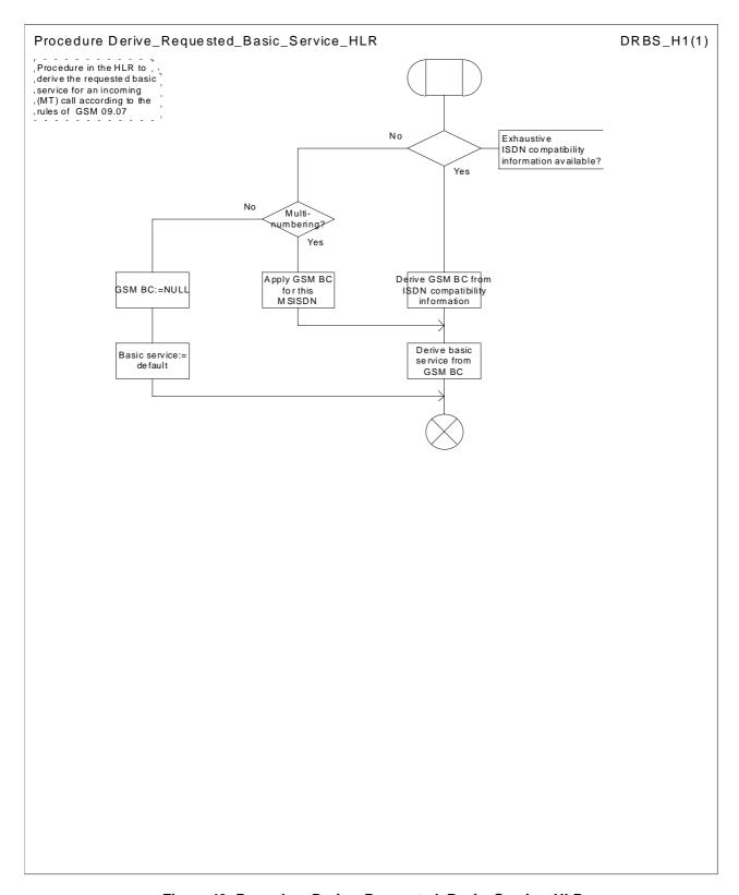
Figure 49: Procedure Derive\_Requested\_Basic\_Service\_HLR
