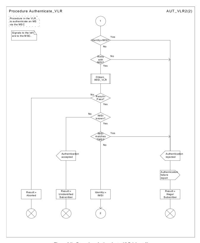
Figure 24b: Procedure Authenticate\_VLR (sheet 2)
