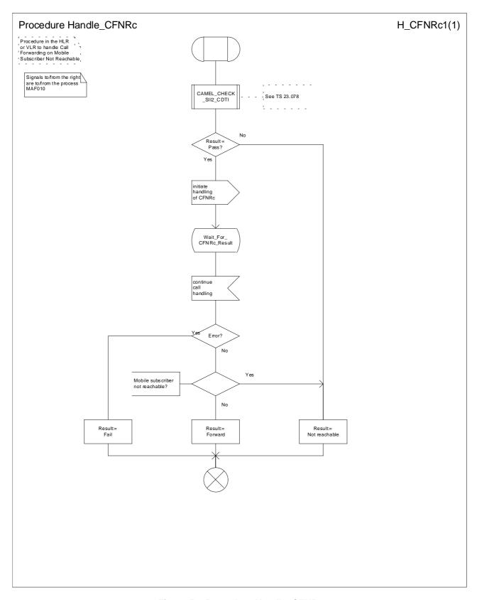
Figure 53: Procedure Handle\_CFNRc
