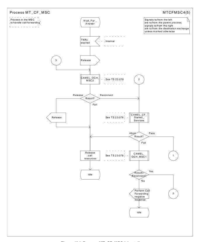
Figure 42d: Process MT\_CF\_MSC (sheet 4)
