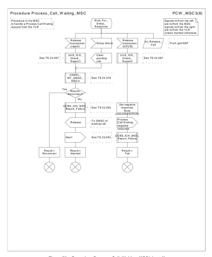
Figure 70c: Procedure Process\_Call\_Waiting\_MSC(sheet 3)
