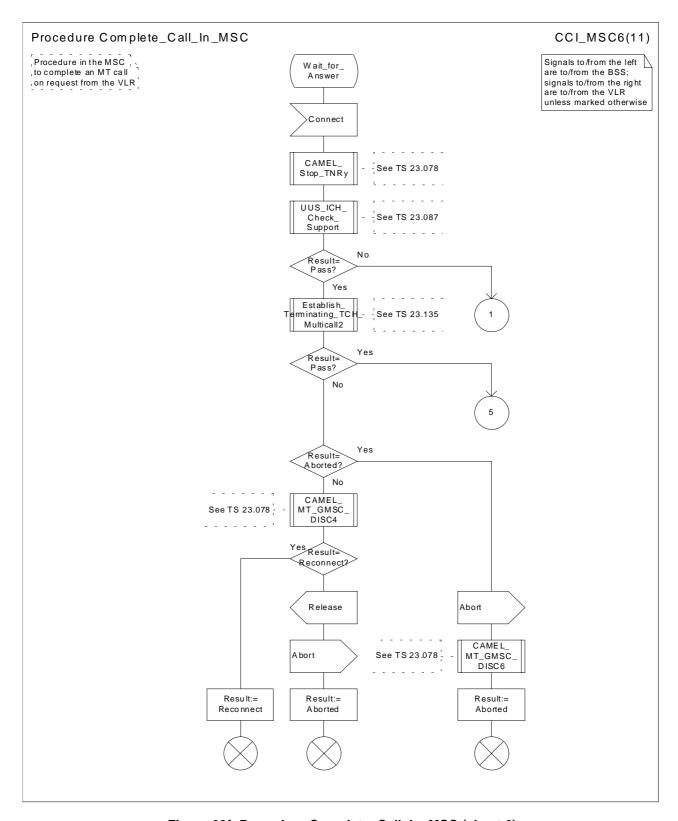
Figure 69f: Procedure Complete\_Call\_In\_MSC (sheet 6)
