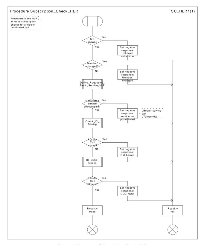
Figure 45: Procedure Subscription\_Check\_HLR
