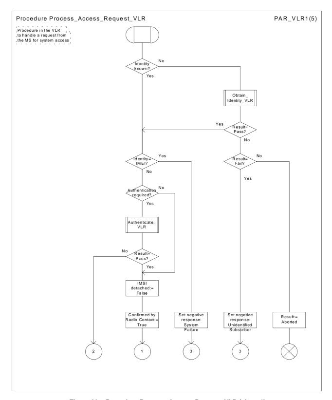
Figure 20a: Procedure Process\_Access\_Request\_VLR (sheet 1)
