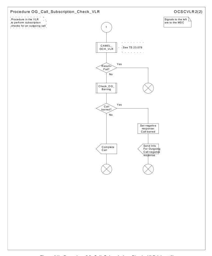
Figure 21b: Procedure OG\_Call\_Subscription\_Check \_VLR (sheet 2)
