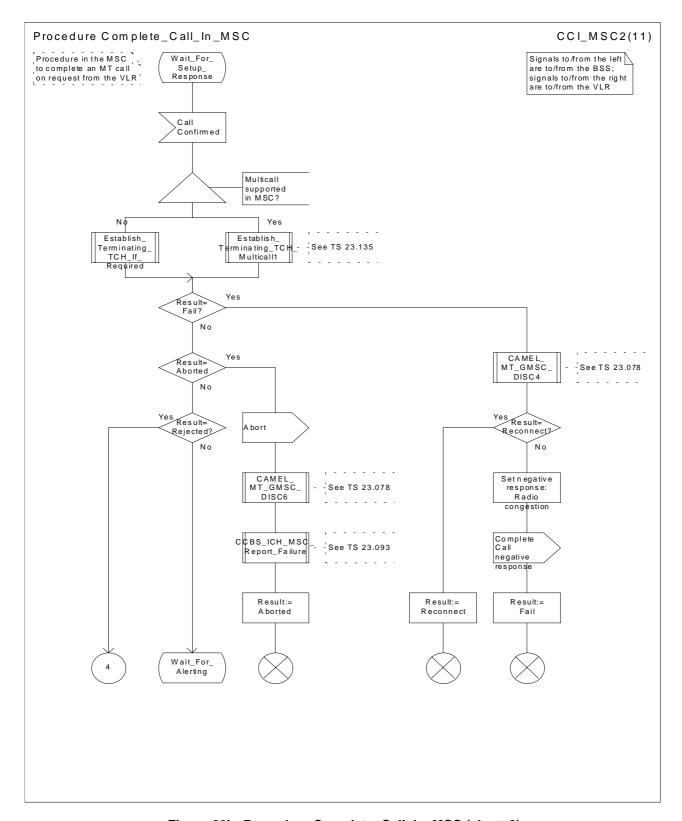
Figure 69b: Procedure Complete\_Call\_In\_MSC (sheet 2)
