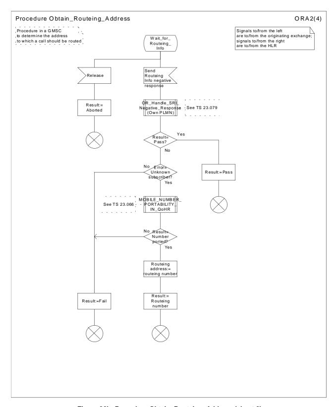
Figure 36b: Procedure Obtain\_Routeing\_Address (sheet 2)
