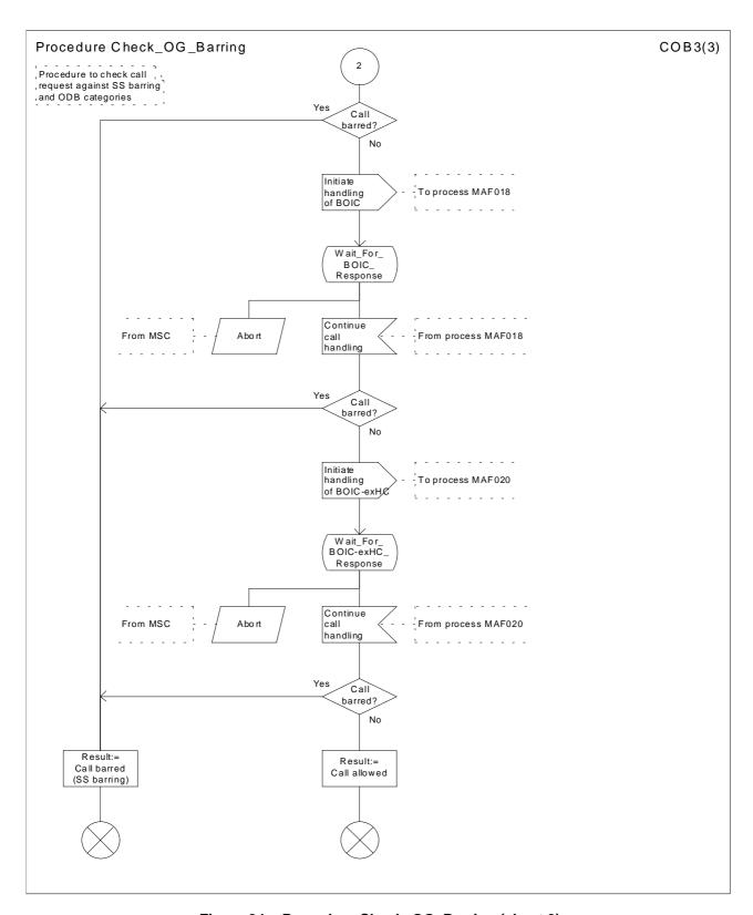
Figure 34c: Procedure Check\_OG\_Barring (sheet 3)
