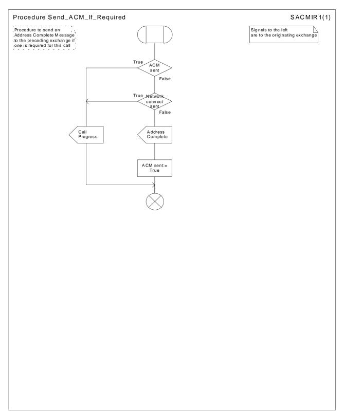
Figure 37: Procedure Send\_ACM\_If\_Required
