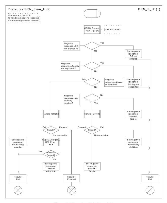
Figure 47: Procedure PRN\_Error\_HLR
