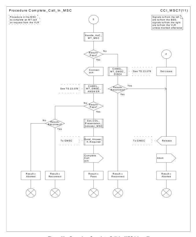
Figure 69g: Procedure Complete\_Call\_In\_MSC (sheet 7)
