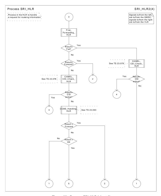
Figure 43b: Process SRI\_HLR (sheet 2)
