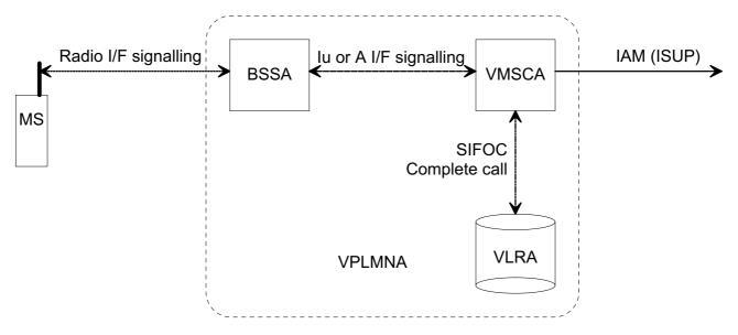
Figure 1: Architecture for a basic mobile originated call
