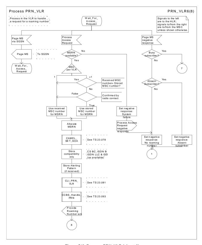
Figure 54f: Process PRN\_VLR (sheet 6)
