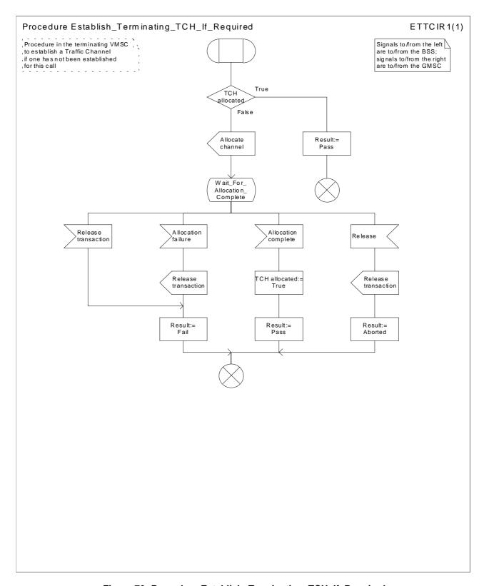
Figure 73: Procedure Establish\_Terminating\_TCH\_If\_Required
