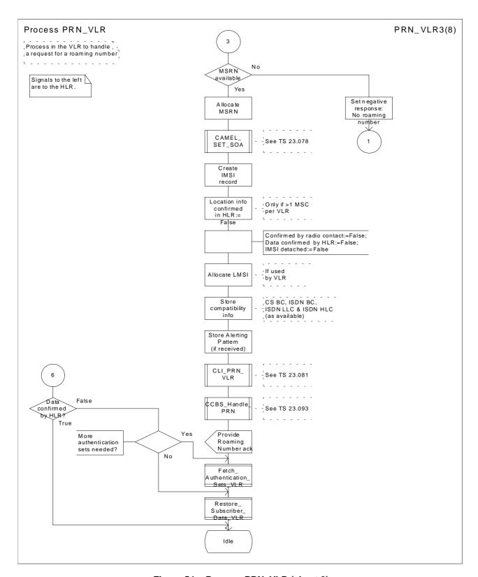
Figure 54c: Process PRN\_VLR (sheet 3)
