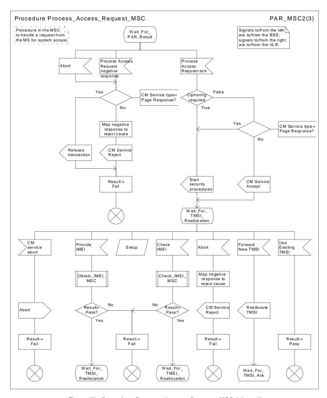
Figure 7b: Procedure Process\_Access\_Request\_MSC (sheet 2)
