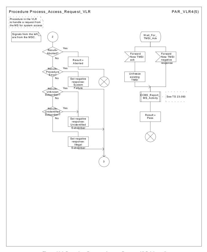
Figure 20d: Procedure Process\_Access\_Request\_VLR (sheet 4)
