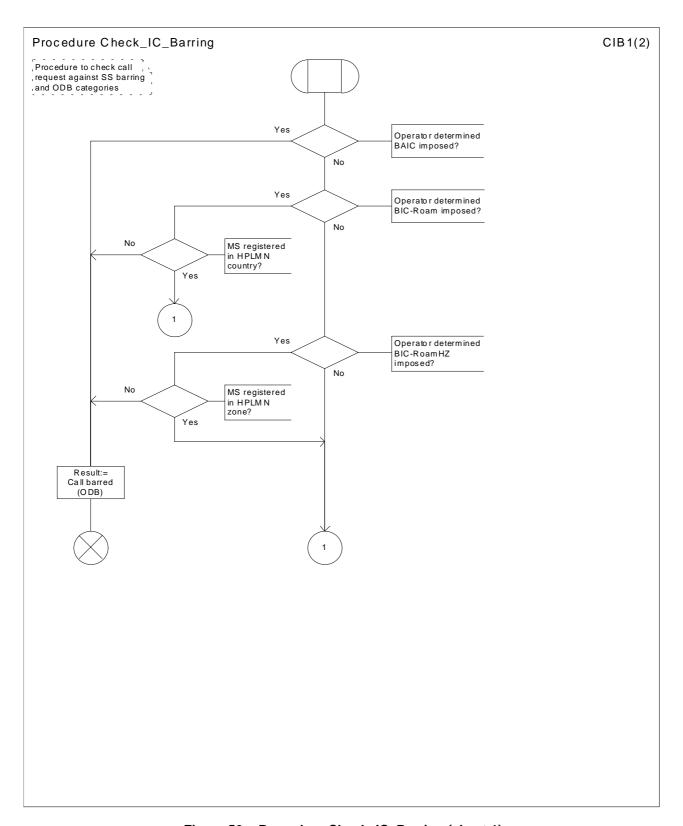
Figure 50a: Procedure Check\_IC\_Barring (sheet 1)
