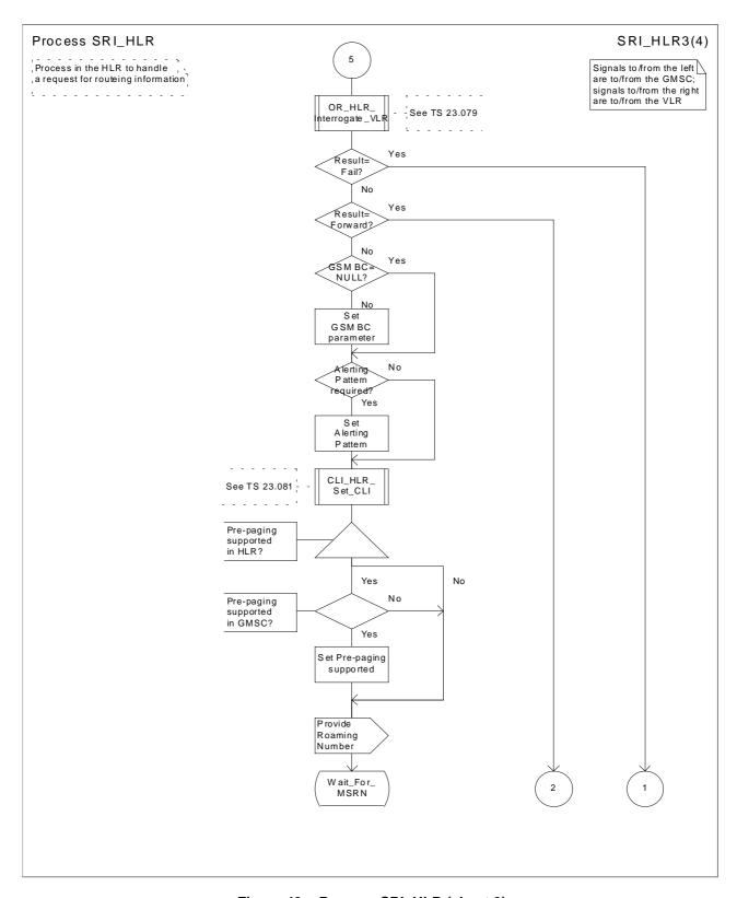
Figure 43c: Process SRI\_HLR (sheet 3)
