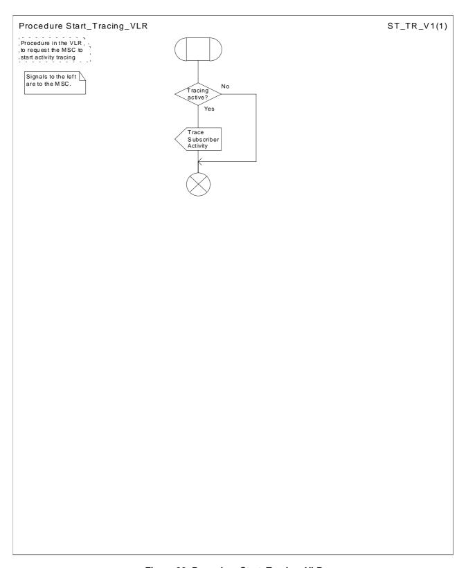
Figure 26: Procedure Start\_Tracing\_VLR
