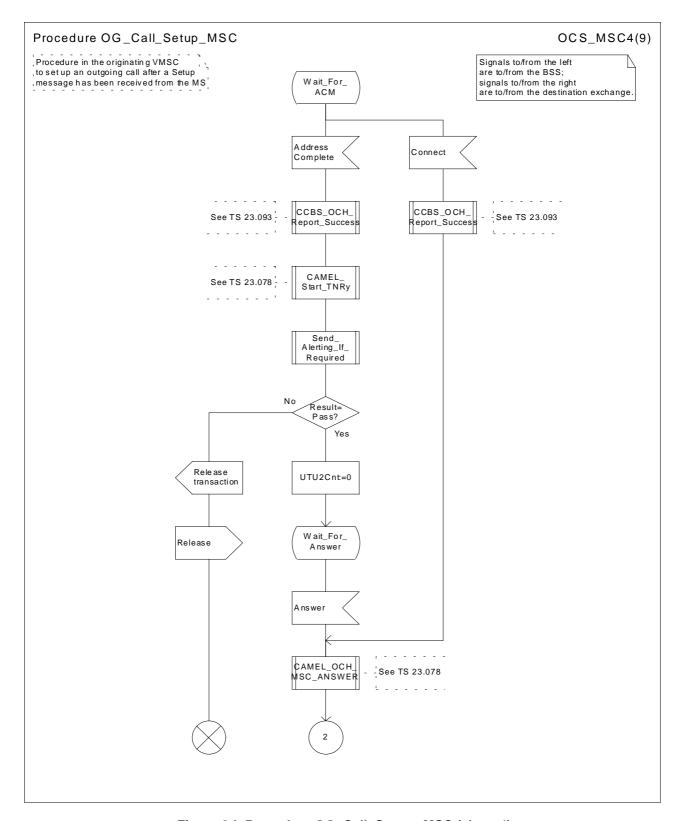
Figure 8d: Procedure OG\_Call\_Setup \_MSC (sheet 4)
