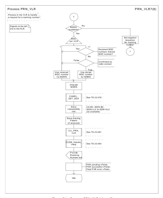
Figure 54g: Process PRN\_VLR (sheet 7)
