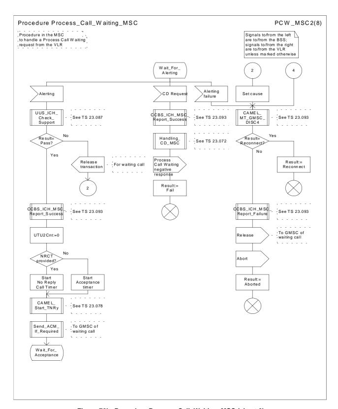
Figure 70b: Procedure Process\_Call\_Waiting\_MSC (sheet 2)
