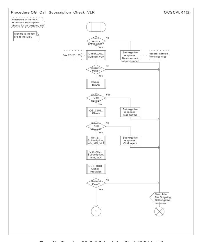
Figure 21a: Procedure OG\_Call\_Subscription\_Check\_VLR (sheet 1)
