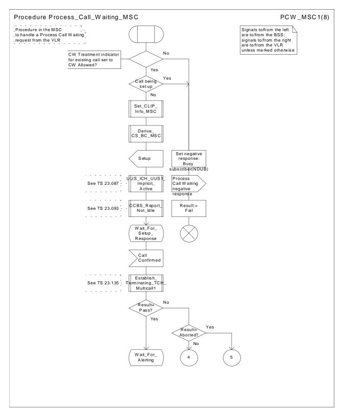
Figure 70a: Procedure Process\_Call\_Waiting\_MSC (sheet 1)
