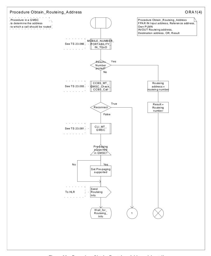
Figure 36a: Procedure Obtain\_Routeing\_Address (sheet 1)
