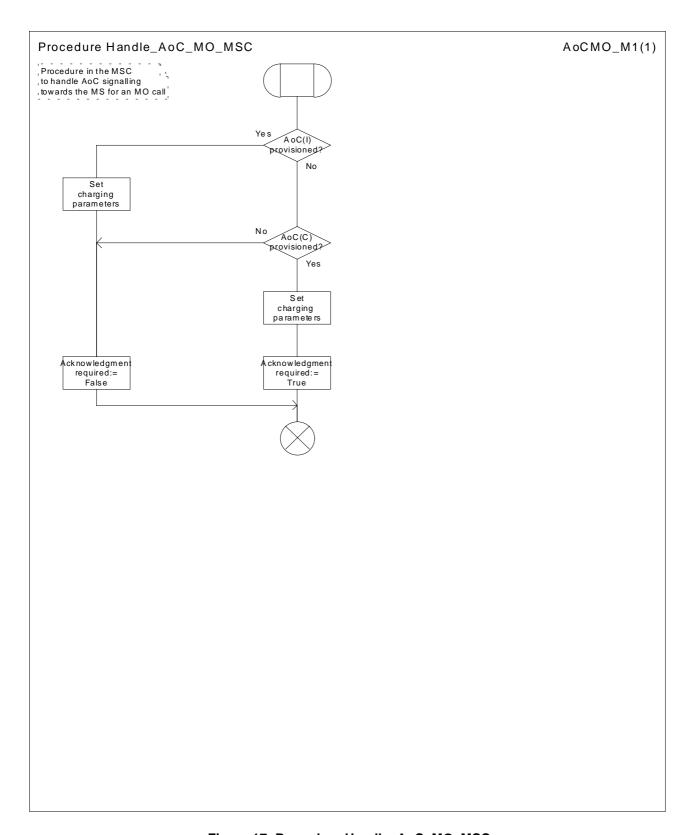
Figure 17: Procedure Handle\_AoC\_MO\_MSC
