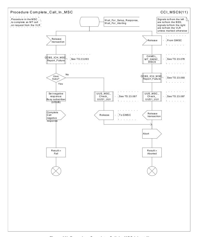
Figure 69i: Procedure Complete\_Call\_In\_MSC (sheet 9)
