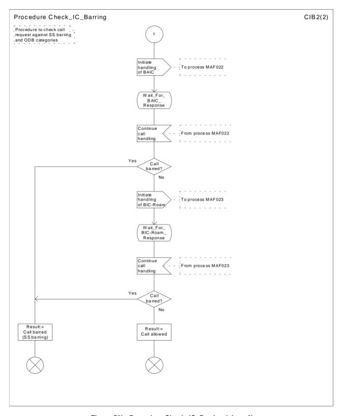
Figure 50b: Procedure Check\_IC\_Barring (sheet 2)
