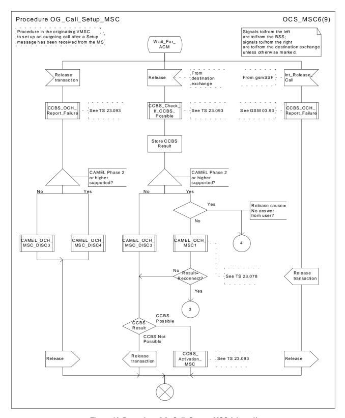
Figure 8f: Procedure OG\_Call\_Setup \_MSC (sheet 6)
