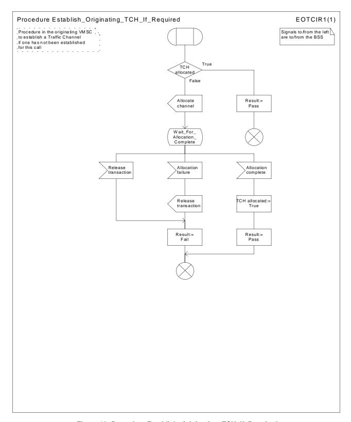
Figure 13: Procedure Establish\_Originating\_TCH\_If\_Required
