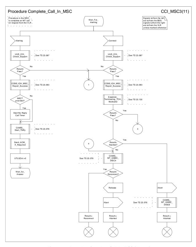
Figure 69c: Procedure Complete\_Call\_In\_MSC (sheet 3)
