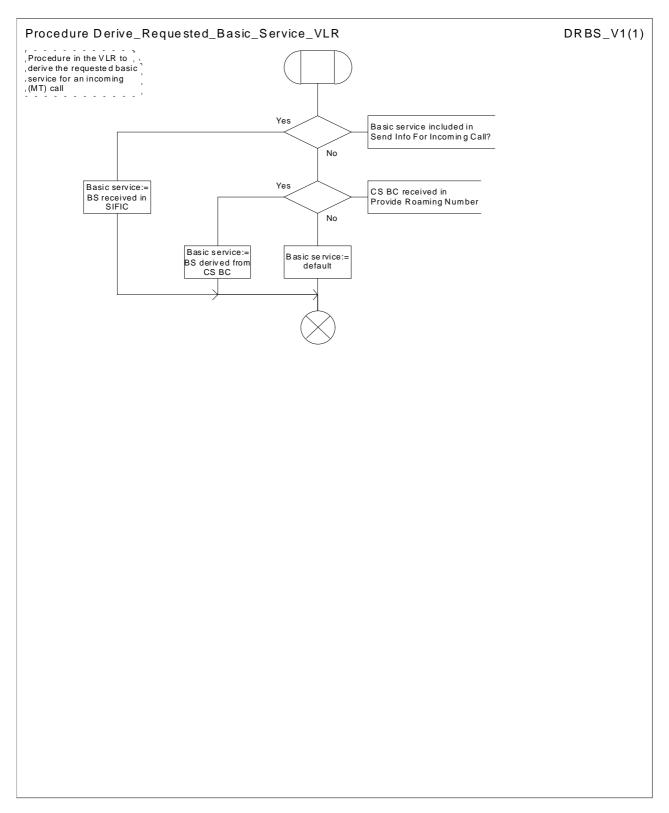
Figure 77: Procedure Derive\_Requested\_Basic\_Service\_VLR
