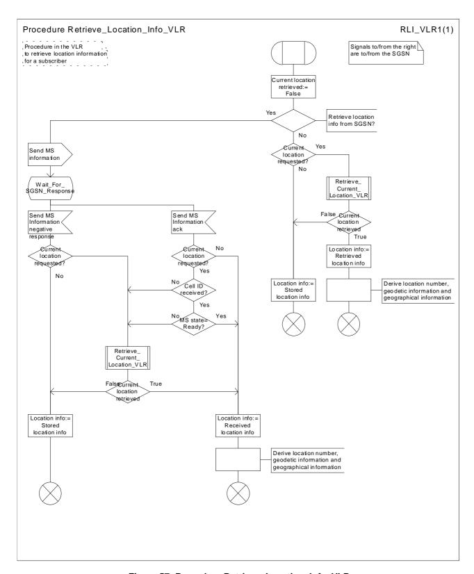
Figure 57: Procedure Retrieve\_Location\_Info\_VLR
