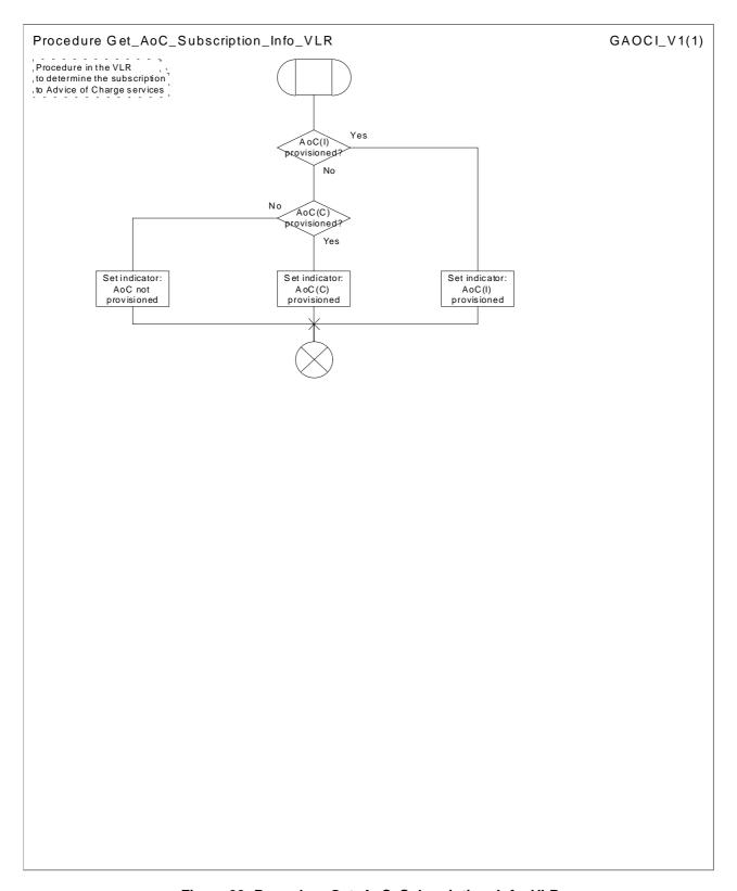
Figure 33: Procedure Get\_AoC\_Subscription\_Info\_VLR
