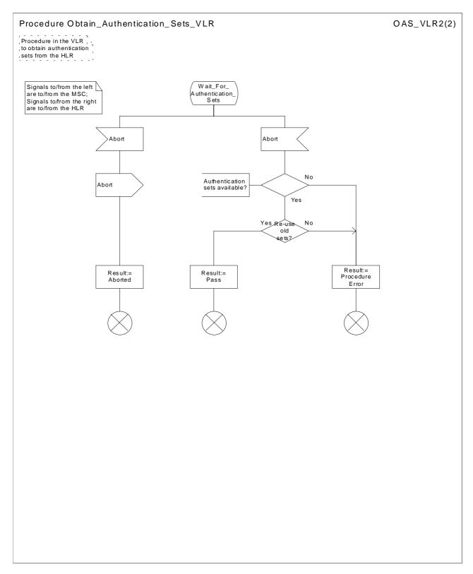
Figure 25b: Procedure Obtain\_Authentication\_Sets\_VLR (sheet 2)
