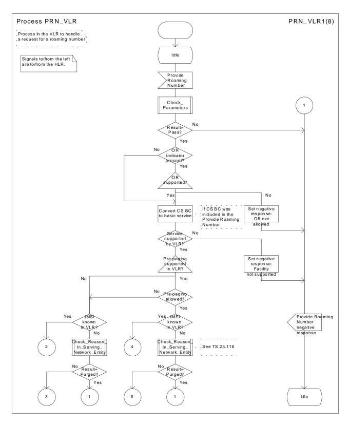
Figure 54a: Process PRN\_VLR (sheet 1)
