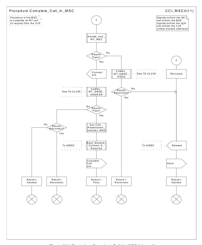
Figure 69d: Procedure Complete\_Call\_In\_MSC (sheet 4)
