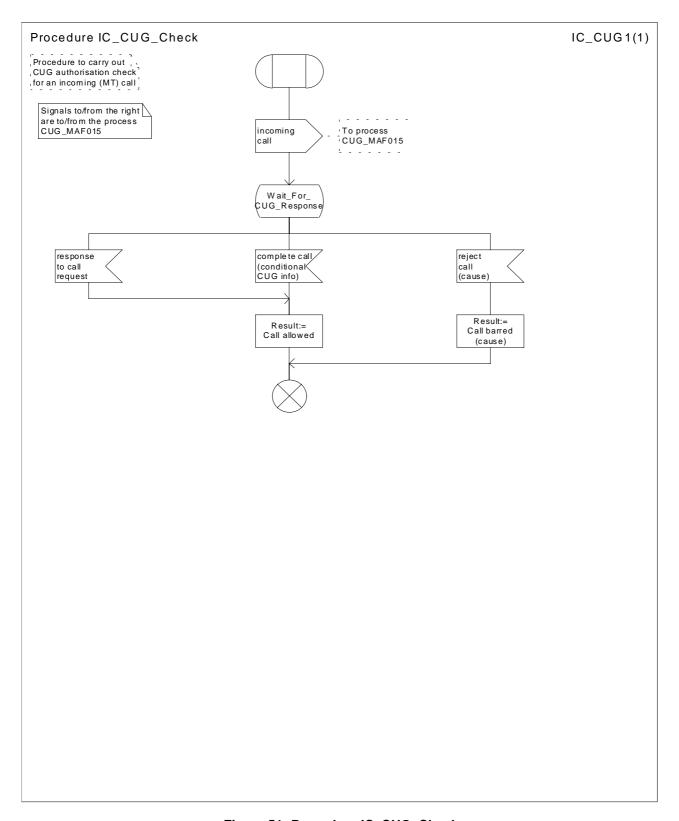
Figure 51: Procedure IC\_CUG\_Check
