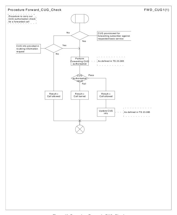
Figure 48: Procedure Forward \_CUG\_Check
