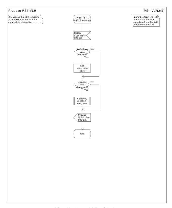
Figure 56b: Process PSI\_VLR (sheet 2)
