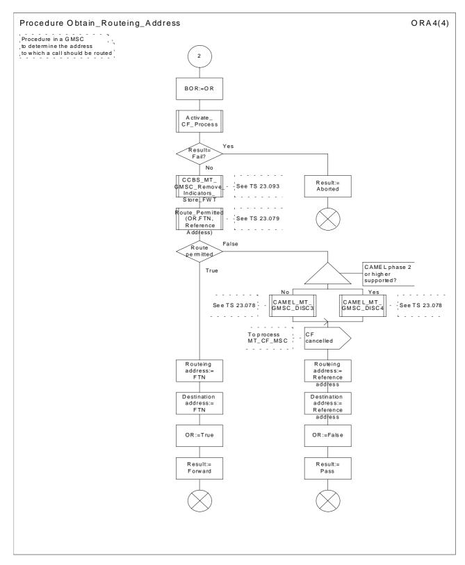
Figure 36d: Procedure Obtain\_Routeing\_Address (sheet 4)
