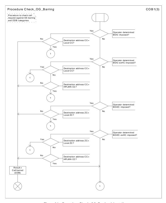
Figure 34a: Procedure Check\_OG\_Barring (sheet 1)
