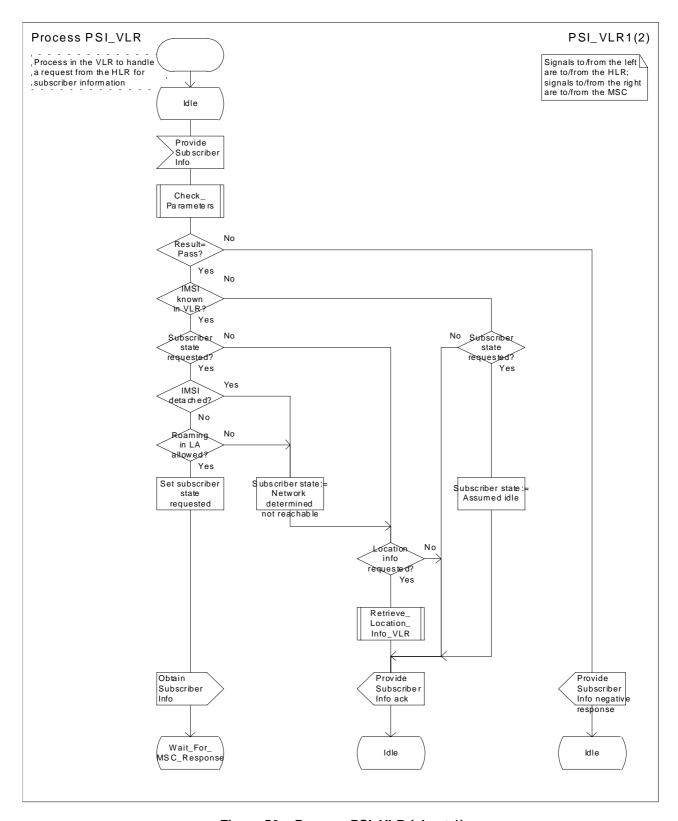
Figure 56a: Process PSI\_VLR (sheet 1)
