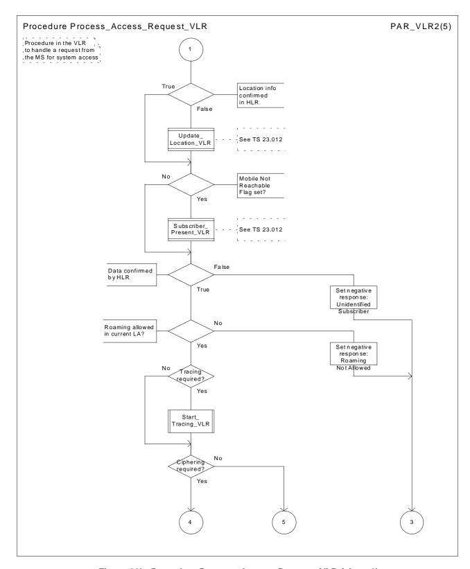
Figure 20b: Procedure Process\_Access\_Request\_VLR (sheet 2)
