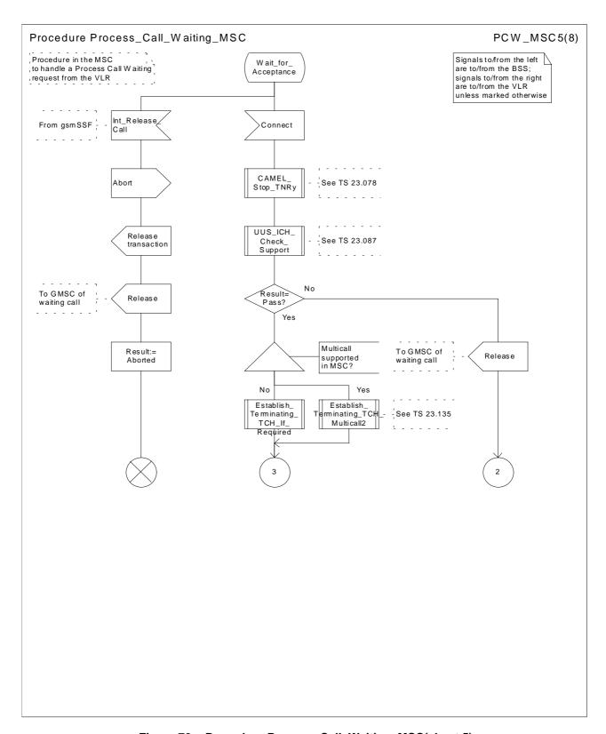
Figure 70e: Procedure Process\_Call\_Waiting\_MSC(sheet 5)
