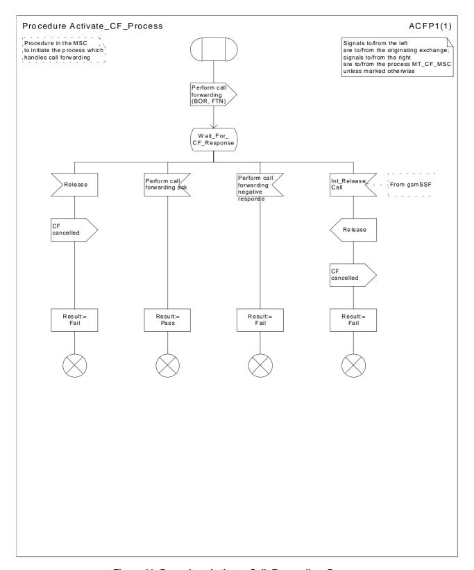
Figure 41: Procedure Activate\_Call\_Forwarding\_Process
