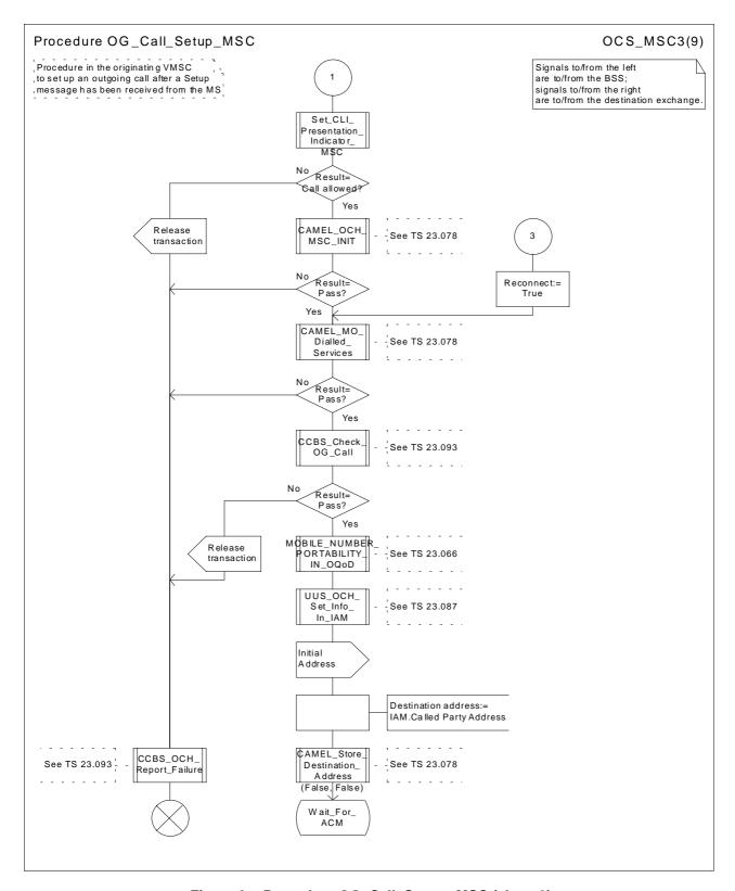
Figure 8c: Procedure OG\_Call\_Setup \_MSC (sheet 3)
