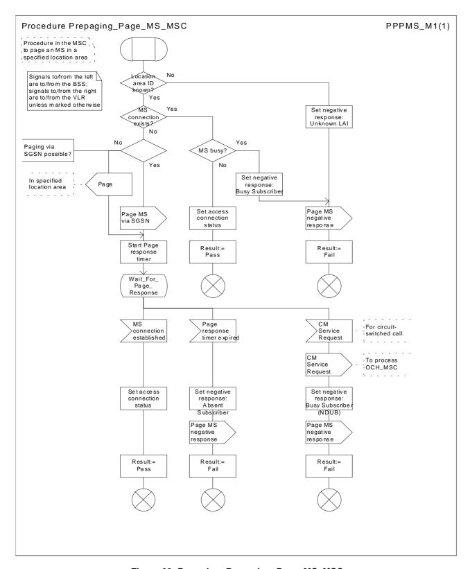
Figure 60: Procedure Prepaging\_Page\_MS\_MSC
