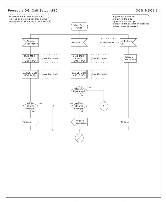
Figure 8i: Procedure OG\_Call\_Setup \_MSC (sheet 9)
