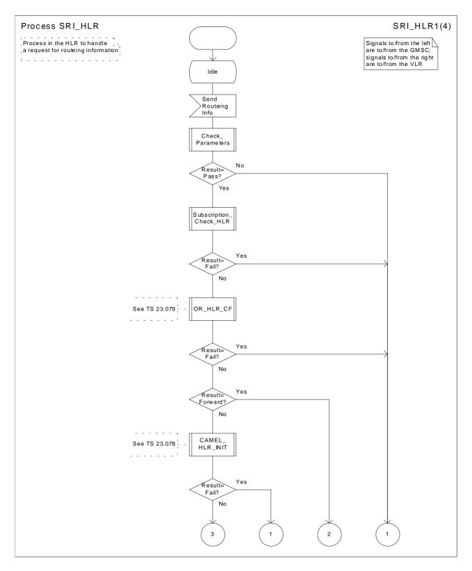
Figure 43a: Process SRI\_HLR (sheet 1)
