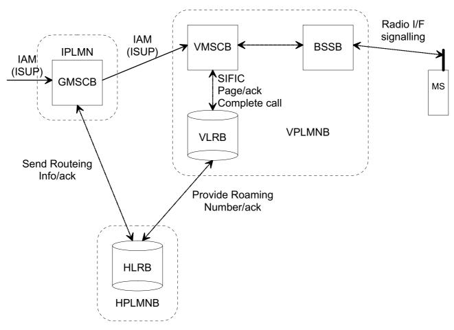
Figure 2: Architecture for a basic mobile terminated call
