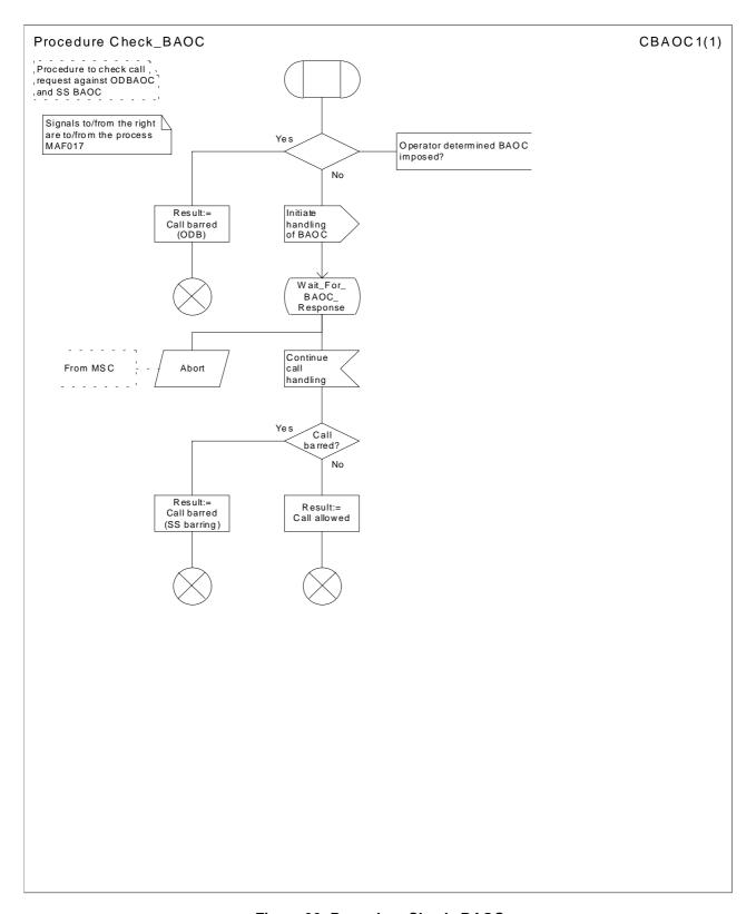
Figure 30: Procedure Check\_BAOC
