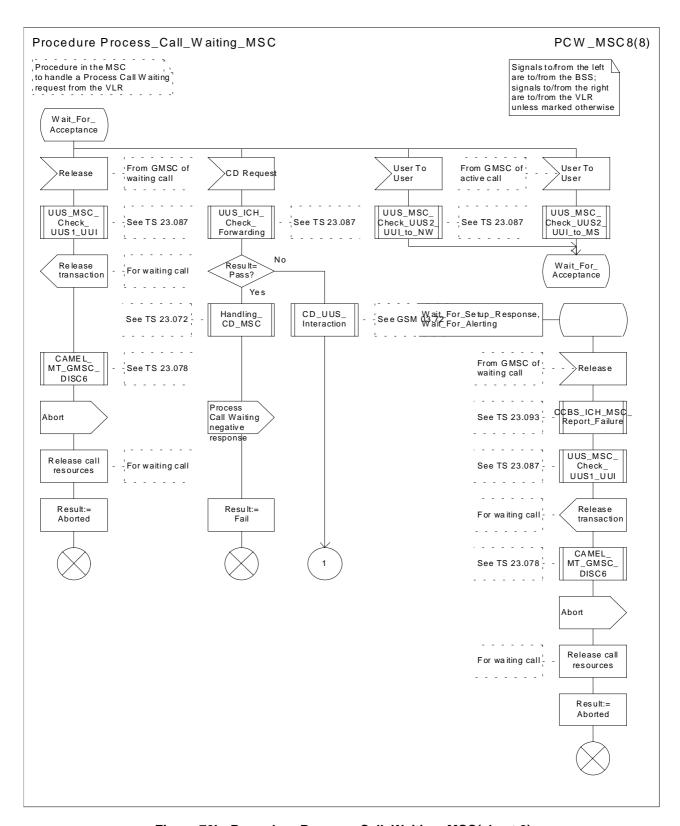
Figure 70h: Procedure Process\_Call\_Waiting\_MSC(sheet 8)
