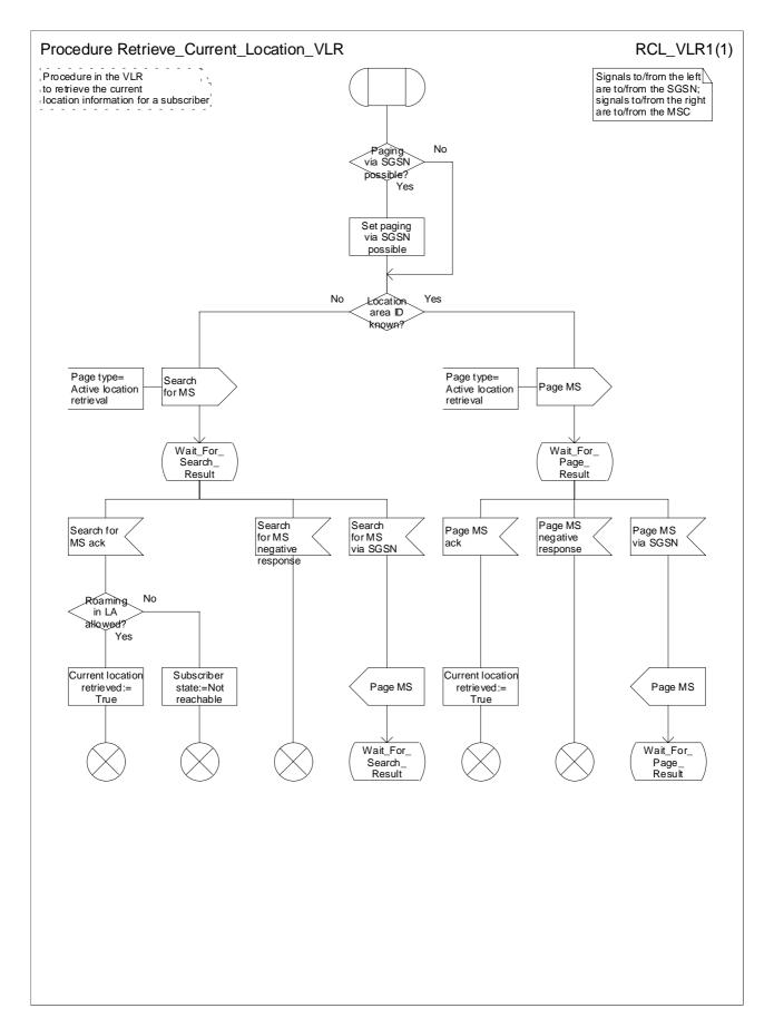
Figure 58: Procedure Retrieve\_Current\_Location\_VLR
