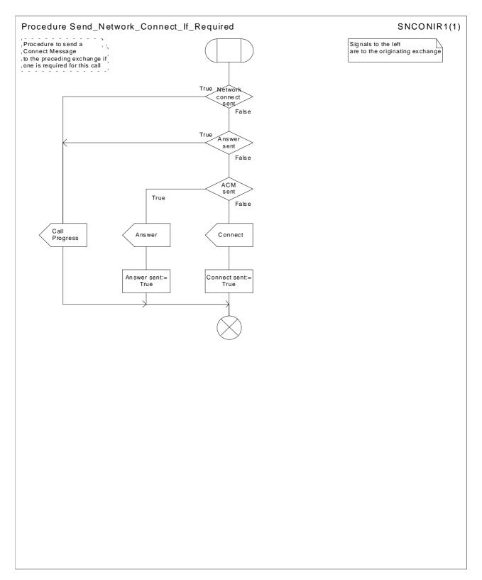
Figure 39: Procedure Send\_Network\_Connect\_If\_Required
