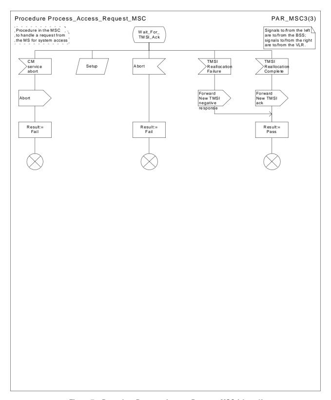
Figure 7c: Procedure Process\_Access\_Request\_MSC (sheet 3)
