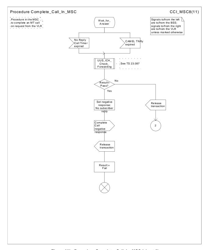
Figure 69h: Procedure Complete\_Call\_In\_MSC (sheet 8)
