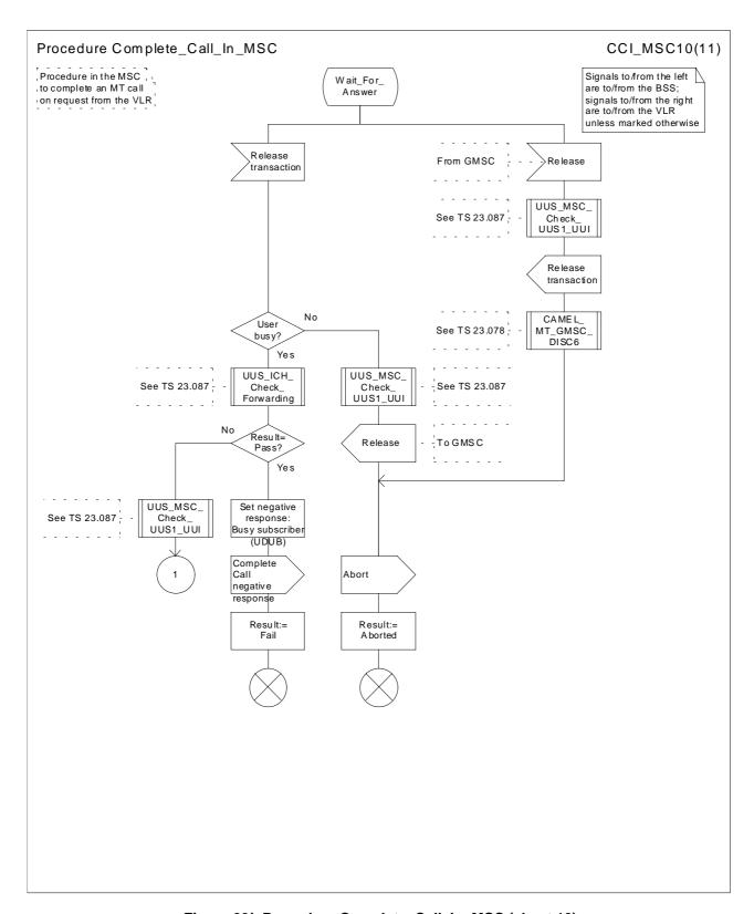
Figure 69j: Procedure Complete\_Call\_In\_MSC (sheet 10)
