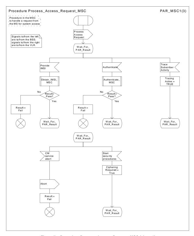
Figure 7a: Procedure Process\_Access\_Request\_MSC (sheet 1)
