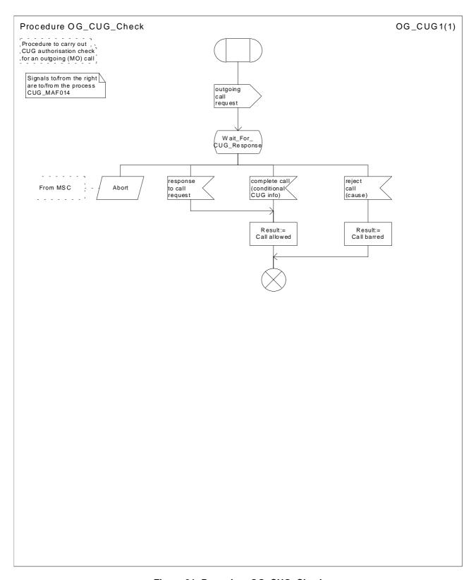
Figure 31: Procedure OG\_CUG\_Check
