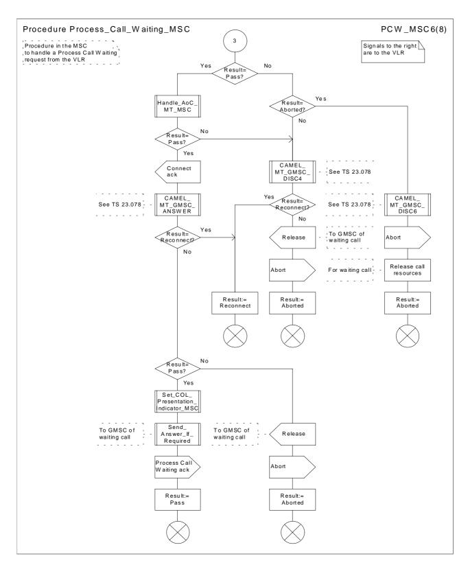
Figure 70f: Procedure Process\_Call\_Waiting\_MSC(sheet 6)
