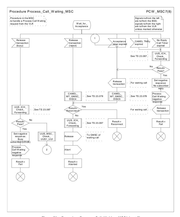
Figure 70g: Procedure Process\_Call\_Waiting\_MSC(sheet 7)
