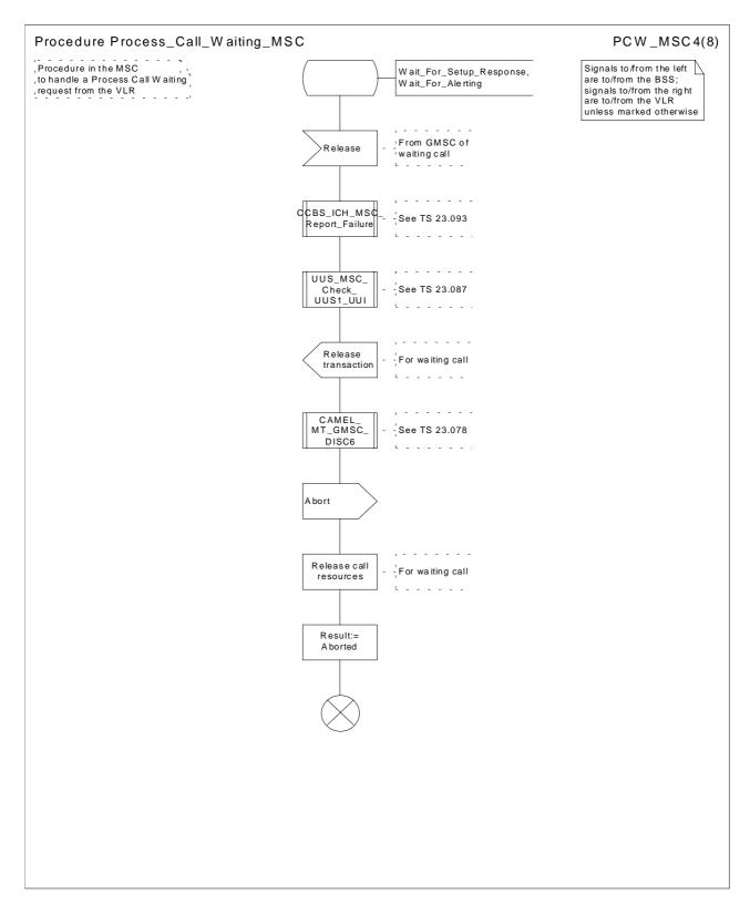
Figure 70d: Procedure Process\_Call\_Waiting\_MSC(sheet 4)
