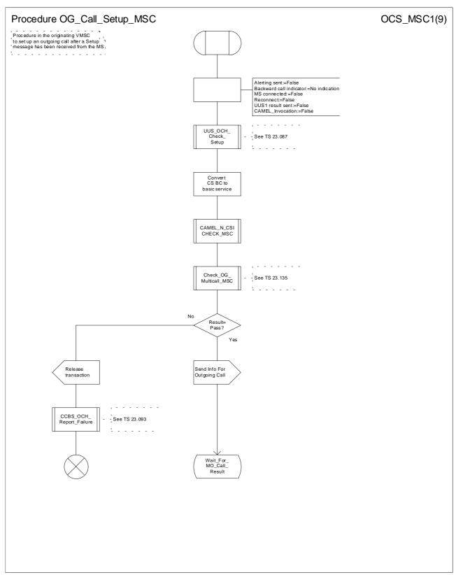
Figure 8a: Procedure OG\_Call\_Setup\_MSC (sheet 1)
