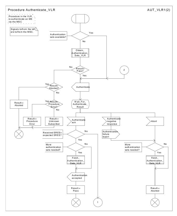
Figure 24a: Procedure Authenticate\_VLR (sheet 1)
