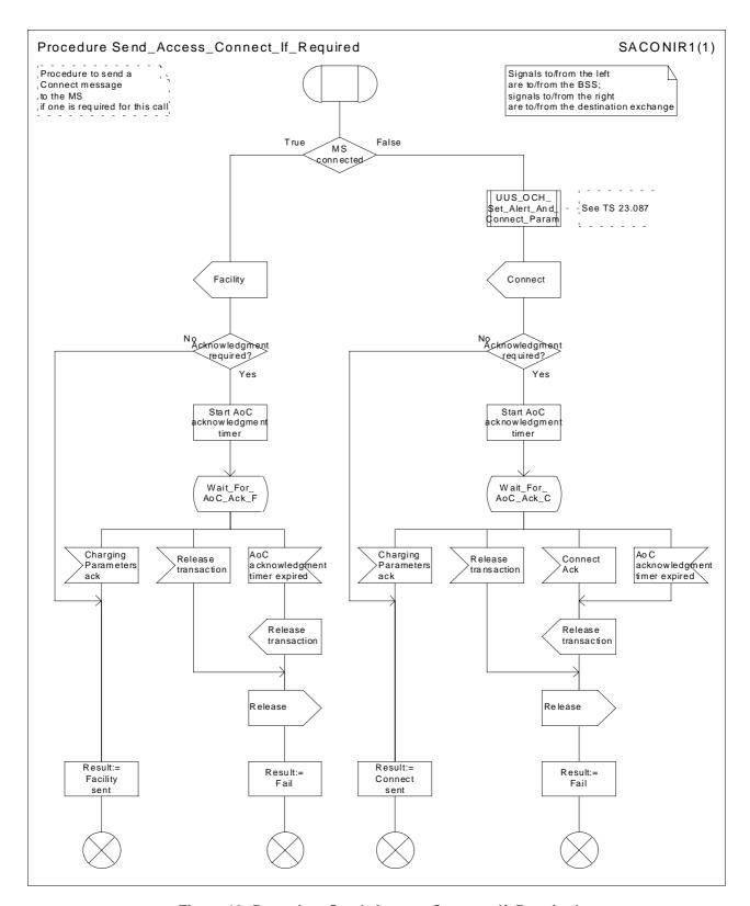
Figure 18: Procedure Send\_Access\_Connect\_If\_Required
