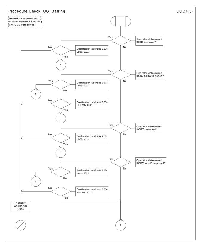
Figure 7.1.2.16a: Procedure Check\_OG\_Barring (sheet 1)
