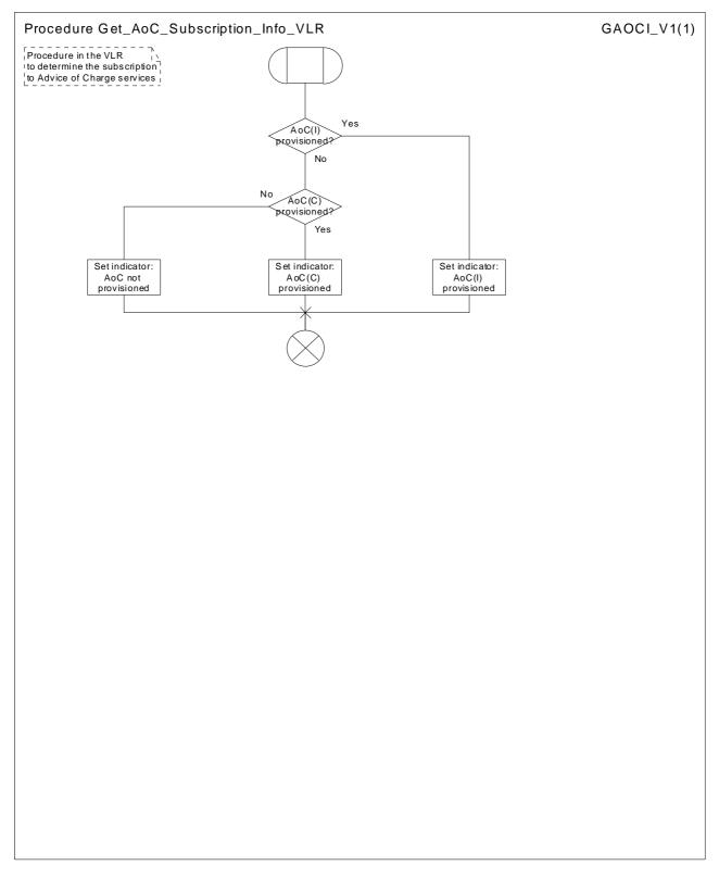
Figure 7.1.2.15: Procedure Get\_AoC\_Subscription\_Info\_VLR
