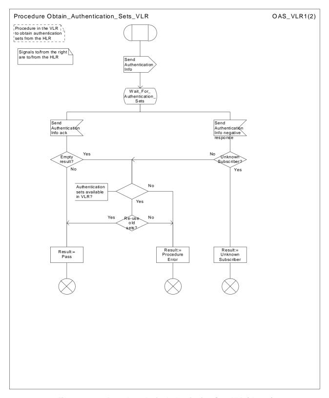
Figure 7.1.2.7a: Procedure Obtain\_Authentication\_Sets\_VLR (sheet 1)
