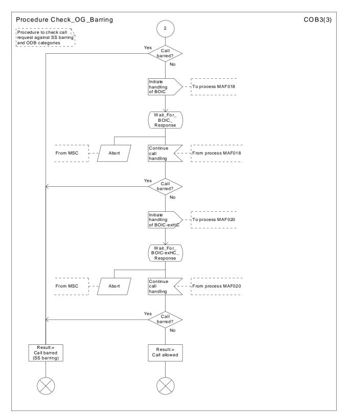
Figure 7.1.2.16c: Procedure Check\_OG\_Barring (sheet 3)
