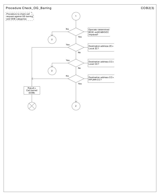
Figure 7.1.2.16b: Procedure Check\_OG\_Barring (sheet 2)
