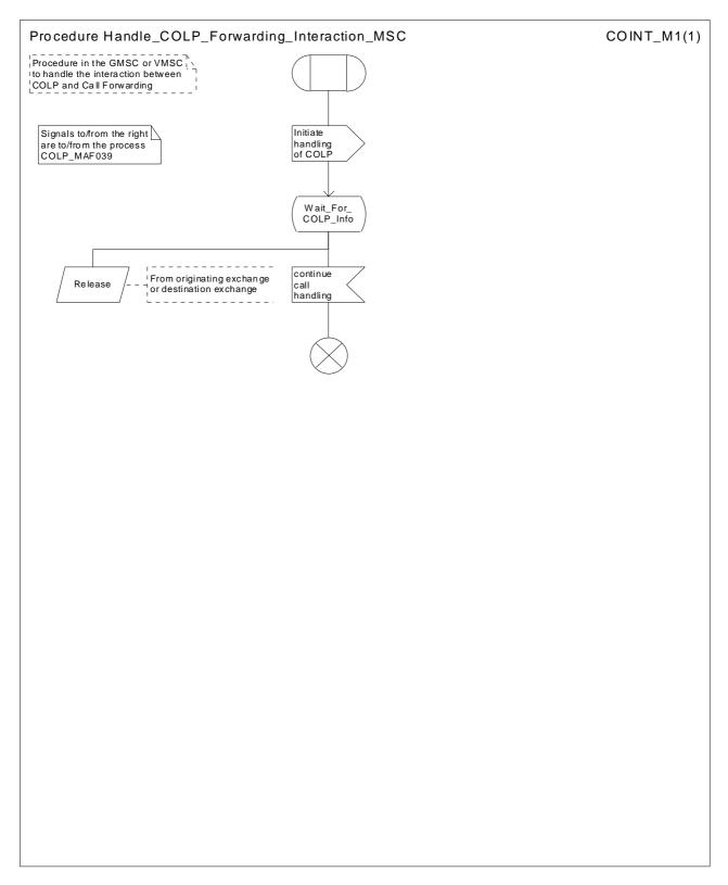
Figure 41: Procedure Handle\_COLP\_Forwarding\_Interaction\_MSC
