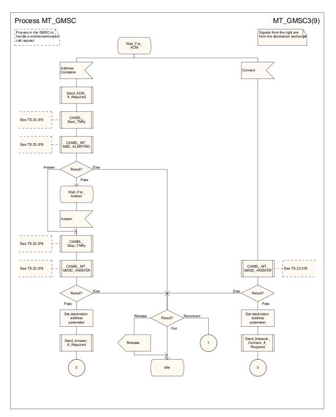
Figure 36c: Process MT\_GMSC (sheet 3)
