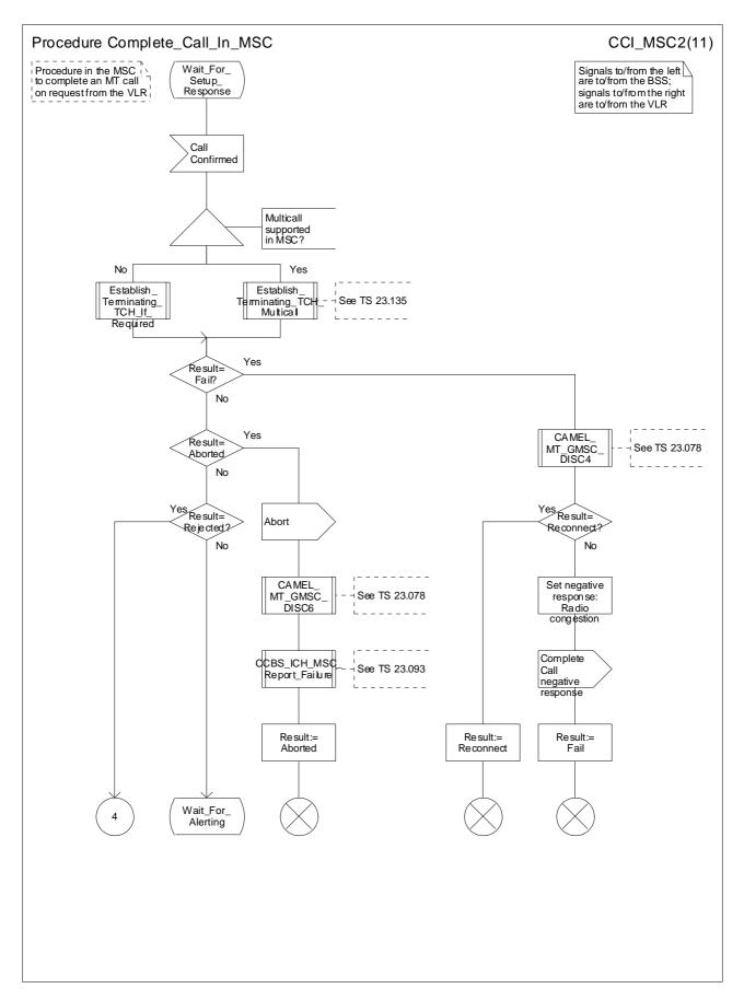
Figure 70b: Procedure Complete\_Call\_In\_MSC (sheet 2)
