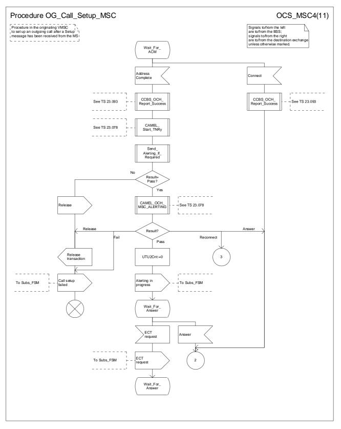
Figure 8d: Procedure OG\_Call\_Setup \_MSC (sheet 4)
