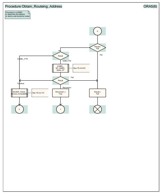
Figure 37e: Procedure Obtain\_Routeing\_Address (sheet 5)
