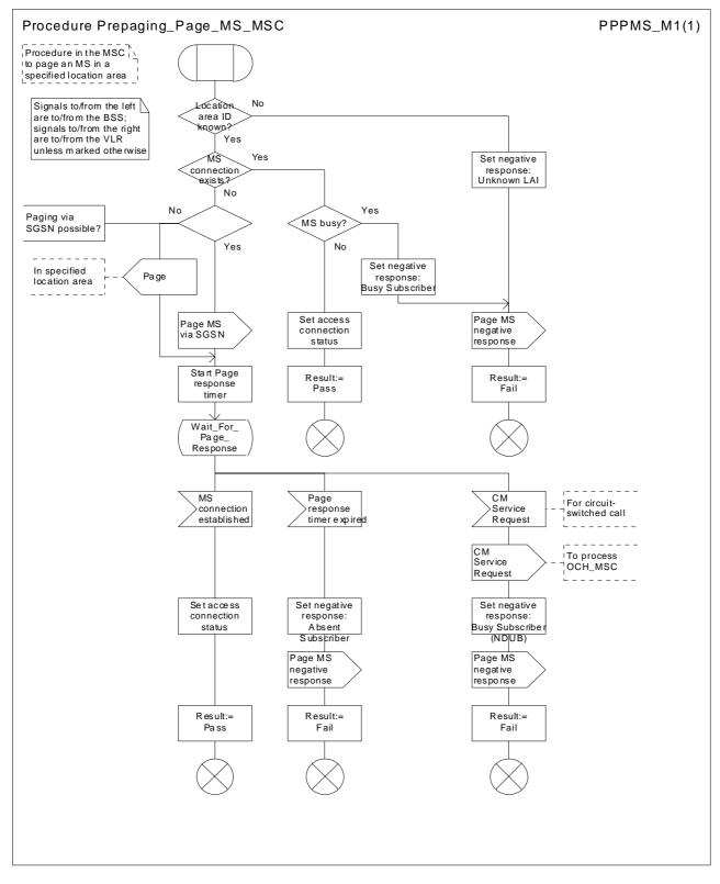
Figure 61: Procedure Prepaging\_Page\_MS\_MSC
