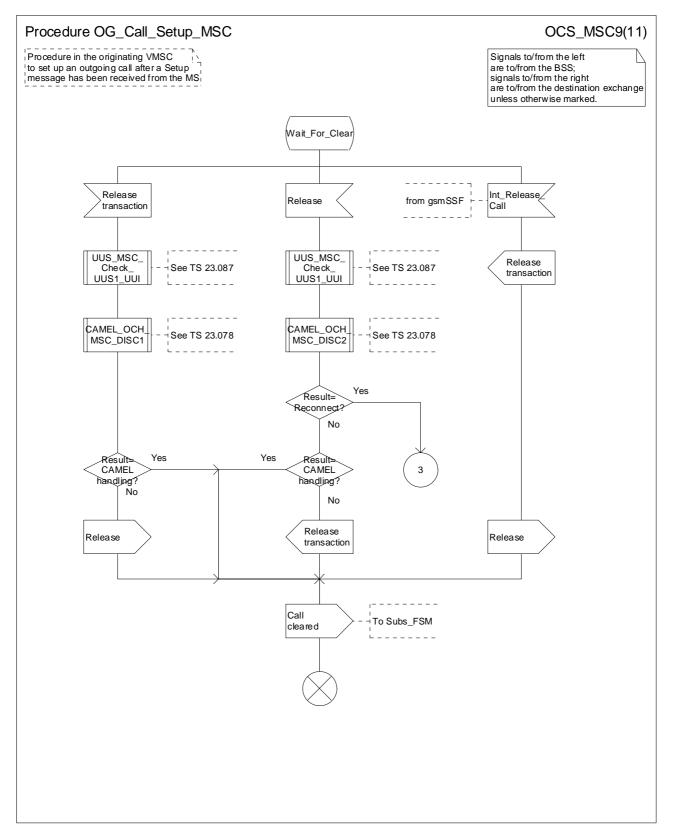
Figure 8i: Procedure OG\_Call\_Setup \_MSC (sheet 9)
