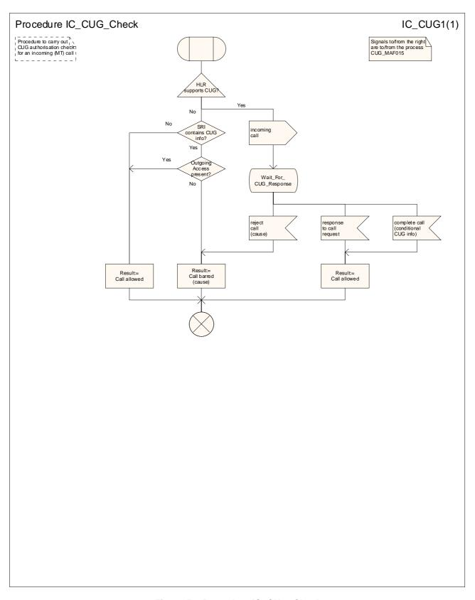
Figure 52: Procedure IC\_CUG\_Check
