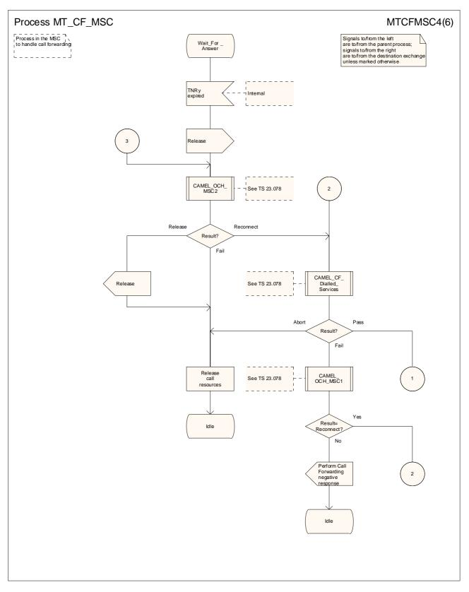
Figure 43d: Process MT\_CF\_MSC (sheet 4)
