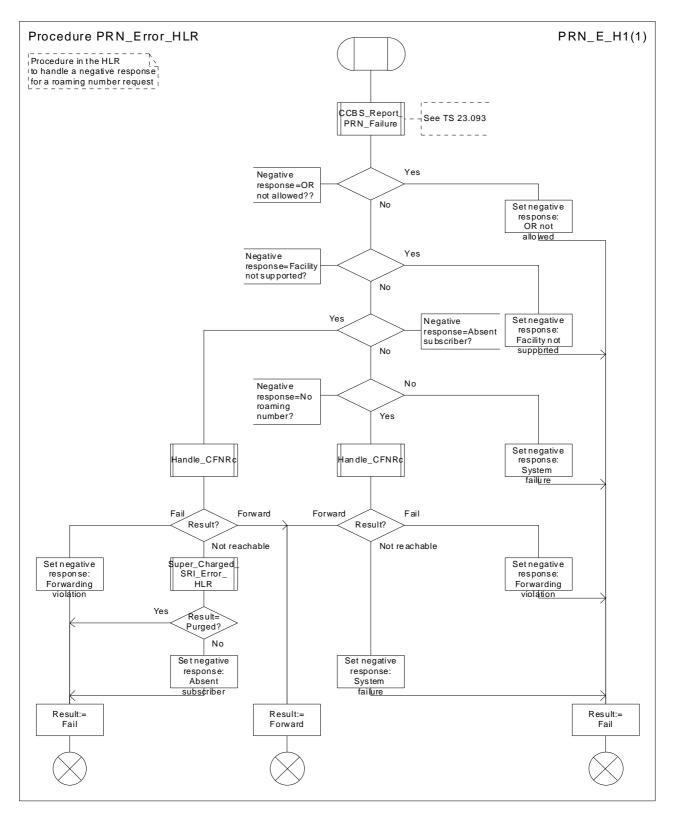
Figure 48: Procedure PRN\_Error\_HLR
