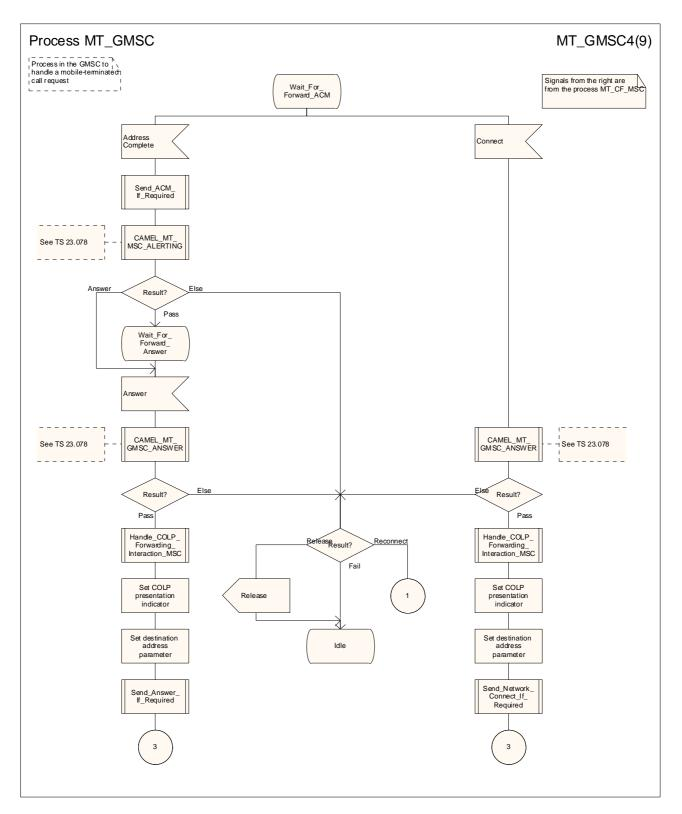
Figure 36d: Process MT\_GMSC (sheet 4)
