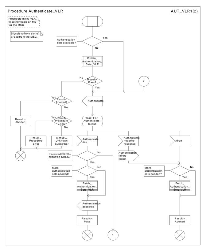
Figure 7.1.2.6a: Procedure Authenticate\_VLR (sheet 1)
