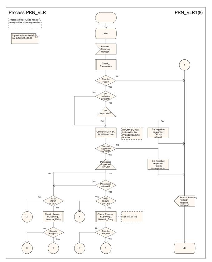
Figure 55a: Process PRN\_VLR (sheet 1)
