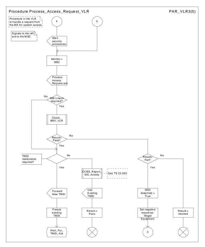
Figure 7.1.2.2c: Procedure Process\_Access\_Request\_VLR (sheet 3)
