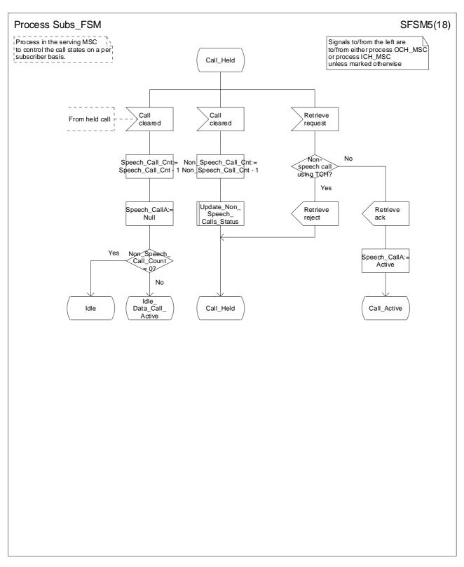
Figure 83e: Process Subs\_FSM (sheet 5)
