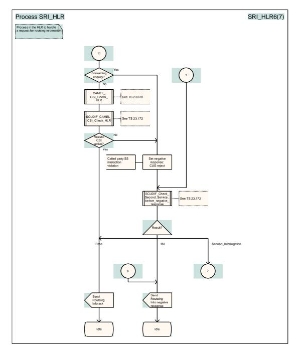
Figure 44f: Process SRI\_HLR (sheet 6)
