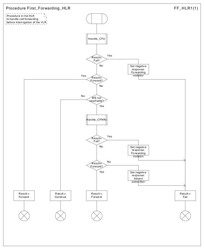
Figure 47: Procedure First\_Forwarding\_HLR
