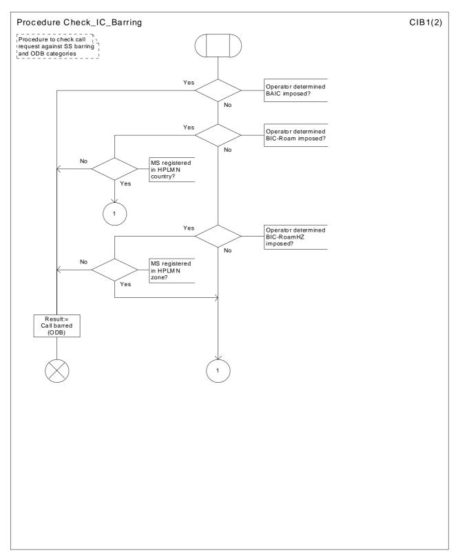
Figure 51a: Procedure Check\_IC\_Barring (sheet 1)
