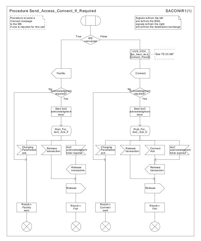
Figure 18: Procedure Send\_Access\_Connect\_If\_Required
