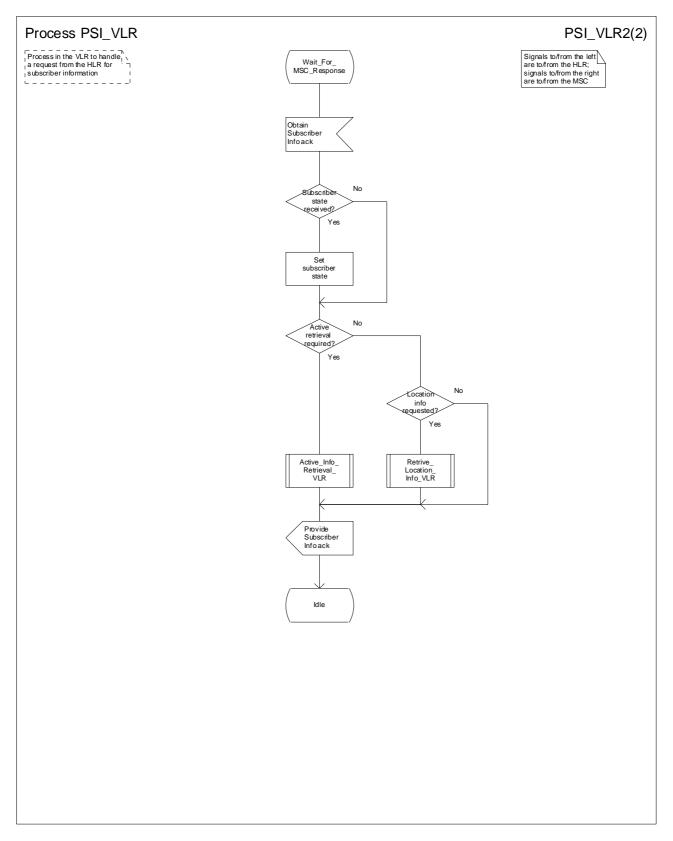
Figure 57b: Process PSI\_VLR (sheet 2)
