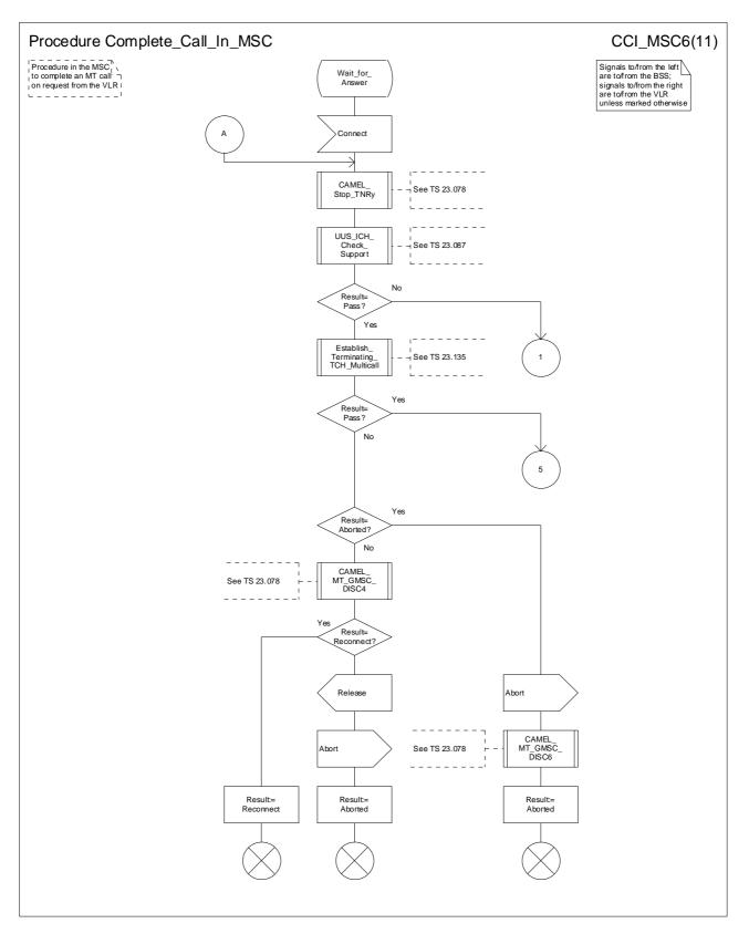
Figure 70f: Procedure Complete\_Call\_In\_MSC (sheet 6)
