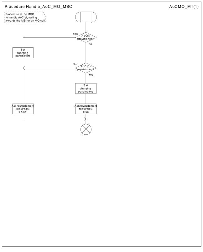
Figure 17: Procedure Handle\_AoC\_MO\_MSC
