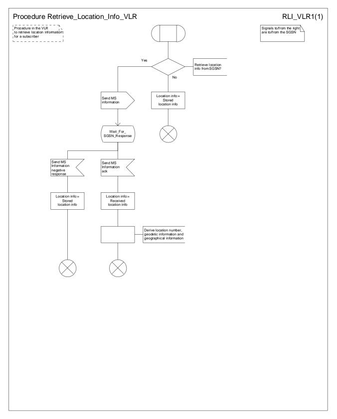
Figure 58: Procedure Retrieve\_Location\_Info\_VLR
