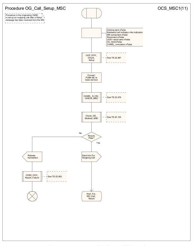
Figure 8a: Procedure OG\_Call\_Setup\_MSC (sheet 1)
