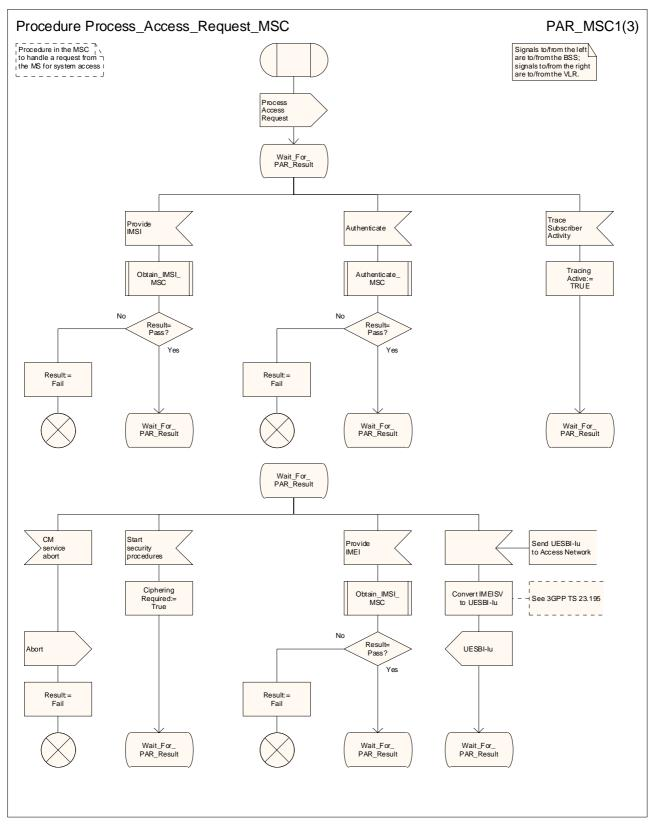
Figure 7a: Procedure Process\_Access\_Request\_MSC (sheet 1)
