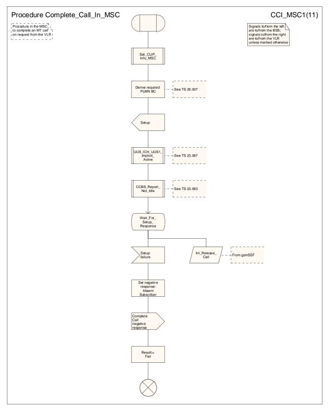
Figure 70a: Procedure Complete\_Call\_In\_MSC (sheet 1)
