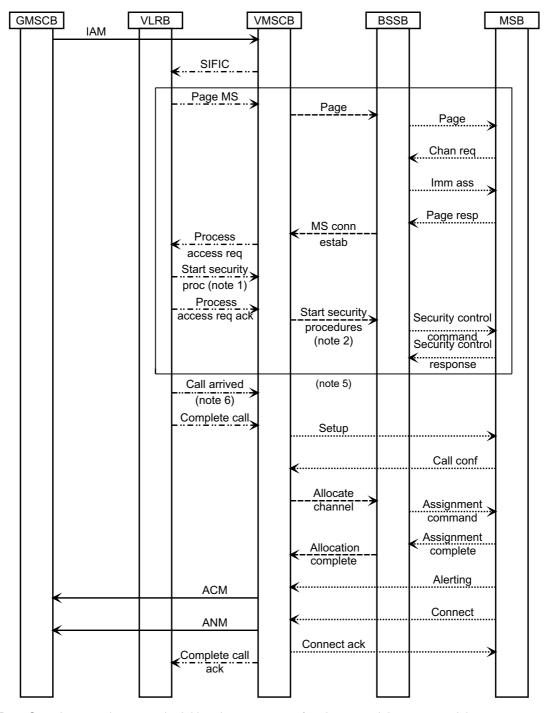
NOTE 1: Security procedures may be initiated at any stage after the network has accepted the page response; the position in this message flow diagram is an example.
