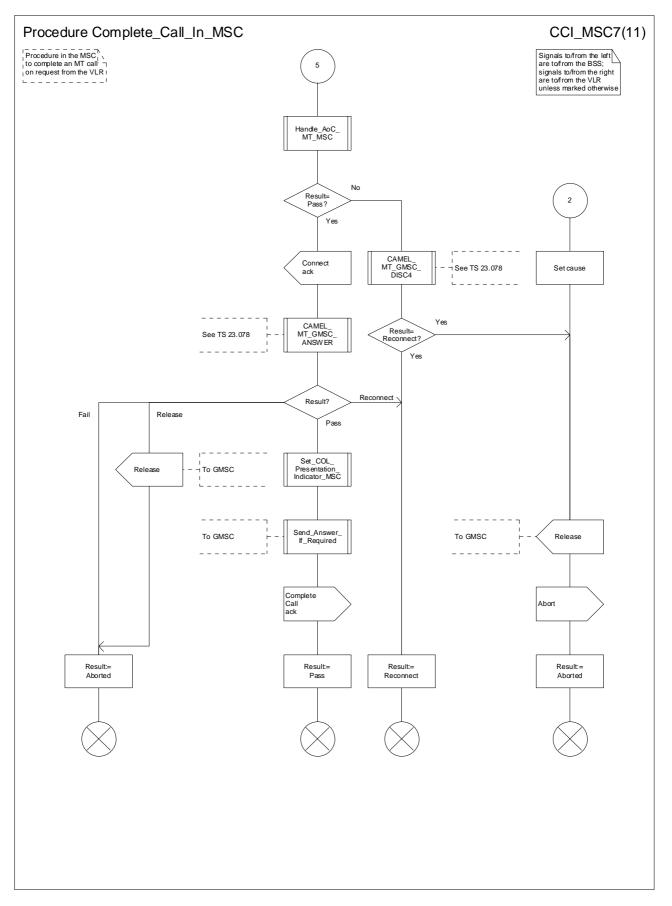
Figure 70g: Procedure Complete\_Call\_In\_MSC (sheet 7)
