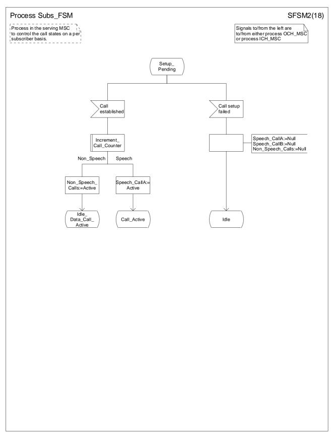
Figure 83b: Process Subs\_FSM (sheet 2)
