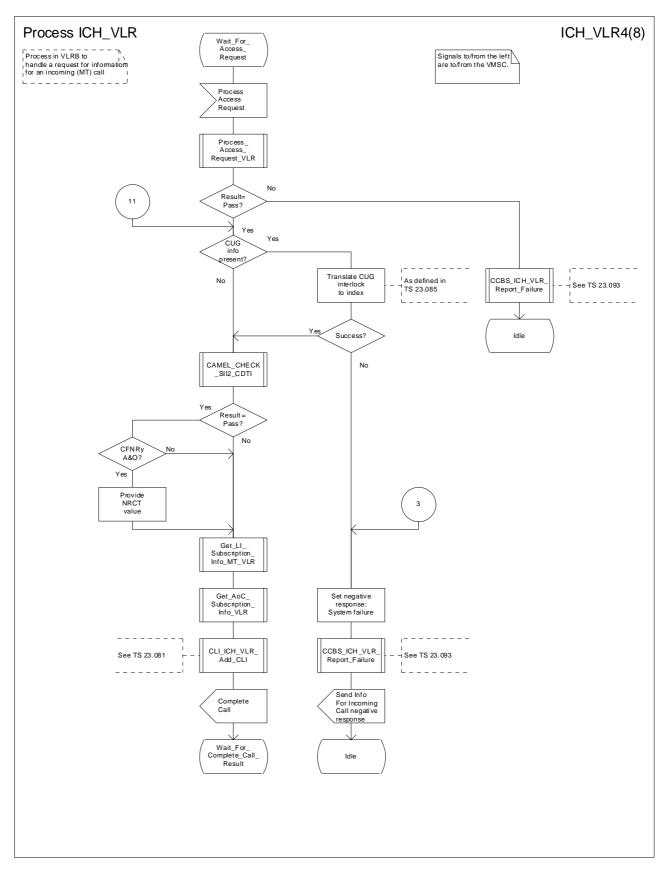
Figure 76d: Process ICH\_VLR (sheet 4)
