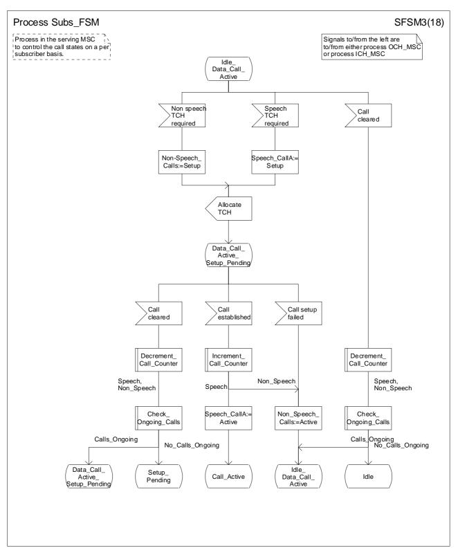
Figure 83c: Process Subs\_FSM (sheet 3)
