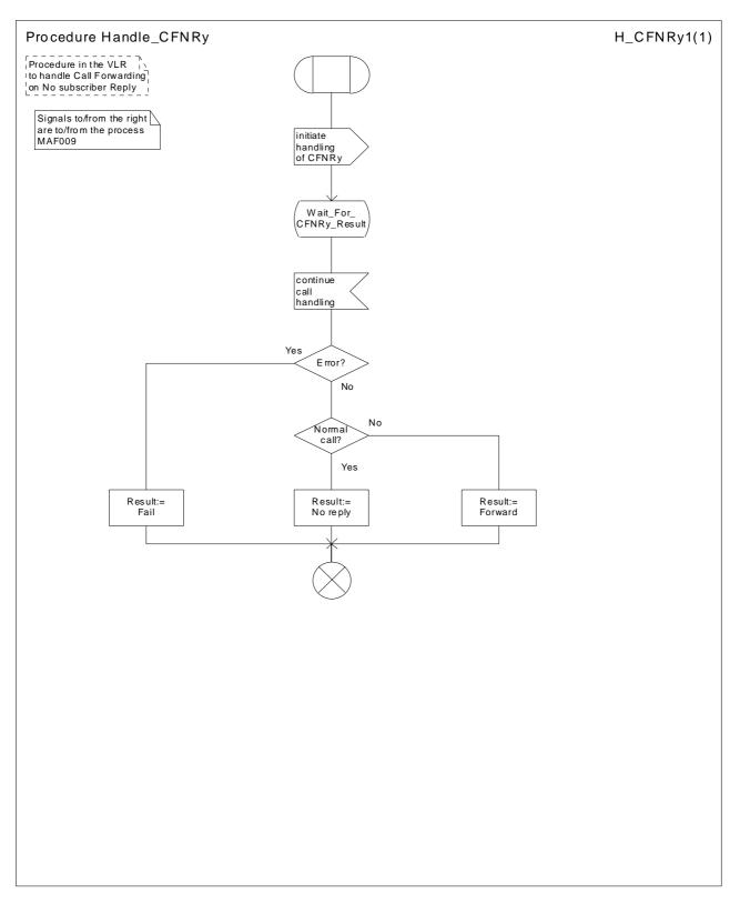
Figure 82: Procedure Handle\_CFNRy
