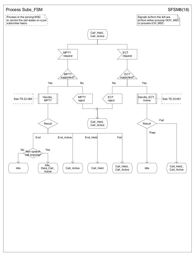
Figure 83h: Process Subs\_FSM (sheet 8)
