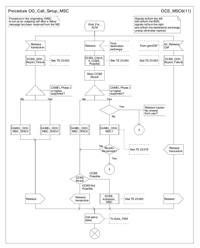
Figure 8f: Procedure OG\_Call\_Setup \_MSC (sheet 6)
