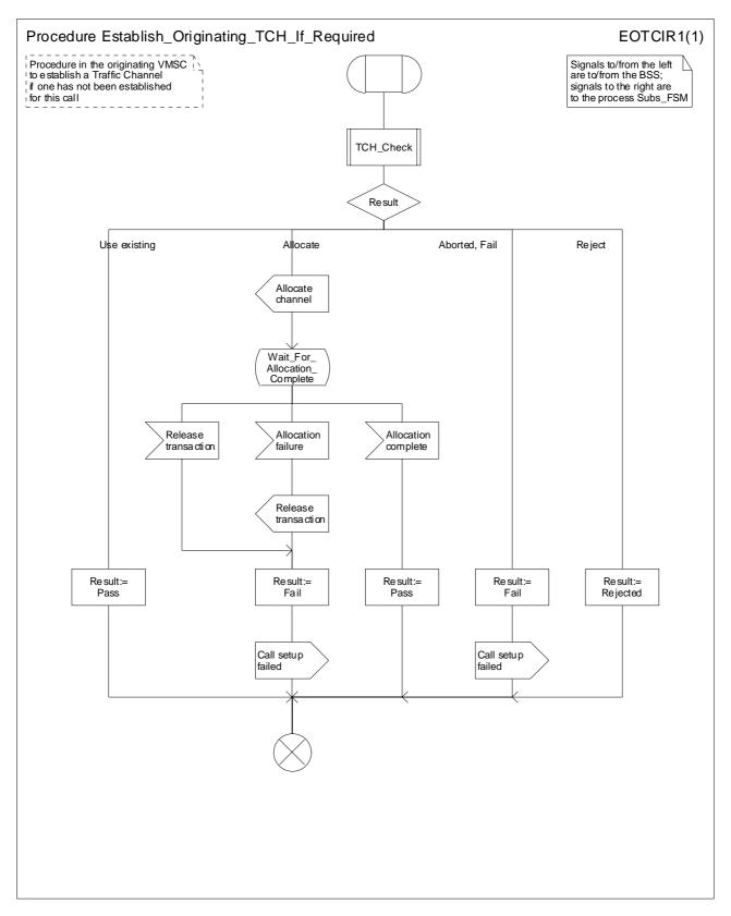
Figure 13: Procedure Establish\_Originating\_TCH\_If\_Required
