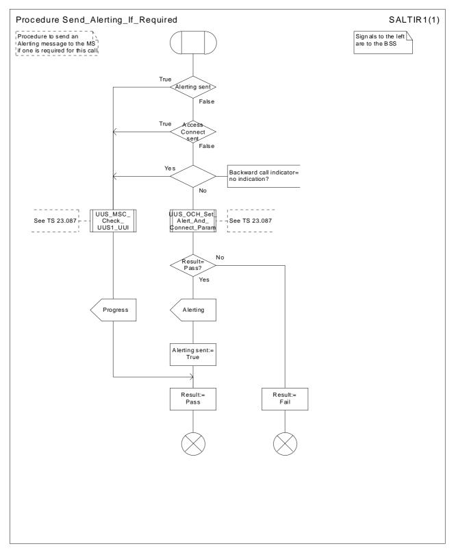
Figure 15: Procedure Send\_Alerting\_If\_Required
