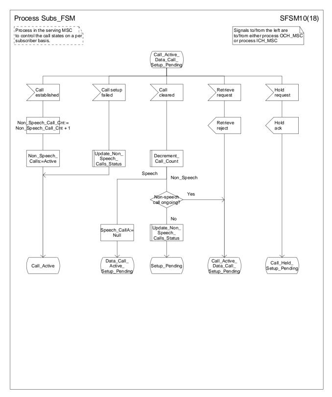
Figure 83j: Process Subs\_FSM (sheet 10)
