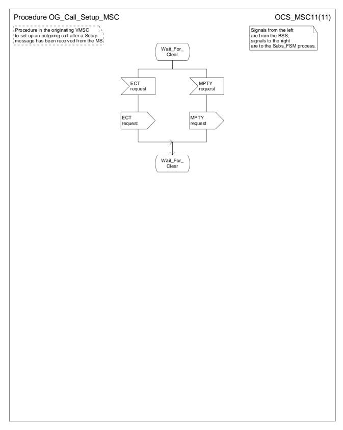
Figure 8k: Procedure OG\_Call\_Setup \_MSC (sheet 11)
