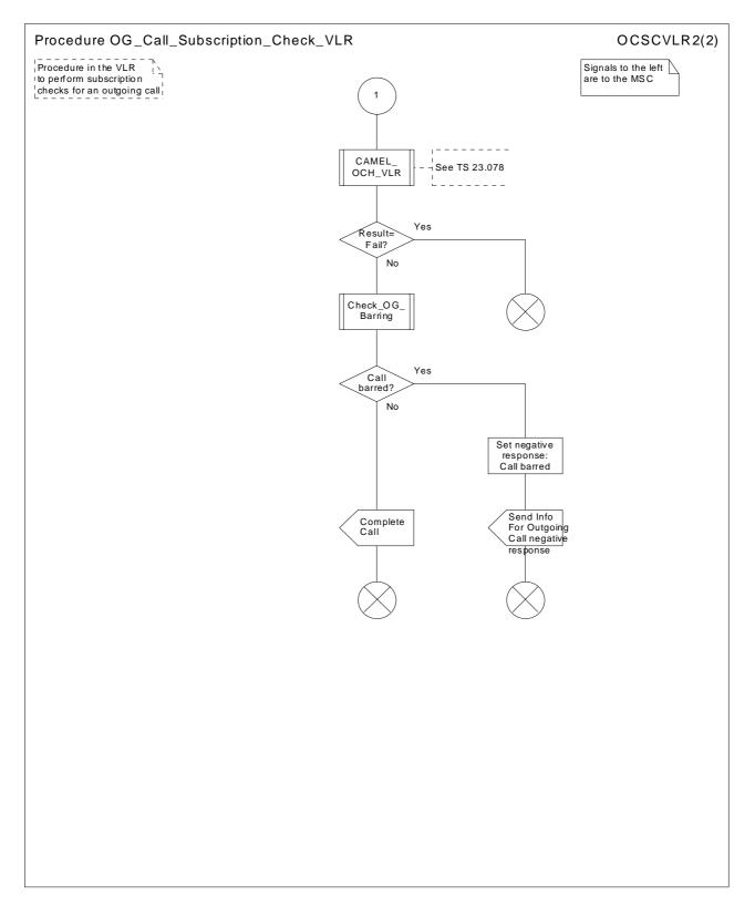
Figure 7.1.2.3b: Procedure OG\_Call\_Subscription\_Check \_VLR (sheet 2)
