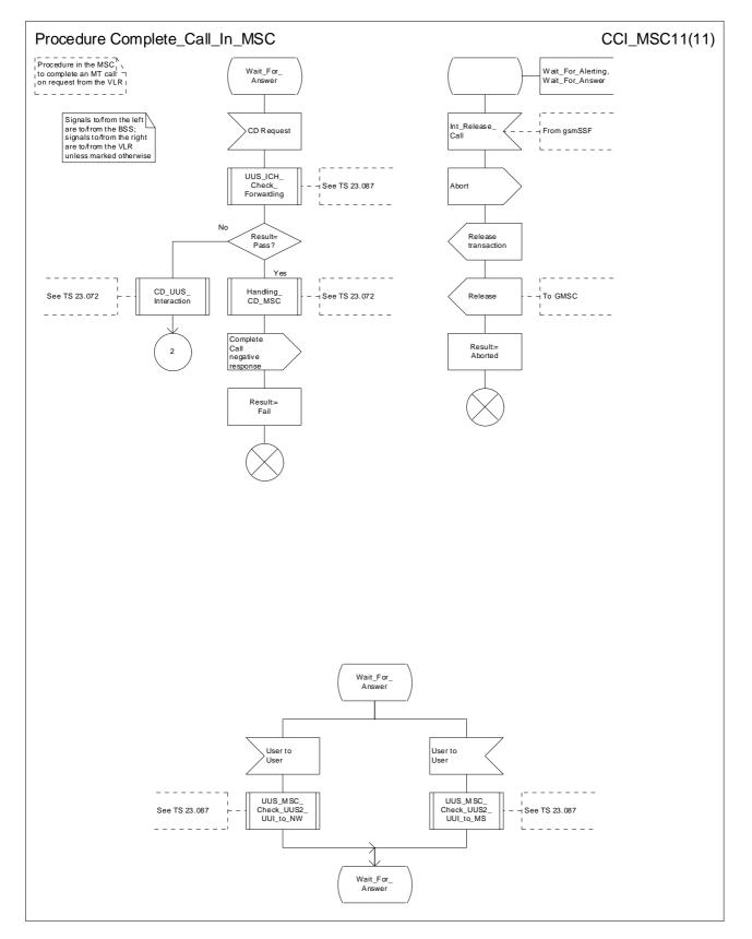
Figure 70k: Procedure Complete\_Call\_In\_MSC (sheet 11)
