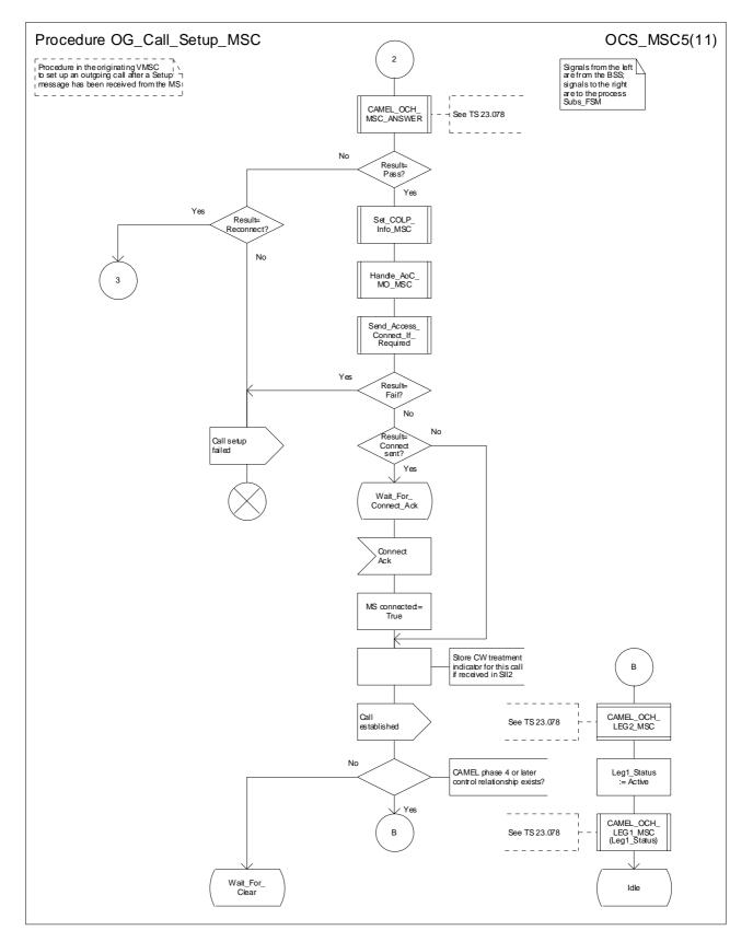
Figure 8e: Procedure OG\_Call\_Setup \_MSC (sheet 5)
