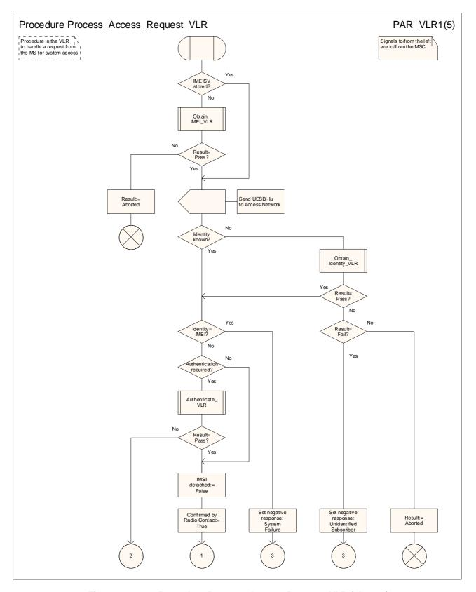
Figure 7.1.2.2a: Procedure Process\_Access\_Request\_VLR (sheet 1)
