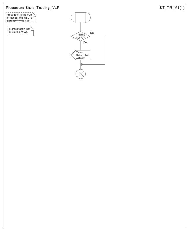
Figure 7.1.2.8: Procedure Start\_Tracing\_VLR
