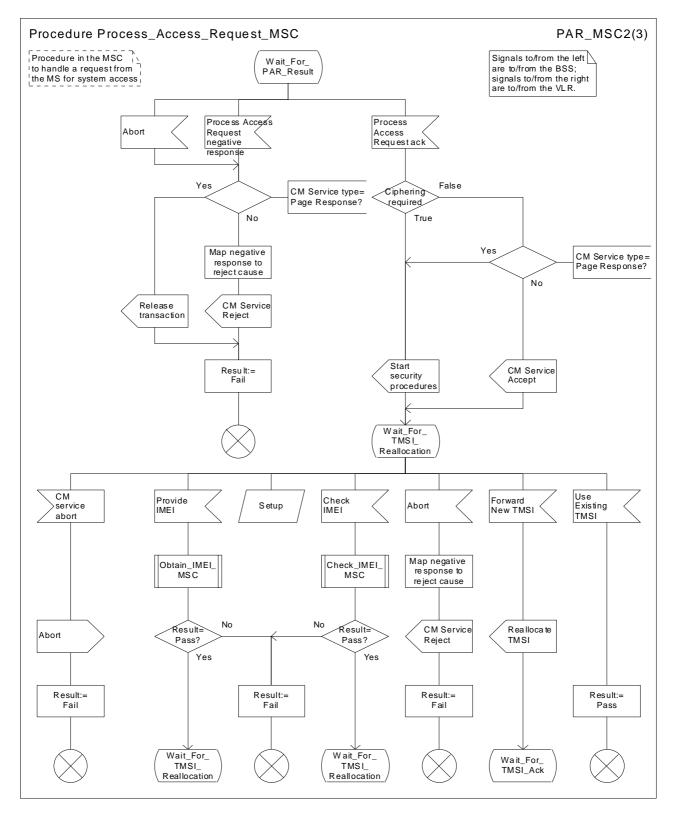
Figure 7b: Procedure Process\_Access\_Request\_MSC (sheet 2)
