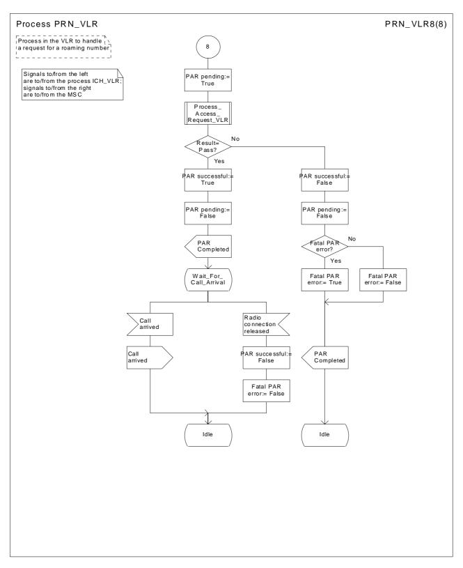
Figure 54h: Process PRN\_VLR (sheet 8)
