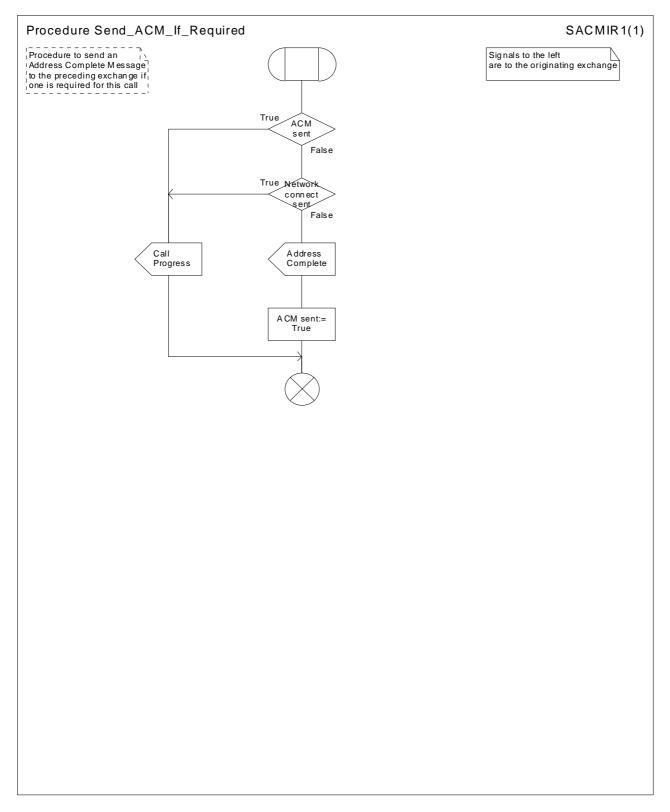
Figure 38: Procedure Send\_ACM\_If\_Required
