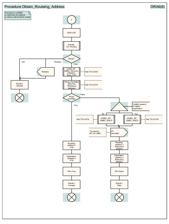
Figure 37f: Procedure Obtain\_Routeing\_Address (sheet 6)
