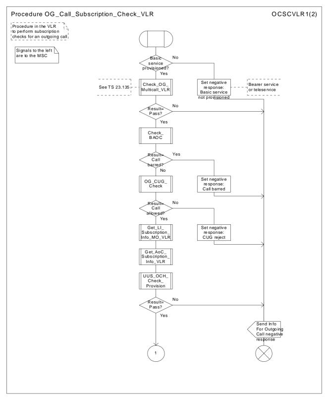
Figure 7.1.2.3a: Procedure OG\_Call\_Subscription\_Check\_VLR (sheet 1)
