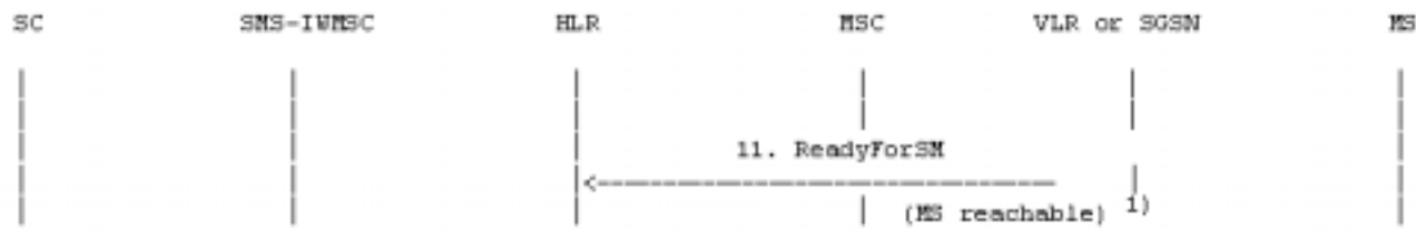
Figure 20a: The alert procedure when the MS becomes reachable, MNR, MNRG or both are set and MCEF is not set
