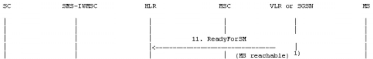
Figure 20a: The alert procedure when the MS becomes reachable, MNR, MNRG or both are set and MCEF is not set
