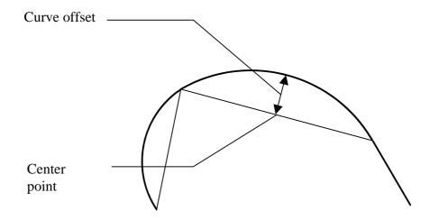
Curve offset values are within the range -0.5 to 0.5, inclusive. A value of 0.5 or -0.5 identifies that the curve offset equals half of length of the connecting line. The value indicates that the curve is close to a half circle. A positive value indicates that the curve is at the left side of the base line viewed from the curve direction. A negative value indicates that the curve is at the right side of the base line viewed from the curve direction.
