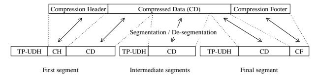
Figure 9.2.3.24.1 (a): Concatenation of a Compressed short message
