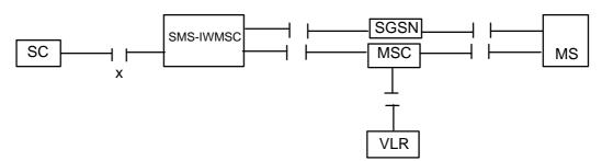
Figure 17: Interfaces involved in the Short message mobile originated procedure
