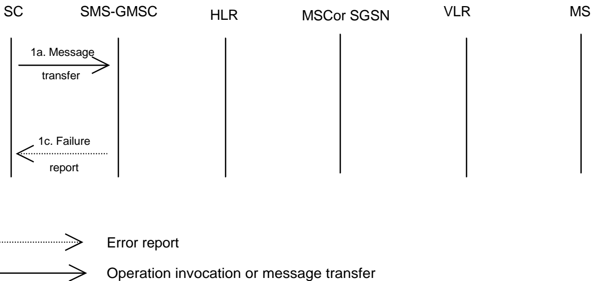
Figure 15b): Short message transfer attempt failing due to error at the SMS-GMSC
