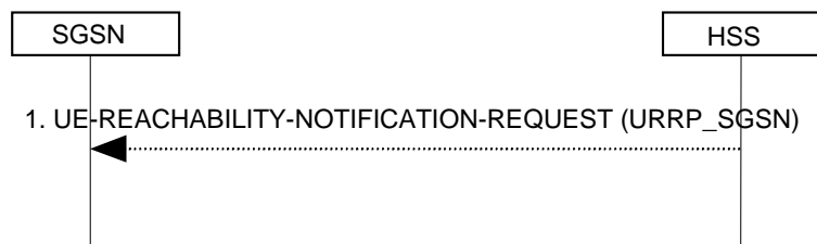
Figure 6.15-1: UE Reachability Notification Request Procedure
