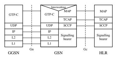
Figure 15: Control Plane GGSN - HLR Using GTP and MAP
