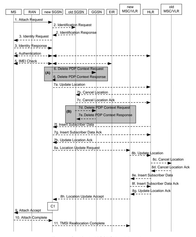
Figure 22: Combined GPRS / IMSI Attach Procedure
