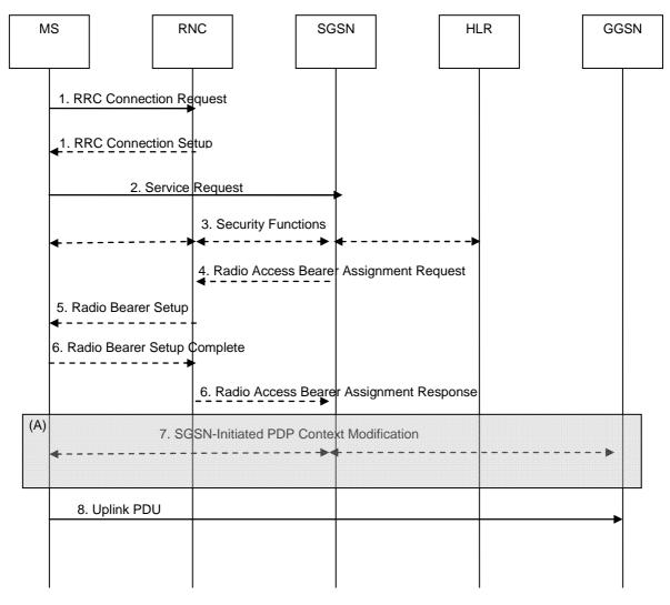
Figure 50: MS Initiated Service Request Procedure using Gn/Gp
