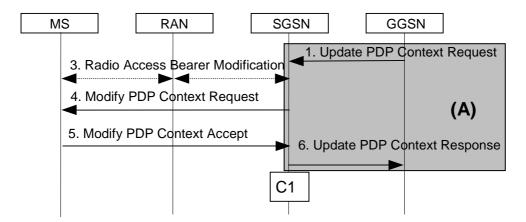
Figure 71b: GGSN-Initiated PDP Context Modification Procedure, lu mode
