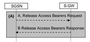
Figure 89b: Iu Release Procedure Using S4
