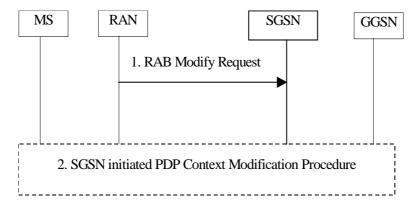
Figure 73: RAN-initiated RAB Modification Procedure
