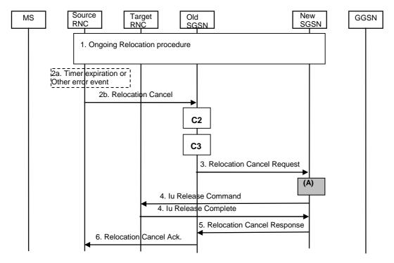
Figure 44: SRNS Cancel Relocation Procedure
