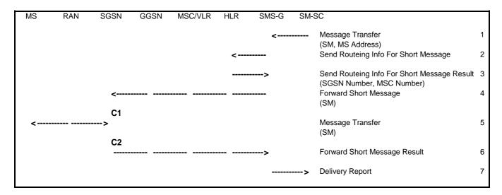
Figure 96: Mobile-terminated SMS Transfer, Successful
