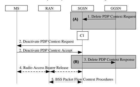
Figure 77: GGSN-initiated PDP Context Deactivation Procedure
