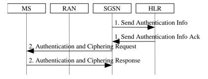
Figure 27: GSM Authentication Procedure
