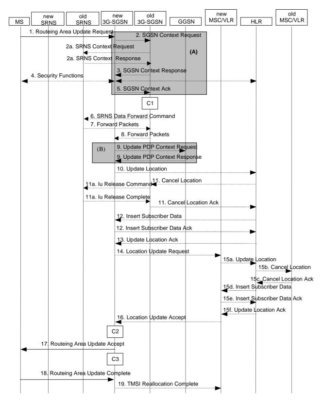
Figure 36: Iu mode RA Update Procedure
