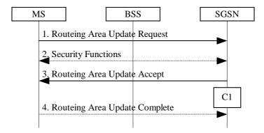
Figure 32: Intra SGSN Routeing Area Update Procedure
