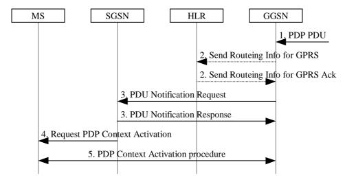
Figure 67: Successful Network-Requested PDP Context Activation Procedure
