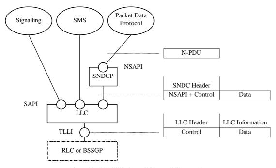
Figure 80: Multiplexing of Network Protocols
