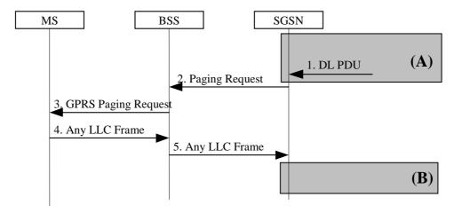
Figure 56: GPRS Paging Procedure (A/Gb mode)
