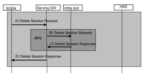
Figure 25A: SGSN interaction when using S4
