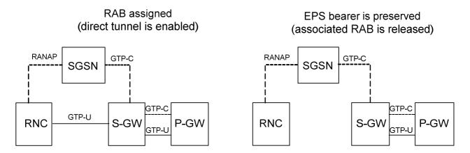
Figure 15.6-1: IDLE mode handling for S4 connectivity
