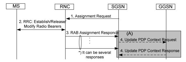
Figure 90a: RAB Assignment Procedure Using Gn/Gp
