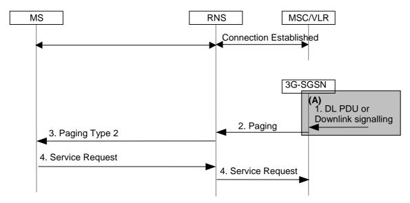
Figure 59: PS Paging by SGSN (Iu mode) With RRC Connection for CS
