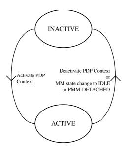
Figure 61: Functional PDP State Model
