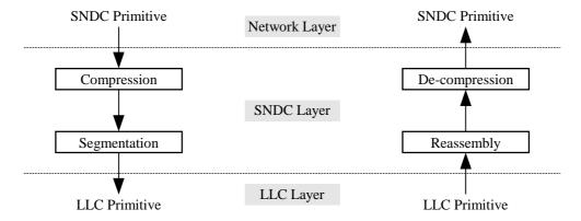
Figure 81: Sequential Invocation of SNDC Functionality
