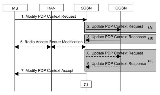
Figure 72b: MS-Initiated PDP Context Modification Procedure, lu mode
