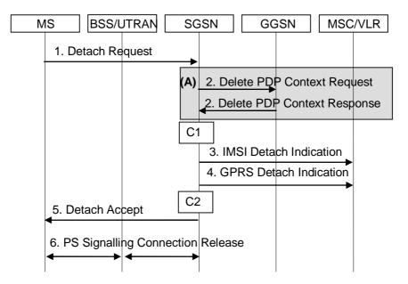
Figure 23: MS-Initiated Combined GPRS / IMSI Detach Procedure
