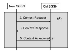
Figure 36a: Step 2, 3 and 5 for Iu Mode Routeing Area Update Procedure between S4-SGSNs
