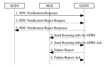
**Figure 68: Protection Procedure**
