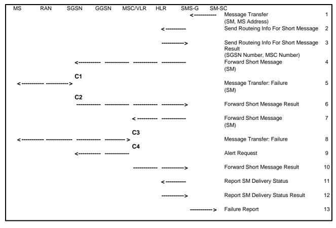
Figure 97: Mobile-terminated SMS Transfer, Unsuccessful
