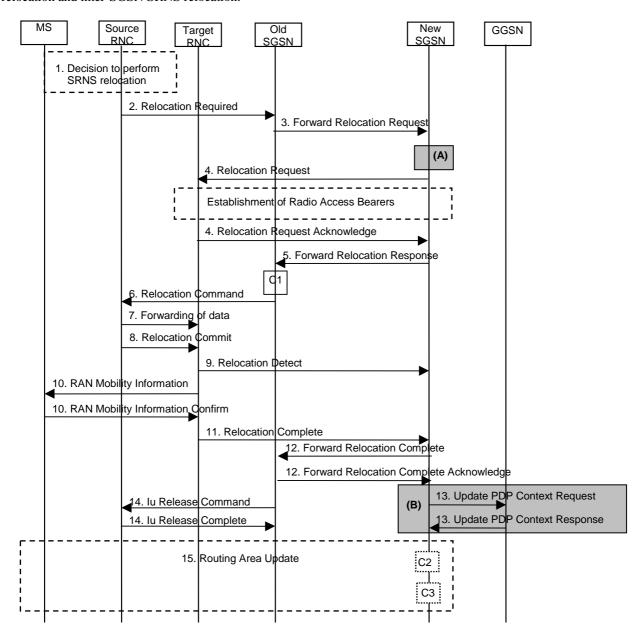
Figure 39: SRNS Relocation Procedure
