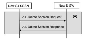
Figure 44a1: A) for SRNS Relocation Cancel Procedure Using S4
