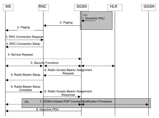
Figure 51: Network Initiated Service Request Procedure
