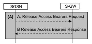
Figure 88b: RAB Release Procedure Using S4
