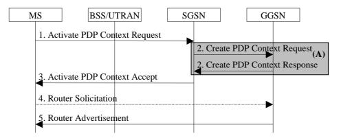
Figure 62: IPv6 Stateless Address Autoconfiguration Procedure
