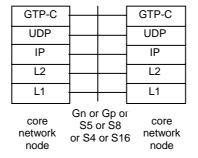
Figure 13: Control Plane for GTP-based Interfaces between Core Network Nodes
