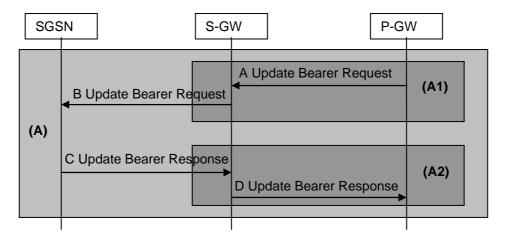
Figure 71c: PDN GW-Initiated EPS Bearer Modification Procedure
