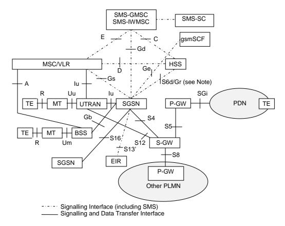
NOTE: Between S4-SGSN and HSS, the interface is Diameter based (S6d). However, to assist with the SGSN transition the use of MAP based Gr between the S4-SGSN and the HSS is not precluded.
