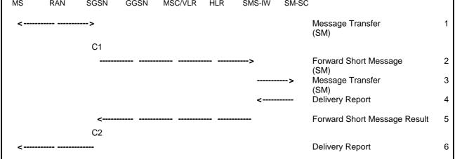
Figure 98: Mobile-originated SMS Transfer, Successful
