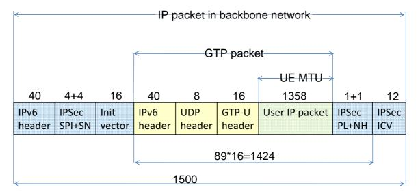
Figure C.1: Overhead for MTU calculation
