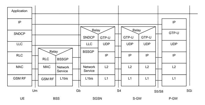
Figure 4a: User Plane for A/Gb mode and for GTP-based S5/S8
