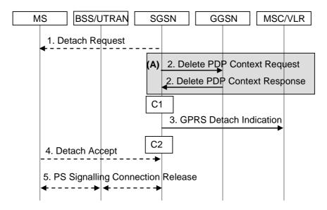
Figure 24: SGSN-Initiated GPRS Detach Procedure
