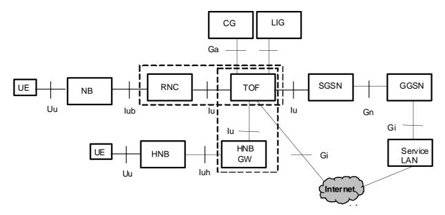
Figure B.1: Selected IP Traffic Offload from Traffic Offload Function (TOF) deployed at lu-PS
