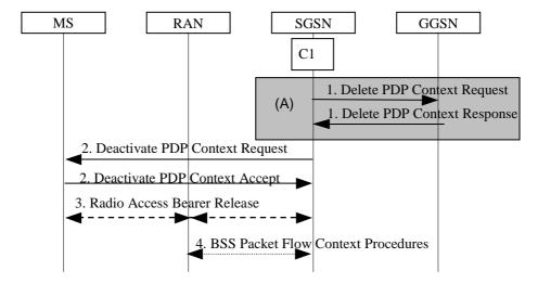
Figure 76: SGSN-initiated PDP Context Deactivation Procedure
