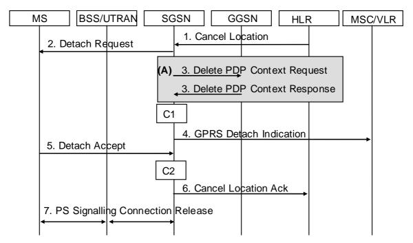
Figure 25: HLR-Initiated GPRS Detach Procedure
