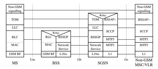
Figure 45: Control Plane MS - Non-GSM MSC/VLR
