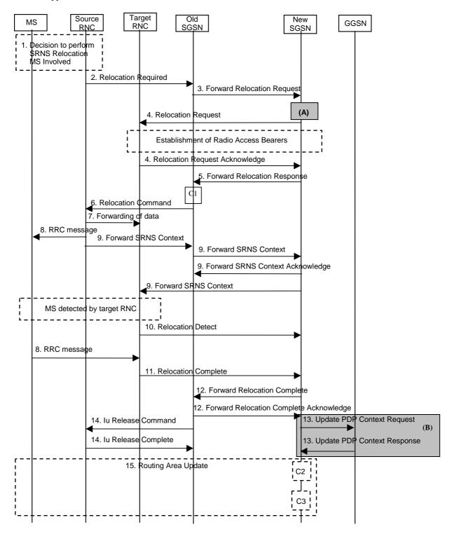
Figure 42: Combined Hard Handover and SRNS Relocation Procedure
