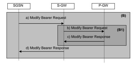
Figure 54-3: step 10 for lu mode to A/Gb mode Inter-SGSN Change using S4
