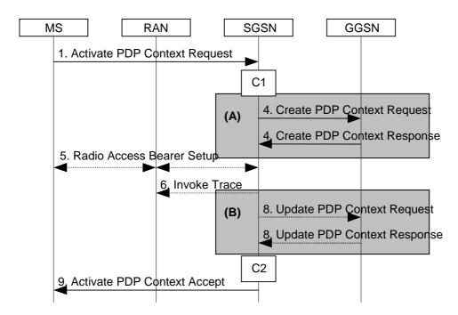
Figure 64: PDP Context Activation Procedure for lu mode
