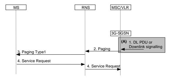
Figure 58: PS Paging by SGSN (lu mode) Without RRC Connection for CS
