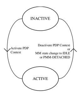
Figure 61: Functional PDP State Model
