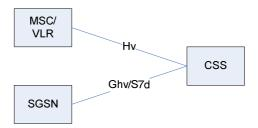
Figure 5.4.10-1: CSS connected to SGSN and MSC/VLR
