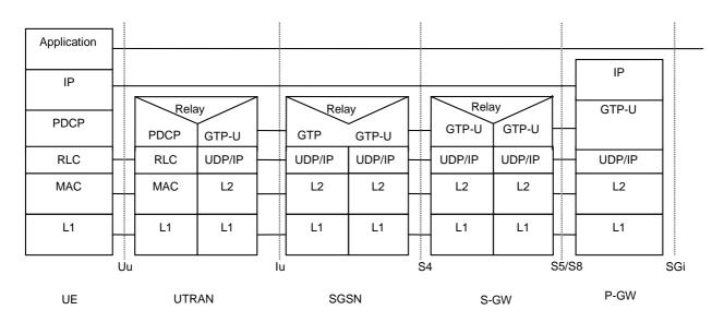
Figure 6c: User Plane with UTRAN for GTP-based S5/S8
