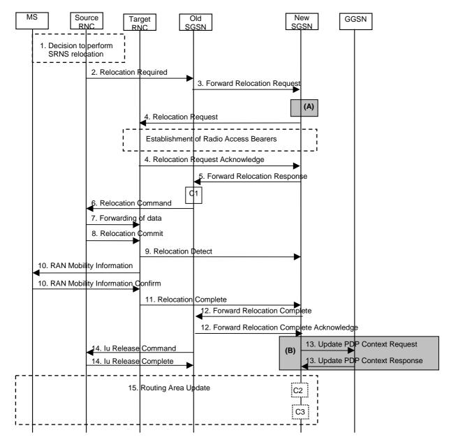
Figure 39: SRNS Relocation Procedure
