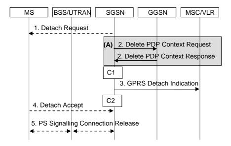
Figure 24: SGSN-Initiated GPRS Detach Procedure
