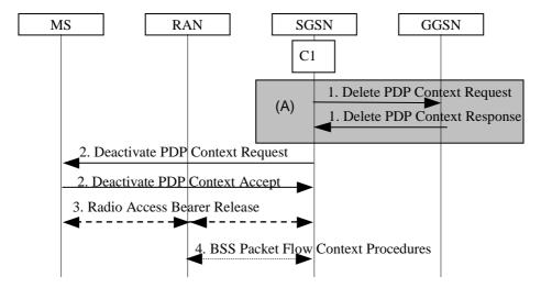
Figure 76: SGSN-initiated PDP Context Deactivation Procedure
