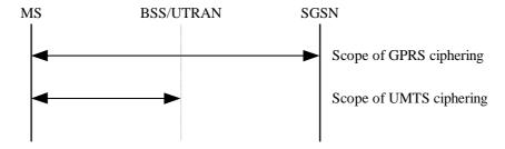
Figure 30: Scope of Ciphering
