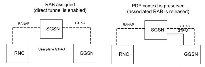
Figure 15.6-1: IDLE mode handling for Gn/Gp connectivity
