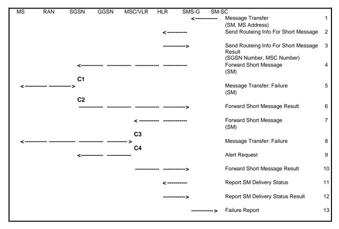
Figure 97: Mobile-terminated SMS Transfer, Unsuccessful
