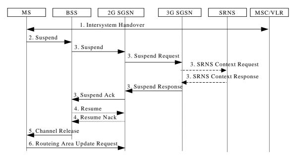
Figure 102: Suspend and Resume Procedure for inter-SGSN
