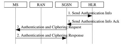
Figure 27: GSM Authentication Procedure
