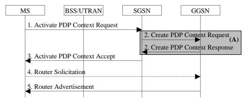
Figure 62: IPv6 Stateless Address Autoconfiguration Procedure
