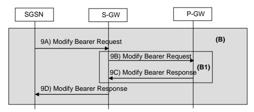
Figure 36b: Step 9 for lu Mode Routeing Area Update Procedure using S4
