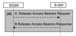
Figure 88b: RAB Release Procedure Using S4
