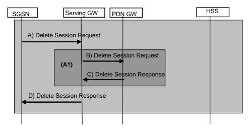
Figure 25A: SGSN interaction when using S4
