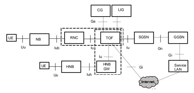
Figure B.1: Selected IP Traffic Offload from Traffic Offload Function (TOF) deployed at lu-PS
