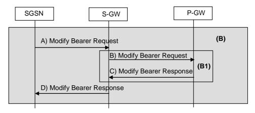
Figure 39b: Step 13 for Serving RNS Relocation Procedure, Combined Hard Handover and SRNS Relocation Procedure, and Combined Cell / URA Update and SRNS Relocation Procedure Using S4
