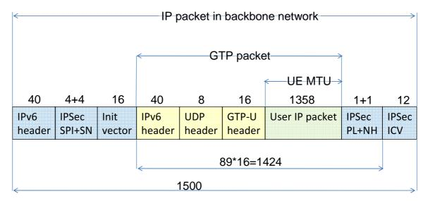
Figure C.1: Overhead for MTU calculation
