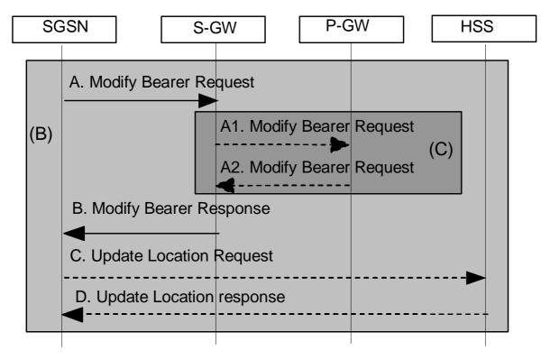
Figure 64b: PDP Context Activation Procedure steps (B) using S4
