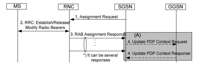
Figure 90a: RAB Assignment Procedure Using Gn/Gp
