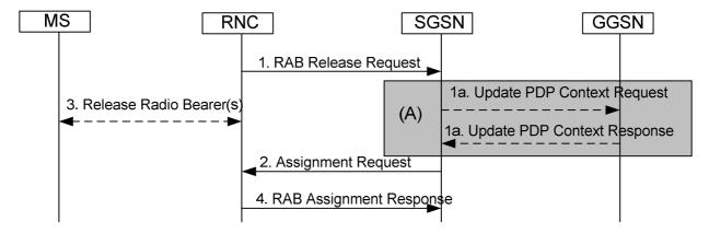
Figure 88a: RAB Release Procedure Using Gn/Gp
