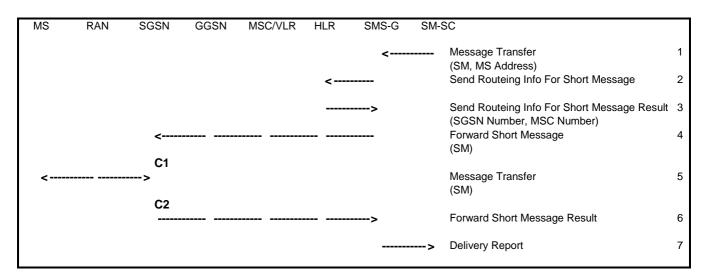
Figure 96: Mobile-terminated SMS Transfer, Successful
