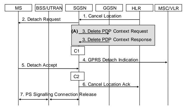
Figure 25: HLR-Initiated GPRS Detach Procedure
