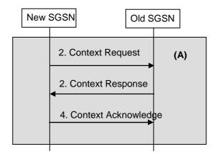
Figure 33a: Step 2 and 4 for Inter SGSN Routeing Area Update Procedure and Combined Inter SGSN RA / LA Update between S4-SGSNs
