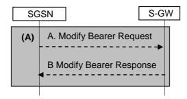
Figure 90b: RAB Assignment Procedure Using S4
