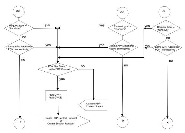
NOTE: This process is only applied by an SGSN when S4 is used.
