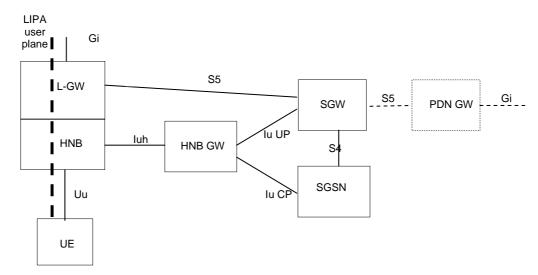
Figure 5.4.9-1: LIPA architecture for HNB subsystem connected to EPC
