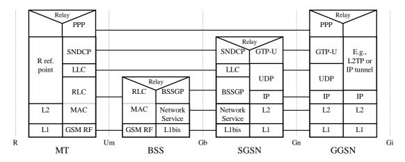
Figure 82: A/Gb mode User Plane for PDP Type PPP
