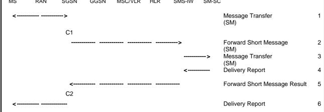
Figure 98: Mobile-originated SMS Transfer, Successful
