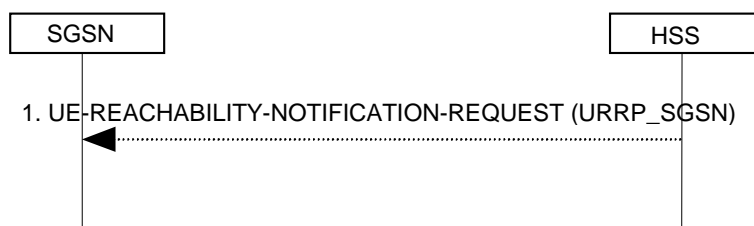
Figure 6.15-1: UE Reachability Notification Request Procedure
