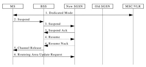
Figure 98: Suspend and Resume Procedure for inter-SGSN
