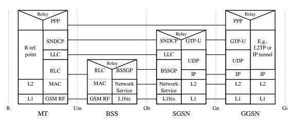
Figure 80: GSM User Plane for PDP Type PPP
