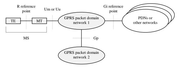
Figure 1: Packet Domain Access Interfaces and Reference Points
