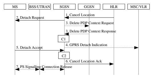
Figure 25: HLR-Initiated GPRS Detach Procedure
