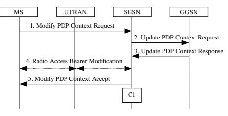
Figure 71: MS-Initiated PDP Context Modification Procedure
