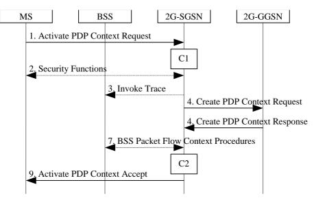
Figure 62: PDP Context Activation Procedure for GSM
