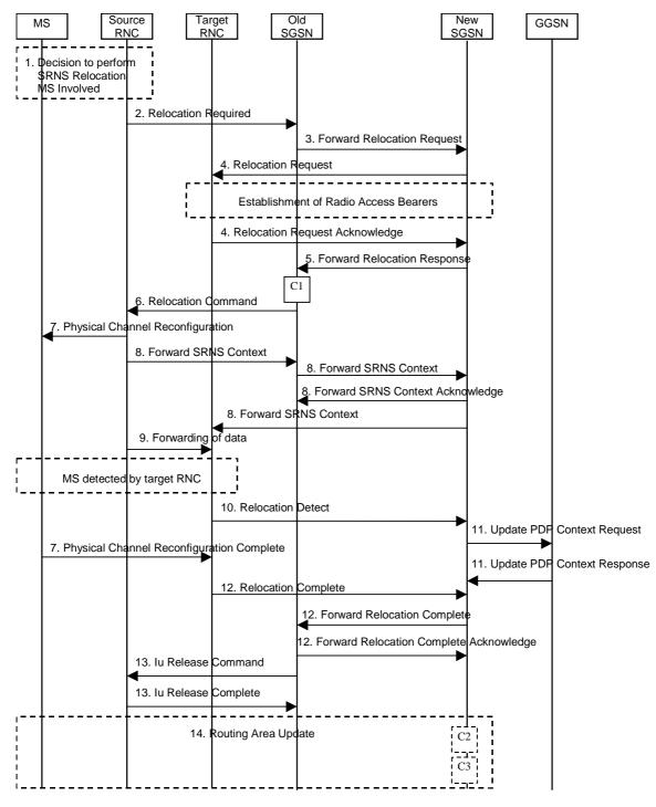
Figure 42: Combined Hard Handover and SRNS Relocation Procedure
