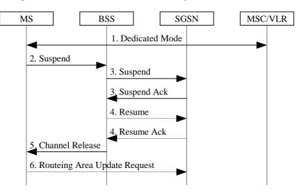
Figure 97: Suspend and Resume Procedure for intra SGSN
