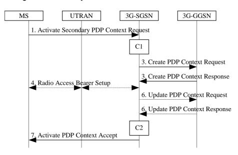
Figure 65: Secondary PDP Context Activation Procedure for UMTS
