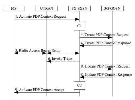
Figure 63: PDP Context Activation Procedure for UMTS
