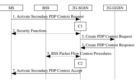
Figure 64: Secondary PDP Context Activation Procedure for GSM
