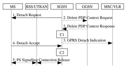
Figure 24: SGSN-Initiated GPRS Detach Procedure
