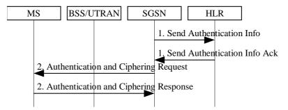
Figure 27: GSM Authentication Procedure
