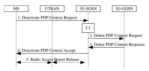
Figure 73: MS Initiated PDP Context Deactivation Procedure for UMTS
