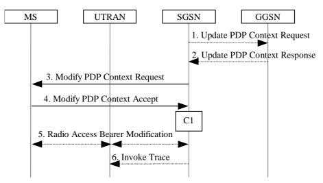
Figure 69: SGSN-Initiated PDP Context Modification Procedure
