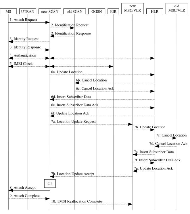
Figure 22: Combined GPRS / IMSI Attach Procedure
