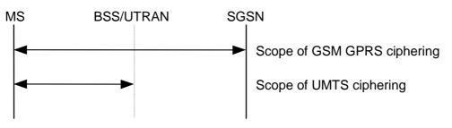
Figure 30: Scope of Ciphering
