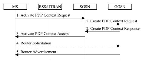
Figure 61: IPv6 Stateless Address Autoconfiguration Procedure
