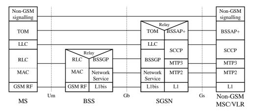
Figure 44: Control Plane MS - Non-GSM MSC/VLR
