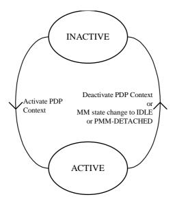
Figure 60: Functional PDP State Model
