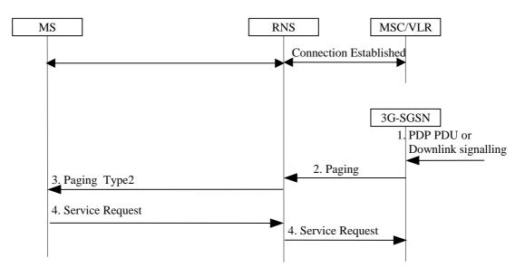
Figure 58: PS Paging With RRC Connection for CS
