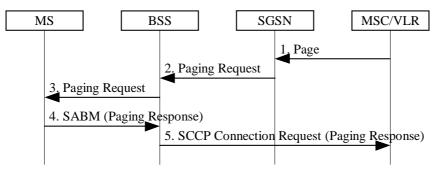
Figure 18: CS Paging Procedure in A/Gb mode
