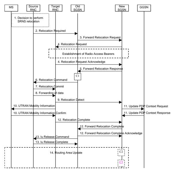
Figure 39: Serving SRNS Relocation Procedure
