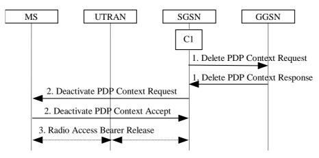
Figure 74: PDP Context Deactivation Initiated by SGSN Procedure
