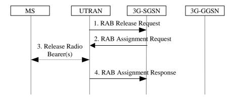
Figure 78: RAB Release Procedure
