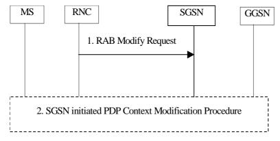
Figure 73: RNC-initiated RAB Modification Procedure
