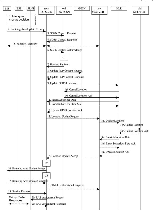
Figure 55: GSM to UMTS Inter SGSN Change
