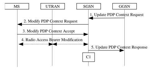
Figure 71: GGSN-Initiated PDP Context Modification Procedure
