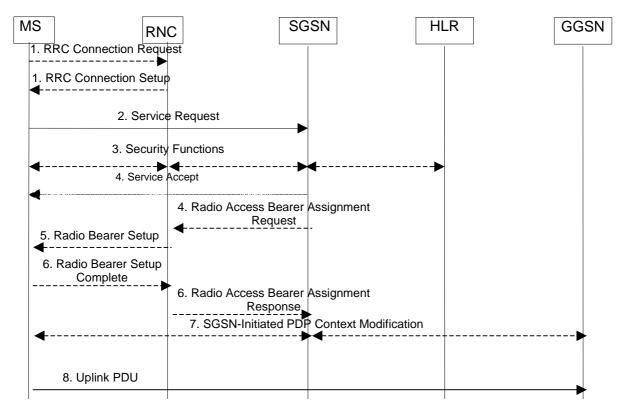
Figure 50: MS Initiated Service Request Procedure
