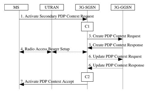
Figure 66: Secondary PDP Context Activation Procedure for UMTS
