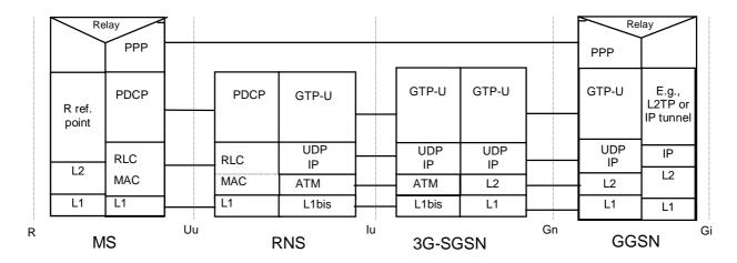
Figure 83: UMTS User Plane for PDP Type PPP
