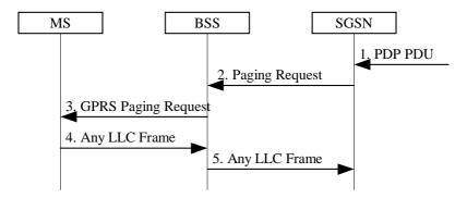
Figure 56: GPRS Paging Procedure
