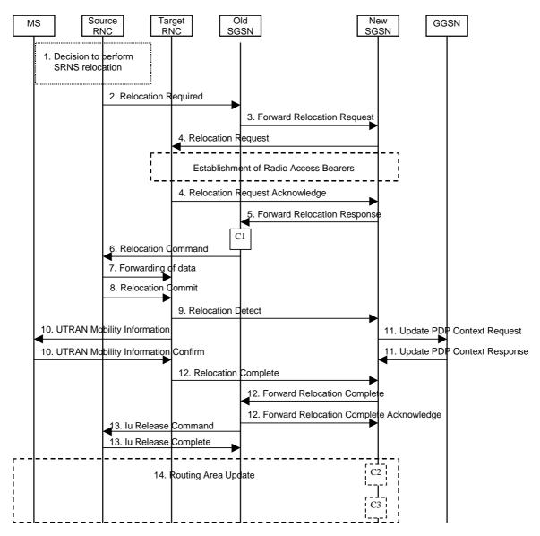
Figure 39: SRNS Relocation Procedure
