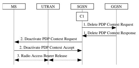
Figure 76: SGSN-initiated PDP Context Deactivation Procedure
