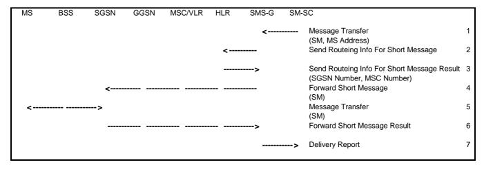
Figure 96: MT SMS Transfer, Successful
