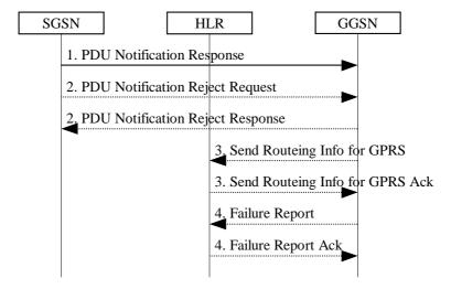
**Figure 68: Protection Procedure**
