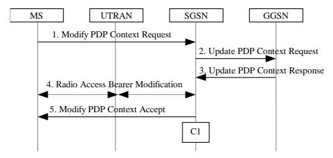
Figure 72: MS-Initiated PDP Context Modification Procedure
