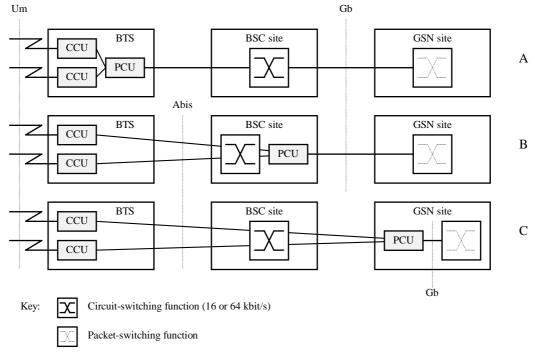
Figure 92: Remote Packet Control Unit (PCU) Positions
