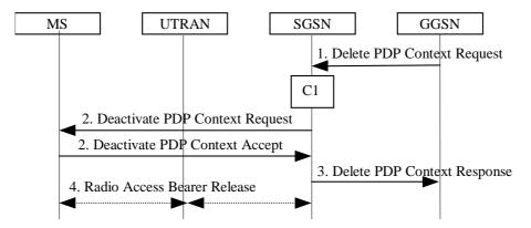
Figure 77: GGSN-initiated PDP Context Deactivation Procedure
