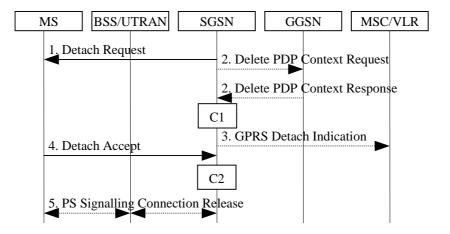
Figure 24: SGSN-Initiated GPRS Detach Procedure
