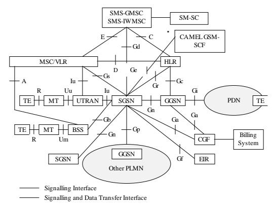
Figure 2: Overview of the Packet Domain Logical Architecture
