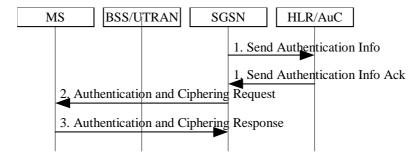
Figure 28: UMTS Authentication Procedure
