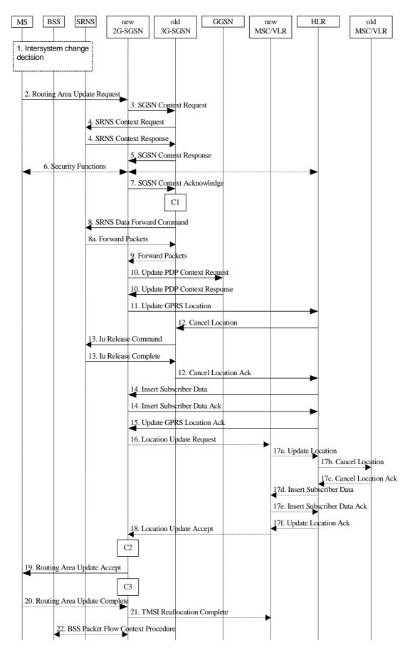
Figure 54: UMTS to GSM Inter-SGSN Change
