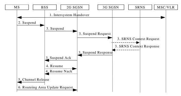
Figure 102: Suspend and Resume Procedure for inter-SGSN
