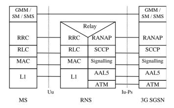
Figure 8: Control Plane MS - 3G-SGSN
