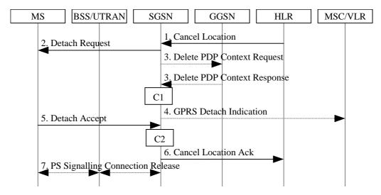
Figure 25: HLR-Initiated GPRS Detach Procedure
