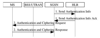
Figure 27: GSM Authentication Procedure
