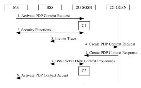
Figure 63: PDP Context Activation Procedure for GSM
