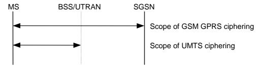
Figure 30: Scope of Ciphering
