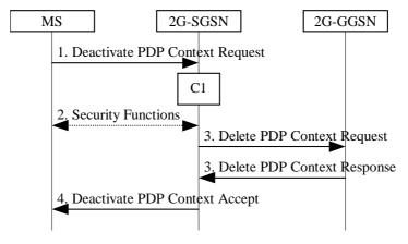
Figure 74: MS Initiated PDP Context Deactivation Procedure for GSM
