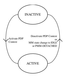
Figure 61: Functional PDP State Model
