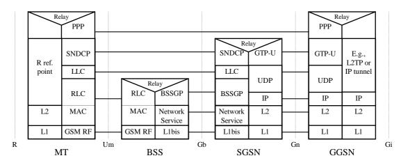
Figure 82: GSM User Plane for PDP Type PPP
