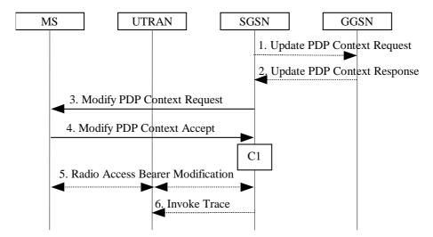
Figure 70: SGSN-Initiated PDP Context Modification Procedure
