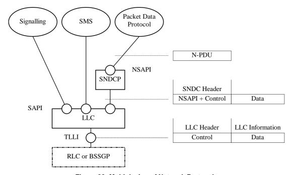
Figure 80: Multiplexing of Network Protocols
