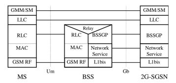
Figure 7: Control Plane MS - 2G-SGSN
