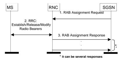
Figure 90: RAB Assignment Procedure
