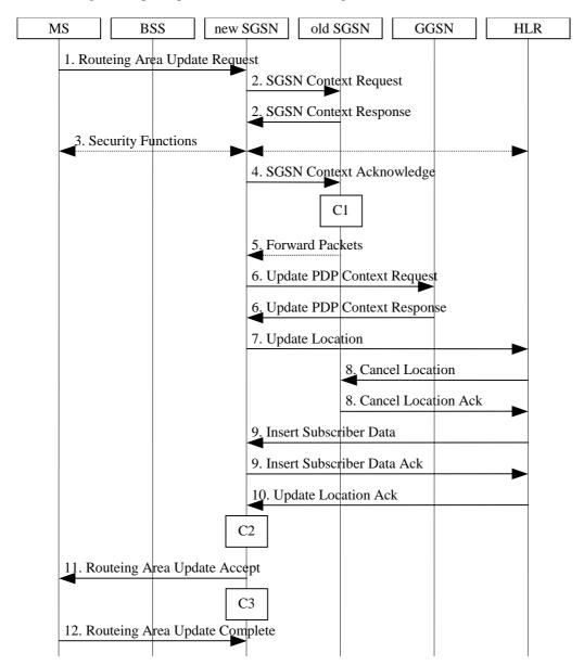
Figure 33: Inter SGSN Routeing Area Update Procedure
