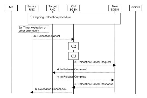
Figure 44: SRNS Cancel Relocation Procedure
