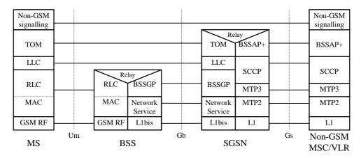
Figure 45: Control Plane MS - Non-GSM MSC/VLR
