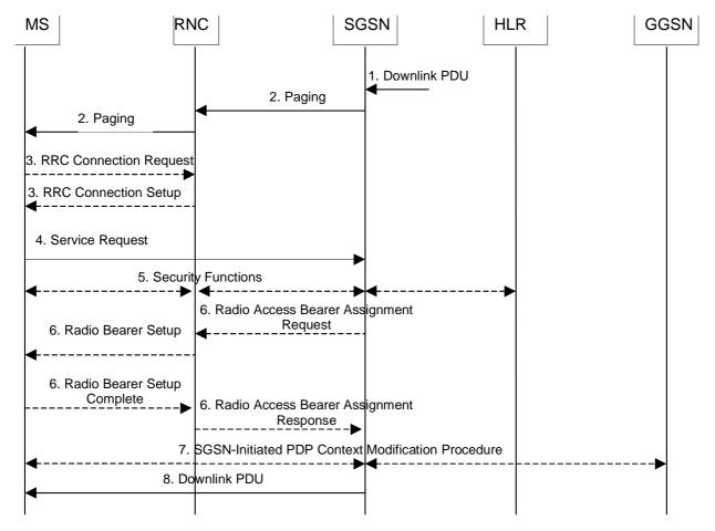
Figure 51: Network Initiated Service Request Procedure
