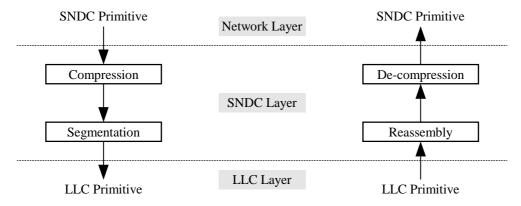
Figure 81: Sequential Invocation of SNDC Functionality
