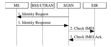
Figure 31: Identity Check Procedure
