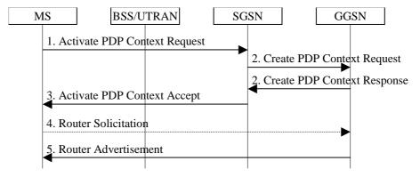
Figure 62: IPv6 Stateless Address Autoconfiguration Procedure
