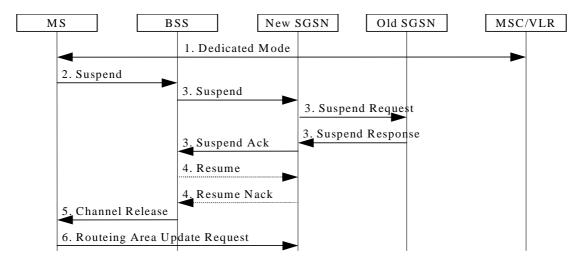
Figure 100: Suspend and Resume Procedure for inter-SGSN
