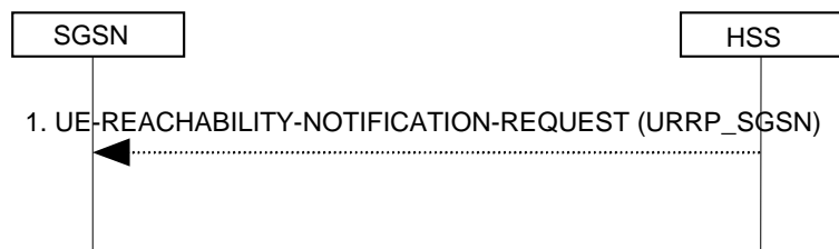
Figure 6.15-1: UE Reachability Notification Request Procedure
