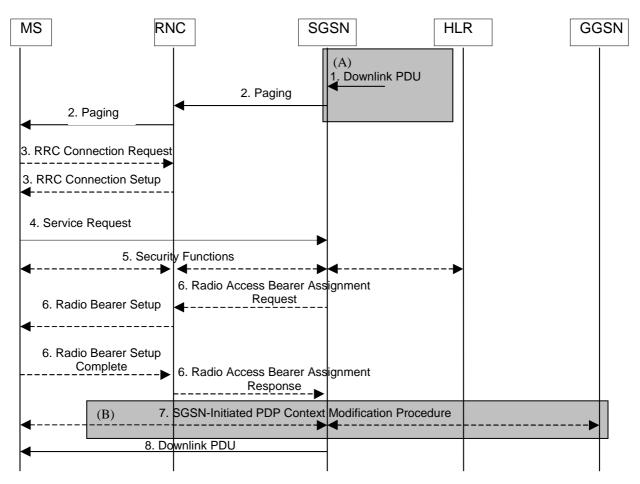
Figure 51: Network Initiated Service Request Procedure
