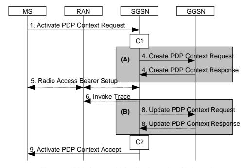
Figure 64: PDP Context Activation Procedure for lu mode
