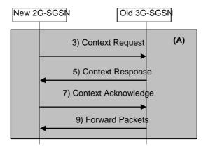
Figure 54-2: steps 3, 5, 7, 9 for lu mode to A/Gb mode Inter-SGSN Change using S4
