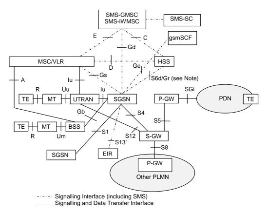
NOTE: Between S4-SGSN and HSS, the interface is Diameter based (S6d). However, to assist with the SGSN transition the use of MAP based Gr between the S4-SGSN and the HSS is not precluded.
