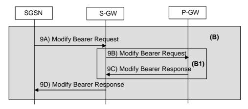
Figure 36b: Step 9 for Iu Mode Routeing Area Update Procedure using S4
