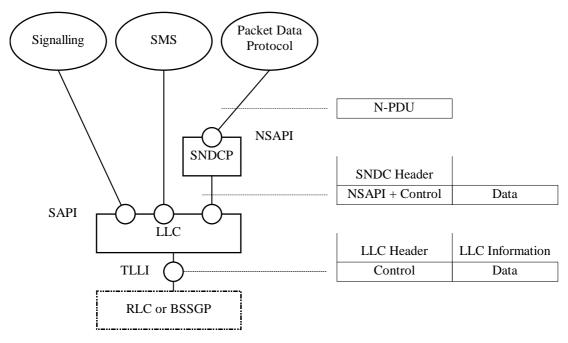
Figure 80: Multiplexing of Network Protocols
