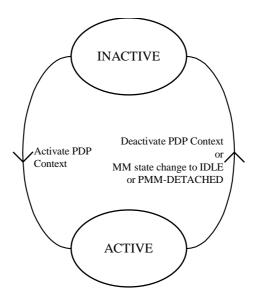
Figure 61: Functional PDP State Model
