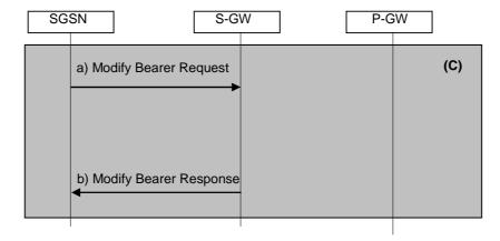
Figure 55-4: step 10 for A/Gb mode to lu mode Inter-SGSN Change using S4
