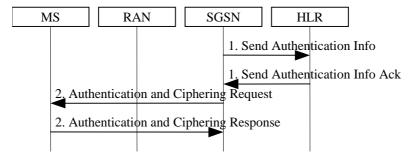
Figure 27: GSM Authentication Procedure
