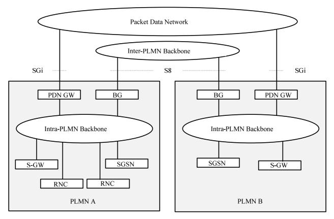
Figure 3a: Intra- and Inter-PLMN Backbone Networks when based on S5/S8 interfaces
