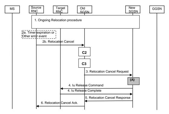
Figure 44: SRNS Cancel Relocation Procedure
