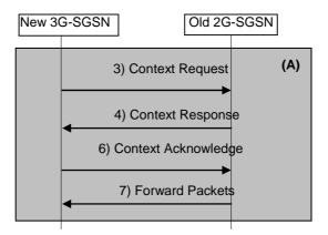
Figure 55-2: steps 3, 4, 6, 7 for A/Gb mode to lu mode Inter-SGSN Change using S4
