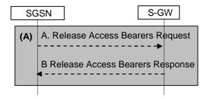
Figure 89b: Iu Release Procedure Using S4
