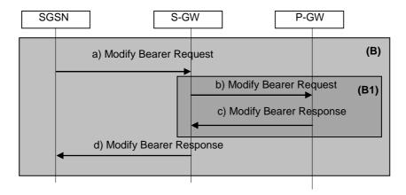
Figure 55-3: step 8 for A/Gb mode to lu mode Inter-SGSN Change using S4
