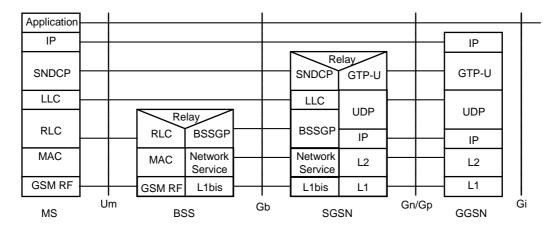
Figure 4: User Plane for A/Gb mode and for Gn/Gp
