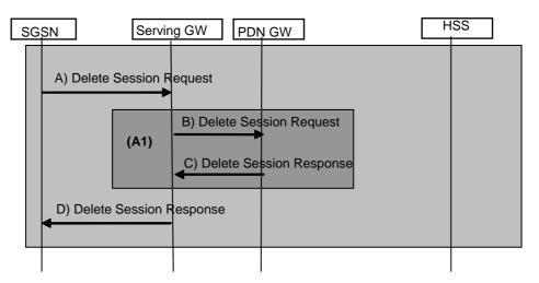
Figure 25A: SGSN interaction when using S4
