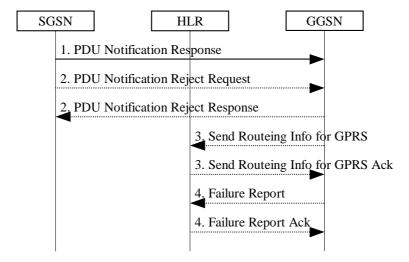
**Figure 68: Protection Procedure**
