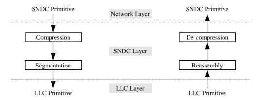
Figure 81: Sequential Invocation of SNDC Functionality
