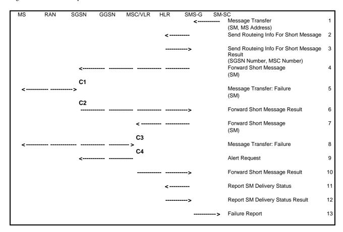
Figure 97: Mobile-terminated SMS Transfer, Unsuccessful
