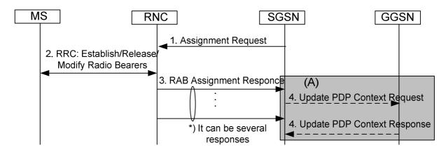
Figure 90a: RAB Assignment Procedure Using Gn/Gp
