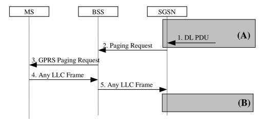
Figure 56: GPRS Paging Procedure (A/Gb mode)
