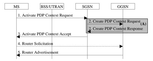
Figure 62: IPv6 Stateless Address Autoconfiguration Procedure
