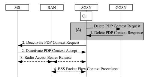
Figure 76: SGSN-initiated PDP Context Deactivation Procedure
