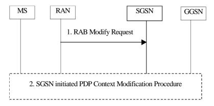
Figure 73: RAN-initiated RAB Modification Procedure
