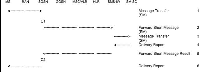
Figure 98: Mobile-originated SMS Transfer, Successful
