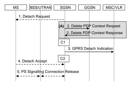
Figure 24: SGSN-Initiated GPRS Detach Procedure
