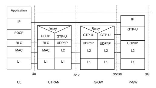
Figure 6d: User Plane with UTRAN for GTP-based S5/S8 and Direct Tunnel
