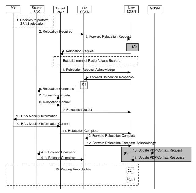
Figure 39: SRNS Relocation Procedure
