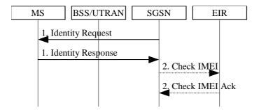
Figure 31: Identity Check Procedure
