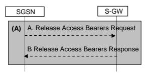
Figure 88b: RAB Release Procedure Using S4
