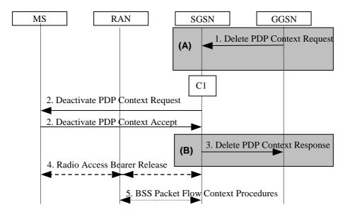
Figure 77: GGSN-initiated PDP Context Deactivation Procedure
