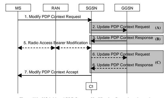
Figure 72b: MS-Initiated PDP Context Modification Procedure, lu mode
