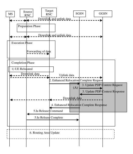
Figure 44a2: Enhanced Serving RNS Relocation
