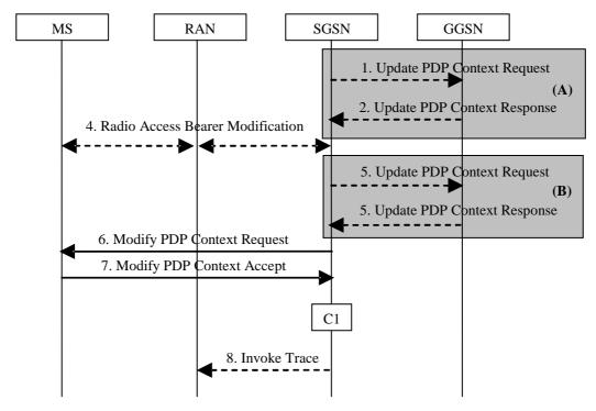
Figure 70b: SGSN-Initiated PDP Context Modification Procedure, lu mode
