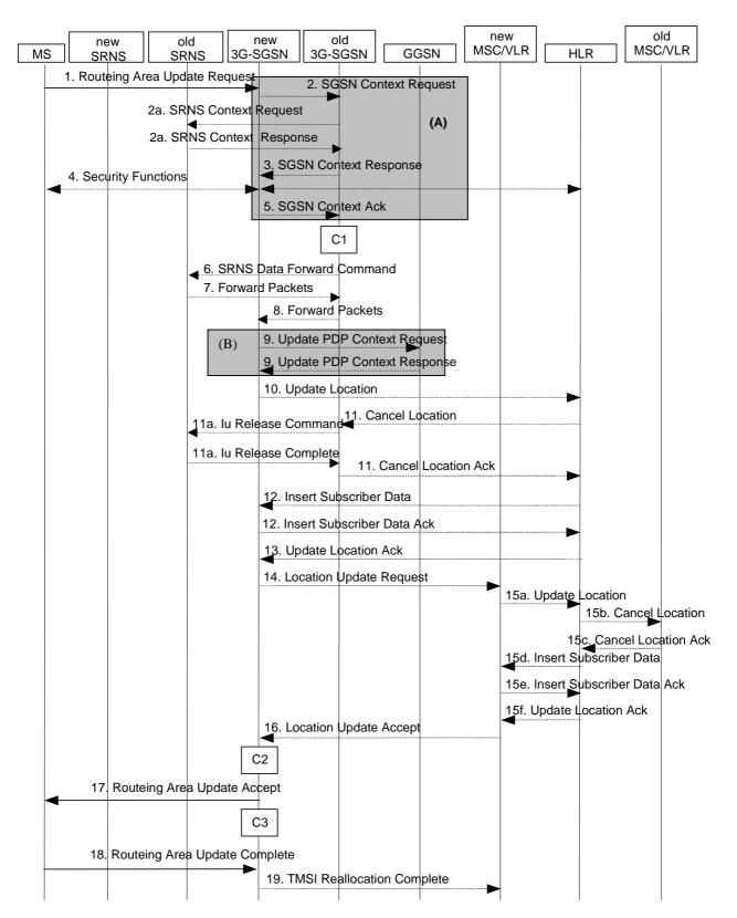
Figure 36: Iu mode RA Update Procedure
