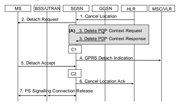
Figure 25: HLR-Initiated GPRS Detach Procedure
