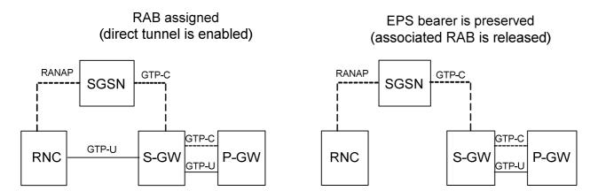
Figure 15.6-1: IDLE mode handling for S4 connectivity
