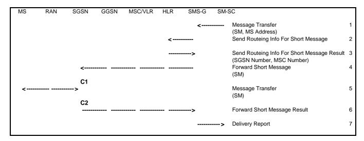
Figure 96: Mobile-terminated SMS Transfer, Successful
