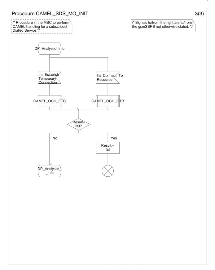
Figure 4.11c: Procedure CAMEL\_SDS\_MO\_INIT (sheet 3)
