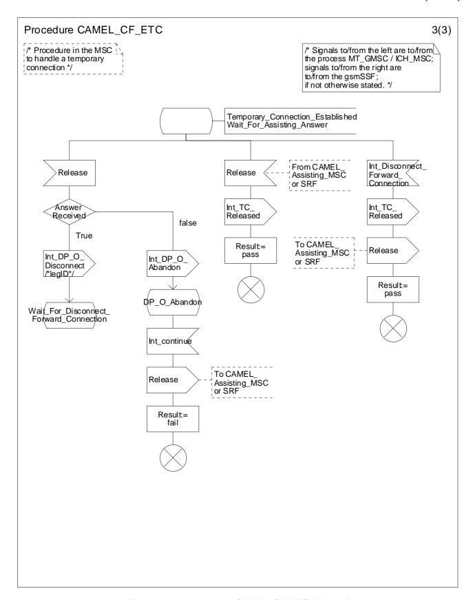
Figure 4.61c: Procedure CAMEL\_CF\_ETC (sheet 3)
