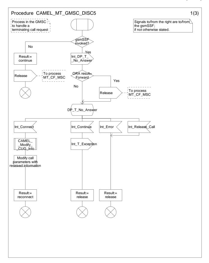
Figure 4.36a: Procedure CAMEL\_MT\_GMSC\_DISC5 (sheet 1)
