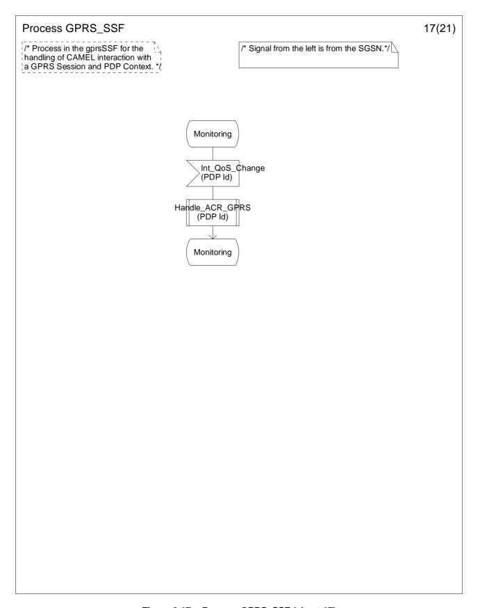
Figure 6.17q: Process GPRS\_SSF (sheet 17)
