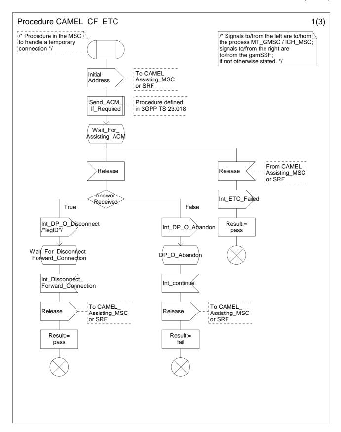
Figure 4.61a: Process CAMEL\_CF\_ETC (sheet 1)
