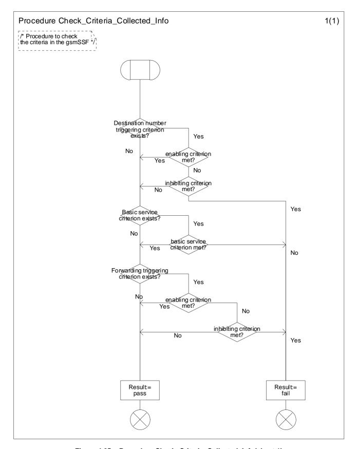
Figure 4.65a: Procedure Check\_Criteria\_Collected\_Info(sheet 1)
