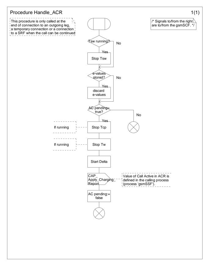
Figure 4.70a: Procedure Handle\_ACR (sheet 1)
