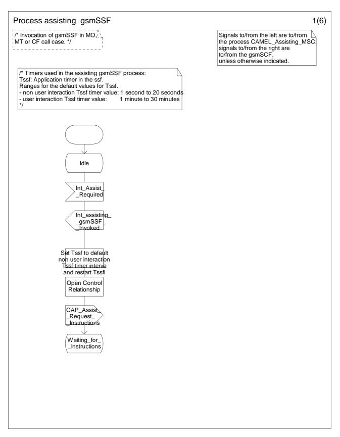
Figure 4.81a: Process Assisting\_gsmSSF (sheet 1)
