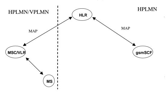
Figure 11.1a: Functional architecture for Any Time Interrogation
