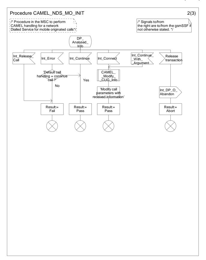
Figure 4.12b: Procedure CAMEL\_NDS\_MO\_INIT (sheet 2)
