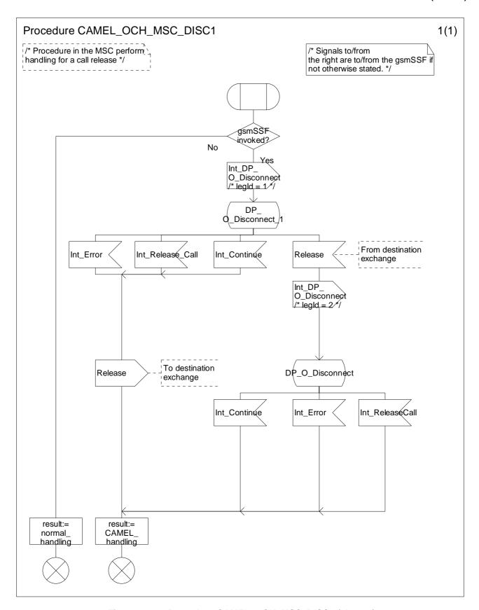
Figure 4.16a: Procedure CAMEL\_OCH\_MSC\_DISC1 (sheet 1)
