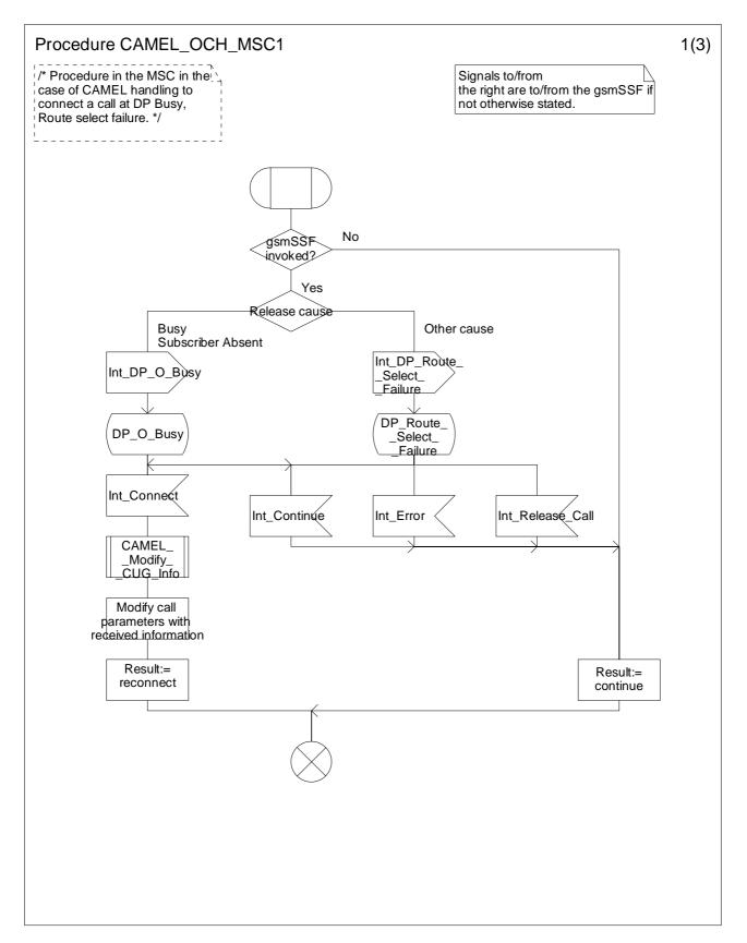
Figure 4.14a: Procedure CAMEL\_OCH\_MSC1 (sheet 1)
