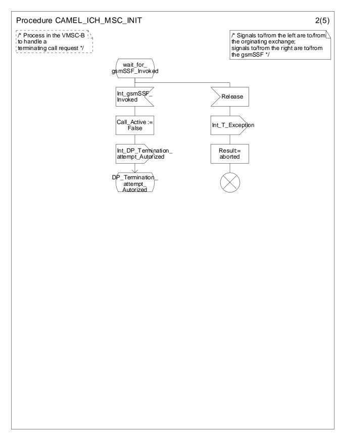
Figure 4.52b: Procedure CAMEL\_ICH\_MSC\_INIT (sheet 2)
