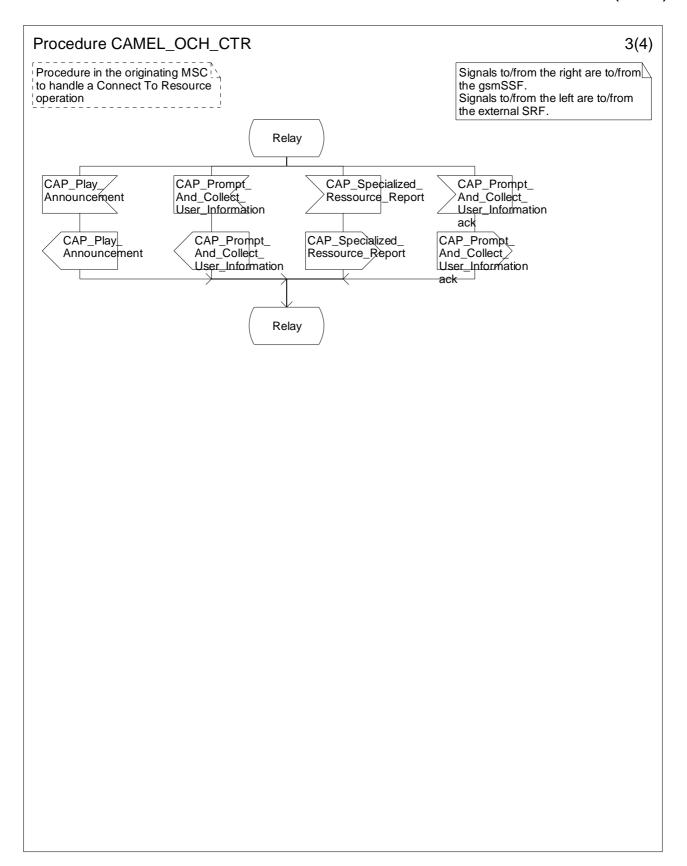
Figure 4.21c: Procedure CAMEL\_OCH\_CTR (sheet 3)
