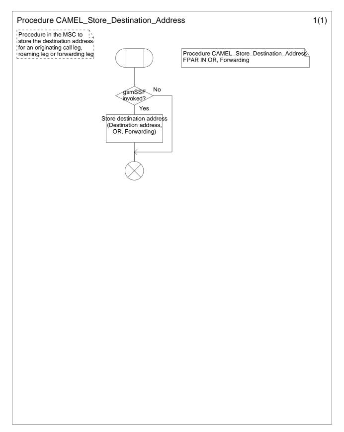
Figure 4.24: Procedure CAMEL\_Store\_Destination\_Address (sheet 1)
