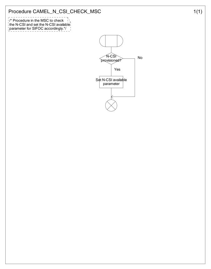
Figure 4.26: Procedure CAMEL\_N\_CSI\_CHECK\_MSC (sheet 1)
