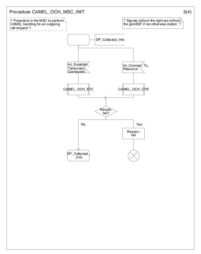
Figure 4.10c: Procedure CAMEL\_OCH\_MSC\_INIT (sheet 3)
