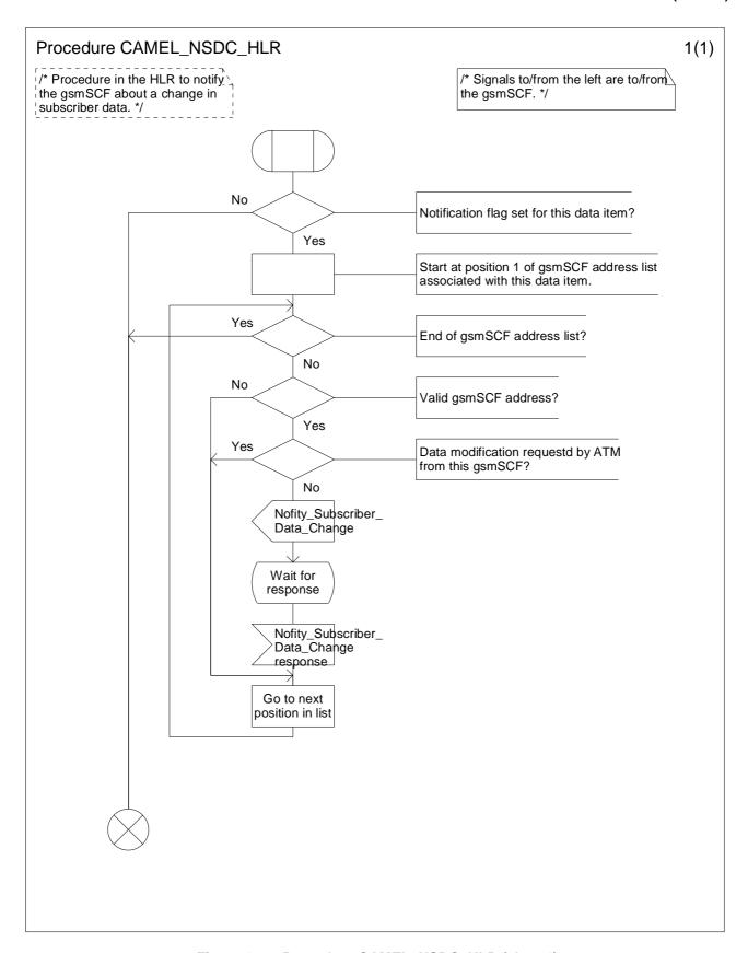
Figure 10.8: Procedure CAMEL\_NSDC\_HLR (sheet1)
