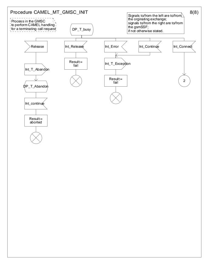
Figure 4.30h: Procedure CAMEL\_MT\_GMSC\_INIT (sheet 8)
