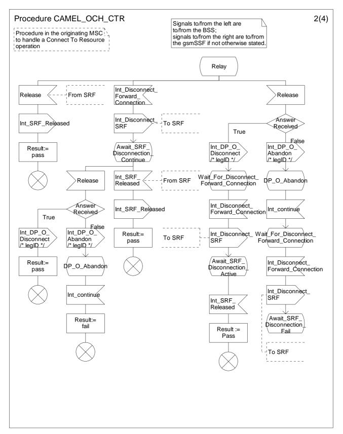
Figure 4.21b: Procedure CAMEL\_OCH\_CTR (sheet 2)
