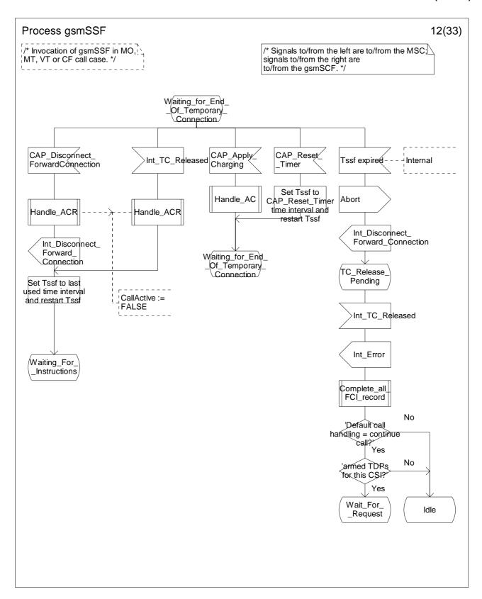
Figure 4.64I: Process gsmSSF (sheet 12)
