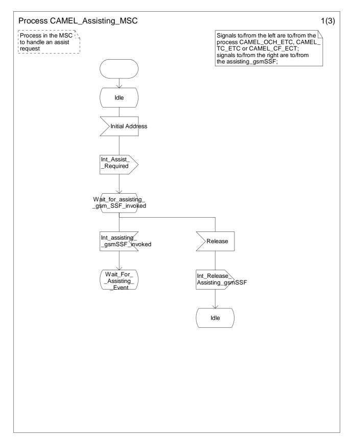
Figure 4.80a: Process CAMEL\_Assisting\_MSC (sheet 1)
