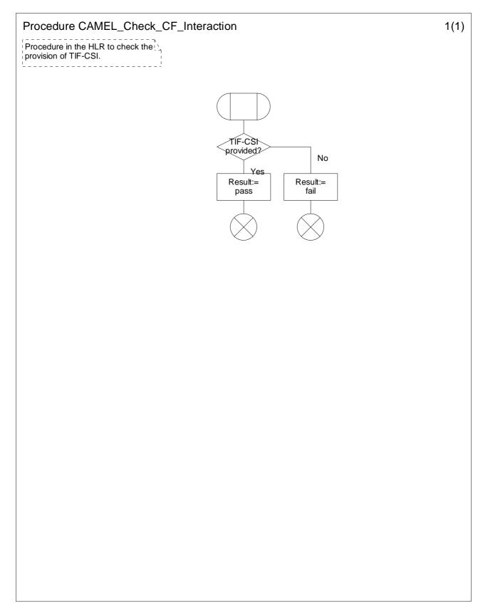
Figure 4.83: Procedure CAMEL\_Check\_CF\_Interaction
