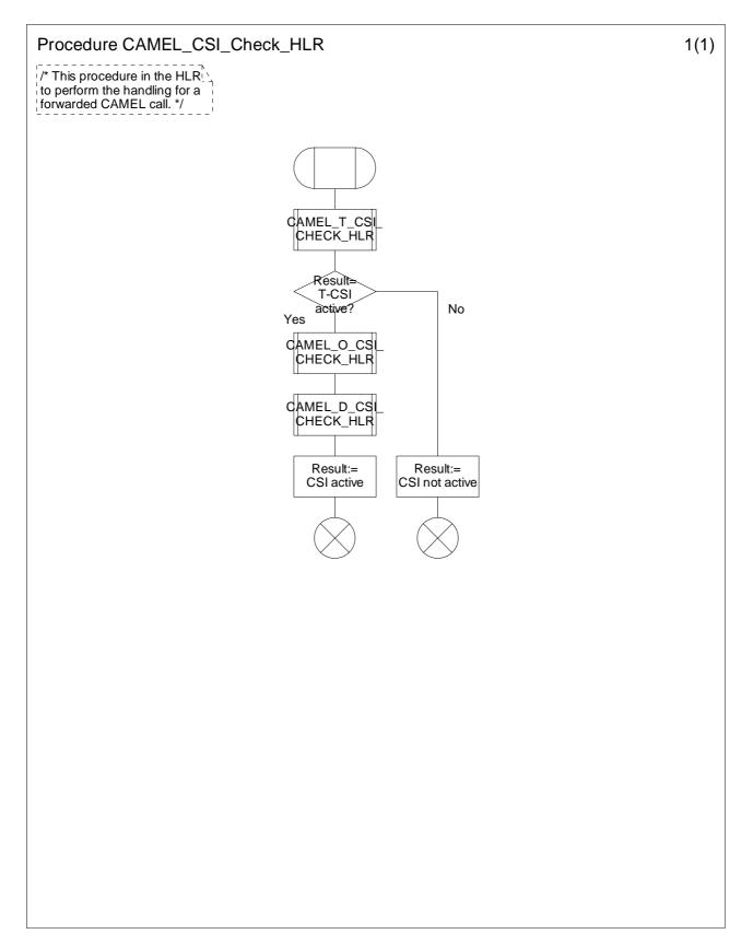
Figure 4.42: Procedure CAMEL\_CSI\_Check\_HLR (sheet 1)
