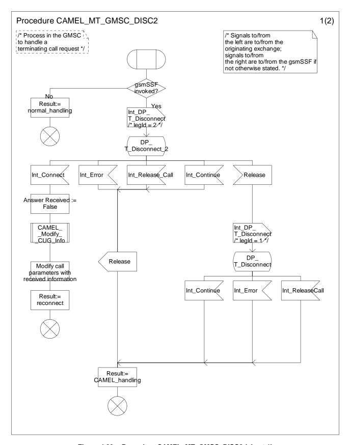
Figure 4.33a: Procedure CAMEL\_MT\_GMSC\_DISC2 (sheet 1)
