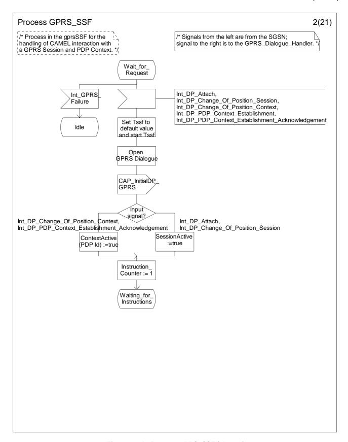
Figure 6.17b: Process GPRS\_SSF (sheet 2)
