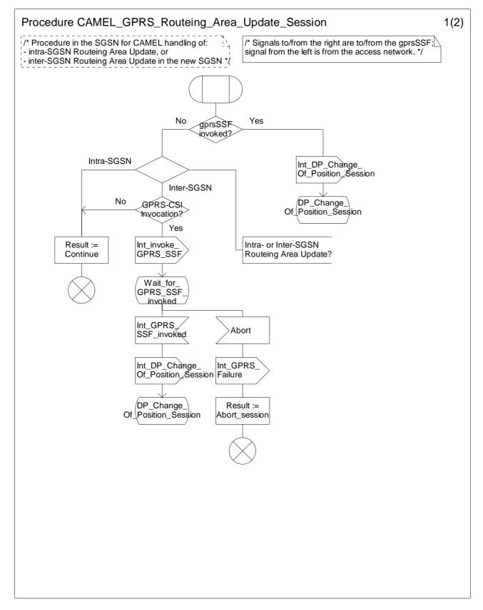
Figure 6.10a: Procedure CAMEL\_GPRS\_Routeing\_Area\_Update\_Session (sheet 1)
