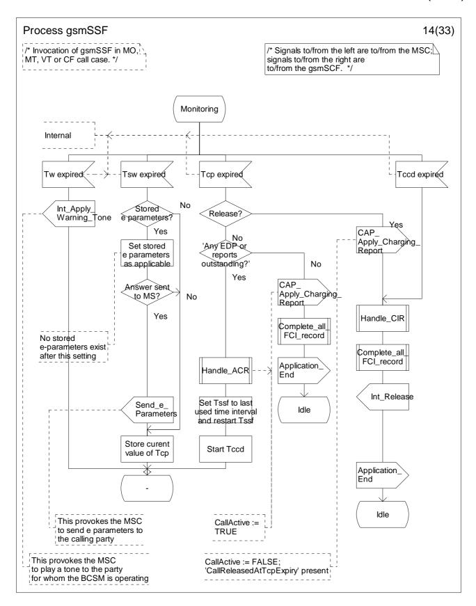
Figure 4.64n: Process gsmSSF (sheet 14)
