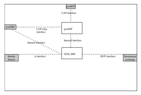
Figure 4.8a: Outgoing case (gsmSSF relay)
