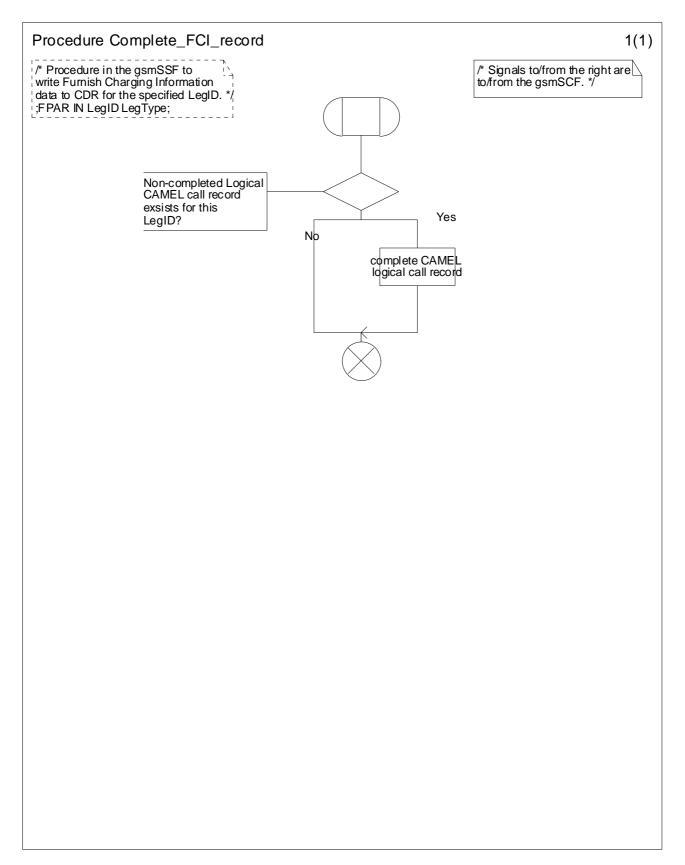
Figure 4.73a: Procedure Complete\_FCI\_record (sheet 1)
