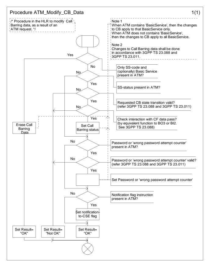
Figure 10.7: Procedure ATM\_Modify\_CB\_Data (sheet 1)
