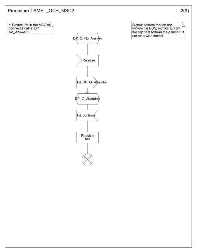
Figure 4.15b: Procedure CAMEL\_OCH\_MSC2 (sheet 2)
