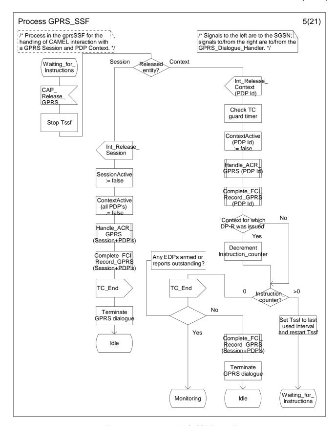
Figure 6.17e: Process GPRS\_SSF (sheet 5)
