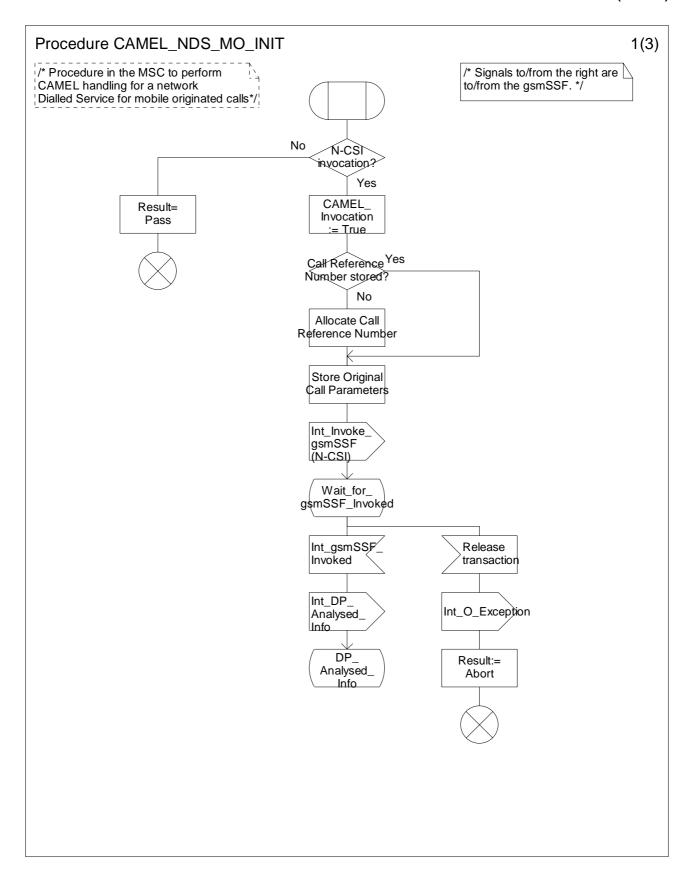
Figure 4.12a: Procedure CAMEL\_NDS\_MO\_INIT (sheet 1)
