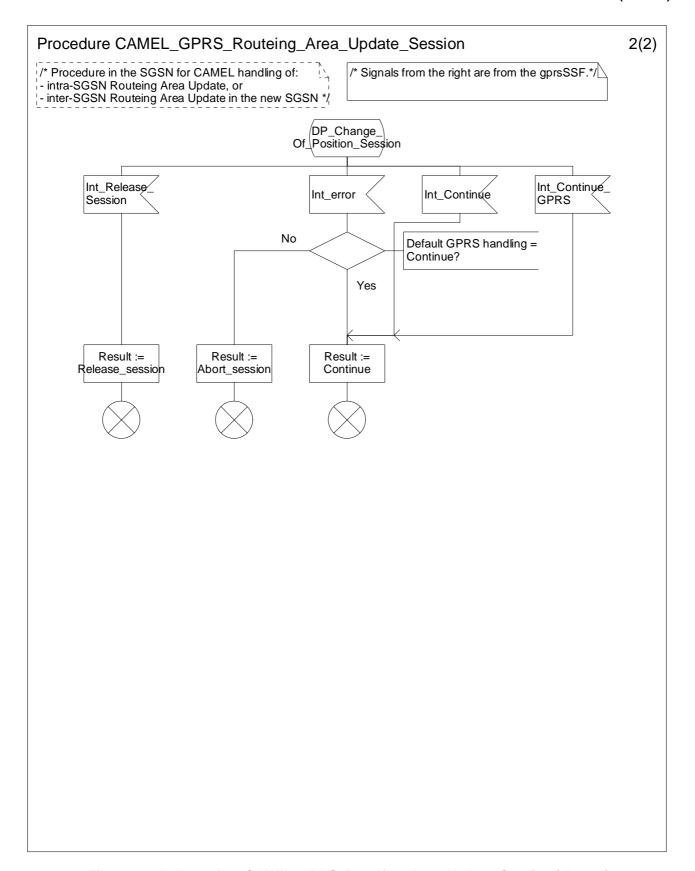
Figure 6.10b: Procedure CAMEL\_GPRS\_Routeing\_Area\_Update\_Session (sheet 2)
