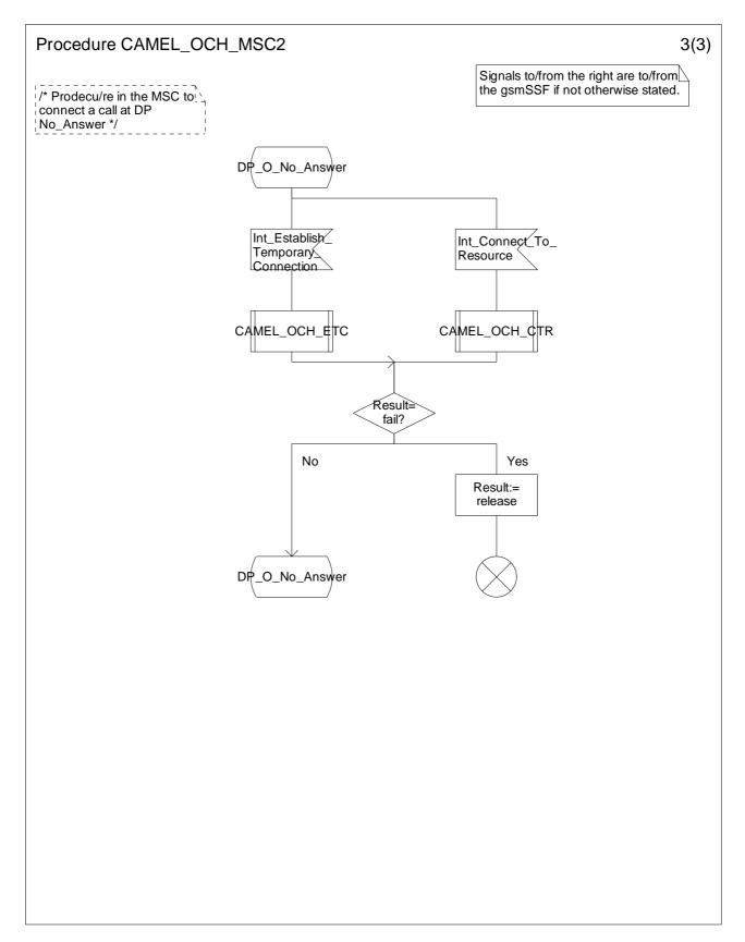
Figure 4.15c: Procedure CAMEL\_OCH\_MSC2 (sheet 3)
