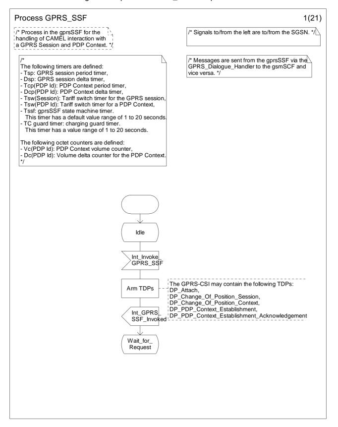
Figure 6.17a: Process GPRS\_SSF (sheet 1)
