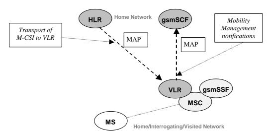
Figure 9.1: Functional architecture for support of CAMEL
