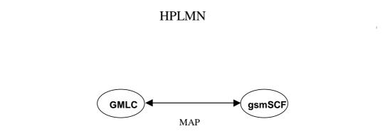
Figure 11.1b: Functional architecture for CAMEL Support of Location Services
