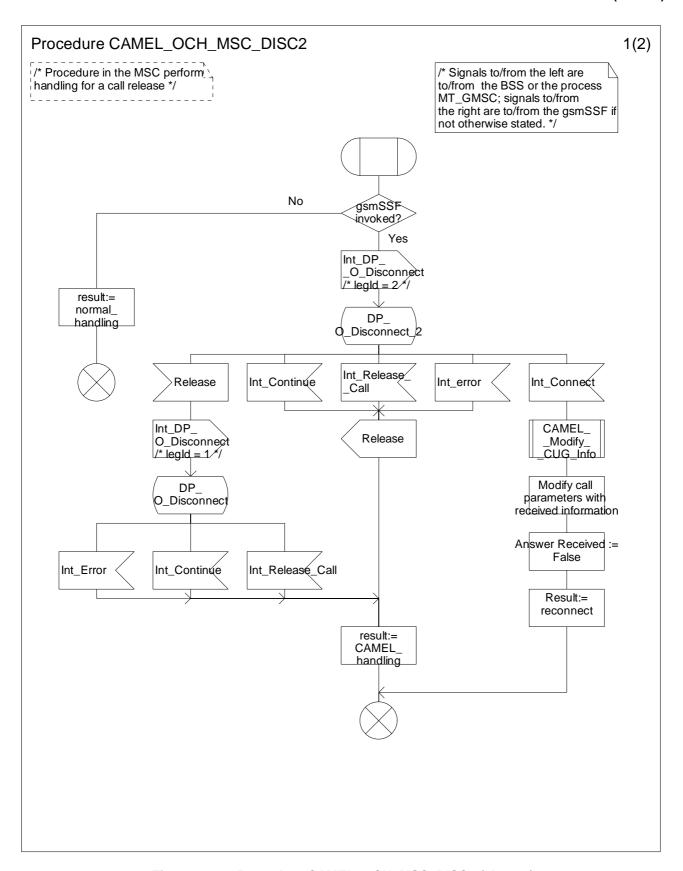
Figure 4.17a: Procedure CAMEL\_OCH\_MSC\_DISC2 (sheet 1)
