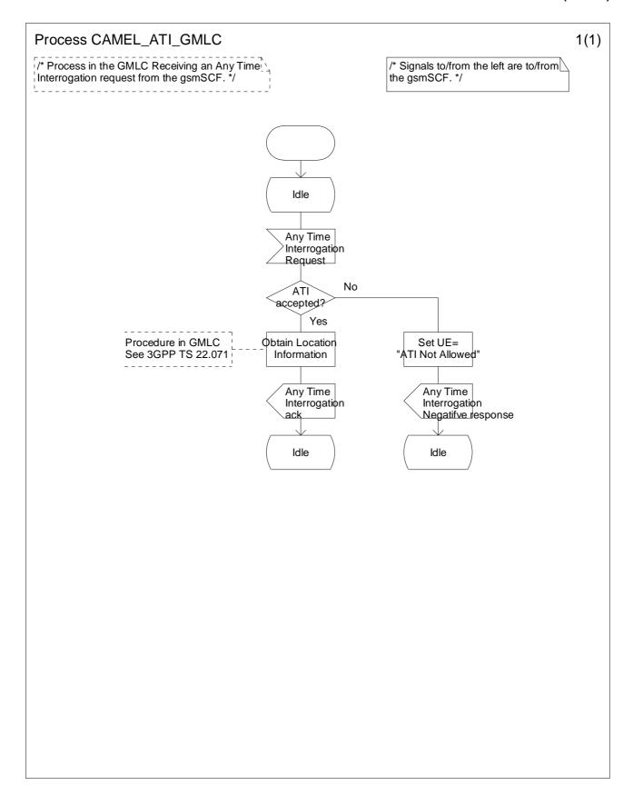
Figure 11.2: Process CAMEL\_ATI\_GMLC (sheet 1)
