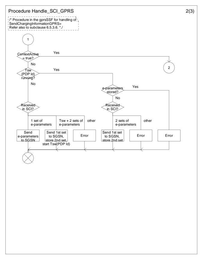
Figure 6.23b: Procedure Handle\_SCI\_GPRS (sheet 2)
