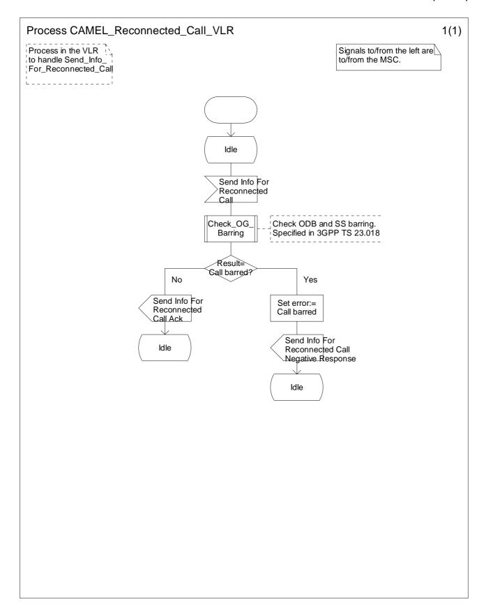
Figure 4.28a: Process CAMEL\_Reconnected\_Call\_VLR (sheet 1)
