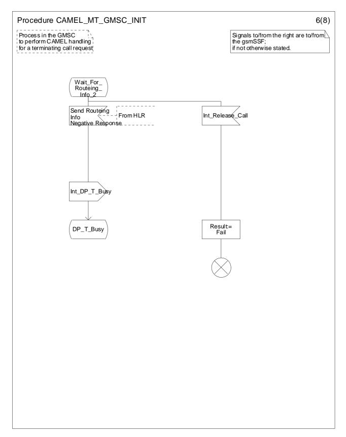
Figure 4.30f: Procedure CAMEL\_MT\_GMSC\_INIT (sheet 6)
