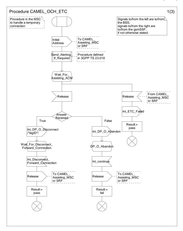
Figure 4.20a: Procedure CAMEL\_OCH\_ETC (sheet 1)
