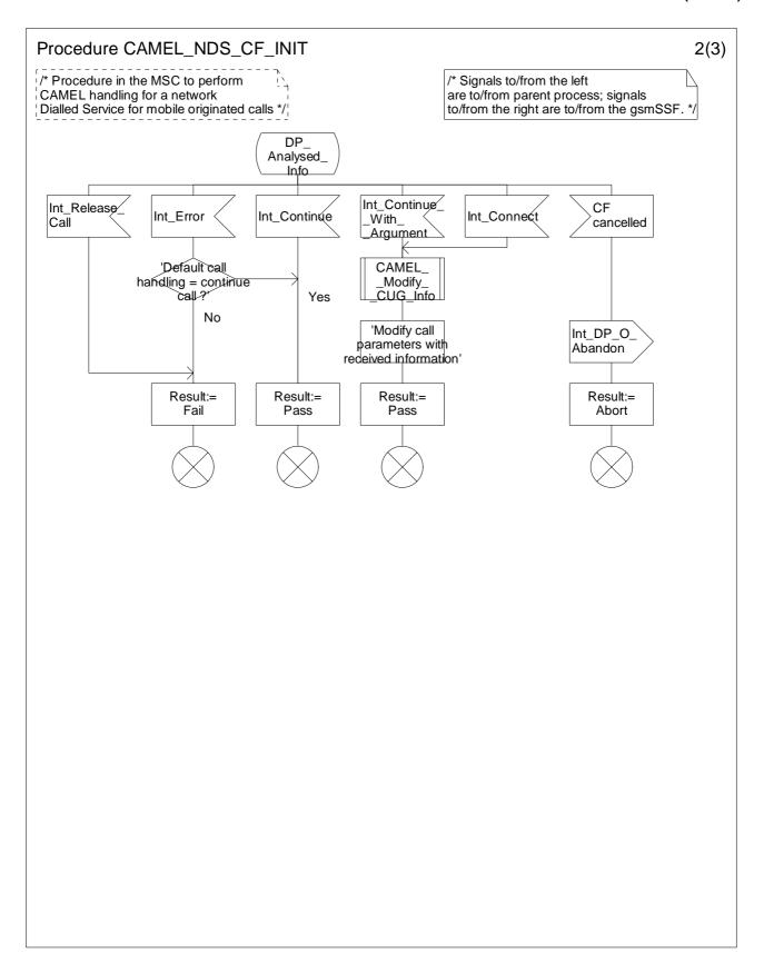
Figure 4.59b: Procedure CAMEL\_NDS\_CF\_INIT (sheet 2)
