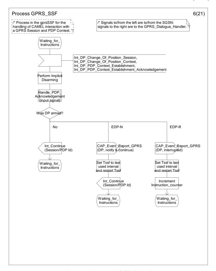
Figure 6.17f: Process GPRS\_SSF (sheet 6)
