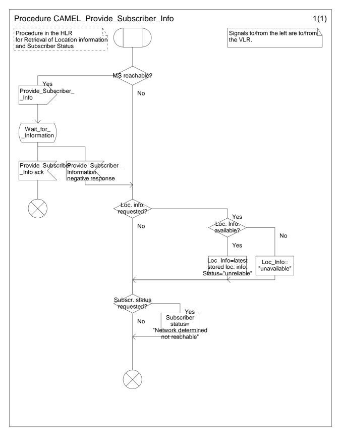
Figure 4.82a: Procedure CAMEL\_Provide\_Subscriber\_Info (sheet 1)
