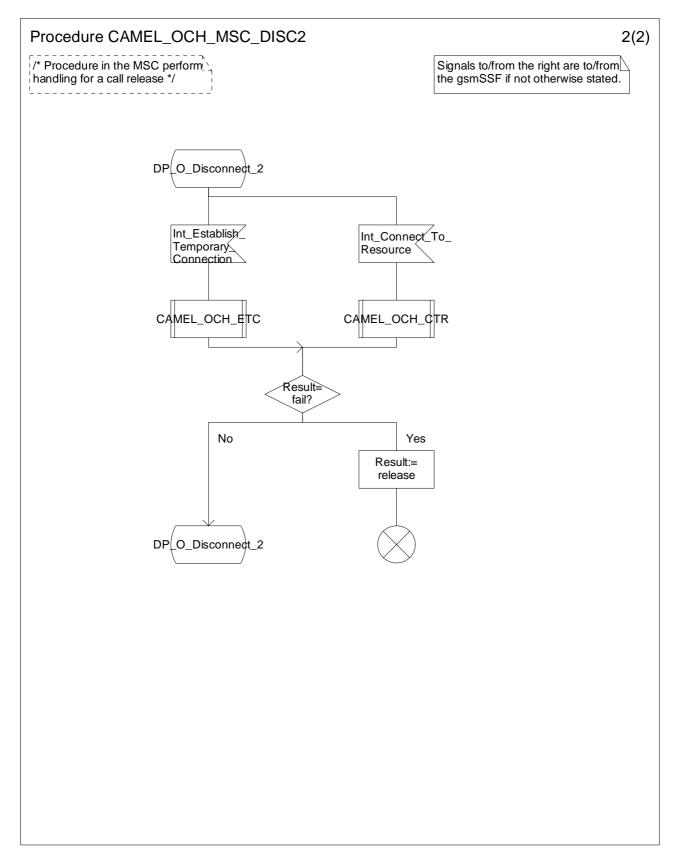
Figure 4.17b: Procedure CAMEL\_OCH\_MSC\_DISC2 (sheet 2)
