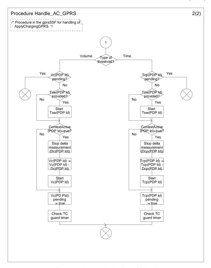
Figure 6.19b: Procedure Handle\_AC\_GPRS (sheet 2)
