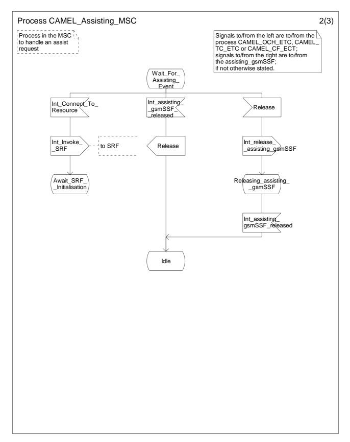
Figure 4.80b: Process CAMEL\_Assisting\_MSC (sheet 2)
