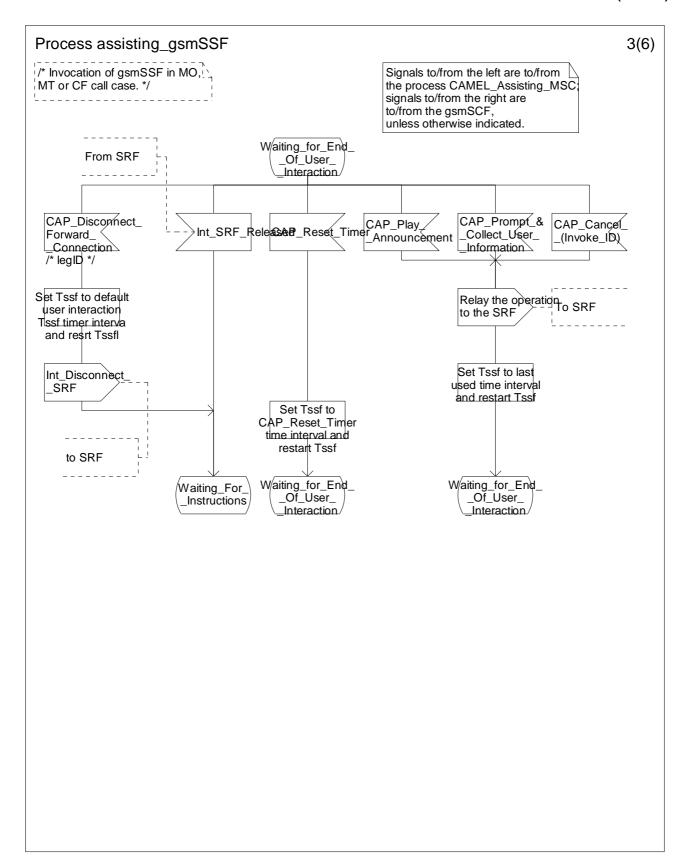
Figure 4.81c: Process Assisting\_gsmSSF (sheet 3)
