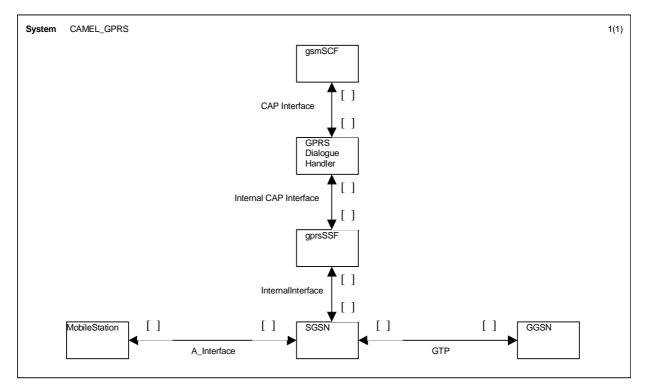
Figure 6.7: Architecture for CAMEL/GPRS interworking
