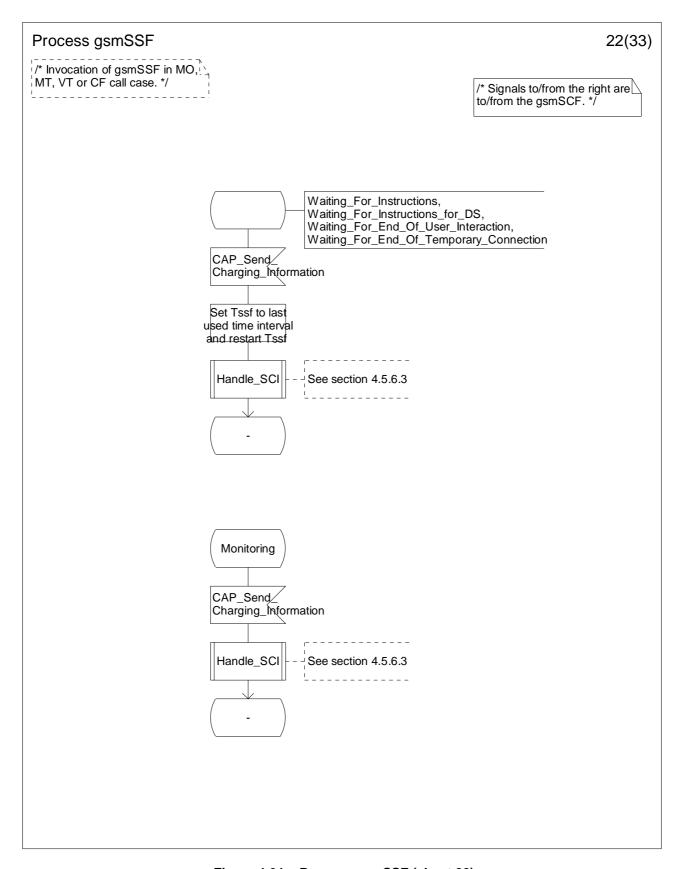
Figure 4.64v: Process gsmSSF (sheet 22)
