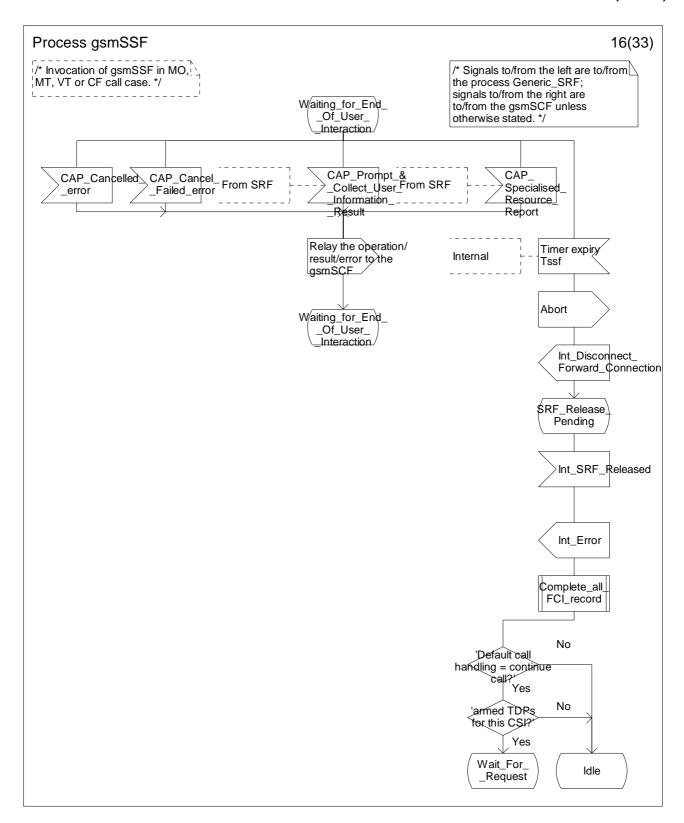
Figure 4.64p: Process gsmSSF (sheet 16)
