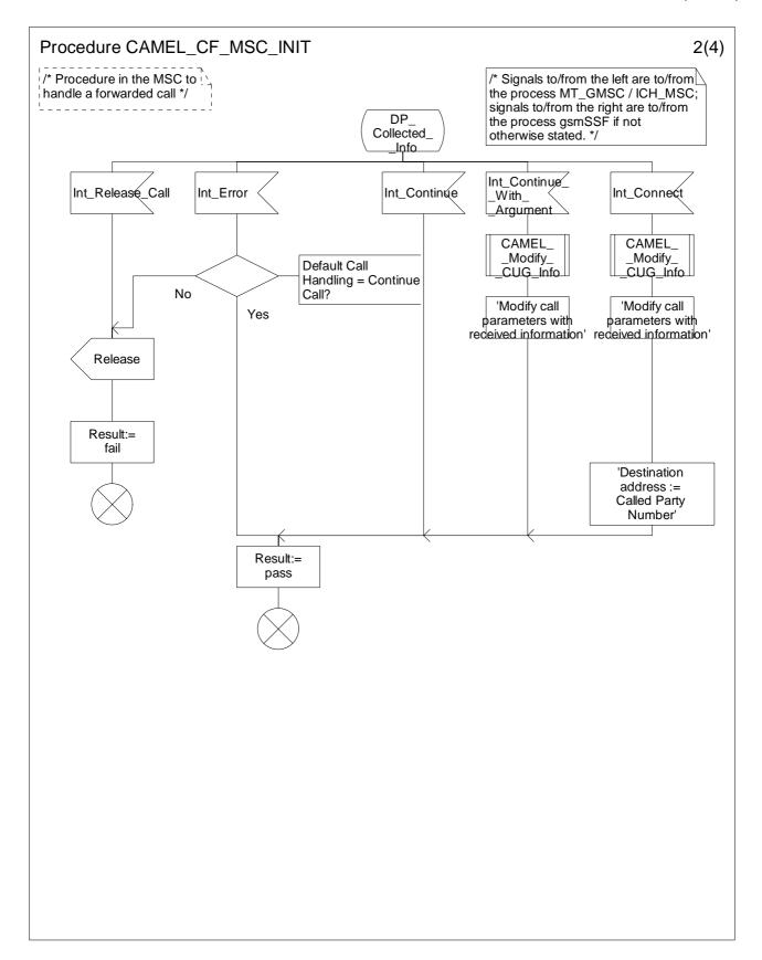
Figure 4.57b: Procedure CAMEL\_CF\_MSC\_INIT (sheet 2)
