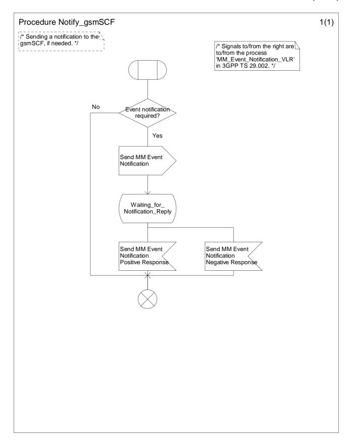
Figure 9.4: Procedure Notify\_gsmSCF (sheet 1)
