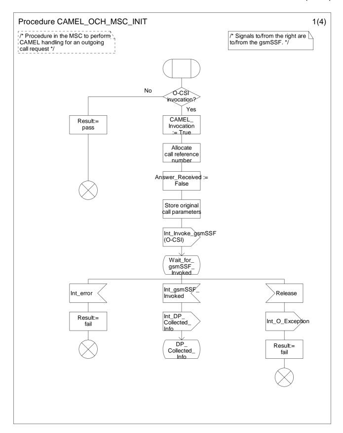
Figure 4.10a: Procedure CAMEL\_OCH\_MSC\_INIT (sheet 1)
