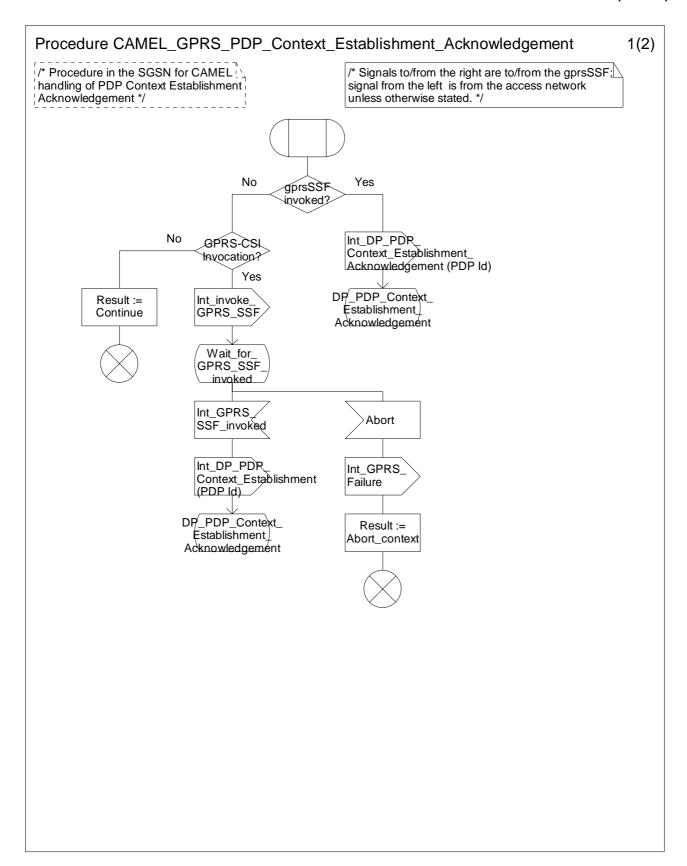
Figure 6.13a: Procedure CAMEL\_GPRS\_PDP\_Context\_Establishment\_Acknowledgement (sheet 1)
