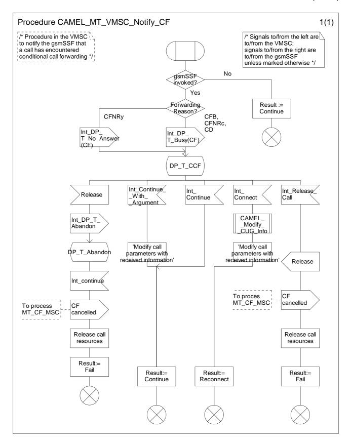
Figure 4.53a: Procedure CAMEL\_MT\_VMSC\_Notify\_CF (sheet 1)
