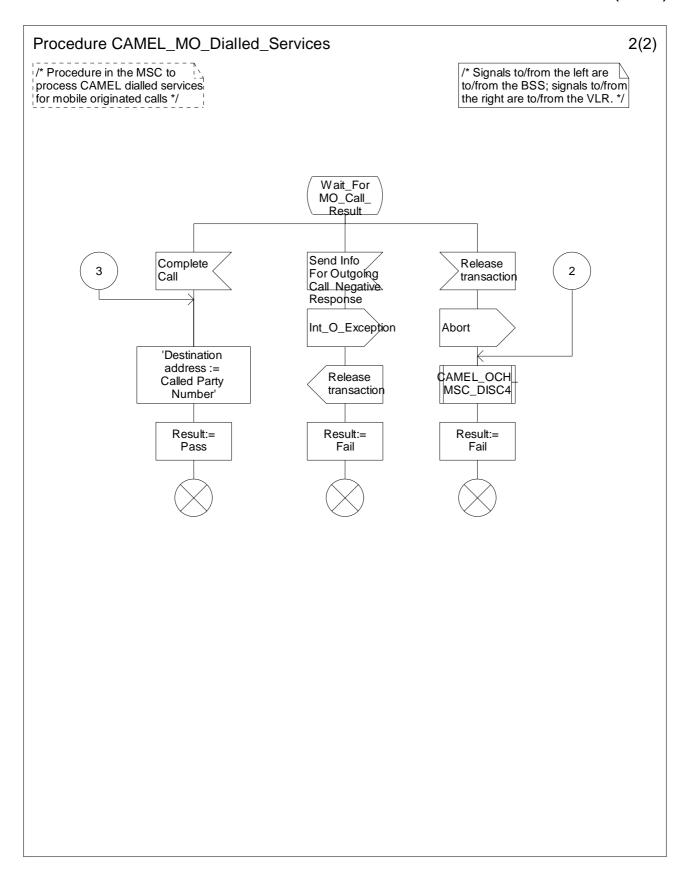
Figure 4.9b: Procedure CAMEL\_MO\_Dialled\_Services (sheet 2)
