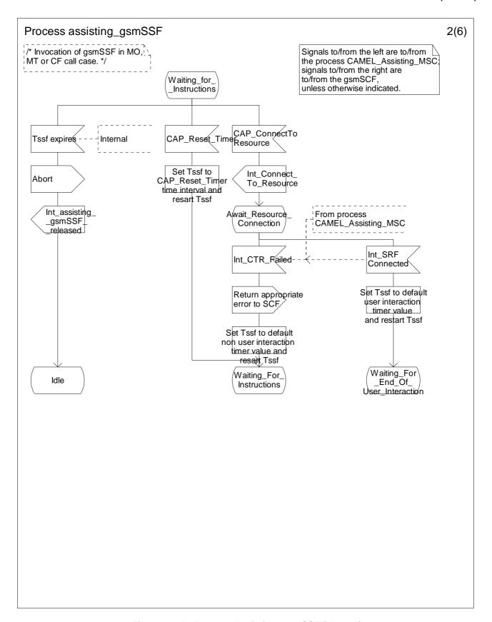
Figure 4.81b: Process Assisting\_gsmSSF (sheet 2)
