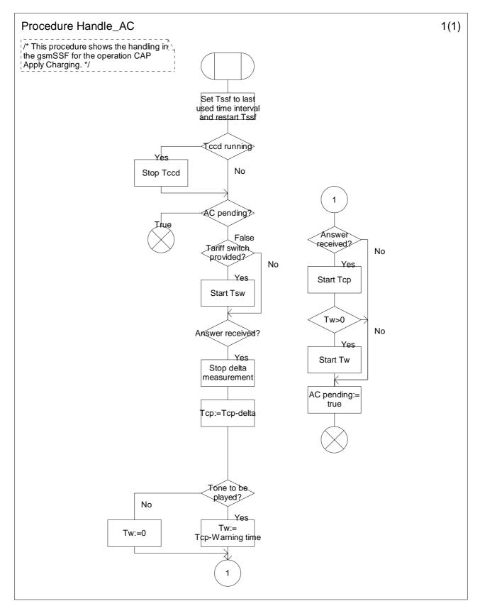
Figure 4.69a: Procedure Handle\_AC (sheet 1)
