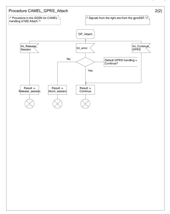
Figure 6.8b: Procedure CAMEL\_GPRS\_Attach (sheet 2)
