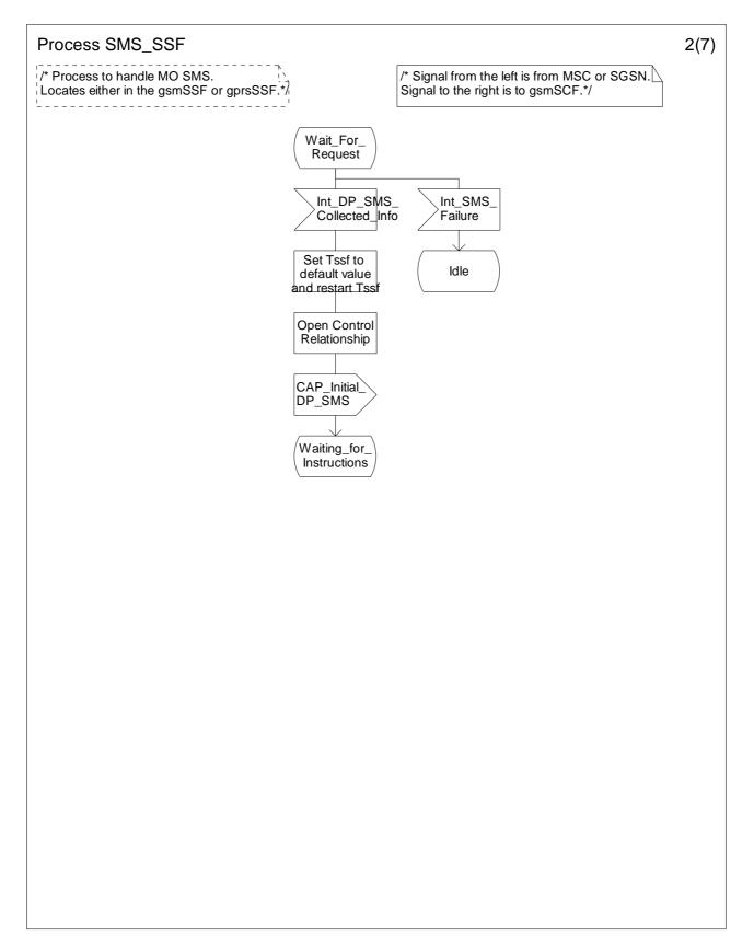
Figure 7.10b: Process SMS\_SSF (sheet 2)
