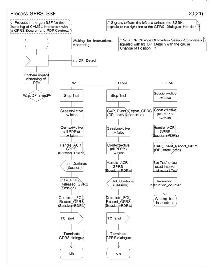
Figure 6.17t: Process GPRS\_SSF (sheet 20)
