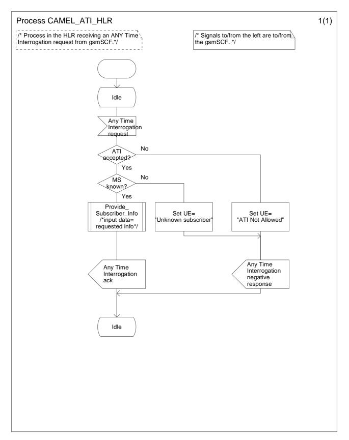
Figure 11.3: Process CAMEL\_ATI\_HLR (sheet 1)
