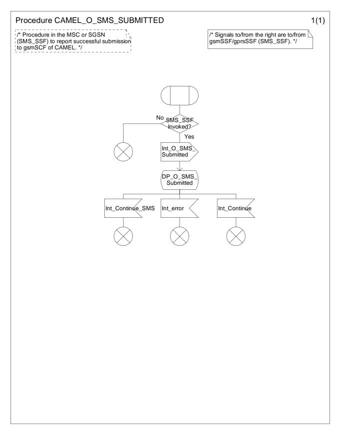
Figure 7.8: Procedure CAMEL\_O\_SMS\_SUBMITTED (sheet 1)
