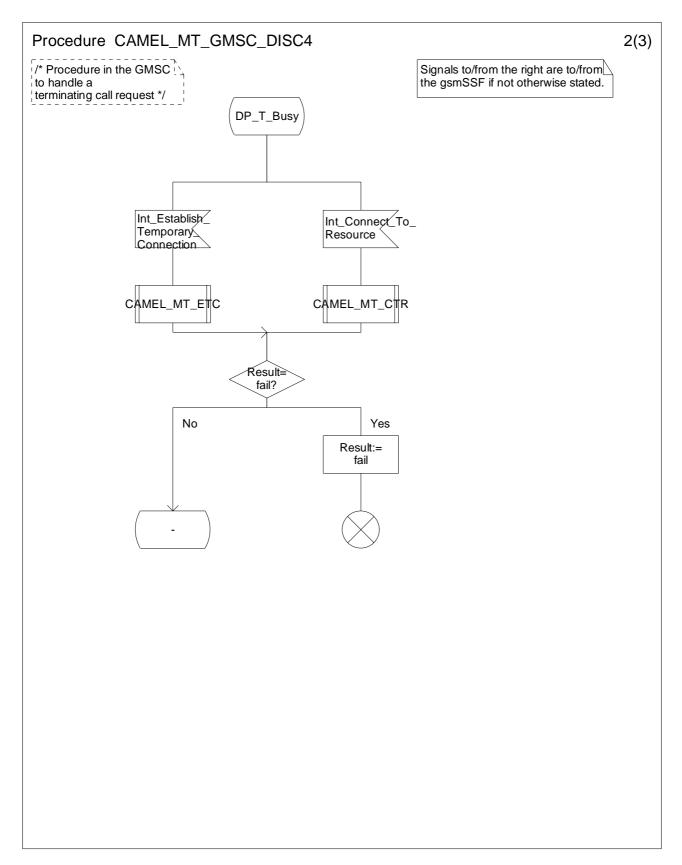
Figure 4.35b: Procedure CAMEL\_MT\_GMSC\_DISC4 (sheet 2)
