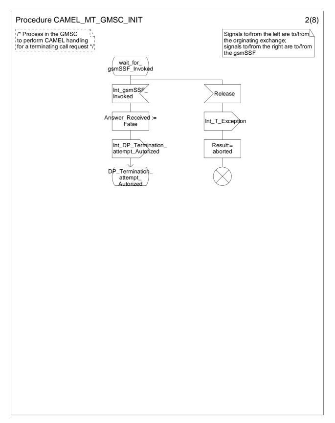
Figure 4.30b: Procedure CAMEL\_MT\_GMSC\_INIT (sheet 2)
