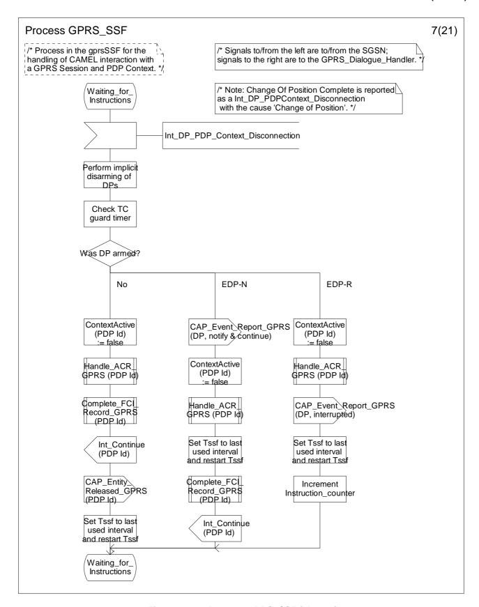
Figure 6.17g: Process GPRS\_SSF (sheet 7)
