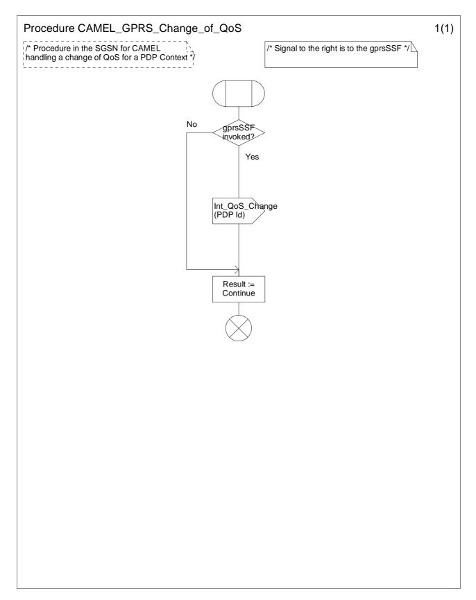
Figure 6.14: Procedure CAMEL\_GPRS\_Change\_Of\_QoS (sheet 1)
