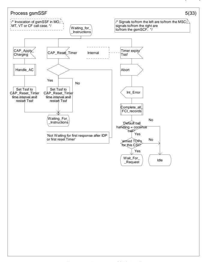
Figure 4.64e: Process gsmSSF (sheet 5)
