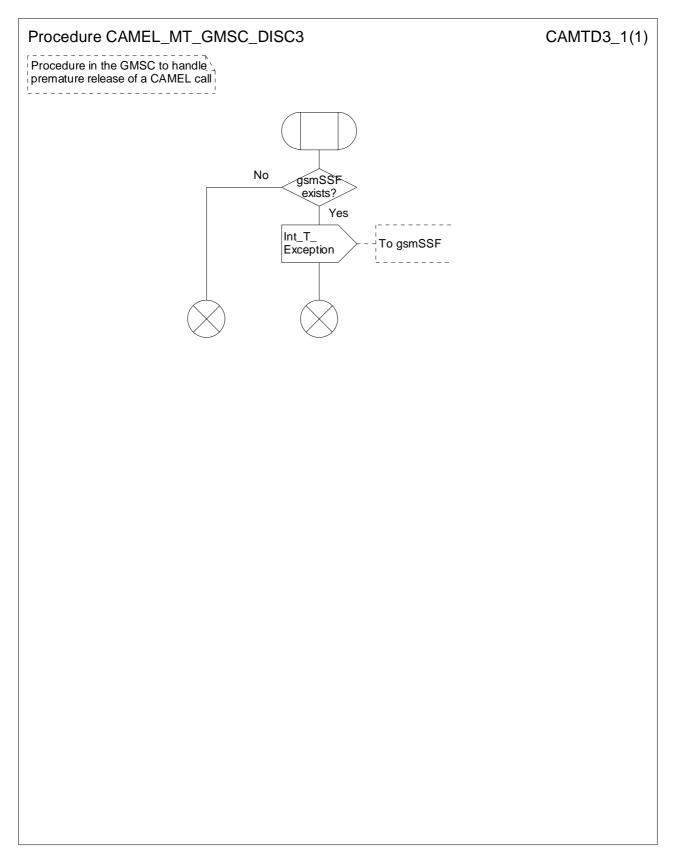
Figure 4.34a: Procedure CAMEL\_MT\_GMSC\_DISC3 (sheet 1)
