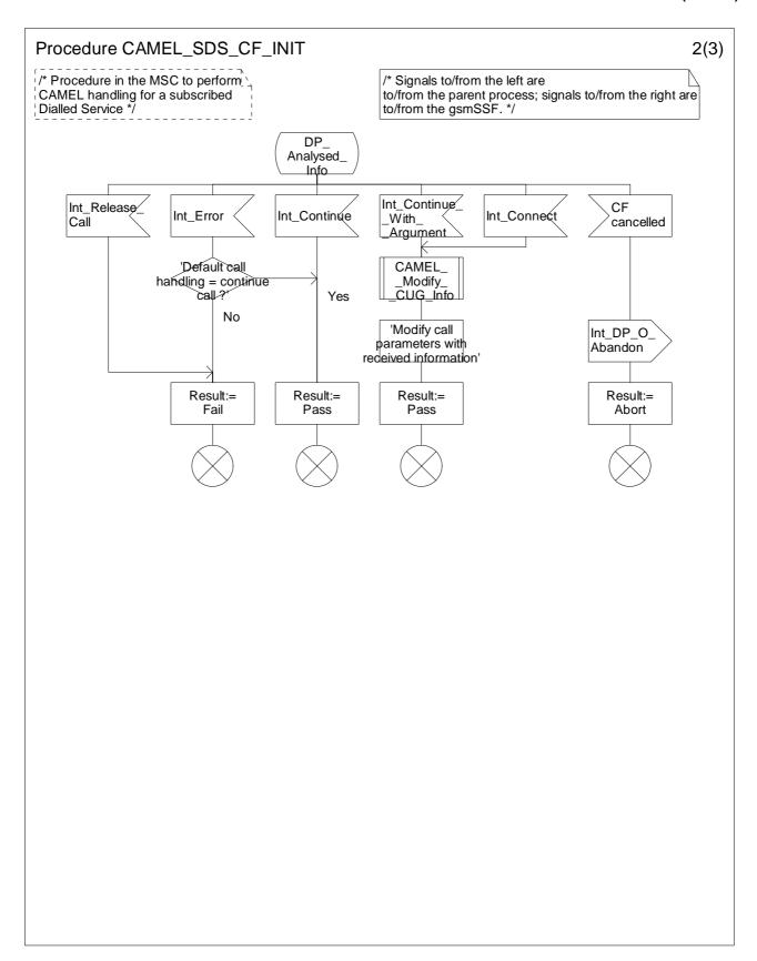
Figure 4.58b: Procedure CAMEL\_SDS\_CF\_INIT (sheet 2)
