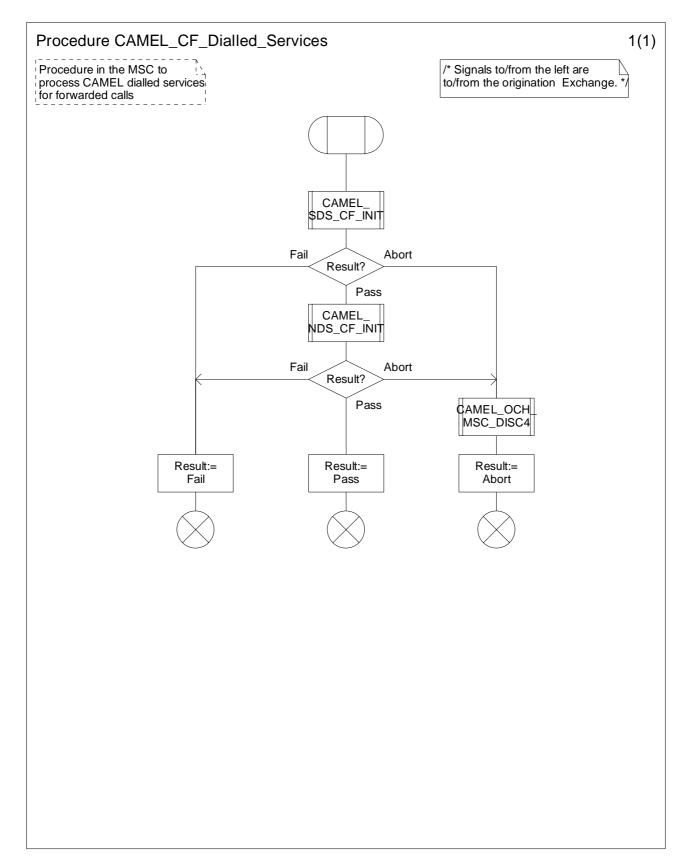
Figure 4.56a: Procedure CAMEL\_CF\_Dialled\_Services (sheet 1)
