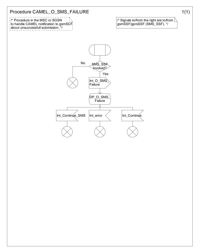
Figure 7.9: Procedure CAMEL\_O\_SMS\_FAILURE (sheet 1)
