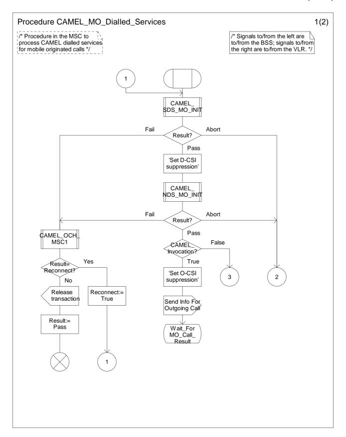
Figure 4.9a: Procedure CAMEL\_MO\_Dialled\_Services (sheet 1)
