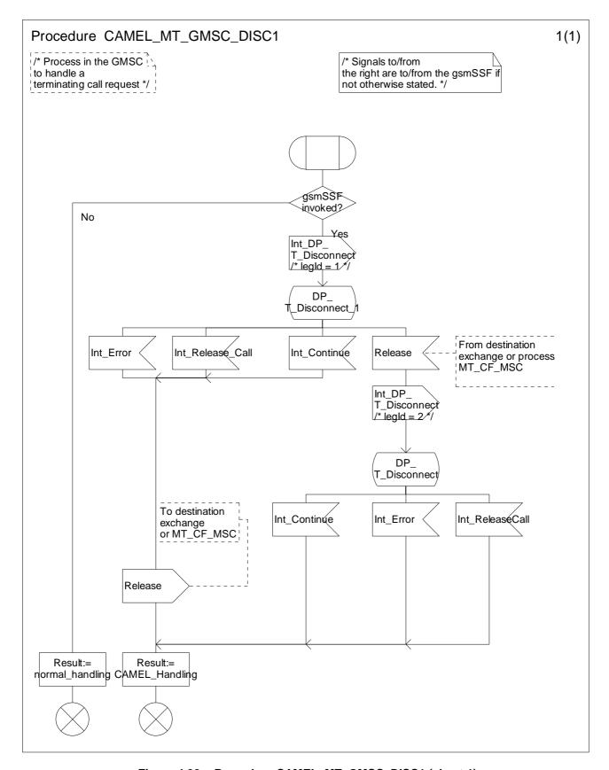
Figure 4.32a: Procedure CAMEL\_MT\_GMSC\_DISC1 (sheet 1)
