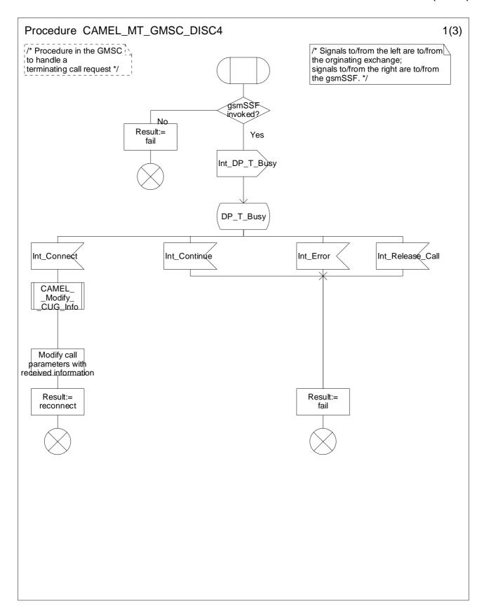
Figure 4.35a: Procedure CAMEL\_MT\_GMSC\_DISC4 (sheet 1)
