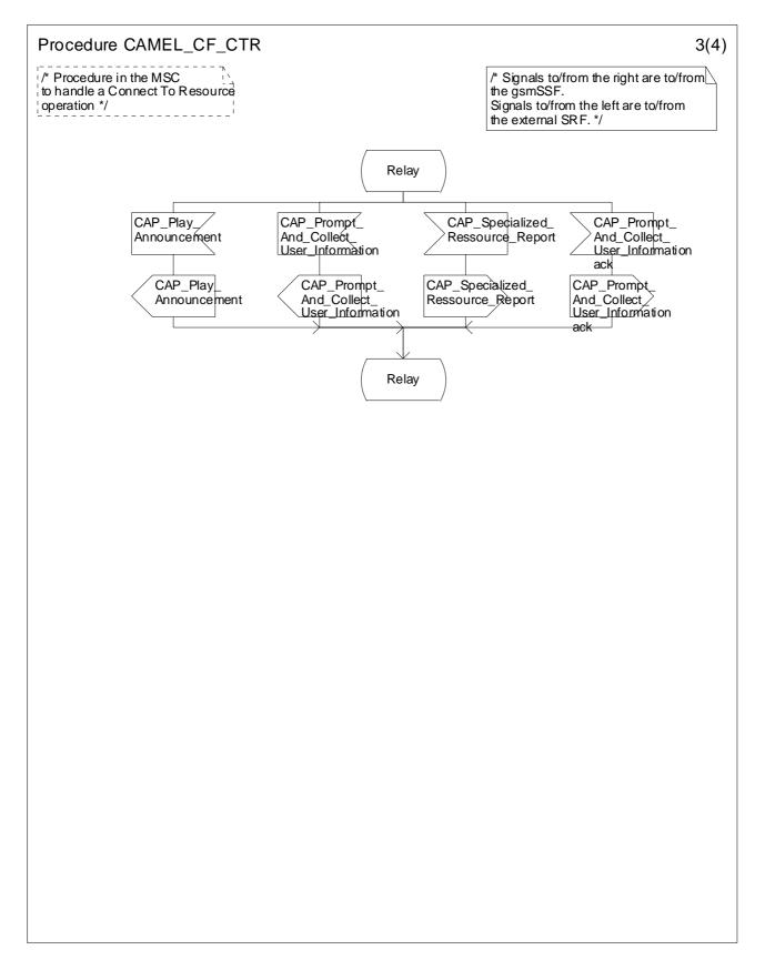
Figure 4.62c: Procedure CAMEL\_CF\_CTR (sheet 3)
