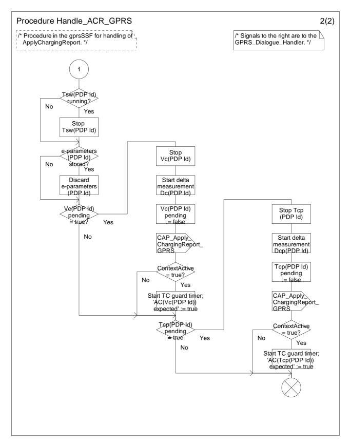
Figure 6.20b: Procedure Handle\_ACR\_GPRS (sheet 2)
