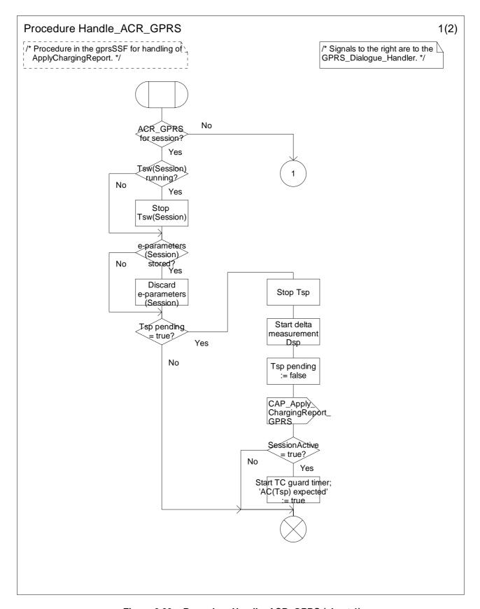
Figure 6.20a: Procedure Handle\_ACR\_GPRS (sheet 1)
