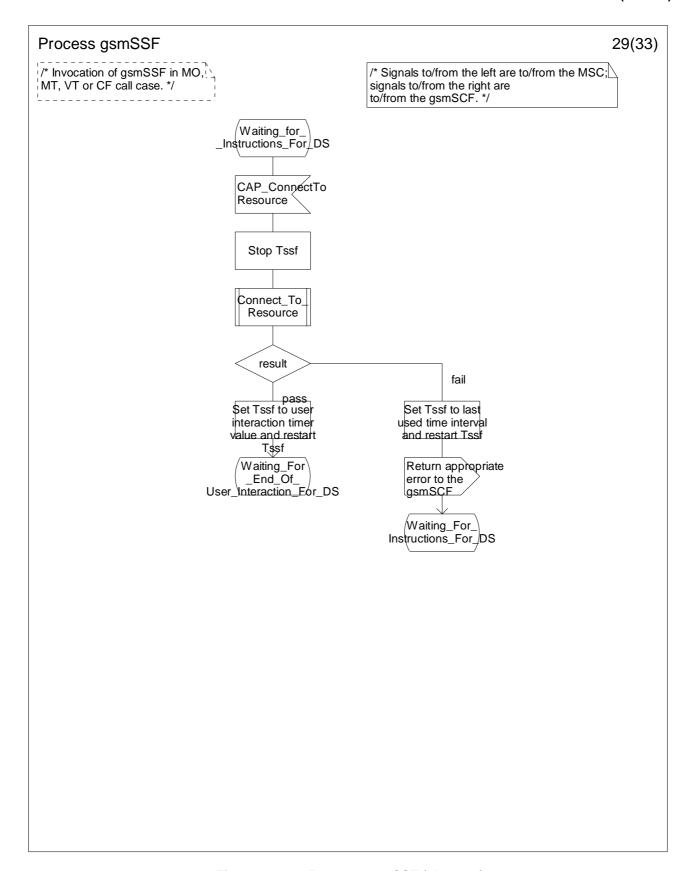
Figure 4.64cc: Process gsmSSF (sheet 29)
