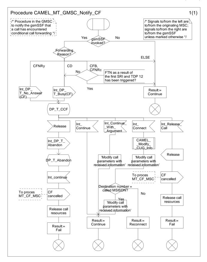
Figure 4.40a: Procedure CAMEL\_MT\_GMSC\_Notify\_CF (sheet 1)
