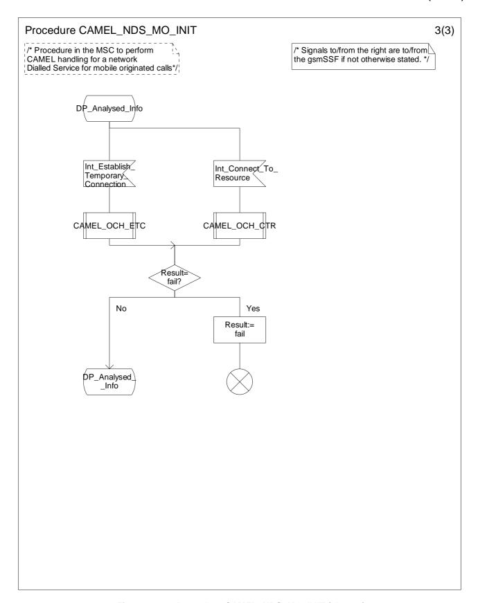
Figure 4.12c: Procedure CAMEL\_NDS\_MO\_INIT (sheet 3)
