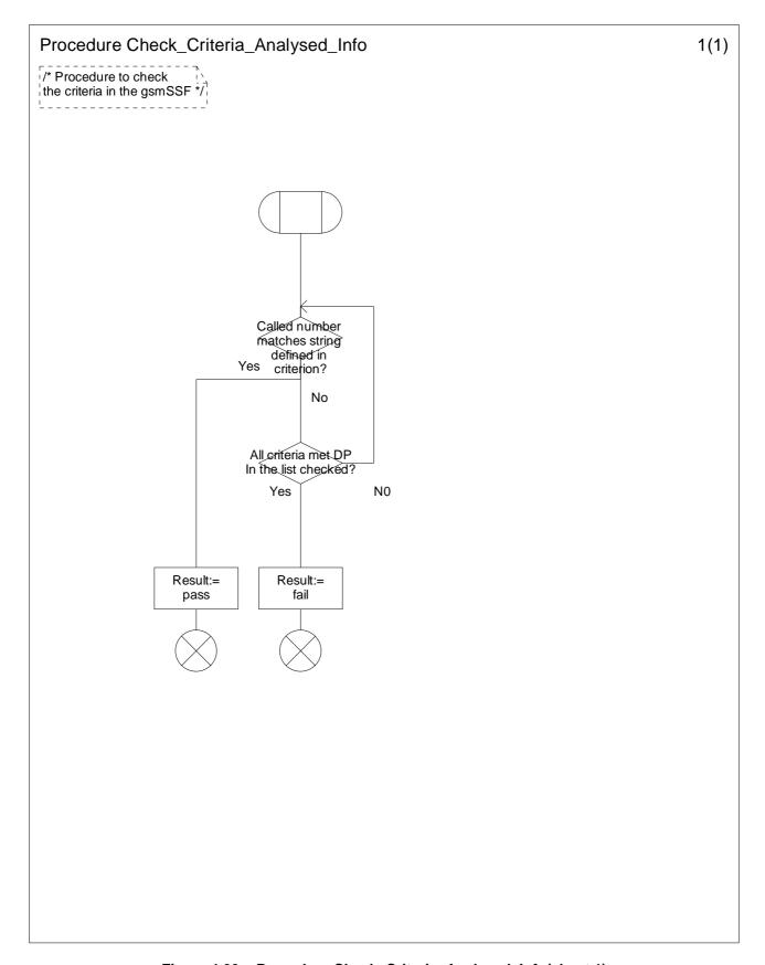
Figure 4.66a: Procedure Check\_Criteria\_Analysed\_Info(sheet 1)
