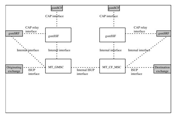
Figure 4.8c: Terminating GMSC case (gsmSSF relay)
