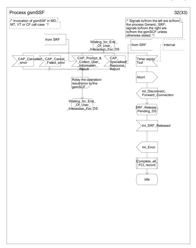
Figure 4.64ff: Process gsmSSF (sheet 32)
