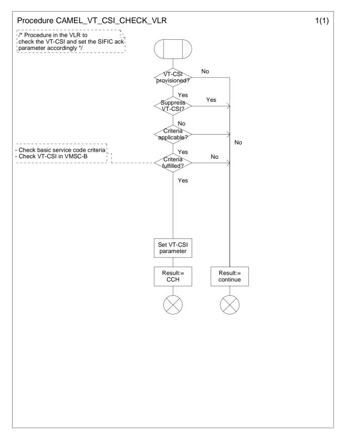
Figure 4.51: Procedure CAMEL\_VT\_CSI\_Check\_VLR (sheet 1)
