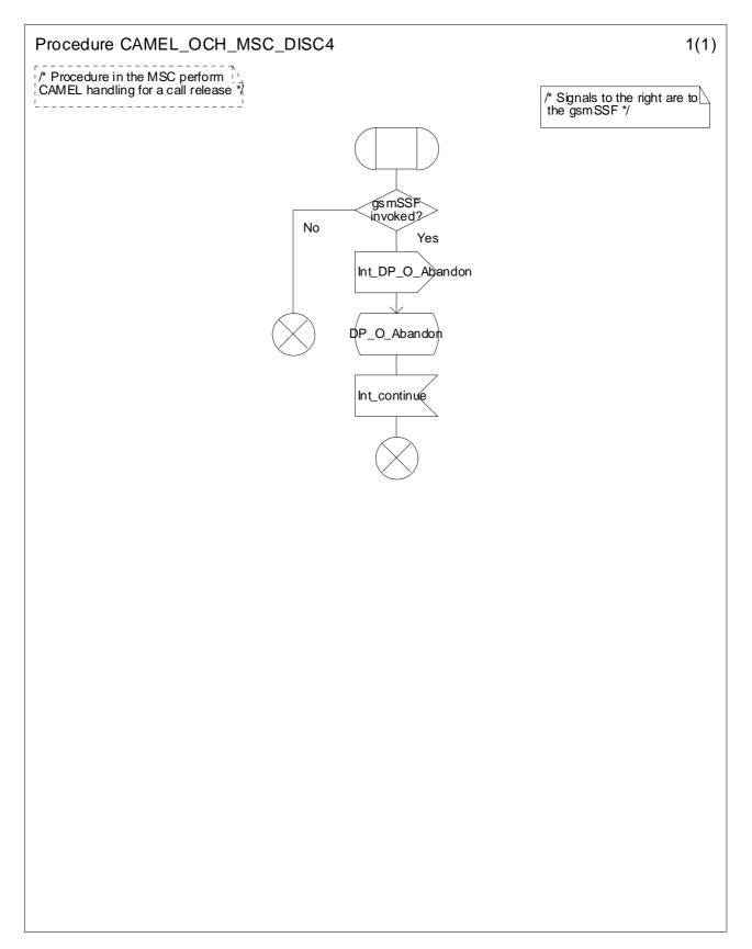
Figure 4.19a: Procedure CAMEL\_OCH\_MSC\_DISC4 (sheet 1)
