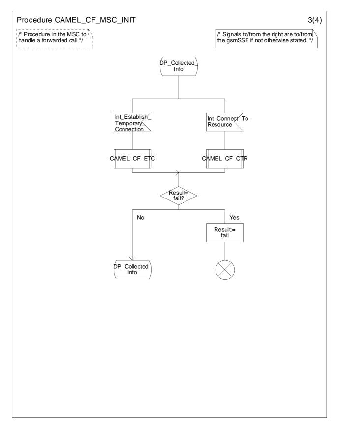
Figure 4.57c: Procedure CAMEL\_CF\_MSC\_INIT (sheet 3)
