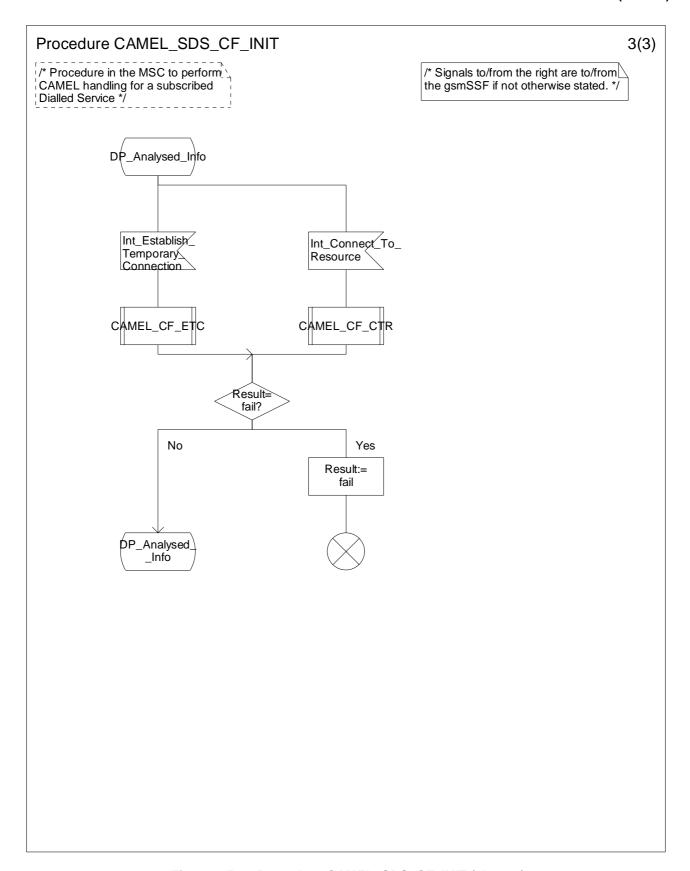
Figure 4.58c: Procedure CAMEL\_SDS\_CF\_INIT (sheet 3)
