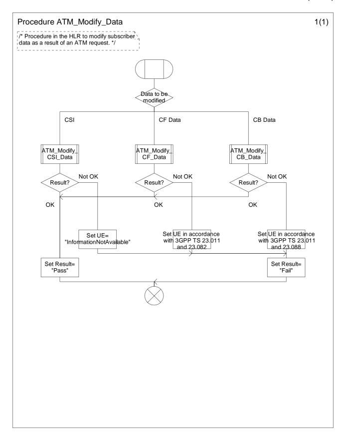
Figure 10.4: Procedure ATM\_Modify\_Data (sheet 1)
