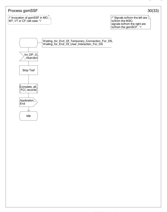
Figure 4.64dd: Process gsmSSF (sheet 30)
