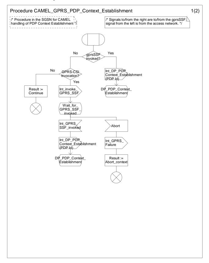
Figure 6.12a: Procedure CAMEL\_GPRS\_PDP\_Context\_Establishment (sheet 1)
