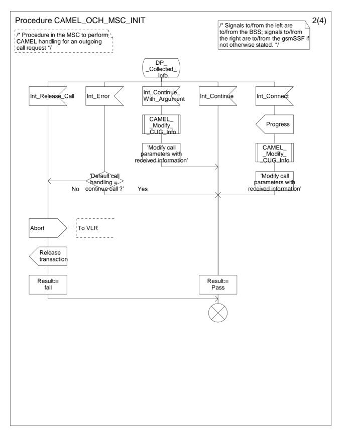
Figure 4.10b: Procedure CAMEL\_OCH\_MSC\_INIT (sheet 2)
