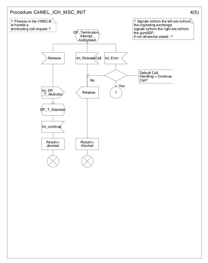
Figure 4.52d: Procedure CAMEL\_ICH\_MSC\_INIT (sheet 4)
