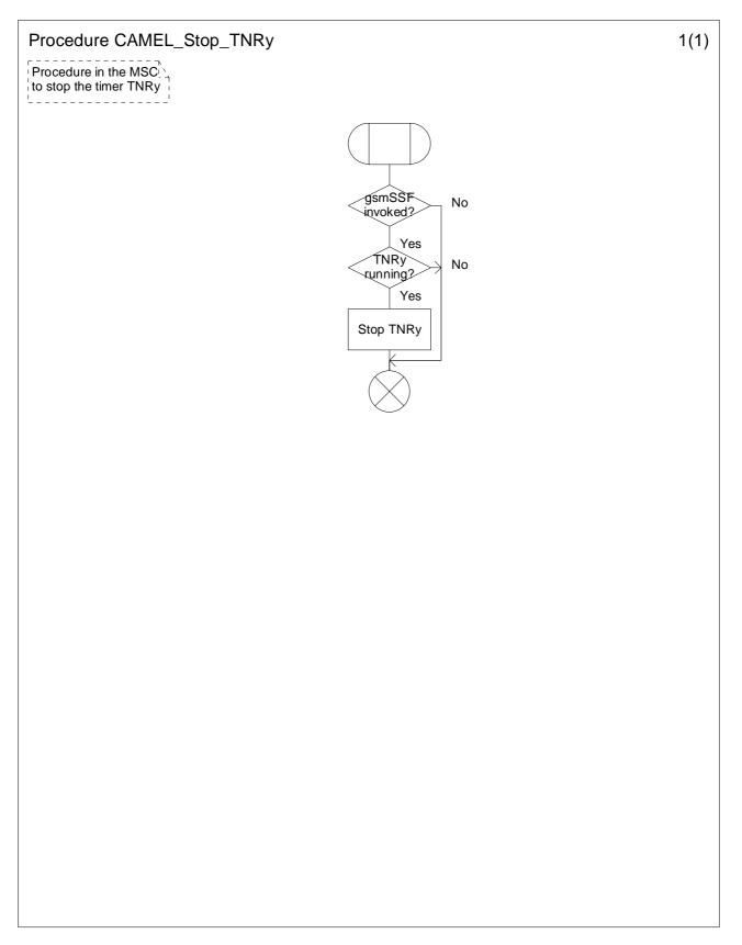
Figure 4.23: Procedure CAMEL\_Stop\_TNRy (sheet 1)
