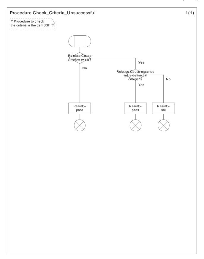
Figure 4.67a: Procedure Check\_Criteria\_Unsuccessful(sheet 1)
