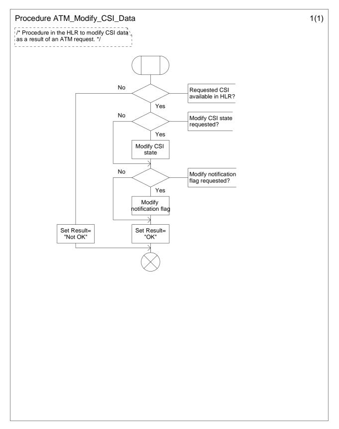
Figure 10.5: Procedure ATM\_Modify\_CSI\_Data (sheet 1)
