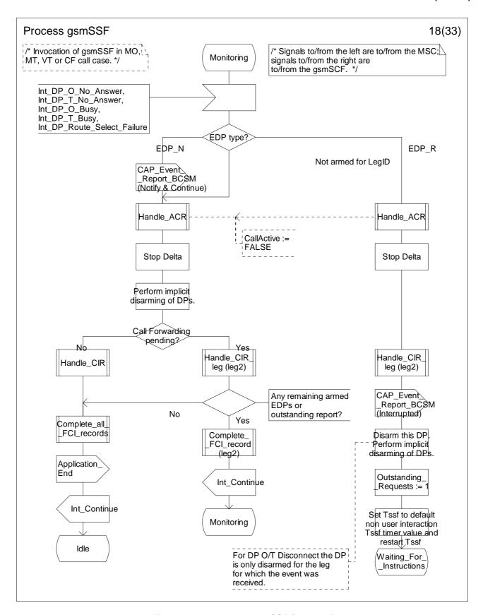
Figure 4.64r: Process gsmSSF (sheet 18)
