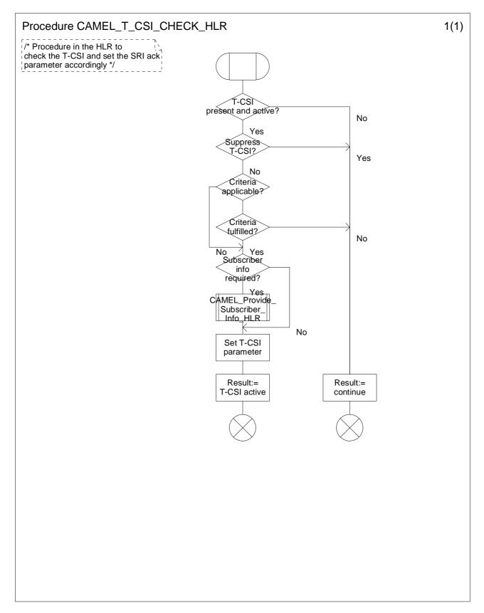
Figure 4.45: Procedure CAMEL\_T\_CSI\_CHECK\_HLR (sheet 1)
