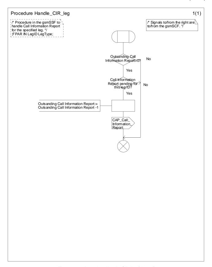
Figure 4.72a: Procedure Handle\_CIR\_leg (sheet 1)
