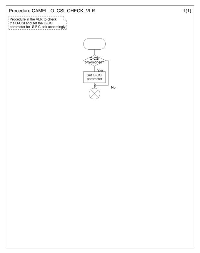
Figure 4.49: Procedure CAMEL\_O\_CSI\_Check\_VLR (sheet 1)
