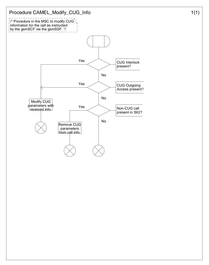
Figure 4.25: Procedure CAMEL\_Modify\_CUG\_Info (sheet 1)
