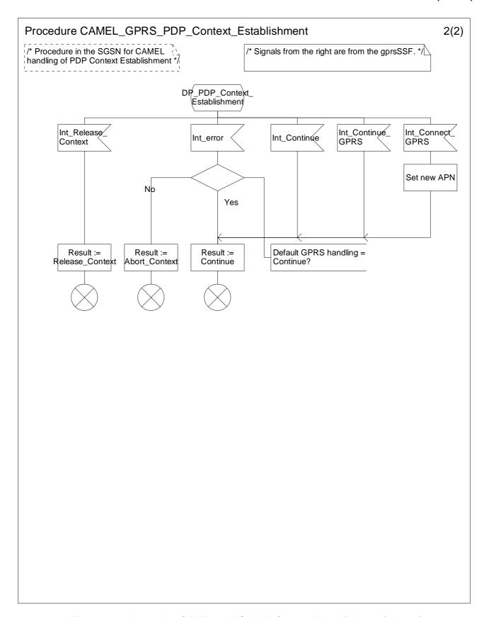
Figure 6.12b: Procedure CAMEL\_GPRS\_PDP\_Context\_Establishment (sheet 2)
