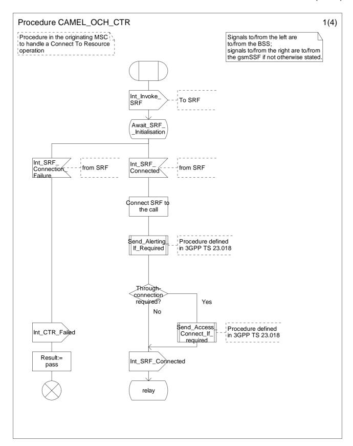
Figure 4.21a: Procedure CAMEL\_OCH\_CTR (sheet 1)
