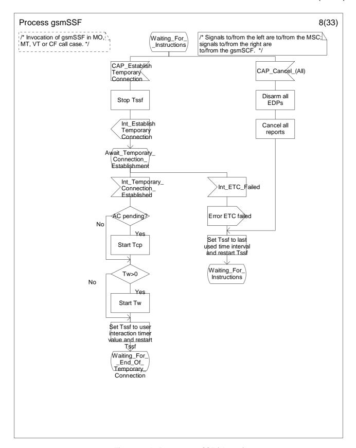
Figure 4.64h: Process gsmSSF (sheet 8)
