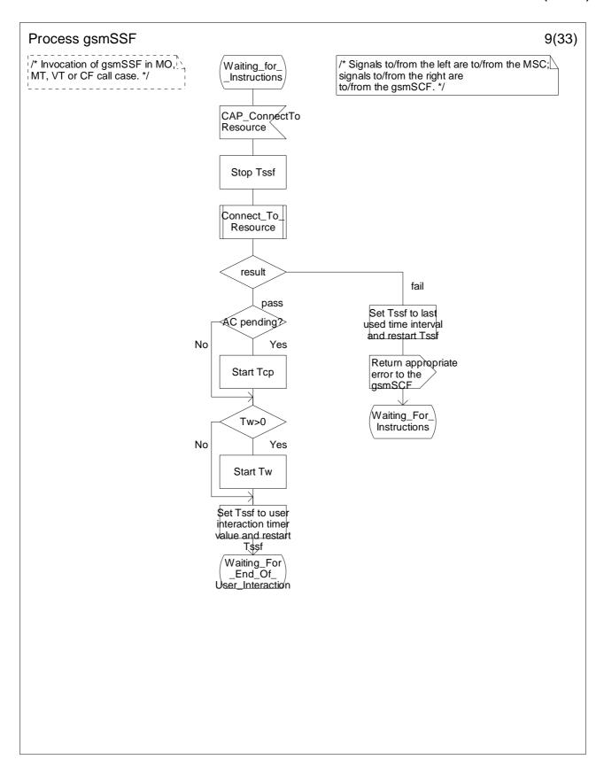
Figure 4.64i: Process gsmSSF (sheet 9)
