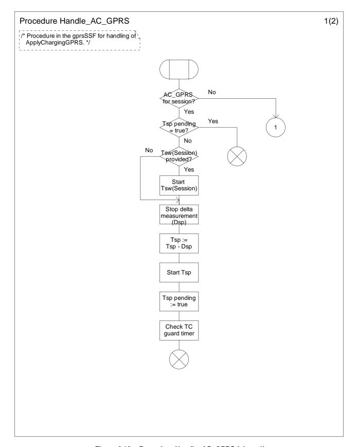
Figure 6.19a: Procedure Handle\_AC\_GPRS (sheet 1)
