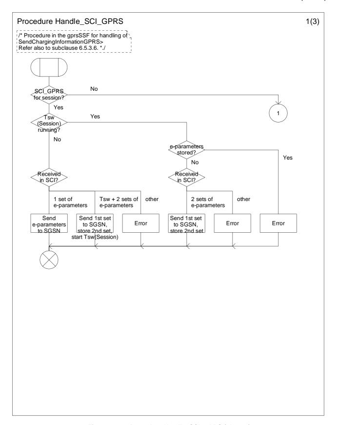
Figure 6.23a: Procedure Handle\_SCI\_GPRS (sheet 1)
