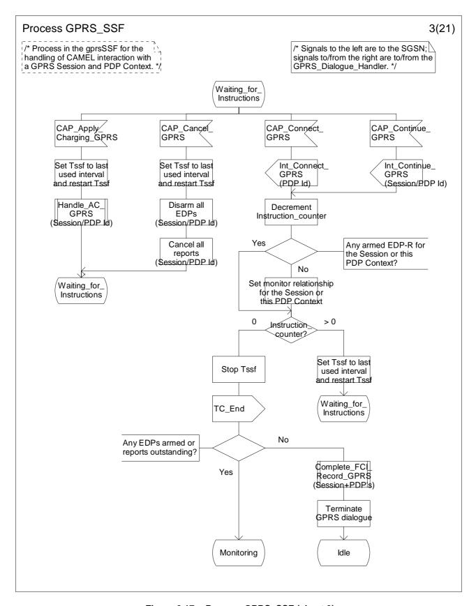
Figure 6.17c: Process GPRS\_SSF (sheet 3)
