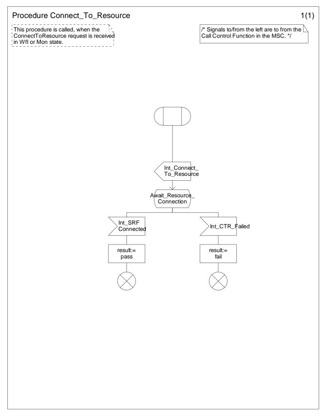
Figure 4.68a: Procedure Connect\_To\_Resource (sheet 1)
