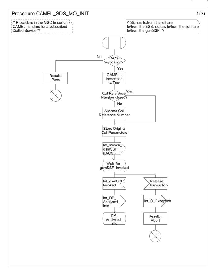
Figure 4.11a: Procedure CAMEL\_SDS\_MO\_Init (sheet 1)
