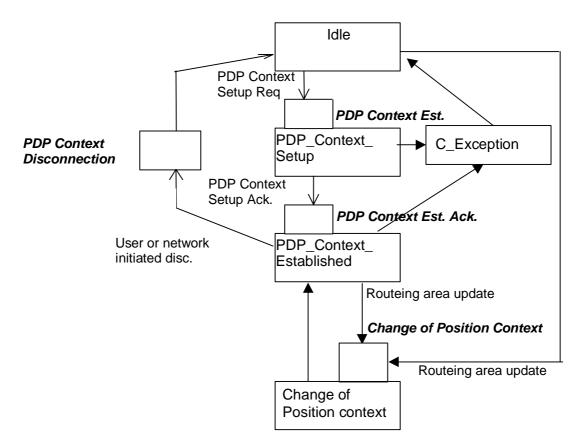
Figure 6.4: GPRS PDP Context State Model
