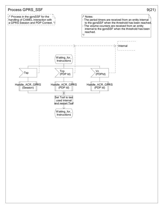
Figure 6.17i: Process GPRS\_SSF (sheet 9)
