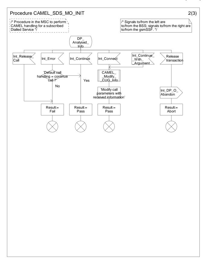
Figure 4.11b: Procedure CAMEL\_SDS\_MO\_INIT (sheet 2)
