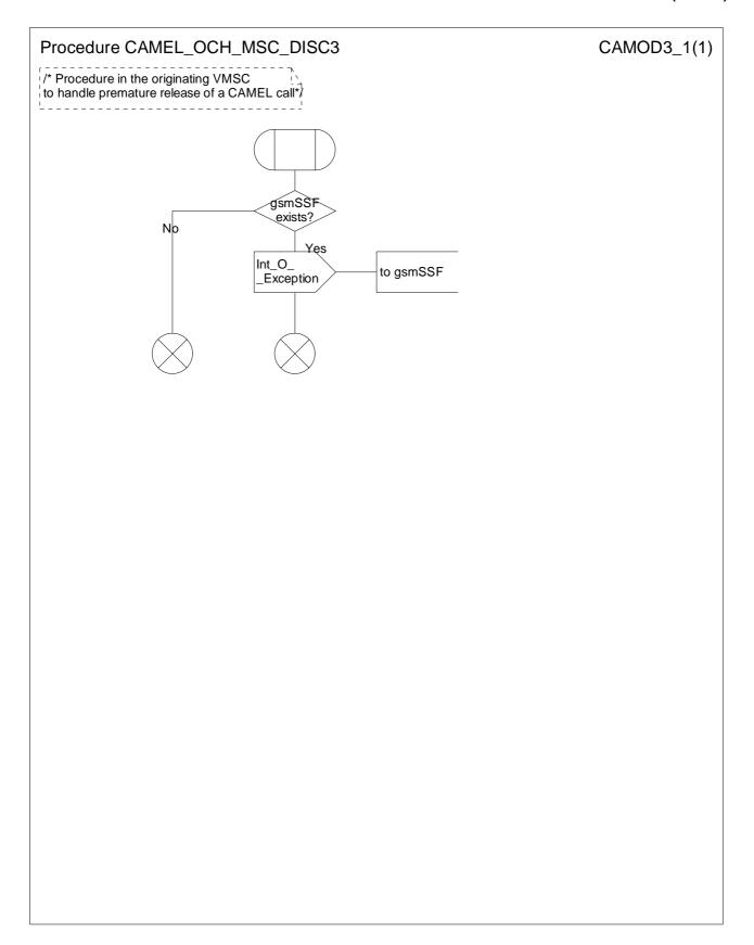
Figure 4.18a: Procedure CAMEL\_OCH\_MSC\_DISC3 (sheet 1)
