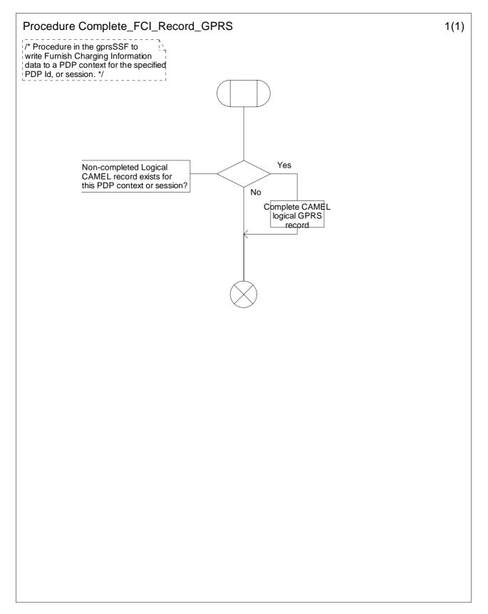
Figure 6.22a: Procedure Complete\_FCI\_Record\_GPRS (sheet 1)
