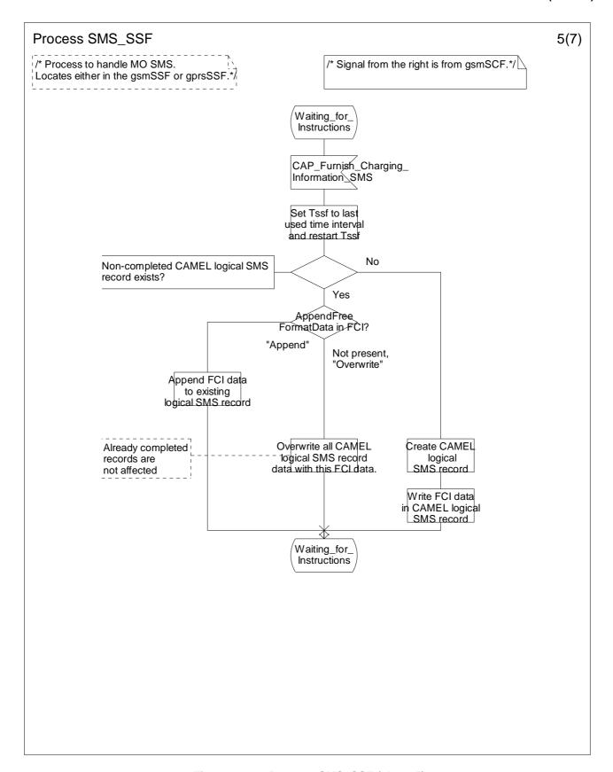
Figure 7.10e: Process SMS\_SSF (sheet 5)
