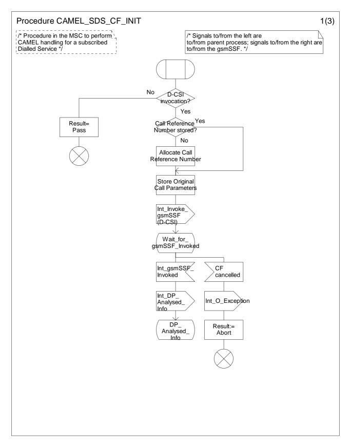
Figure 4.58a: Procedure CAMEL\_SDS\_CF\_INIT (sheet 1)
