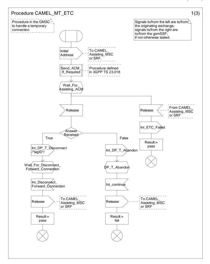
Figure 4.38a: Procedure CAMEL\_MT\_ETC (sheet 1)
