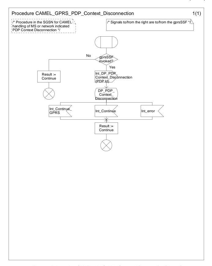
Figure 6.15: Procedure CAMEL\_GPRS\_PDP\_Context\_Disconnection (sheet 1)
