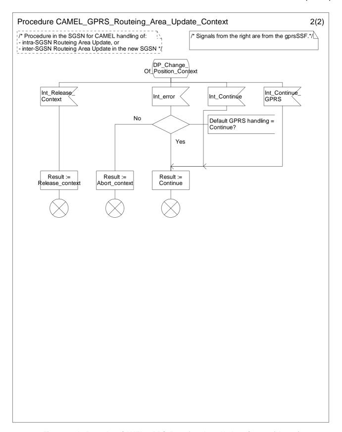
Figure 6.11b: Procedure CAMEL\_GPRS\_Routeing\_Area\_Update\_Context (sheet 2)
