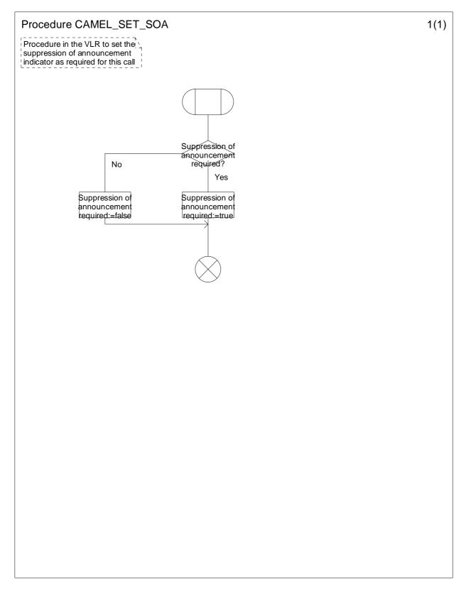
Figure 4.47: Procedure CAMEL\_SET\_SOA (sheet 1)
