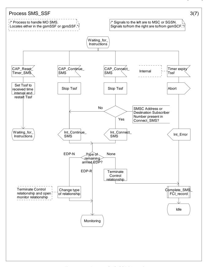
Figure 7.10c: Process SMS\_SSF (sheet 3)
