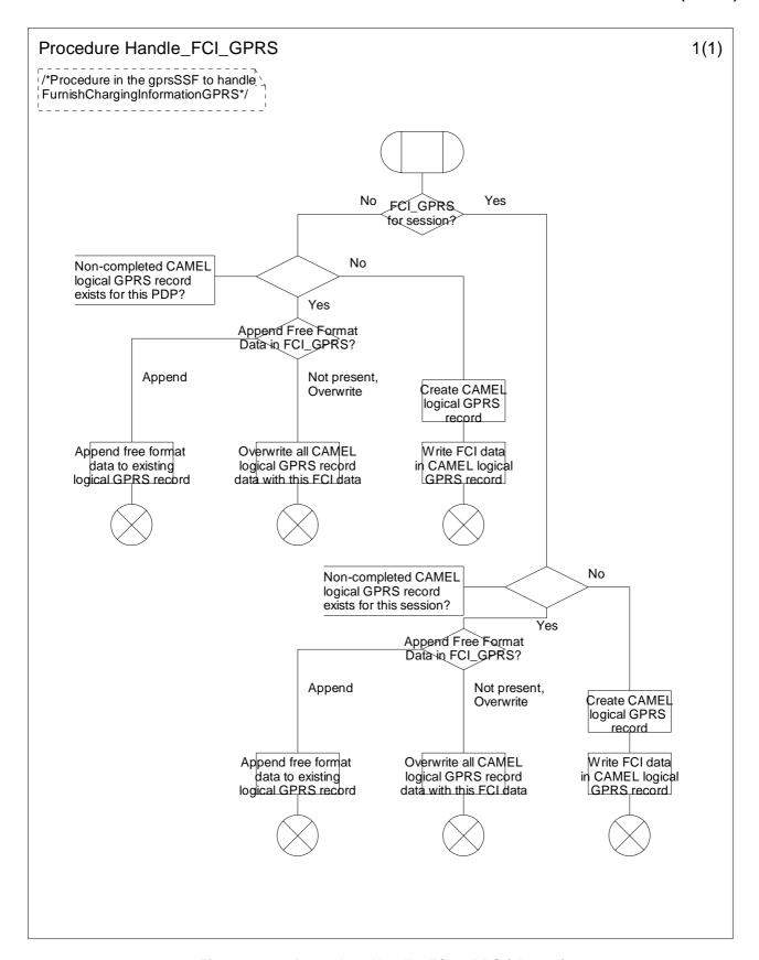
Figure 6.21a: Procedure Handle\_FCI\_GPRS (sheet 1)
