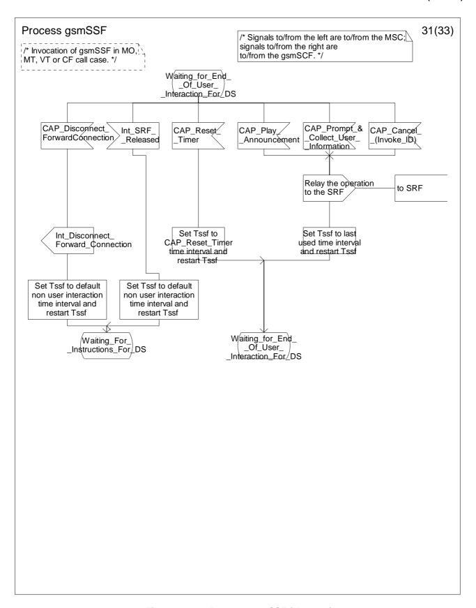
Figure 4.64ee: Process gsmSSF (sheet 31)
