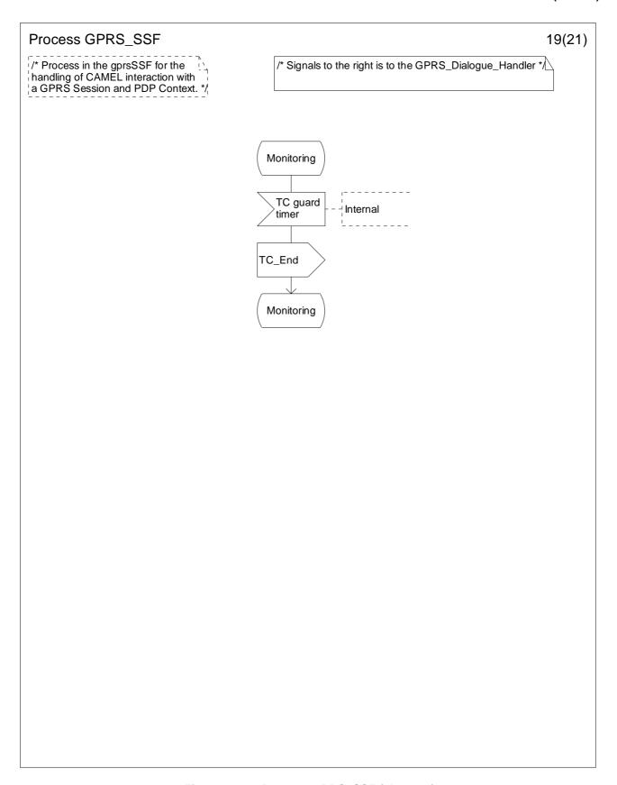
Figure 6.17s: Process GPRS\_SSF (sheet 19)
