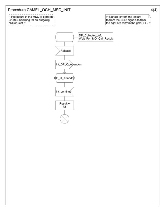
Figure 4.10d: Procedure CAMEL\_OCH\_MSC\_INIT (sheet 4)
