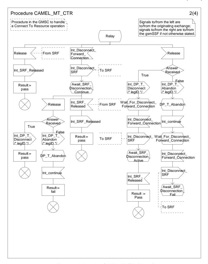
Figure 4.39b: Procedure CAMEL\_MT\_CTR (sheet 2)
