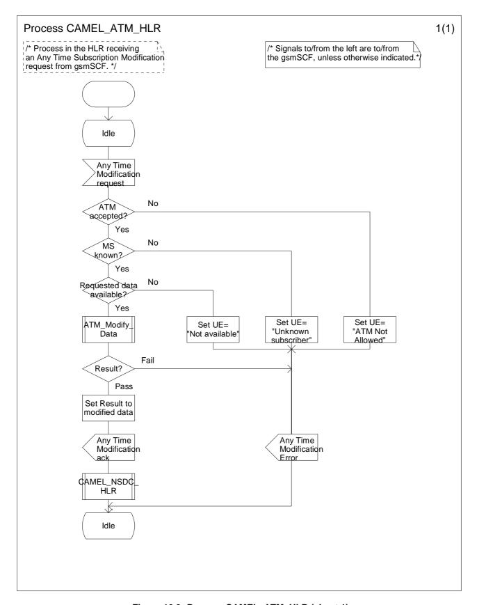
Figure 10.3: Process CAMEL\_ATM\_HLR (sheet 1)
