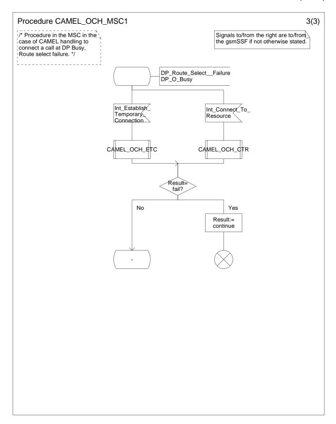
Figure 4.14c: Procedure CAMEL\_OCH\_MSC1 (sheet 3)
