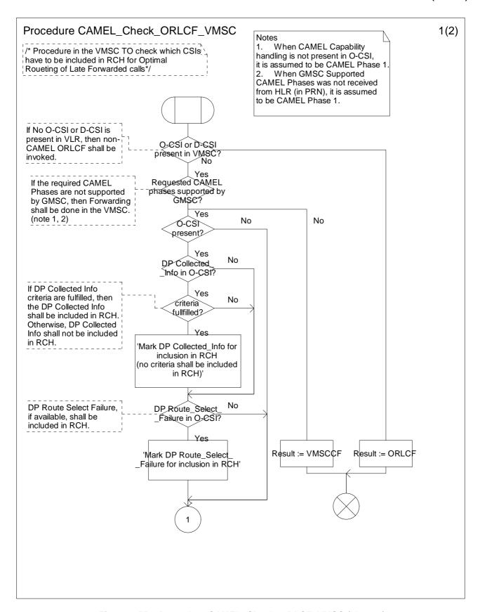
Figure 4.55a: Procedure CAMEL\_Check\_ORLCF\_VMSC (sheet 1)
