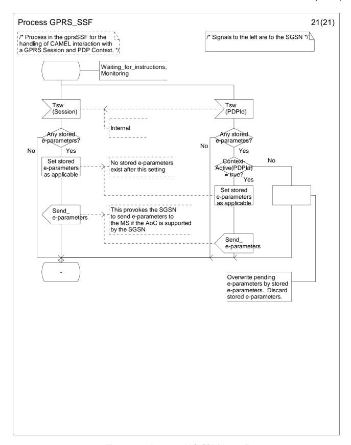
Figure 6.17u: Process GPRS\_SSF (sheet 21)
