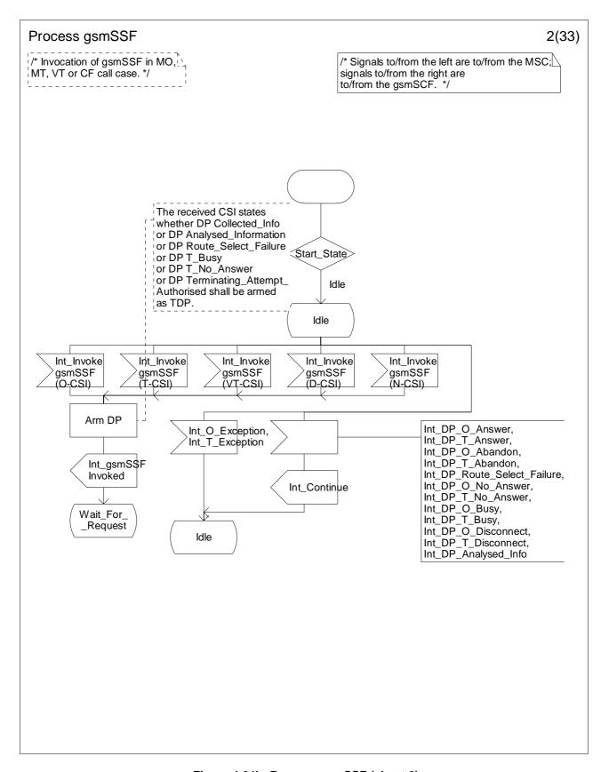
Figure 4.64b: Process gsmSSF (sheet 2)
