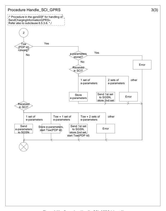
Figure 6.23c: Procedure Handle\_SCI\_GPRS (sheet 3)
