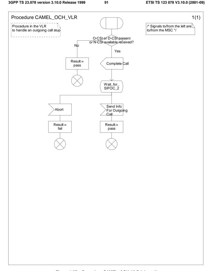
Figure 4.27a: Procedure CAMEL\_OCH\_VLR (sheet 1)
