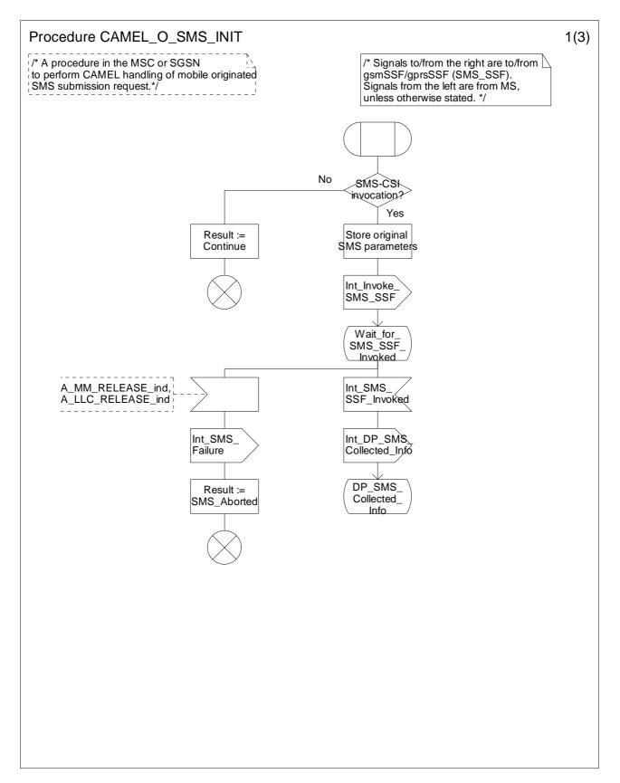
Figure 7.7a: Procedure CAMEL\_O\_SMS\_INIT (sheet 1)
