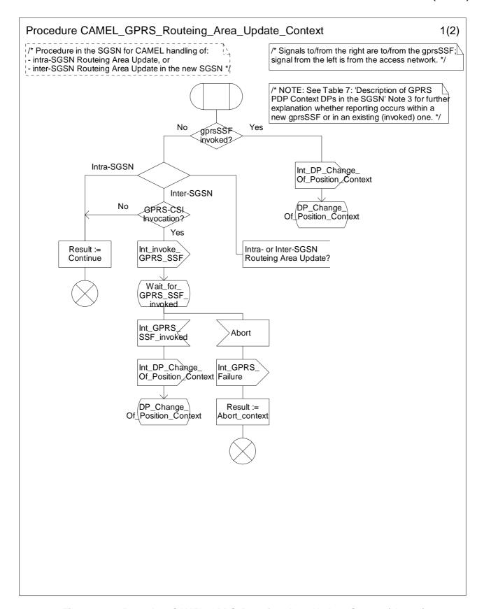
Figure 6.11a: Procedure CAMEL\_GPRS\_Routeing\_Area\_Update\_Context (sheet 1)
