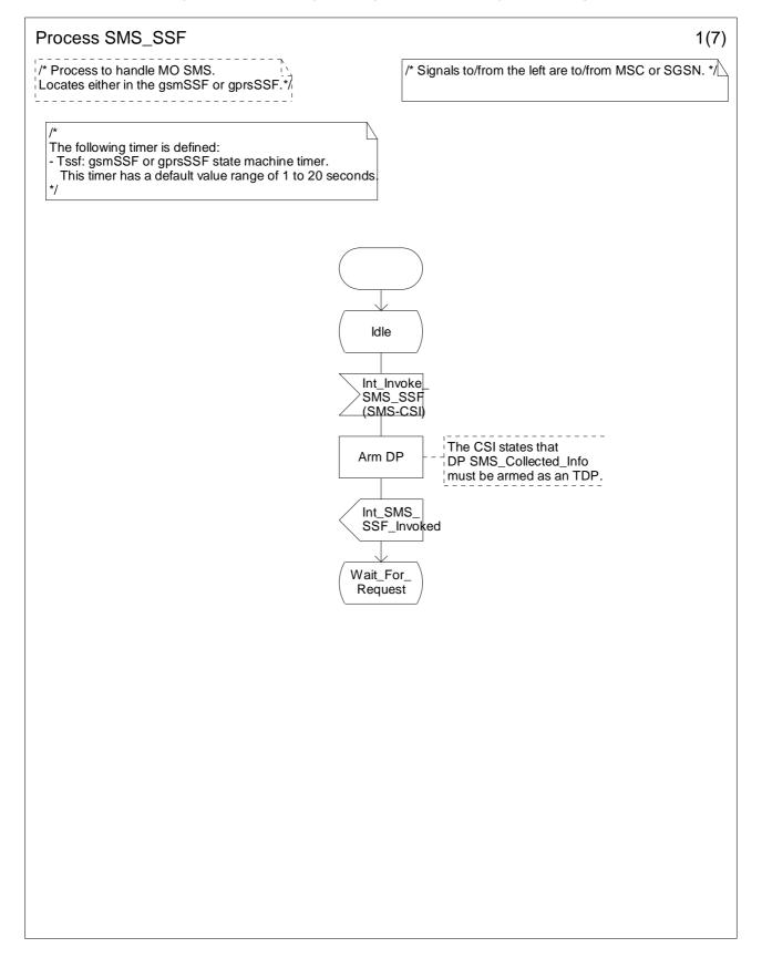
Figure 7.10a: Process SMS\_SSF (sheet 1)
