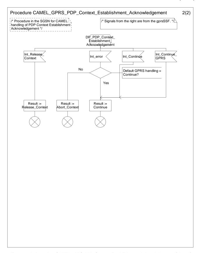
Figure 6.13b: Procedure CAMEL\_GPRS\_PDP\_Context\_Establishment\_Acknowledgement (sheet 2)
