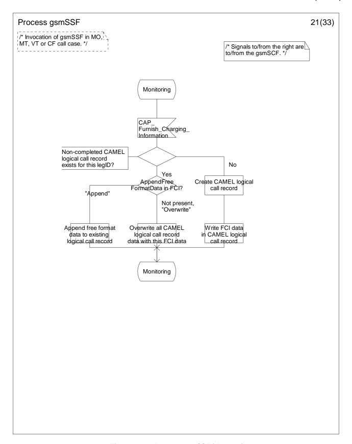
Figure 4.64u: Process gsmSSF (sheet 21)
