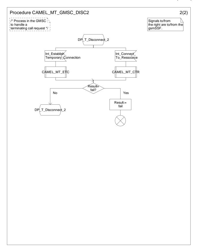
Figure 4.33b: Procedure CAMEL\_MT\_GMSC\_DISC2 (sheet 2)
