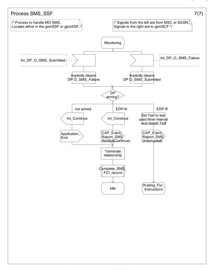
Figure 7.10g: Process SMS\_SSF (sheet 7)
