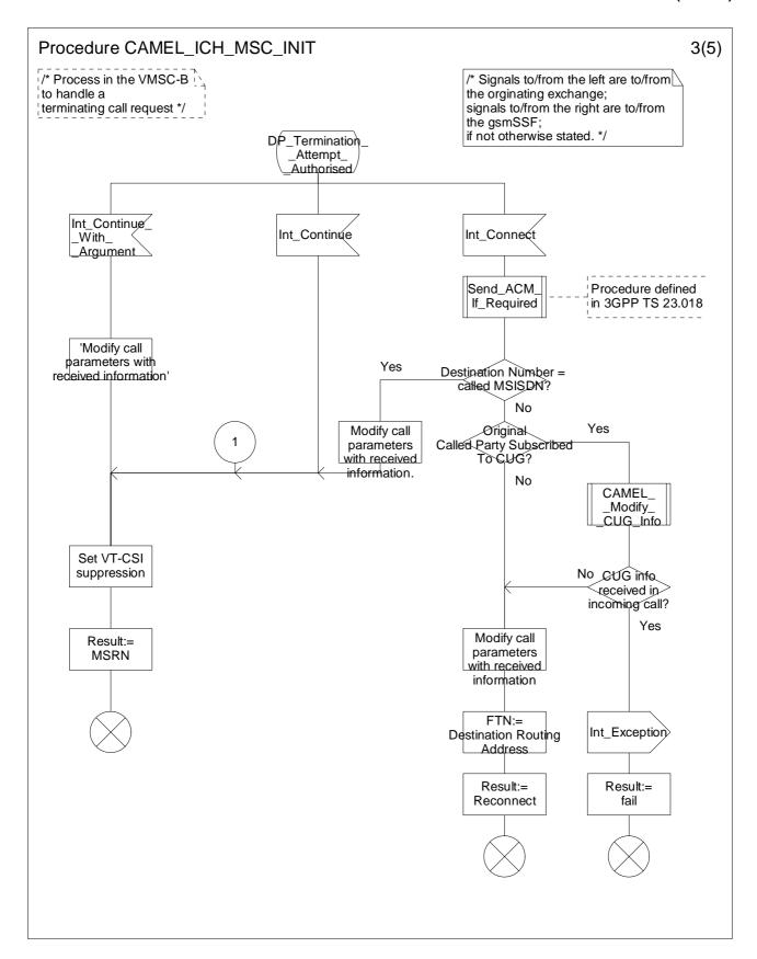
Figure 4.52c: Procedure CAMEL\_ICH\_MSC\_INIT (sheet 3)
