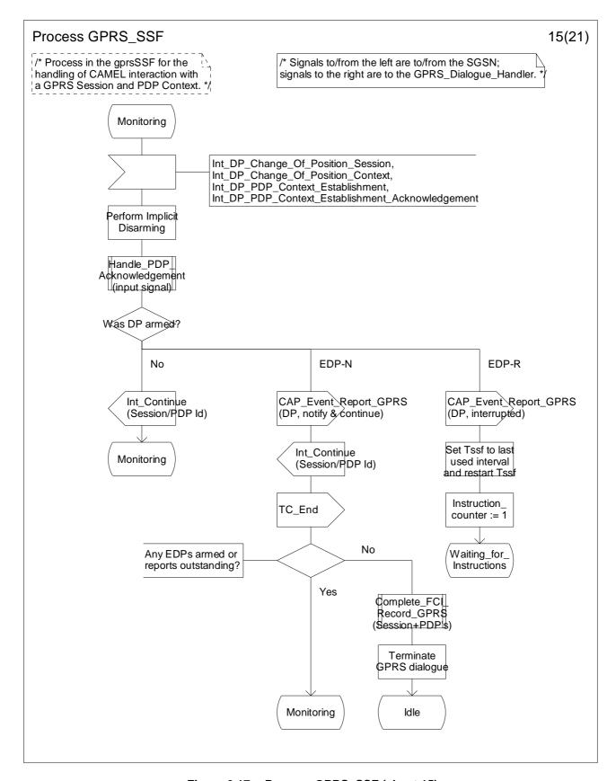
Figure 6.17o: Process GPRS\_SSF (sheet 15)
