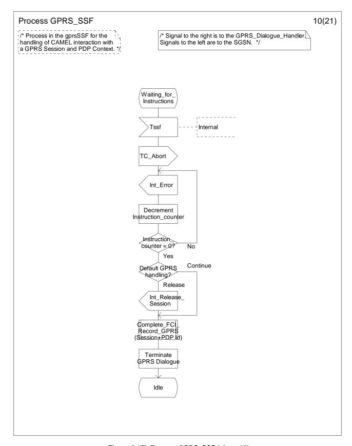
Figure 6.17j: Process GPRS\_SSF (sheet 10)
