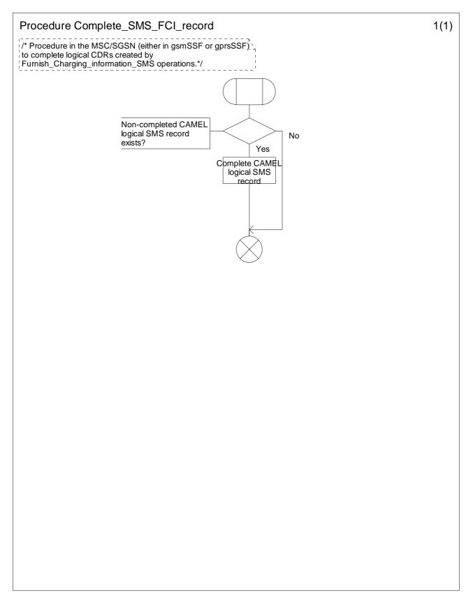
Figure 7.11: Procedure Complete\_SMS\_FCI\_record (sheet 1)
