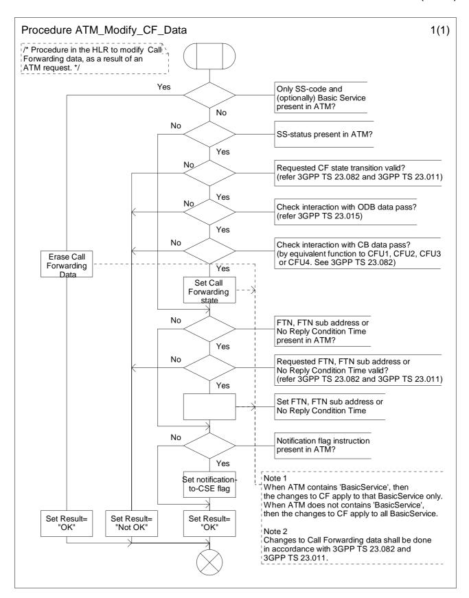
Figure 10.6: Procedure ATM\_Modify\_CF\_Data (sheet 1)
