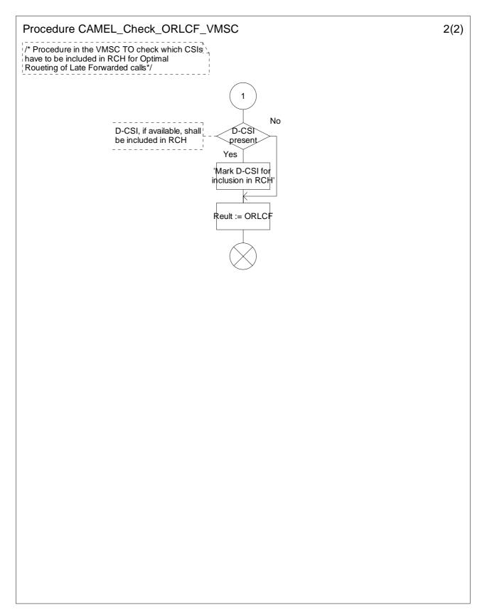
Figure 4.55b: Procedure CAMEL\_Check\_ORLCF\_VMSC (sheet 2)
