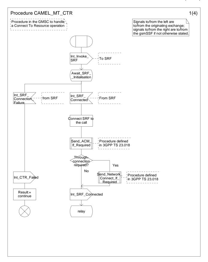
Figure 4.39a: Procedure CAMEL\_MT\_CTR (sheet 1)
