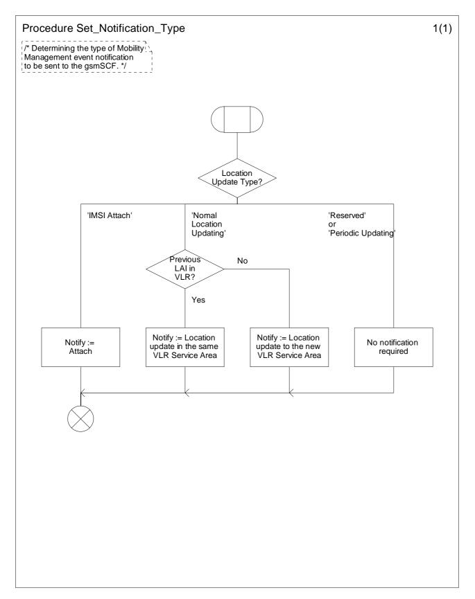
Figure 9.3: Procedure Set\_Notification\_Type (sheet 1)
