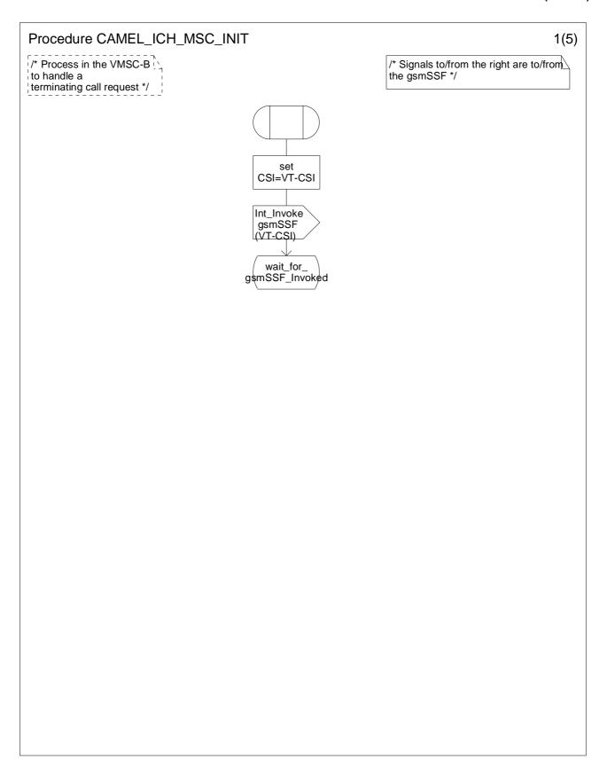
Figure 4.52a: Procedure CAMEL\_ICH\_MSC\_INIT (sheet 1)
