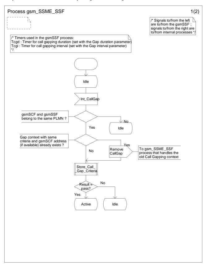
Figure 4.77a: Process gsm\_SSME\_SSF (sheet 1)
