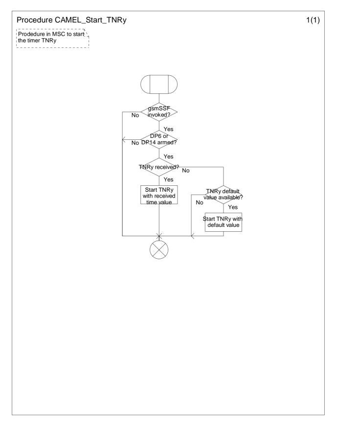
Figure 4.22: Procedure CAMEL\_Start\_TNRy (sheet 1)
