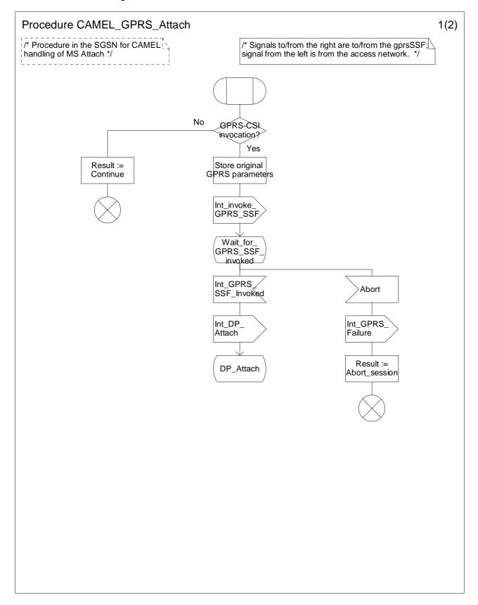
Figure 6.8a: Procedure CAMEL\_GPRS\_Attach (sheet 1)
