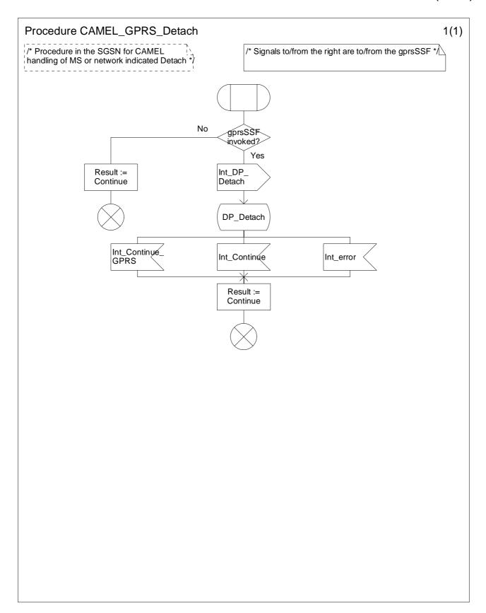
Figure 6.9: Procedure CAMEL\_GPRS\_Detach (sheet 1)
