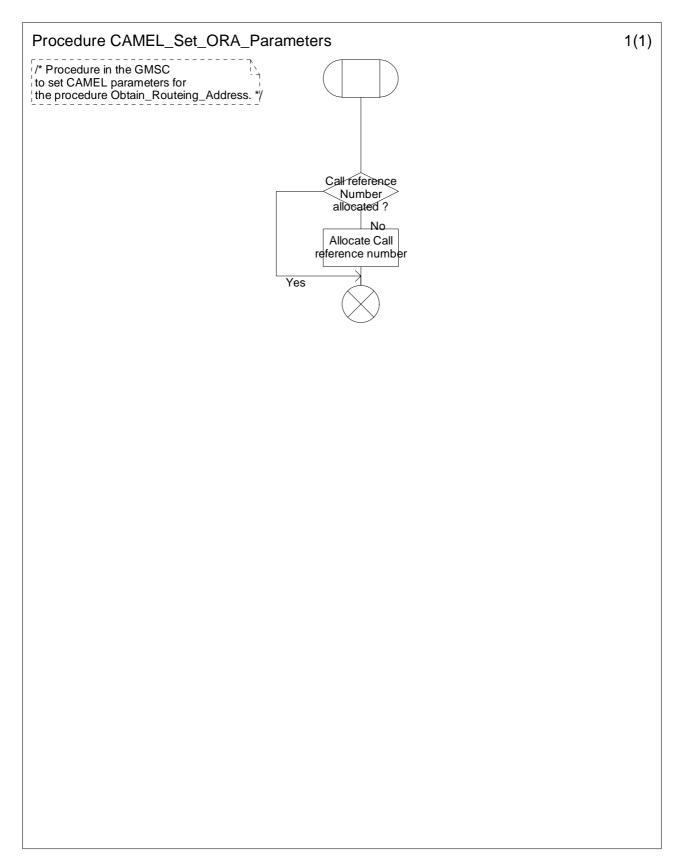
Figure 4.29a: Procedure CAMEL\_Set\_ORA\_Parameters (sheet 1)
