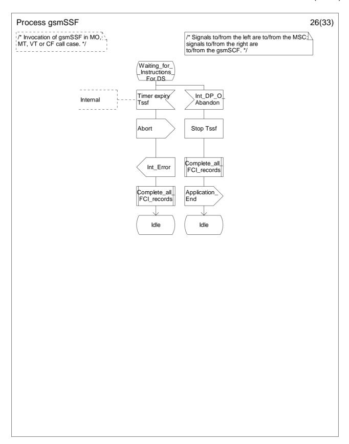
Figure 4.64z: Process gsmSSF (sheet 26)
