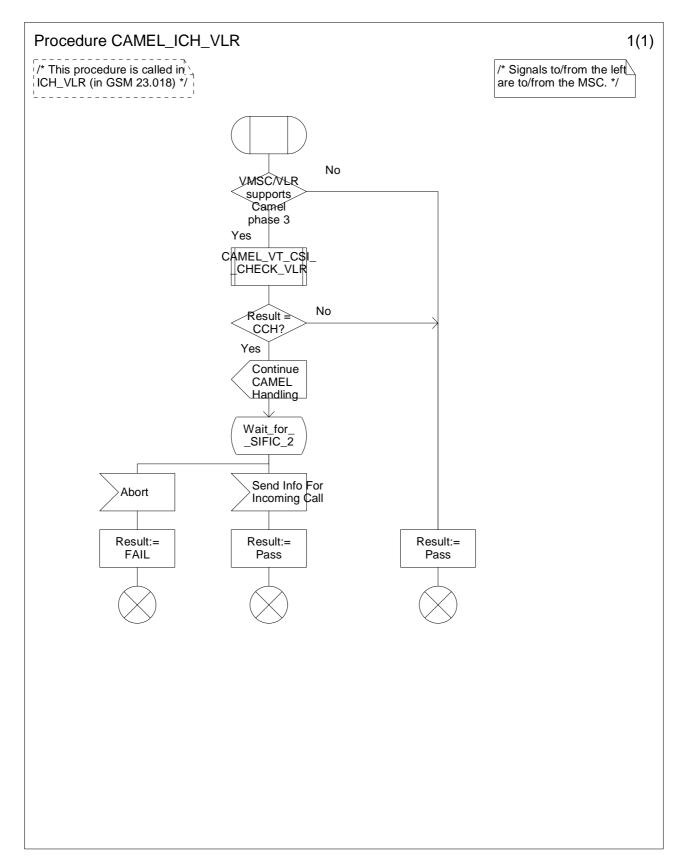
Figure 4.48: Procedure CAMEL\_ICH\_VLR (sheet 1)
