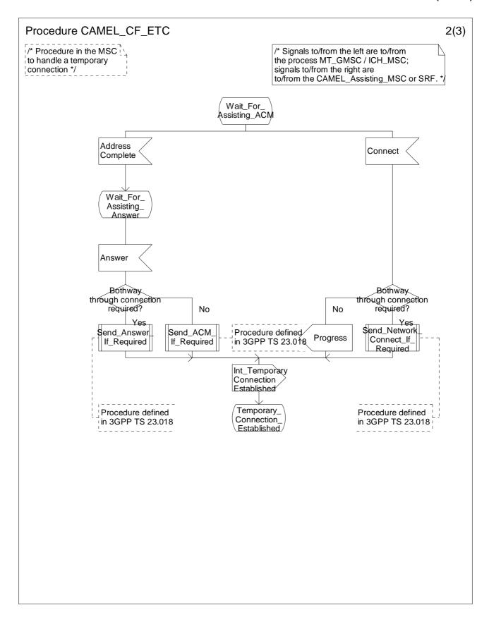
Figure 4.61b: Procedure CAMEL\_CF\_ETC (sheet 2)
