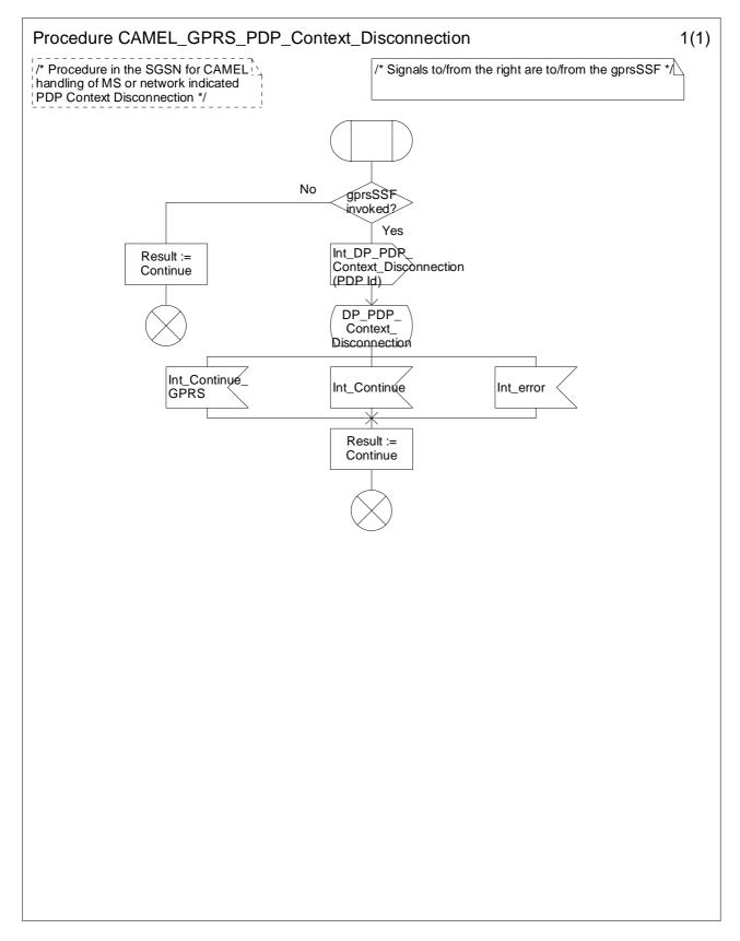
Figure 6.15: Procedure CAMEL\_GPRS\_PDP\_Context\_Disconnection (sheet 1)
