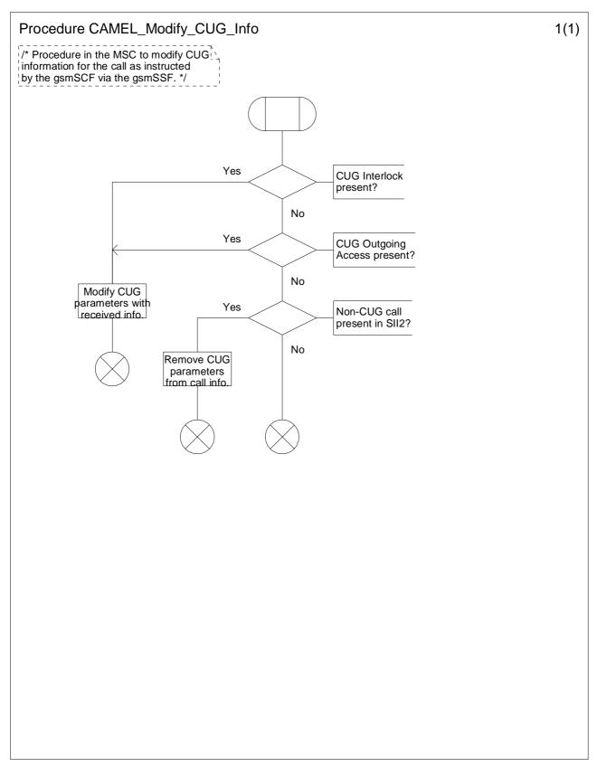
Figure 4.25: Procedure CAMEL\_Modify\_CUG\_Info (sheet 1)
