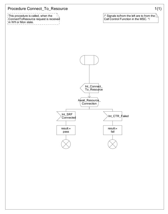
Figure 4.68: Procedure Connect\_To\_Resource (sheet 0)
