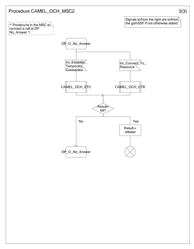
Figure 4.15c: Procedure CAMEL\_OCH\_MSC2 (sheet 3)
