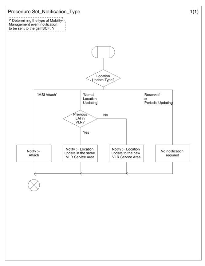
Figure 9.3: Procedure Set\_Notification\_Type (sheet 1)
