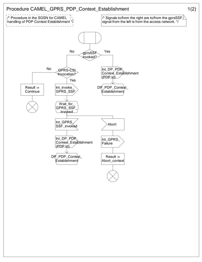
Figure 6.12a: Procedure CAMEL\_GPRS\_PDP\_Context\_Establishment (sheet 1)
