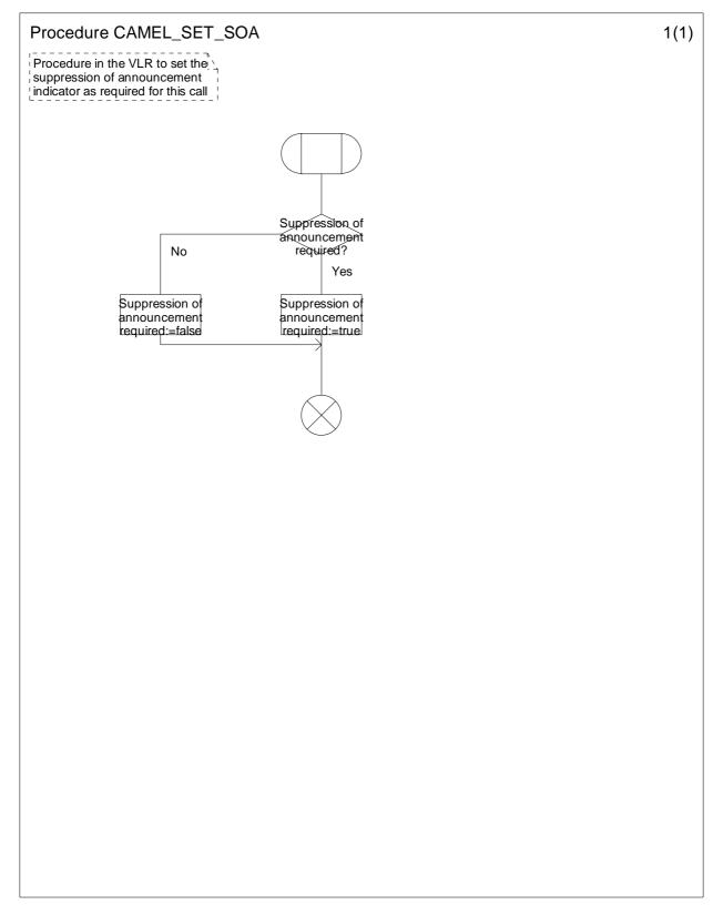
Figure 4.47: Procedure CAMEL\_SET\_SOA (sheet 1)
