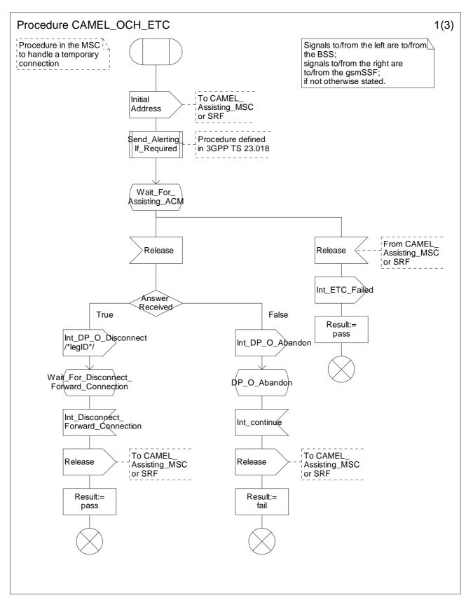
Figure 4.20a: Procedure CAMEL\_OCH\_ETC (sheet 1)
