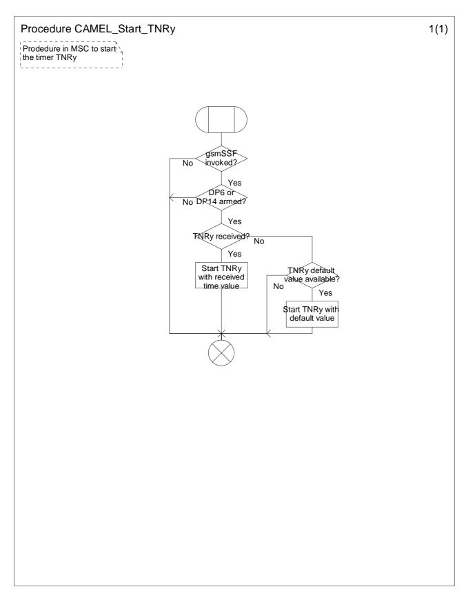
Figure 4.22: Procedure CAMEL\_Start\_TNRy (sheet 1)
