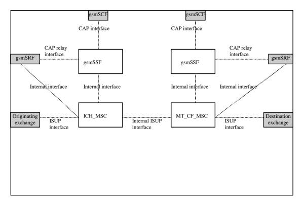
NOTE: The ICH\_MSC may also be connected via an A interface to the terminating Mobile Station.
