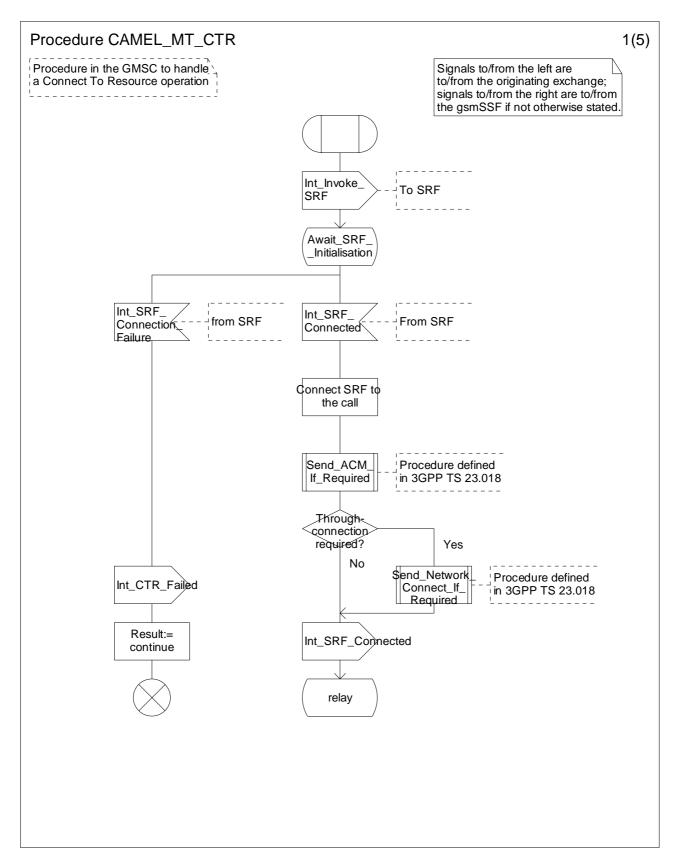
Figure 4.39a: Procedure CAMEL\_MT\_CTR (sheet 1)
