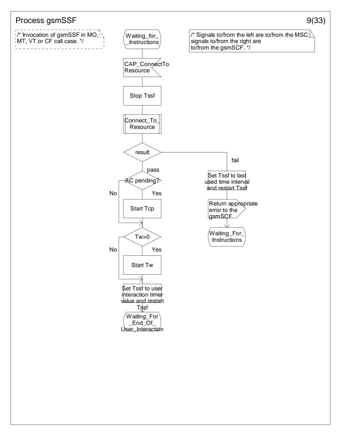
Figure 4.64i: Process gsmSSF (sheet 9)
