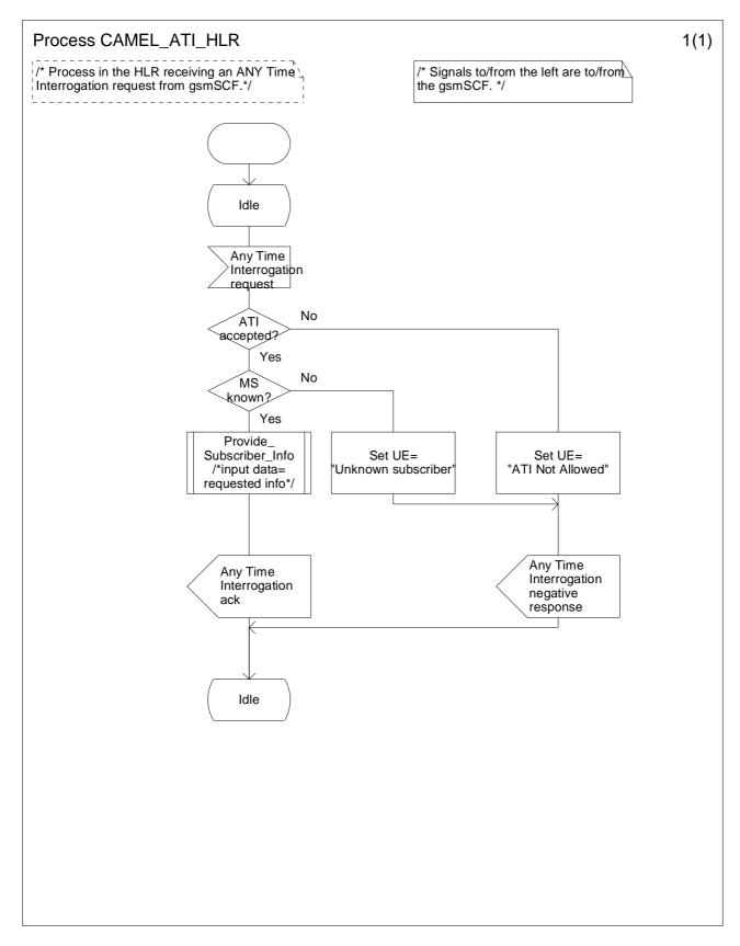
Figure 11.3: Process CAMEL\_ATI\_HLR (sheet 1)
