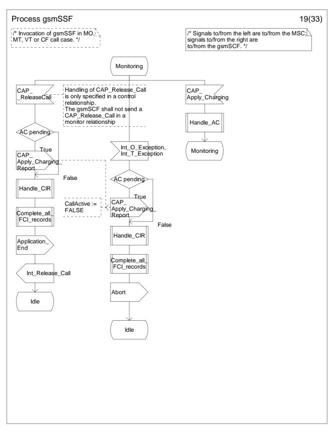
Figure 4.64s: Process gsmSSF (sheet 19)
