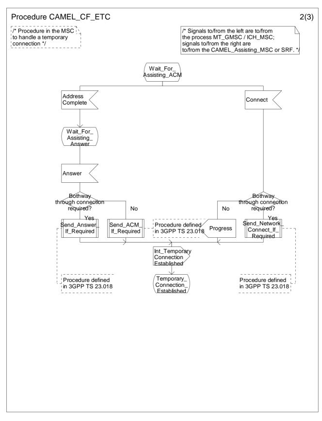
Figure 4.61b: Procedure CAMEL\_CF\_ETC (sheet 2)
