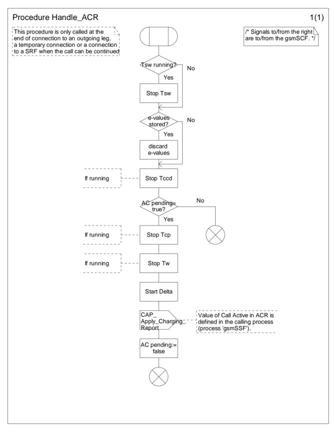
Figure 4.70: Procedure Handle\_ACR (sheet 1)
