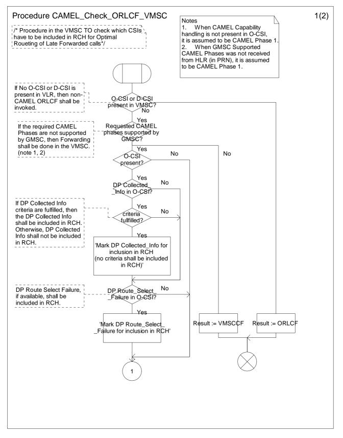
Figure 4.55a: Procedure CAMEL\_Check\_ORLCF\_VMSC (sheet 1)
