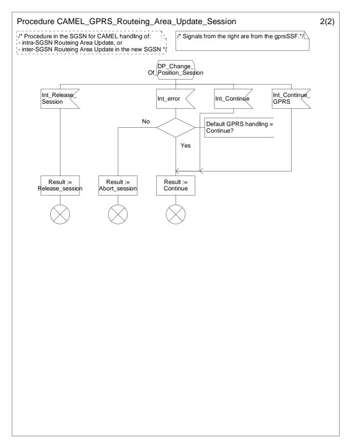
Figure 6.10b: Procedure CAMEL\_GPRS\_Routeing\_Area\_Update\_Session (sheet 2)
