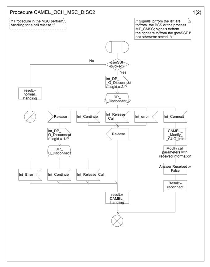
Figure 4.17a: Procedure CAMEL\_OCH\_MSC\_DISC2 (sheet 1)
