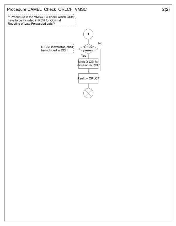
Figure 4.55b: Procedure CAMEL\_Check\_ORLCF\_VMSC (sheet 2)
