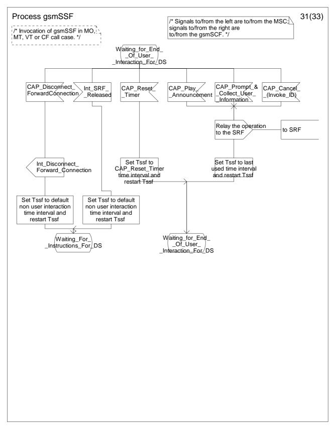
Figure 4.64ee: Process gsmSSF (sheet 31)
