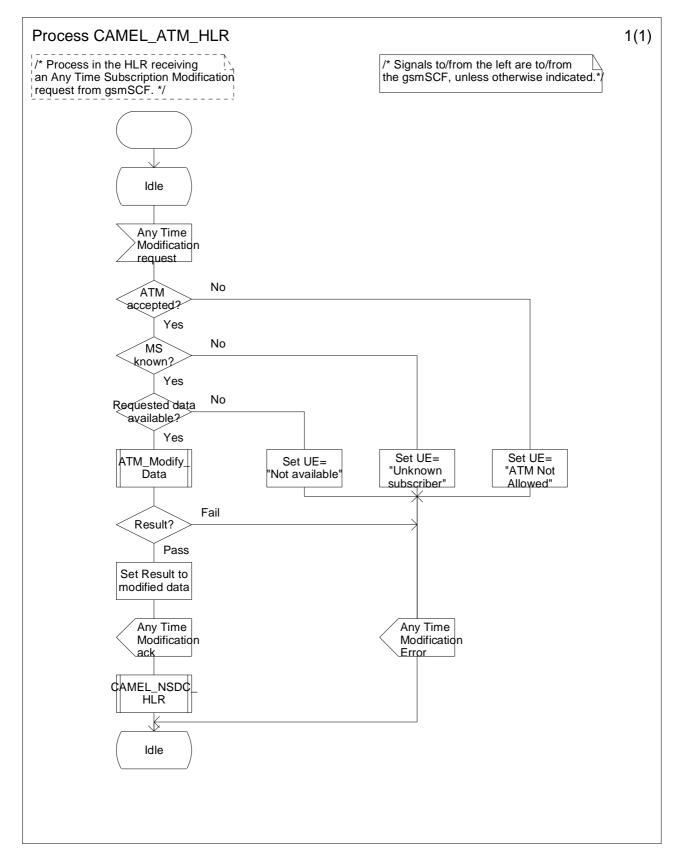
Figure 10.3: Process CAMEL\_ATM\_HLR (sheet 1)
