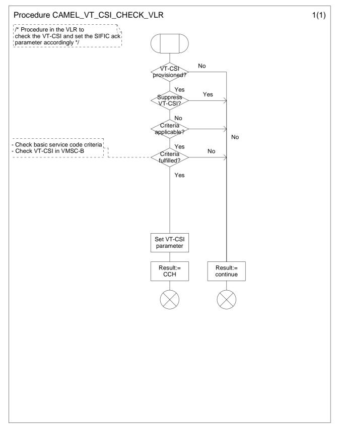
Figure 4.51: Procedure CAMEL\_VT\_CSI\_Check\_VLR (sheet 1)
