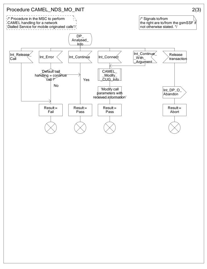
Figure 4.12b: Procedure CAMEL\_NDS\_MO\_INIT (sheet 2)
