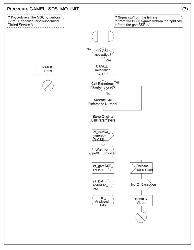
Figure 4.11a: Procedure CAMEL\_SDS\_MO\_Init (sheet 1)
