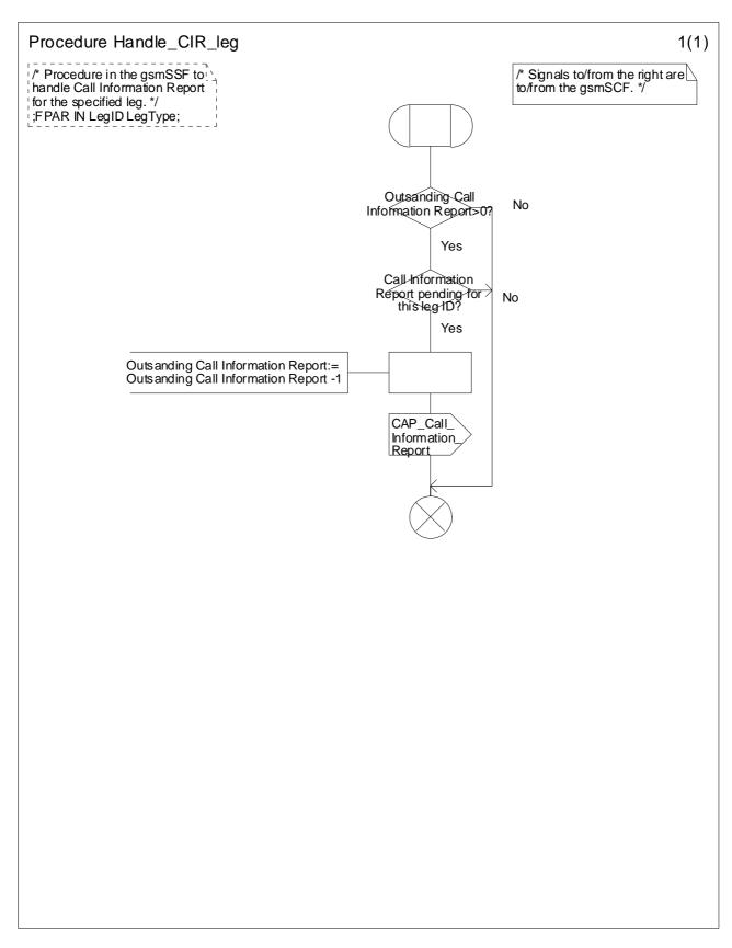
Figure 4.72: Procedure Handle\_CIR\_leg (sheet 1)
