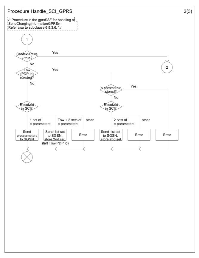
Figure 6.23b: Procedure Handle\_SCI\_GPRS (sheet 2)
