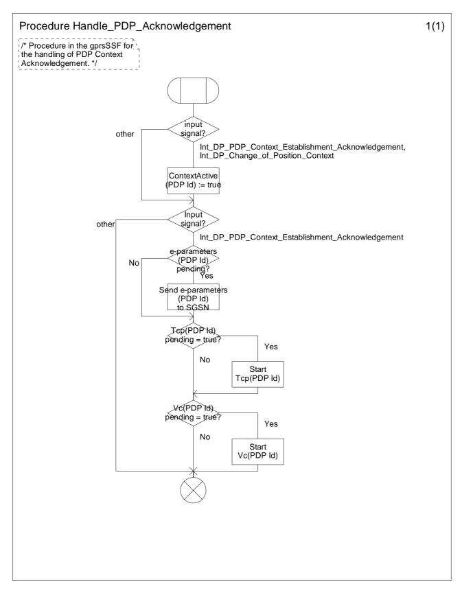
Figure 6.24: Procedure Handle\_PDP\_Acknowledgement (sheet 0)
