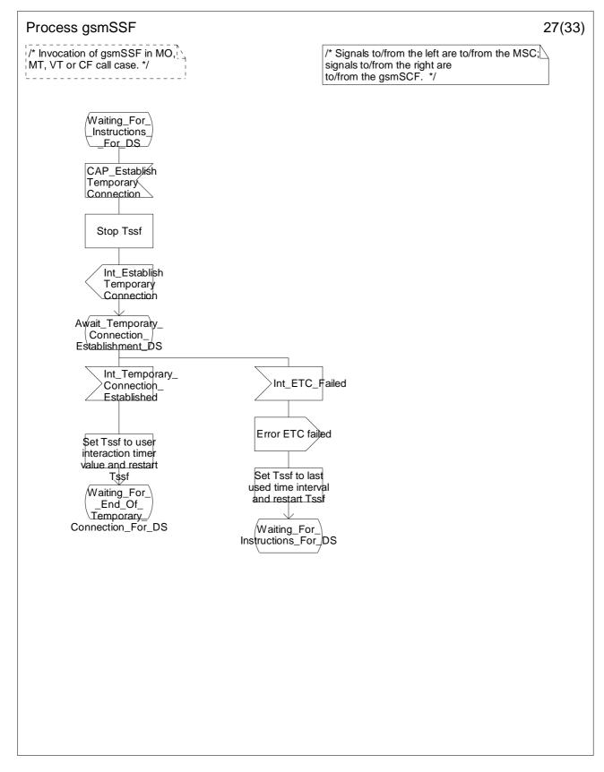
Figure 4.64aa: Process gsmSSF (sheet 27)
