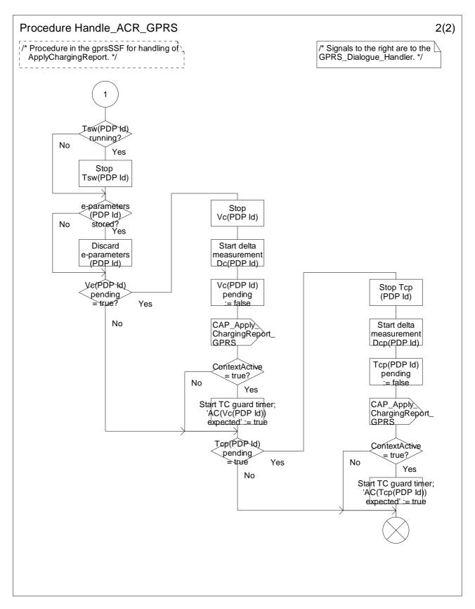
Figure 6.20b: Procedure Handle\_ACR\_GPRS (sheet 2)
