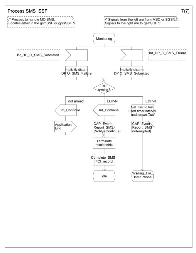
Figure 7.10g: Process SMS\_SSF (sheet 7)
