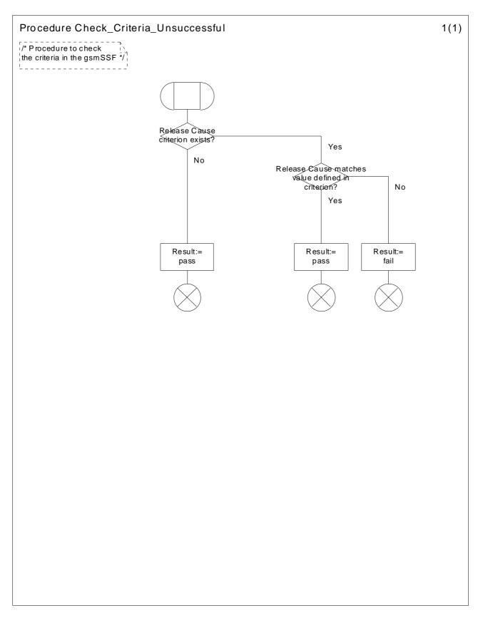
Figure 4.67: Procedure Check\_Criteria\_Unsuccessful(sheet 0)
