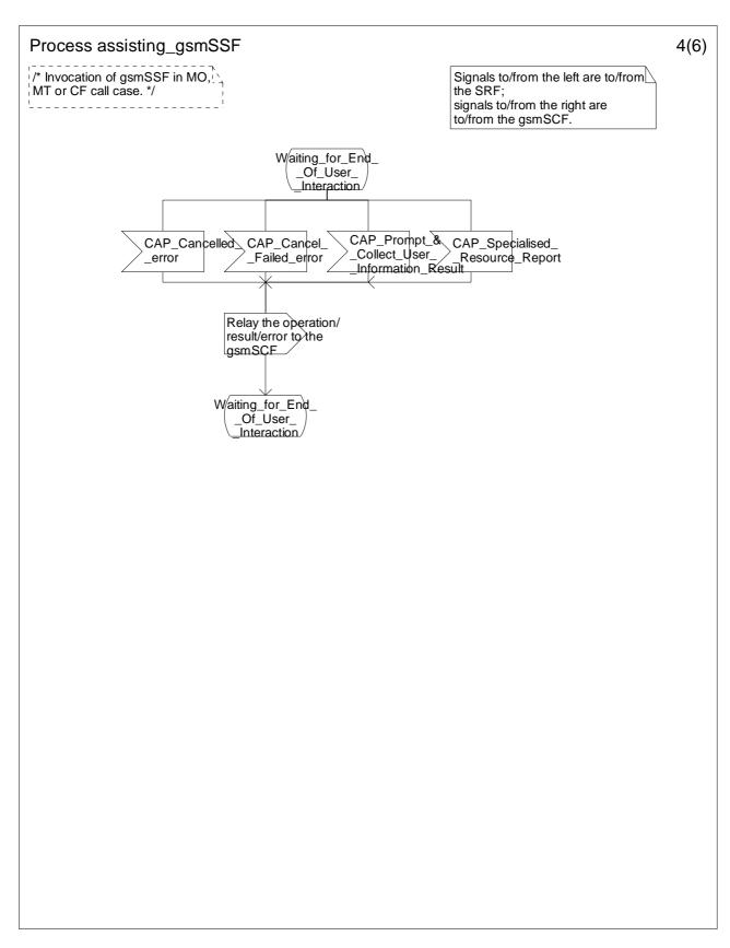
Figure 4.81d: Process Assisting\_gsmSSF (sheet 4)
