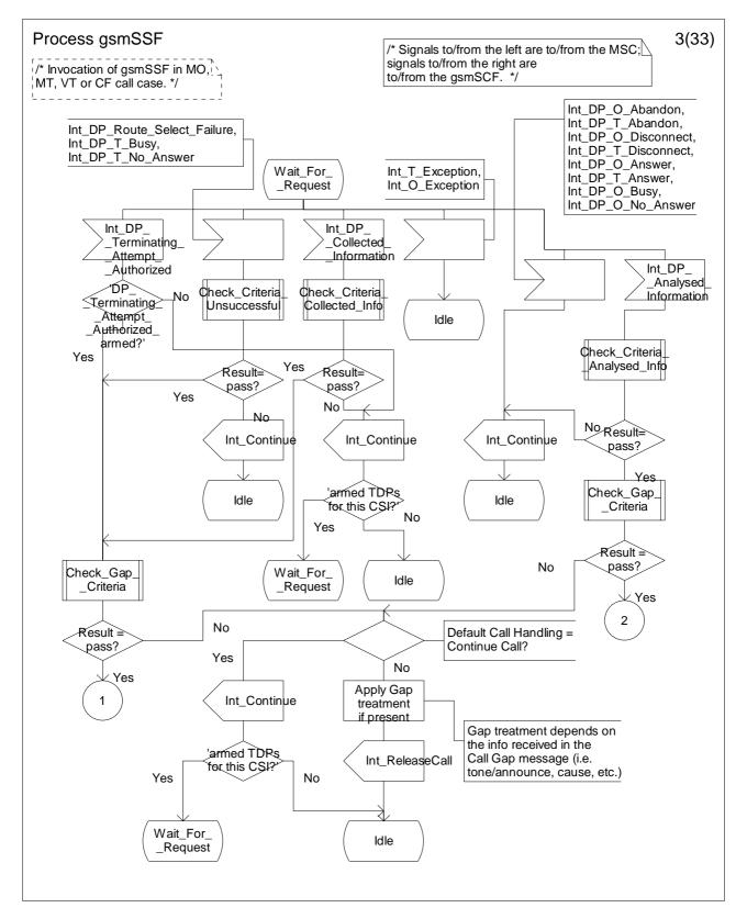
Figure 4.64c: Process gsmSSF (sheet 3)
