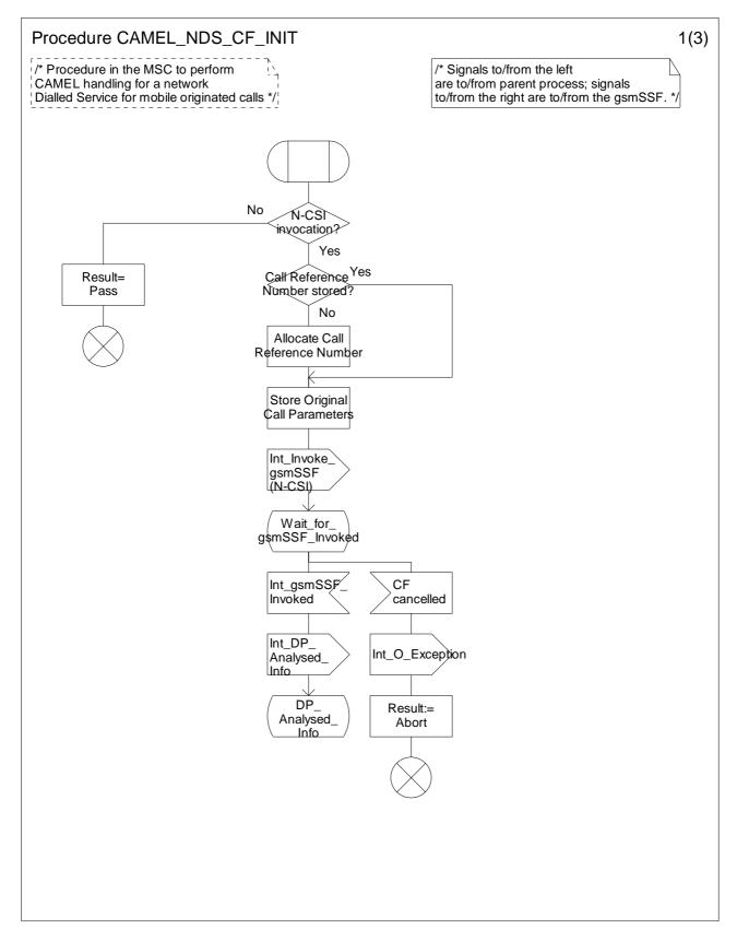
Figure 4.59a: Procedure CAMEL\_NDS\_CF\_INIT (sheet 1)
