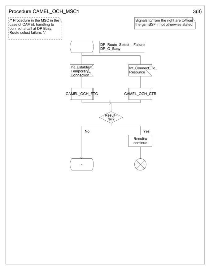
Figure 4.14c: Procedure CAMEL\_OCH\_MSC1 (sheet 3)
