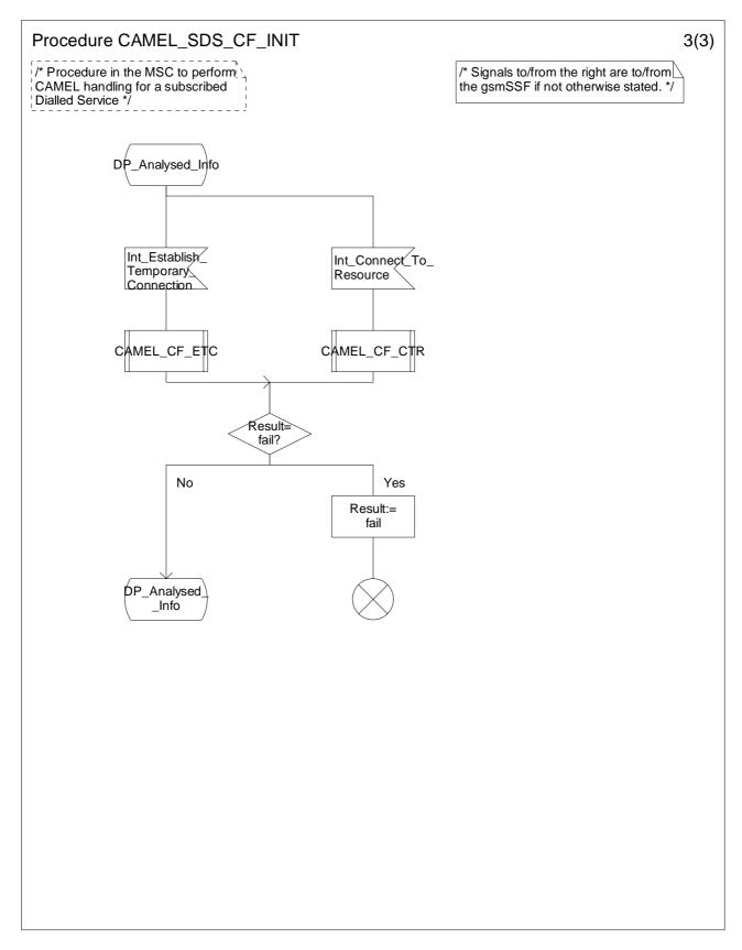
Figure 4.58c: Procedure CAMEL\_SDS\_CF\_INIT (sheet 3)
