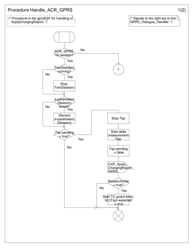
Figure 6.20a: Procedure Handle\_ACR\_GPRS (sheet 1)
