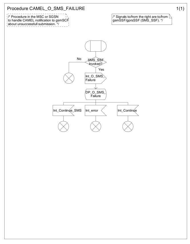
Figure 7.9: Procedure CAMEL\_O\_SMS\_FAILURE (sheet 1)
