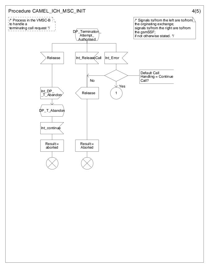
Figure 4.52d: Procedure CAMEL\_ICH\_MSC\_INIT (sheet 4)
