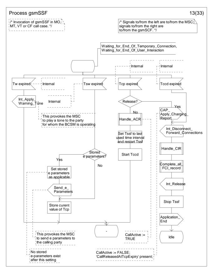
Figure 4.64m: Process gsmSSF (sheet 13)
