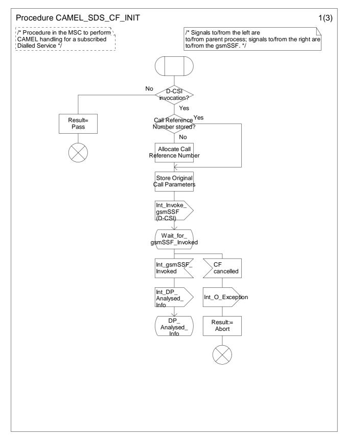
Figure 4.58a: Procedure CAMEL\_SDS\_CF\_INIT (sheet 1)
