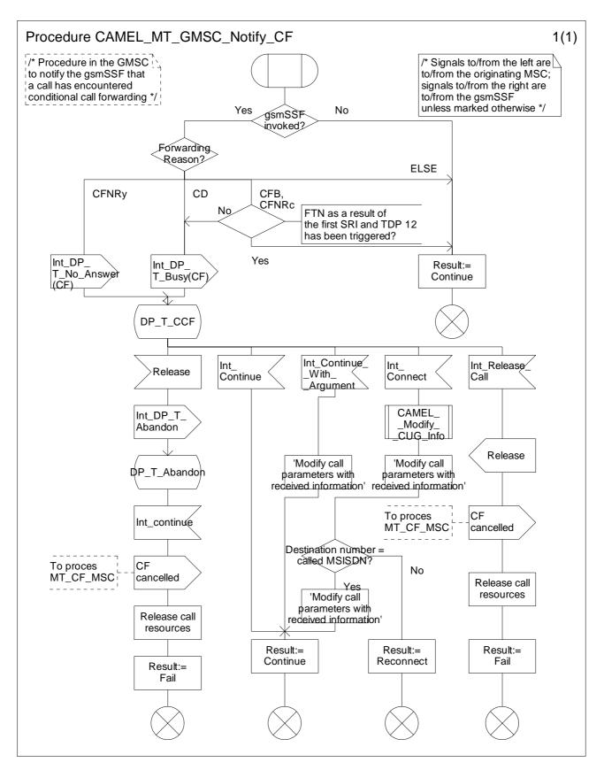
Figure 4.40: Procedure CAMEL\_MT\_GMSC\_Notify\_CF (sheet 0)
