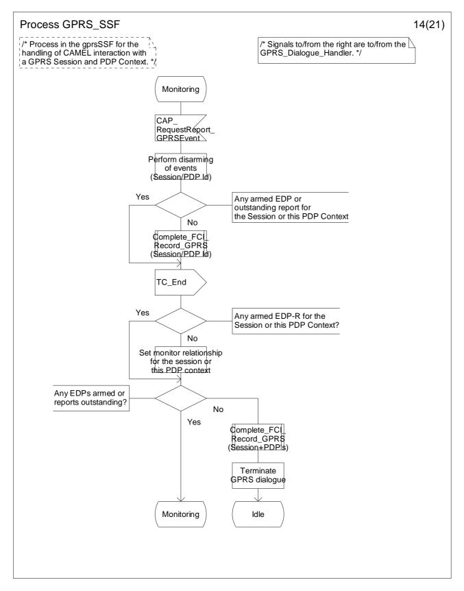
Figure 6.17n: Process GPRS\_SSF (sheet 14)
