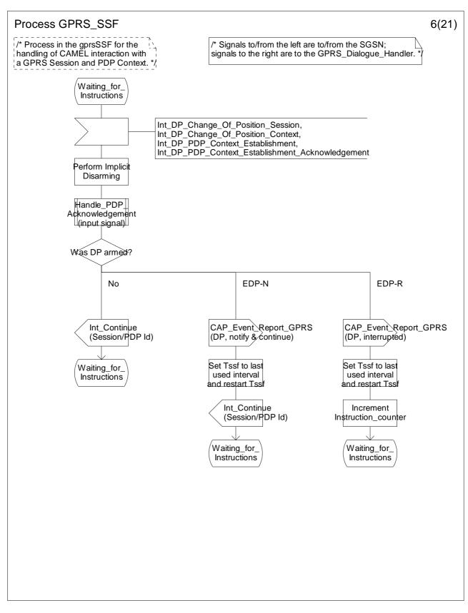
Figure 6.17f: Process GPRS\_SSF (sheet 6)
