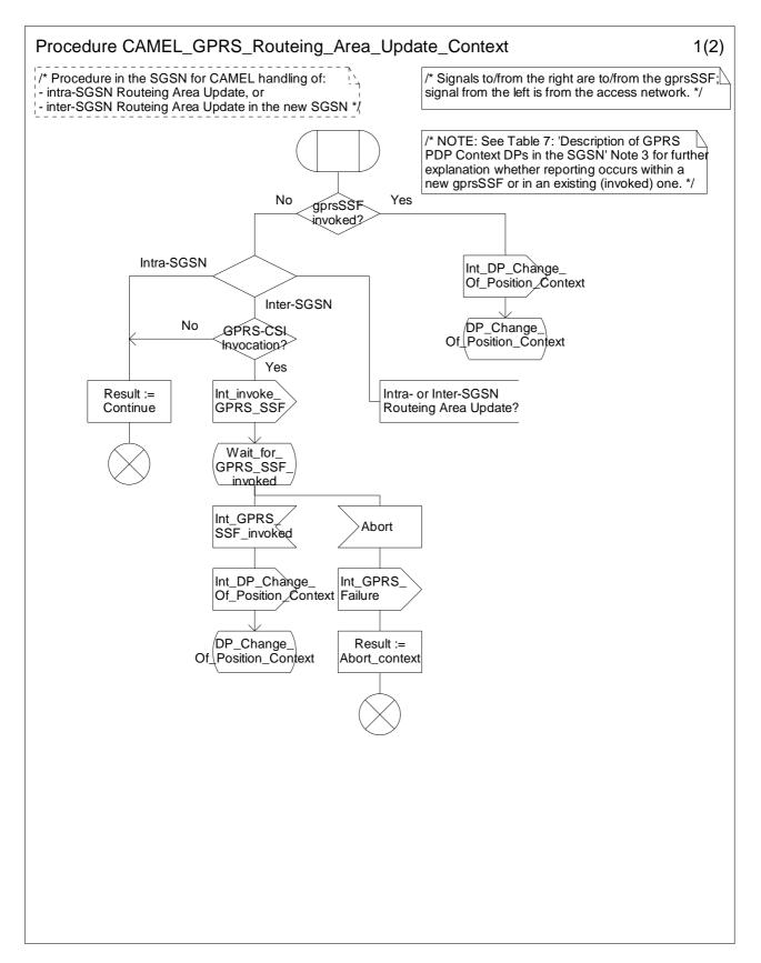
Figure 6.11a: Procedure CAMEL\_GPRS\_Routeing\_Area\_Update\_Context (sheet 1)
