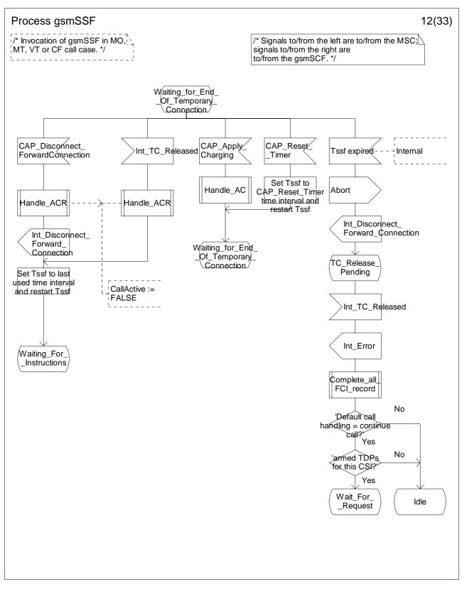
Figure 4.64I: Process gsmSSF (sheet 12)
