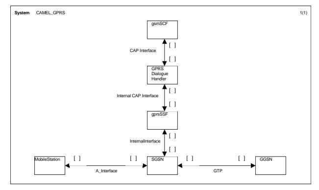
Figure 6.7: Architecture for CAMEL/GPRS interworking
