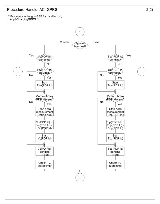
Figure 6.19b: Procedure Handle\_AC\_GPRS (sheet 2)
