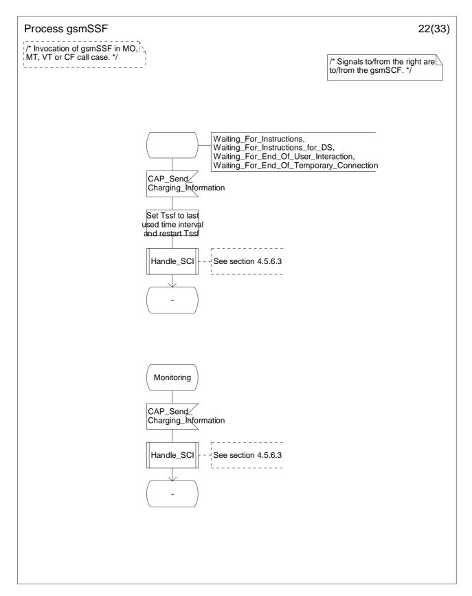
Figure 4.64v: Process gsmSSF (sheet 22)
