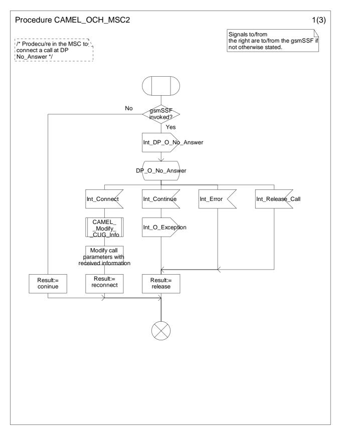
Figure 4.15a: Procedure CAMEL\_OCH\_MSC2 (sheet 1)
