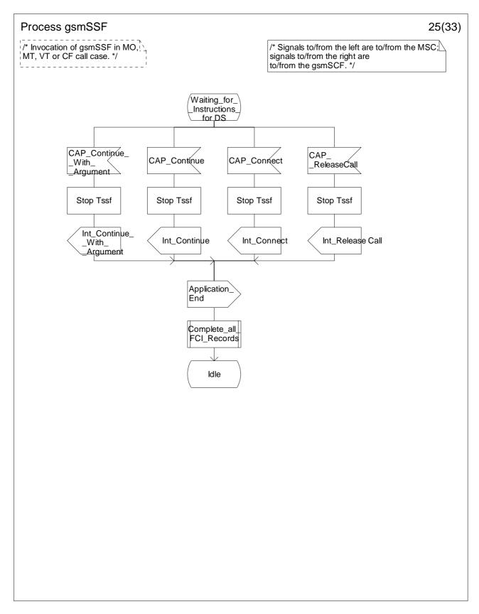
Figure 4.64y: Process gsmSSF (sheet 25)
