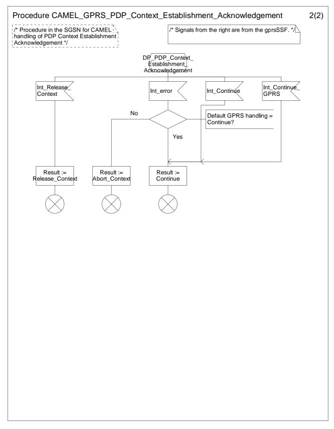
Figure 6.13b: Procedure CAMEL\_GPRS\_PDP\_Context\_Establishment\_Acknowledgement (sheet 2)
