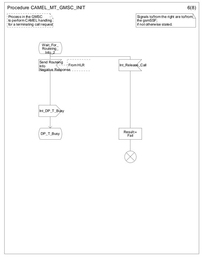
Figure 4.30f: Procedure CAMEL\_MT\_GMSC\_INIT (sheet 6)
