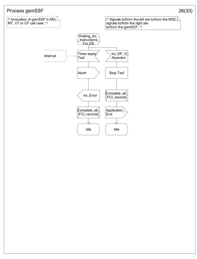
Figure 4.64z: Process gsmSSF (sheet 26)
