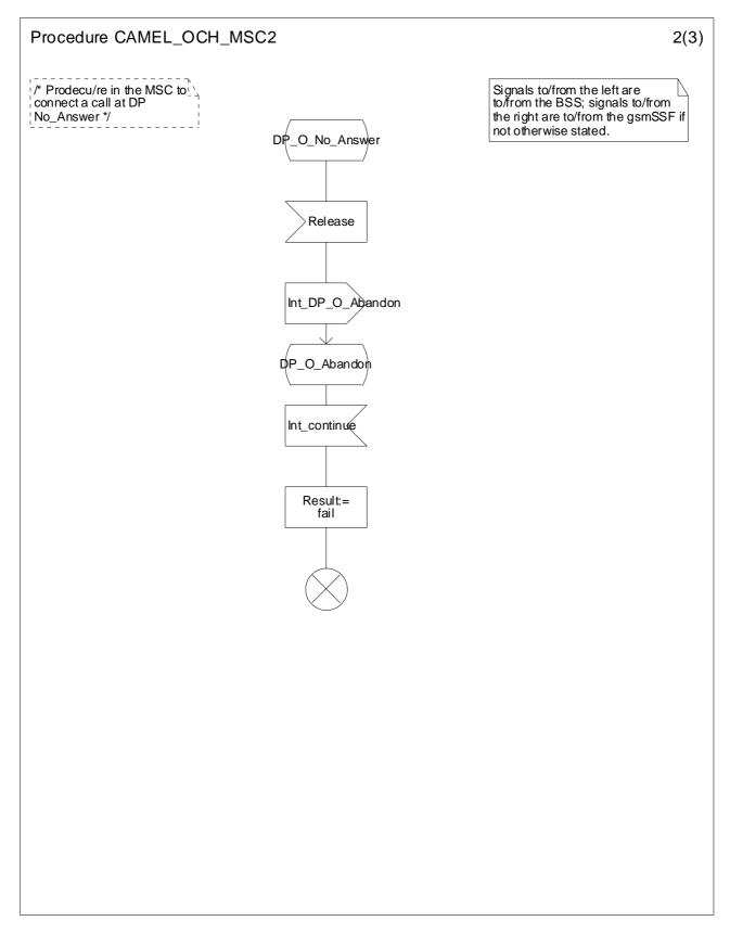
Figure 4.15b: Procedure CAMEL\_OCH\_MSC2 (sheet 2)
