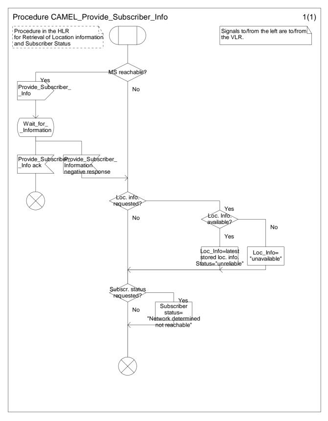
Figure 4.82: Procedure CAMEL\_Provide\_Subscriber\_Info (sheet 1)
