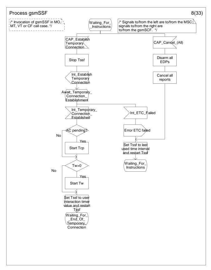
Figure 4.64h: Process gsmSSF (sheet 8)
