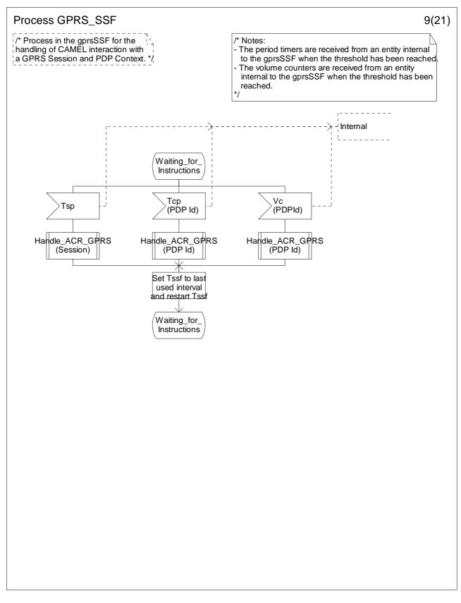
Figure 6.17i: Process GPRS\_SSF (sheet 9)
