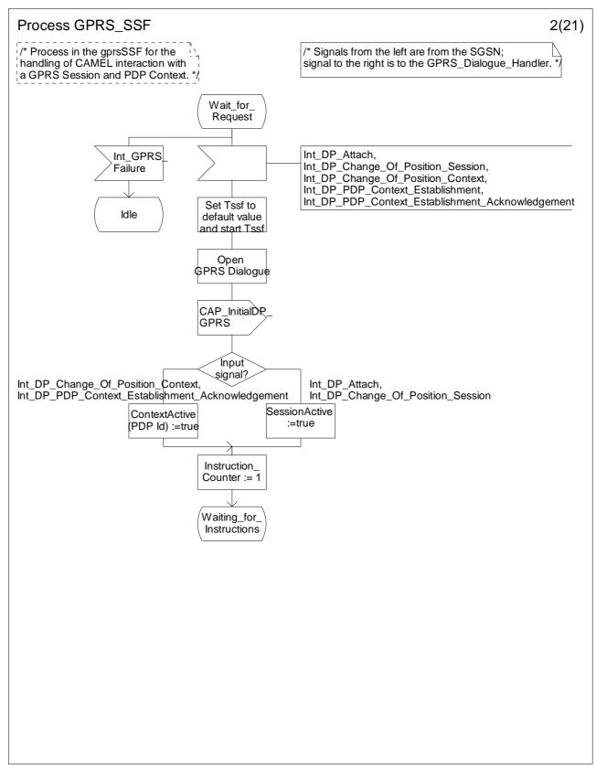
Figure 6.17b: Process GPRS\_SSF (sheet 2)
