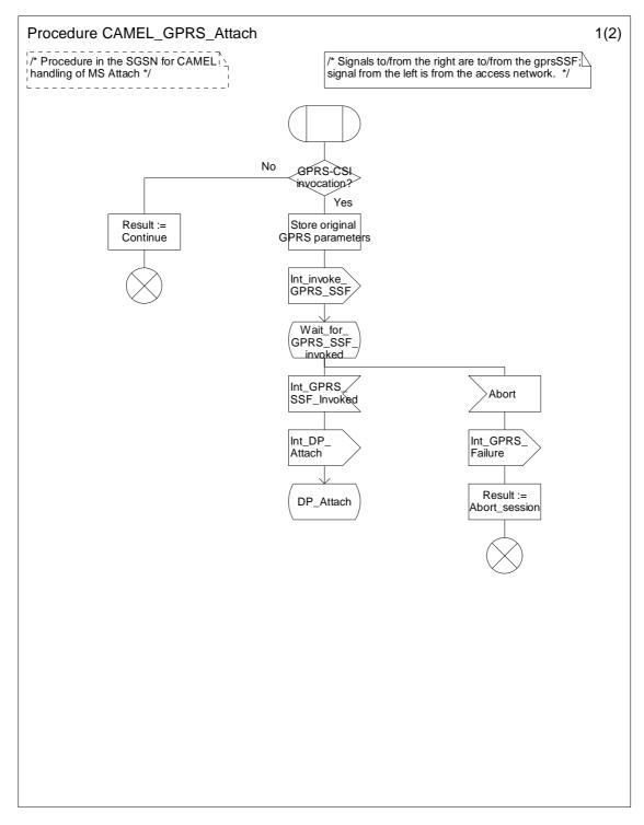
Figure 6.8a: Procedure CAMEL\_GPRS\_Attach (sheet 1)
