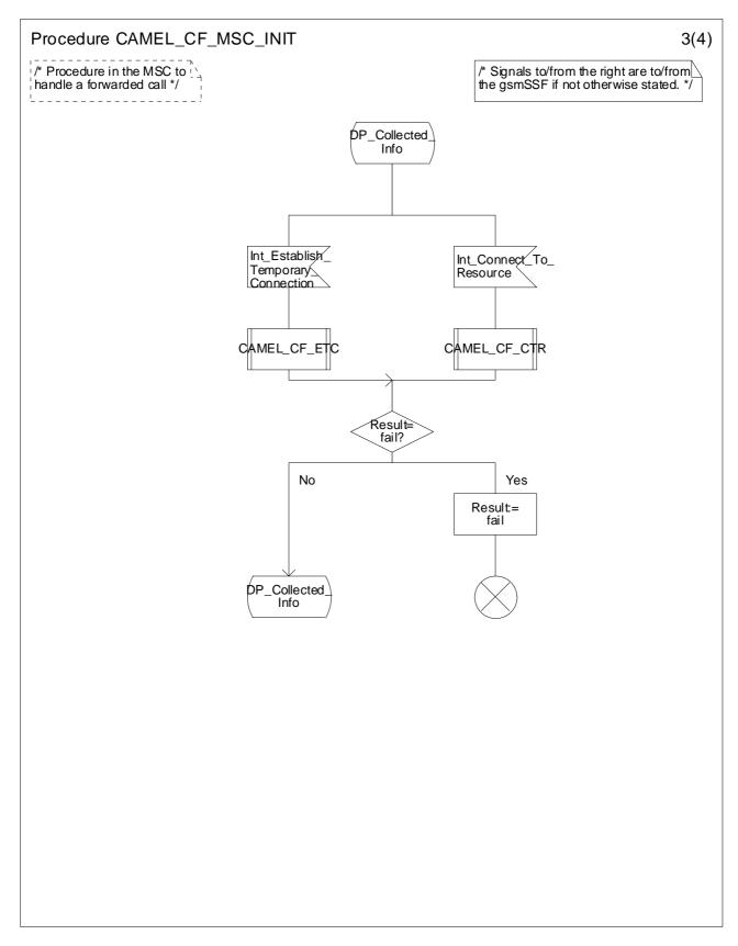
Figure 4.57c: Procedure CAMEL\_CF\_MSC\_INIT (sheet 3)
