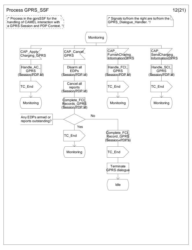
Figure 6.17I: Process GPRS\_SSF (sheet 12)
