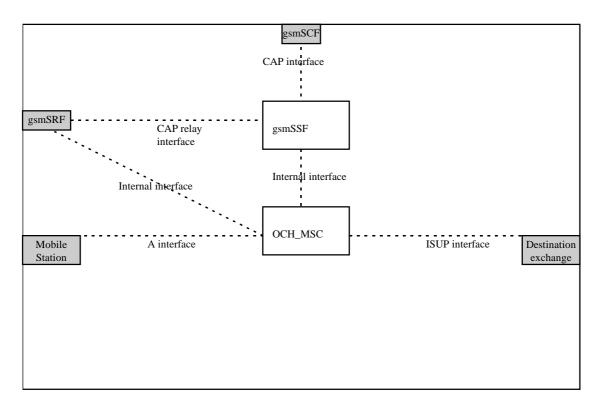
Figure 4.8a: Outgoing case (gsmSSF relay)
