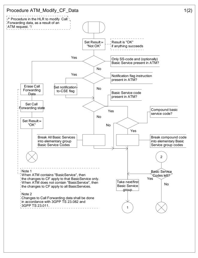
Figure 10.6a: Procedure ATM\_Modify\_CF\_Data (sheet 1)
