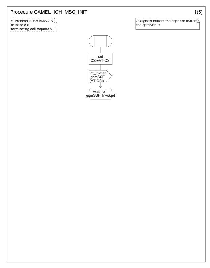
Figure 4.52a: Procedure CAMEL\_ICH\_MSC\_INIT (sheet 1)
