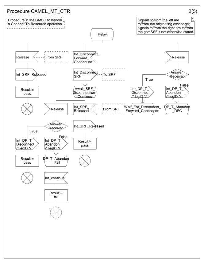
Figure 4.39b: Procedure CAMEL\_MT\_CTR (sheet 2)
