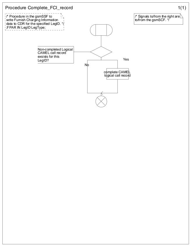
Figure 4.73: Procedure Complete\_FCI\_record (sheet 1)
