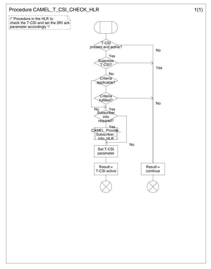
Figure 4.45: Procedure CAMEL\_T\_CSI\_CHECK\_HLR (sheet 1)
