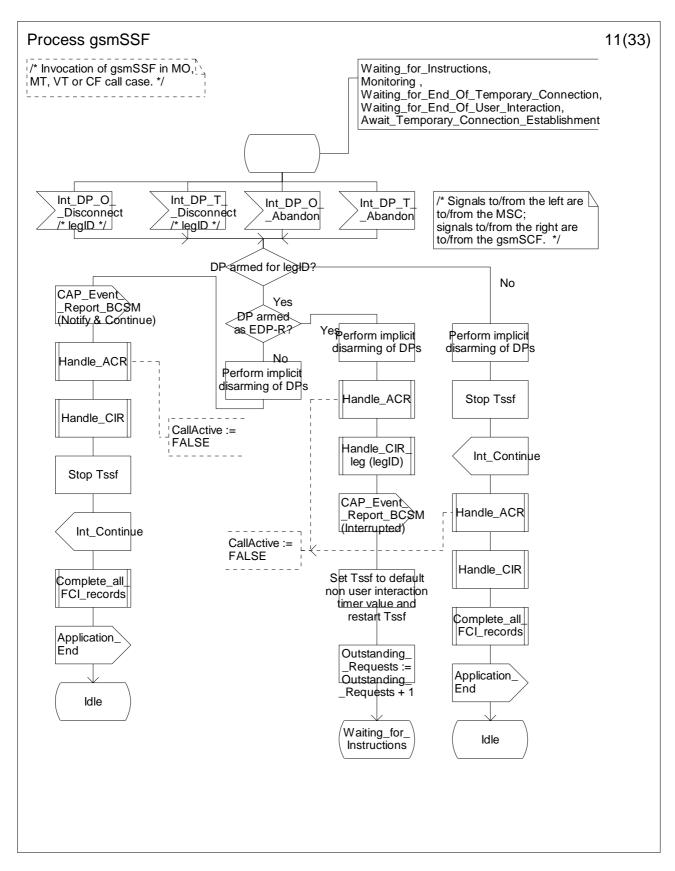
Figure 4.64k: Process gsmSSF (sheet 11)
