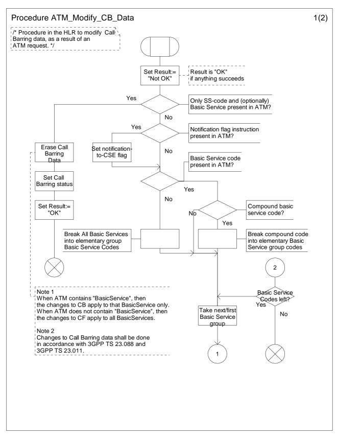
Figure 10.7a: Procedure ATM\_Modify\_CB\_Data (sheet 1)
