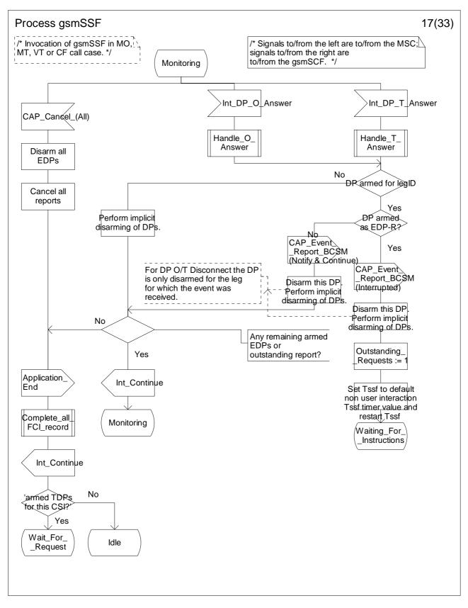
Figure 4.64q: Process gsmSSF (sheet 17)
