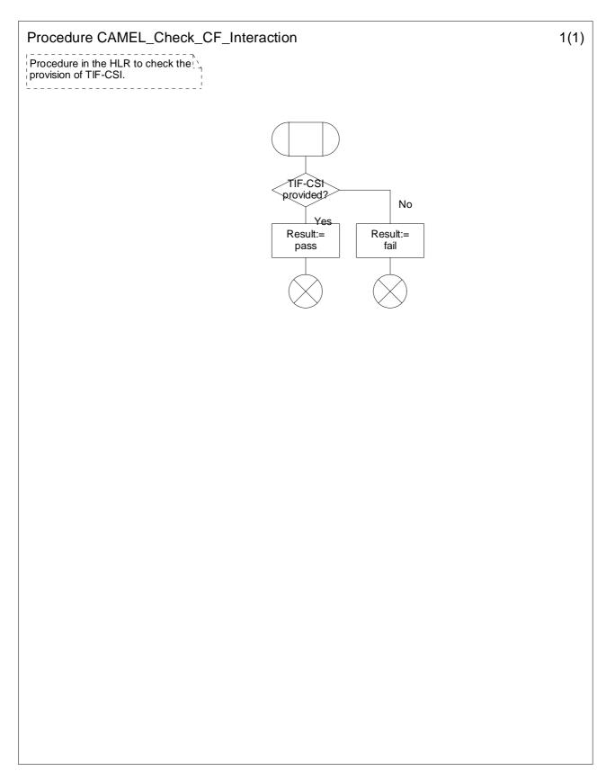
Figure 4.83: Procedure CAMEL\_Check\_CF\_Interaction
