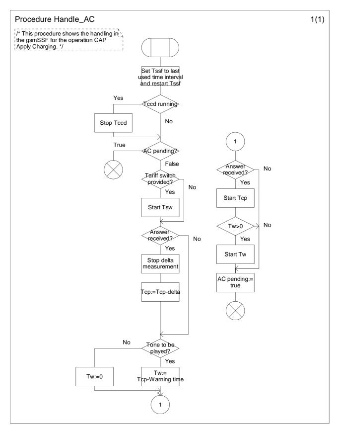
Figure 4.69: Procedure Handle\_AC (sheet 1)
