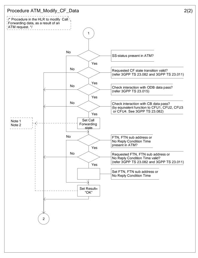
Figure 10.6b: Procedure ATM\_Modify\_CF\_Data (sheet 2)
