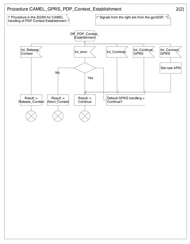
Figure 6.12b: Procedure CAMEL\_GPRS\_PDP\_Context\_Establishment (sheet 2)
