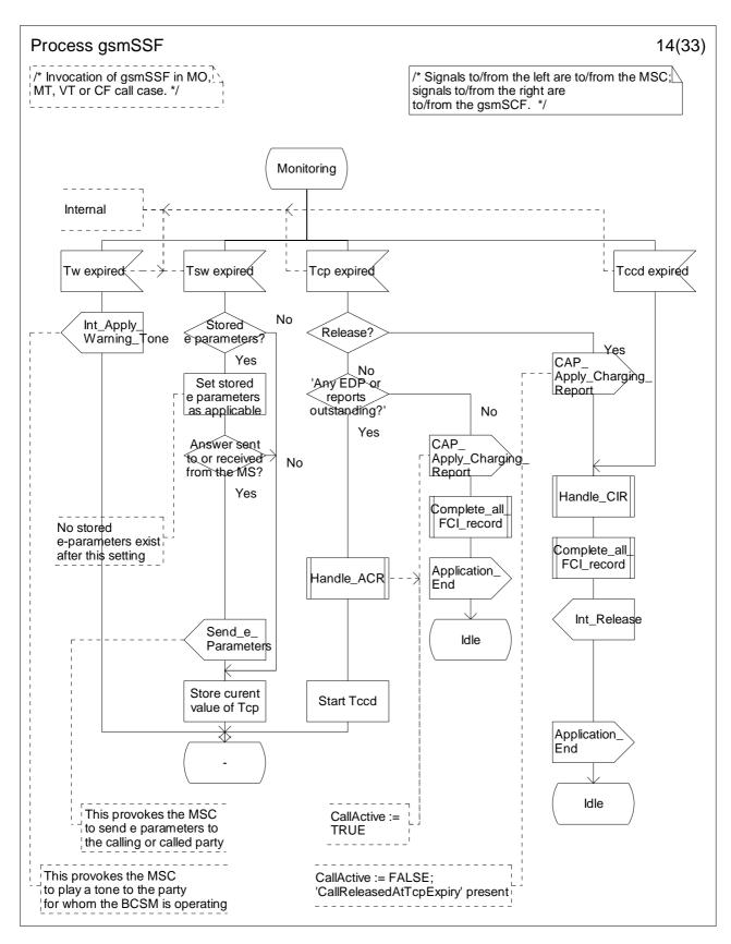
Figure 4.64n: Process gsmSSF (sheet 14)
