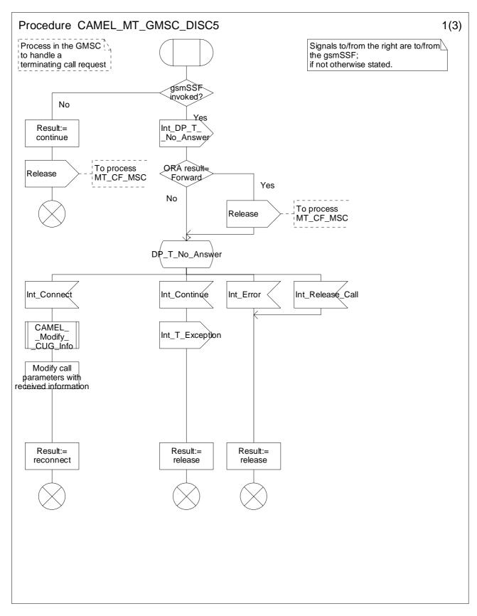
Figure 4.36a: Procedure CAMEL\_MT\_GMSC\_DISC5 (sheet 1)
