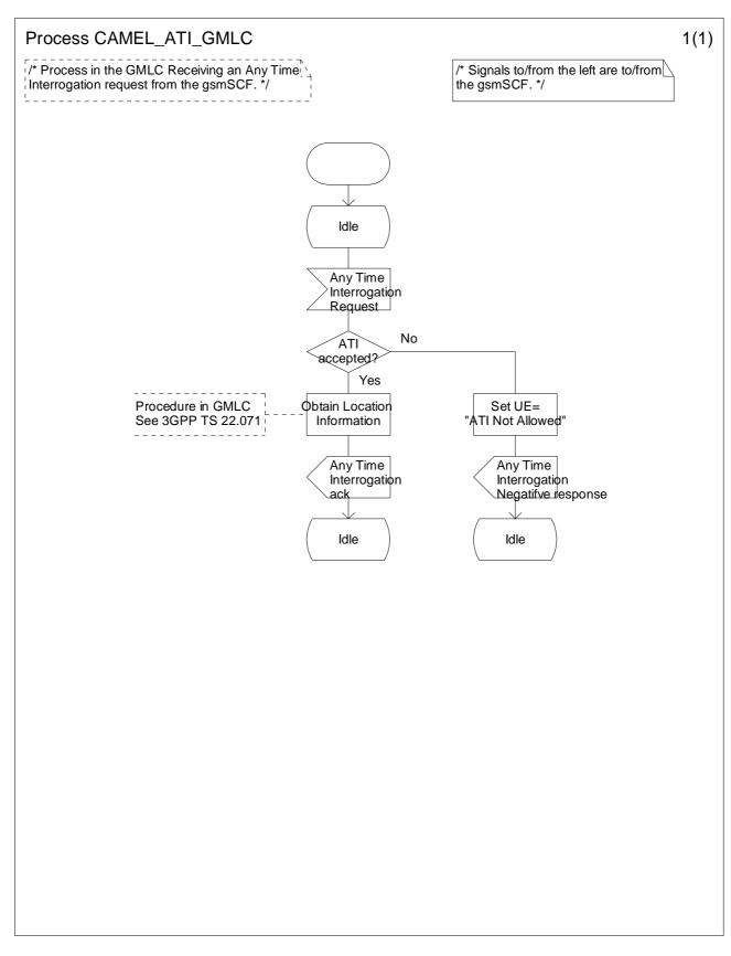
Figure 11.2: Process CAMEL\_ATI\_GMLC (sheet 1)
