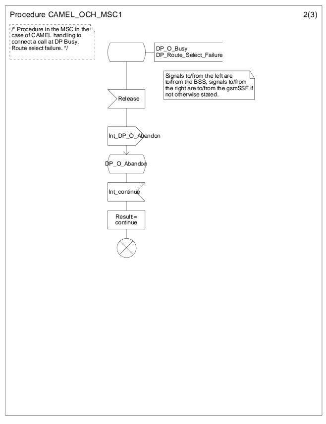
Figure 4.14b: Procedure CAMEL\_OCH\_MSC1 (sheet 2)
