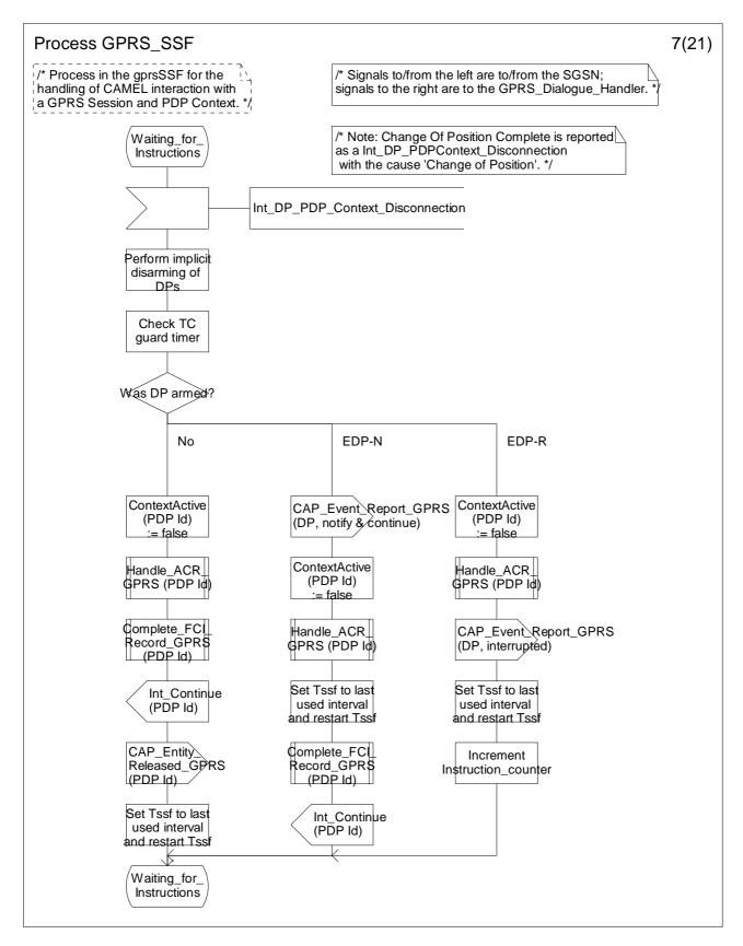
Figure 6.17g: Process GPRS\_SSF (sheet 7)
