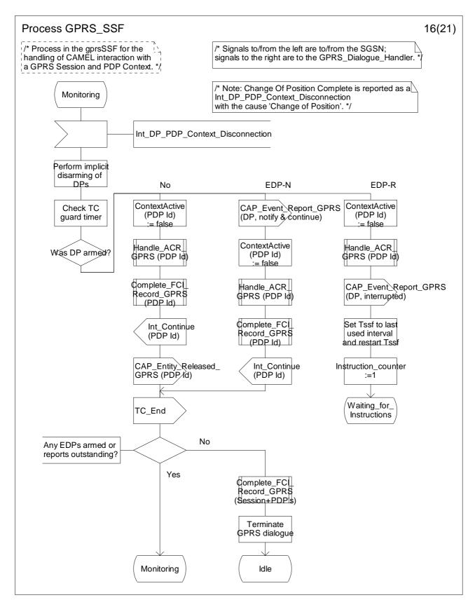
Figure 6.17p: Process GPRS\_SSF (sheet 16)
