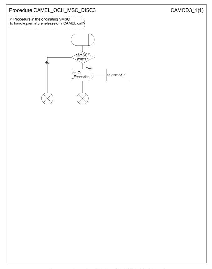
Figure 4.18: Procedure CAMEL\_OCH\_MSC\_DISC3 (sheet 1)
