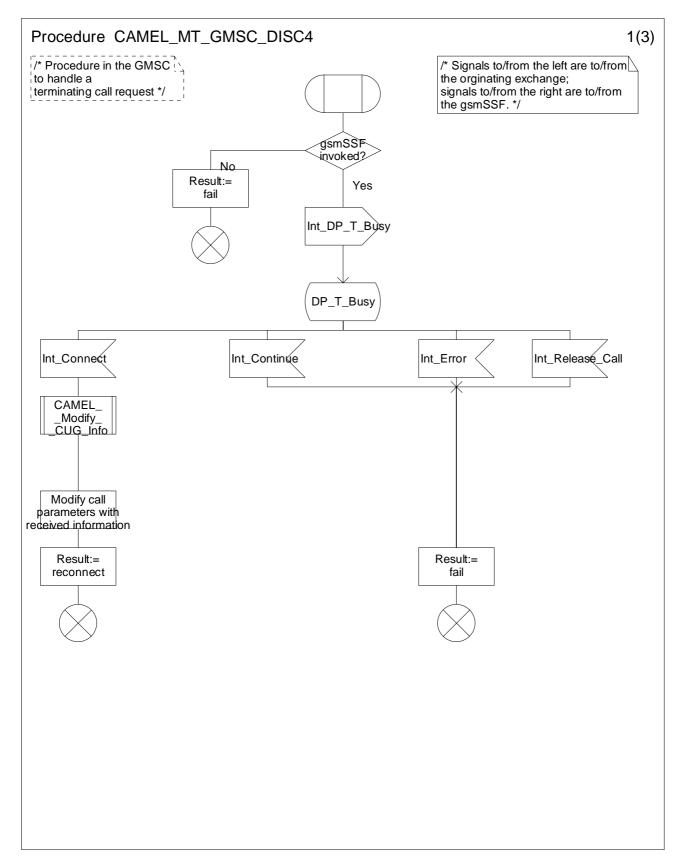
Figure 4.35a: Procedure CAMEL\_MT\_GMSC\_DISC4 (sheet 1)
