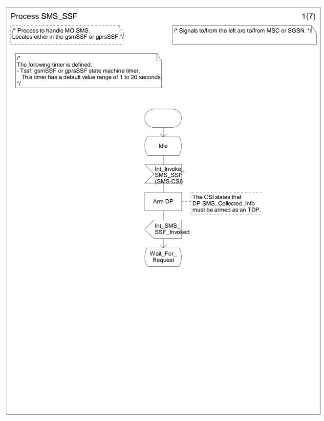
Figure 7.10a: Process SMS\_SSF (sheet 1)
