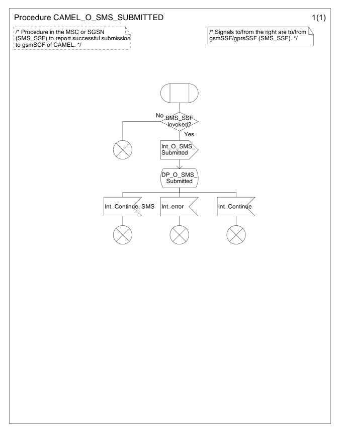
Figure 7.8: Procedure CAMEL\_O\_SMS\_SUBMITTED (sheet 1)
