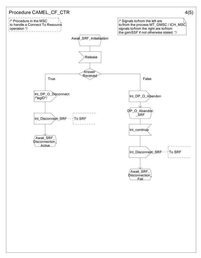
Figure 4.62d: Procedure CAMEL\_CF\_CTR (sheet 4)
