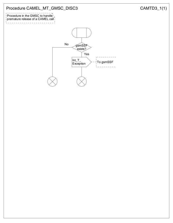
Figure 4.34: Procedure CAMEL\_MT\_GMSC\_DISC3 (sheet 1)
