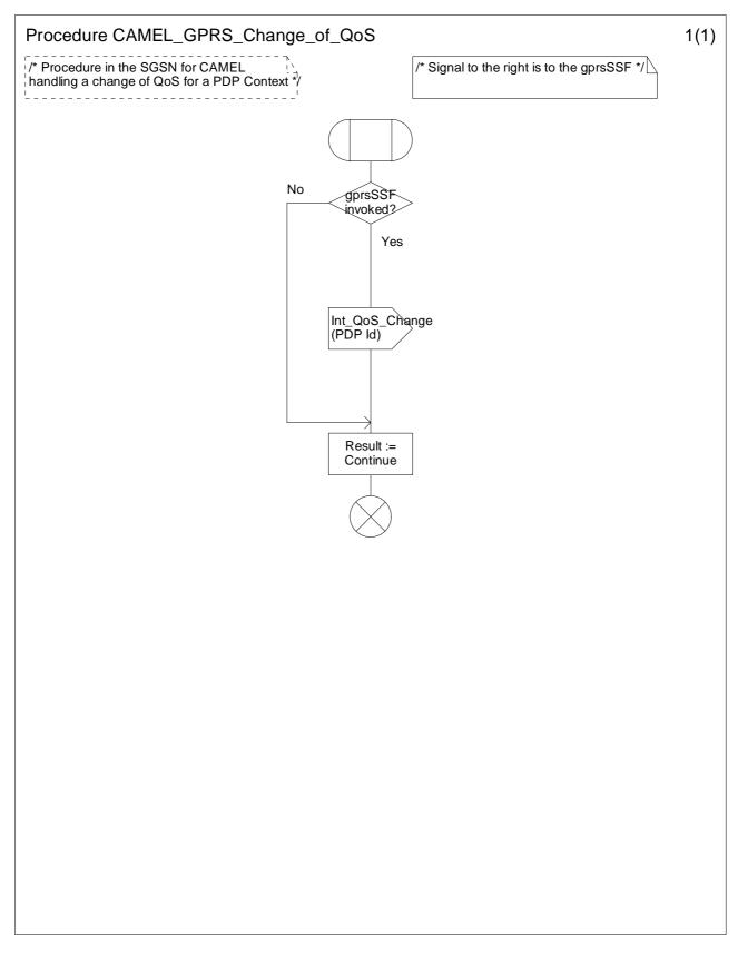
Figure 6.14: Procedure CAMEL\_GPRS\_Change\_Of\_QoS (sheet 1)
