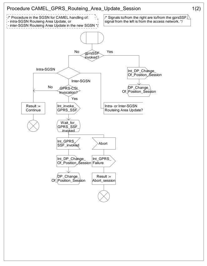
Figure 6.10a: Procedure CAMEL\_GPRS\_Routeing\_Area\_Update\_Session (sheet 1)
