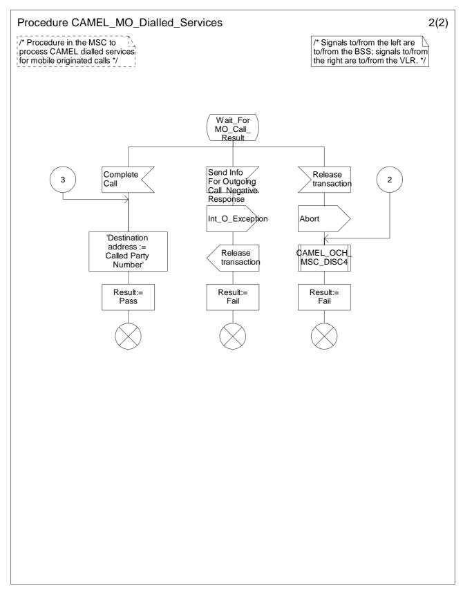
Figure 4.9b: Procedure CAMEL\_MO\_Dialled\_Services (sheet 2)
