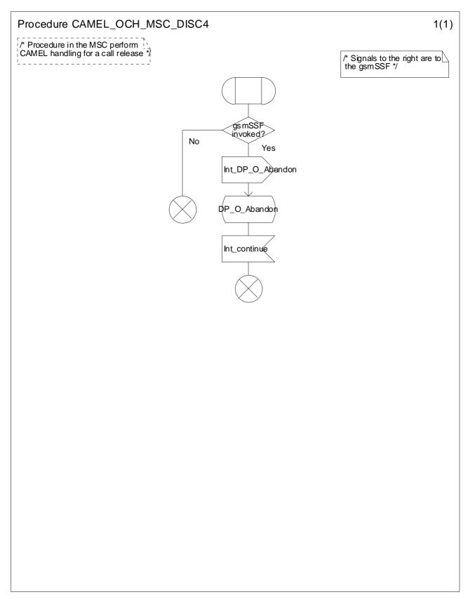
Figure 4.19: Procedure CAMEL\_OCH\_MSC\_DISC4 (sheet 1)
