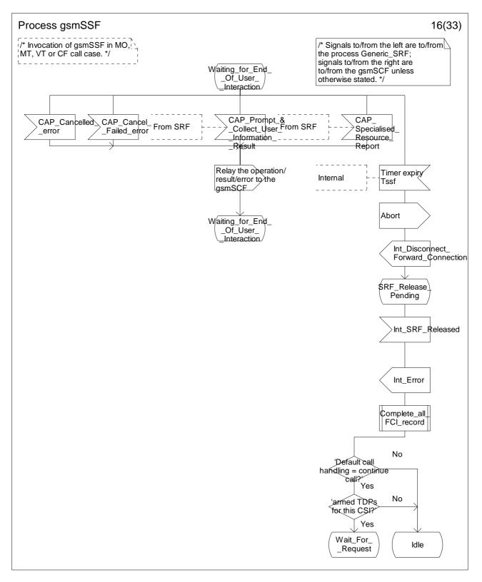
Figure 4.64p: Process gsmSSF (sheet 16)
