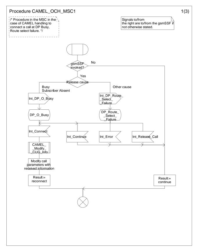
Figure 4.14a: Procedure CAMEL\_OCH\_MSC1 (sheet 1)
