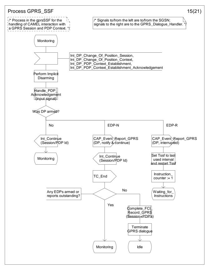
Figure 6.17o: Process GPRS\_SSF (sheet 15)
