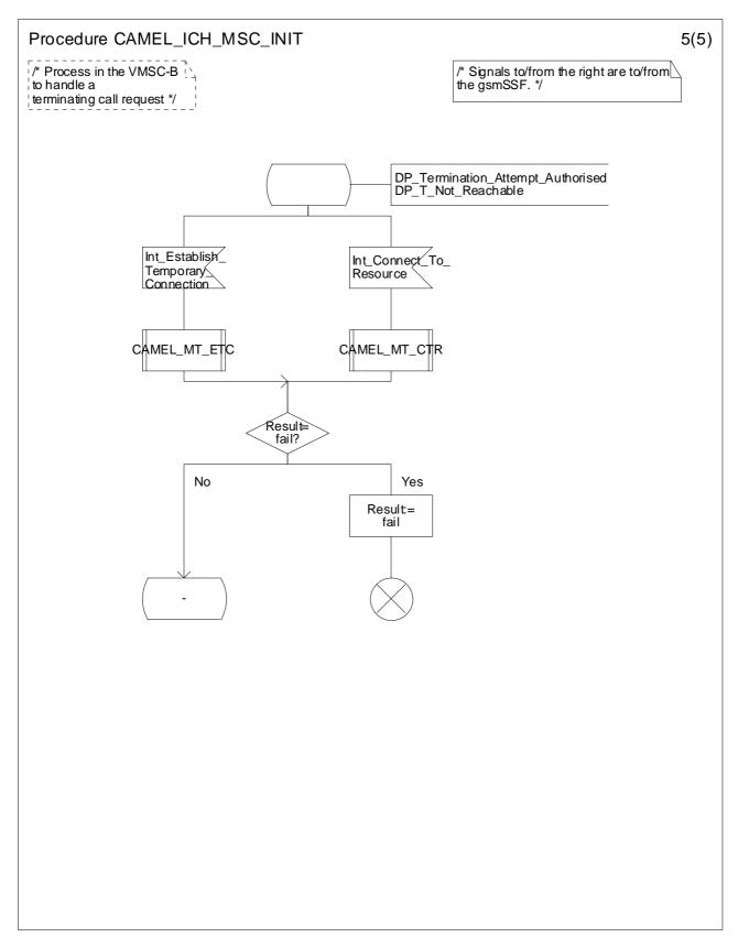
Figure 4.52e: Procedure CAMEL\_ICH\_MSC\_INIT (sheet 5)
