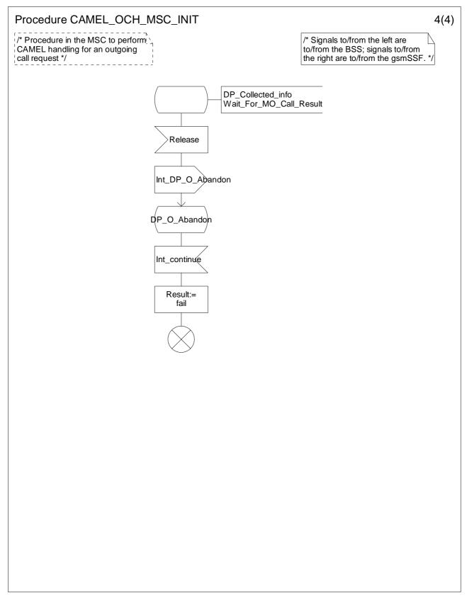
Figure 4.10d: Procedure CAMEL\_OCH\_MSC\_INIT (sheet 4)
