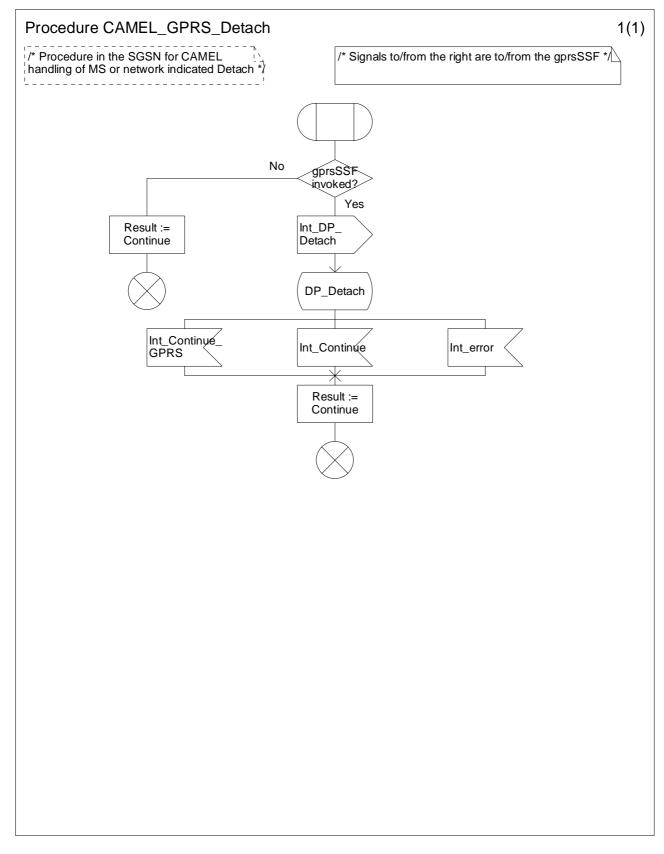
Figure 6.9: Procedure CAMEL\_GPRS\_Detach (sheet 1)
