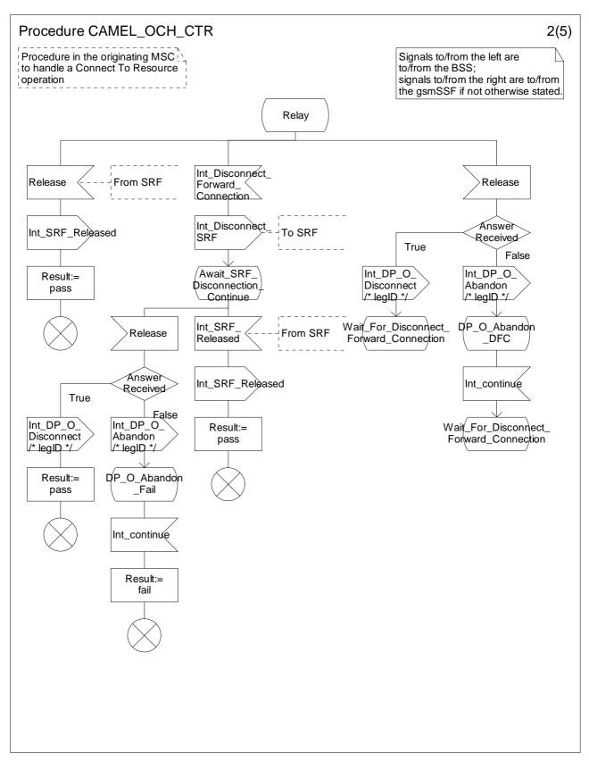
Figure 4.21b: Procedure CAMEL\_OCH\_CTR (sheet 2)
