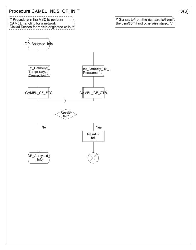
Figure 4.59c: Procedure CAMEL\_NDS\_CF\_INIT (sheet 3)
