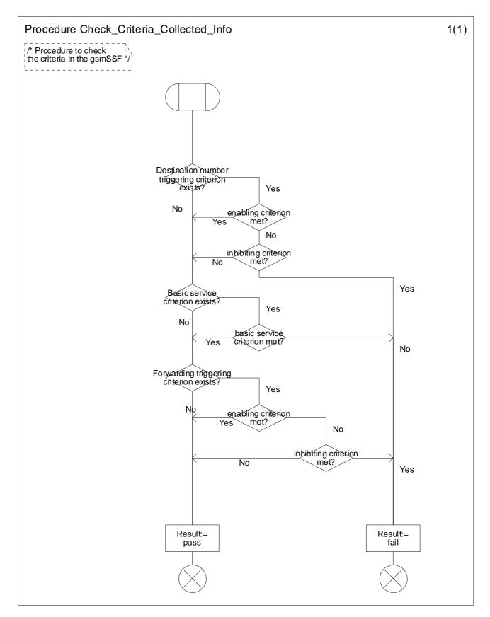
Figure 4.65: Procedure Check\_Criteria\_Collected\_Info(sheet 0)
