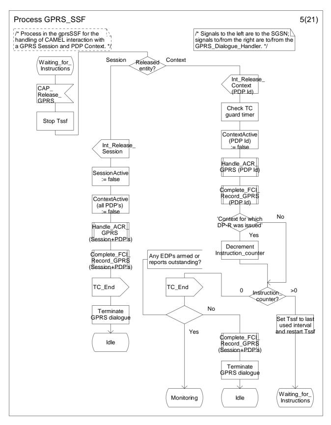
Figure 6.17e: Process GPRS\_SSF (sheet 5)
