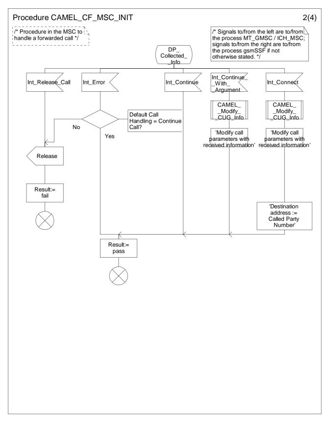
Figure 4.57b: Procedure CAMEL\_CF\_MSC\_INIT (sheet 2)
