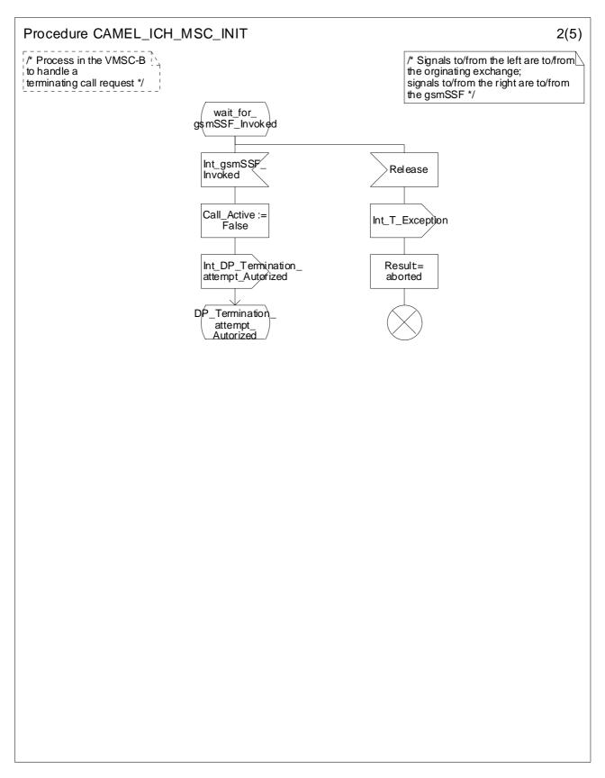
Figure 4.52b: Procedure CAMEL\_ICH\_MSC\_INIT (sheet 2)
