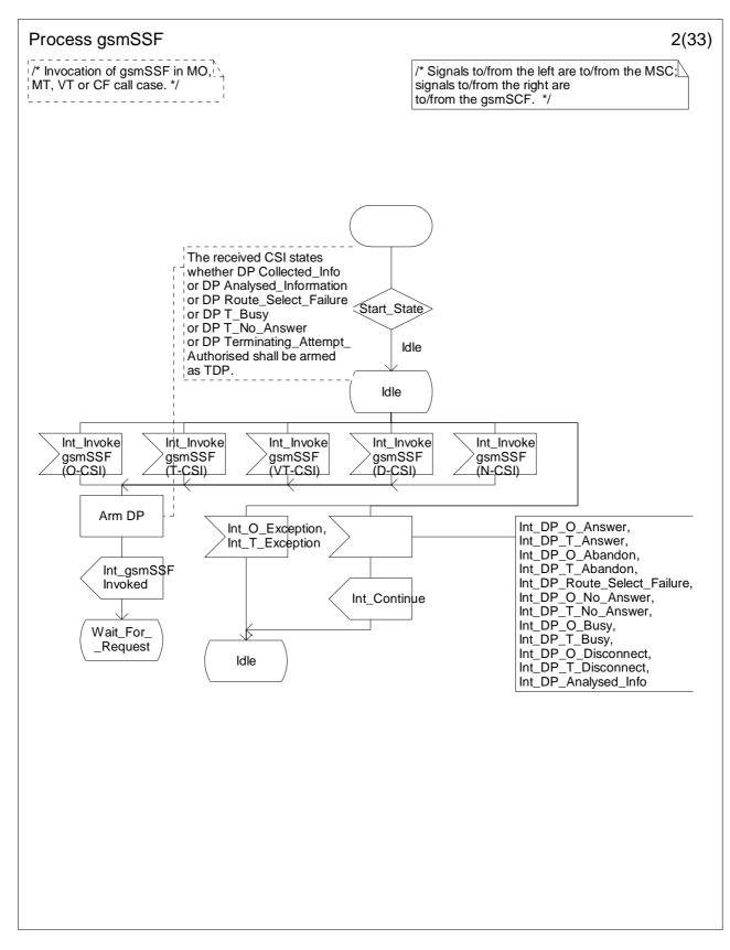
Figure 4.64b: Process gsmSSF (sheet 2)
