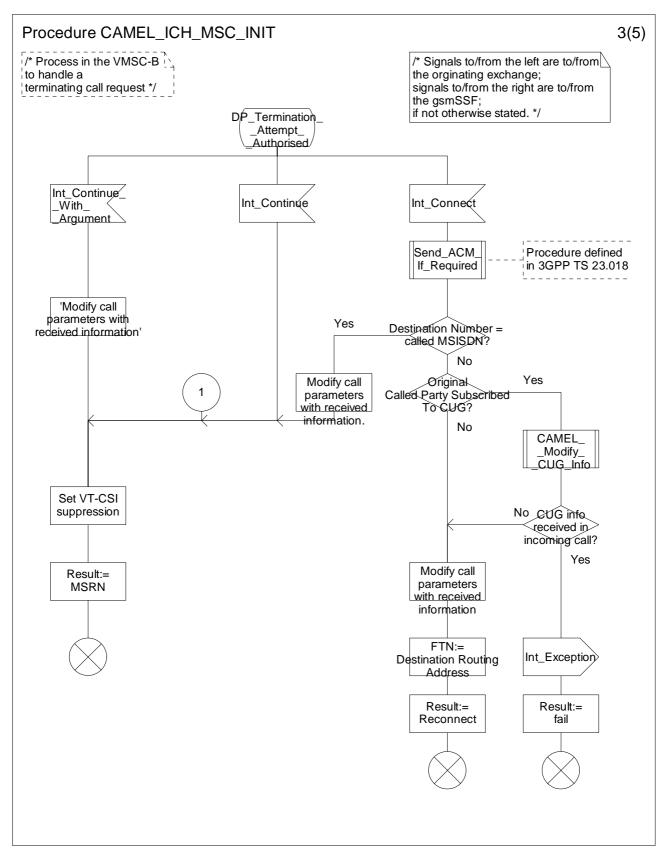
Figure 4.52c: Procedure CAMEL\_ICH\_MSC\_INIT (sheet 3)
