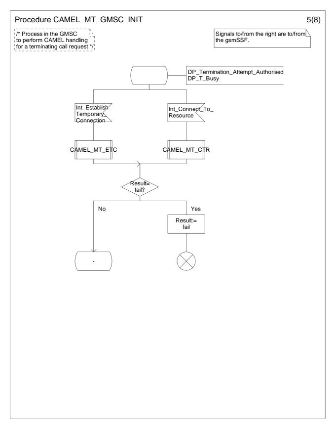
Figure 4.30e: Procedure CAMEL\_MT\_GMSC\_INIT (sheet 5)
