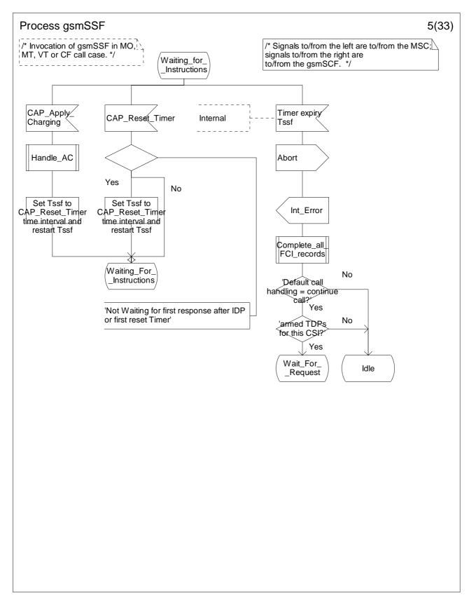
Figure 4.64e: Process gsmSSF (sheet 5)
