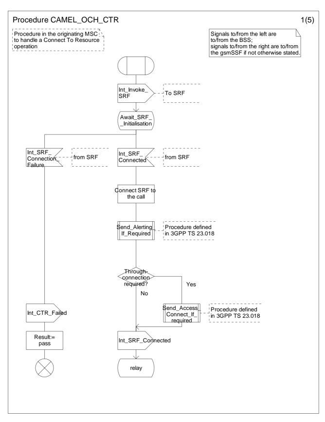
Figure 4.21a: Procedure CAMEL\_OCH\_CTR (sheet 1)
