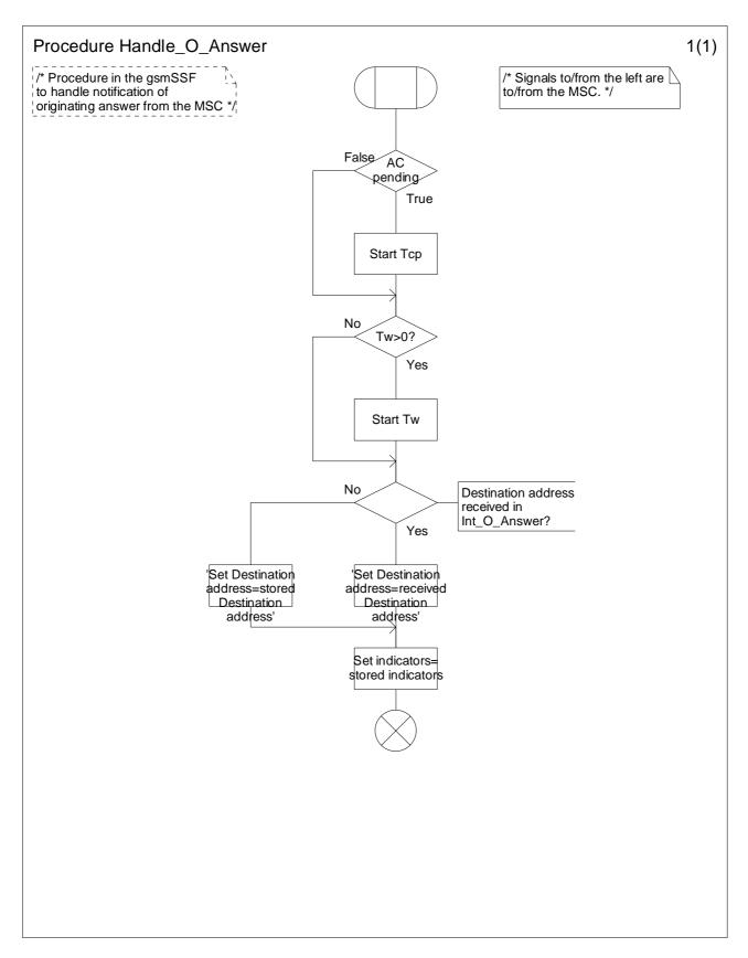
Figure 4.75: Procedure Handle\_O\_Answer (sheet 1)
