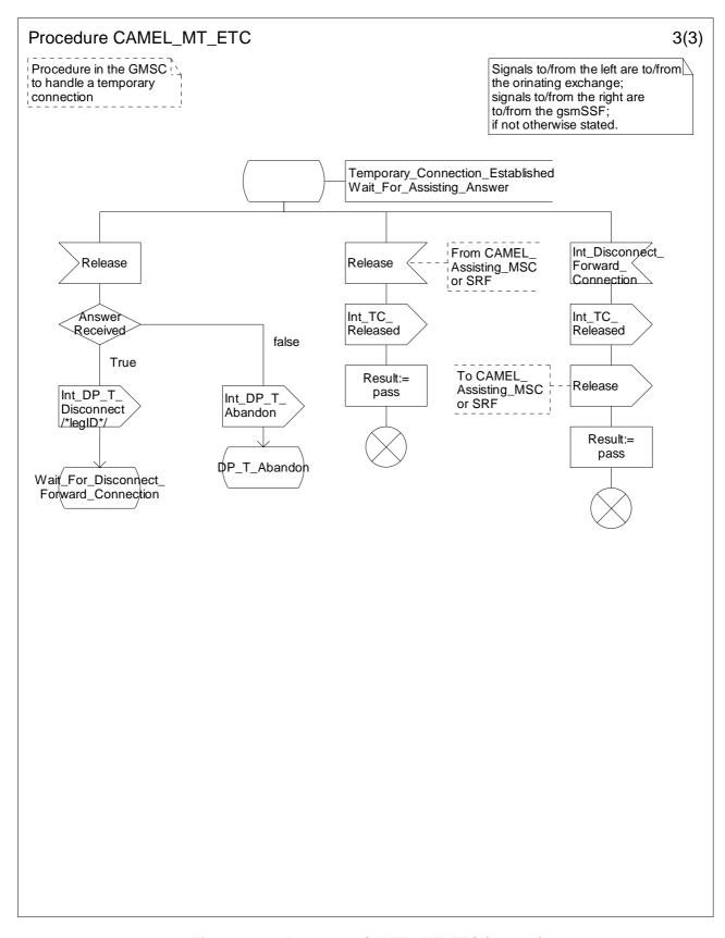
Figure 4.38c: Procedure CAMEL\_MT\_ETC (sheet 3)
