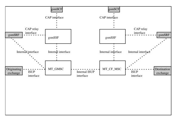
Figure 4.8c: Terminating GMSC case (gsmSSF relay)
