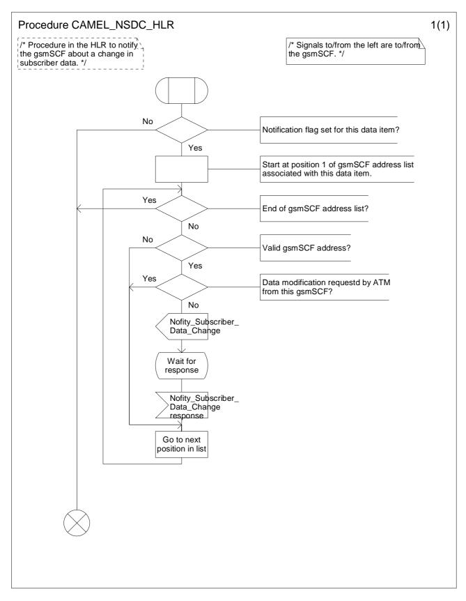
Figure 10.8: Procedure CAMEL\_NSDC\_HLR (sheet1)
