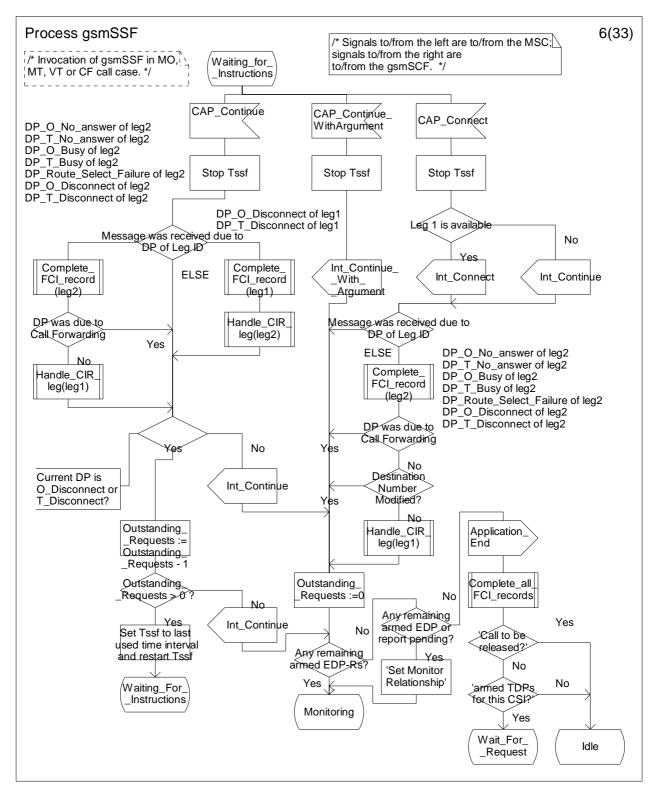
Figure 4.64f: Process gsmSSF (sheet 6)
