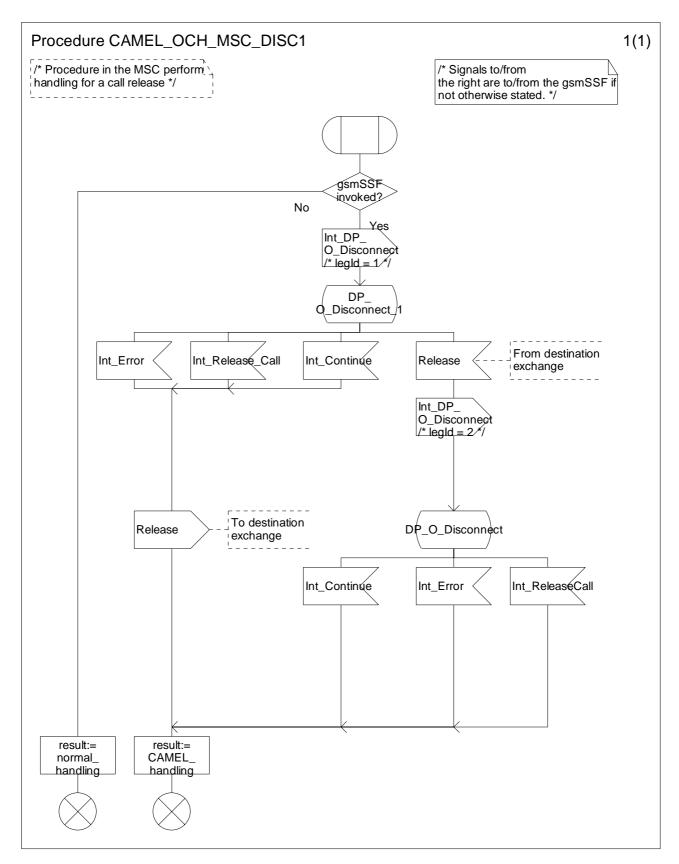
Figure 4.16: Procedure CAMEL\_OCH\_MSC\_DISC1 (sheet 1)
