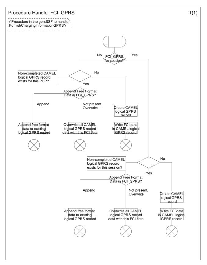
Figure 6.21: Procedure Handle\_FCI\_GPRS (sheet 0)
