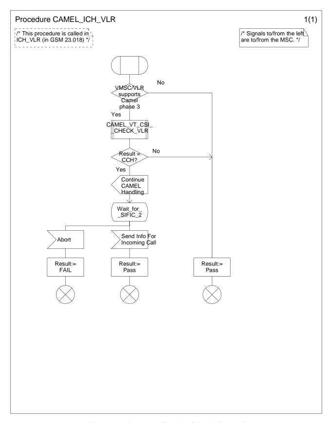
Figure 4.48: Procedure CAMEL\_ICH\_VLR (sheet 1)
