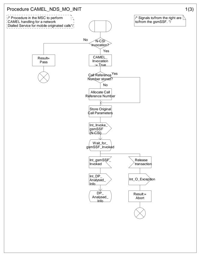
Figure 4.12a: Procedure CAMEL\_NDS\_MO\_INIT (sheet 1)
