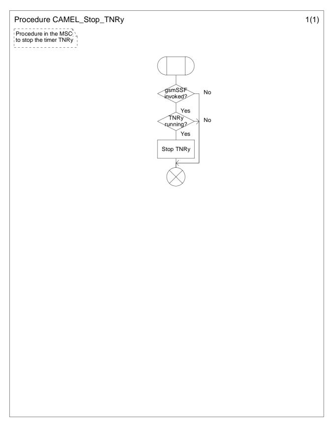
Figure 4.23: Procedure CAMEL\_Stop\_TNRy (sheet 1)
