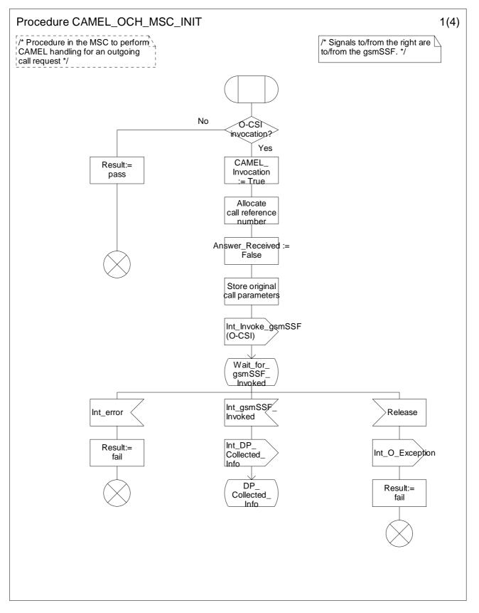
Figure 4.10a: Procedure CAMEL\_OCH\_MSC\_INIT (sheet 1)
