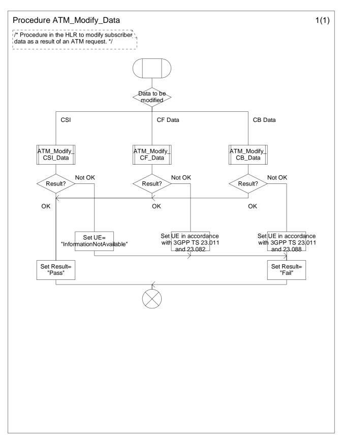
Figure 10.4: Procedure ATM\_Modify\_Data (sheet 1)
