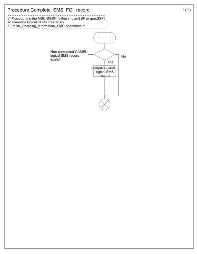
Figure 7.11: Procedure Complete\_SMS\_FCI\_record (sheet 1)
