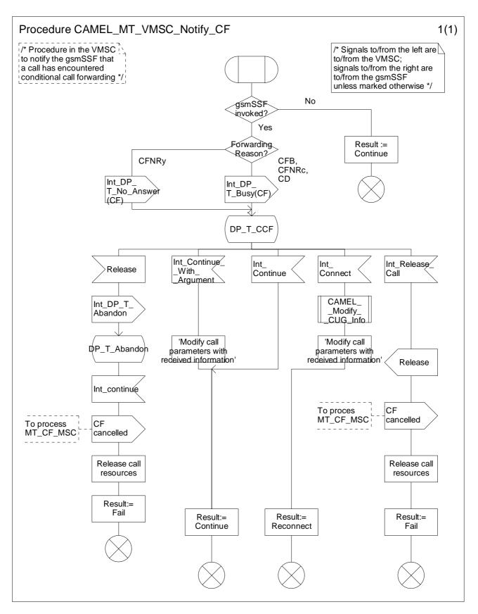
Figure 4.53: Procedure CAMEL\_MT\_VMSC\_Notify\_CF (sheet 0)
