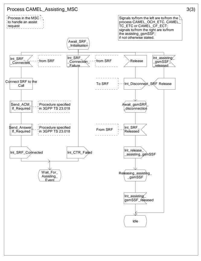
Figure 4.80c: Process CAMEL\_Assisting\_MSC (sheet 3)
