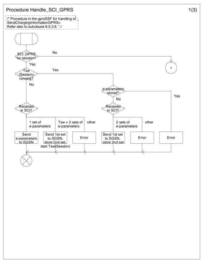
Figure 6.23a: Procedure Handle\_SCI\_GPRS (sheet 1)
