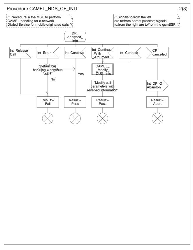
Figure 4.59b: Procedure CAMEL\_NDS\_CF\_INIT (sheet 2)
