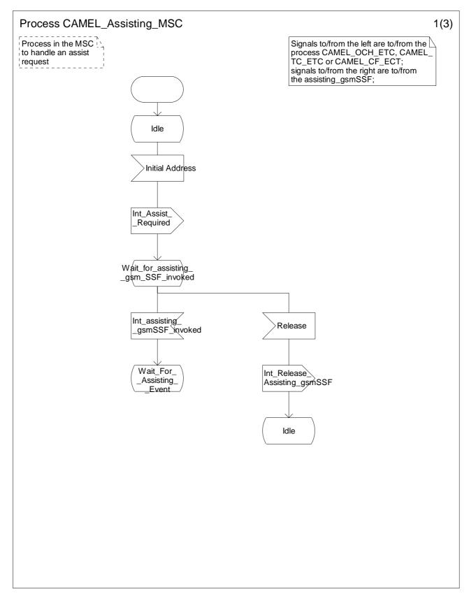
Figure 4.80a: Process CAMEL\_Assisting\_MSC (sheet 1)
