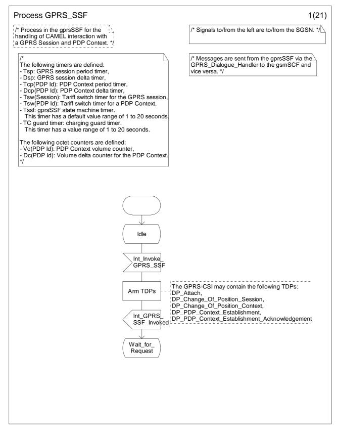
Figure 6.17a: Process GPRS\_SSF (sheet 1)
