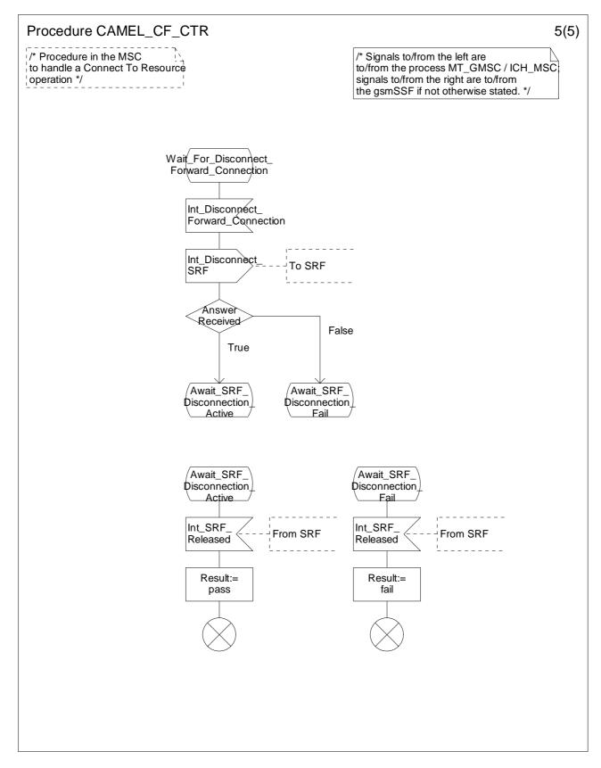
Figure 4.62e: Procedure CAMEL\_CF\_CTR (sheet 5)
