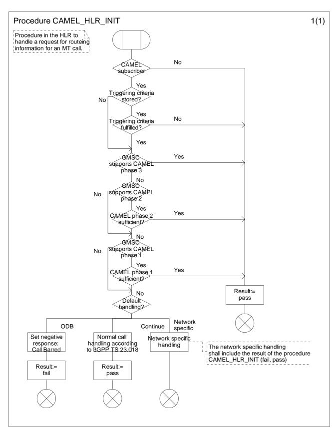
Figure 4.41: Procedure CAMEL\_HLR\_INIT (sheet 1)
