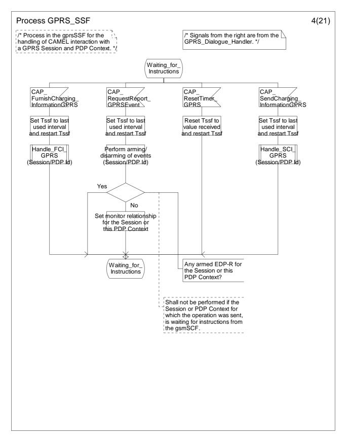
Figure 6.17d: Process GPRS\_SSF (sheet 4)
