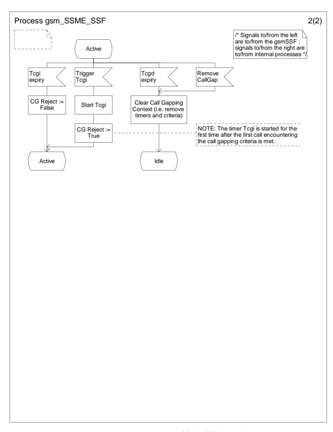
Figure 4.77b: Process gsm\_SSME\_SSF (sheet 2)
