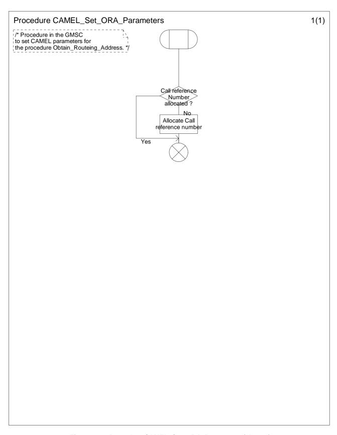
Figure 4.29: Procedure CAMEL\_Set\_ORA\_Parameters (sheet 1)
