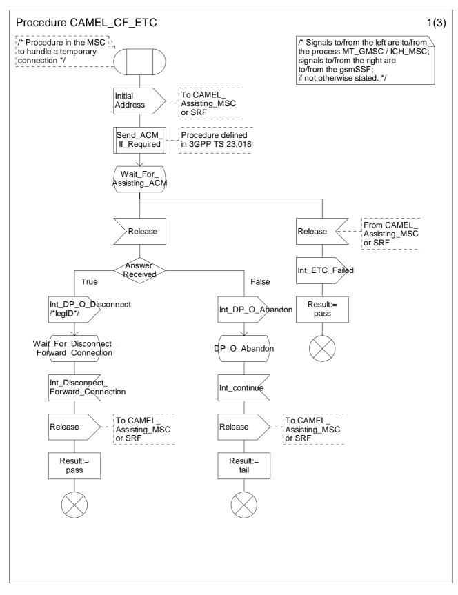
Figure 4.61a: Process CAMEL\_CF\_ETC (sheet 1)
