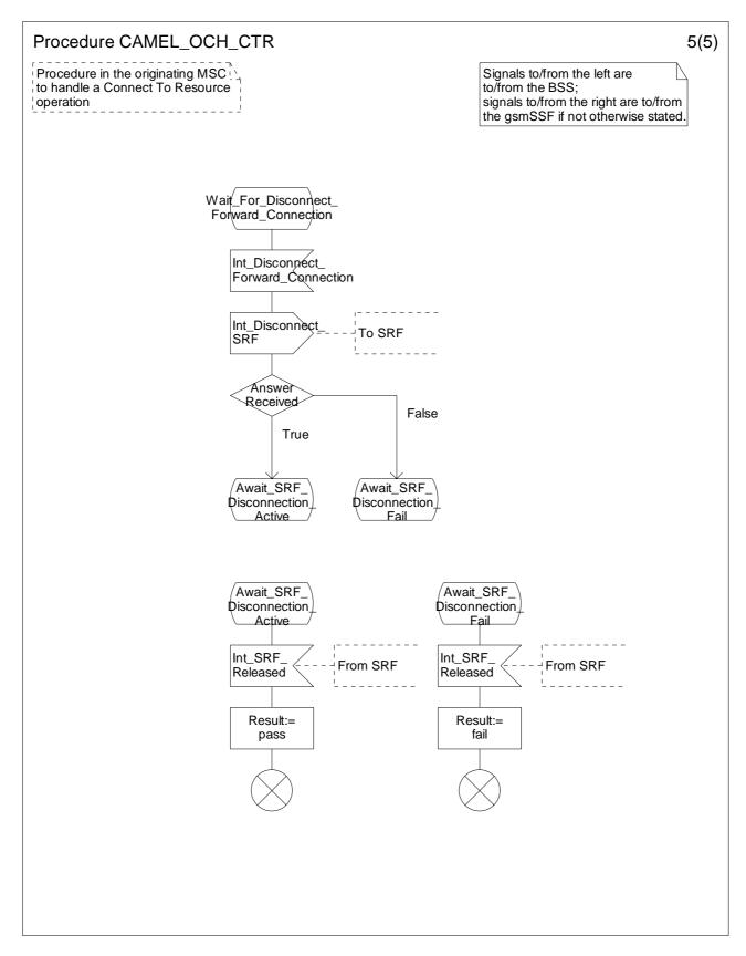
Figure 4.21e: Procedure CAMEL\_OCH\_CTR (sheet 5)
