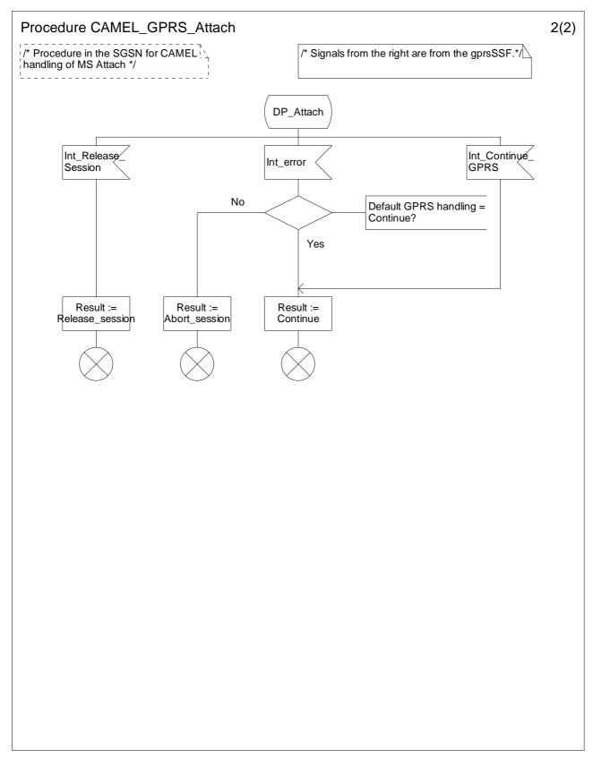
Figure 6.8b: Procedure CAMEL\_GPRS\_Attach (sheet 2)
