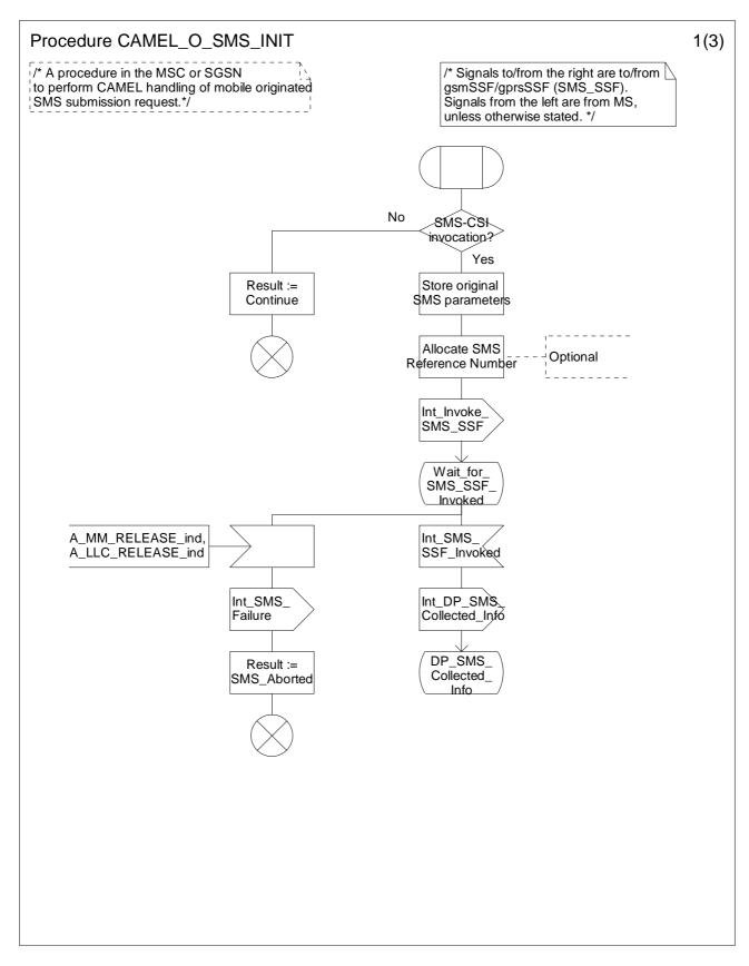
Figure 7.7a: Procedure CAMEL\_O\_SMS\_INIT (sheet 1)
