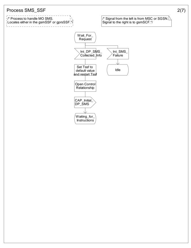
Figure 7.10b: Process SMS\_SSF (sheet 2)
