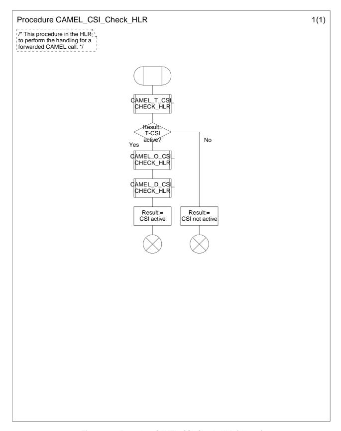
Figure 4.42: Procedure CAMEL\_CSI\_Check\_HLR (sheet 1)
