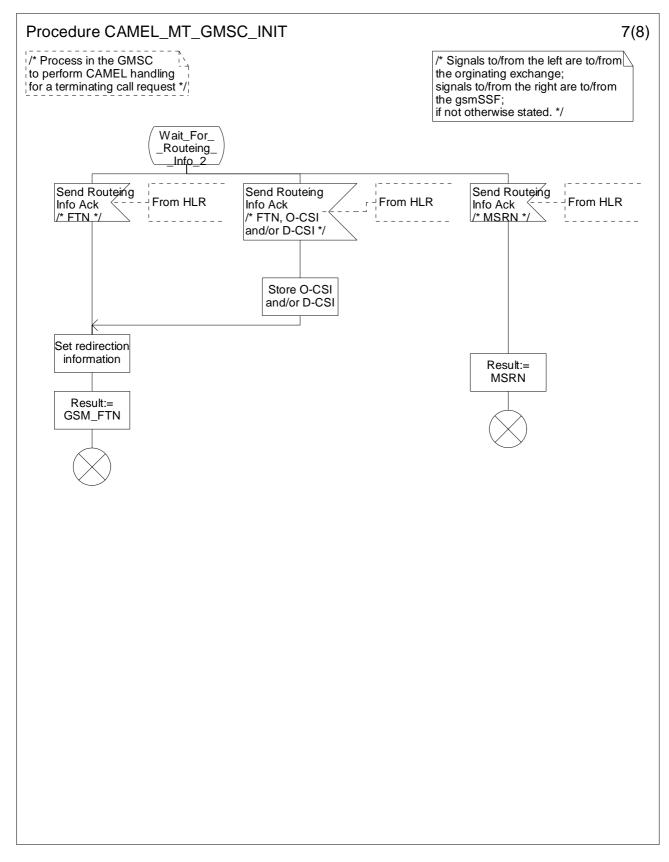
Figure 4.30g: Procedure CAMEL\_MT\_GMSC\_INIT (sheet 7)
