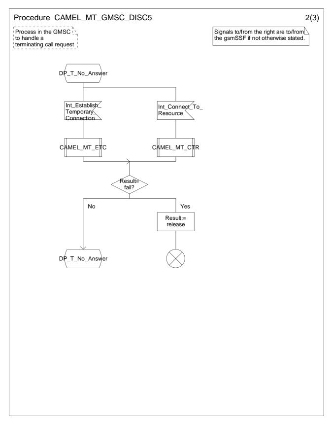
Figure 4.36b: Procedure CAMEL\_MT\_GMSC\_DISC5 (sheet 2)
