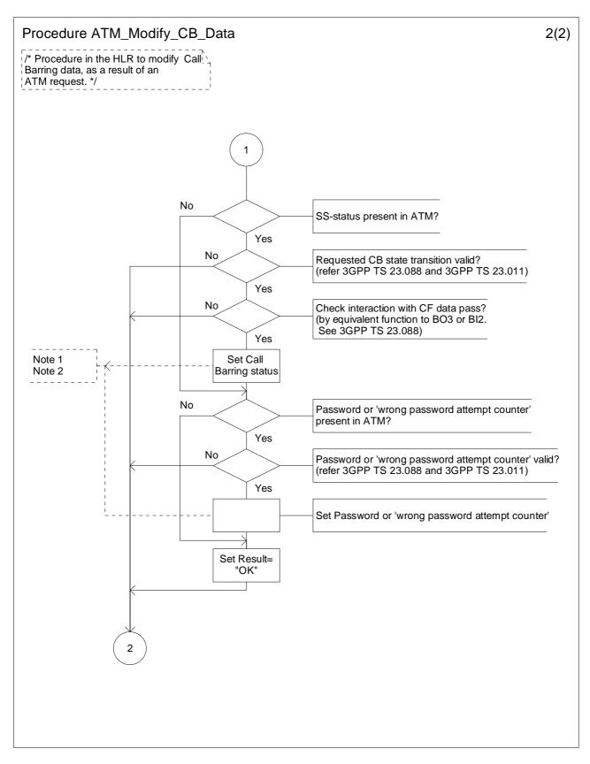
Figure 10.7b: Procedure ATM\_Modify\_CB\_Data (sheet 2)
