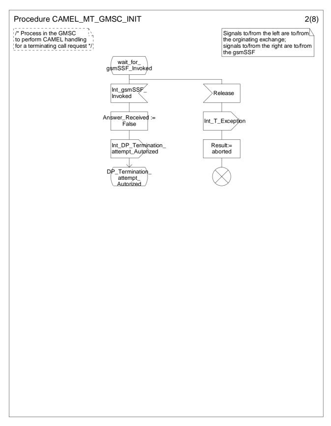
Figure 4.30b: Procedure CAMEL\_MT\_GMSC\_INIT (sheet 2)
