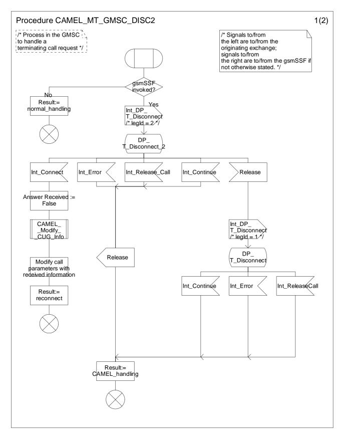
Figure 4.33a: Procedure CAMEL\_MT\_GMSC\_DISC2 (sheet 1)
