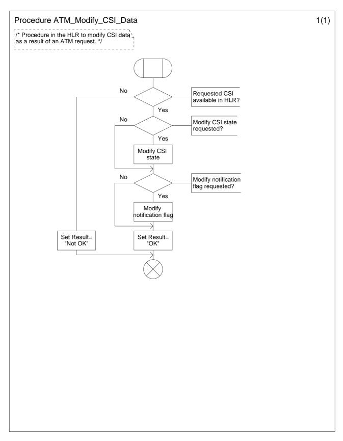
Figure 10.5: Procedure ATM\_Modify\_CSI\_Data (sheet 1)
