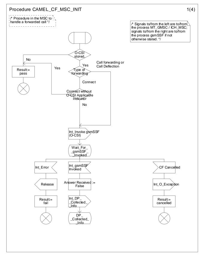
Figure 4.57a: Procedure CAMEL\_CF\_MSC\_INIT (sheet 1)
