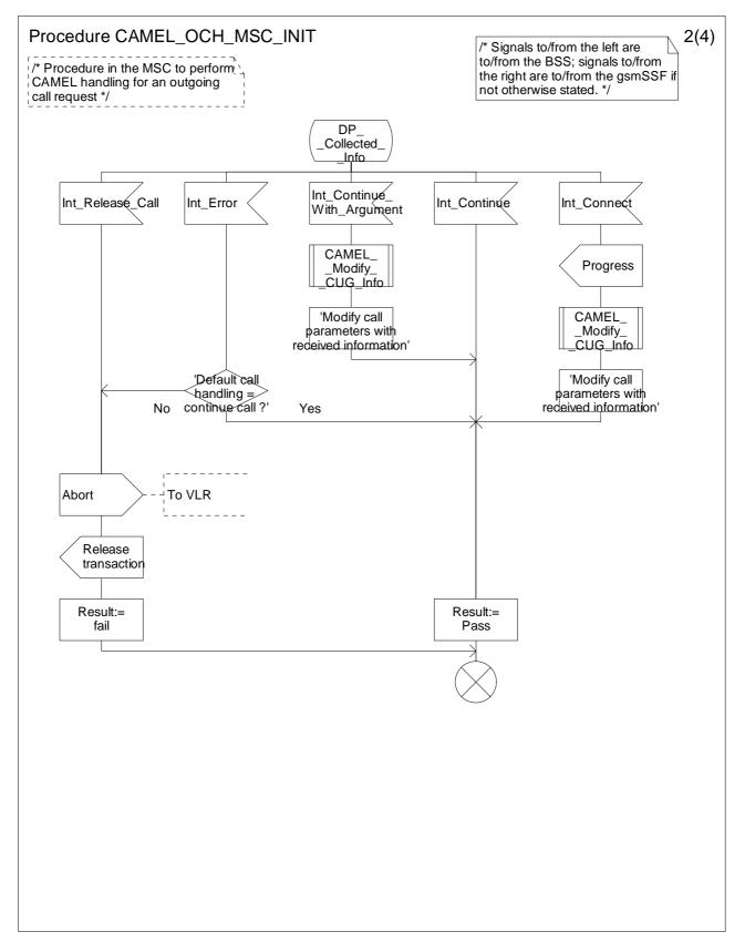
Figure 4.10b: Procedure CAMEL\_OCH\_MSC\_INIT (sheet 2)
