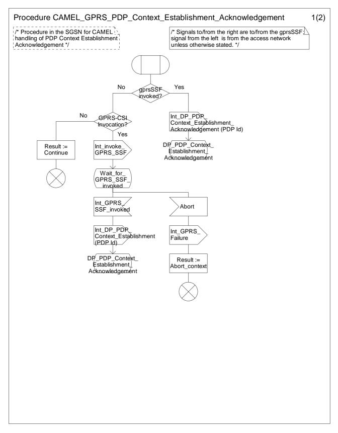
Figure 6.13a: Procedure CAMEL\_GPRS\_PDP\_Context\_Establishment\_Acknowledgement (sheet 1)
