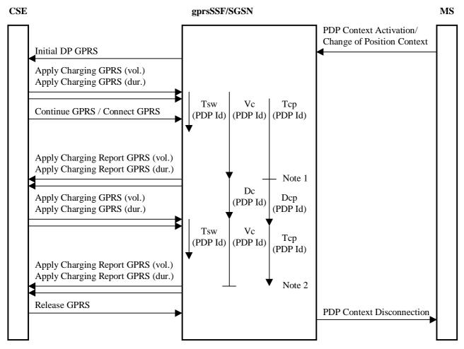
NOTE 1: Vc threshold reached, Tcp is stopped. NOTE 2: Tcp time out, Vc is stopped.
