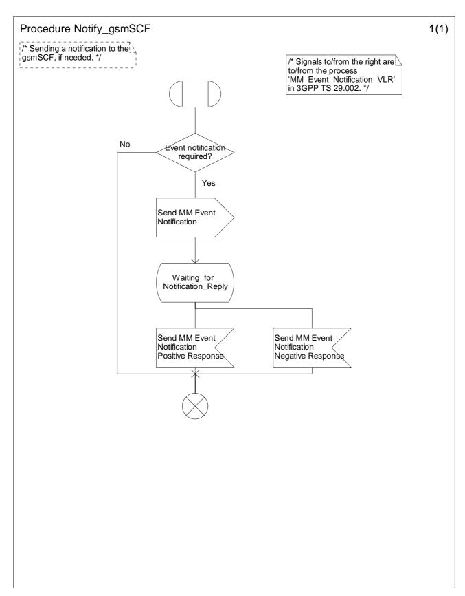
Figure 9.4: Procedure Notify\_gsmSCF (sheet 1)
