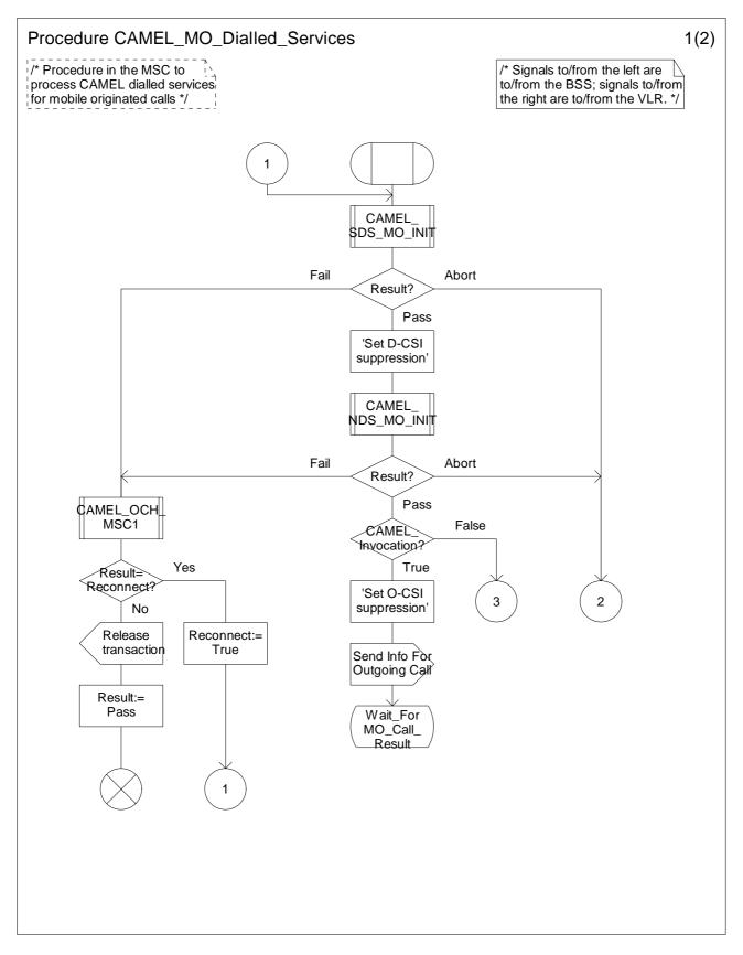
Figure 4.9a: Procedure CAMEL\_MO\_Dialled\_Services (sheet 1)
