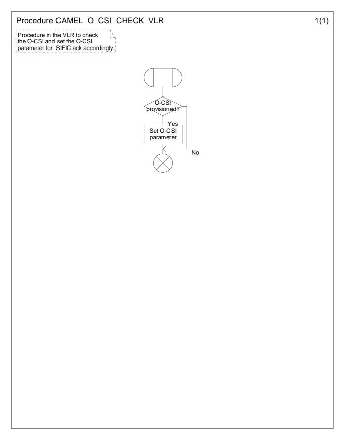
Figure 4.49: Procedure CAMEL\_O\_CSI\_Check\_VLR (sheet 1)
