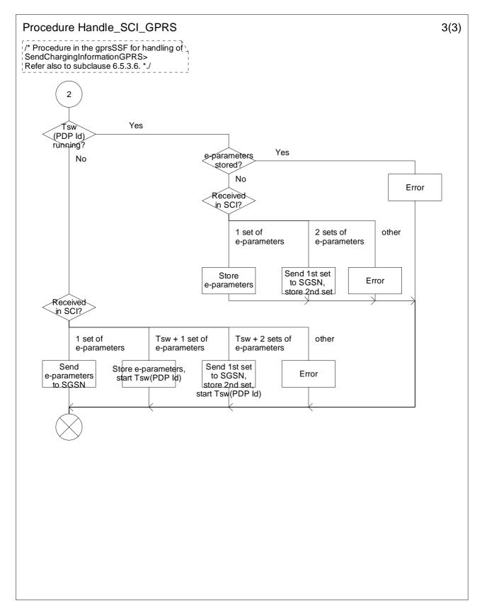
Figure 6.23c: Procedure Handle\_SCI\_GPRS (sheet 3)
