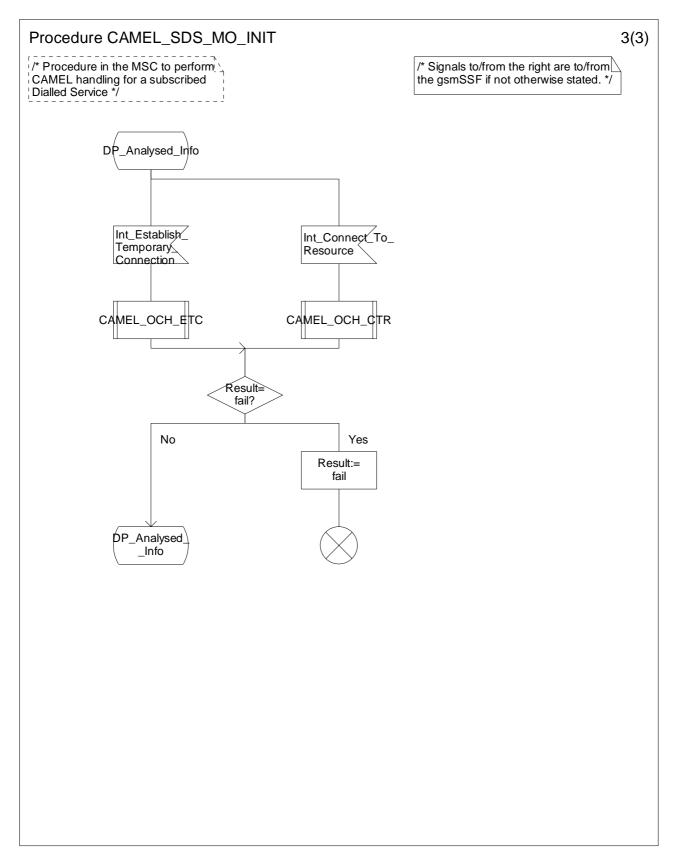
Figure 4.11c: Procedure CAMEL\_SDS\_MO\_INIT (sheet 3)
