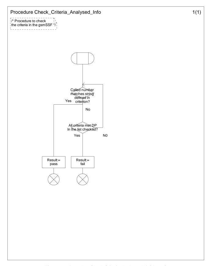
Figure 4.66: Procedure Check\_Criteria\_Analysed\_Info(sheet 0)
