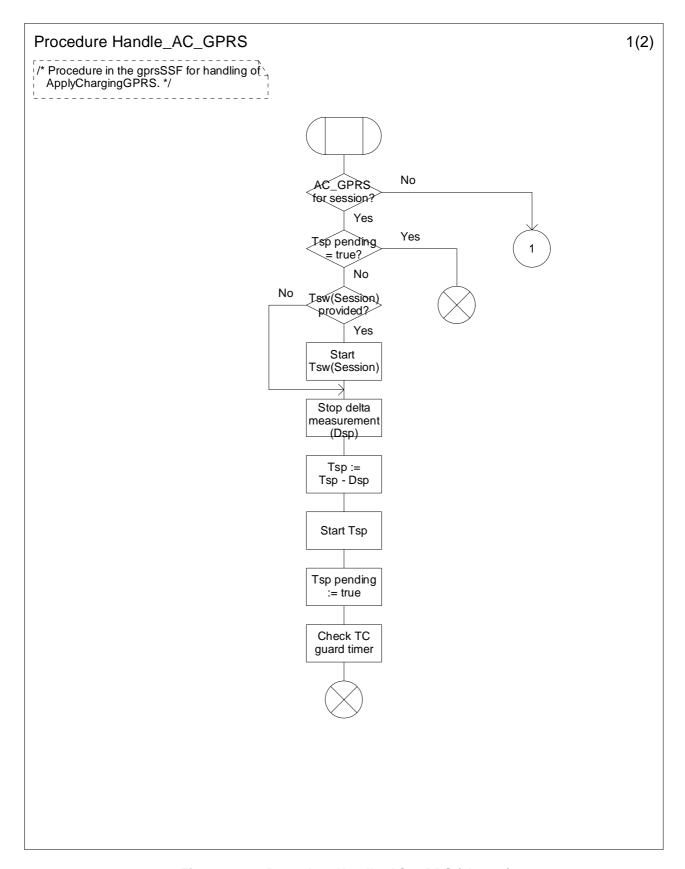
Figure 6.19a: Procedure Handle\_AC\_GPRS (sheet 1)
