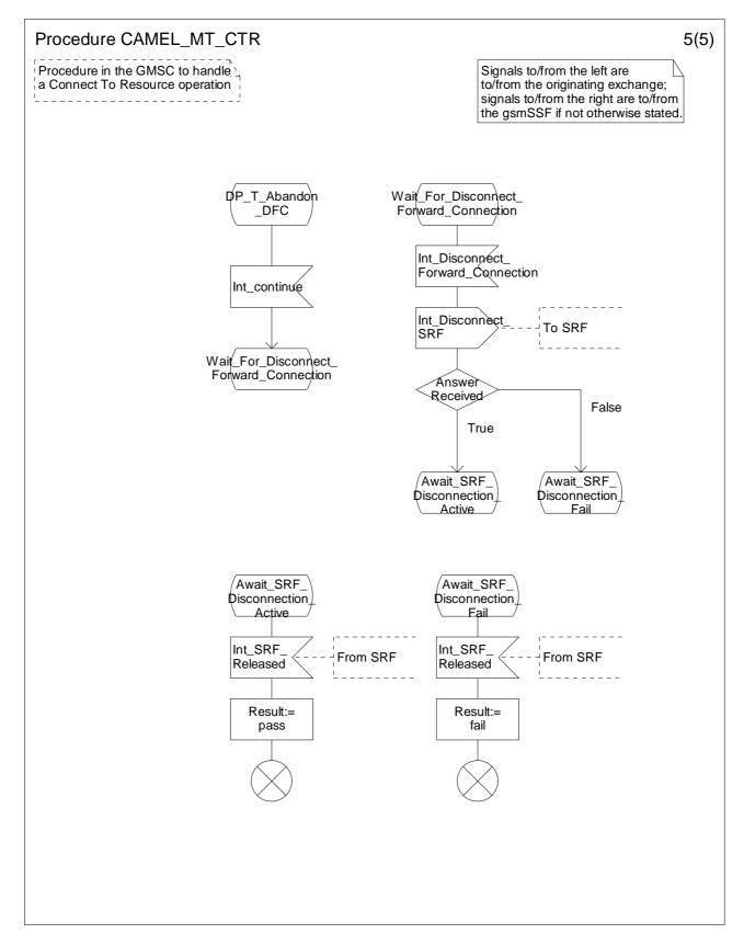
Figure 4.39e: Procedure CAMEL\_MT\_CTR (sheet 5)
