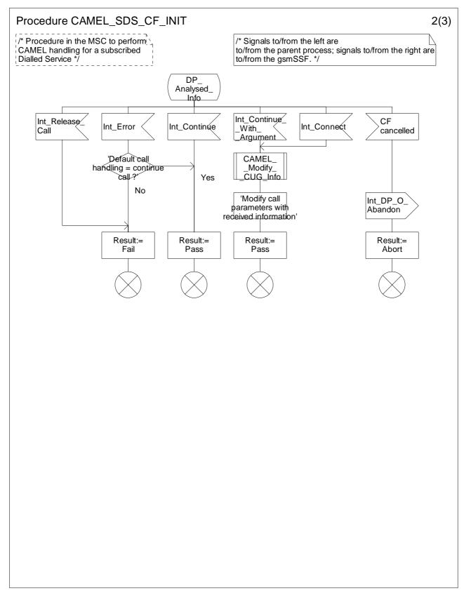
Figure 4.58b: Procedure CAMEL\_SDS\_CF\_INIT (sheet 2)
