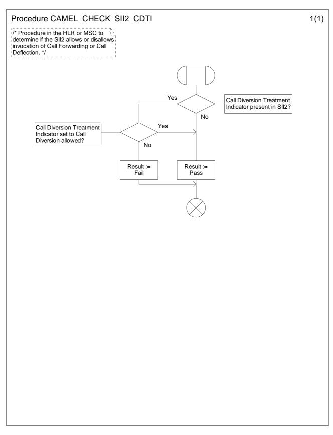
Figure 4.46: Procedure CAMEL\_CHECK\_SII2\_CDTI (sheet 1)
