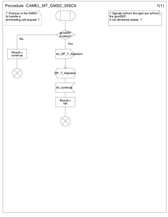
Figure 4.37: Procedure CAMEL\_MT\_GMSC\_DISC6 (sheet 1)
