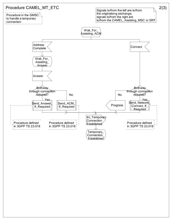
Figure 4.38b: Procedure CAMEL\_MT\_ETC (sheet 2)
