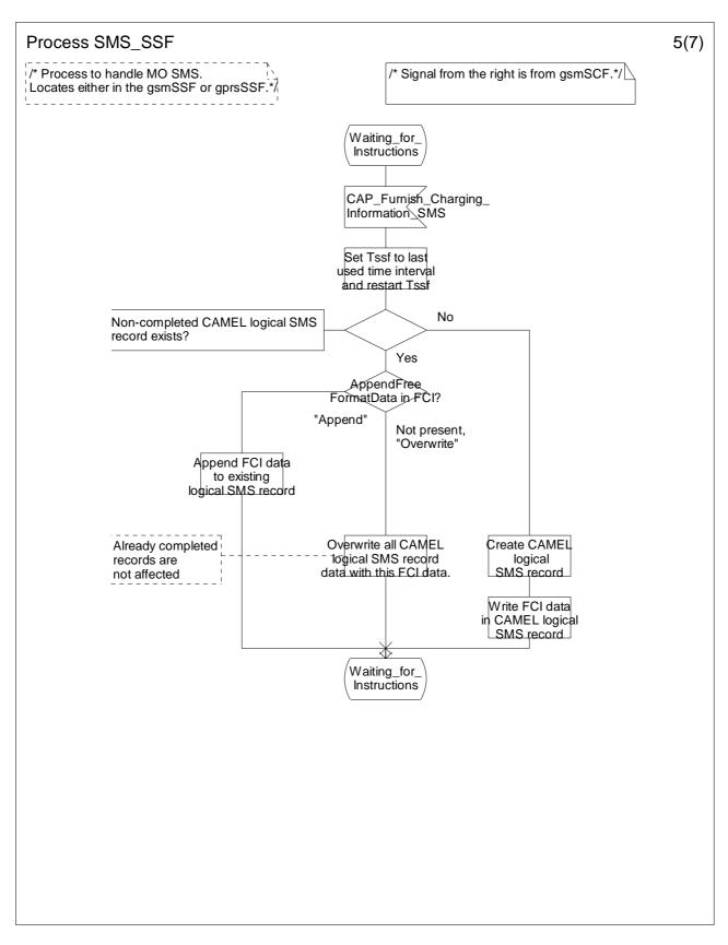
Figure 7.10e: Process SMS\_SSF (sheet 5)
