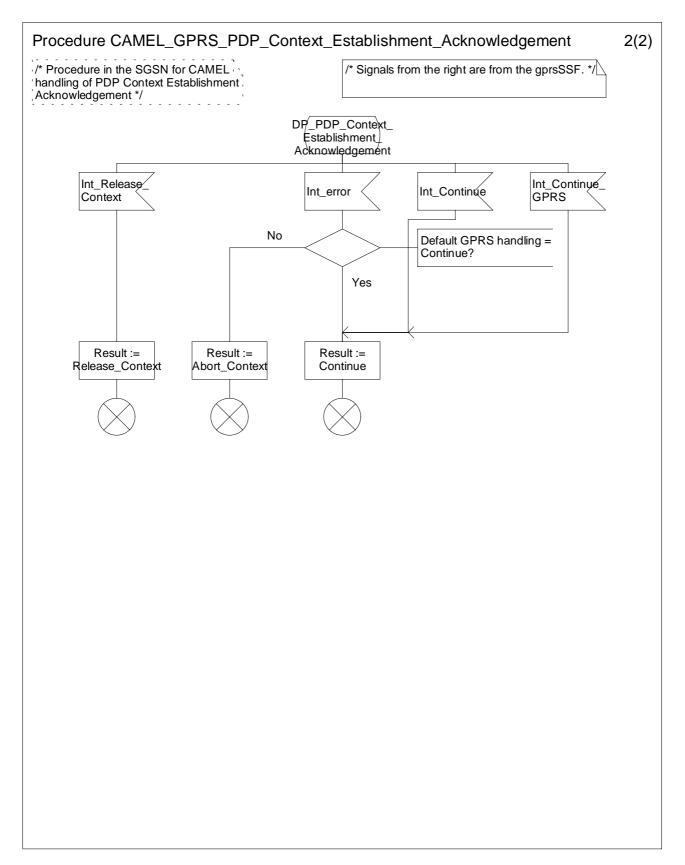
Figure 6.13b: Procedure CAMEL\_GPRS\_PDP\_Context\_Establishment\_Acknowledgement (sheet 2)
