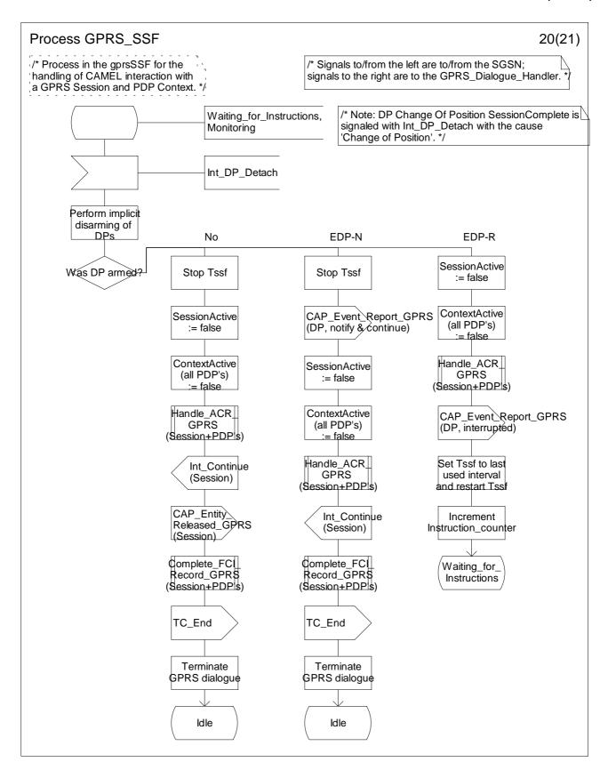
Figure 6.17t: Process GPRS\_SSF (sheet 20)
