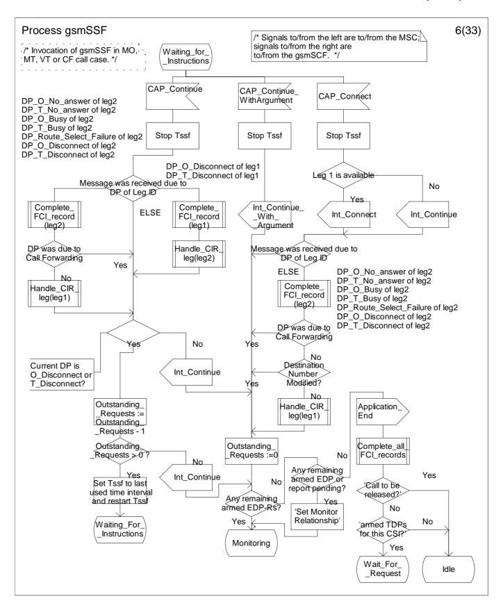
Figure 4.64f: Process gsmSSF (sheet 6)
