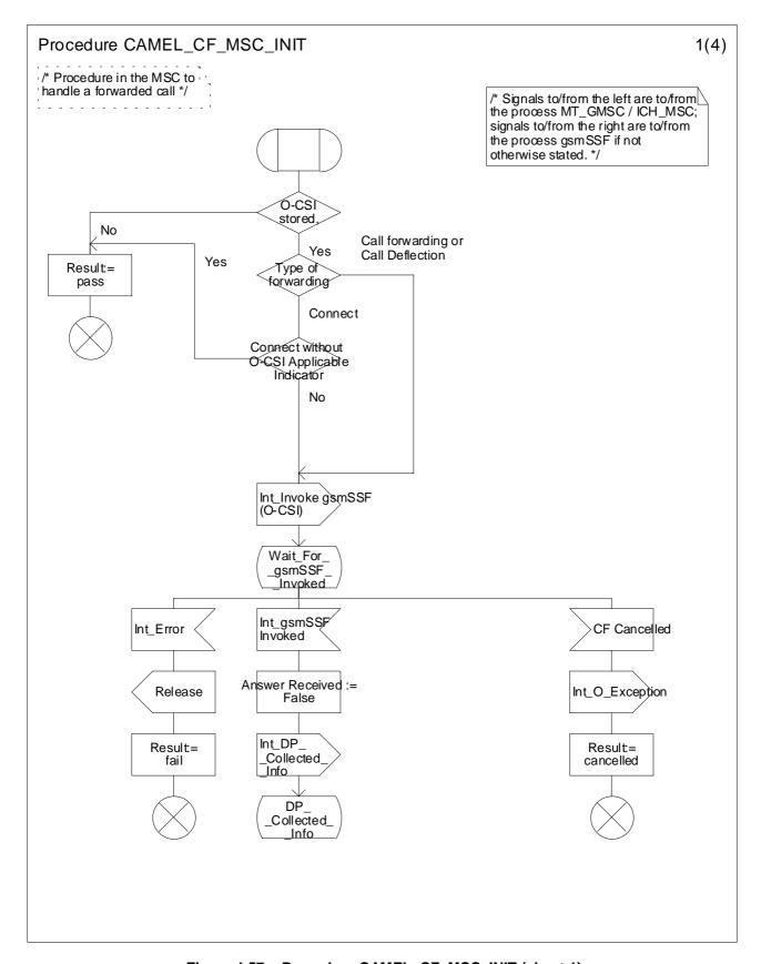
Figure 4.57a: Procedure CAMEL\_CF\_MSC\_INIT (sheet 1)
