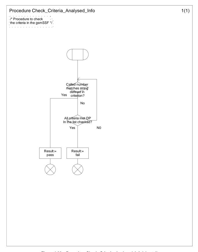
Figure 4.66a: Procedure Check\_Criteria\_Analysed\_Info(sheet 1)
