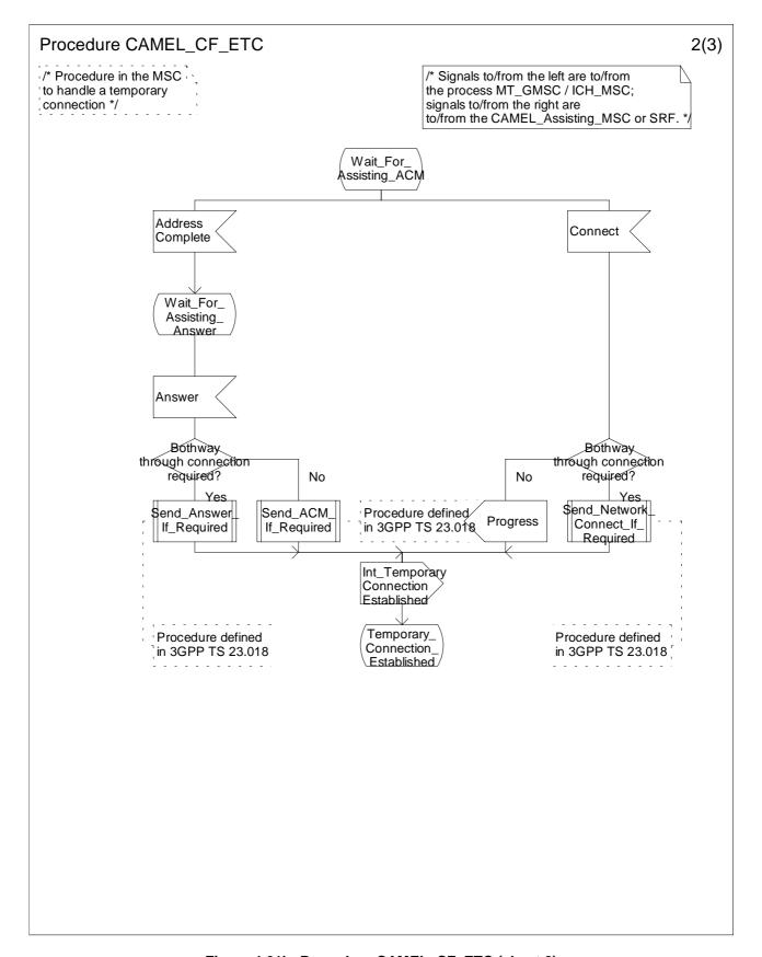
Figure 4.61b: Procedure CAMEL\_CF\_ETC (sheet 2)
