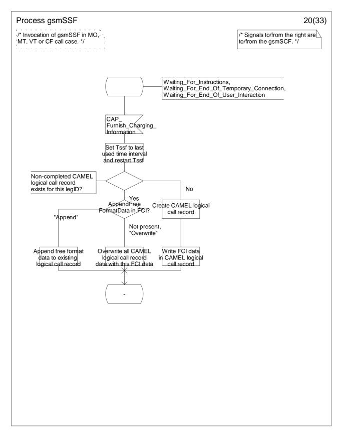
Figure 4.64t: Process gsmSSF (sheet 20)
