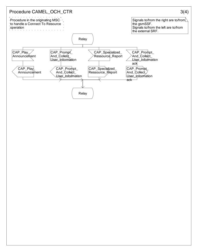
Figure 4.21c: Procedure CAMEL\_OCH\_CTR (sheet 3)
