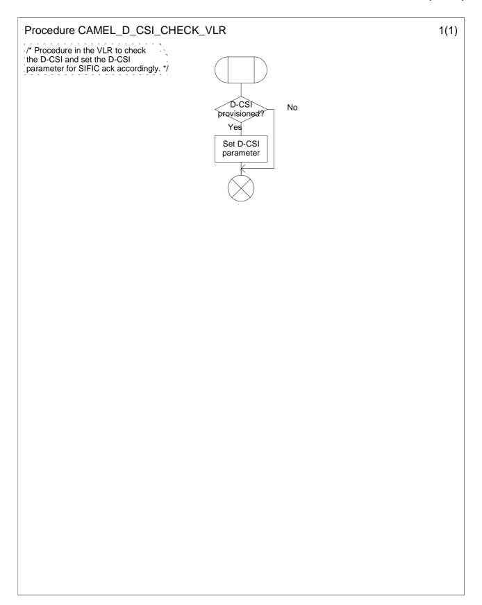
Figure 4.50: Procedure CAMEL\_D\_CSI\_Check\_VLR (sheet 1)
