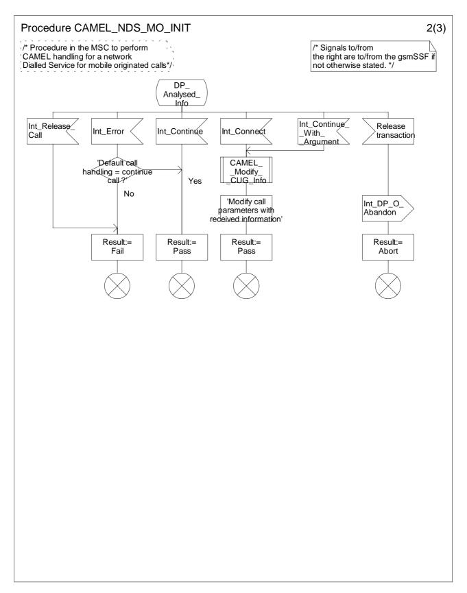
Figure 4.12b: Procedure CAMEL\_NDS\_MO\_INIT (sheet 2)
