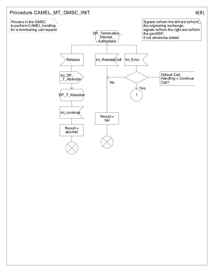
Figure 4.30d: Procedure CAMEL\_MT\_GMSC\_INIT (sheet 4)
