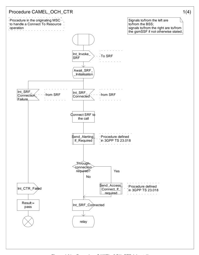
Figure 4.21a: Procedure CAMEL\_OCH\_CTR (sheet 1)
