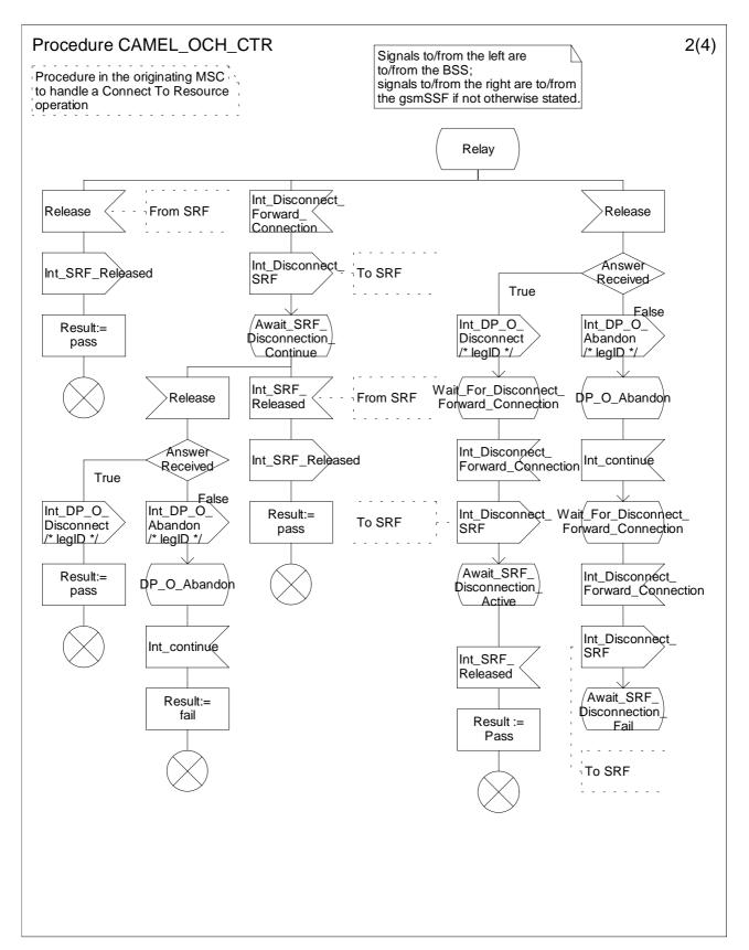
Figure 4.21b: Procedure CAMEL\_OCH\_CTR (sheet 2)
