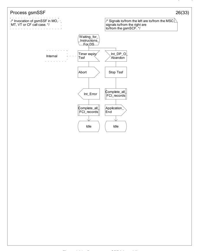
Figure 4.64z: Process gsmSSF (sheet 26)
