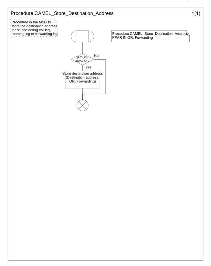
Figure 4.24: Procedure CAMEL\_Store\_Destination\_Address (sheet 1)
