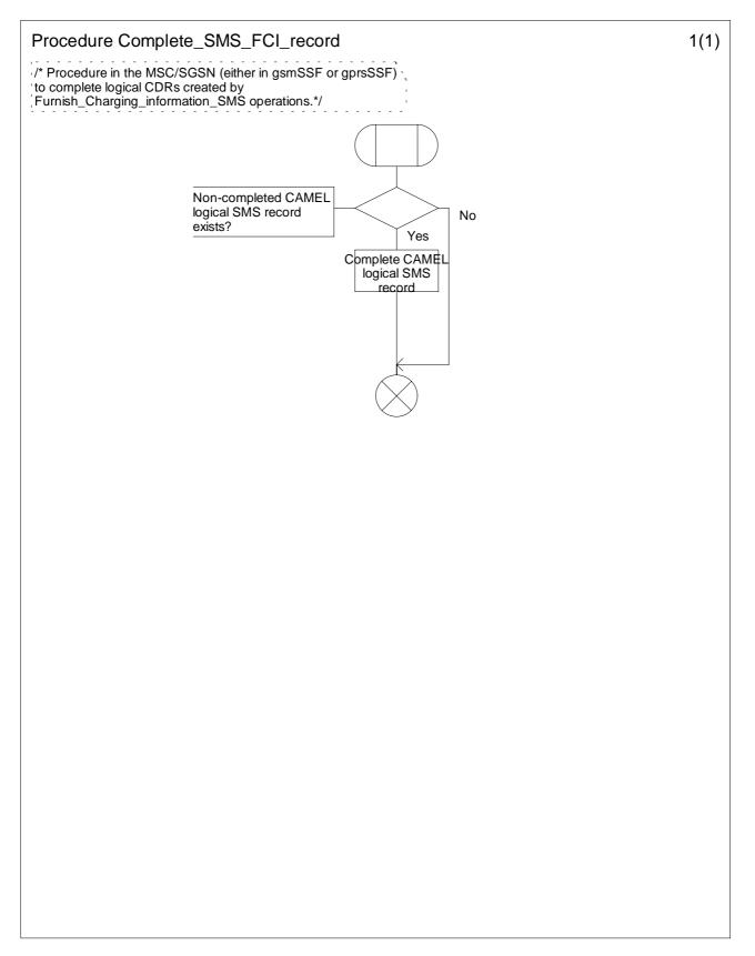
Figure 7.11: Procedure Complete\_SMS\_FCI\_record (sheet 1)
