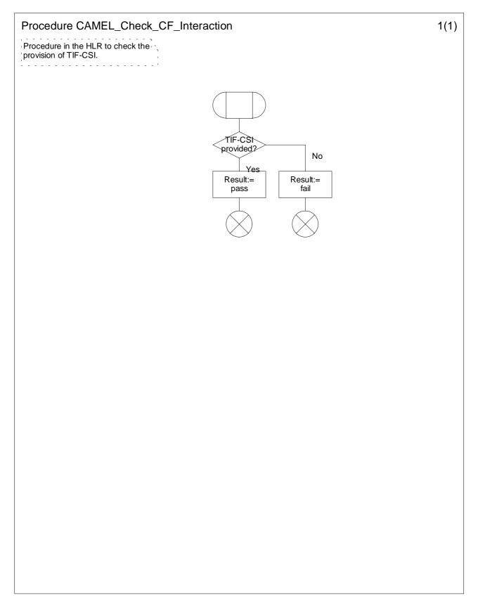
Figure 4.83: Procedure CAMEL\_Check\_CF\_Interaction
