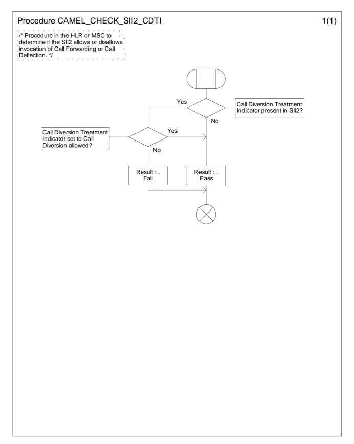
Figure 4.46: Procedure CAMEL\_CHECK\_SII2\_CDTI (sheet 1)
