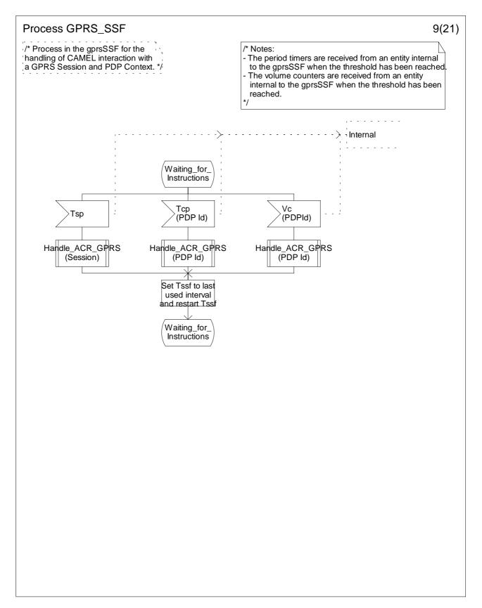
Figure 6.17i: Process GPRS\_SSF (sheet 9)
