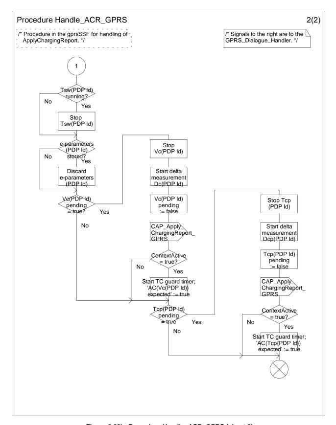
Figure 6.20b: Procedure Handle\_ACR\_GPRS (sheet 2)
