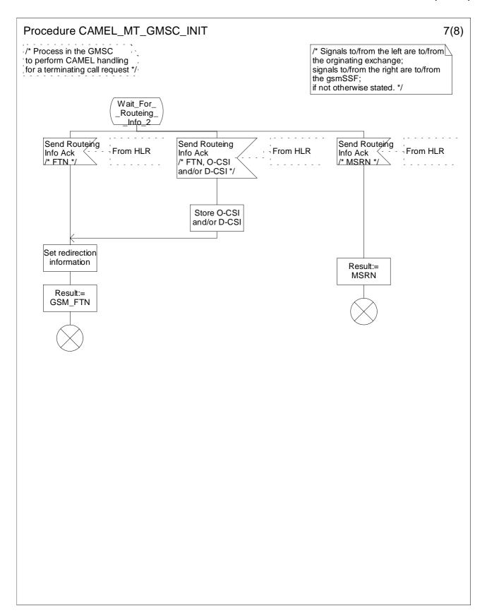
Figure 4.30g: Procedure CAMEL\_MT\_GMSC\_INIT (sheet 7)
