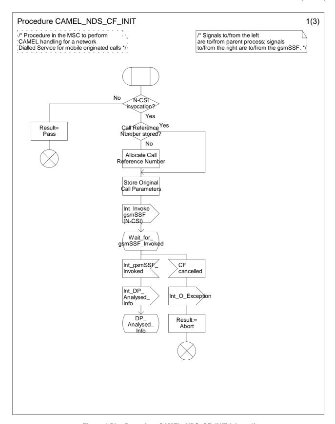
Figure 4.59a: Procedure CAMEL\_NDS\_CF\_INIT (sheet 1)
