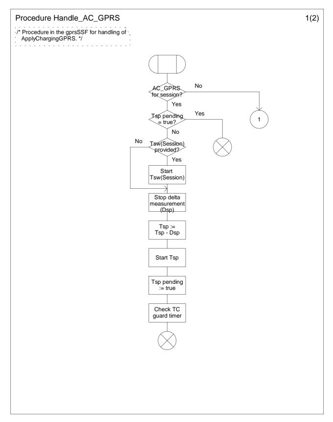
Figure 6.19a: Procedure Handle\_AC\_GPRS (sheet 1)
