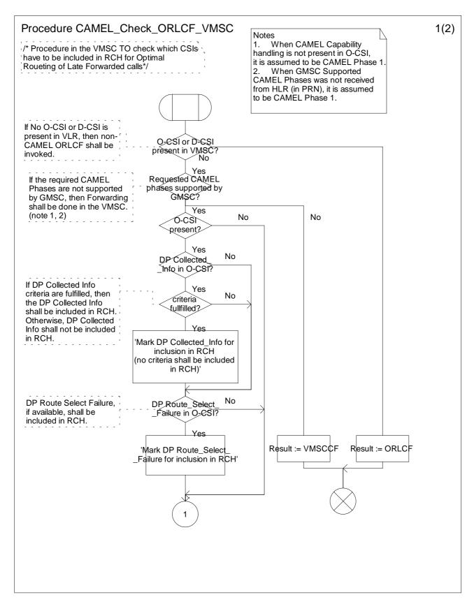
Figure 4.55a: Procedure CAMEL\_Check\_ORLCF\_VMSC (sheet 1)
