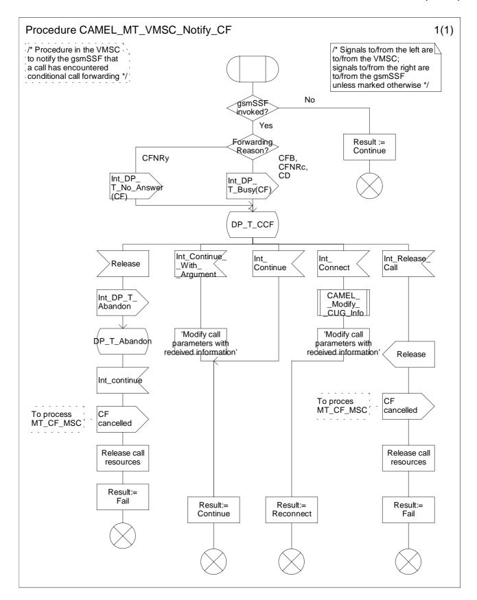
Figure 4.53a: Procedure CAMEL\_MT\_VMSC\_Notify\_CF (sheet 1)
