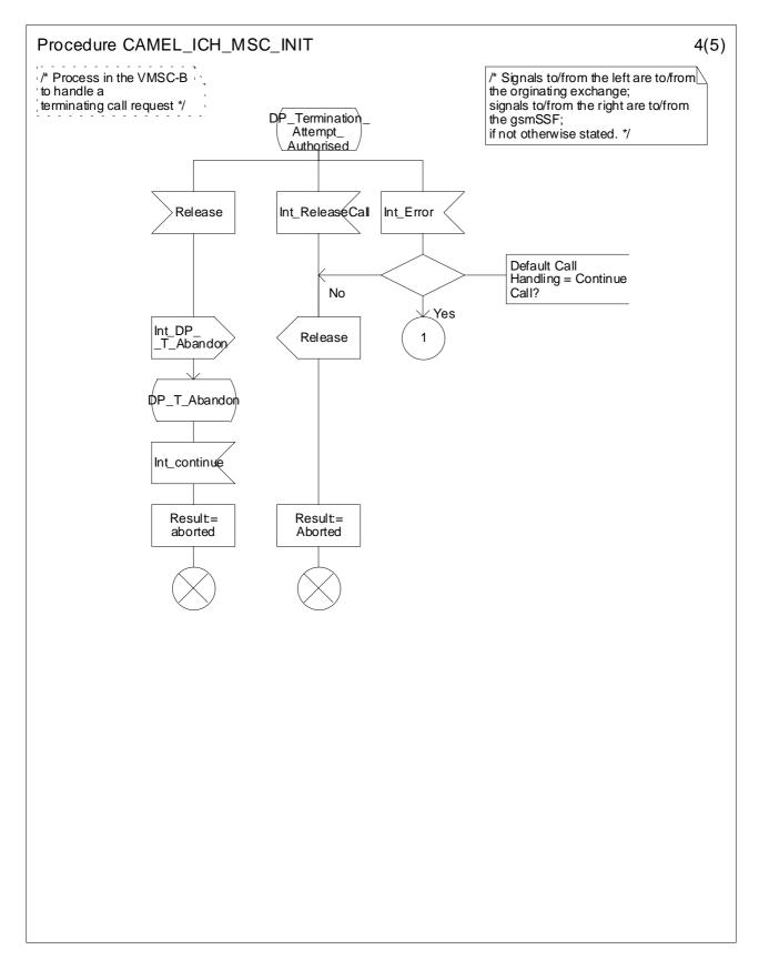
Figure 4.52d: Procedure CAMEL\_ICH\_MSC\_INIT (sheet 4)
