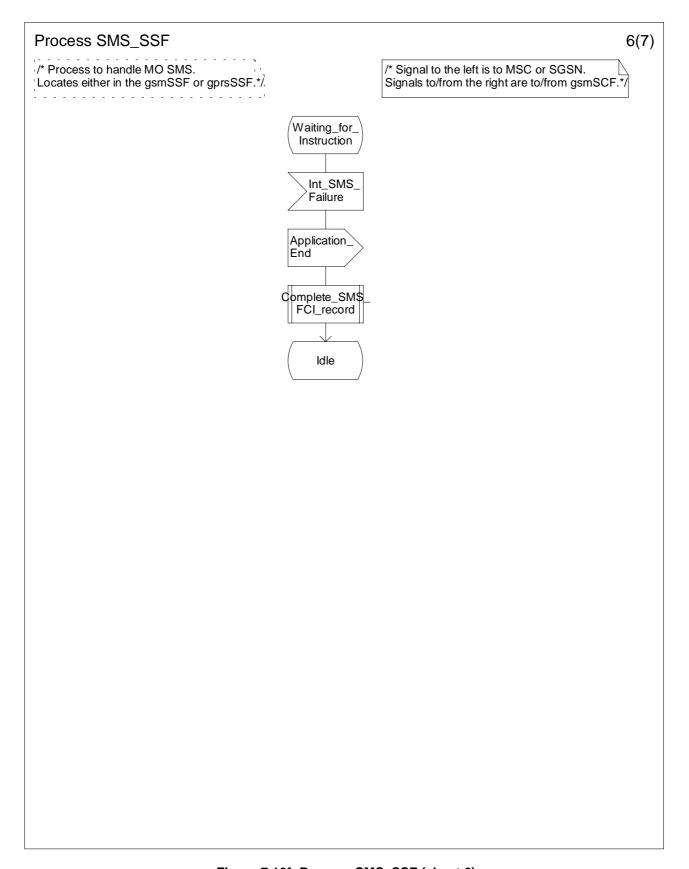
Figure 7.10f: Process SMS\_SSF (sheet 6)
