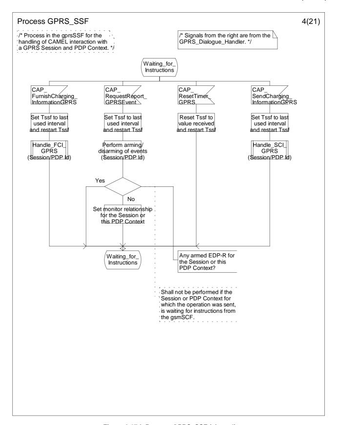
Figure 6.17d: Process GPRS\_SSF (sheet 4)
