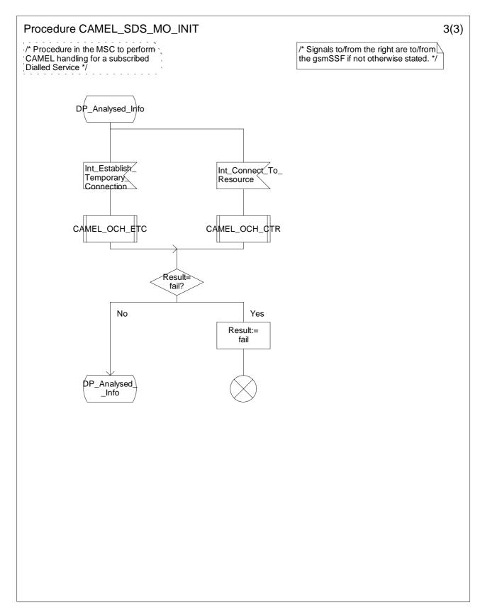
Figure 4.11c: Procedure CAMEL\_SDS\_MO\_INIT (sheet 3)
