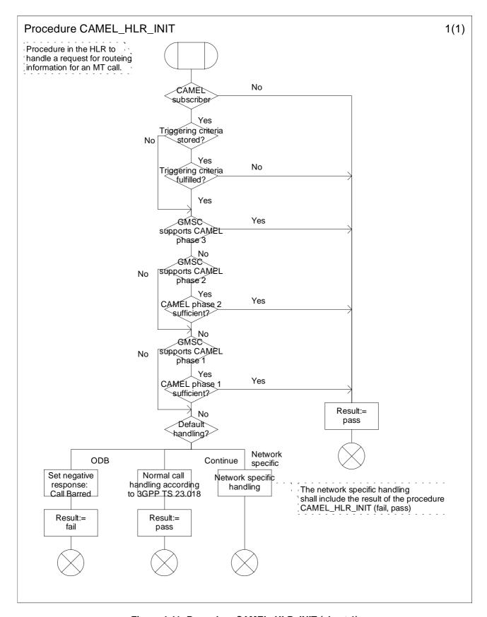
Figure 4.41: Procedure CAMEL\_HLR\_INIT (sheet 1)
