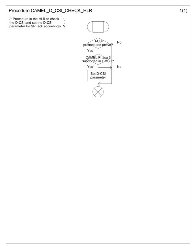
Figure 4.44: Procedure CAMEL\_D\_CSI\_CHECK\_HLR (sheet 1)
