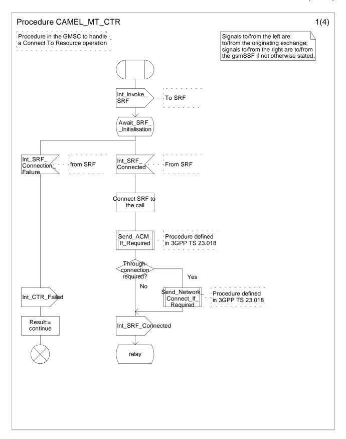
Figure 4.39a: Procedure CAMEL\_MT\_CTR (sheet 1)
