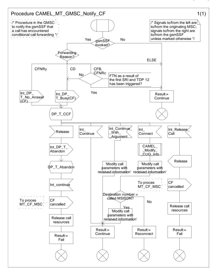
Figure 4.40a: Procedure CAMEL\_MT\_GMSC\_Notify\_CF (sheet 1)
