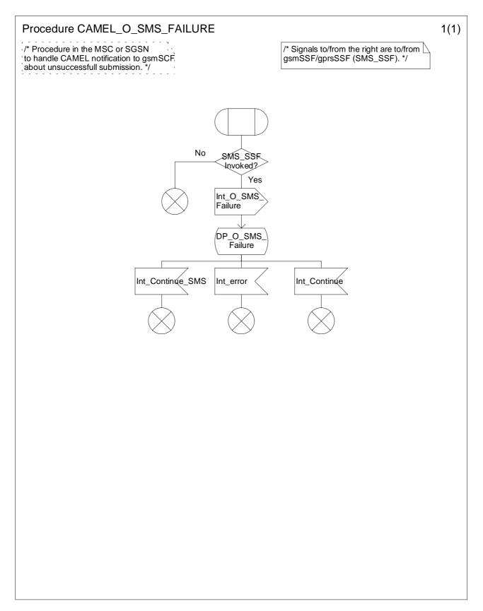
Figure 7.9: Procedure CAMEL\_O\_SMS\_FAILURE (sheet1)
