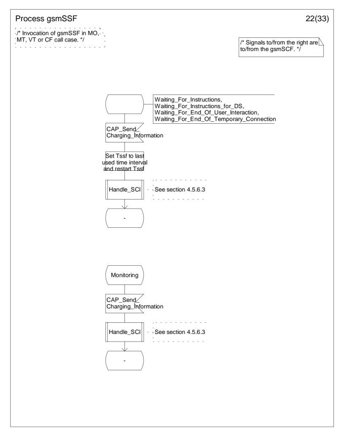
Figure 4.64v: Process gsmSSF (sheet 22)
