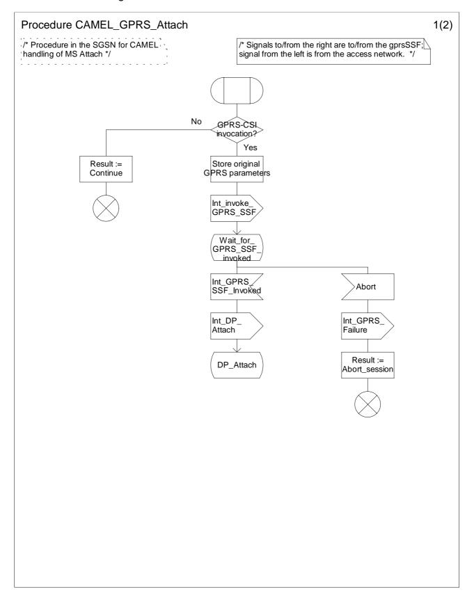
Figure 6.8a: Procedure CAMEL\_GPRS\_Attach (sheet 1)
