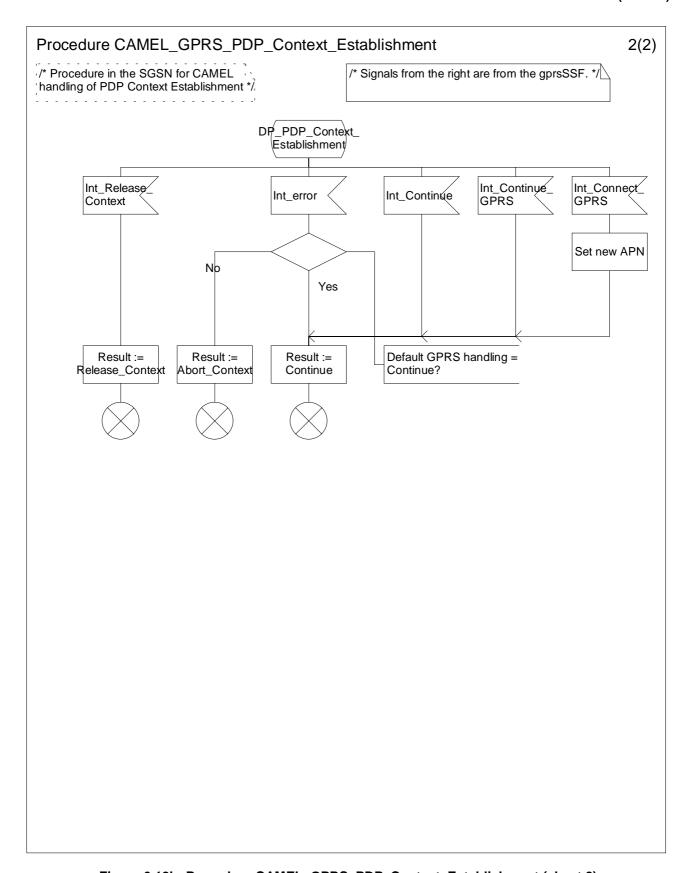
Figure 6.12b: Procedure CAMEL\_GPRS\_PDP\_Context\_Establishment (sheet 2)
