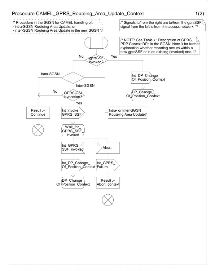
Figure 6.11a: Procedure CAMEL\_GPRS\_Routeing\_Area\_Update\_Context (sheet 1)
