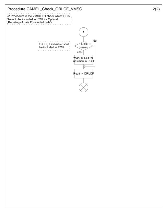
Figure 4.55b: Procedure CAMEL\_Check\_ORLCF\_VMSC (sheet 2)
