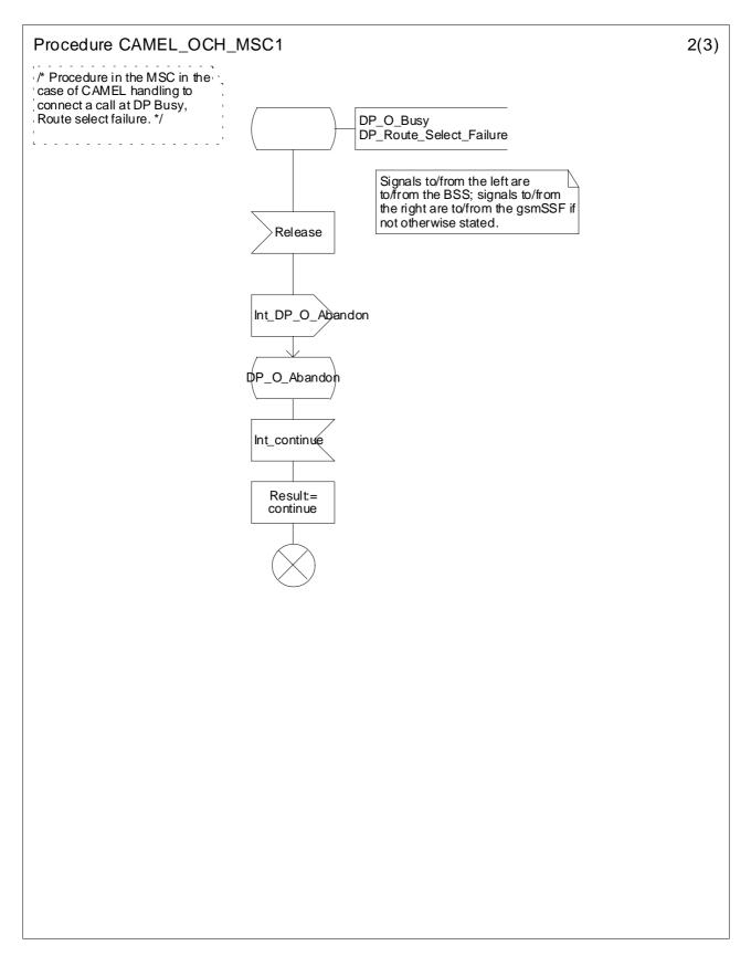
Figure 4.14b: Procedure CAMEL\_OCH\_MSC1 (sheet 2)
