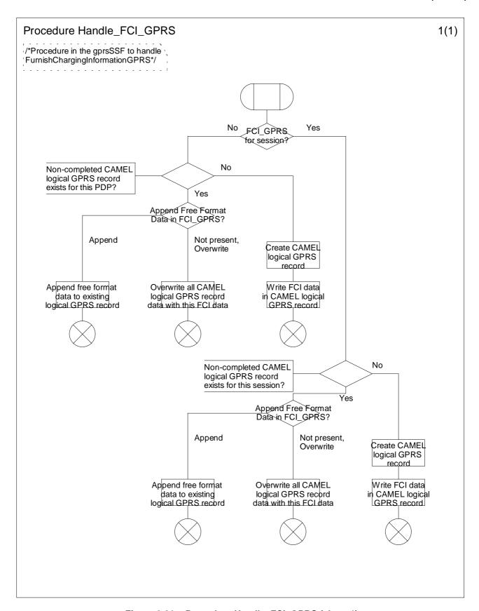
Figure 6.21a: Procedure Handle\_FCI\_GPRS (sheet 1)
