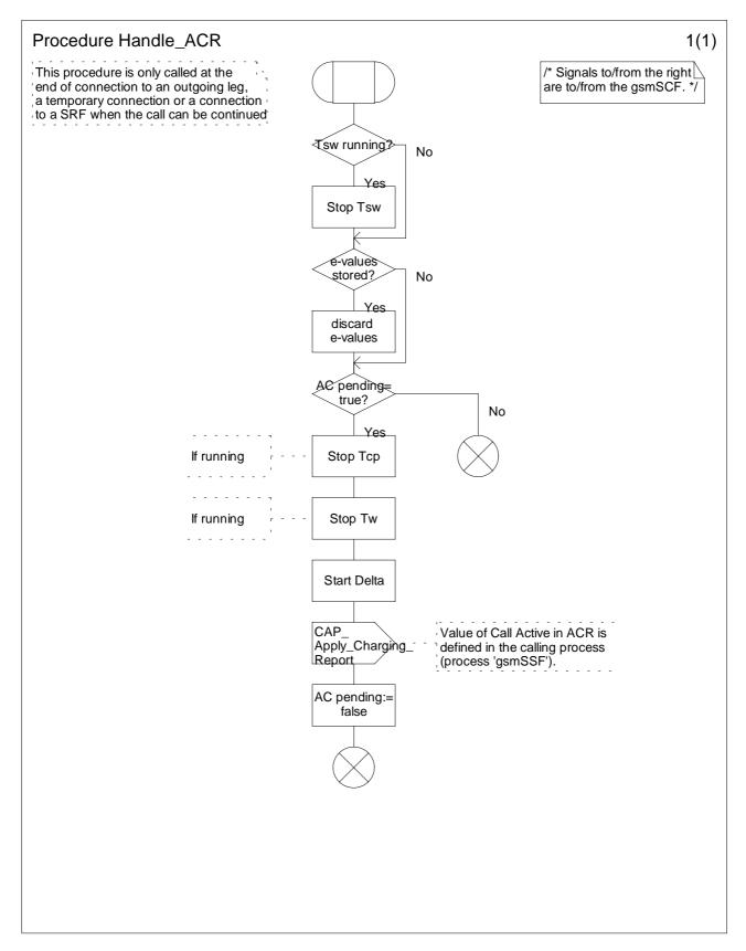
Figure 4.70a: Procedure Handle\_ACR (sheet 1)
