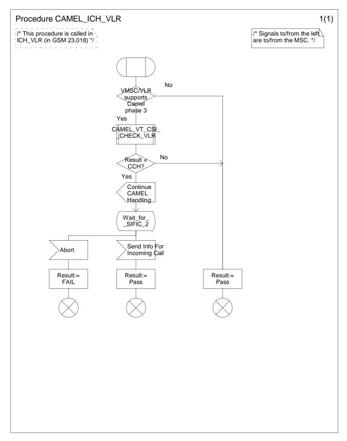
Figure 4.48: Procedure CAMEL\_ICH\_VLR (sheet 1)
