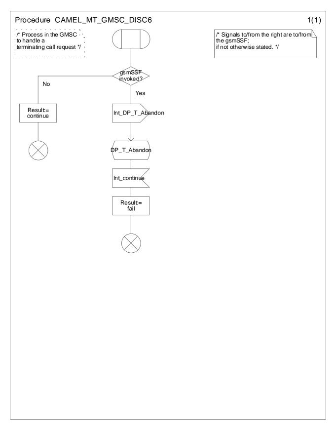
Figure 4.37a: Procedure CAMEL\_MT\_GMSC\_DISC6 (sheet 1)
