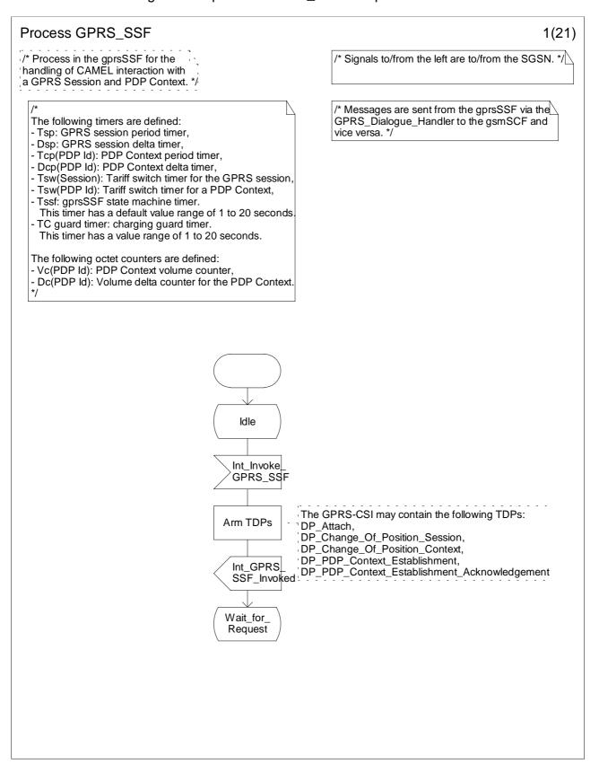
Figure 6.17a: Process GPRS\_SSF (sheet 1)
