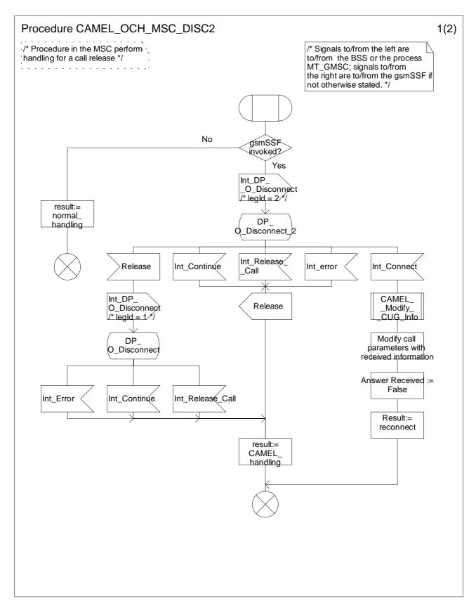
Figure 4.17a: Procedure CAMEL\_OCH\_MSC\_DISC2 (sheet 1)
