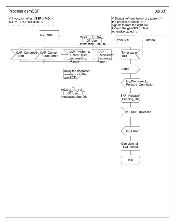
Figure 4.64ff: Process gsmSSF (sheet 32)
