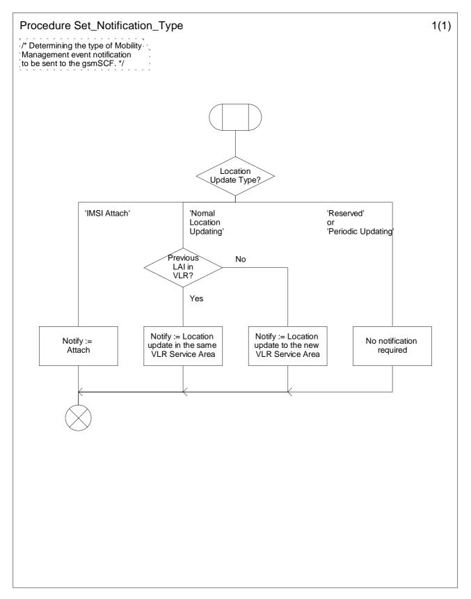
Figure 9.3: Procedure Set\_Notification\_Type (sheet 1)
