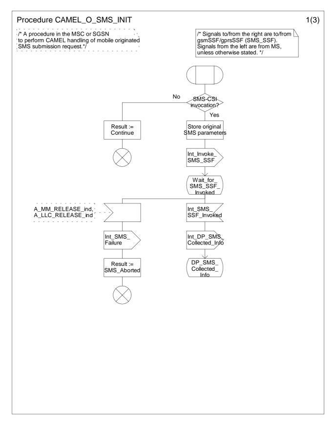
Figure 7.7a: Procedure CAMEL\_O\_SMS\_INIT (sheet1)
