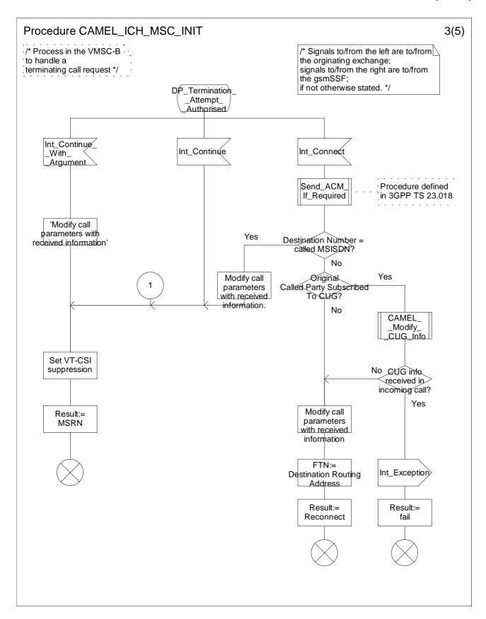
Figure 4.52c: Procedure CAMEL\_ICH\_MSC\_INIT (sheet 3)
