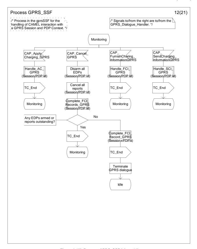
Figure 6.17I: Process GPRS\_SSF (sheet 12)
