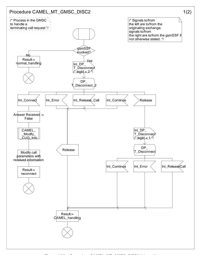
Figure 4.33a: Procedure CAMEL\_MT\_GMSC\_DISC2 (sheet 1)
