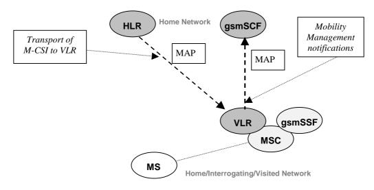
Figure 9.1: Functional architecture for support of CAMEL
