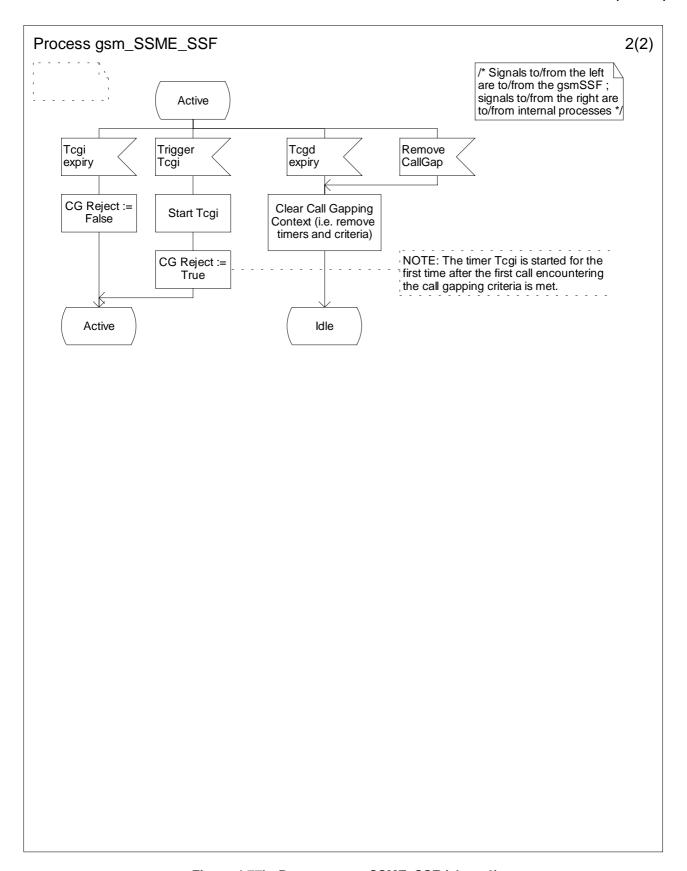
Figure 4.77b: Process gsm\_SSME\_SSF (sheet 2)
