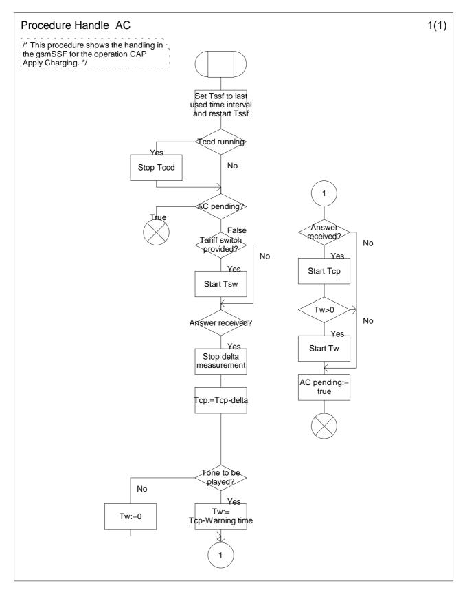
Figure 4.69a: Procedure Handle\_AC (sheet 1)
