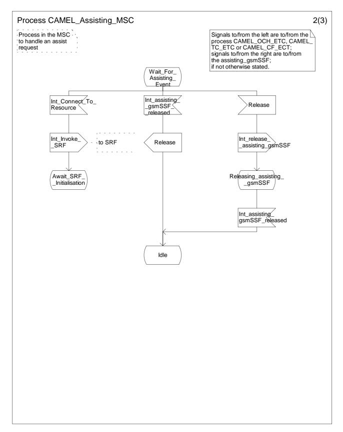
Figure 4.80b: Process CAMEL\_Assisting\_MSC (sheet 2)
