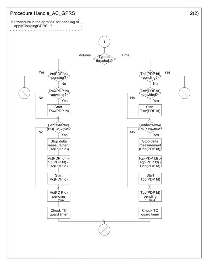
Figure 6.19b: Procedure Handle\_AC\_GPRS (sheet 2)
