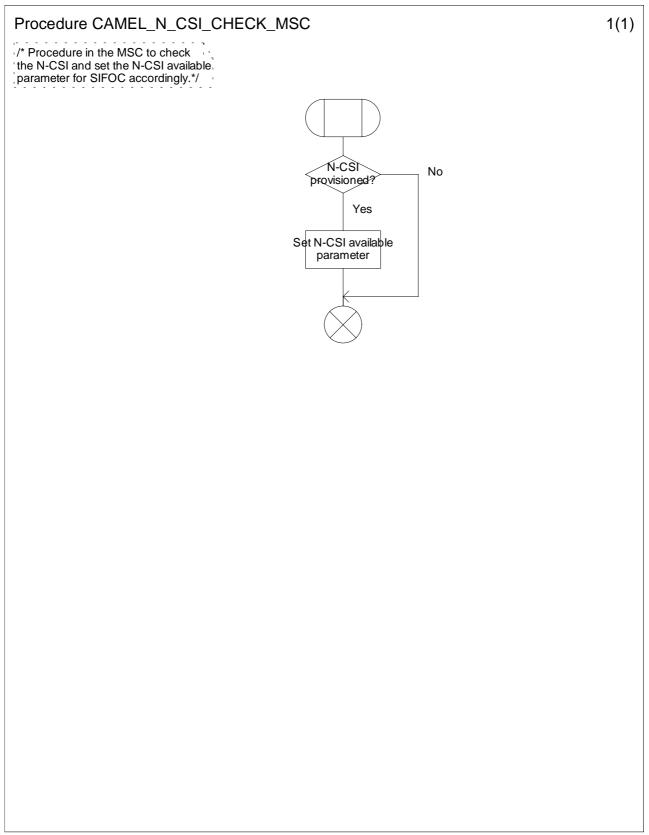
Figure 4.26: Procedure CAMEL\_N\_CSI\_CHECK\_MSC (sheet 1)
