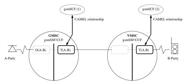
Figure 4.6: BCSM Scenario for Mobile Terminated Calls at the GMSC / VMSC
