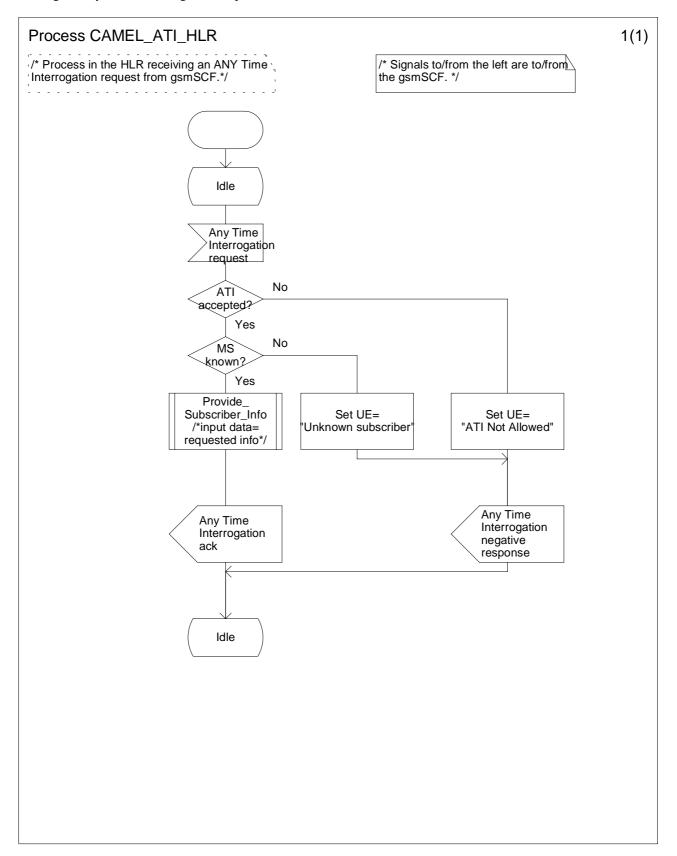
Figure 11.3: Process CAMEL\_ATI\_HLR (sheet 1)
