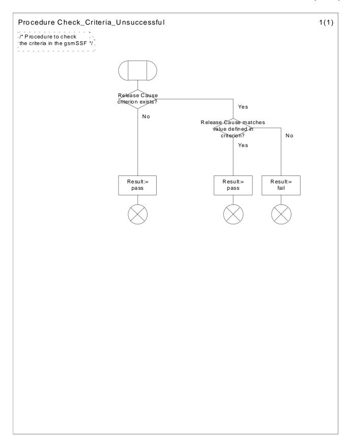
Figure 4.67a: Procedure Check\_Criteria\_Unsuccessful(sheet 1)
