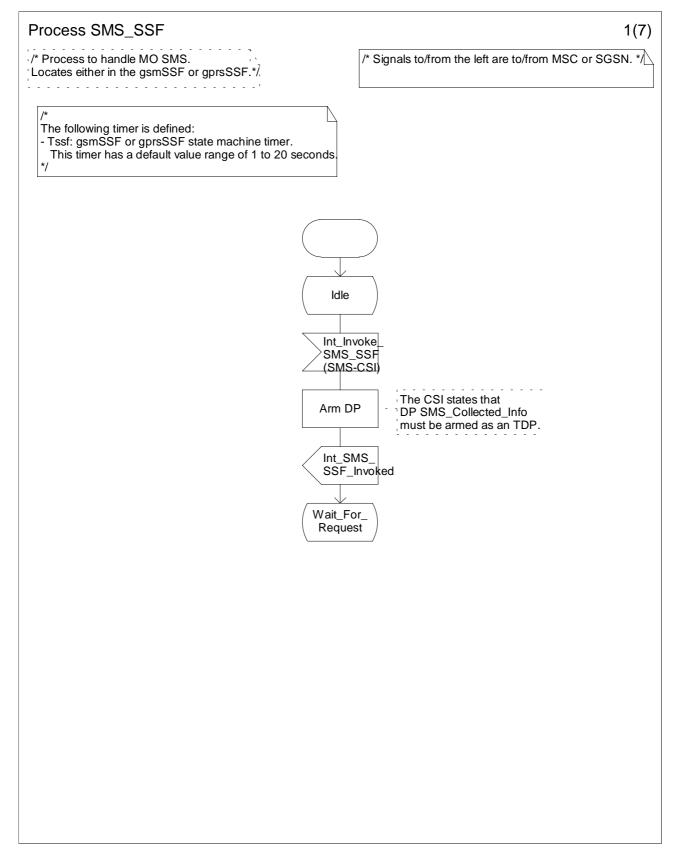
Figure 7.10a: Process SMS\_SSF (sheet 1)
