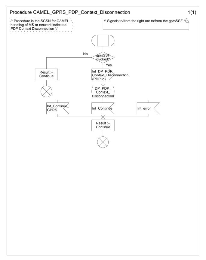
Figure 6.15: Procedure CAMEL\_GPRS\_PDP\_Context\_Disconnection (sheet 1)
