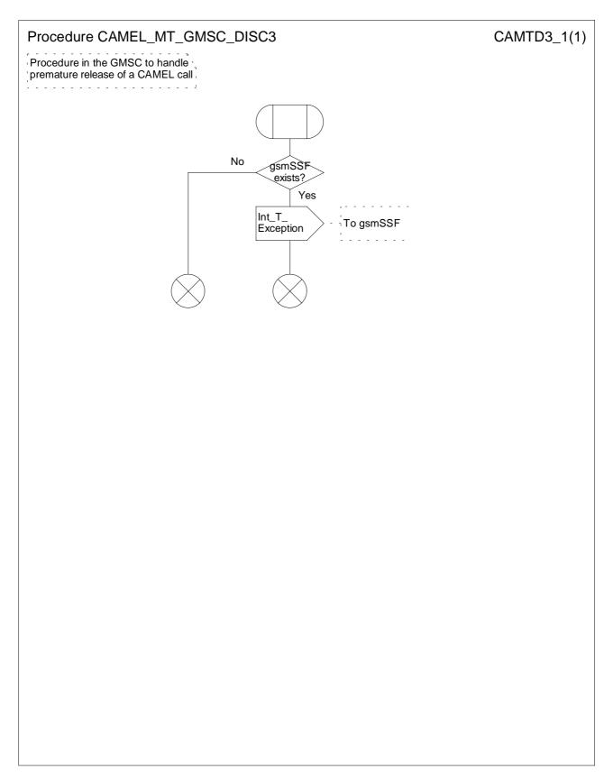
Figure 4.34a: Procedure CAMEL\_MT\_GMSC\_DISC3 (sheet 1)
