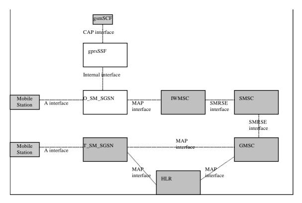
Figure 7.6: Case of MO SMS via GPRS SGSN
