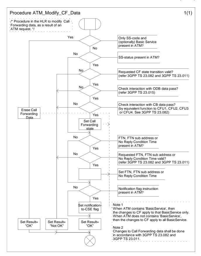
Figure 10.6: Procedure ATM\_Modify\_CF\_Data (sheet 1)
