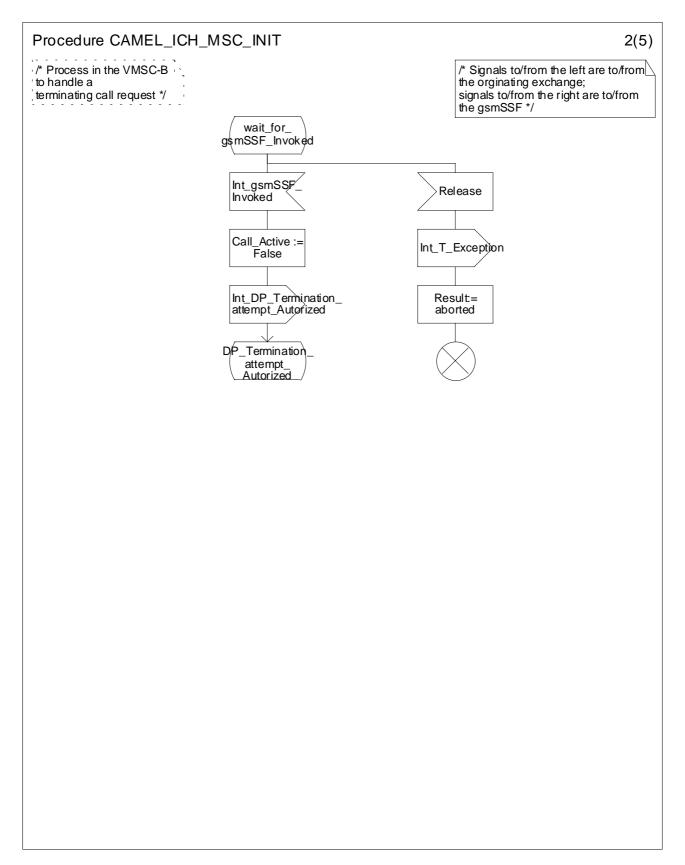
Figure 4.52b: Procedure CAMEL\_ICH\_MSC\_INIT (sheet 2)
