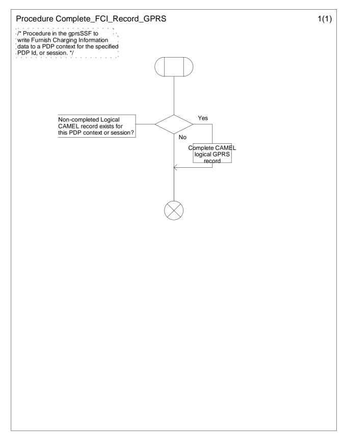
Figure 6.22a: Procedure Complete\_FCI\_Record\_GPRS (sheet 1)
