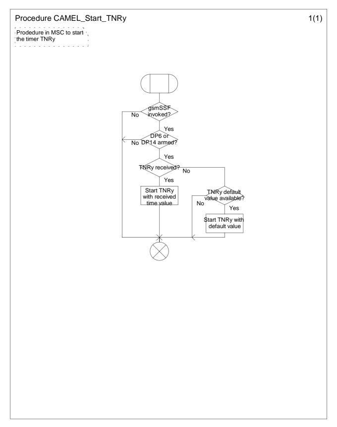
Figure 4.22: Procedure CAMEL\_Start\_TNRy (sheet 1)
