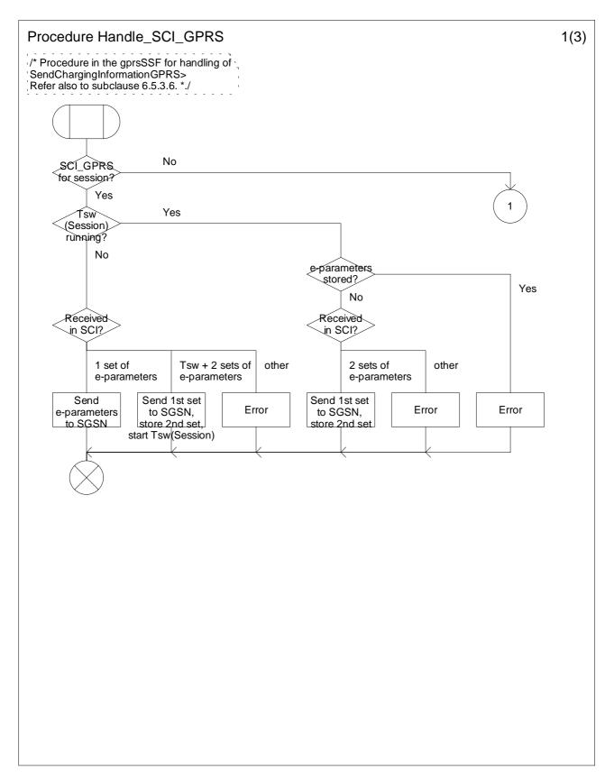
Figure 6.23a: Procedure Handle\_SCI\_GPRS (sheet 1)
