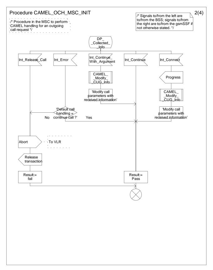
Figure 4.10b: Procedure CAMEL\_OCH\_MSC\_INIT (sheet 2)
