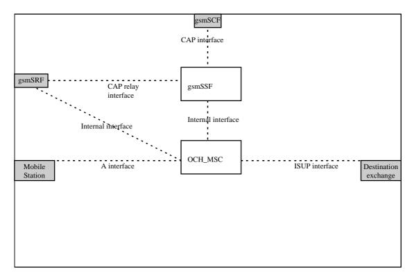
Figure 4.8a: Outgoing case (gsmSSF relay)
