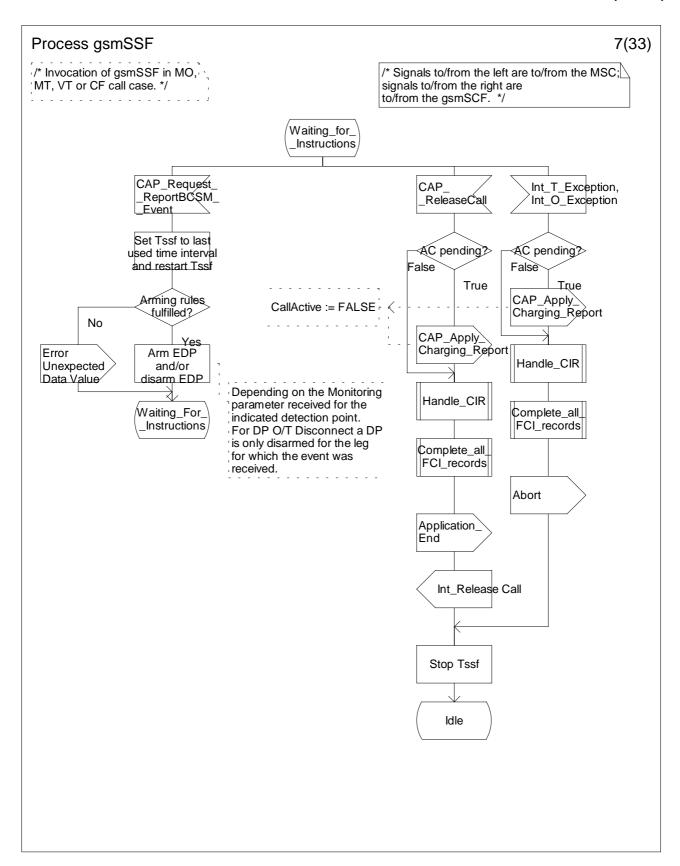
Figure 4.64g: Process gsmSSF (sheet 7)
