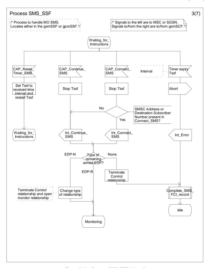
Figure 7.10c: Process SMS\_SSF (sheet 3)
