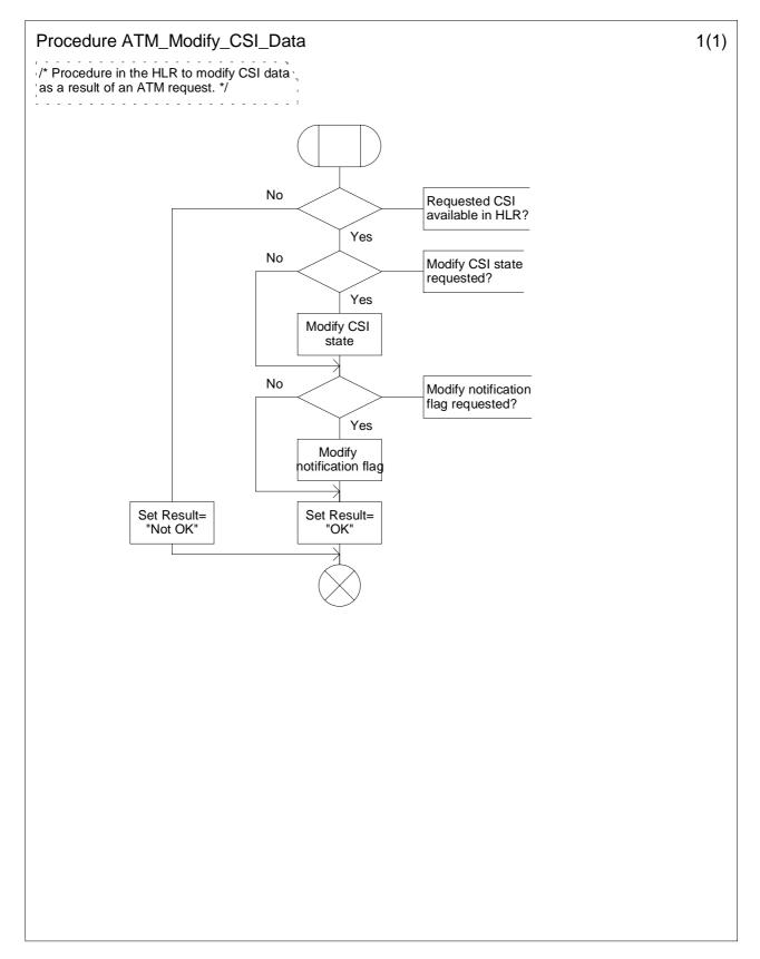
Figure 10.5: Procedure ATM\_Modify\_CSI\_Data (sheet 1)
