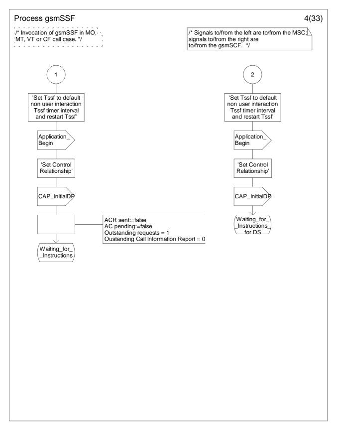
Figure 4.64d: Process gsmSSF (sheet 4)
