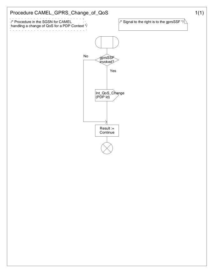
Figure 6.14: Procedure CAMEL\_GPRS\_Change\_Of\_QoS (sheet 1)
