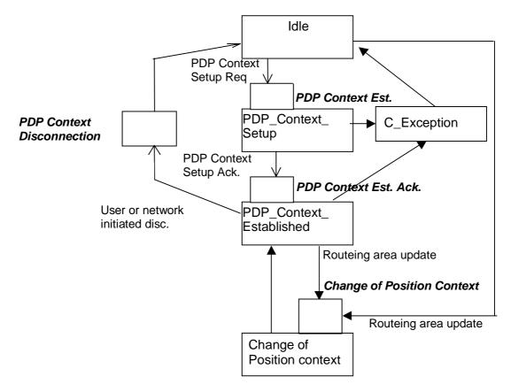
Figure 6.4: GPRS PDP Context State Model
