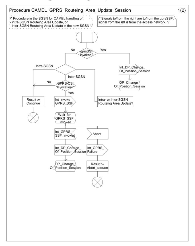
Figure 6.10a: Procedure CAMEL\_GPRS\_Routeing\_Area\_Update\_Session (sheet 1)
