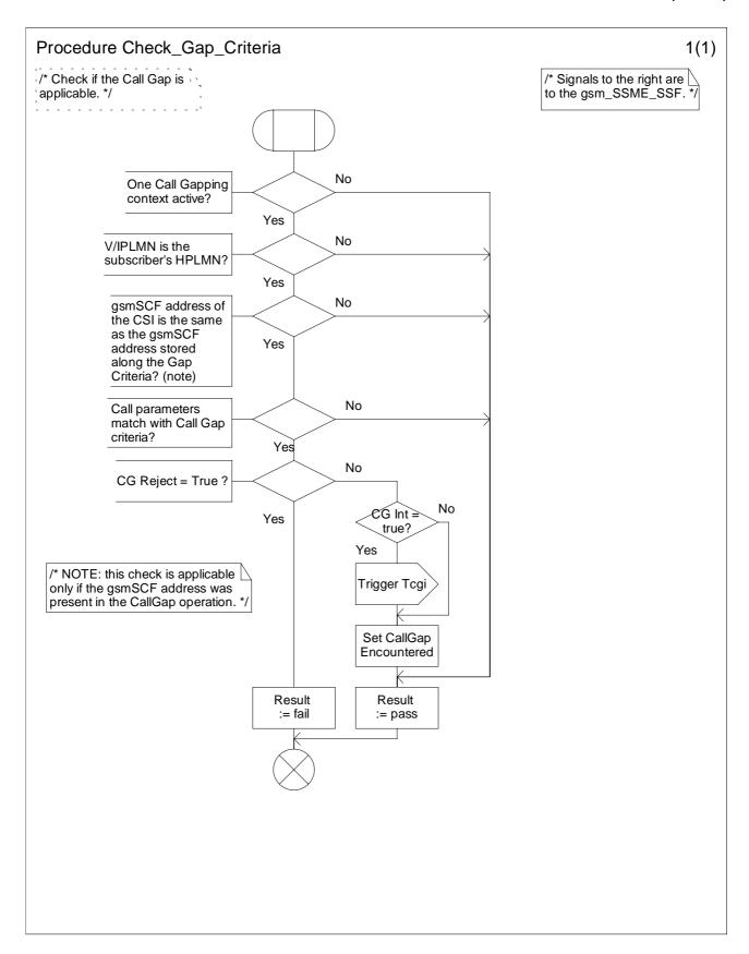
Figure 4.79a: Procedure Check\_Gap\_Criteria (sheet 1)
