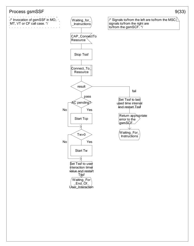
Figure 4.64i: Process gsmSSF (sheet 9)
