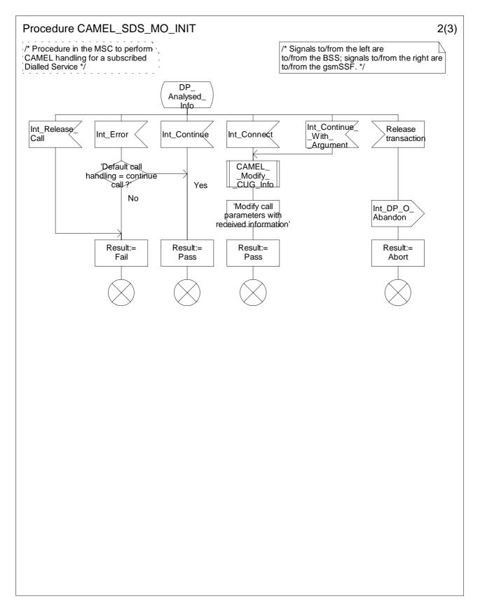
Figure 4.11b: Procedure CAMEL\_SDS\_MO\_INIT (sheet 2)
