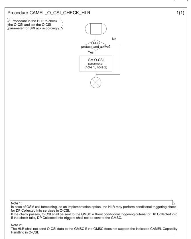
Figure 4.43: Procedure CAMEL\_O\_CSI\_CHECK\_HLR (sheet 1)
