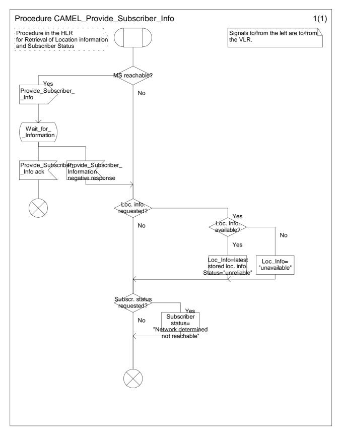
Figure 4.82a: Procedure CAMEL\_Provide\_Subscriber\_Info (sheet 1)
