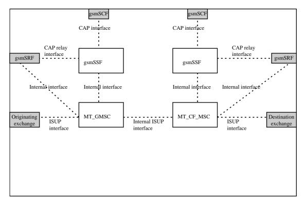
Figure 4.8c: Terminating GMSC case (gsmSSF relay)
