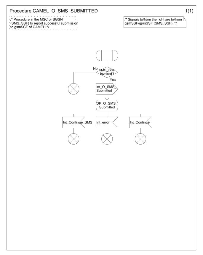
Figure 7.8: Procedure CAMEL\_O\_SMS\_SUBMITTED (sheet1)
