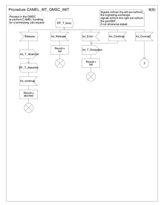
Figure 4.30h: Procedure CAMEL\_MT\_GMSC\_INIT (sheet 8)
