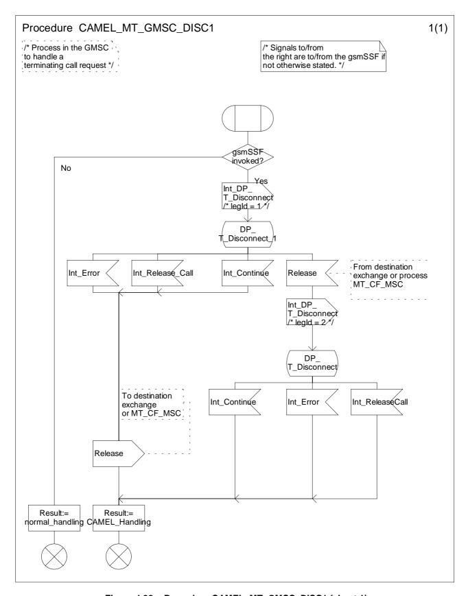
Figure 4.32a: Procedure CAMEL\_MT\_GMSC\_DISC1 (sheet 1)
