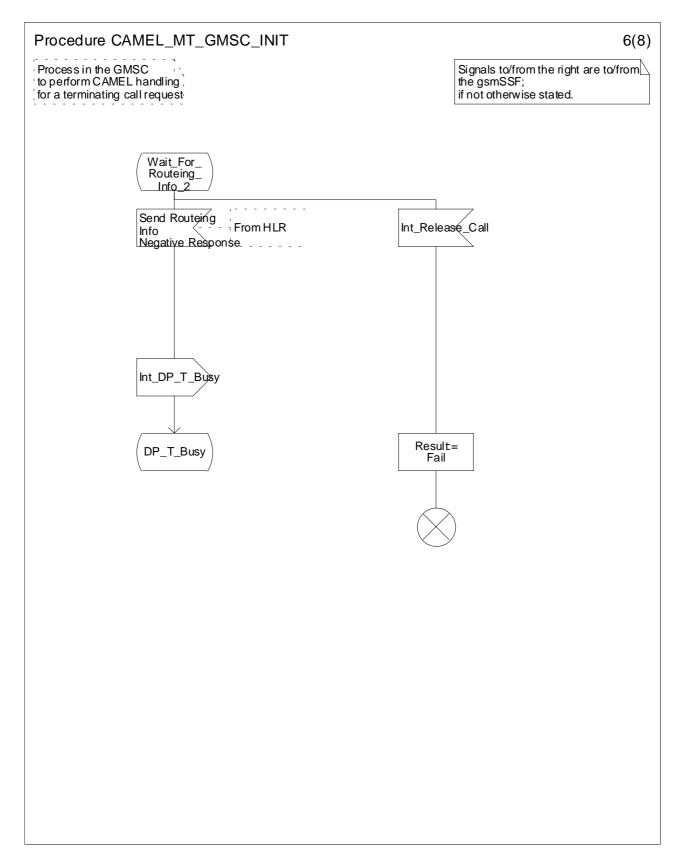
Figure 4.30f: Procedure CAMEL\_MT\_GMSC\_INIT (sheet 6)
