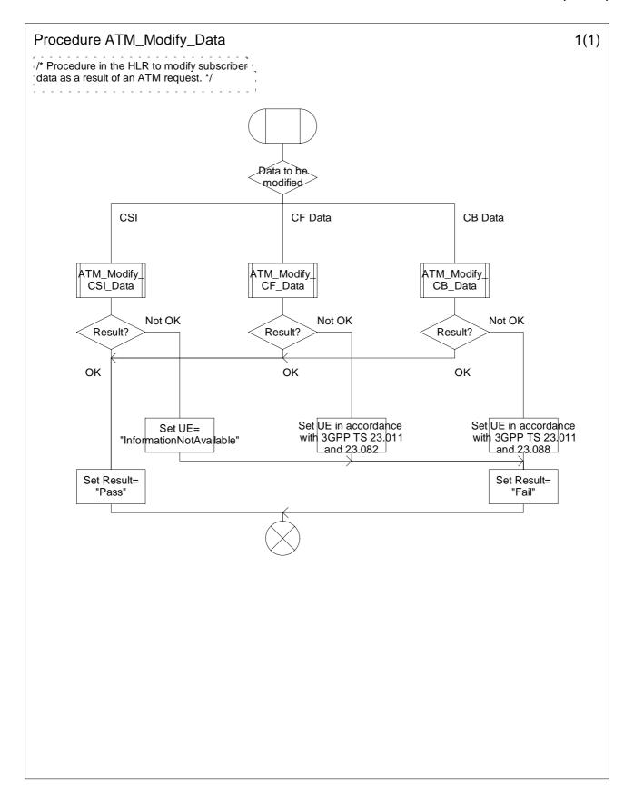
Figure 10.4: Procedure ATM\_Modify\_Data (sheet 1)
