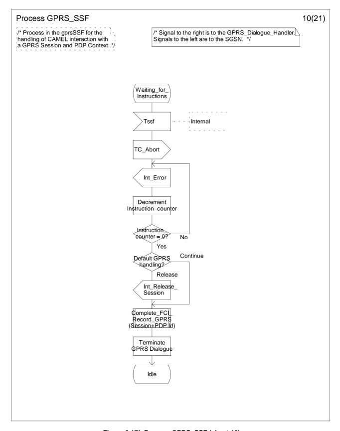
Figure 6.17j: Process GPRS\_SSF (sheet 10)
