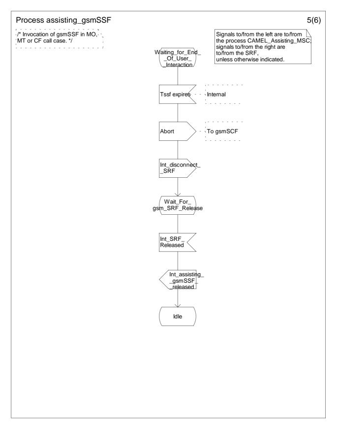
Figure 4.81e: Process Assisting\_gsmSSF (sheet 5)
