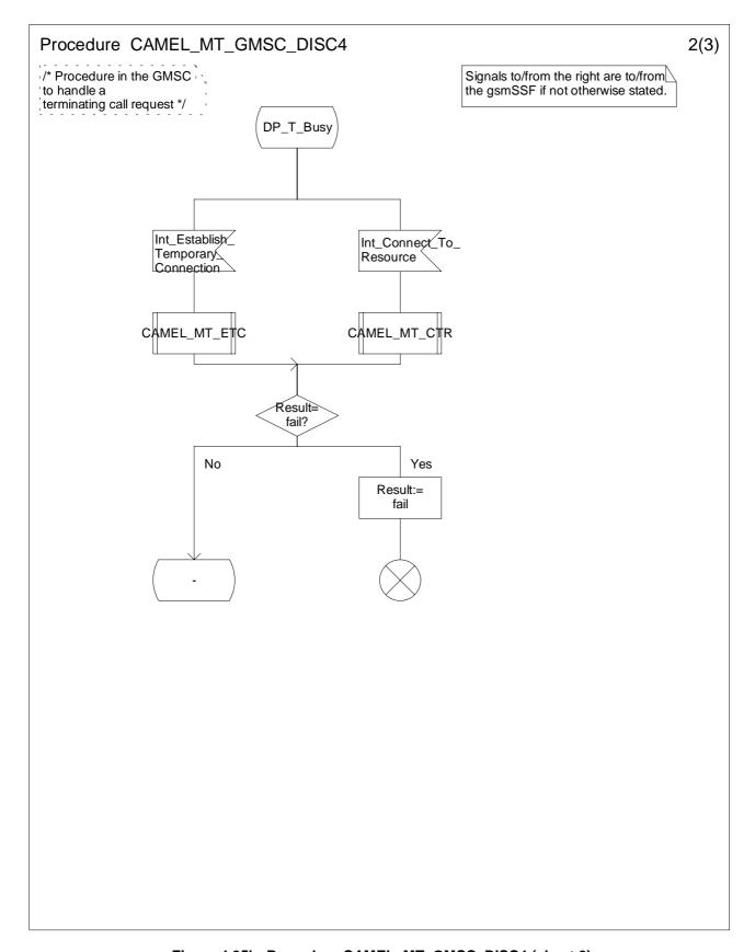
Figure 4.35b: Procedure CAMEL\_MT\_GMSC\_DISC4 (sheet 2)
