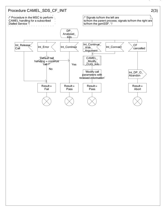
Figure 4.58b: Procedure CAMEL\_SDS\_CF\_INIT (sheet 2)
