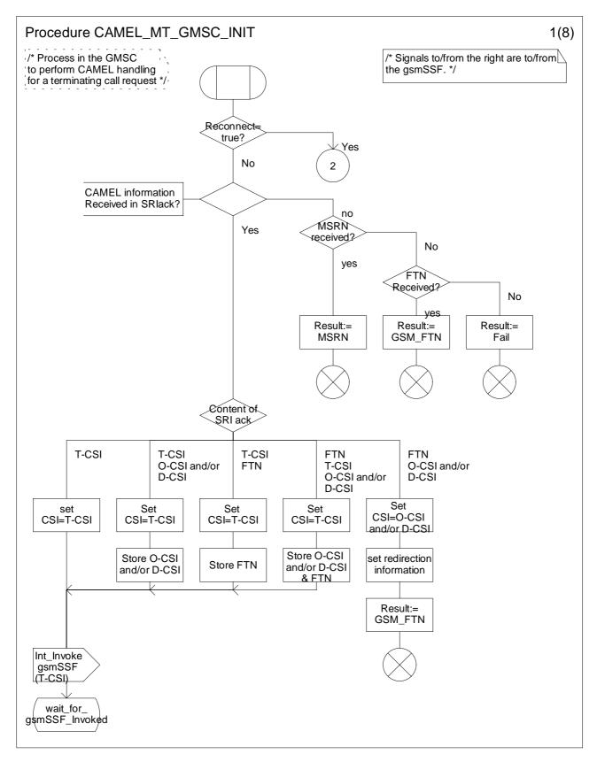
Figure 4.30a: Procedure CAMEL\_MT\_GMSC\_INIT (sheet 1)
