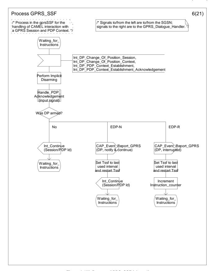
Figure 6.17f: Process GPRS\_SSF (sheet 6)
