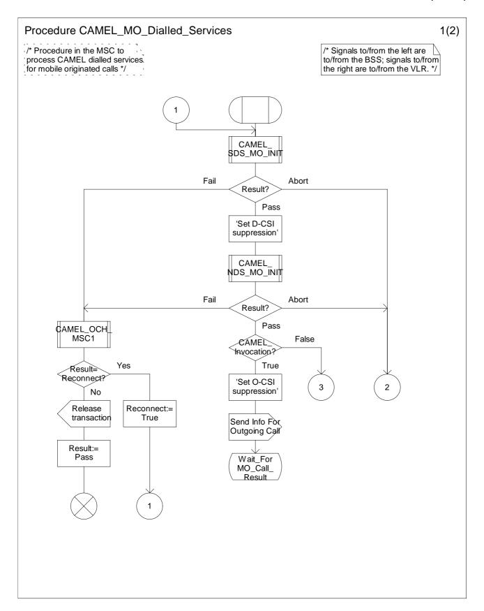
Figure 4.9a: Procedure CAMEL\_MO\_Dialled\_Services (sheet 1)
