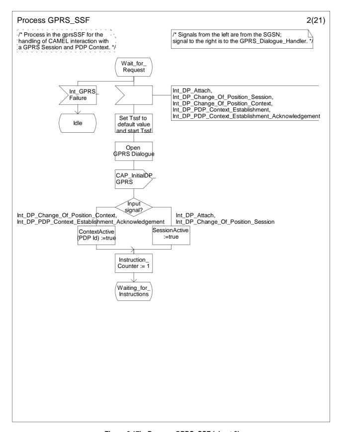
Figure 6.17b: Process GPRS\_SSF (sheet 2)
