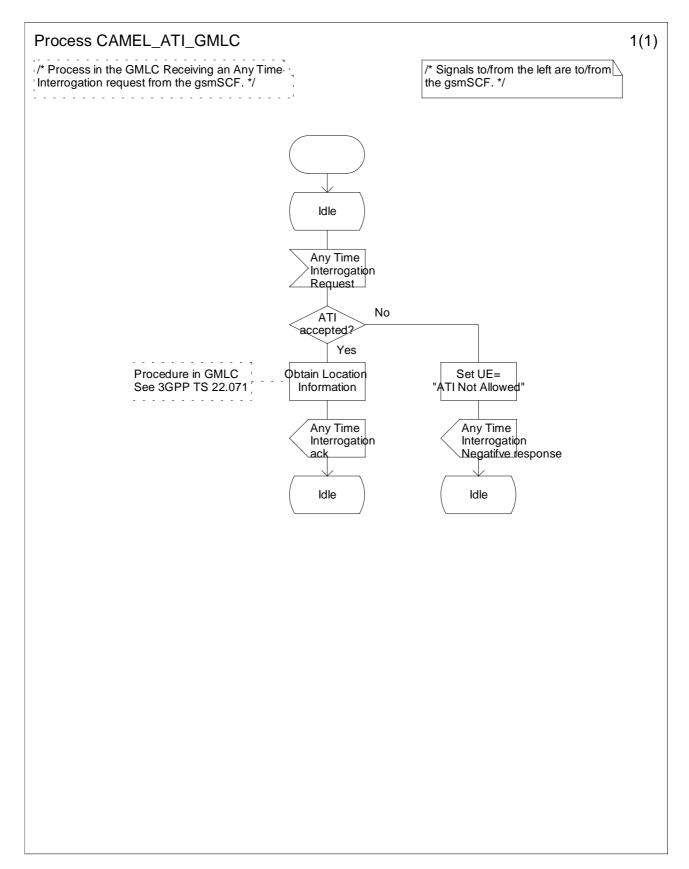
Figure 11.2: Process CAMEL\_ATI\_GMLC (sheet 1)
