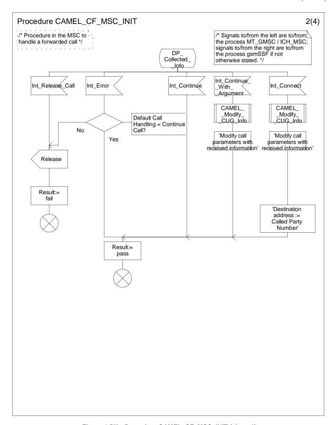
Figure 4.57b: Procedure CAMEL\_CF\_MSC\_INIT (sheet 2)
