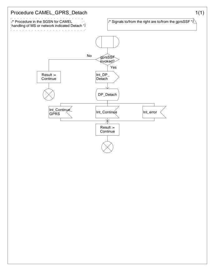
Figure 6.9: Procedure CAMEL\_GPRS\_Detach (sheet 1)
