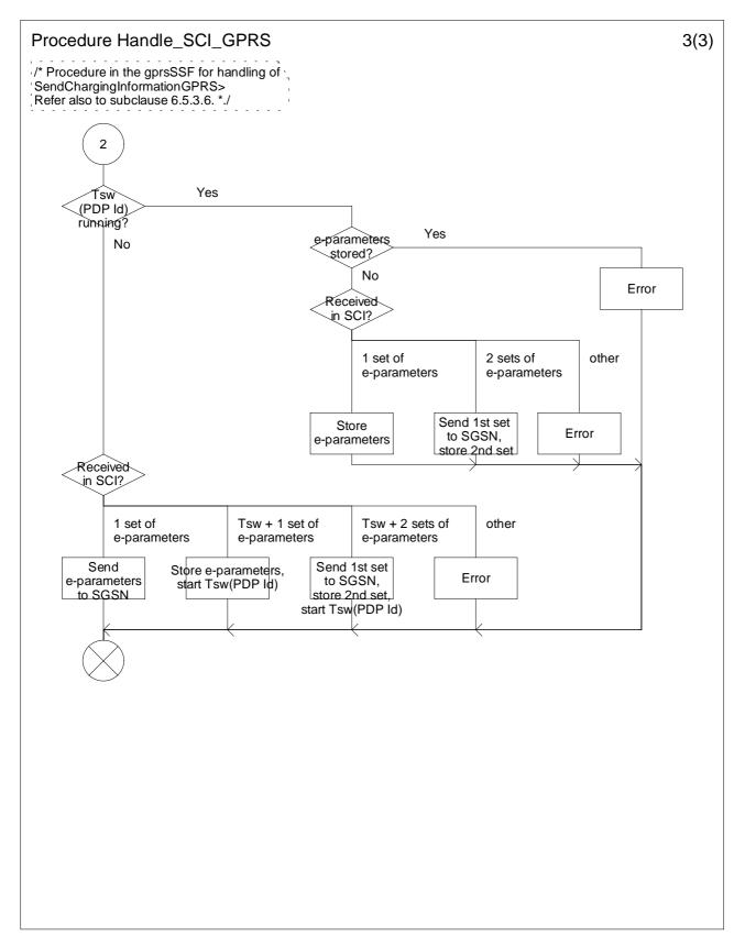
Figure 6.23c: Procedure Handle\_SCI\_GPRS (sheet 3)
