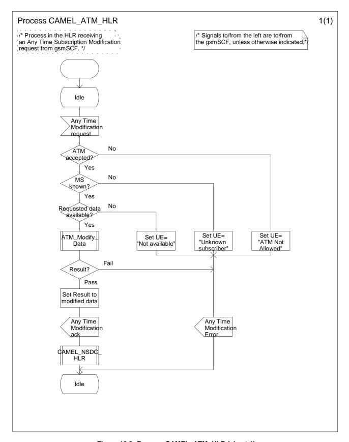
Figure 10.3: Process CAMEL\_ATM\_HLR (sheet 1)
