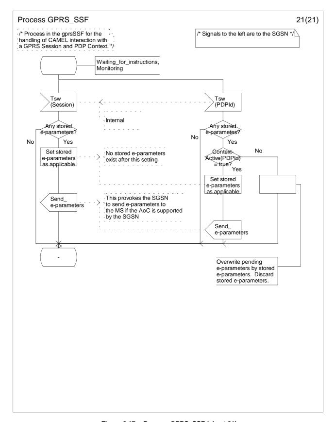
Figure 6.17u: Process GPRS\_SSF (sheet 21)
