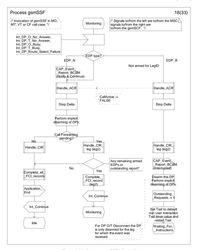
Figure 4.64r: Process gsmSSF (sheet 18)
