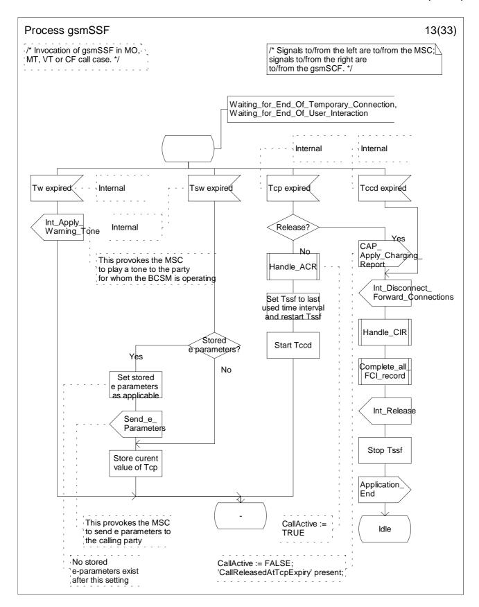
Figure 4.64m: Process gsmSSF (sheet 13)
