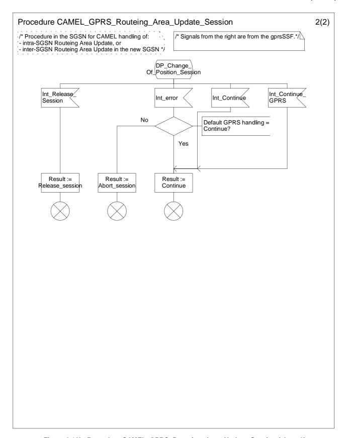
Figure 6.10b: Procedure CAMEL\_GPRS\_Routeing\_Area\_Update\_Session (sheet 2)
