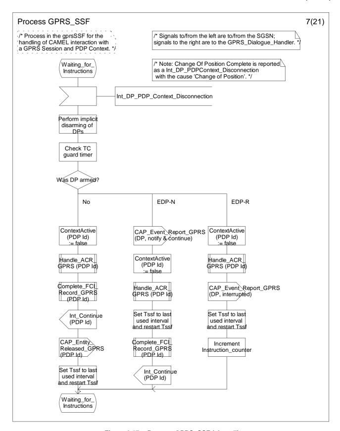
Figure 6.17g: Process GPRS\_SSF (sheet 7)
