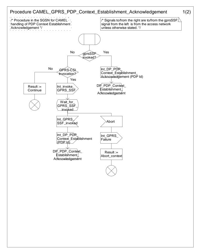
Figure 6.13a: Procedure CAMEL\_GPRS\_PDP\_Context\_Establishment\_Acknowledgement (sheet 1)
