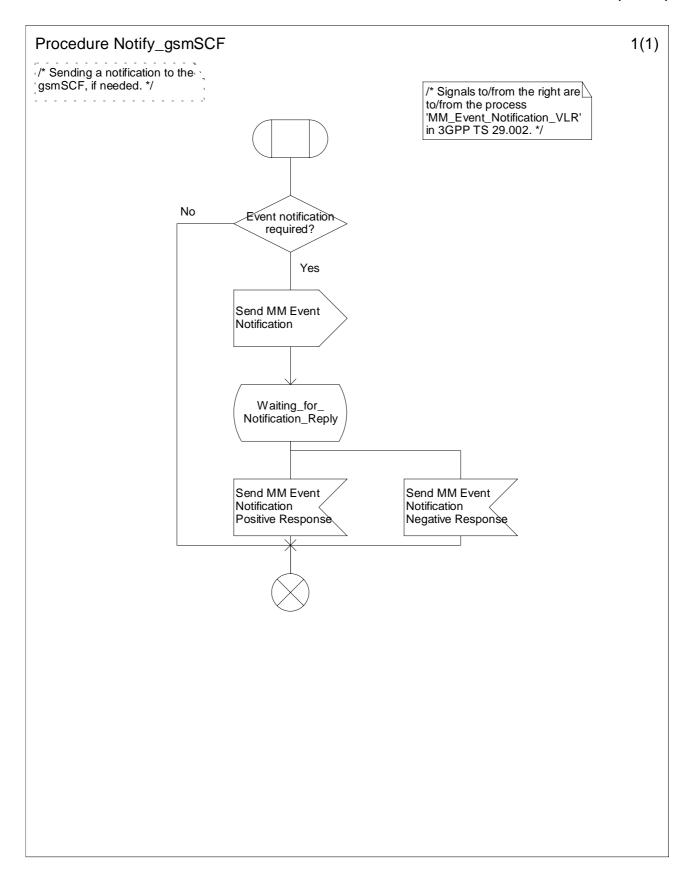
Figure 9.4: Procedure Notify\_gsmSCF (sheet 1)
