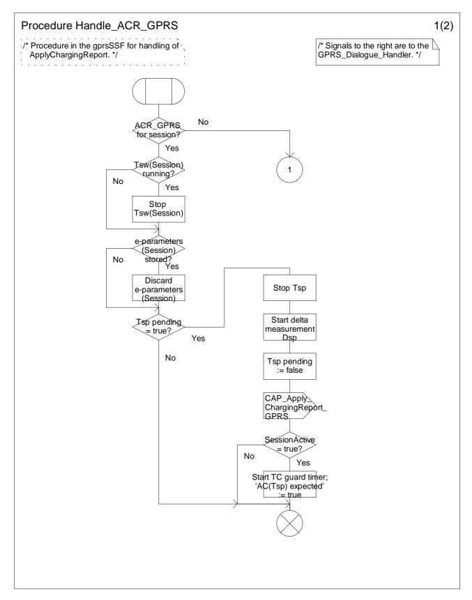
Figure 6.20a: Procedure Handle\_ACR\_GPRS (sheet 1)
