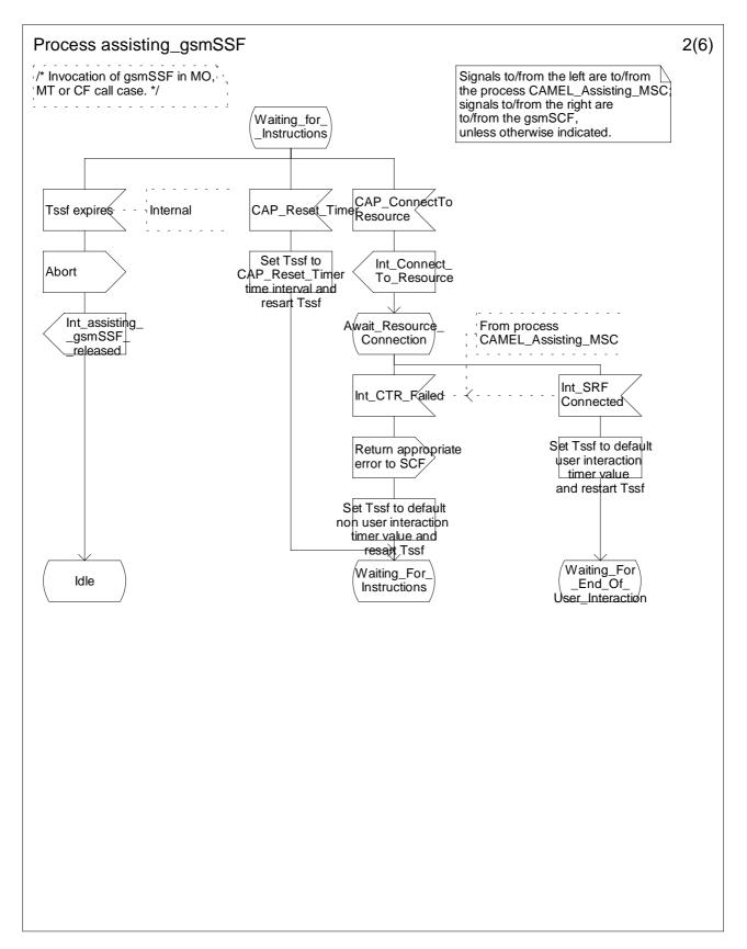
Figure 4.81b: Process Assisting\_gsmSSF (sheet 2)
