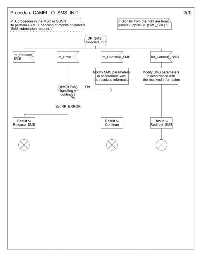
Figure 7.7b: Procedure CAMEL\_O\_SMS\_INIT (sheet2)
