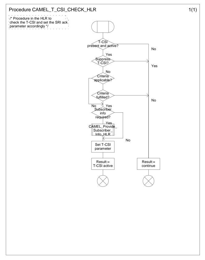
Figure 4.45: Procedure CAMEL\_T\_CSI\_CHECK\_HLR (sheet 1)
