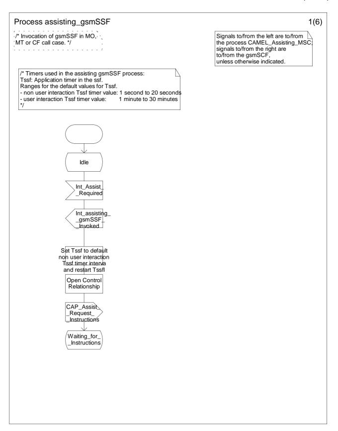
Figure 4.81a: Process Assisting\_gsmSSF (sheet 1)
