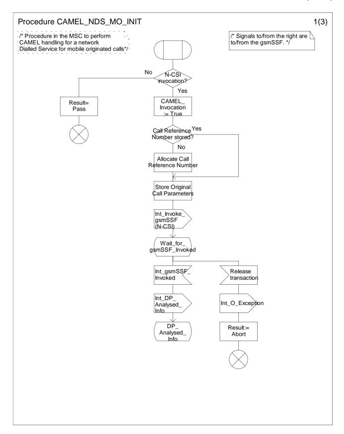
Figure 4.12a: Procedure CAMEL\_NDS\_MO\_INIT (sheet 1)
