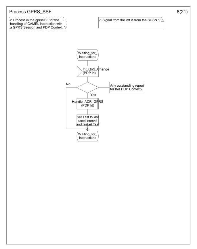
Figure 6.17h: Process GPRS\_SSF (sheet 8)
