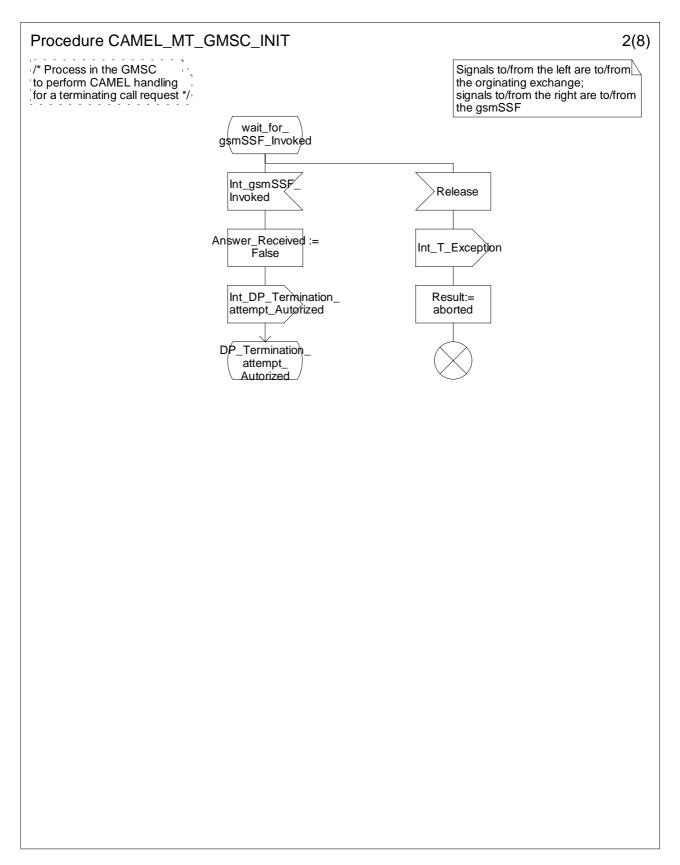
Figure 4.30b: Procedure CAMEL\_MT\_GMSC\_INIT (sheet 2)
