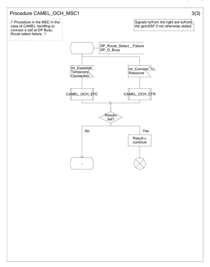
Figure 4.14c: Procedure CAMEL\_OCH\_MSC1 (sheet 3)
