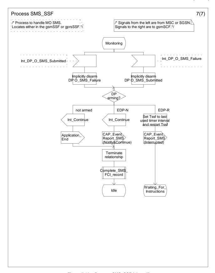
Figure 7.10g: Process SMS\_SSF (sheet 7)
