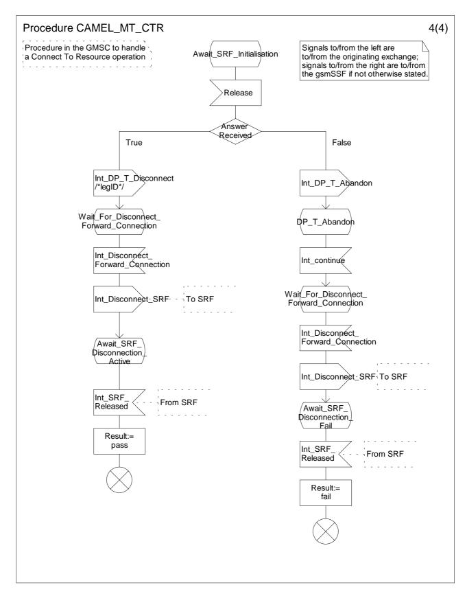
Figure 4.39d: Procedure CAMEL\_MT\_CTR (sheet 4)
