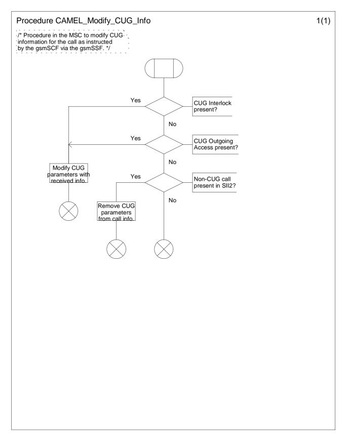
Figure 4.25: Procedure CAMEL\_Modify\_CUG\_Info (sheet 1)
