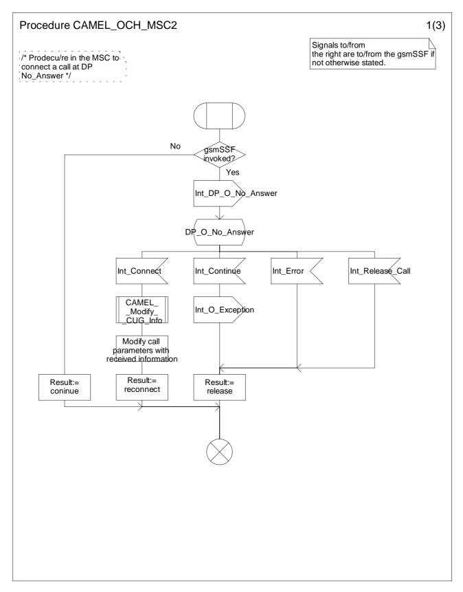
Figure 4.15a: Procedure CAMEL\_OCH\_MSC2 (sheet 1)
