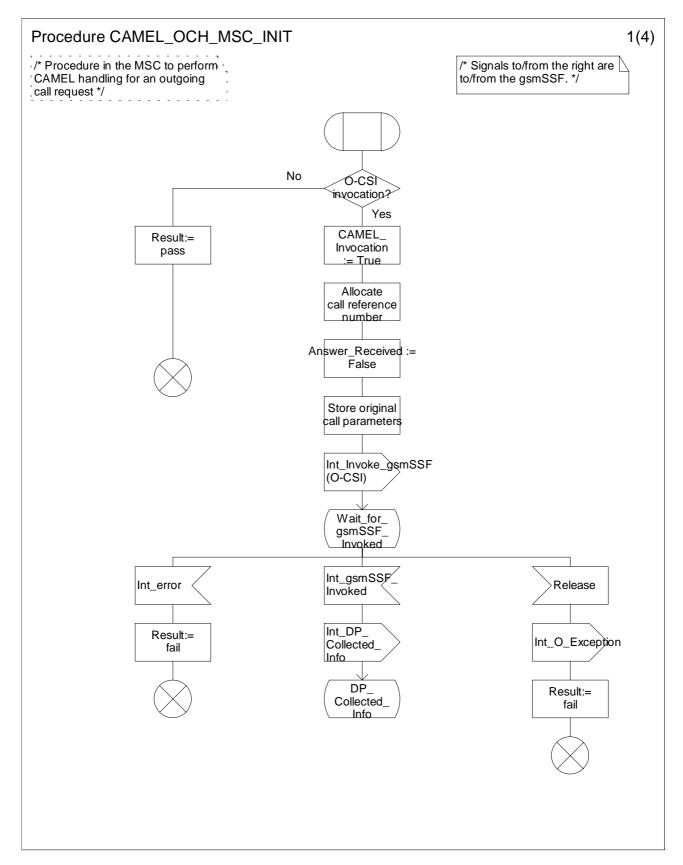
Figure 4.10a: Procedure CAMEL\_OCH\_MSC\_INIT (sheet 1)
