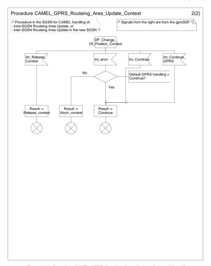
Figure 6.11b: Procedure CAMEL\_GPRS\_Routeing\_Area\_Update\_Context (sheet 2)
