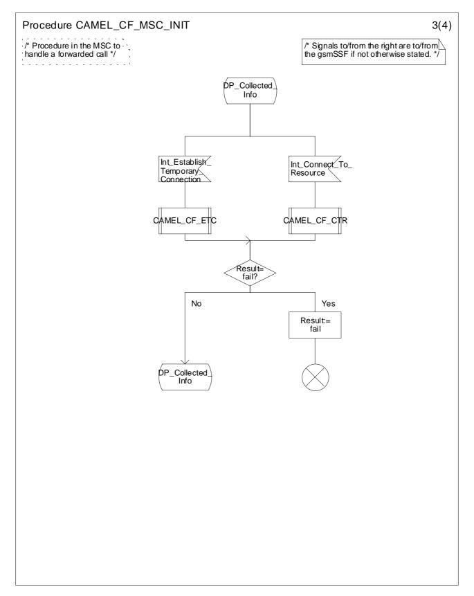
Figure 4.57c: Procedure CAMEL\_CF\_MSC\_INIT (sheet 3)
