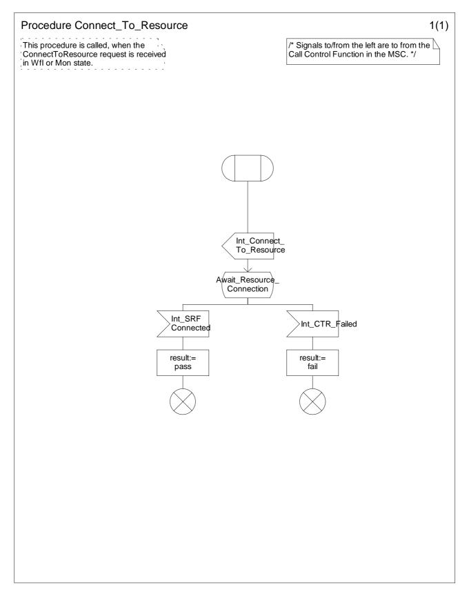
Figure 4.68a: Procedure Connect\_To\_Resource (sheet 1)
