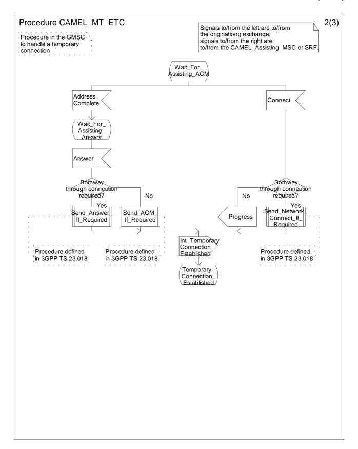
Figure 4.38b: Procedure CAMEL\_MT\_ETC (sheet 2)
