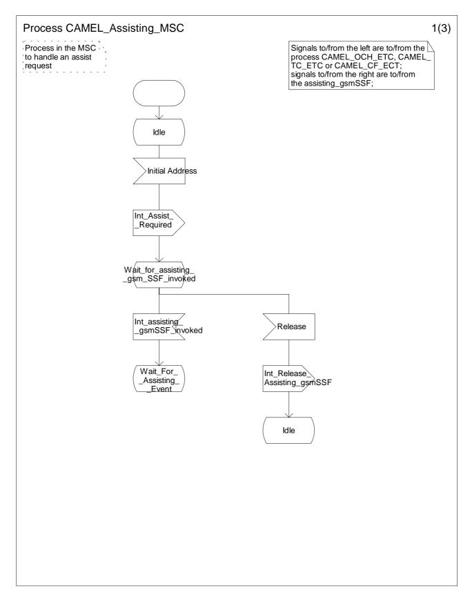
Figure 4.80a: Process CAMEL\_Assisting\_MSC (sheet 1)
