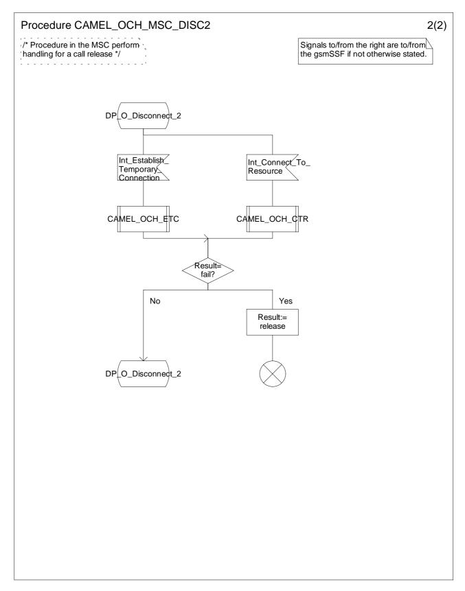
Figure 4.17b: Procedure CAMEL\_OCH\_MSC\_DISC2 (sheet 2)
