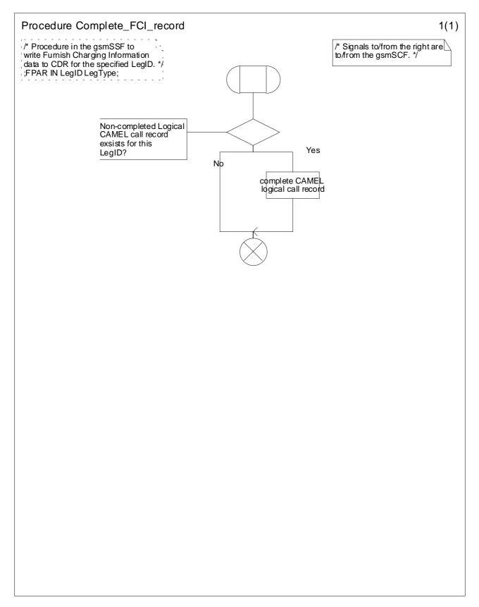
Figure 4.73a: Procedure Complete\_FCI\_record (sheet 1)
