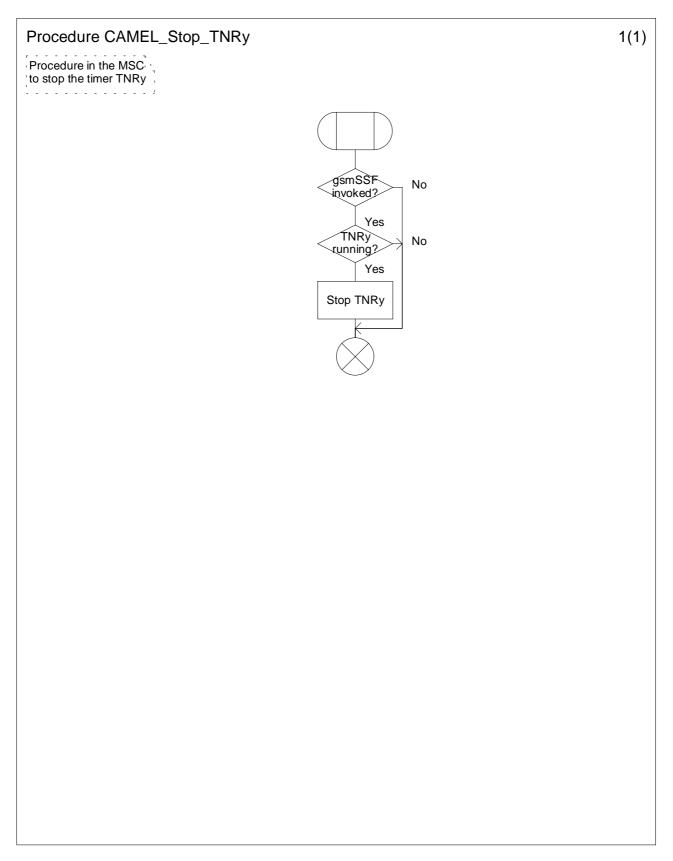
Figure 4.23: Procedure CAMEL\_Stop\_TNRy (sheet 1)
