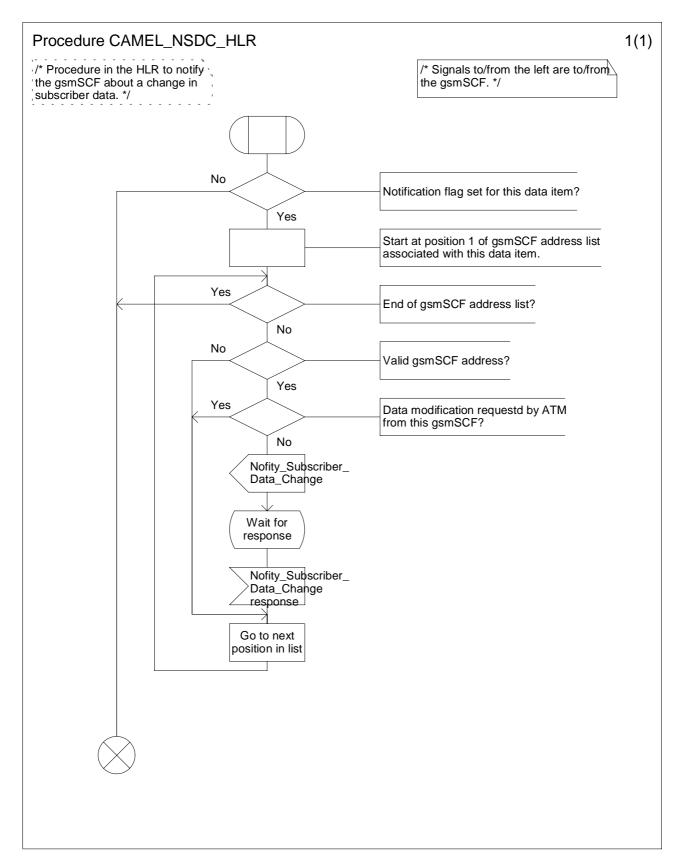
Figure 10.8: Procedure CAMEL\_NSDC\_HLR (sheet1)
