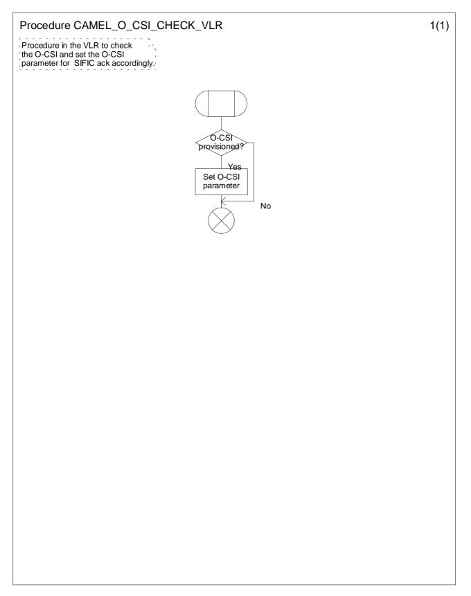
Figure 4.49: Procedure CAMEL\_O\_CSI\_Check\_VLR (sheet 1)
