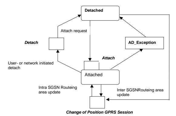
Figure 6.3: GPRS Attach/Detach State Model
