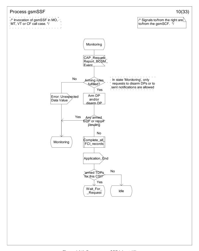
Figure 4.64j: Process gsmSSF (sheet 10)
