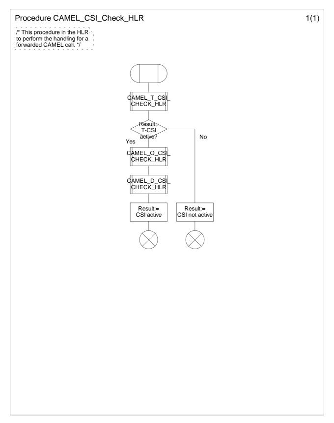
Figure 4.42: Procedure CAMEL\_CSI\_Check\_HLR (sheet 1)
