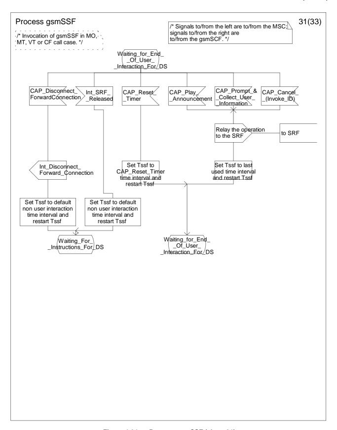
Figure 4.64ee: Process gsmSSF (sheet 31)
