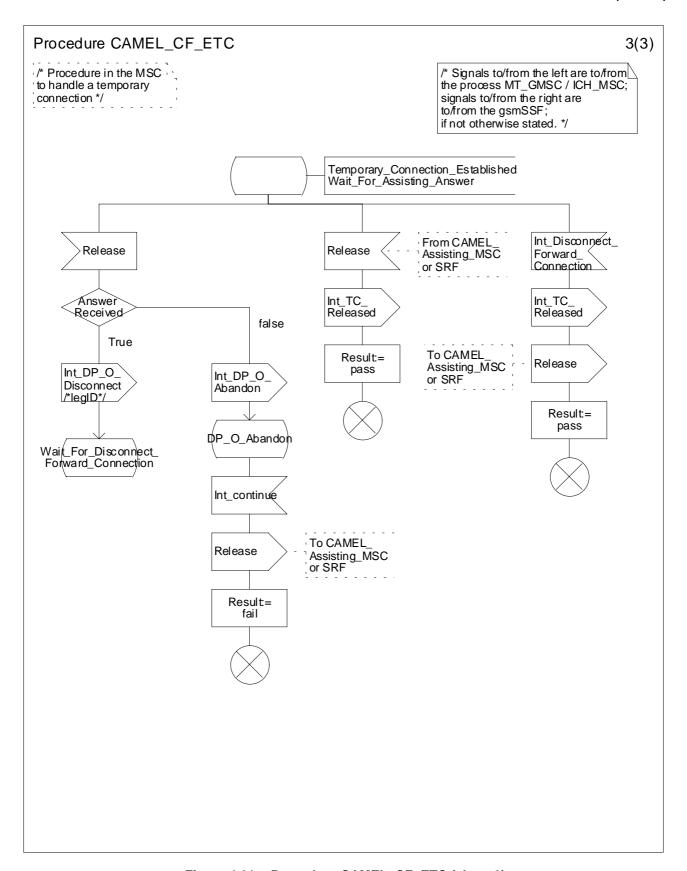
Figure 4.61c: Procedure CAMEL\_CF\_ETC (sheet 3)
