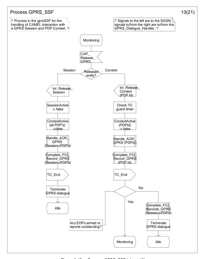
Figure 6.17m: Process GPRS\_SSF (sheet 13)
