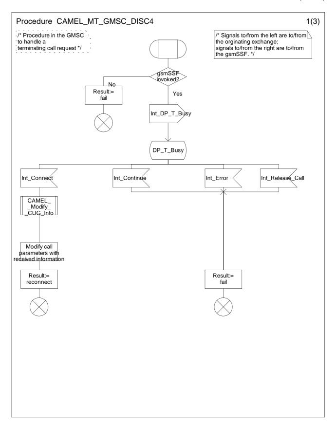
Figure 4.35a: Procedure CAMEL\_MT\_GMSC\_DISC4 (sheet 1)
