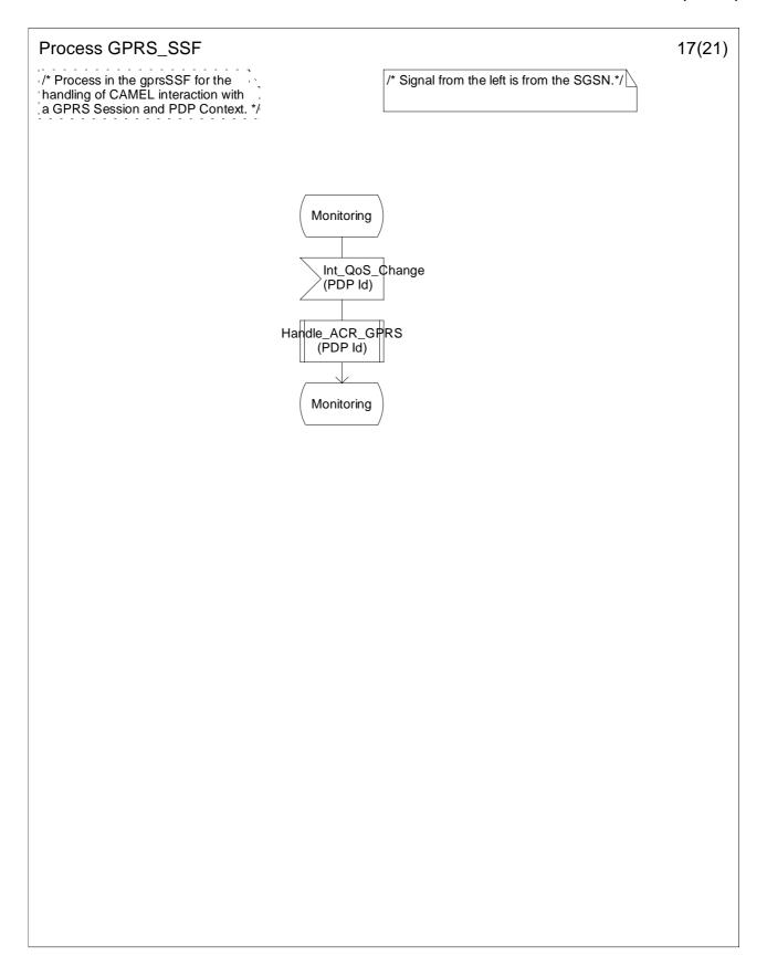
Figure 6.17q: Process GPRS\_SSF (sheet 17)
