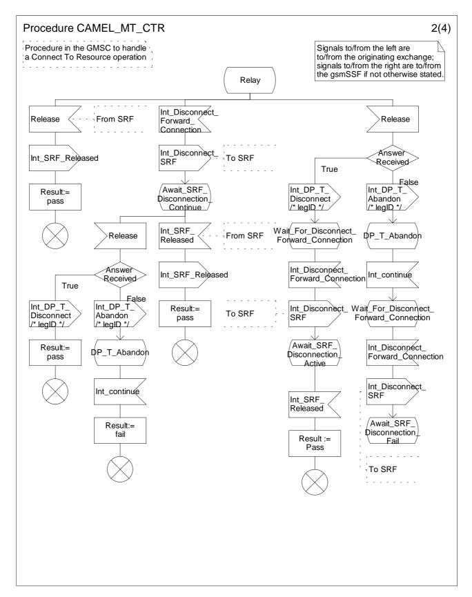
Figure 4.39b: Procedure CAMEL\_MT\_CTR (sheet 2)
