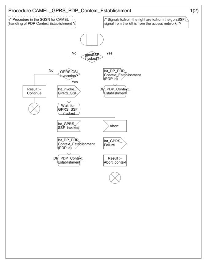
Figure 6.12a: Procedure CAMEL\_GPRS\_PDP\_Context\_Establishment (sheet 1)
