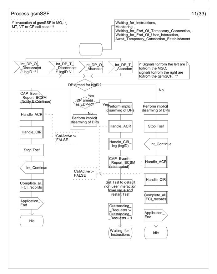
Figure 4.64k: Process gsmSSF (sheet 11)
