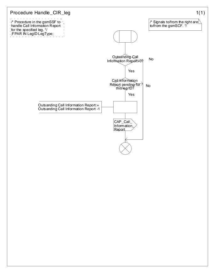
Figure 4.72a: Procedure Handle\_CIR\_leg (sheet 1)
