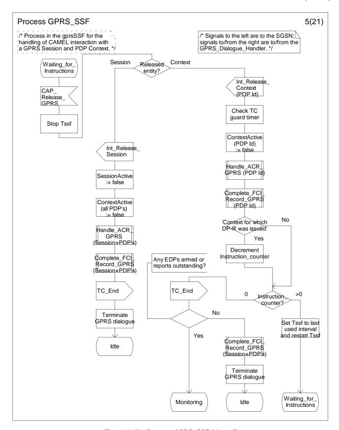
Figure 6.17e: Process GPRS\_SSF (sheet 5)
