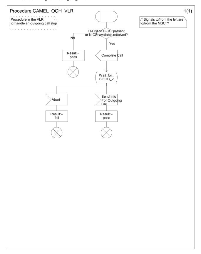
Figure 4.27a: Procedure CAMEL\_OCH\_VLR (sheet 1)
