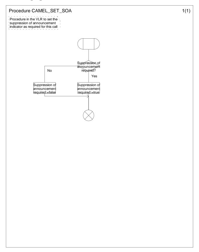
Figure 4.47: Procedure CAMEL\_SET\_SOA (sheet 1)
