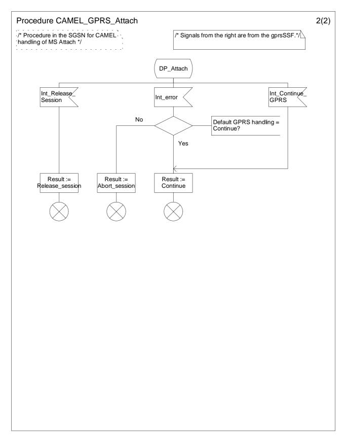
Figure 6.8b: Procedure CAMEL\_GPRS\_Attach (sheet 2)
