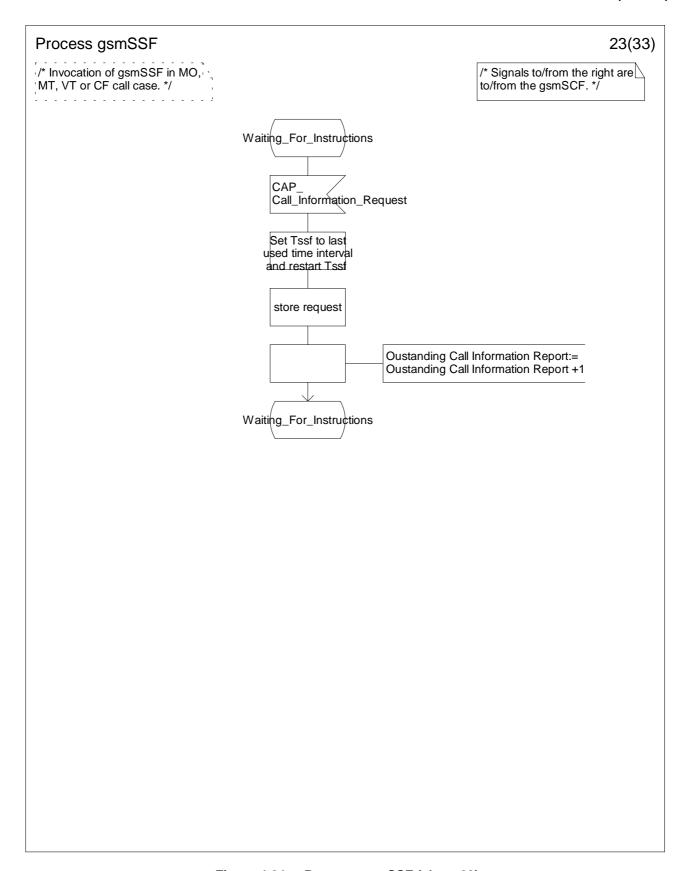
Figure 4.64w: Process gsmSSF (sheet 23)
