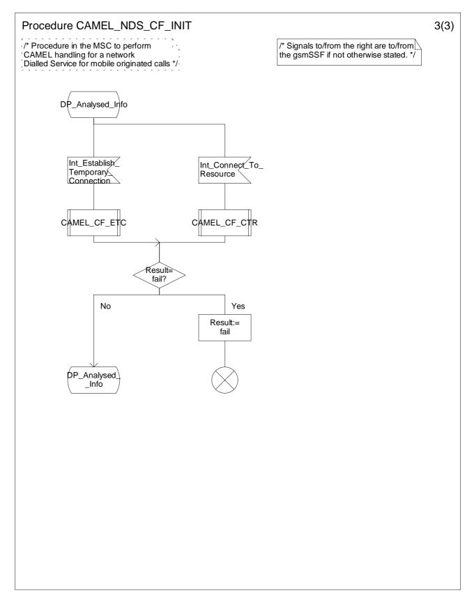
Figure 4.59c: Procedure CAMEL\_NDS\_CF\_INIT (sheet 3)
