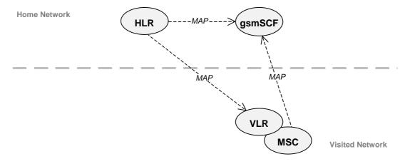
Figure 8.1: Functional architecture for support of SS Notifications
