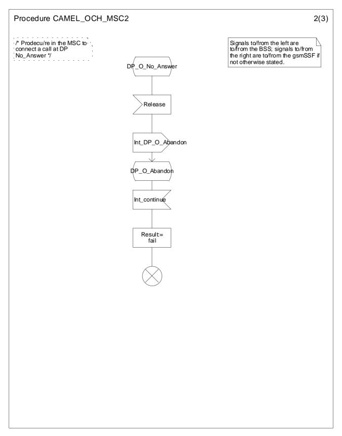
Figure 4.15b: Procedure CAMEL\_OCH\_MSC2 (sheet 2)
