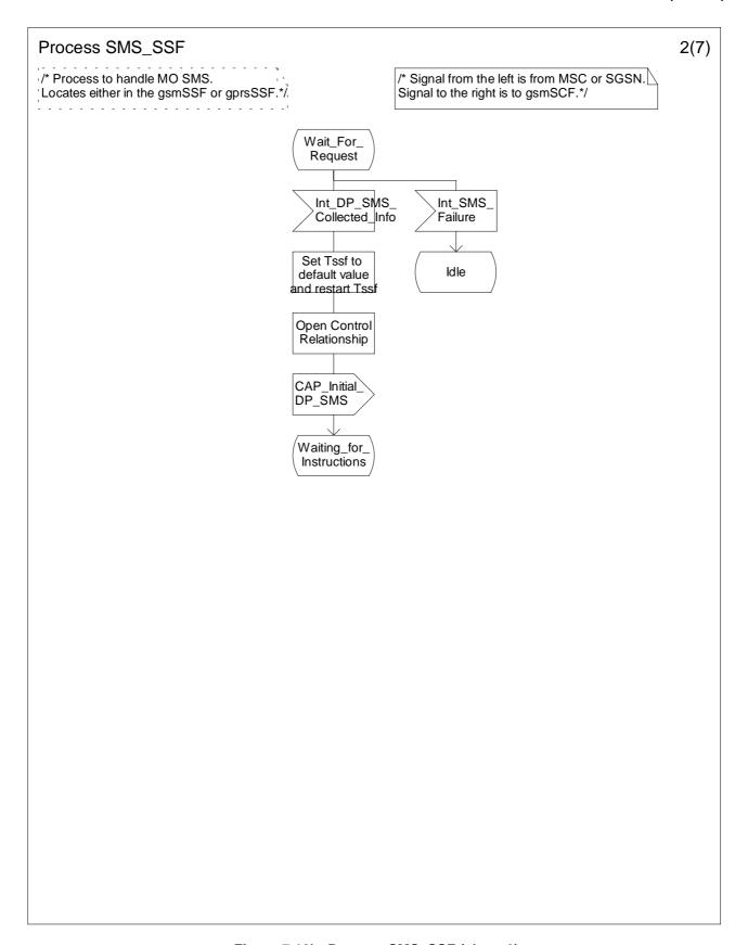
Figure 7.10b: Process SMS\_SSF (sheet 2)
