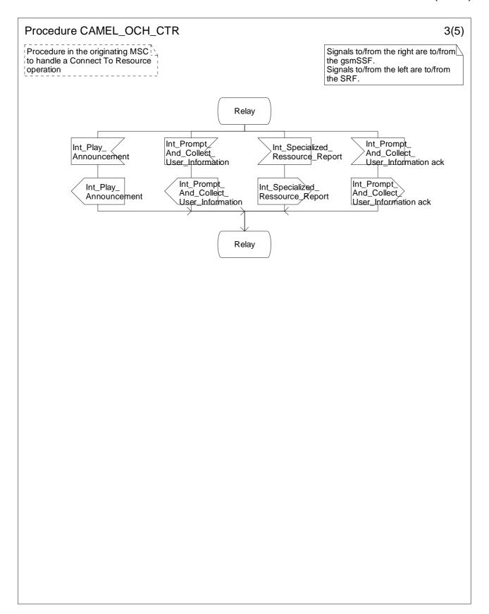
Figure 4.24-3: Procedure CAMEL\_OCH\_CTR (sheet 3)
