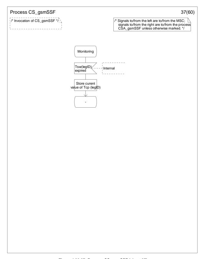
Figure 4.96-37: Process CS\_gsmSSF (sheet 37)
