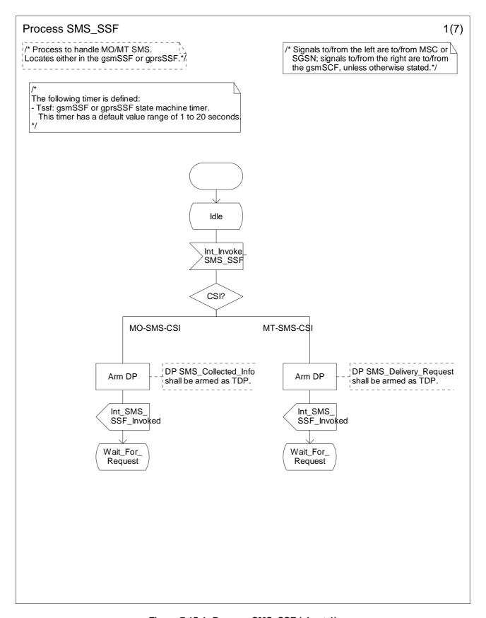
Figure 7.15-1: Process SMS\_SSF (sheet 1)
