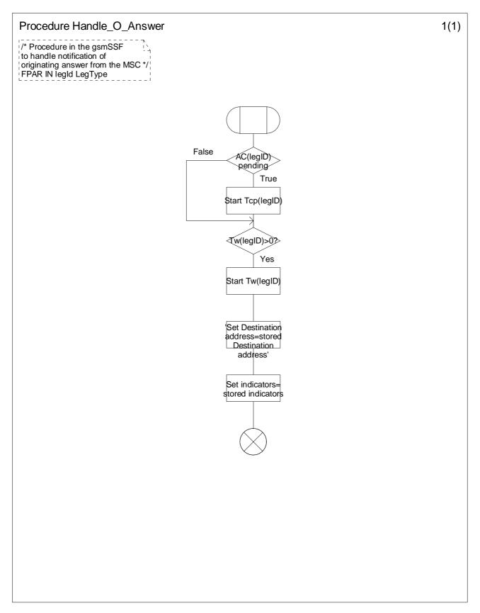
Figure 4.107-1: Procedure Handle\_O\_Answer (sheet 1)
