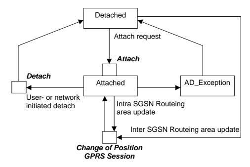
Figure 6.3: GPRS Attach/Detach State Model
