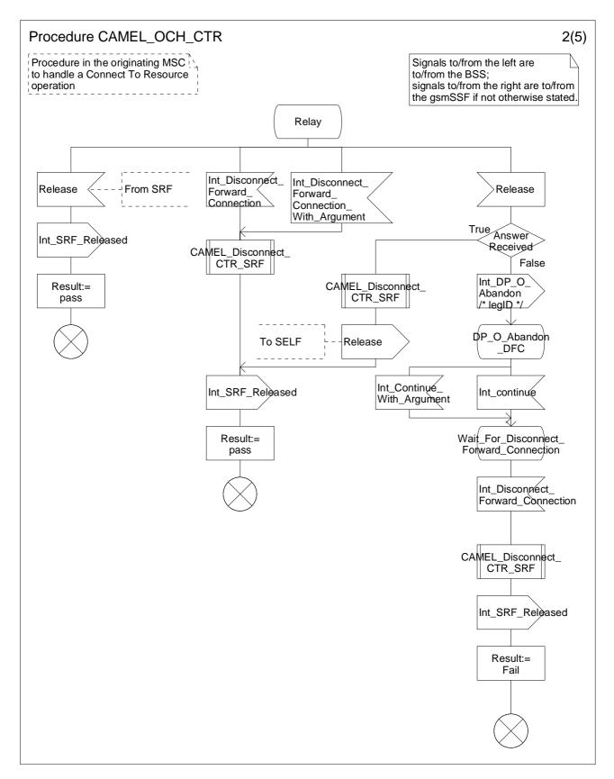
Figure 4.24-2: Procedure CAMEL\_OCH\_CTR (sheet 2)
