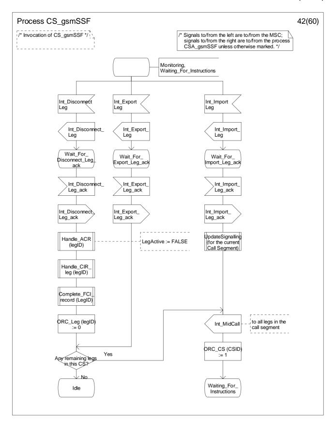
Figure 4.96-42: Process CS\_gsmSSF (sheet 42)
