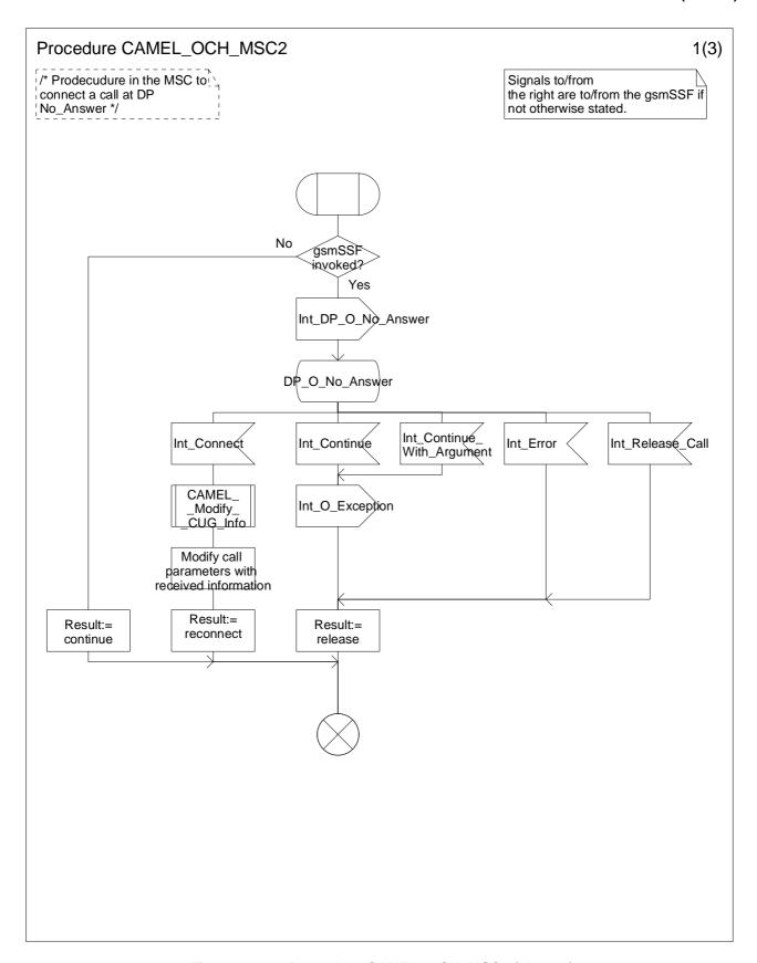
Figure 4.17-1: Procedure CAMEL\_OCH\_MSC2 (sheet 1)
