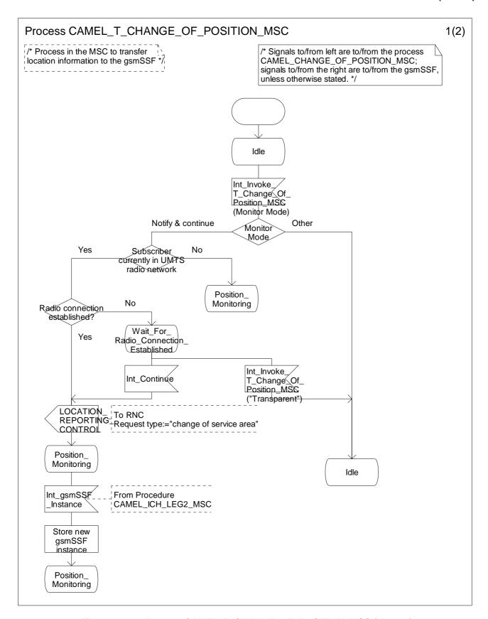
Figure 4.72-1: Process CAMEL\_T\_CHANGE\_OF\_POSITION\_MSC (sheet 1)
