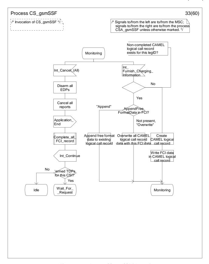
Figure 4.96-33: Process CS\_gsmSSF (sheet 33)
