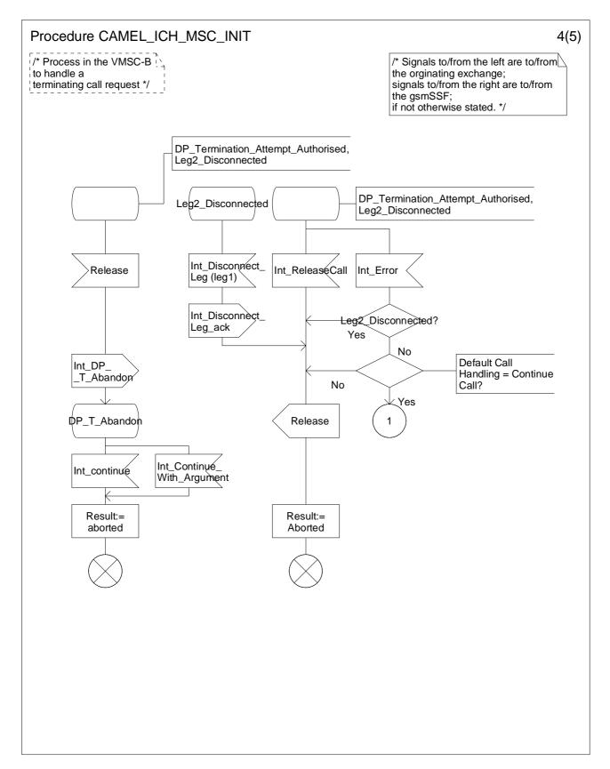
Figure 4.66-4: Procedure CAMEL\_ICH\_MSC\_INIT (sheet 4)
