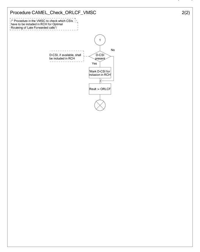
Figure 4.74-2: Procedure CAMEL\_Check\_ORLCF\_VMSC (sheet 2)
