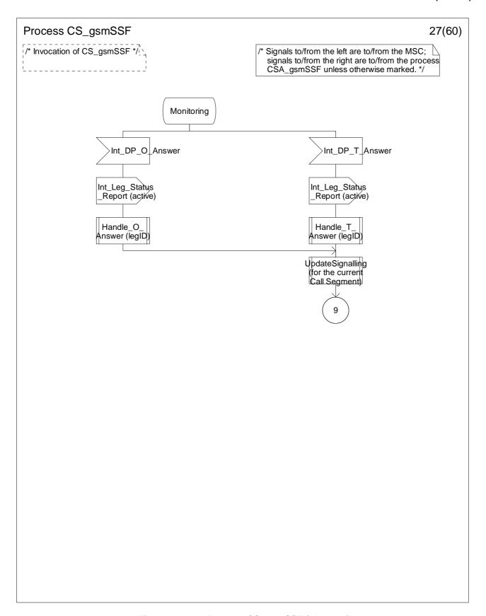
Figure 4.96-27: Process CS\_gsmSSF (sheet 27)
