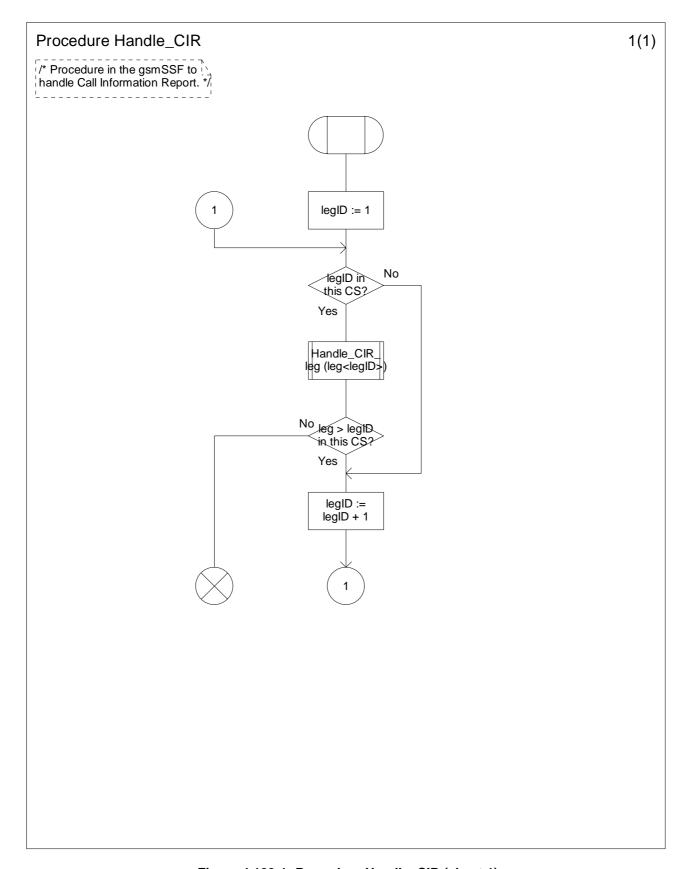
Figure 4.103-1: Procedure Handle\_CIR (sheet 1)
