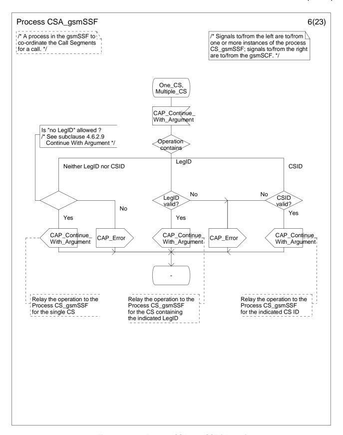
Figure 4.113-6: Process CSA\_gsmSSF (sheet 6)
