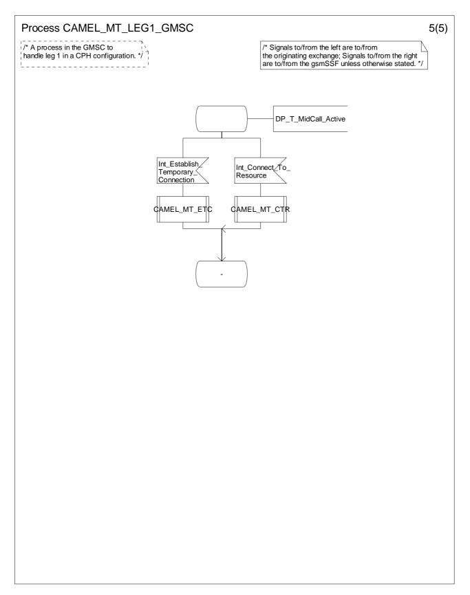
Figure 4.53-5: Process CAMEL\_MT\_LEG1\_GMSC (sheet 5)
