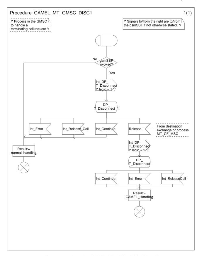
Figure 4.43-1: Procedure CAMEL\_MT\_GMSC\_DISC1 (sheet 1)
