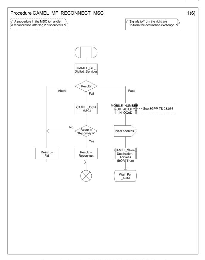
Figure 4.85-1: Procedure CAMEL\_MF\_RECONNECT\_MSC (sheet 1)
