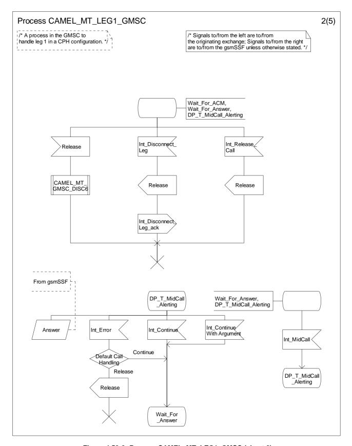
Figure 4.53-2: Process CAMEL\_MT\_LEG1\_GMSC (sheet 2)
