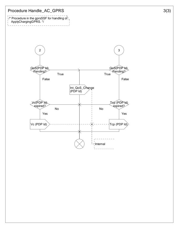
Figure 6.19-3: Procedure Handle\_AC\_GPRS (sheet 3)
