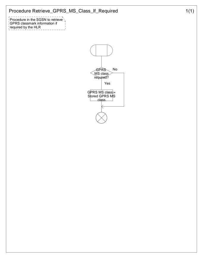
Figure 11.6-1: Procedure Retrieve\_GPRS\_MS\_Class\_If\_Required (sheet 1)
