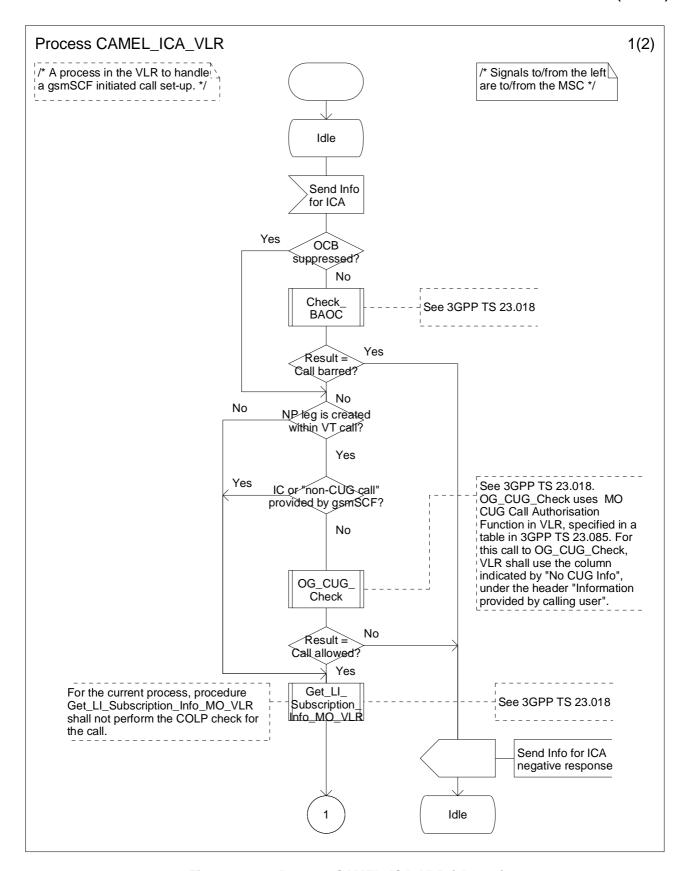
Figure 4.92-1: Process CAMEL\_ICA\_VLR (sheet 1)
