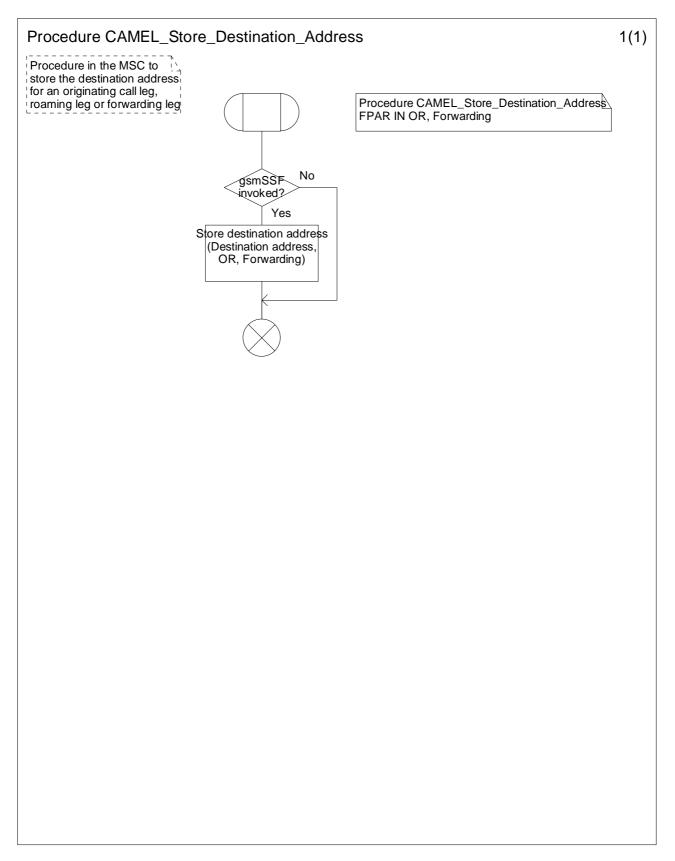
Figure 4.27-1: Procedure CAMEL\_Store\_Destination\_Address (sheet 1)
