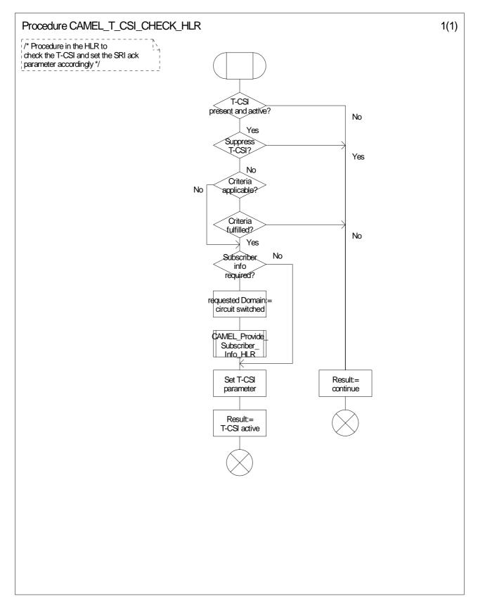
Figure 4.59-1: Procedure CAMEL\_T\_CSI\_CHECK\_HLR (sheet 1)
