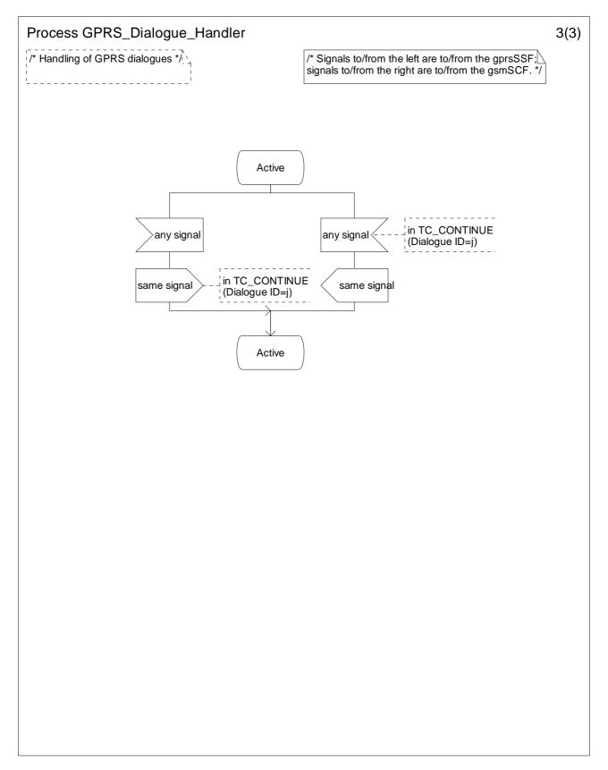
Figure 6.18-3: Process GPRS\_Dialogue\_Handler (sheet 3)
