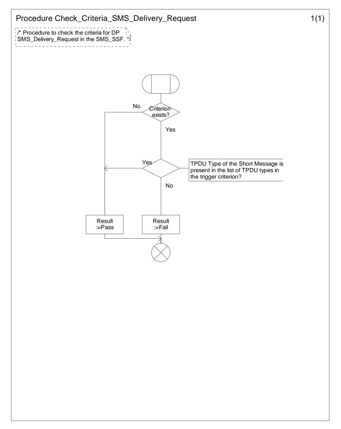
Figure 7.16-1: Procedure Check\_Criteria\_SMS\_Delivery\_Request (Sheet 1)
