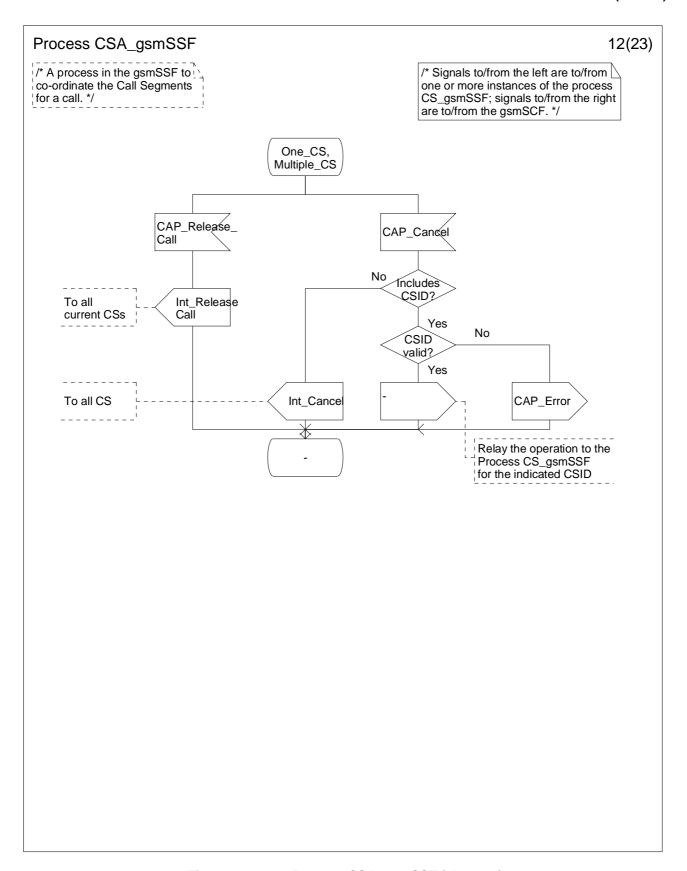
Figure 4.113-12: Process CSA\_gsmSSF (sheet 12)
