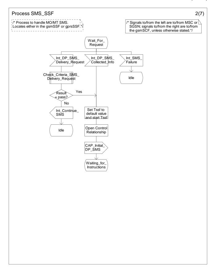
Figure 7.15-2: Process SMS\_SSF (sheet 2)
