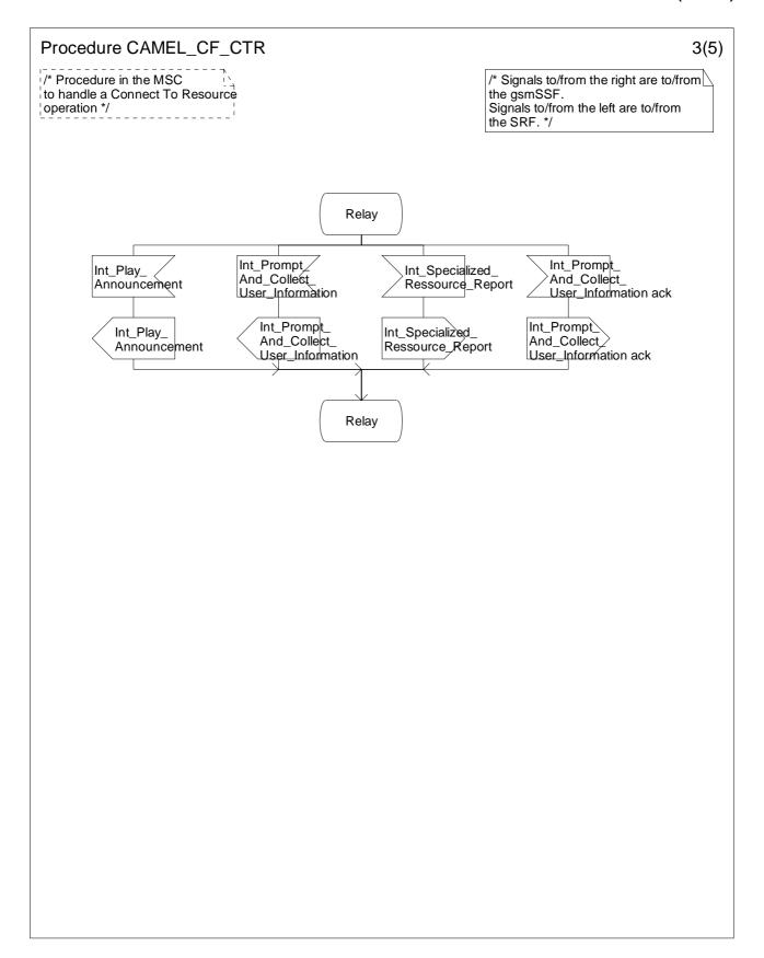
Figure 4.82-3: Procedure CAMEL\_CF\_CTR (sheet 3)
