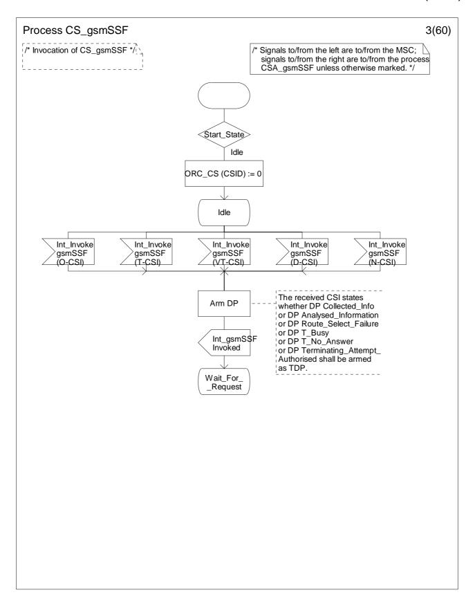
Figure 4.96-3: Process CS\_gsmSSF (sheet 3)
