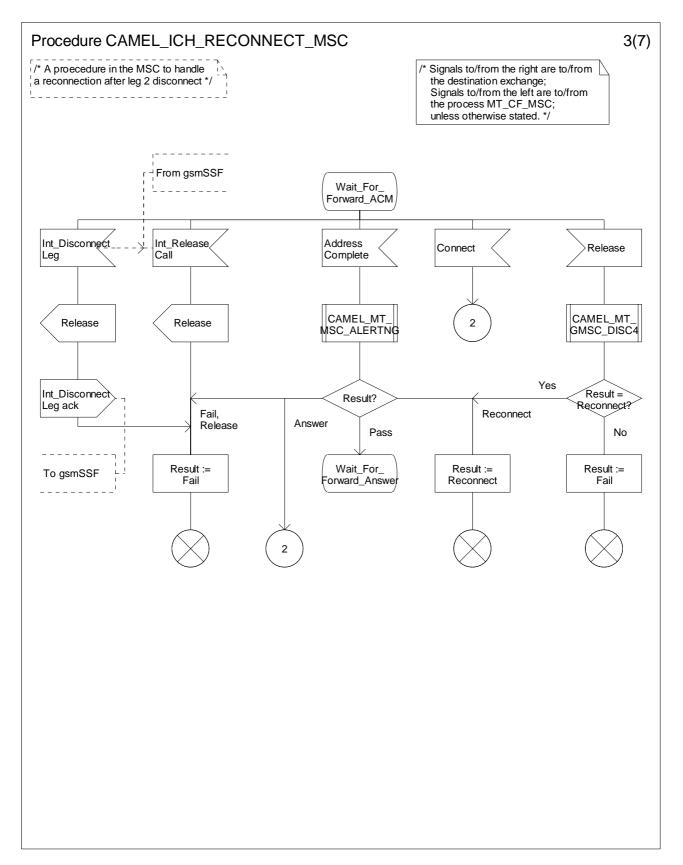
Figure 4.71-3: Procedure CAMEL\_ICH\_RECONNECT\_MSC (sheet 3)
