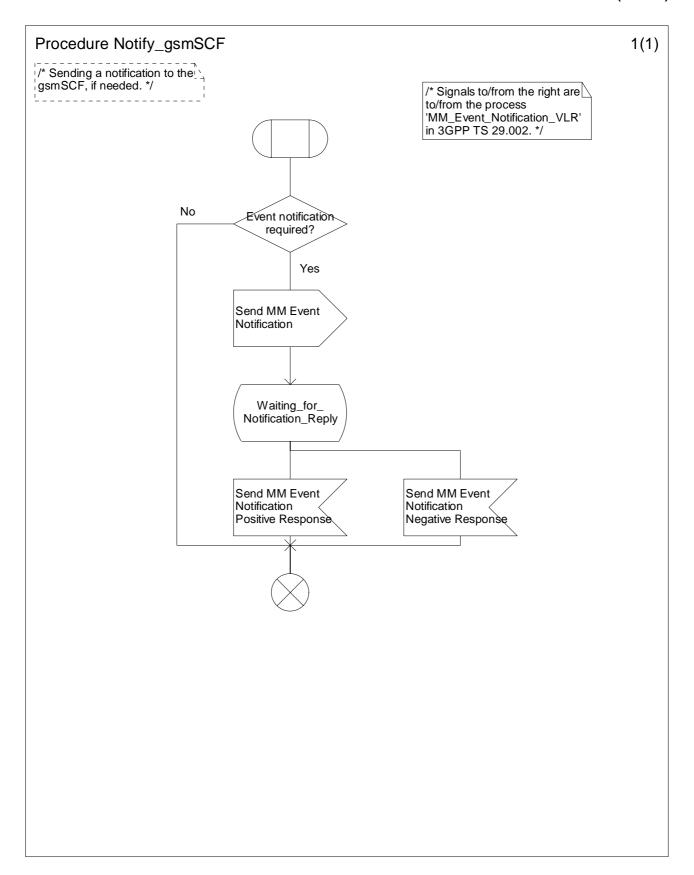
Figure 9.3-1: Procedure Notify\_gsmSCF (sheet 1)
