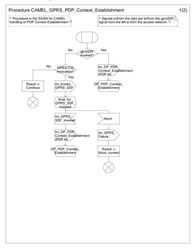
Figure 6.12-1: Procedure CAMEL\_GPRS\_PDP\_Context\_Establishment (sheet 1)
