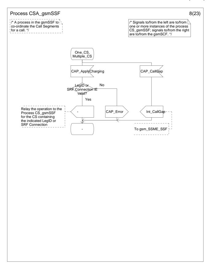
Figure 4.113-8: Process CSA\_gsmSSF (sheet 8)
