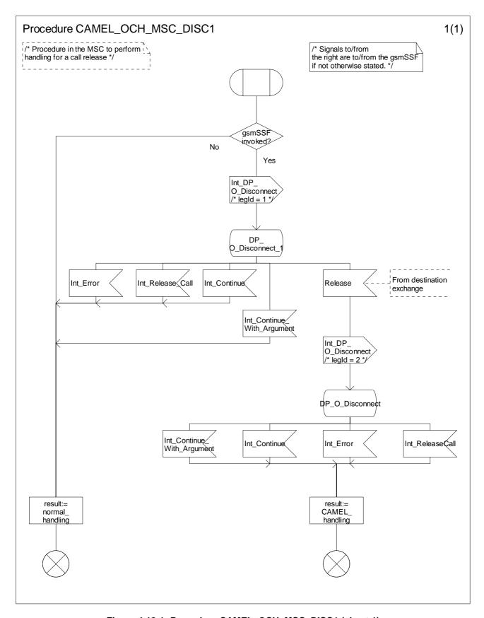
Figure 4.18-1: Procedure CAMEL\_OCH\_MSC\_DISC1 (sheet 1)
