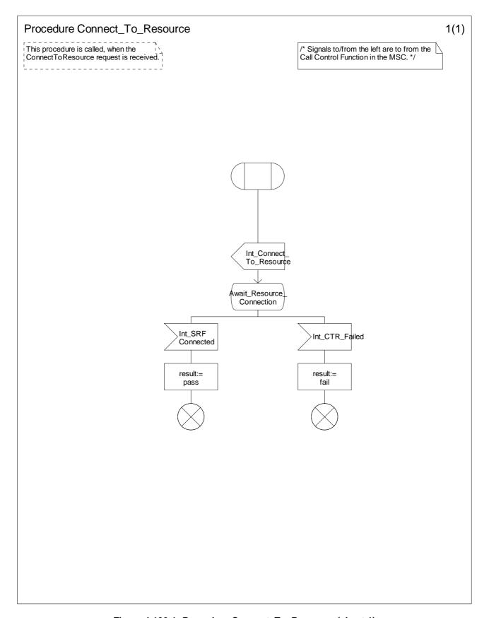
Figure 4.100-1: Procedure Connect\_To\_Resource (sheet 1)
