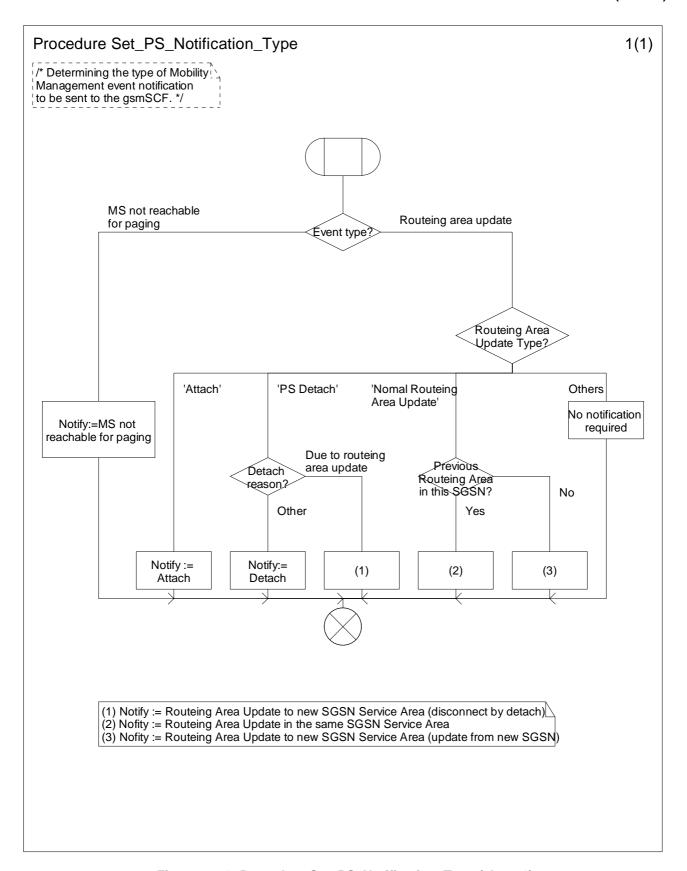
Figure 9.6-1: Procedure Set\_PS\_Notification\_Type (sheet 1)
