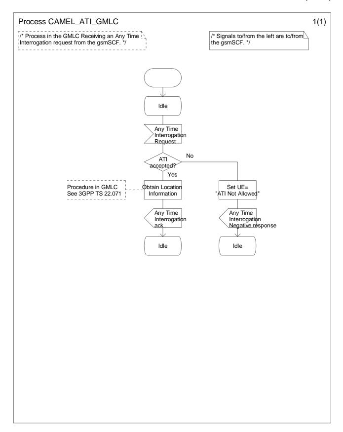
Figure 11.2-1: Process CAMEL\_ATI\_GMLC (sheet 1)
