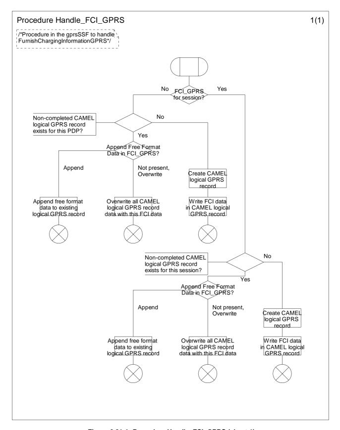
Figure 6.21-1: Procedure Handle\_FCI\_GPRS (sheet 1)
