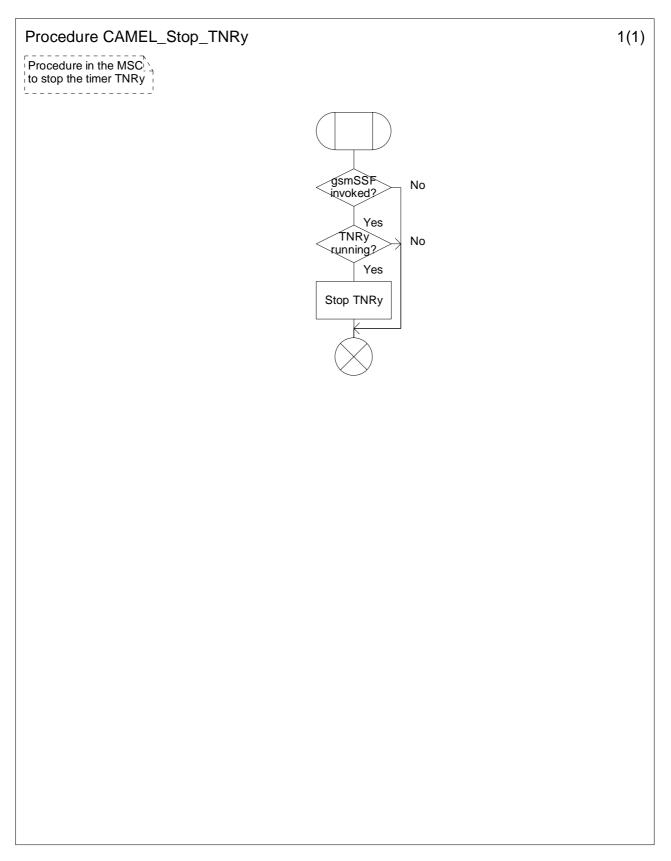
Figure 4.26-1: Procedure CAMEL\_Stop\_TNRy (sheet 1)
