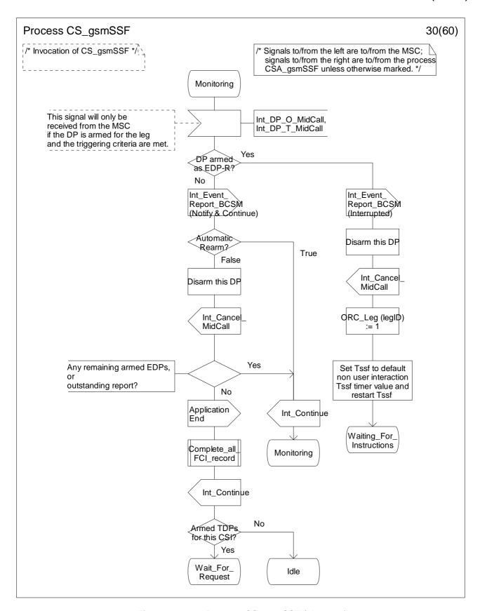
Figure 4.96-30: Process CS\_gsmSSF (sheet 30)
