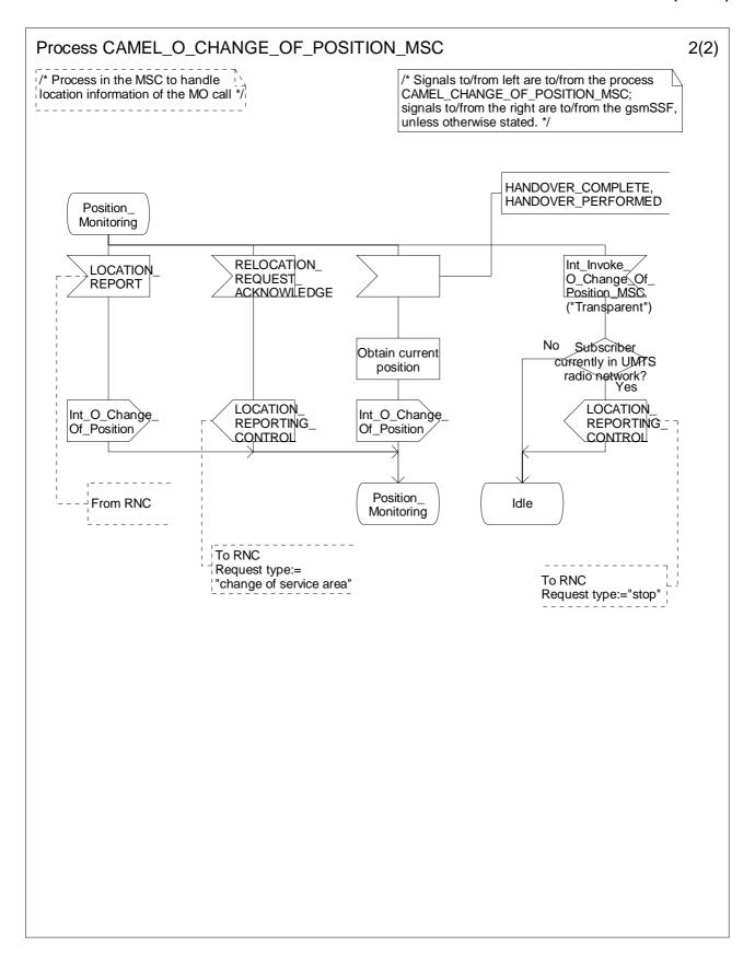
Figure 4.36-2: Process CAMEL\_O\_CHANGE\_OF\_POSITION\_MSC (sheet 2)
