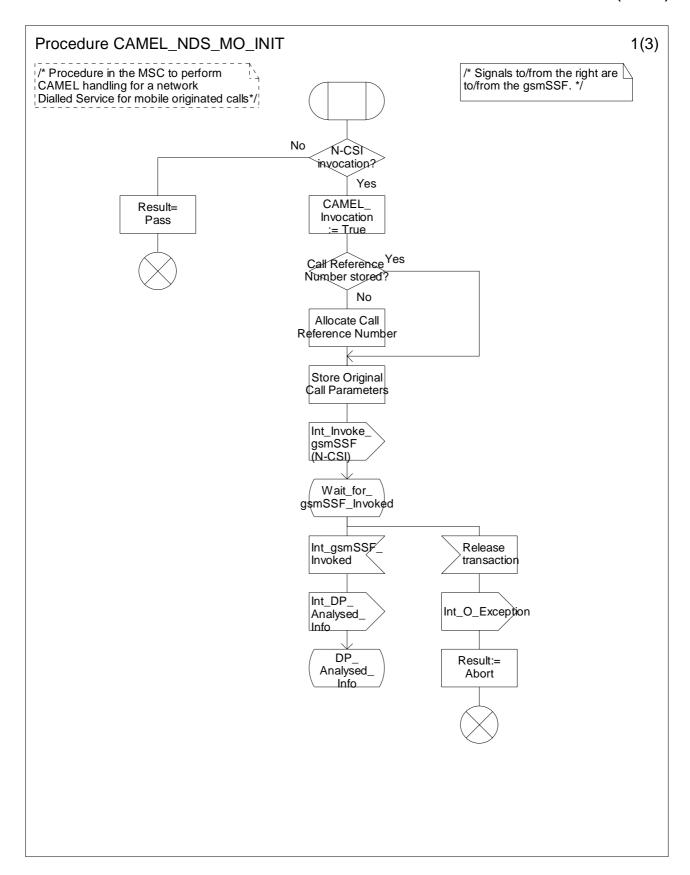
Figure 4.13-1: Procedure CAMEL\_NDS\_MO\_INIT (sheet 1)
