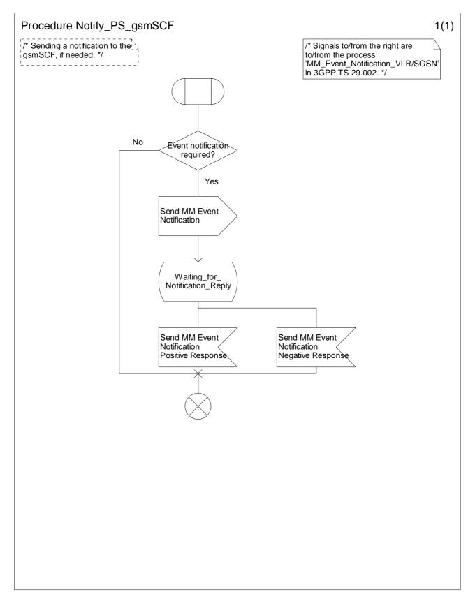
Figure 9.7-1: Procedure Notify\_PS\_gsmSCF (sheet 1)
