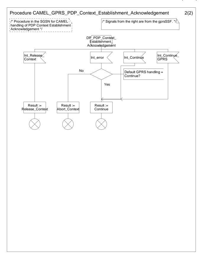
Figure 6.13-2: Procedure CAMEL\_GPRS\_PDP\_Context\_Establishment\_Acknowledgement (sheet 2)
