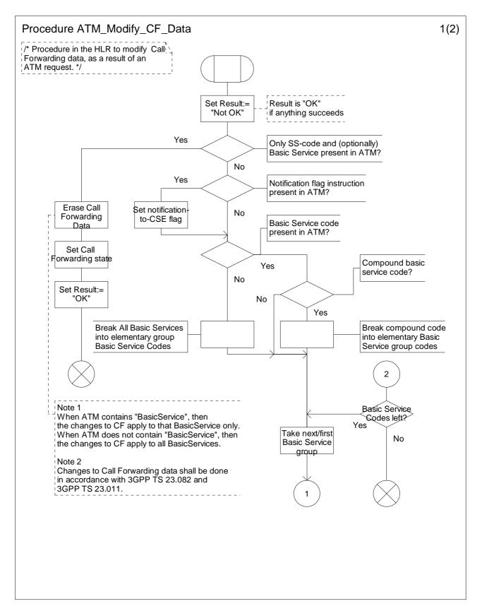
Figure 10.6-1: Procedure ATM\_Modify\_CF\_Data (sheet 1)
