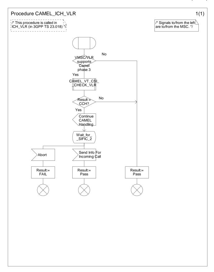
Figure 4.62-1: Procedure CAMEL\_ICH\_VLR (sheet 1)
