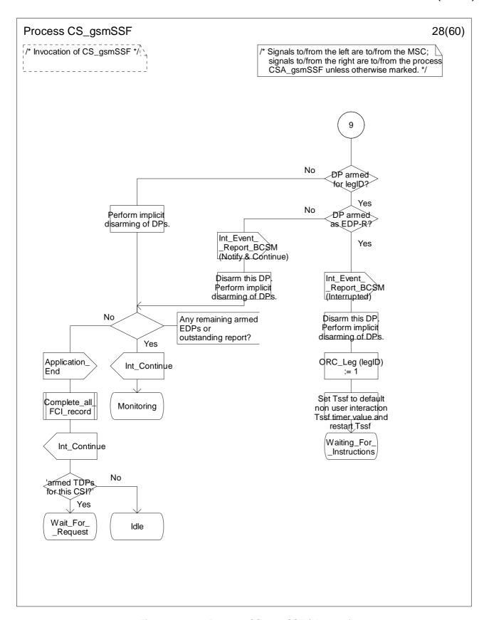
Figure 4.96-28: Process CS\_gsmSSF (sheet 28)
