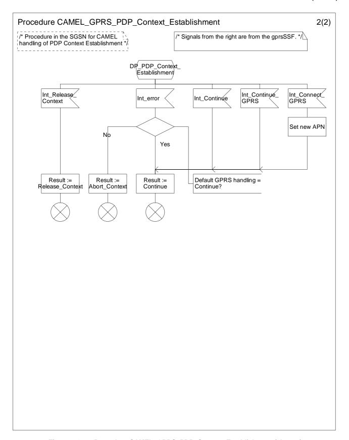
Figure 6.12-2: Procedure CAMEL\_GPRS\_PDP\_Context\_Establishment (sheet 2)
