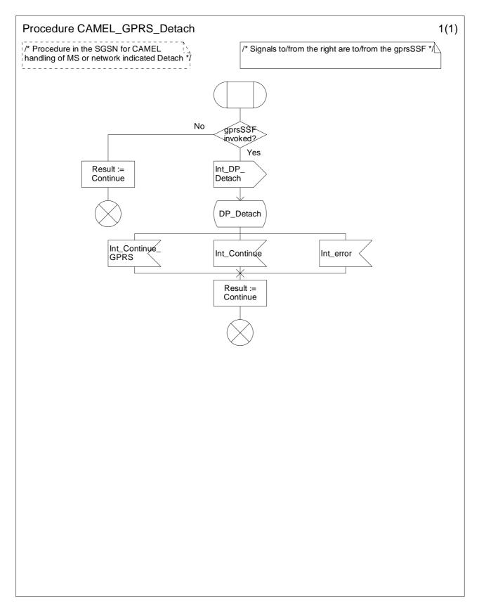
Figure 6.9-1: Procedure CAMEL\_GPRS\_Detach (sheet 1)
