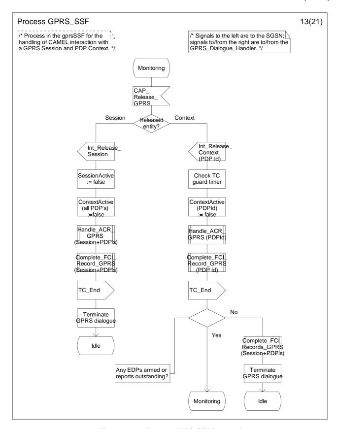
Figure 6.17-13: Process GPRS\_SSF (sheet 13)
