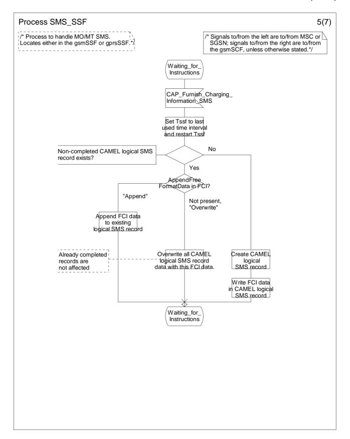
Figure 7.15-5: Process SMS\_SSF (sheet 5)
