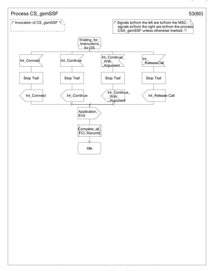
Figure 4.96-53: Process CS\_gsmSSF (sheet 53)
