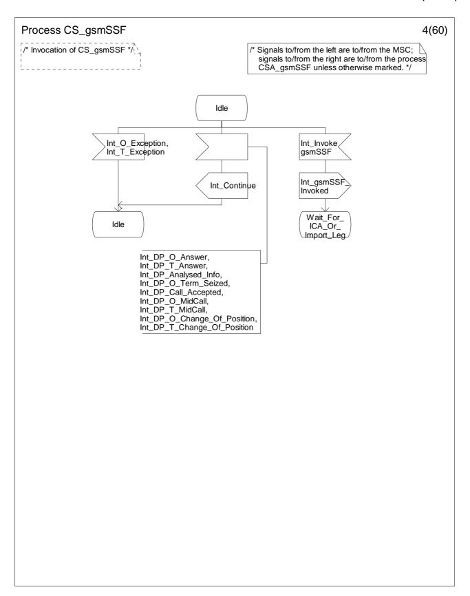
Figure 4.96-4: Process CS\_gsmSSF (sheet 4)
