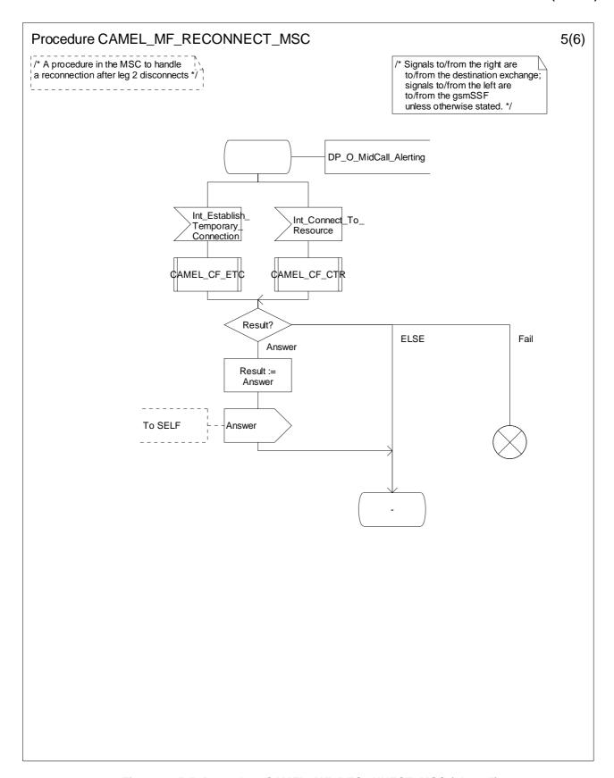
Figure 4.85-5: Procedure CAMEL\_MF\_RECONNECT\_MSC (sheet 5)
