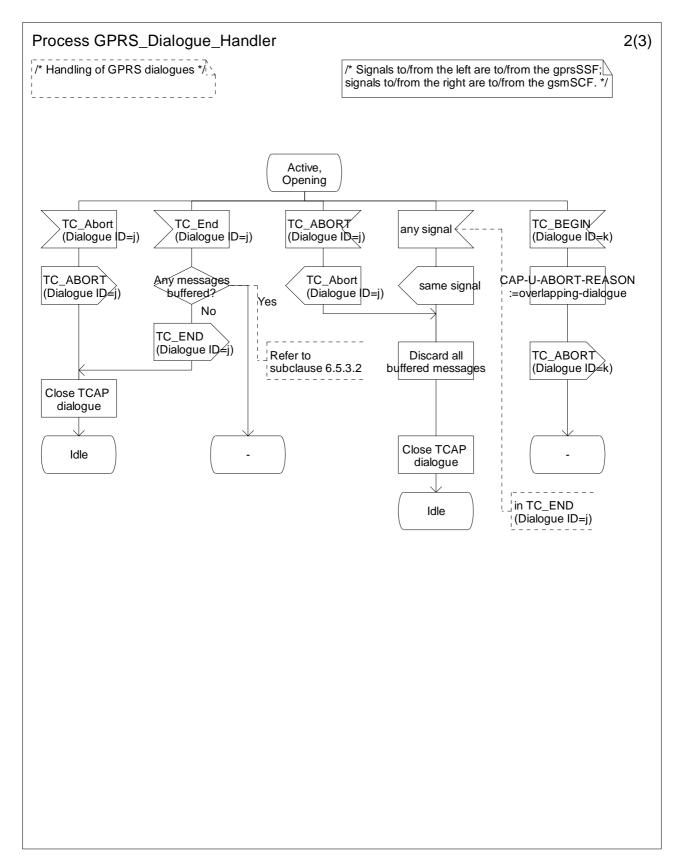
Figure 6.18-2: Process GPRS\_Dialogue\_Handler (sheet 2)
