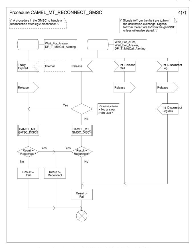
Figure 4.54-4: Procedure CAMEL\_MT\_RECONNECT\_GMSC (sheet 4)
