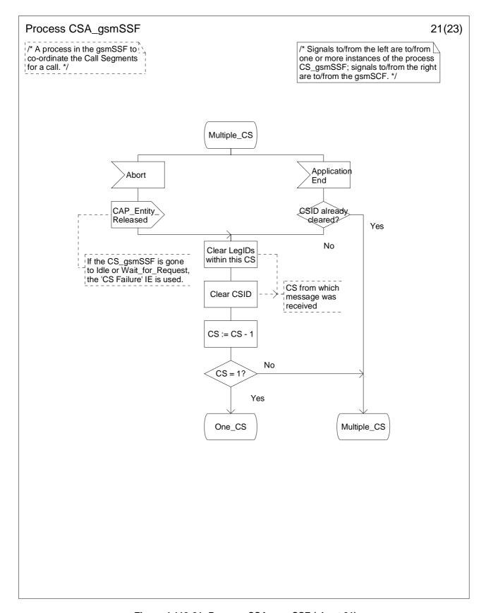
Figure 4.113-21: Process CSA\_gsmSSF (sheet 21)
