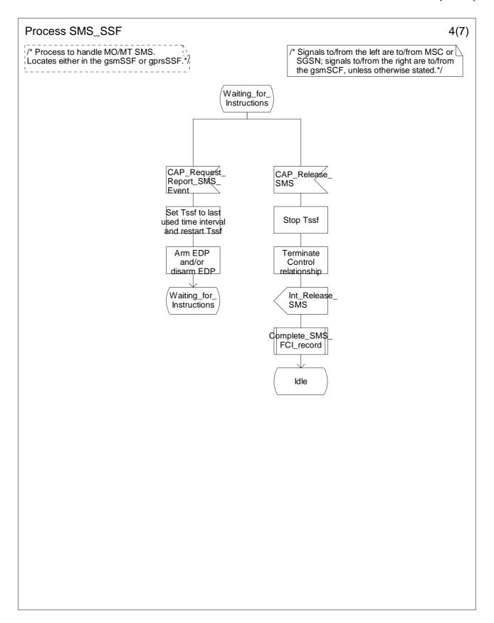
Figure 7.15-4: Process SMS\_SSF (sheet 4)
