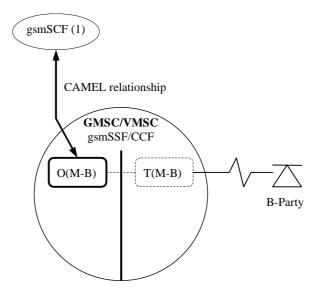
Figure 4.8: BCSM Scenario for gsmSCF Initiated New Call
