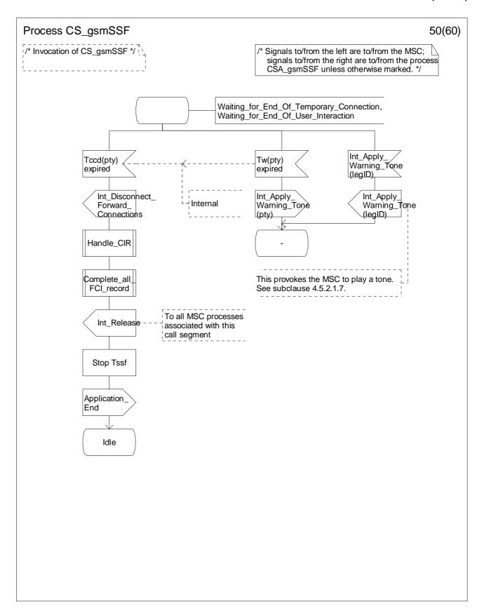
Figure 4.96-50: Process CS\_gsmSSF (sheet 50)
