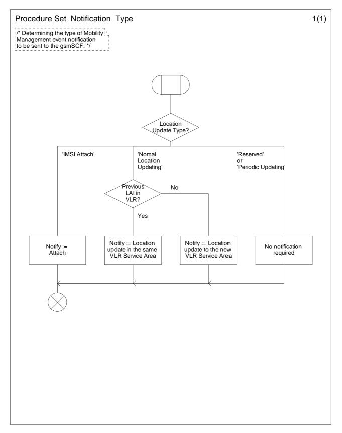
Figure 9.-1a: Procedure Set\_Notification\_Type (sheet 1)
