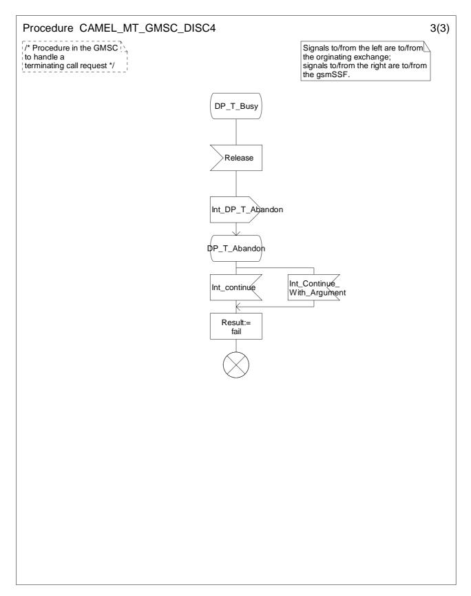
Figure 4.46-3: Procedure CAMEL\_MT\_GMSC\_DISC4 (sheet 3)
