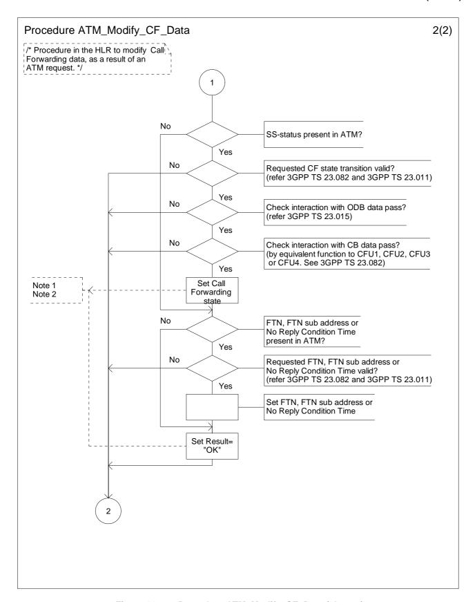
Figure 10.6-2: Procedure ATM\_Modify\_CF\_Data (sheet 2)
