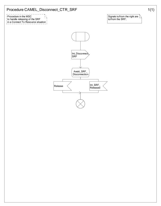
Figure 4.22-1: Procedure CAMEL\_Disconnect\_CTR\_SRF (sheet 1)
