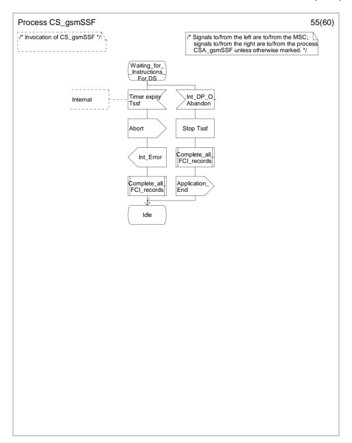
Figure 4.96-55: Process CS\_gsmSSF (sheet 55)
