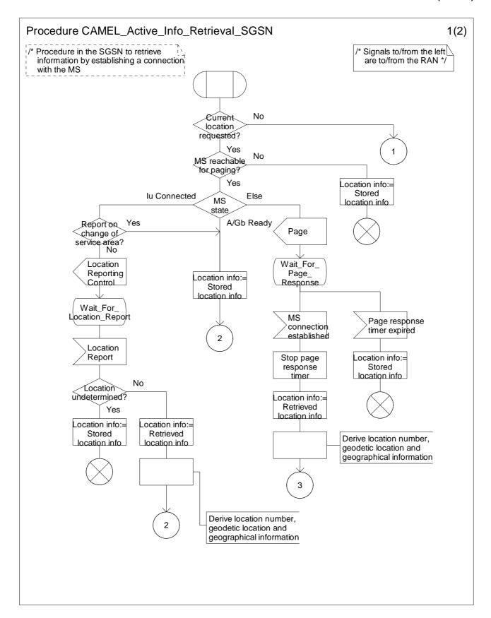
Figure 11.5-1: Procedure CAMEL\_Active\_Info\_Retrieval\_SGSN (sheet 1)
