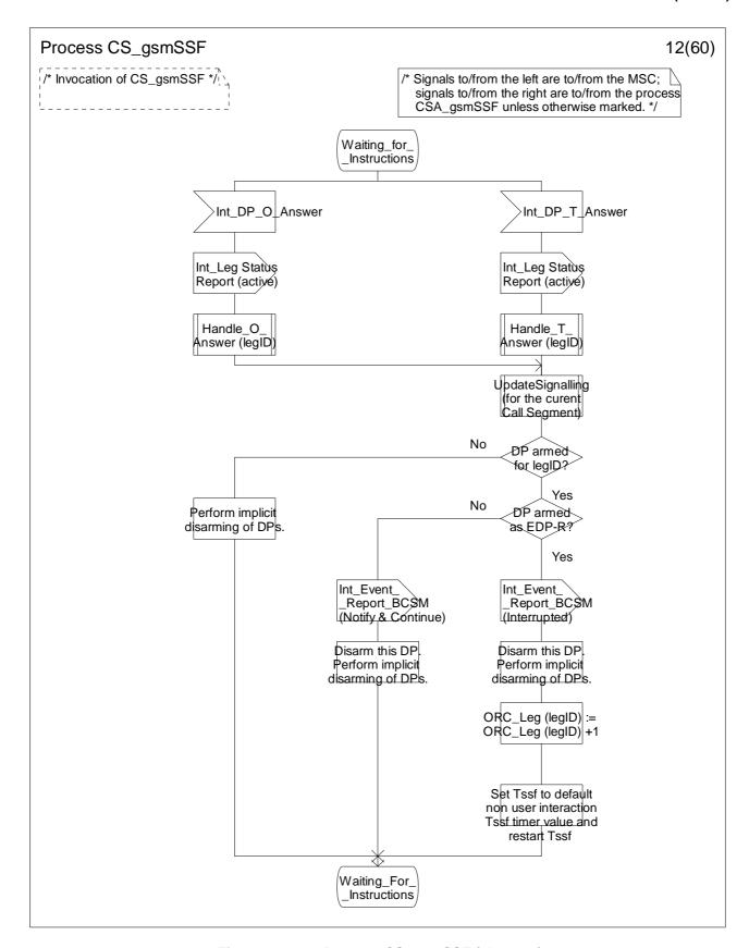
Figure 4.96-12: Process CS\_gsmSSF (sheet 12)
