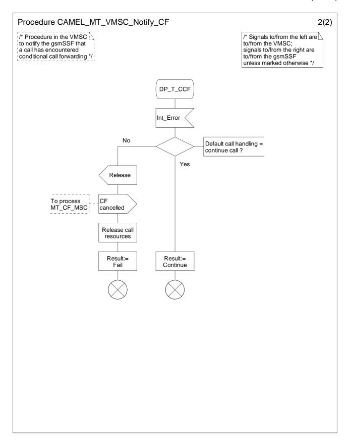
Figure 4.67-2: Procedure CAMEL\_MT\_VMSC\_Notify\_CF (sheet 2)
