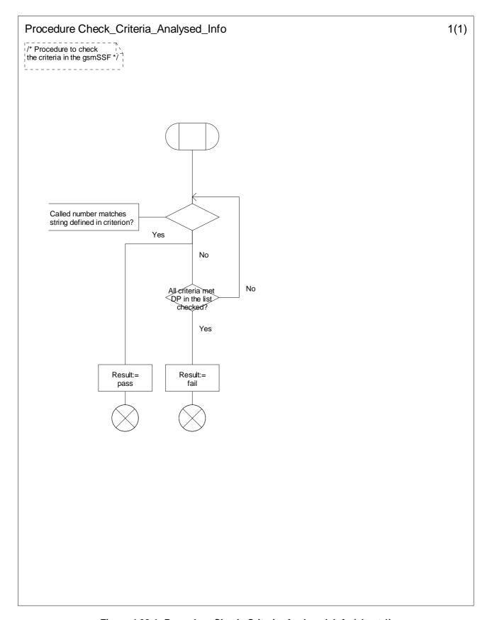
Figure 4.98-1: Procedure Check\_Criteria\_Analysed\_Info (sheet 1)
