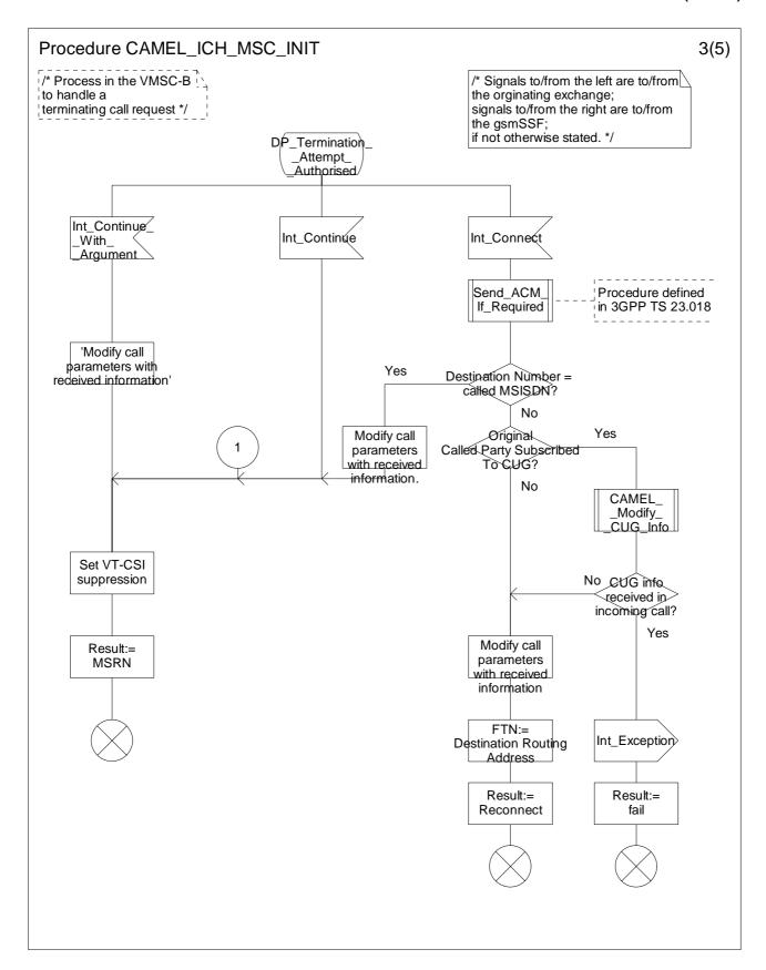
Figure 4.66-3: Procedure CAMEL\_ICH\_MSC\_INIT (sheet 3)
