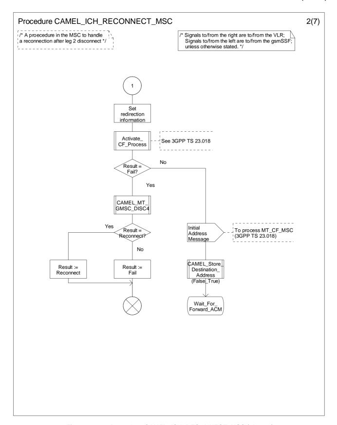
Figure 4.71-2: Procedure CAMEL\_ICH\_RECONNECT\_MSC (sheet 2)
