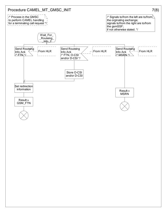
Figure 4.40-7: Procedure CAMEL\_MT\_GMSC\_INIT (sheet 7)
