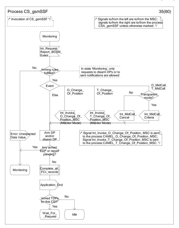
Figure 4.96-35: Process CS\_gsmSSF (sheet 35)
