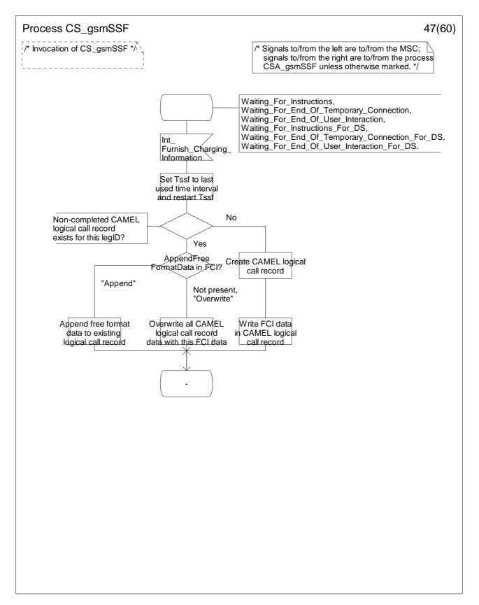
Figure 4.96-47: Process CS\_gsmSSF (sheet 47)
