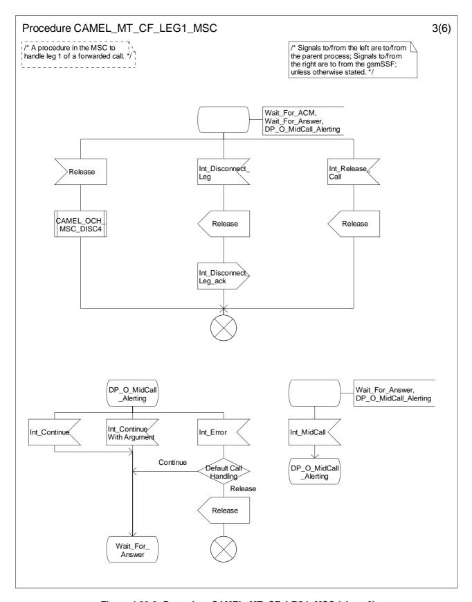
Figure 4.83-3: Procedure CAMEL\_MT\_CF\_LEG1\_MSC (sheet 3)
