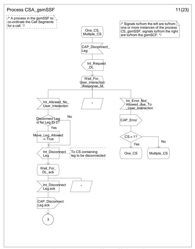
Figure 4.113-11: Process CSA\_gsmSSF (sheet 11)
