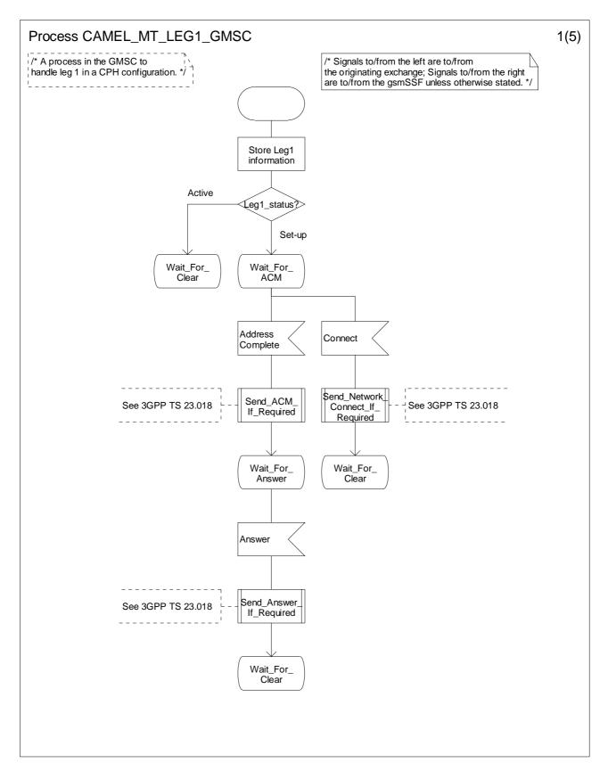
Figure 4.53-1: Process CAMEL\_MT\_LEG1\_GMSC (sheet 1)
