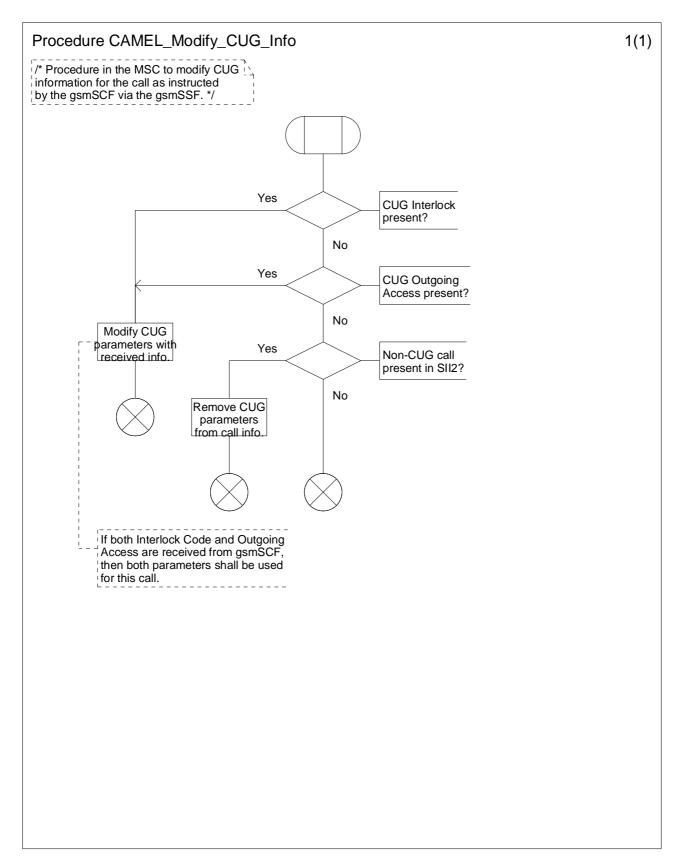
Figure 4.28-1: Procedure CAMEL\_Modify\_CUG\_Info (sheet 1)
