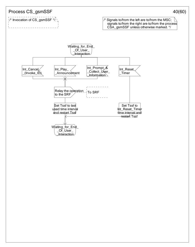
Figure 4.96-40: Process CS\_gsmSSF (sheet 40)
