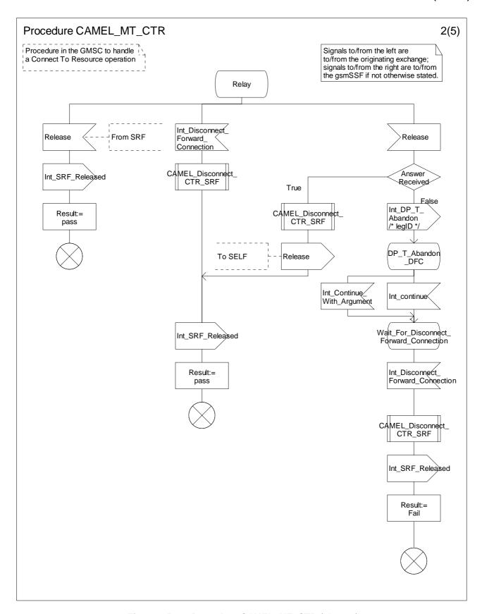
Figure 4.50-2: Procedure CAMEL\_MT\_CTR (sheet 2)
