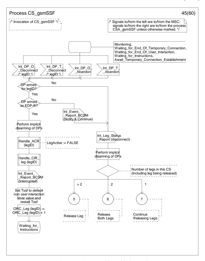
Figure 4.96-45: Process CS\_gsmSSF (sheet 45)
