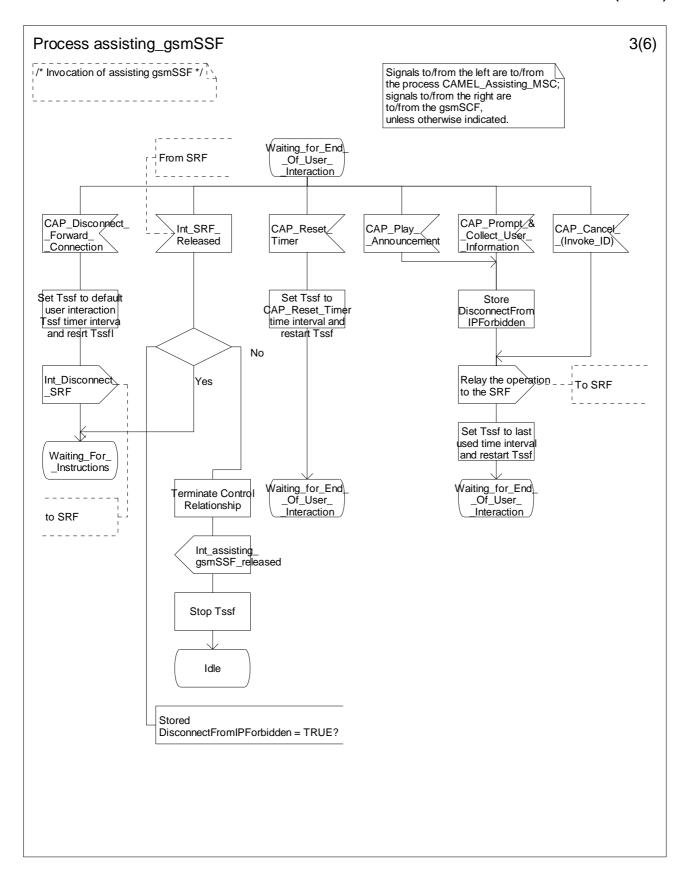
Figure 4.115-3: Process Assisting\_gsmSSF (sheet 3)
