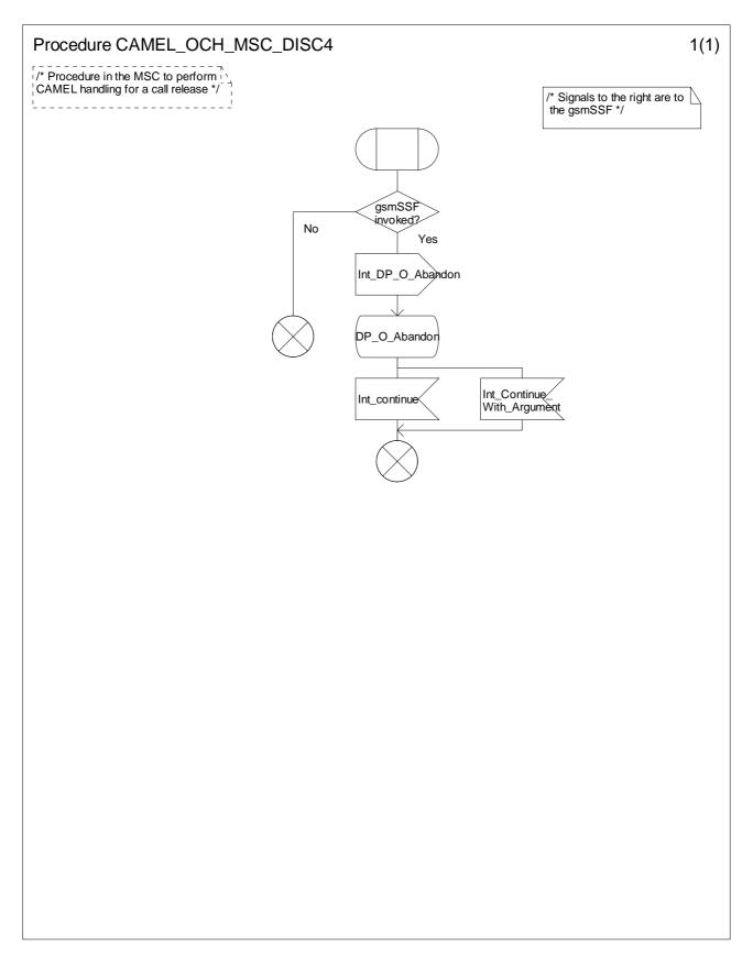
Figure 4.21-1: Procedure CAMEL\_OCH\_MSC\_DISC4 (sheet 1)
