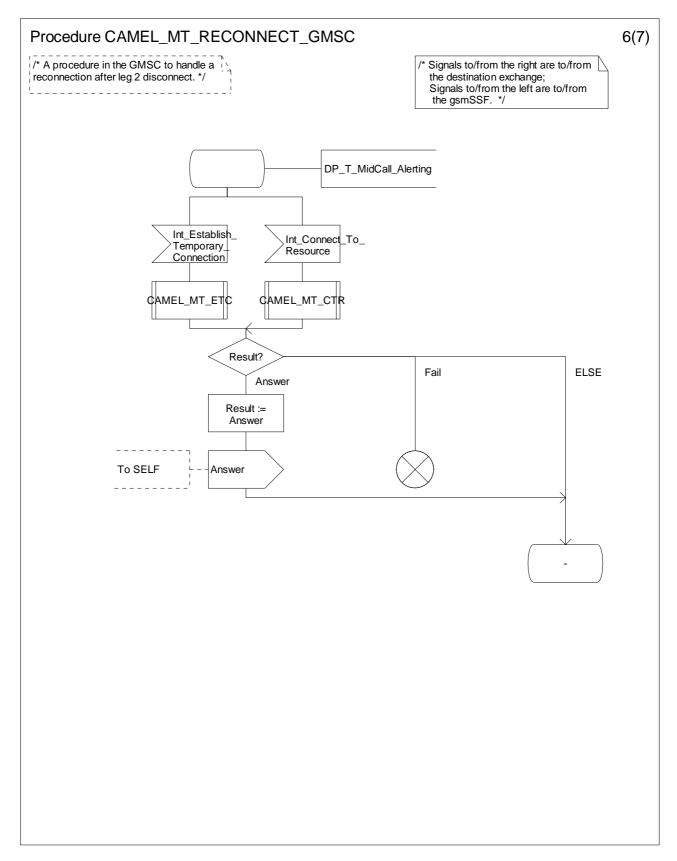
Figure 4.54-6: Procedure CAMEL\_MT\_RECONNECT\_GMSC (sheet 6)
