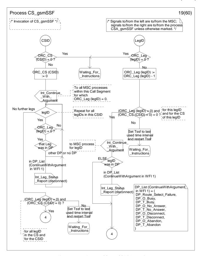
Figure 4.96-19: Process CS\_gsmSSF (sheet 19)
