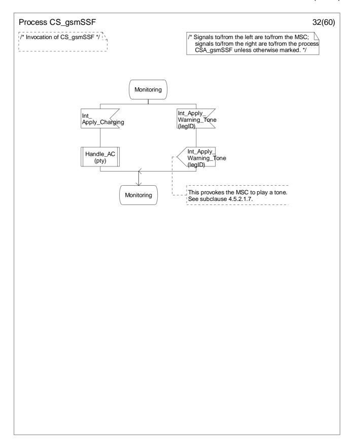
Figure 4.96-32: Process CS\_gsmSSF (sheet 32)
