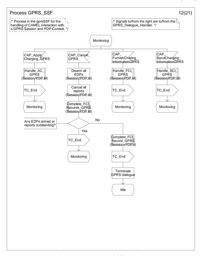
Figure 6.17-12: Process GPRS\_SSF (sheet 12)
