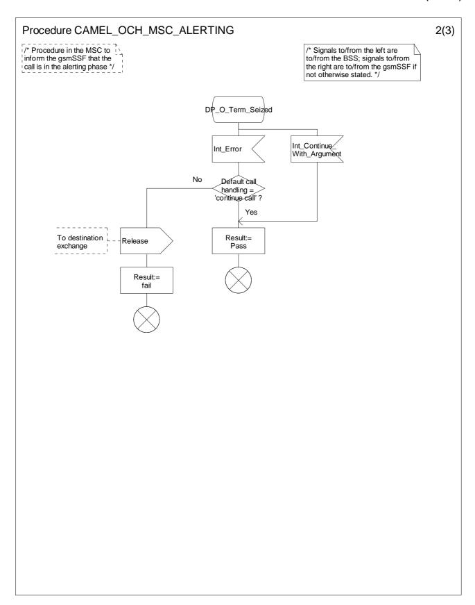
Figure 4.14-2: Procedure CAMEL\_OCH\_MSC\_ALERTING (sheet 2)
