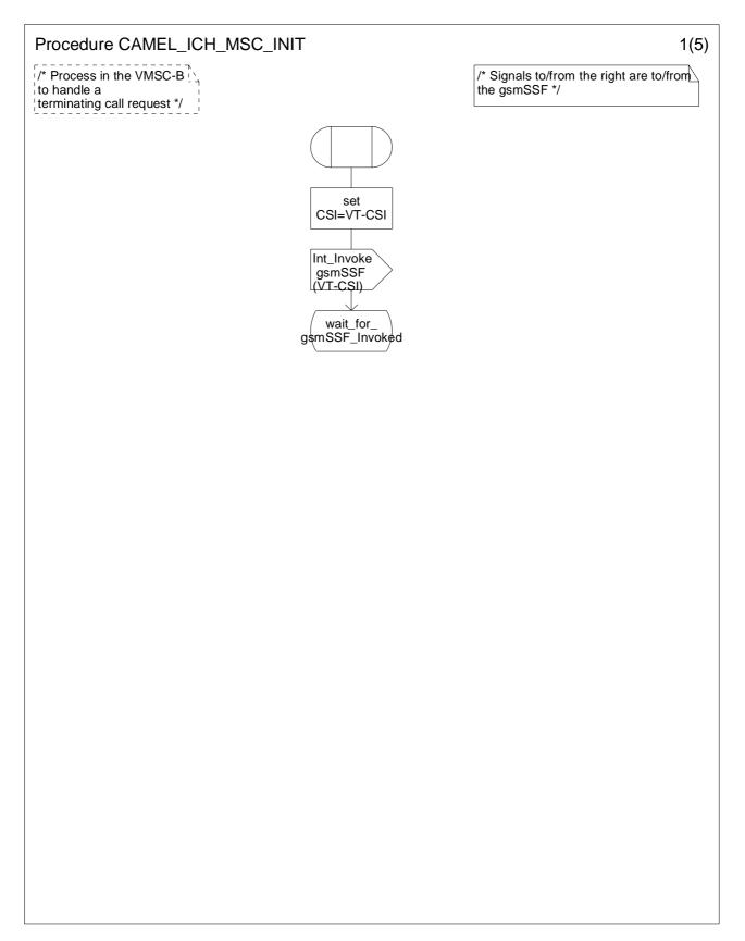
Figure 4.66-1: Procedure CAMEL\_ICH\_MSC\_INIT (sheet 1)
