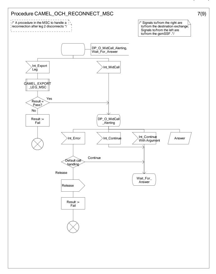
Figure 4.33-7: Procedure CAMEL\_OCH\_RECONNECT\_MSC (sheet 7)
