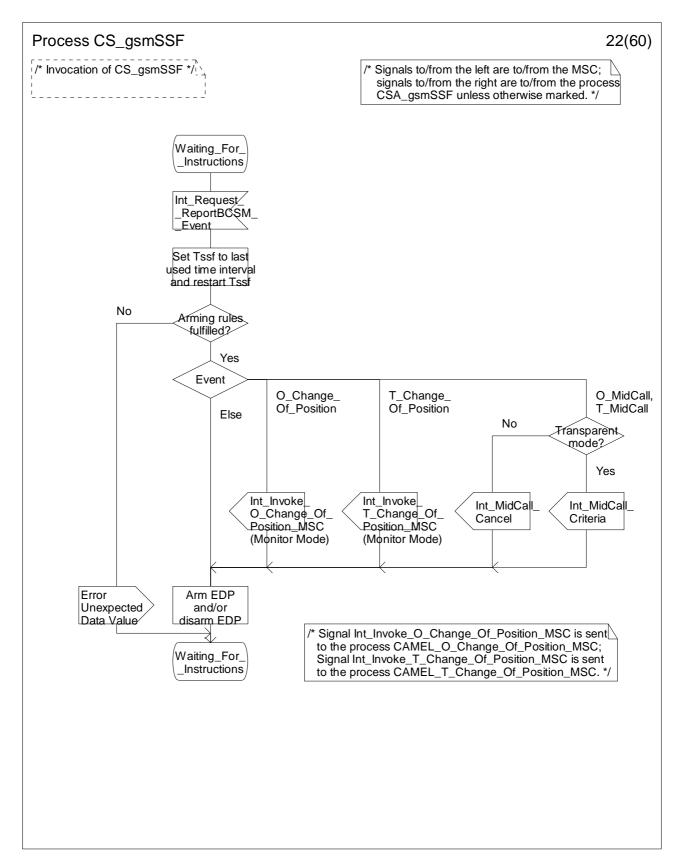
Figure 4.96-22: Process CS\_gsmSSF (sheet 22)
