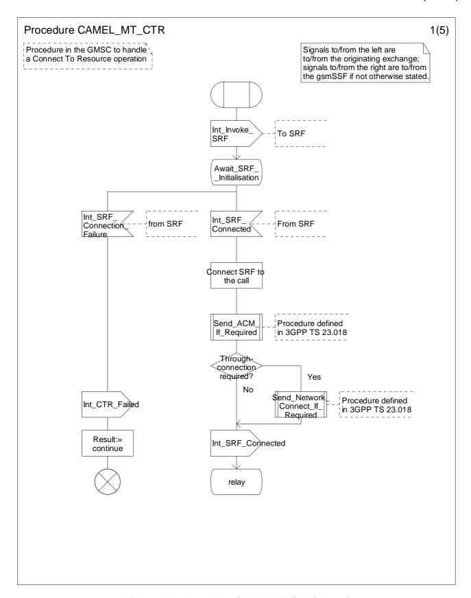
Figure 4.50-1: Procedure CAMEL\_MT\_CTR (sheet 1)
