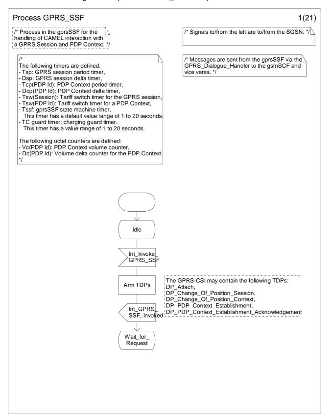
Figure 6.17-1: Process GPRS\_SSF (sheet 1)
