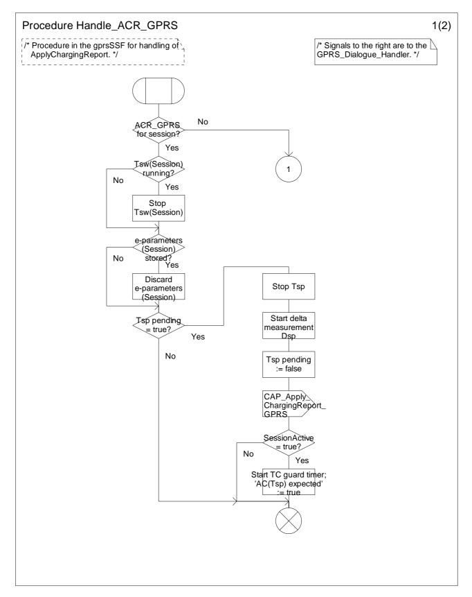
Figure 6.20-1: Procedure Handle\_ACR\_GPRS (sheet 1)
