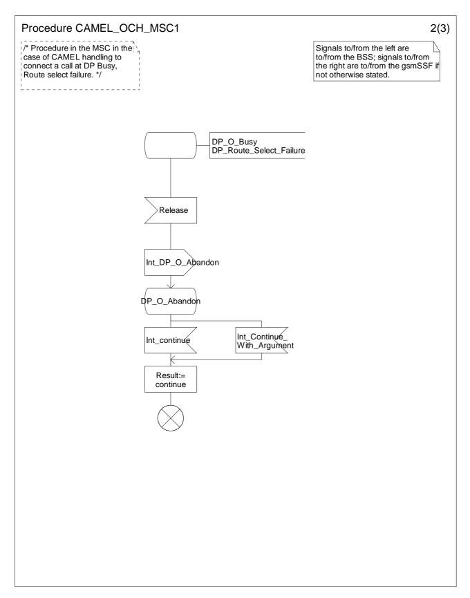
Figure 4.16-2: Procedure CAMEL\_OCH\_MSC1 (sheet 2)
