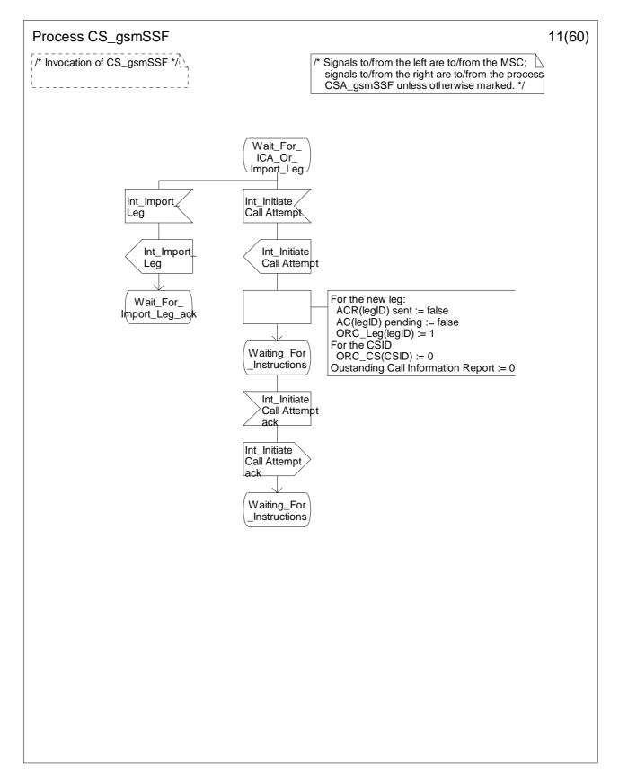
Figure 4.96-11: Process CS\_gsmSSF (sheet 11)
