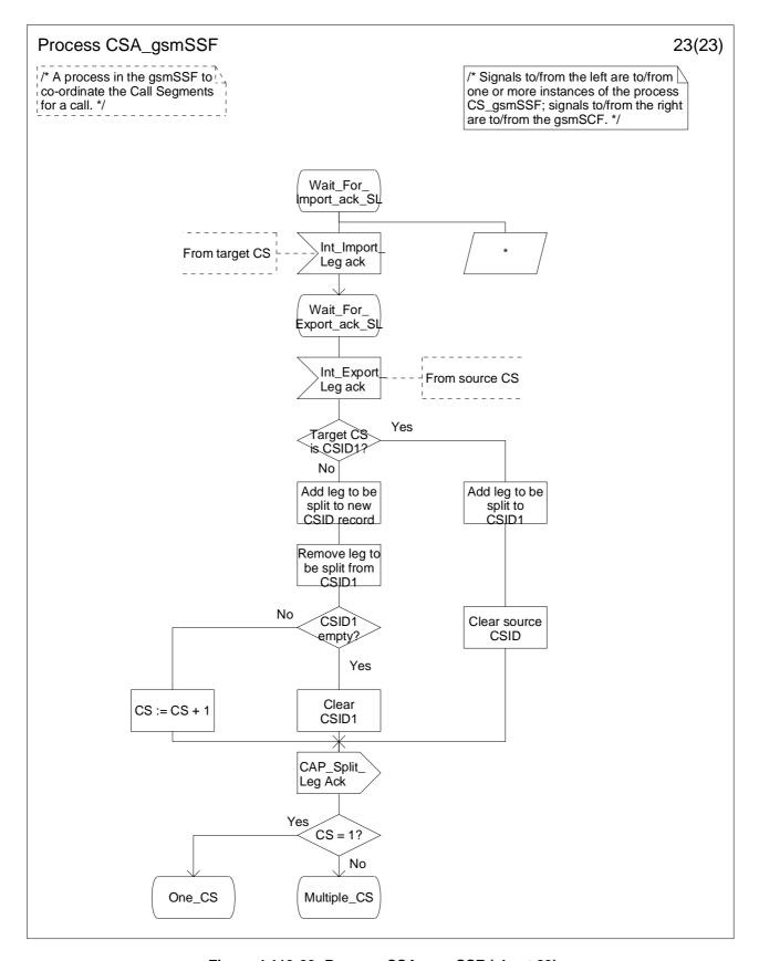
Figure 4.113-23: Process CSA\_gsmSSF (sheet 23)
