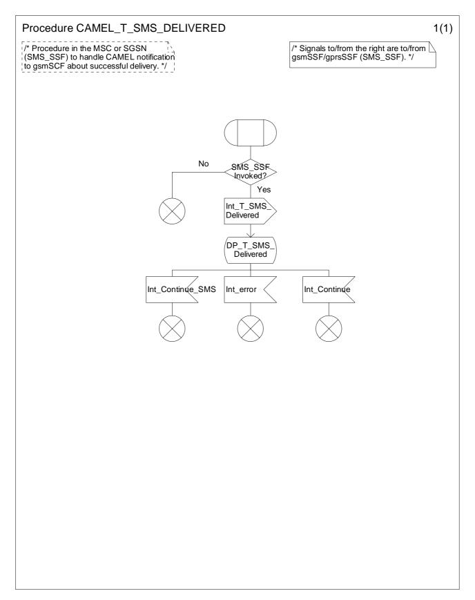
Figure 7.12-1: Procedure CAMEL\_T\_SMS\_DELIVERED (sheet 1)
