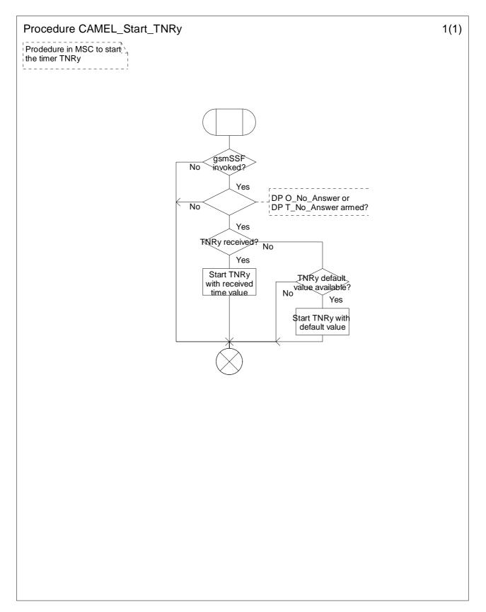
Figure 4.25-1: Procedure CAMEL\_Start\_TNRy (sheet 1)
