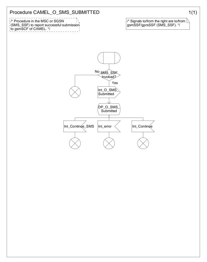
Figure 7.6-1: Procedure CAMEL\_O\_SMS\_SUBMITTED (sheet 1)
