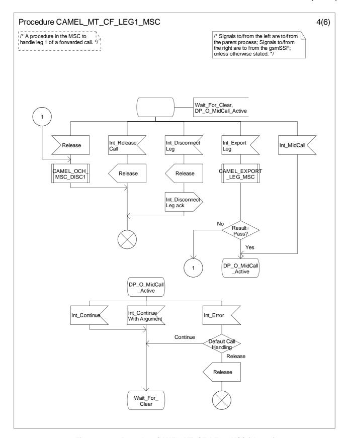
Figure 4.83-4: Procedure CAMEL\_MT\_CF\_LEG1\_MSC (sheet 4)
