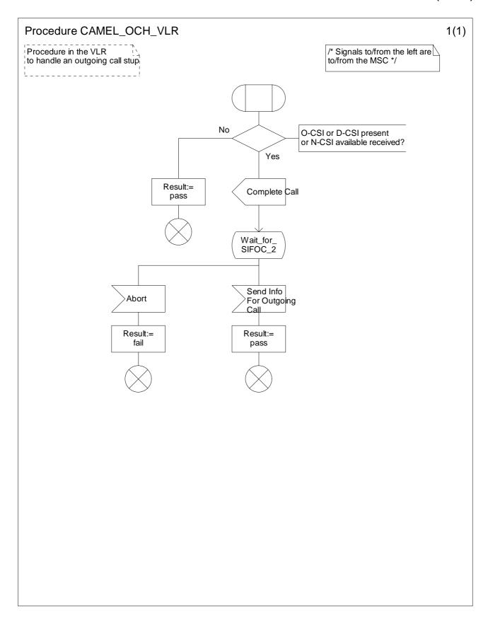
Figure 4.37-1: Procedure CAMEL\_OCH\_VLR (sheet 1)
