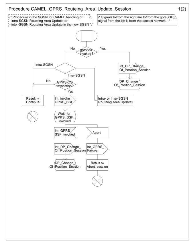
Figure 6.10-1: Procedure CAMEL\_GPRS\_Routeing\_Area\_Update\_Session (sheet 1)
