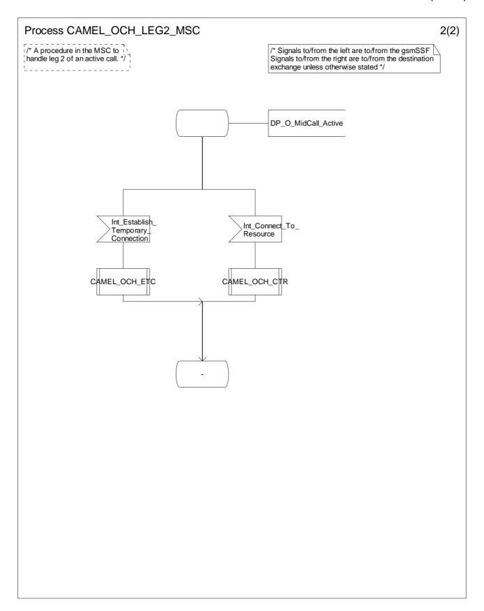
Figure 4.32-2: Process CAMEL\_OCH\_LEG2\_MSC (sheet 2)
