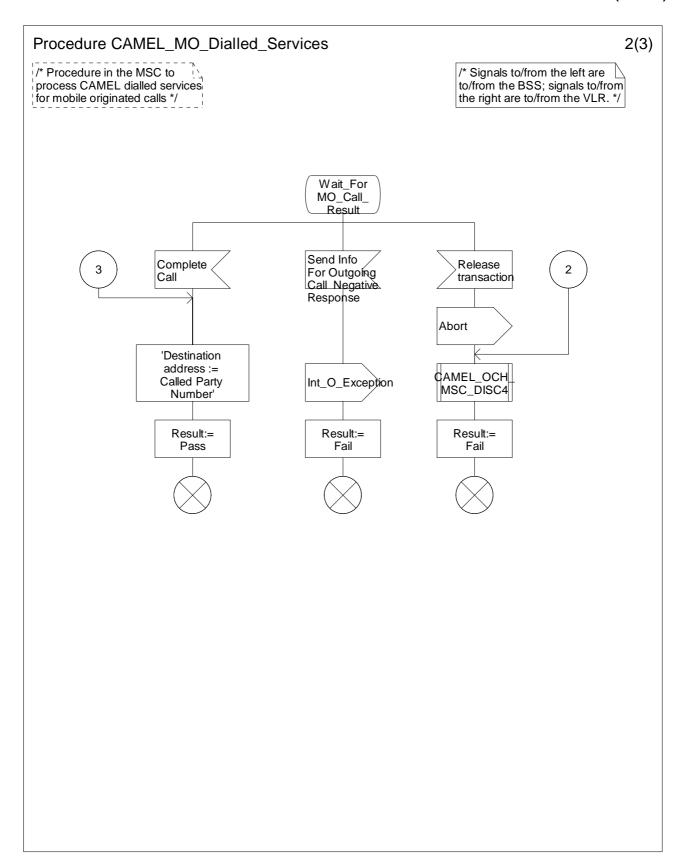
Figure 4.11-2: Procedure CAMEL\_MO\_Dialled\_Services (sheet 2)
