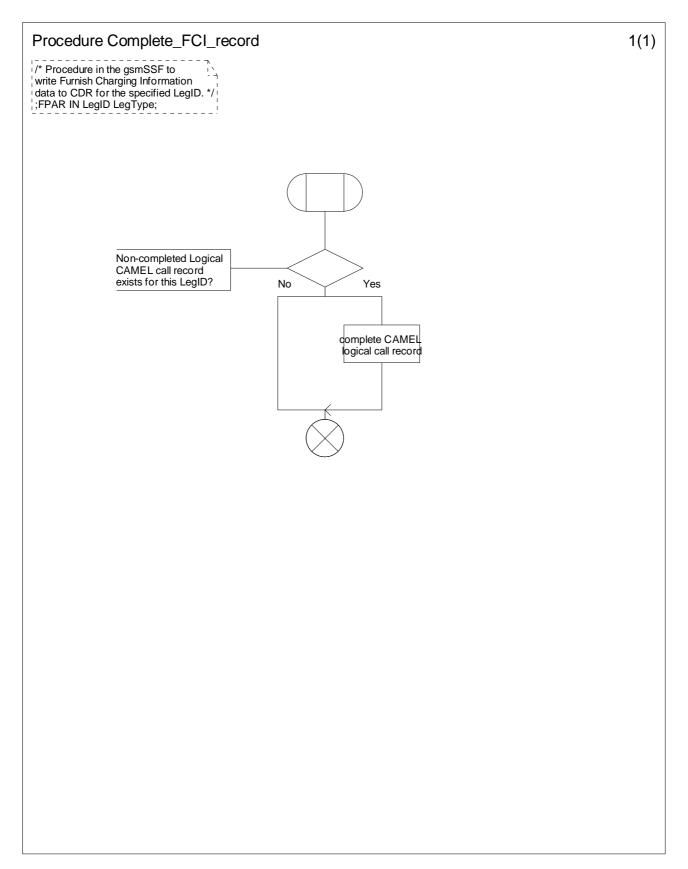
Figure 4.105-1: Procedure Complete\_FCI\_record (sheet 1)
