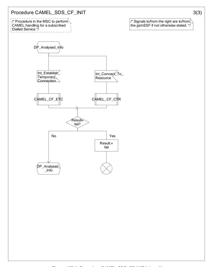
Figure 4.77-3: Procedure CAMEL\_SDS\_CF\_INIT (sheet 3)
