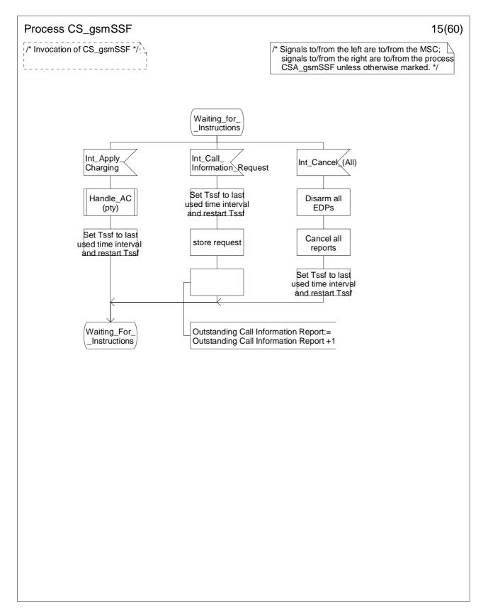
Figure 4.96-15: Process CS\_gsmSSF (sheet 15)
