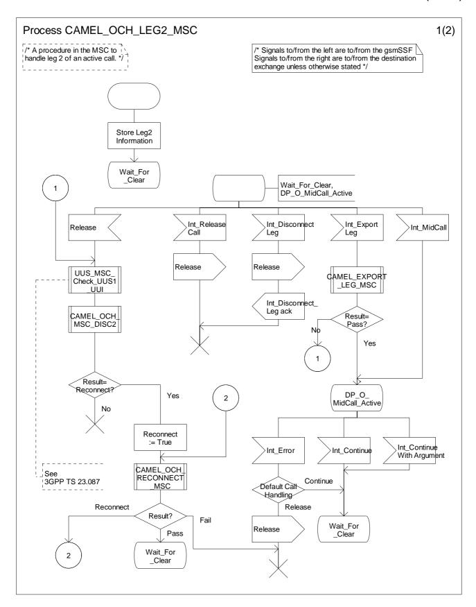
Figure 4.32-1: Process CAMEL\_OCH\_LEG2\_MSC (sheet 1)
