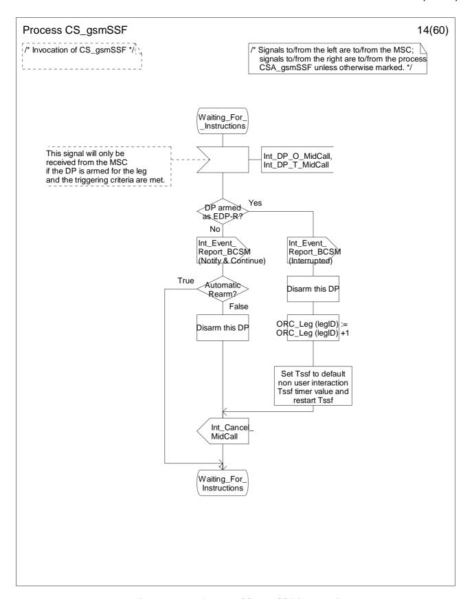
Figure 4.96-14: Process CS\_gsmSSF (sheet 14)
