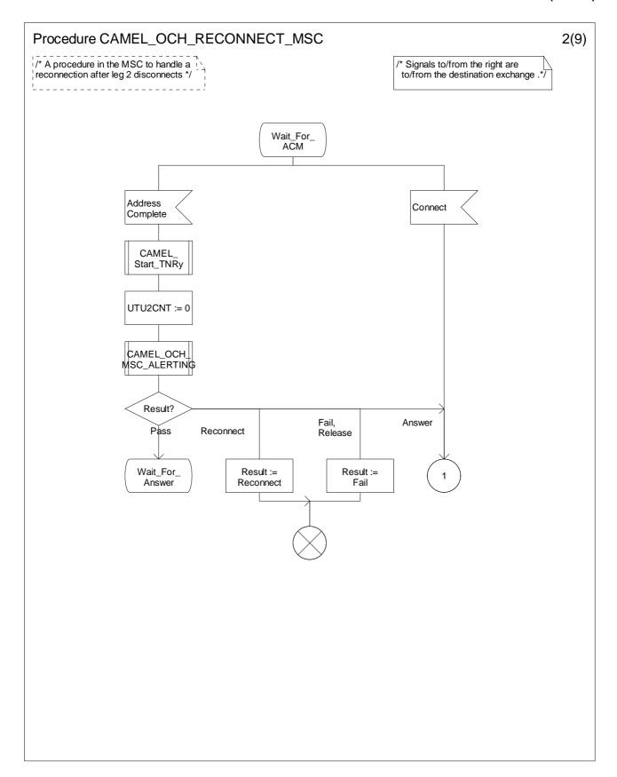
Figure 4.33-2: Procedure CAMEL\_OCH\_RECONNECT\_MSC (sheet 2)
