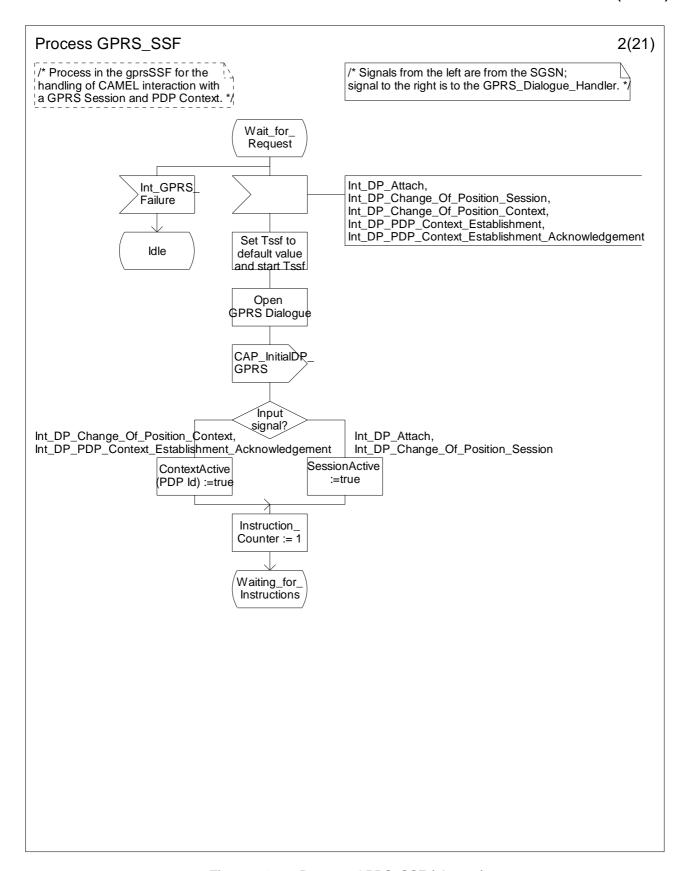
Figure 6.17-2: Process GPRS\_SSF (sheet 2)
