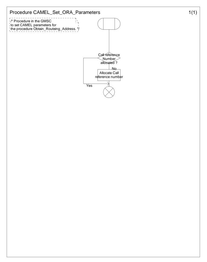
Figure 4.39-1: Procedure CAMEL\_Set\_ORA\_Parameters (sheet 1)
