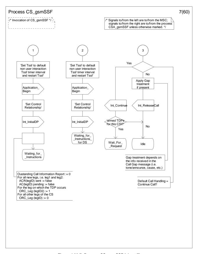
Figure 4.96-7: Process CS\_gsmSSF (sheet 7)
