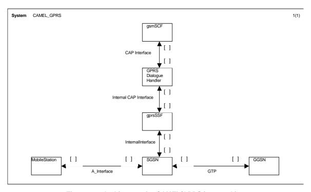
Figure 6.7: Architecture for CAMEL/GPRS interworking
