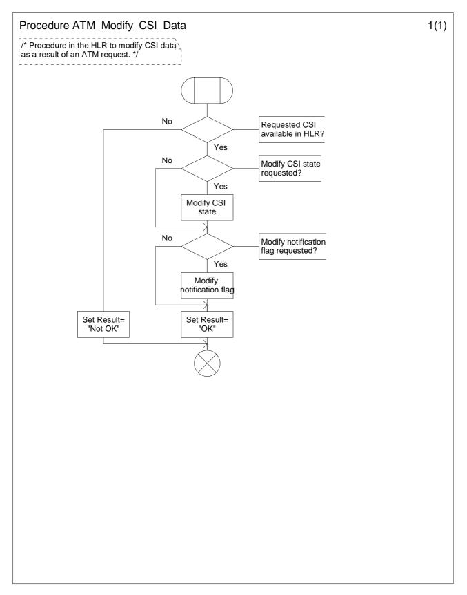
Figure 10.5-1: Procedure ATM\_Modify\_CSI\_Data (sheet 1)
