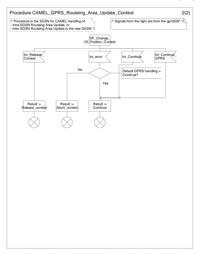
Figure 6.11-2: Procedure CAMEL\_GPRS\_Routeing\_Area\_Update\_Context (sheet 2)
