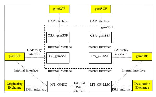
Figure 4.9-3: Terminating GMSC case (gsmSSF relay)
