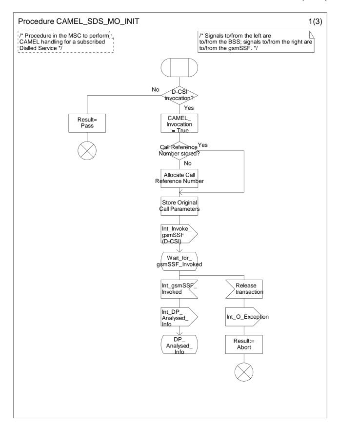
Figure 4.12-1: Procedure CAMEL\_SDS\_MO\_Init (sheet 1)
