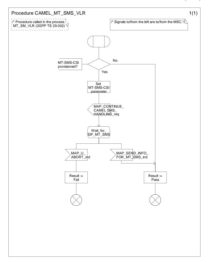
Figure 7.13-1: Procedure CAMEL\_MT\_SMS\_VLR (sheet 1)
