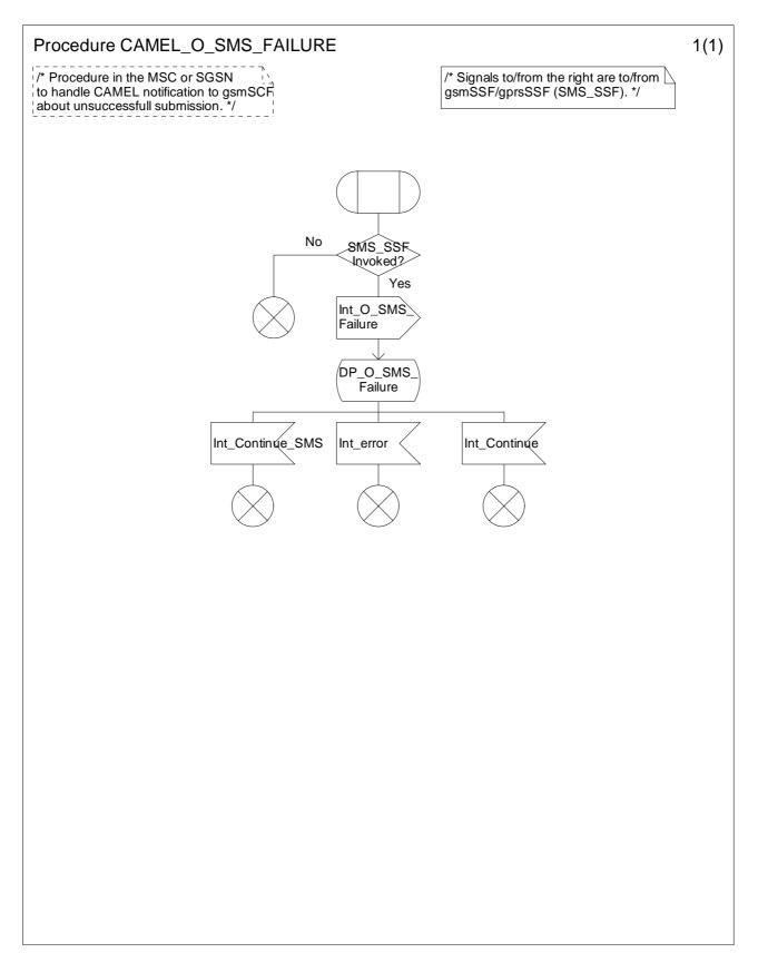
Figure 7.7-1: Procedure CAMEL\_O\_SMS\_FAILURE (sheet 1)
