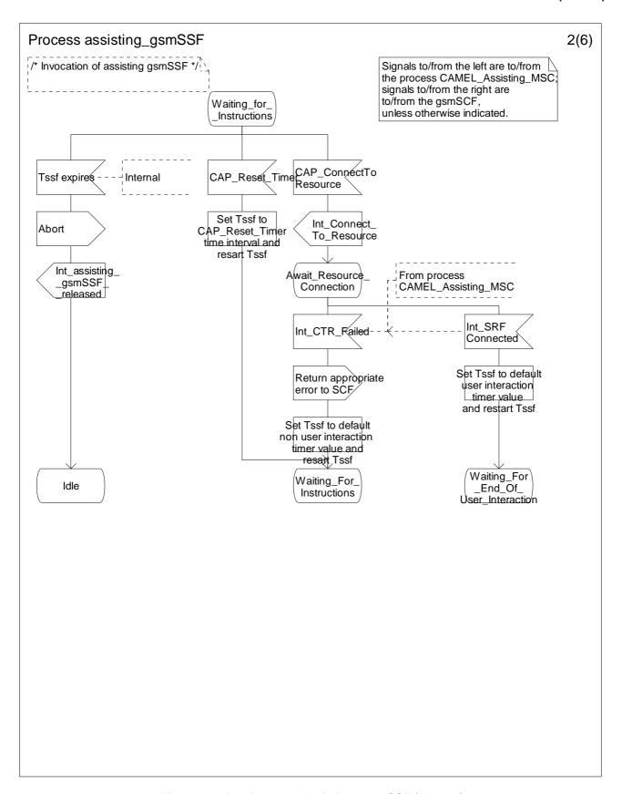
Figure 4.115-2: Process Assisting\_gsmSSF (sheet 2)
