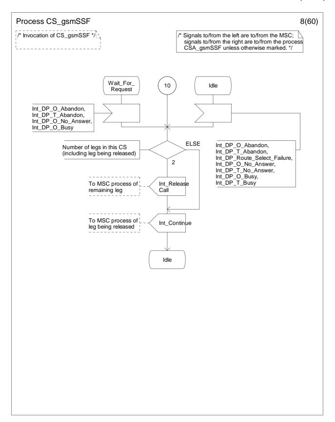
Figure 4.96-8: Process CS\_gsmSSF (sheet 8)
