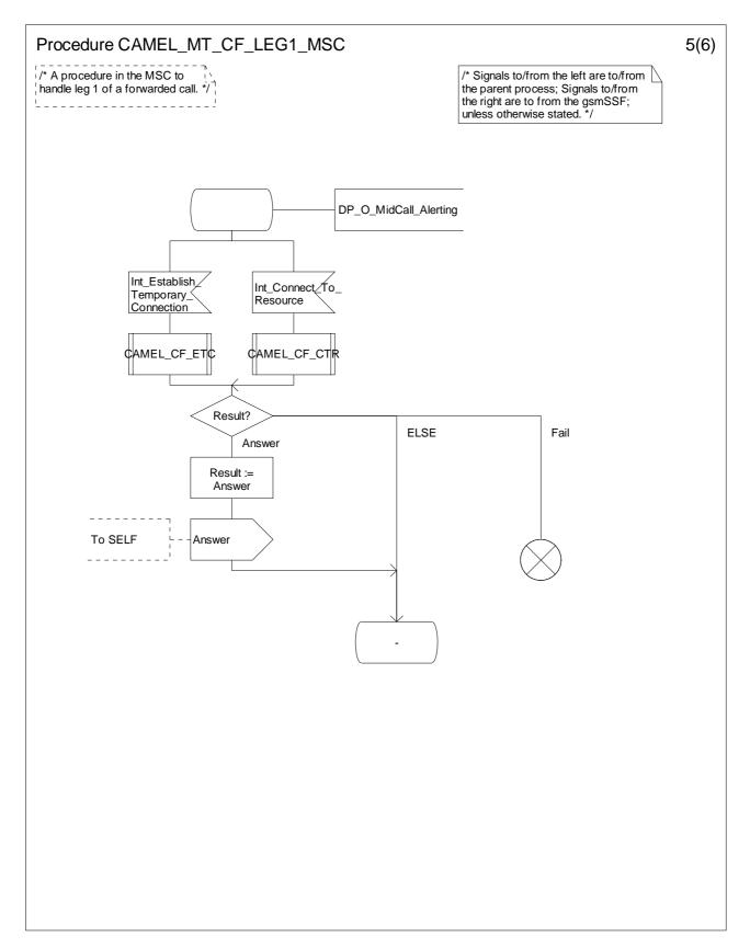
Figure 4.83-5: Procedure CAMEL\_MT\_CF\_LEG1\_MSC (sheet 5)
