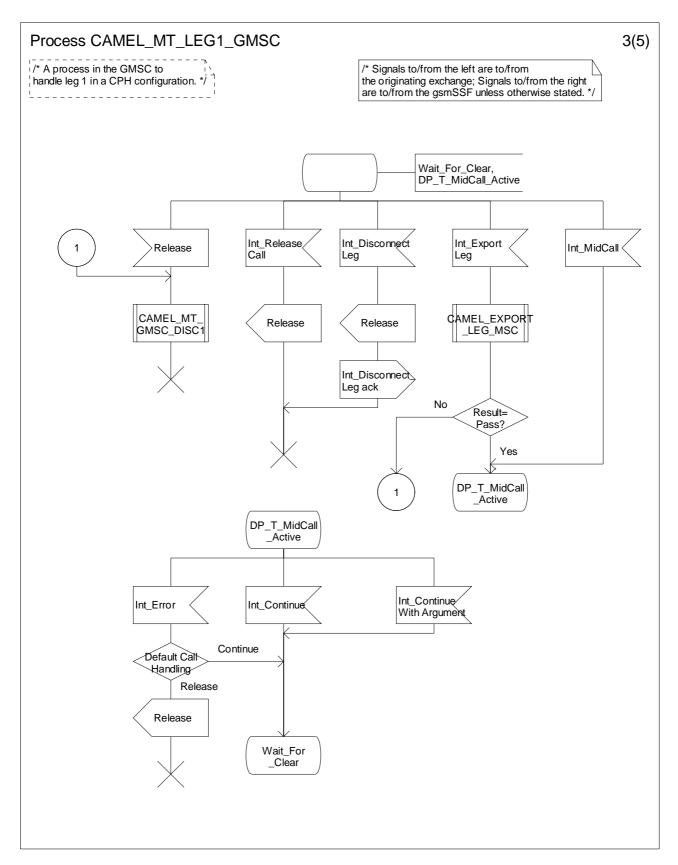
Figure 4.53-3: Process CAMEL\_MT\_LEG1\_GMSC (sheet 3)
