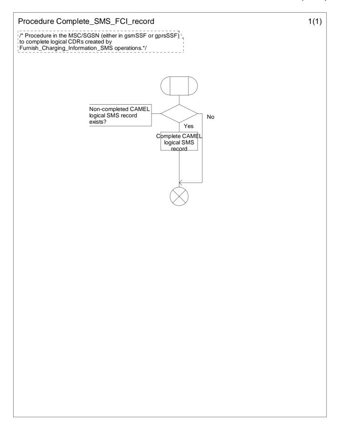
Figure 7.17-1: Procedure Complete\_SMS\_FCI\_record (sheet 1)
