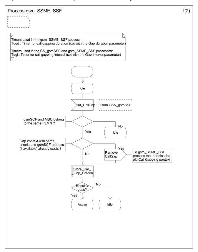
Figure 4.110-1: Process gsm\_SSME\_SSF (sheet 1)
