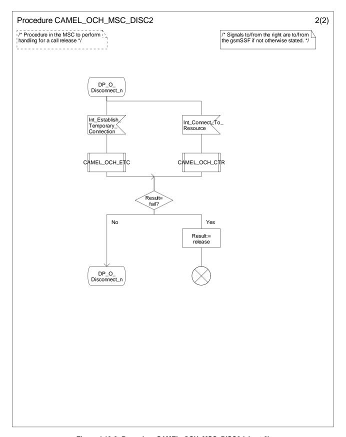
Figure 4.19-2: Procedure CAMEL\_OCH\_MSC\_DISC2 (sheet 2)
