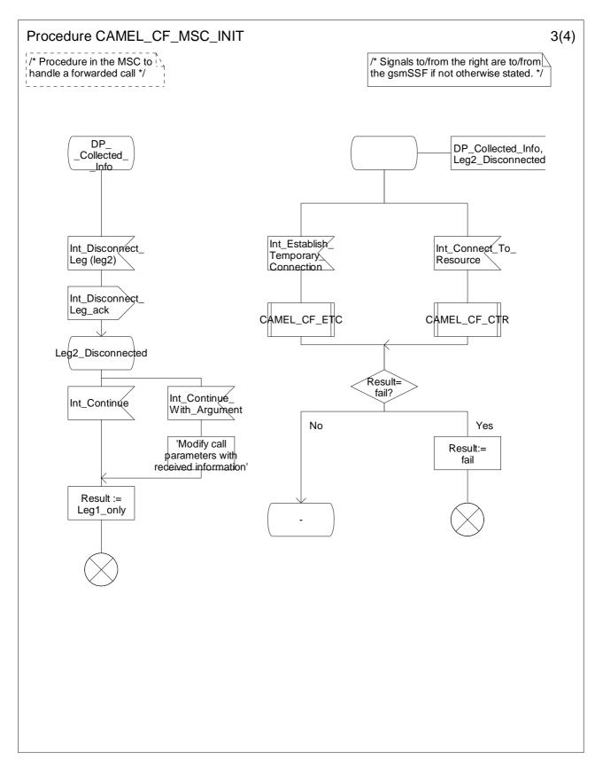
Figure 4.76-3: Procedure CAMEL\_CF\_MSC\_INIT (sheet 3)
