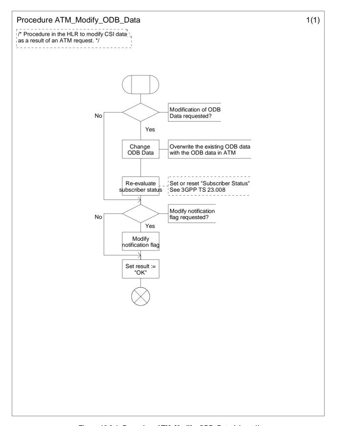
Figure 10.8-1: Procedure ATM\_Modify\_ODB\_Data (sheet 1)
