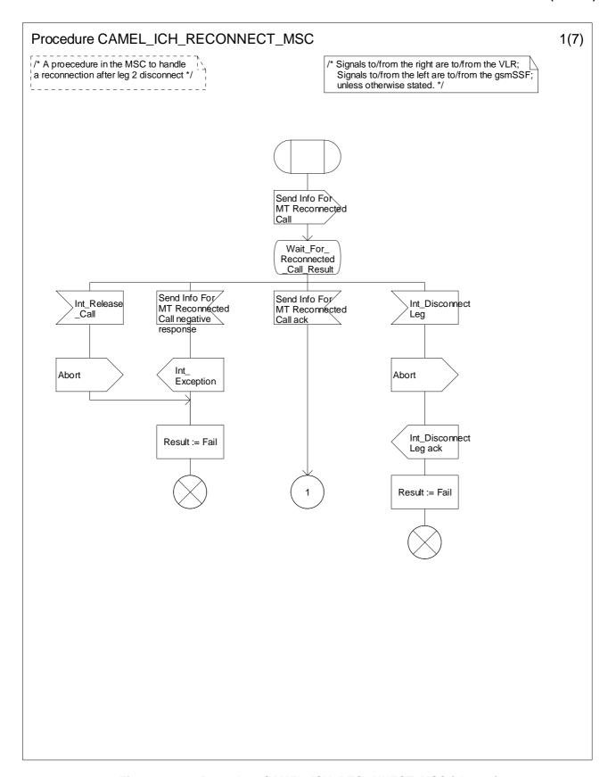
Figure 4.71-1: Procedure CAMEL\_ICH\_RECONNECT\_MSC (sheet 1)
