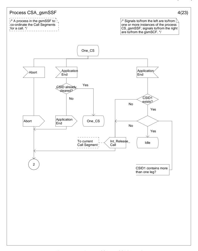
Figure 4.113-4: Process CSA\_gsmSSF (sheet 4)
