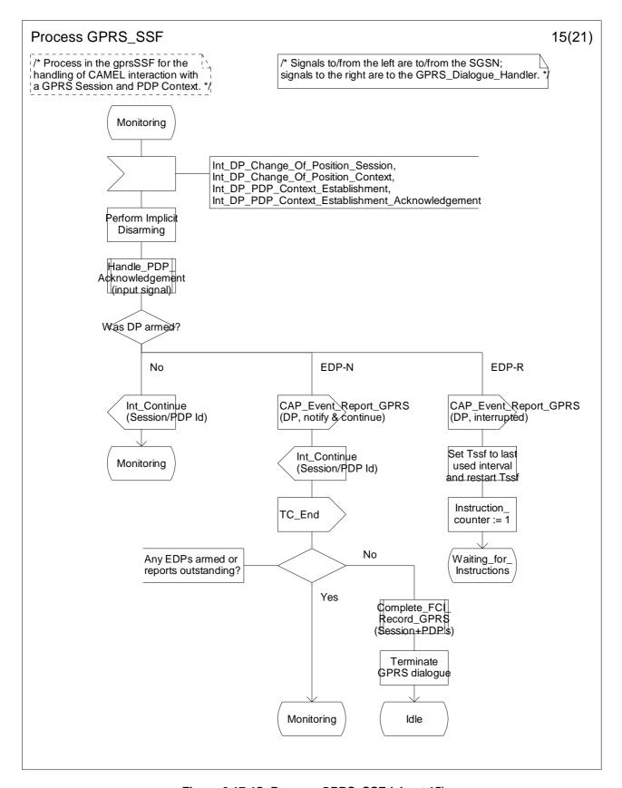
Figure 6.17-15: Process GPRS\_SSF (sheet 15)
