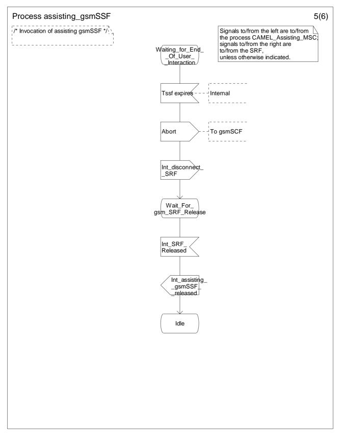
Figure 4.115-5: Process Assisting\_gsmSSF (sheet 5)
