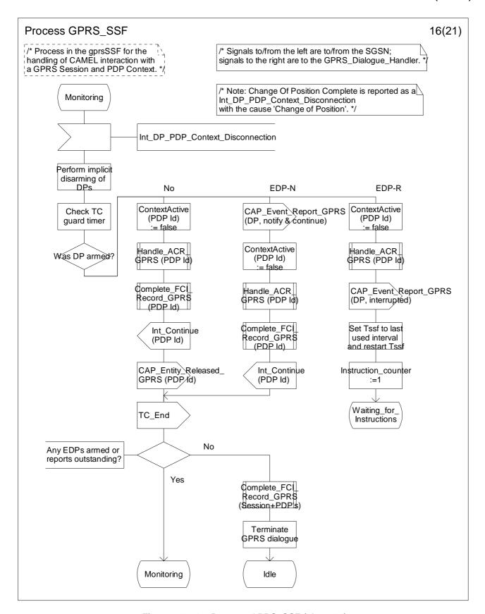
Figure 6.17-16: Process GPRS\_SSF (sheet 16)
