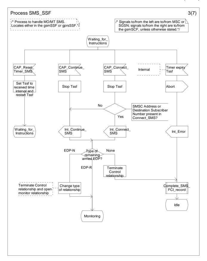
Figure 7.15-3: Process SMS\_SSF (sheet 3)
