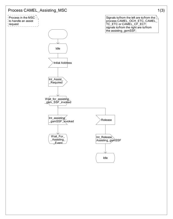
Figure 4.114-1: Process CAMEL\_Assisting\_MSC (sheet 1)
