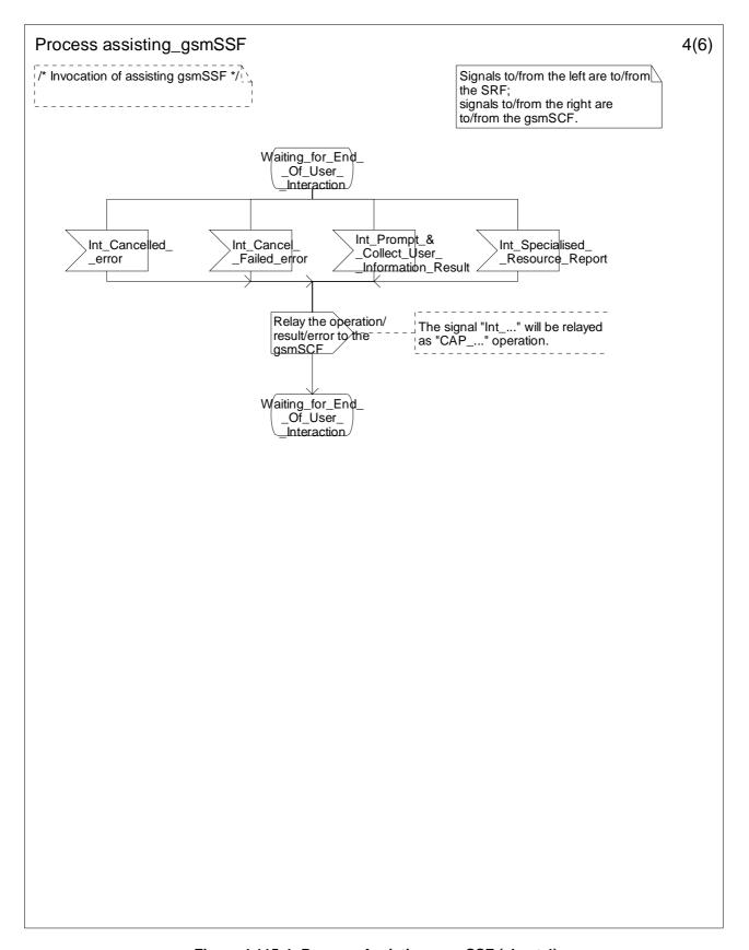
Figure 4.115-4: Process Assisting\_gsmSSF (sheet 4)
