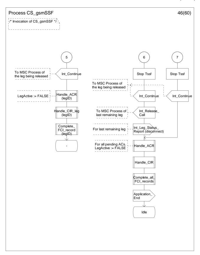
Figure 4.96-46: Process CS\_gsmSSF (sheet 46)
