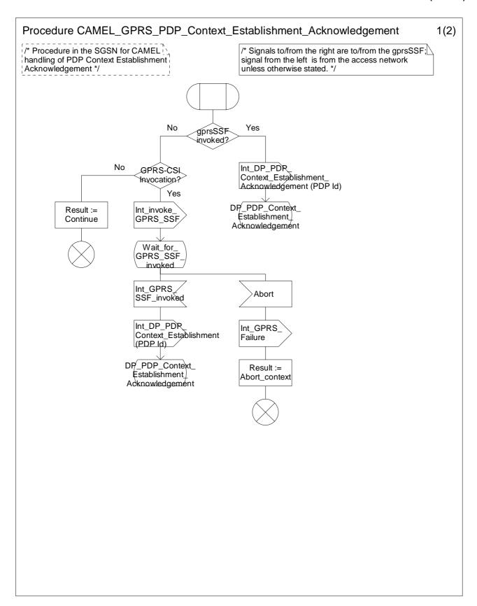
Figure 6.13-1: Procedure CAMEL\_GPRS\_PDP\_Context\_Establishment\_Acknowledgement (sheet 1)
