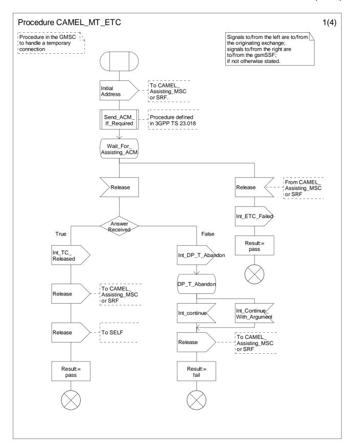
Figure 4.49-1: Procedure CAMEL\_MT\_ETC (sheet 1)
