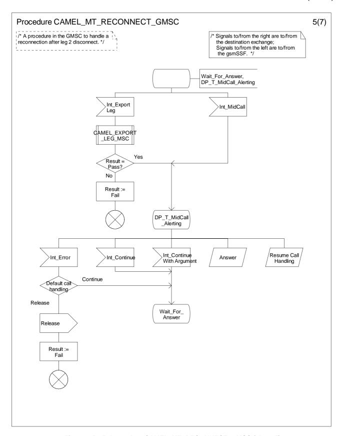
Figure 4.54-5: Procedure CAMEL\_MT\_RECONNECT\_GMSC (sheet 5)
