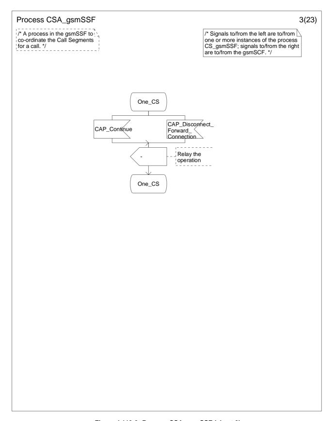
Figure 4.113-3: Process CSA\_gsmSSF (sheet 3)
