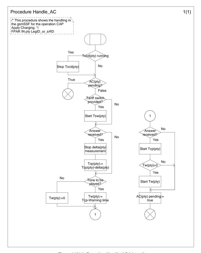
Figure 4.101-1: Procedure Handle\_AC (sheet 1)
