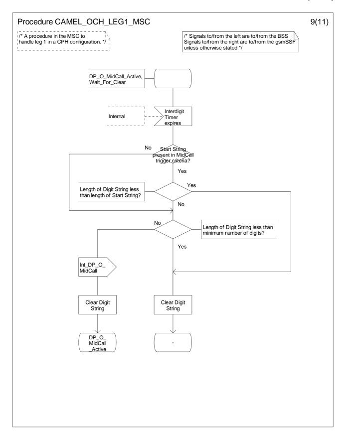
Figure 4.30-9: Procedure CAMEL\_OCH\_LEG1\_MSC (sheet 9)
