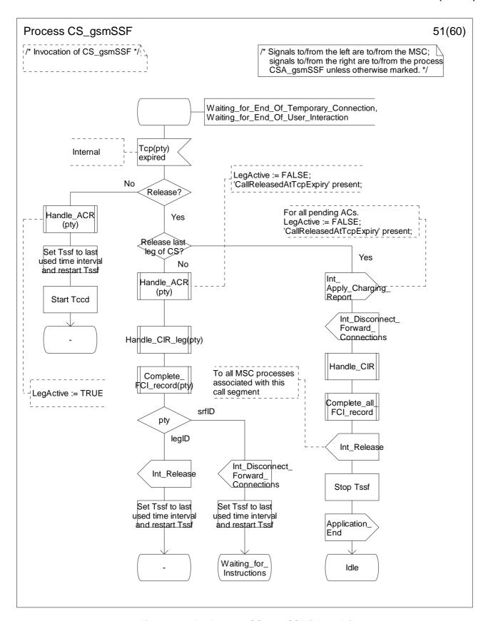
Figure 4.96-51: Process CS\_gsmSSF (sheet 51)
