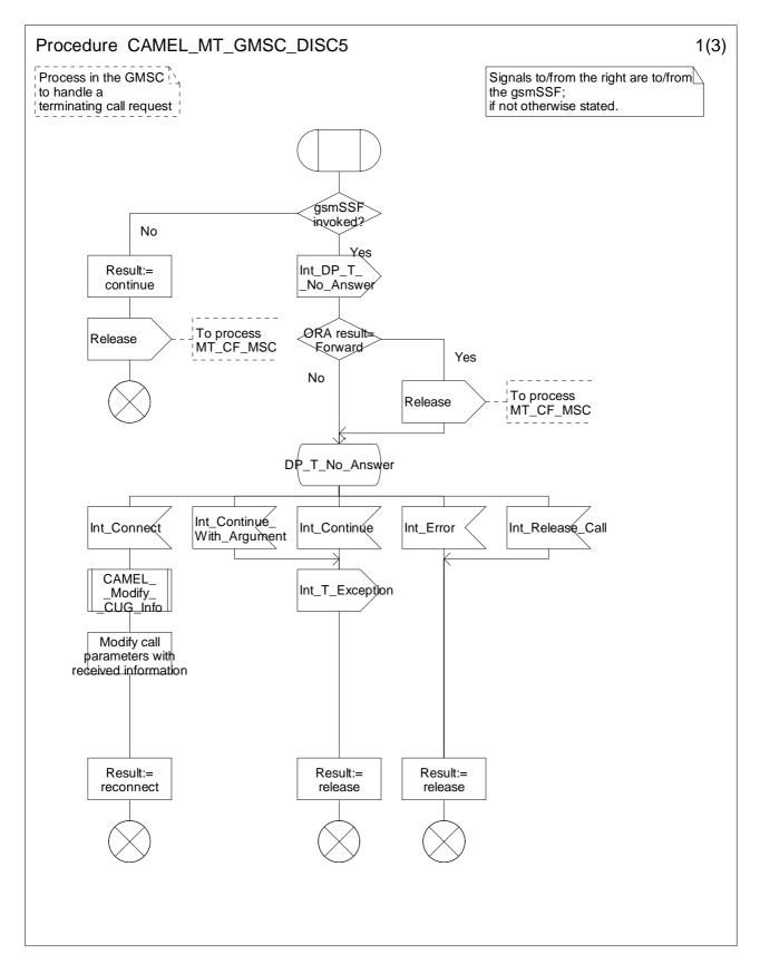
Figure 4.47-1: Procedure CAMEL\_MT\_GMSC\_DISC5 (sheet 1)
