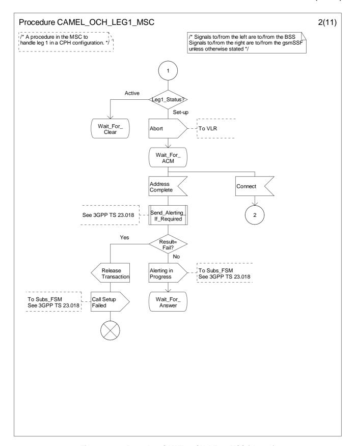
Figure 4.30-2: Procedure CAMEL\_OCH\_LEG1\_MSC (sheet 2)
