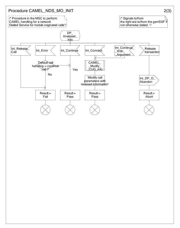
Figure 4.13-2: Procedure CAMEL\_NDS\_MO\_INIT (sheet 2)
