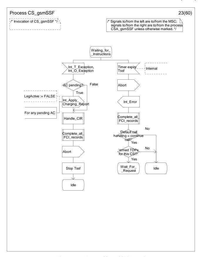
Figure 4.96-23: Process CS\_gsmSSF (sheet 23)
