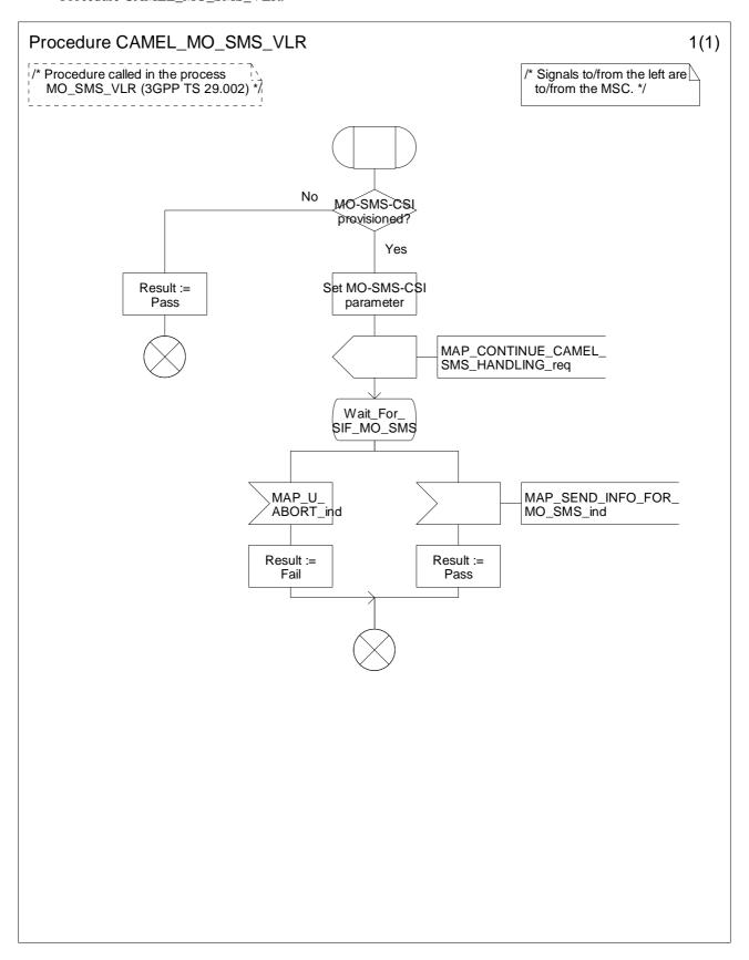
Figure 7.8-1: Procedure CAMEL\_MO\_SMS\_VLR (sheet 1)
