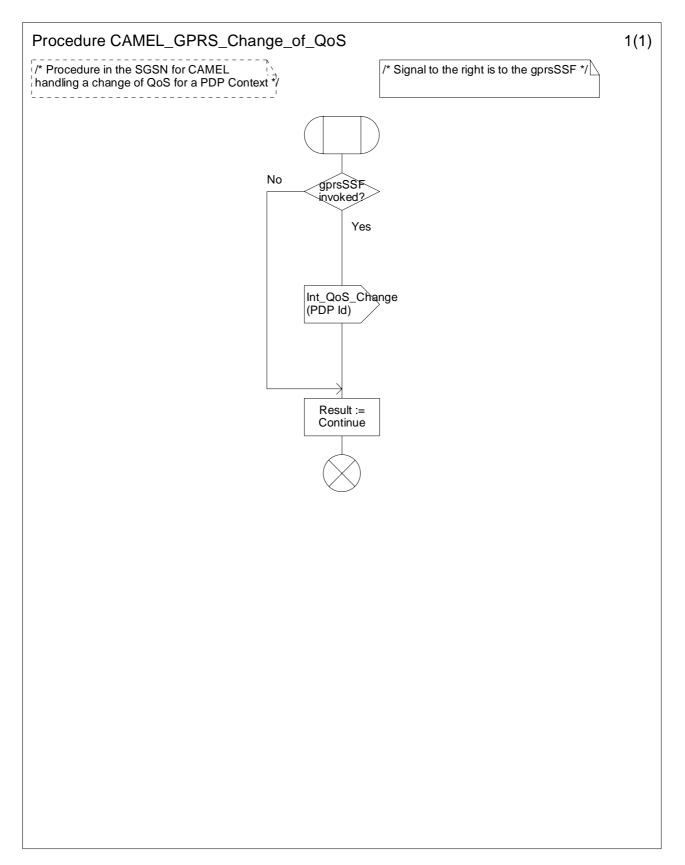
Figure 6.14-1: Procedure CAMEL\_GPRS\_Change\_Of\_QoS (sheet 1)
