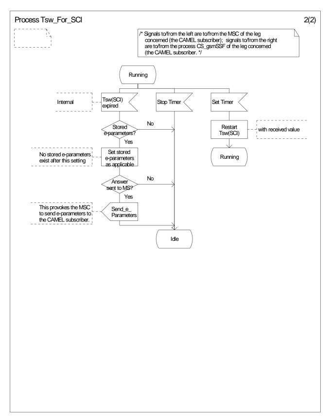
Figure 4.95-2: Process Tsw\_For\_SCI (sheet 2)
