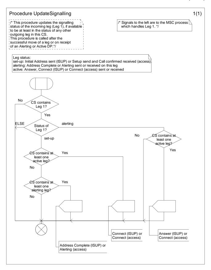
Figure 4.109-1: Procedure UpdateSignalling (sheet 1)
