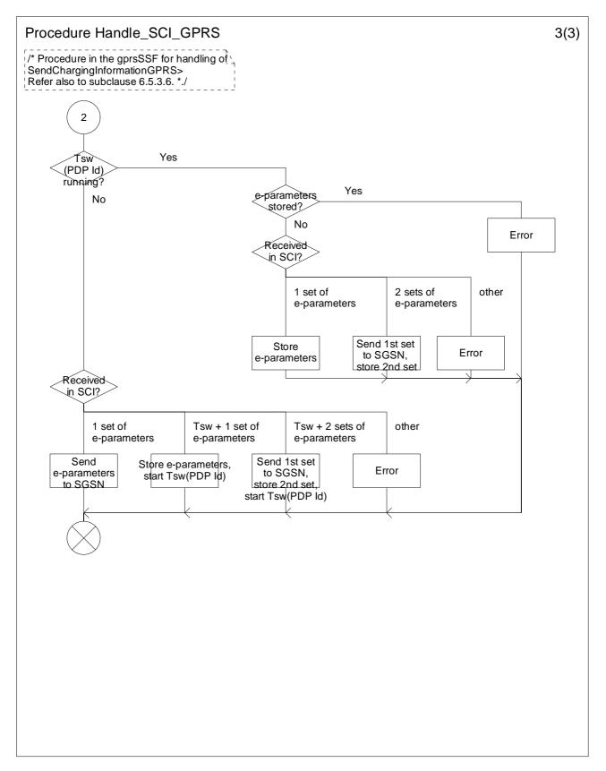
Figure 6.23-3: Procedure Handle\_SCI\_GPRS (sheet 3)
