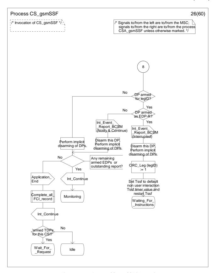
Figure 4.96-26: Process CS\_gsmSSF (sheet 26)
