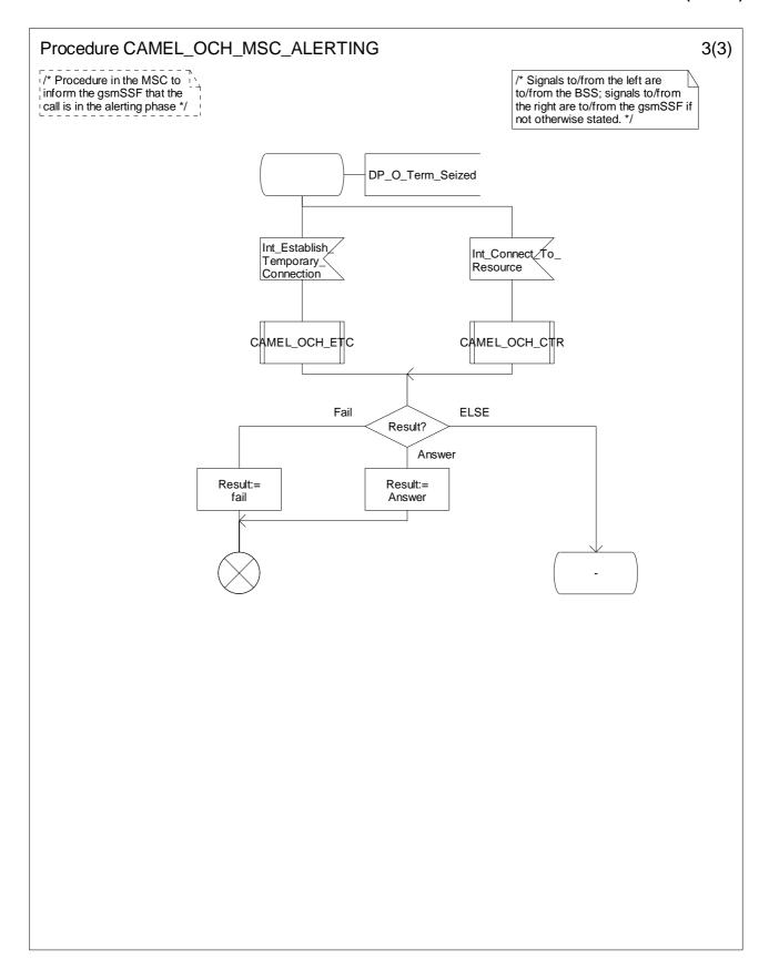
Figure 4.14-3: Procedure CAMEL\_OCH\_MSC\_ALERTING (sheet 3)
