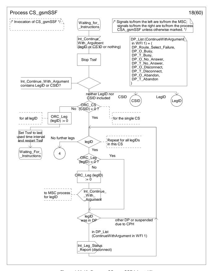
Figure 4.96-18: Process CS\_gsmSSF (sheet 18)
