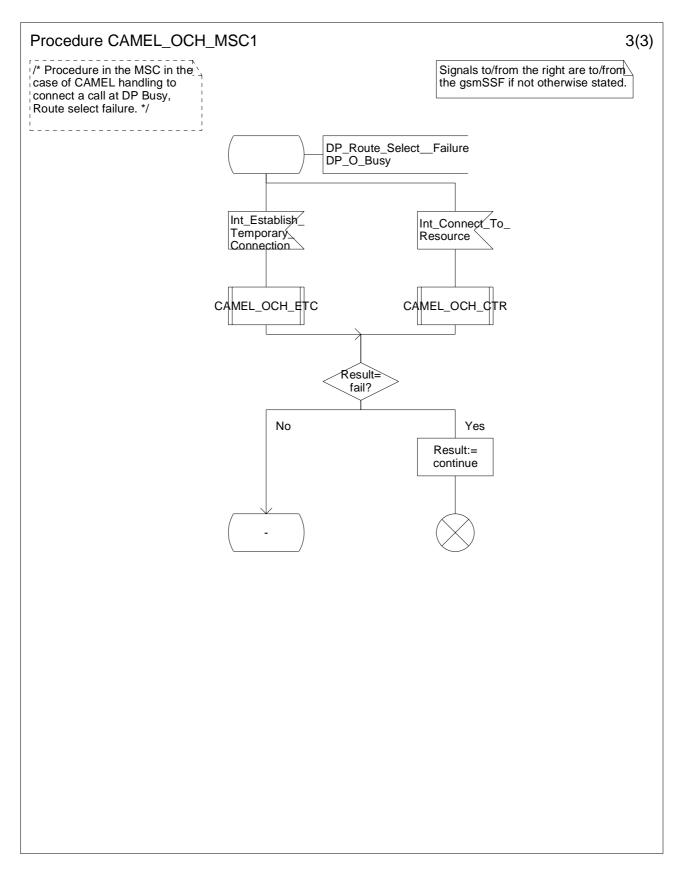
Figure 4.16-3: Procedure CAMEL\_OCH\_MSC1 (sheet 3)
