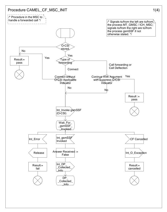
Figure 4.76-1: Procedure CAMEL\_CF\_MSC\_INIT (sheet 1)
