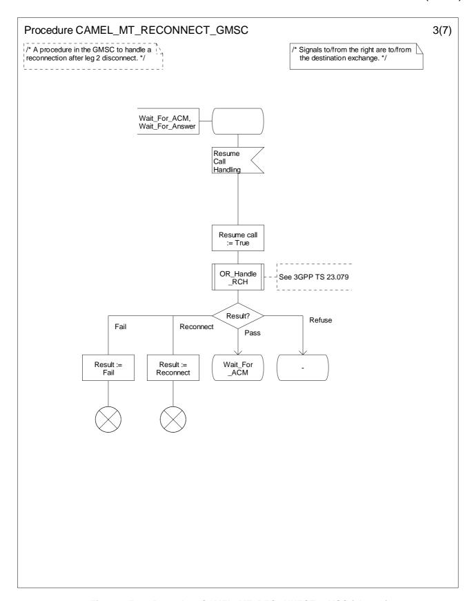
Figure 4.54-3: Procedure CAMEL\_MT\_RECONNECT\_GMSC (sheet 3)
