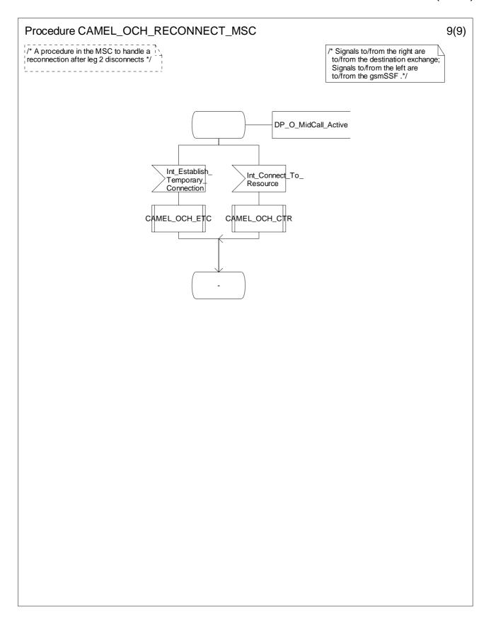
Figure 4.33-9: Procedure CAMEL\_OCH\_RECONNECT\_MSC (sheet 9)
