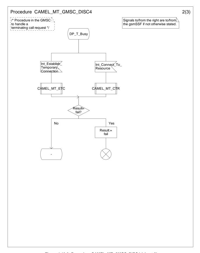
Figure 4.46-2: Procedure CAMEL\_MT\_GMSC\_DISC4 (sheet 2)
