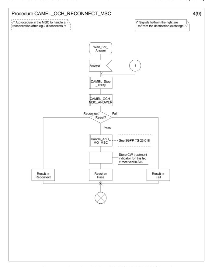
Figure 4.33-4: Procedure CAMEL\_OCH\_RECONNECT\_MSC (sheet 4)
