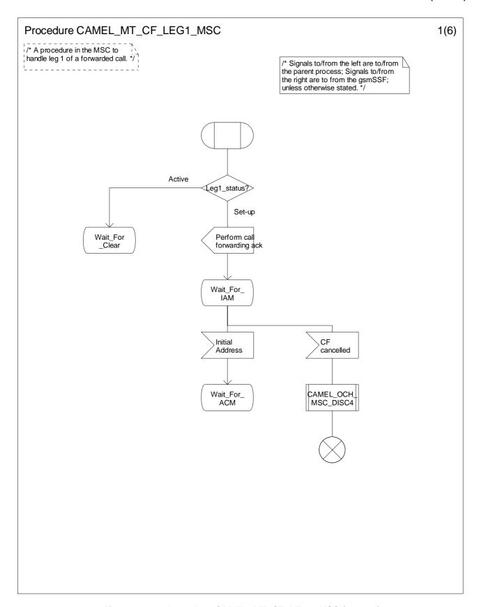
Figure 4.83-1: Procedure CAMEL\_MT\_CF\_LEG1\_MSC (sheet 1)
