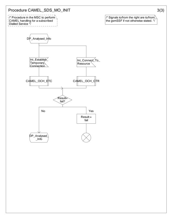
Figure 4.12-3: Procedure CAMEL\_SDS\_MO\_INIT (sheet 3)
