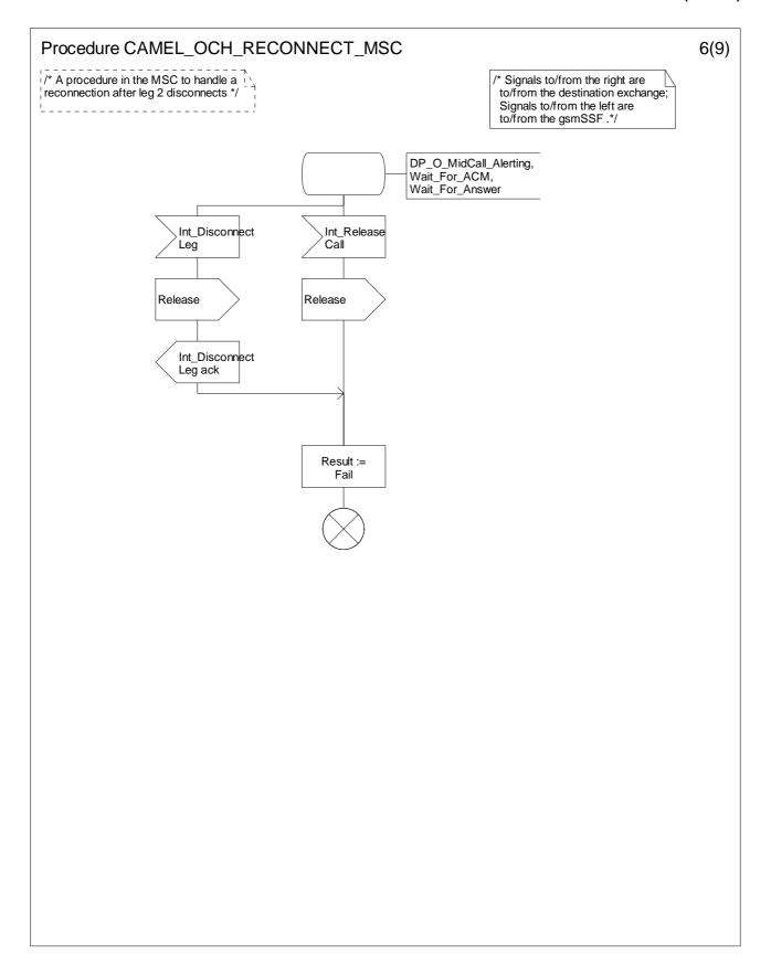
Figure 4.33-6: Procedure CAMEL\_OCH\_RECONNECT\_MSC (sheet 6)
