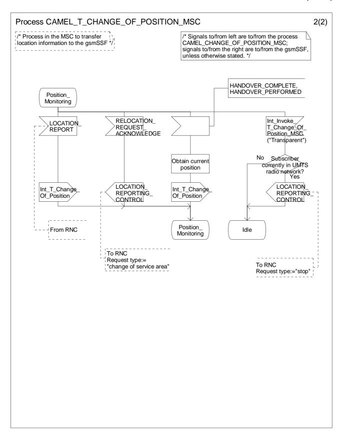
Figure 4.72-2: Procedure CAMEL\_T\_CHANGE\_OF\_POSITION\_MSC (sheet 2)
