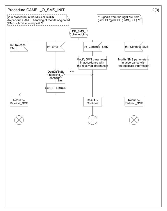
Figure 7.5-2: Procedure CAMEL\_O\_SMS\_INIT (sheet 2)
