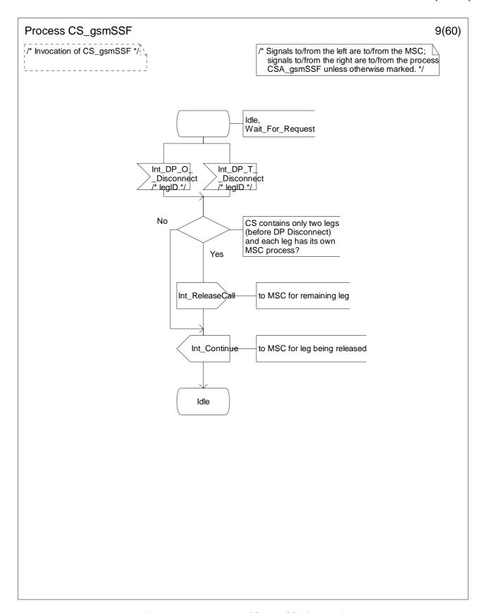
Figure 4.96-9: Process CS\_gsmSSF (sheet 9)
