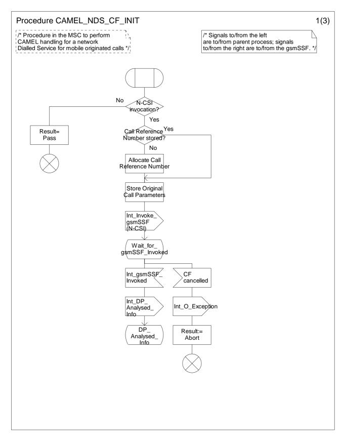
Figure 4.78-1: Procedure CAMEL\_NDS\_CF\_INIT (sheet 1)
