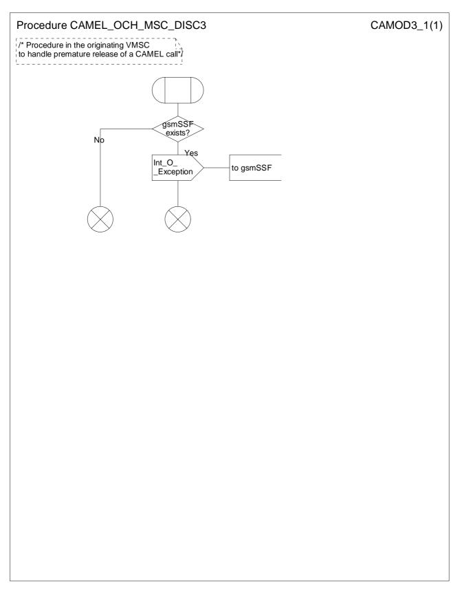
Figure 4.20-1: Procedure CAMEL\_OCH\_MSC\_DISC3 (sheet 1)
