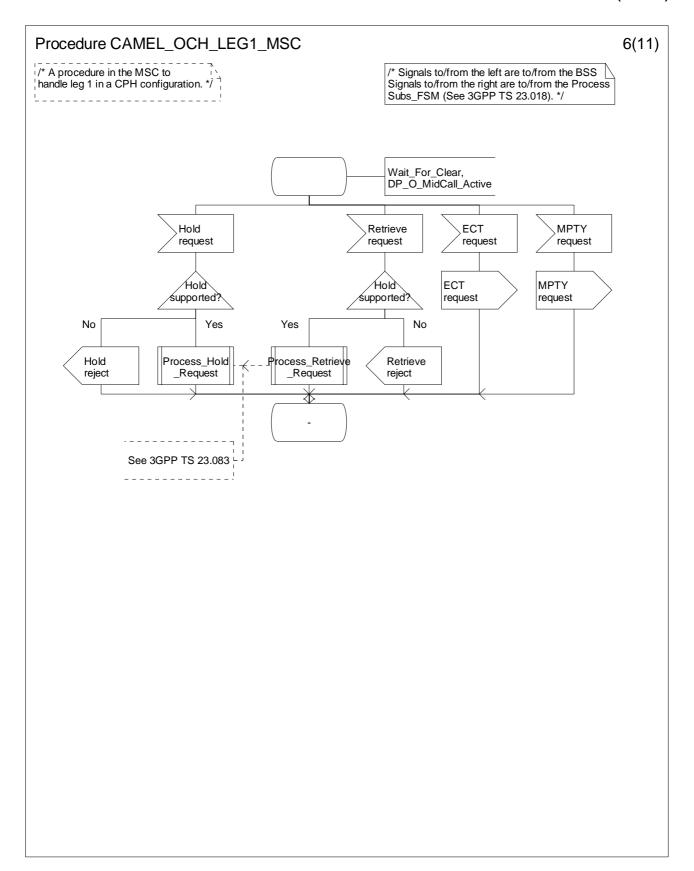
Figure 4.30-6: Procedure CAMEL\_OCH\_LEG1\_MSC (sheet 6)
