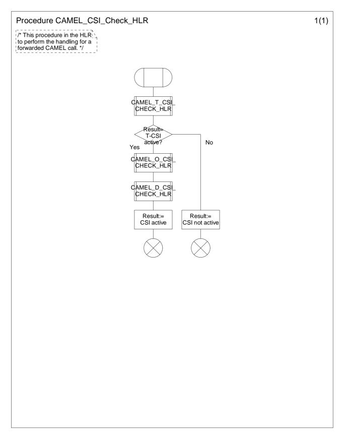
Figure 4.56-1: Procedure CAMEL\_CSI\_Check\_HLR (sheet 1)
