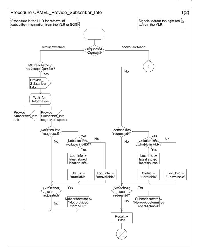
Figure 4.116-1: Procedure CAMEL\_Provide\_Subscriber\_Info (sheet 1)
