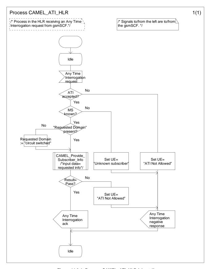
Figure 11.3-1: Process CAMEL\_ATI\_HLR (sheet 1)
