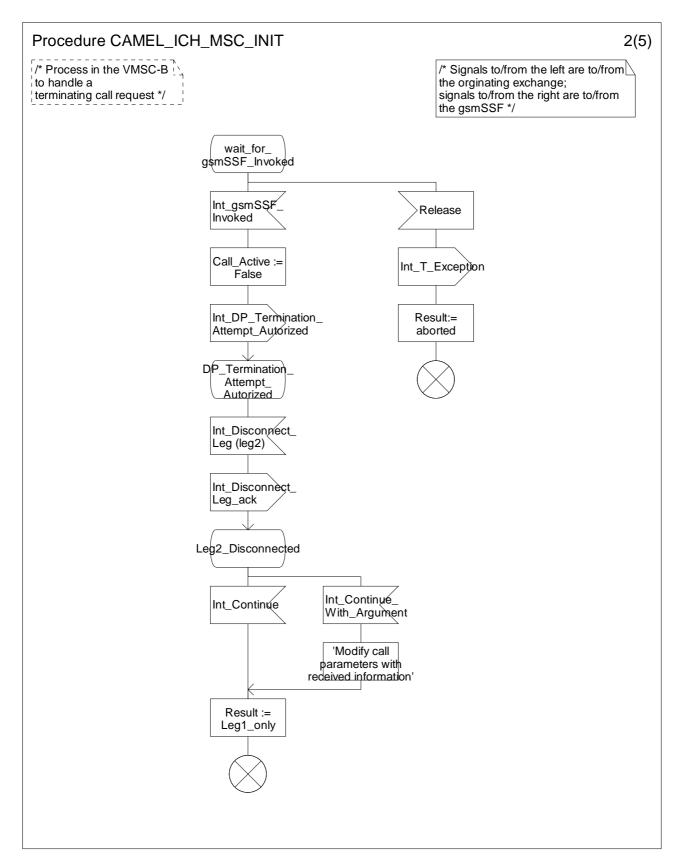
Figure 4.66-2: Procedure CAMEL\_ICH\_MSC\_INIT (sheet 2)
