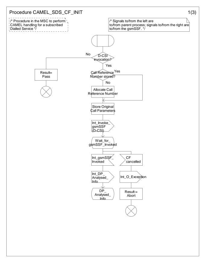
Figure 4.77-1: Procedure CAMEL\_SDS\_CF\_INIT (sheet 1)
