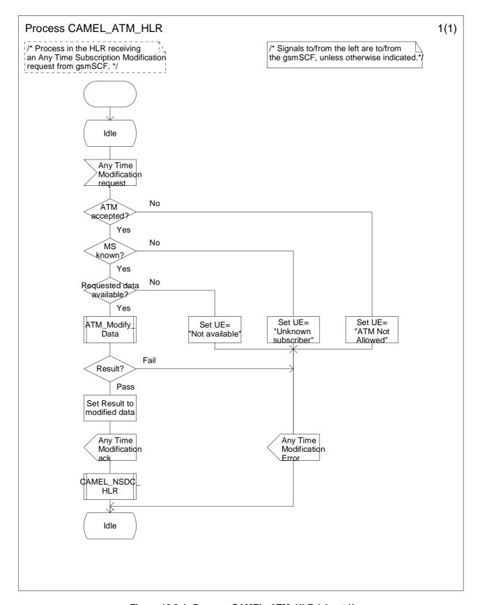
Figure 10.3-1: Process CAMEL\_ATM\_HLR (sheet 1)
