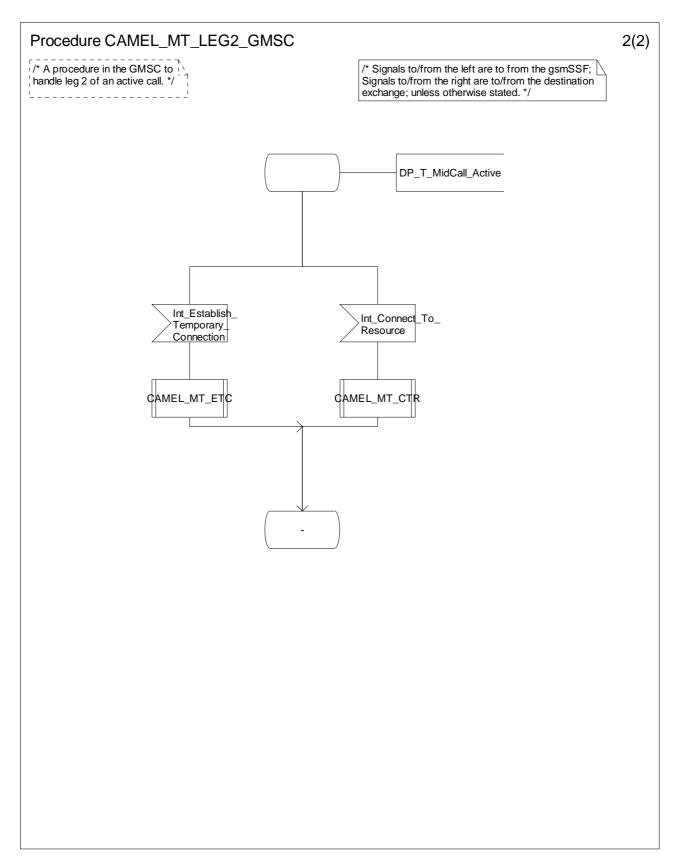
Figure 4.52-2: Procedure CAMEL\_MT\_LEG2\_GMSC (sheet 2)
