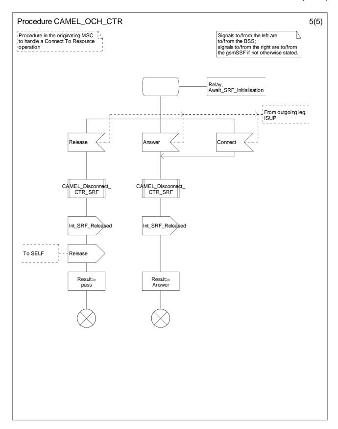
Figure 4.24-5: Procedure CAMEL\_OCH\_CTR (sheet 5)
