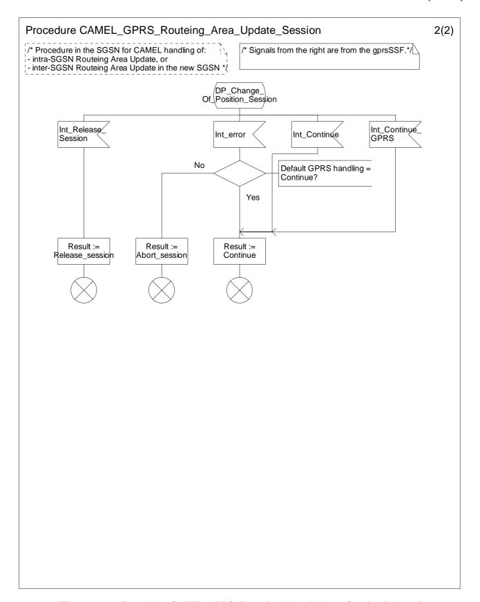
Figure 6.10-2: Procedure CAMEL\_GPRS\_Routeing\_Area\_Update\_Session (sheet 2)
