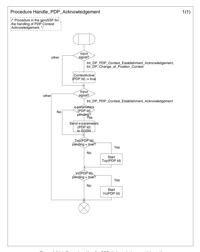
Figure 6.24-1: Procedure Handle\_PDP\_Acknowledgement (sheet 1)
