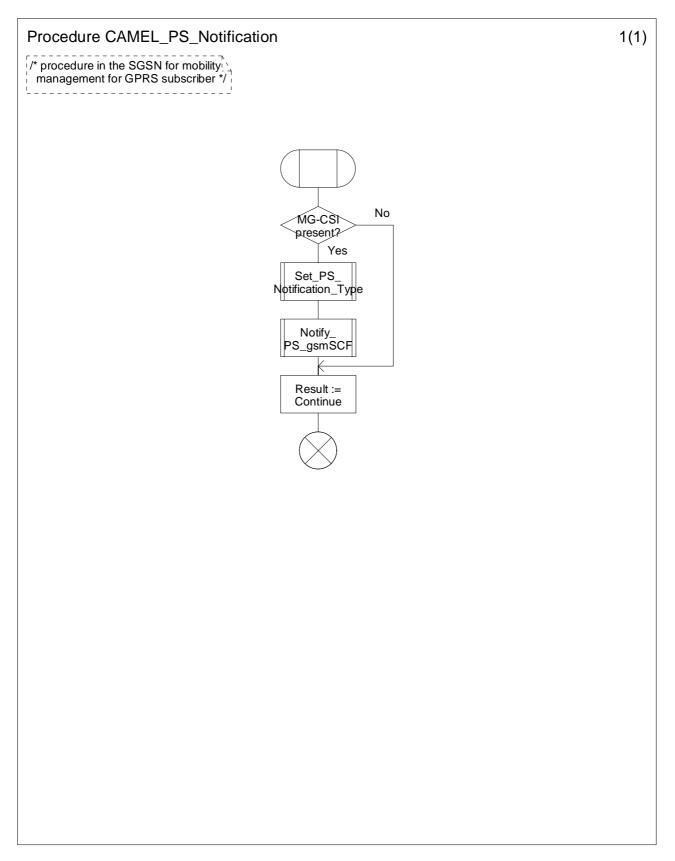
Figure 9.5-1: Procedure CAMEL\_PS\_Notification (sheet 1)
