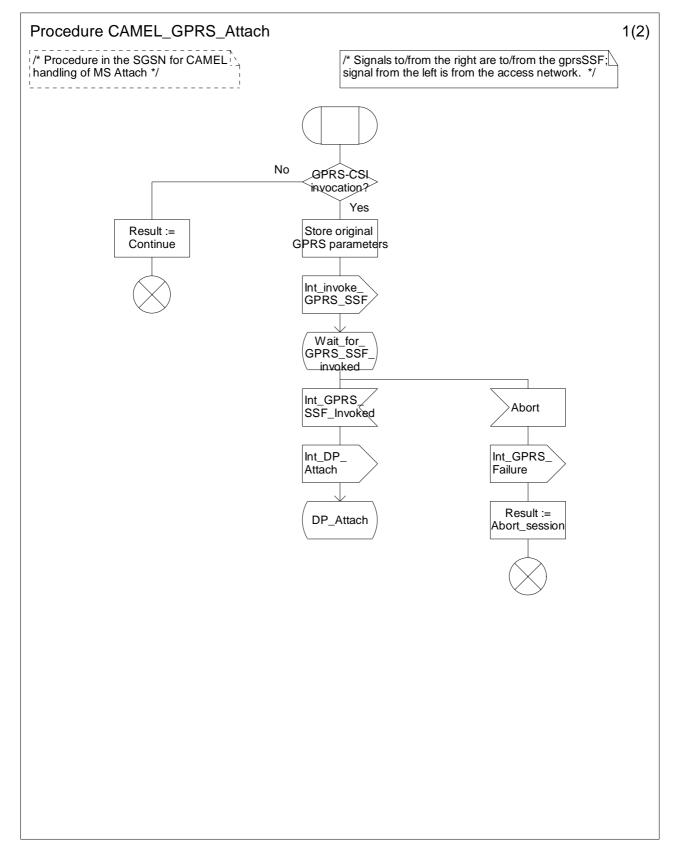
Figure 6.8-1: Procedure CAMEL\_GPRS\_Attach (sheet 1)
