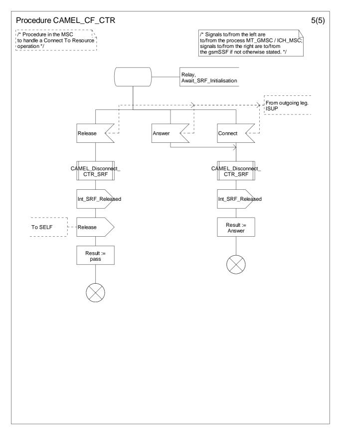
Figure 4.82-5: Procedure CAMEL\_CF\_CTR (sheet 5)
