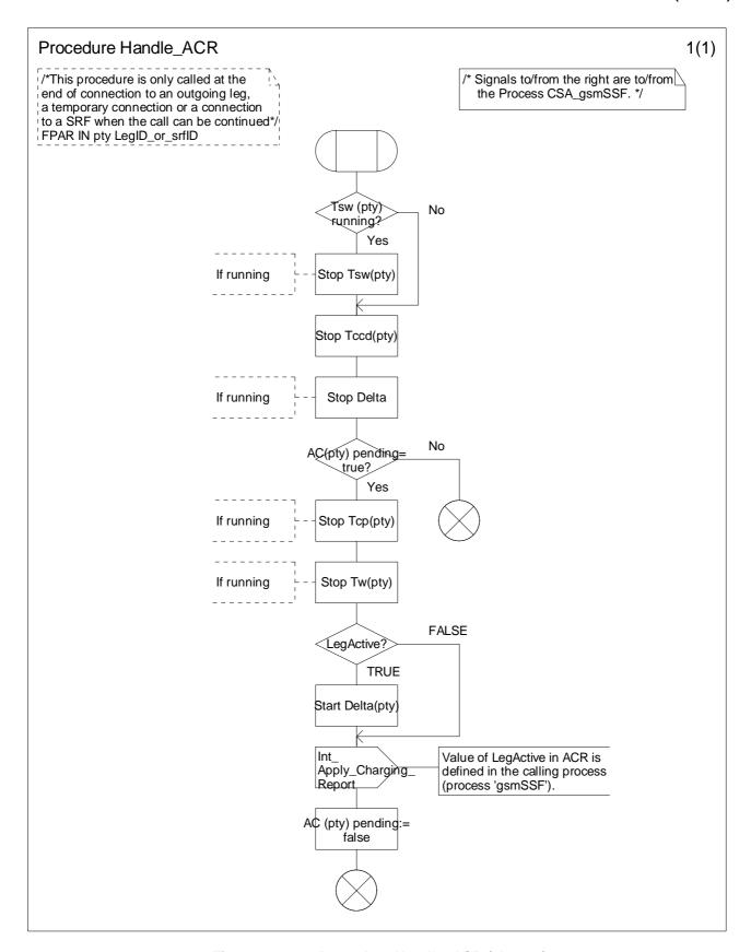
Figure 4.102-1: Procedure Handle\_ACR (sheet 1)
