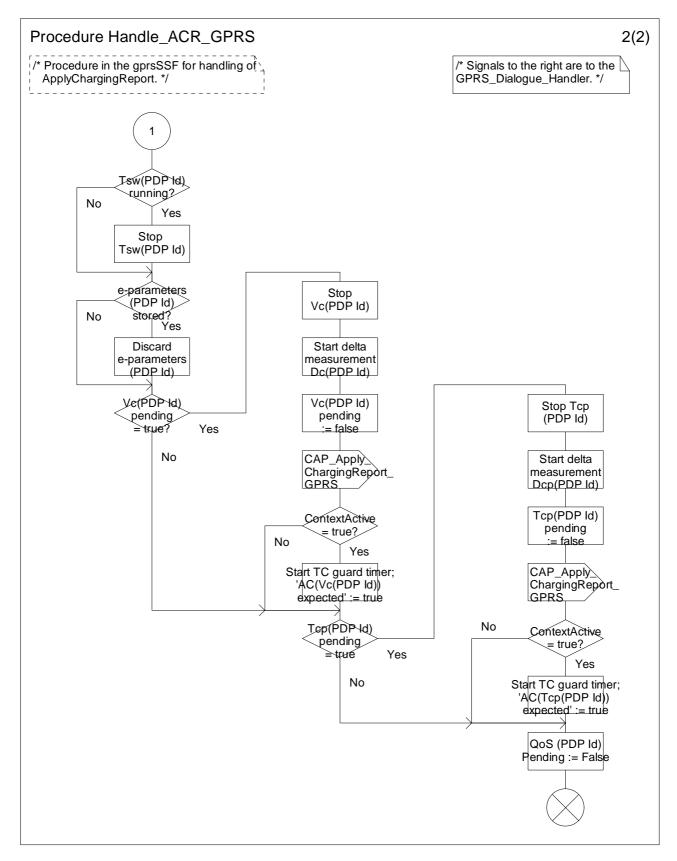
Figure 6.20-2: Procedure Handle\_ACR\_GPRS (sheet 2)
