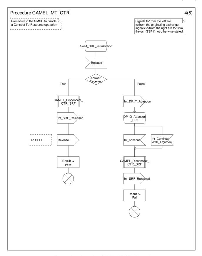
Figure 4.50-4: Procedure CAMEL\_MT\_CTR (sheet 4)
