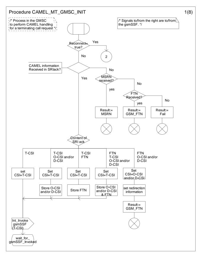
Figure 4.40-1: Procedure CAMEL\_MT\_GMSC\_INIT (sheet 1)
