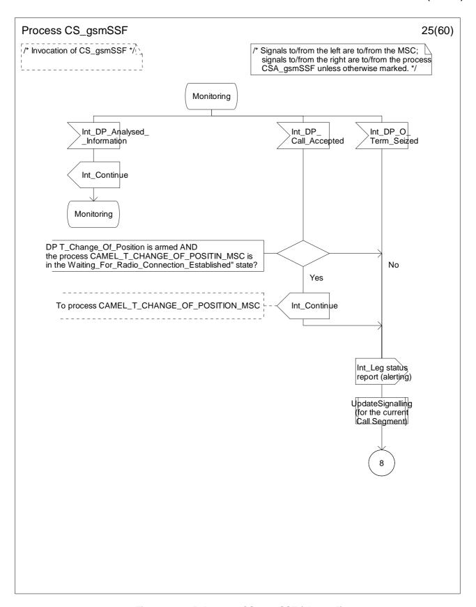
Figure 4.96-25: Process CS\_gsmSSF (sheet 25)
