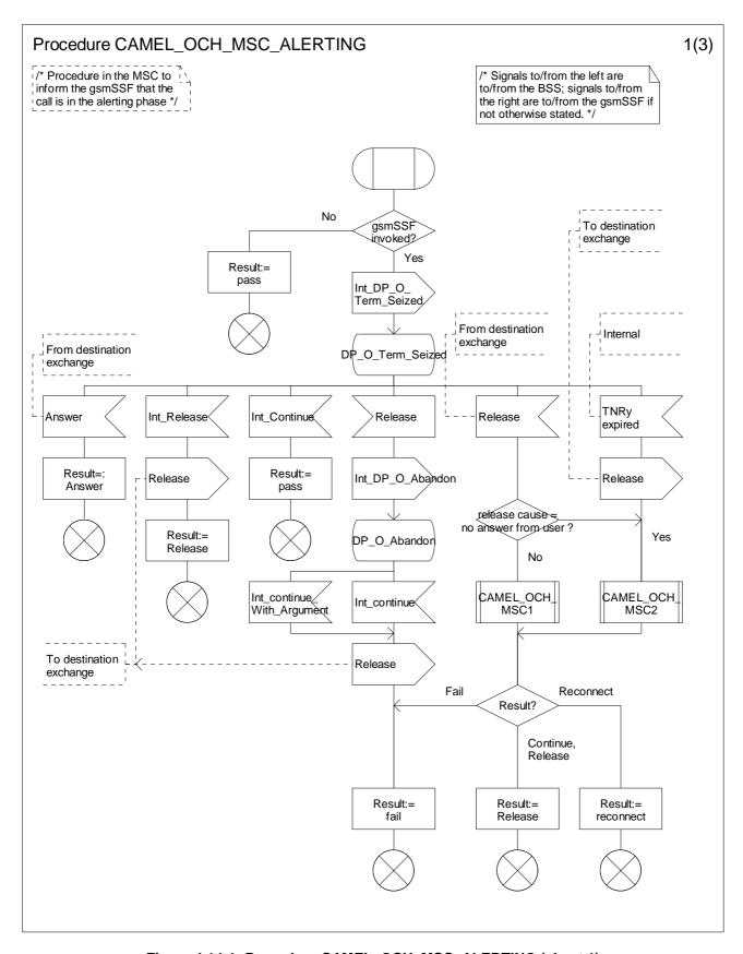
Figure 4.14-1: Procedure CAMEL\_OCH\_MSC\_ALERTING (sheet 1)
