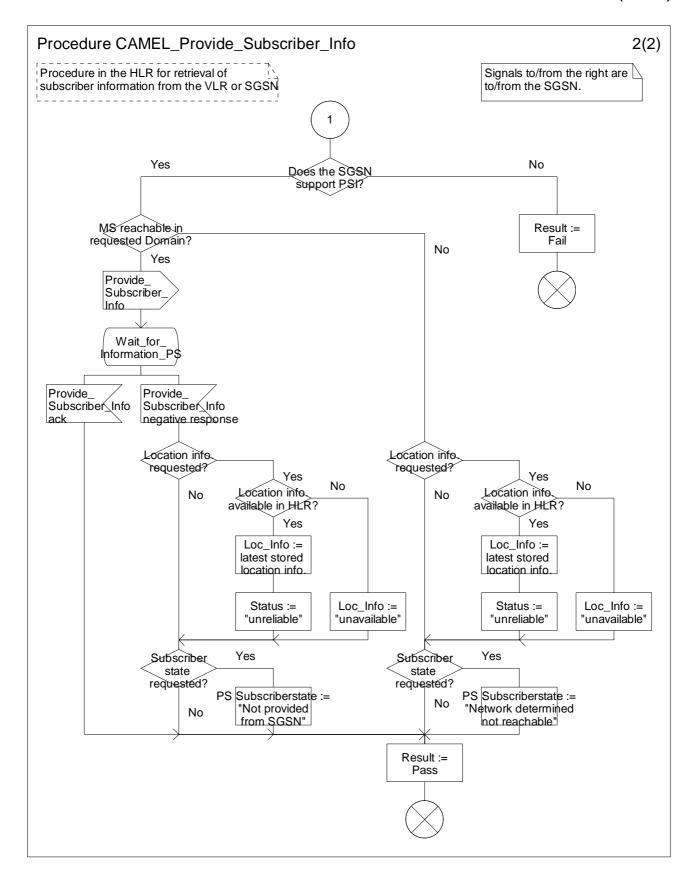
Figure 4.116-2: Procedure CAMEL\_Provide\_Subscriber\_Info (sheet 2)
