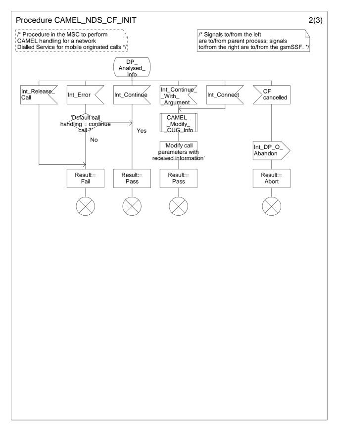
Figure 4.78-2: Procedure CAMEL\_NDS\_CF\_INIT (sheet 2)
