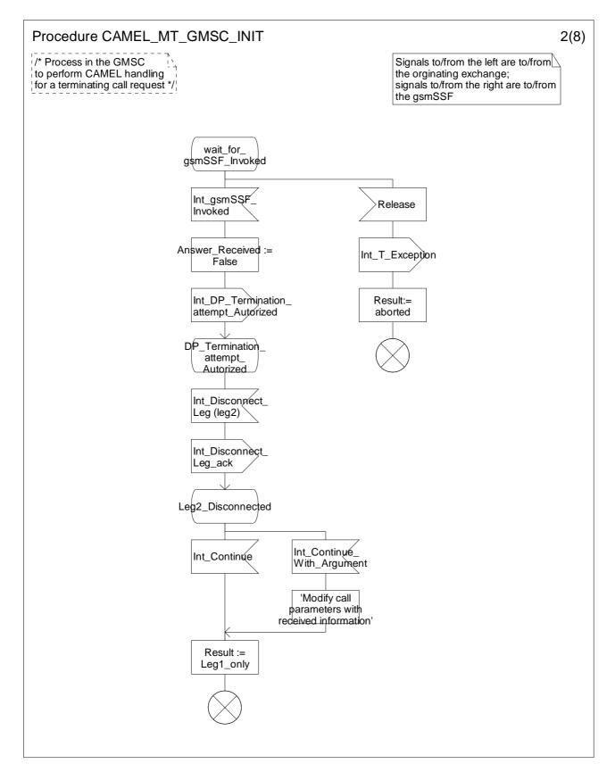
Figure 4.40-2: Procedure CAMEL\_MT\_GMSC\_INIT (sheet 2)
