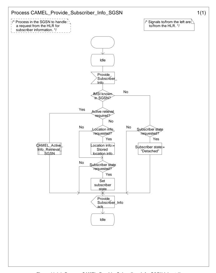
Figure 11.4-1: Process CAMEL\_Provide\_Subscriber\_Info\_SGSN (sheet 1)
