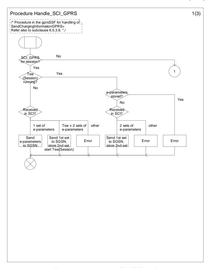
Figure 6.23-1: Procedure Handle\_SCI\_GPRS (sheet 1)
