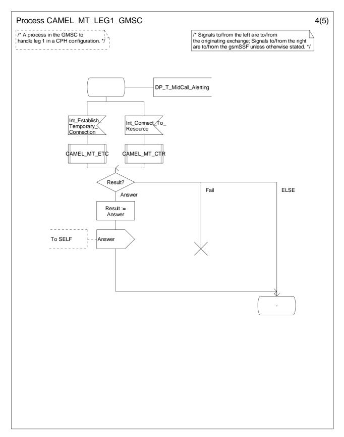
Figure 4.53-4: Process CAMEL\_MT\_LEG1\_GMSC (sheet 4)
