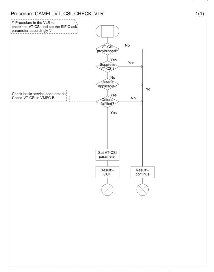
Figure 4.65-1: Procedure CAMEL\_VT\_CSI\_Check\_VLR (sheet 1)
