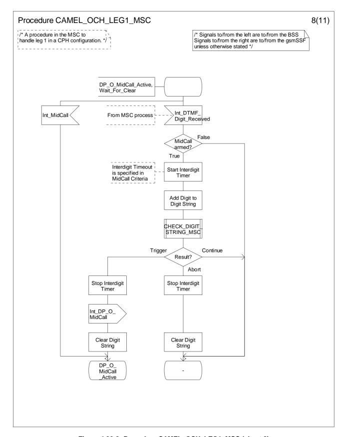
Figure 4.30-8: Procedure CAMEL\_OCH\_LEG1\_MSC (sheet 8)
