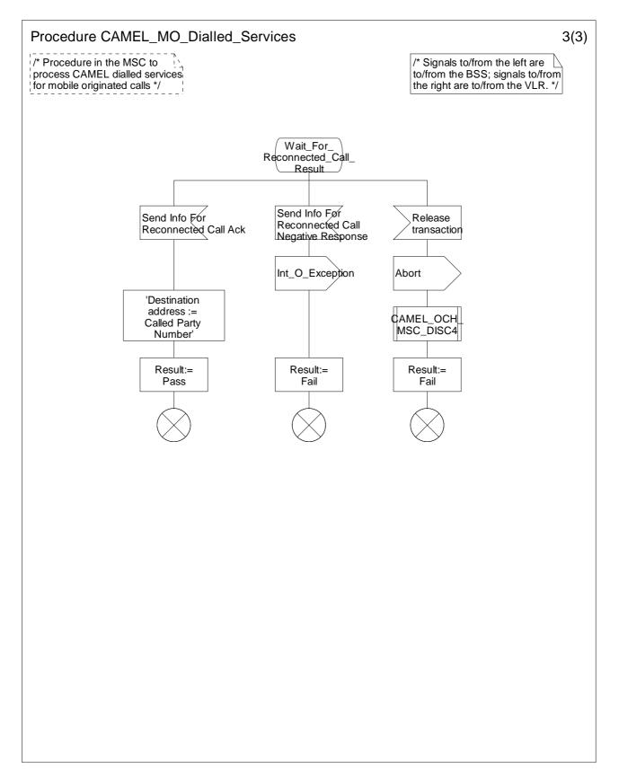
Figure 4.11-3: Procedure CAMEL\_MO\_Dialled\_Services (sheet 3)
