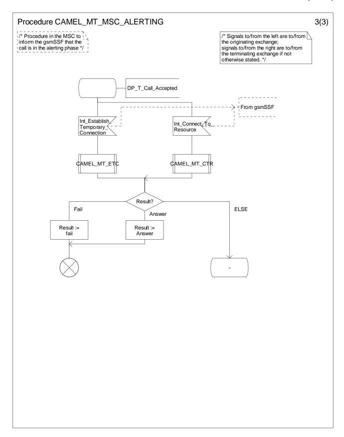
Figure 4.41-3: Procedure CAMEL\_MT\_MSC\_ALERTING (sheet 3)
