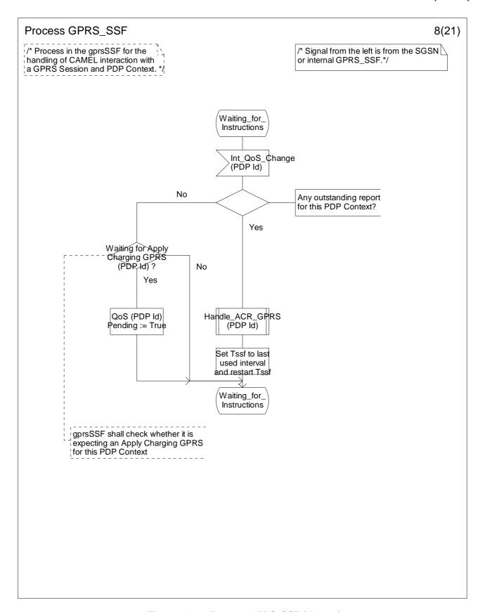
Figure 6.17-8: Process GPRS\_SSF (sheet 8)
