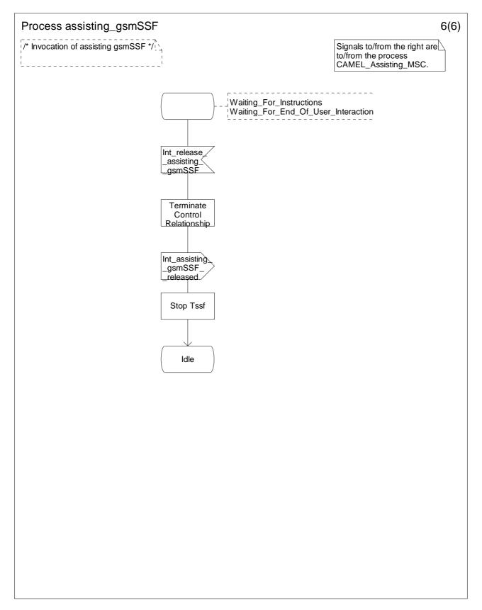
Figure 4.115-6: Process Assisting\_gsmSSF (sheet 6)
