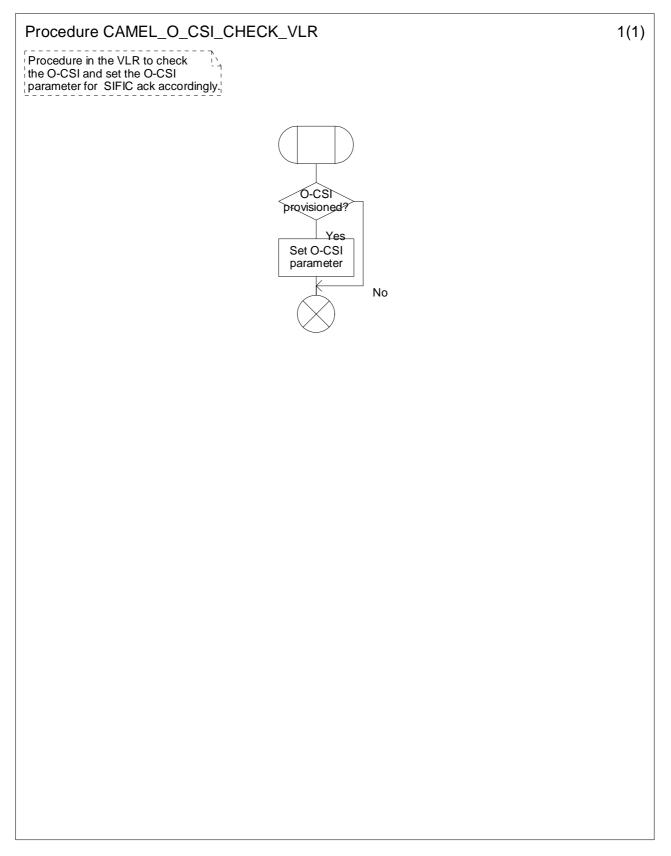
Figure 4.63-1: Procedure CAMEL\_O\_CSI\_Check\_VLR (sheet 1)
