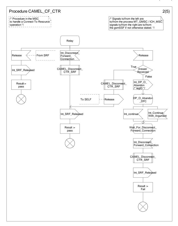
Figure 4.82-2: Procedure CAMEL\_CF\_CTR (sheet 2)
