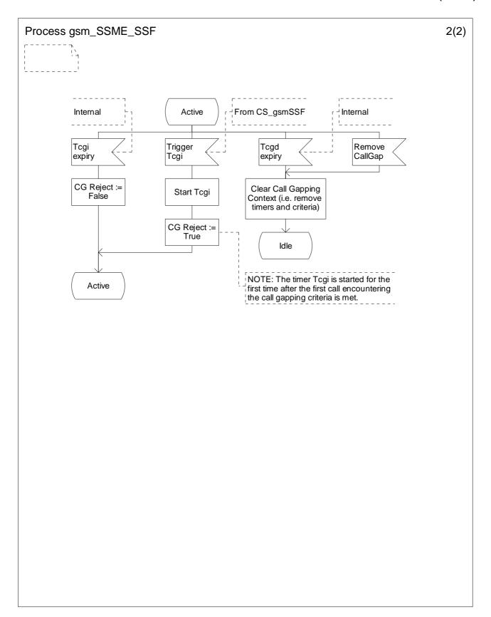
Figure 4.110-2: Process gsm\_SSME\_SSF (sheet 2)
