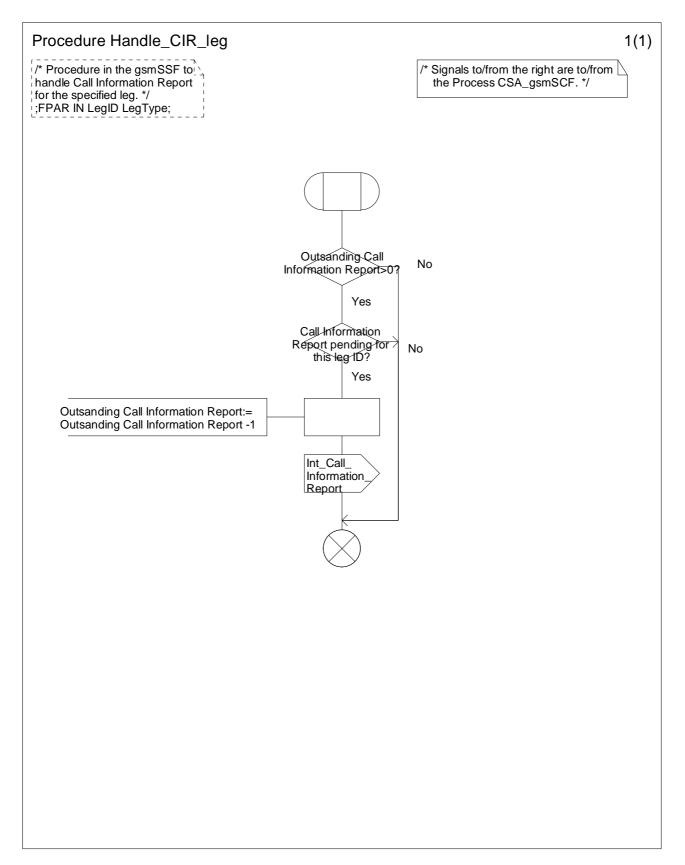
Figure 4.104-1: Procedure Handle\_CIR\_leg (sheet 1)
