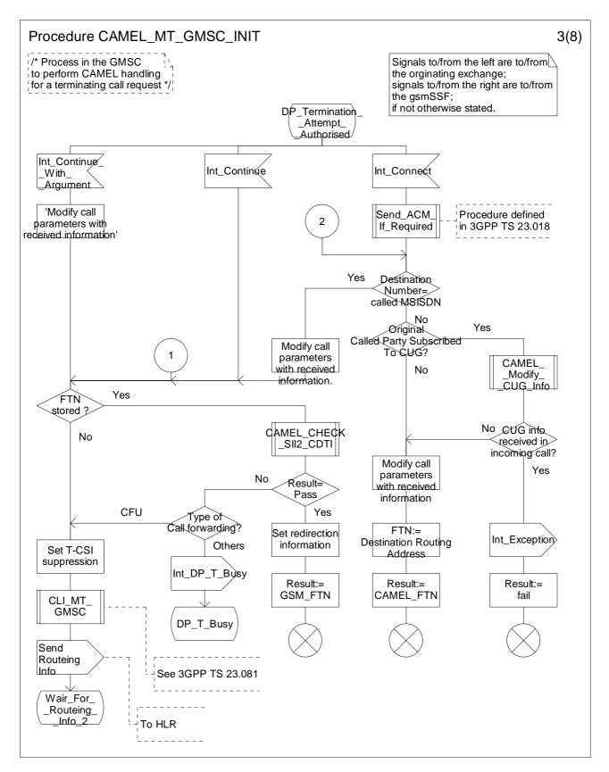
Figure 4.40-3: Procedure CAMEL\_MT\_GMSC\_INIT (sheet 3)
