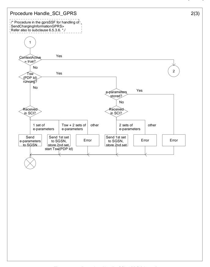
Figure 6.23-2: Procedure Handle\_SCI\_GPRS (sheet 2)
