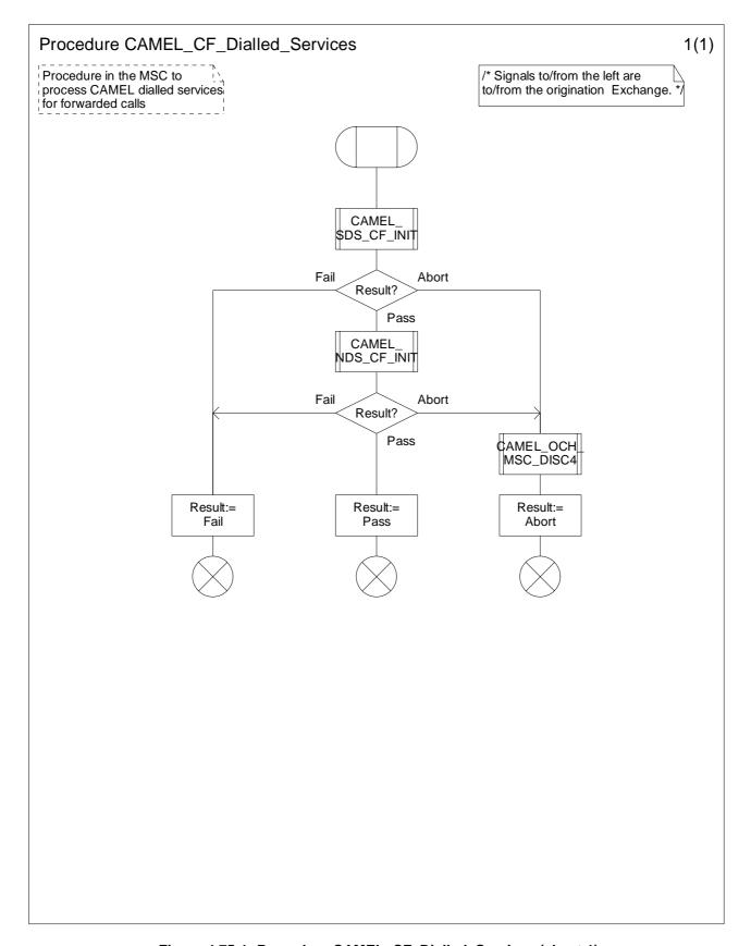
Figure 4.75-1: Procedure CAMEL\_CF\_Dialled\_Services (sheet 1)
