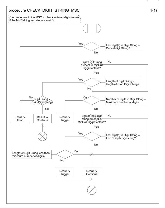
Figure 4.31-1: Procedure CHECK\_DIGIT\_STRING\_MSC (sheet 1)
