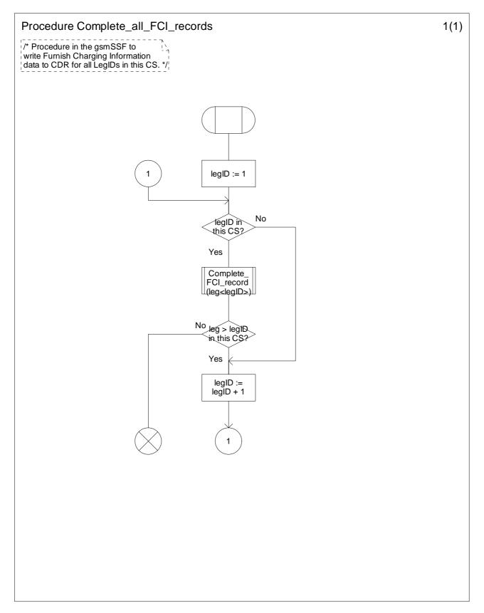
Figure 4.106-1: Procedure Complete\_all\_FCI\_records (sheet 1)
