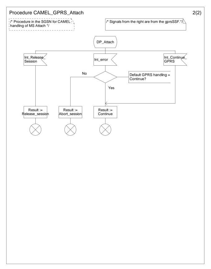
Figure 6.8-2: Procedure CAMEL\_GPRS\_Attach (sheet 2)
