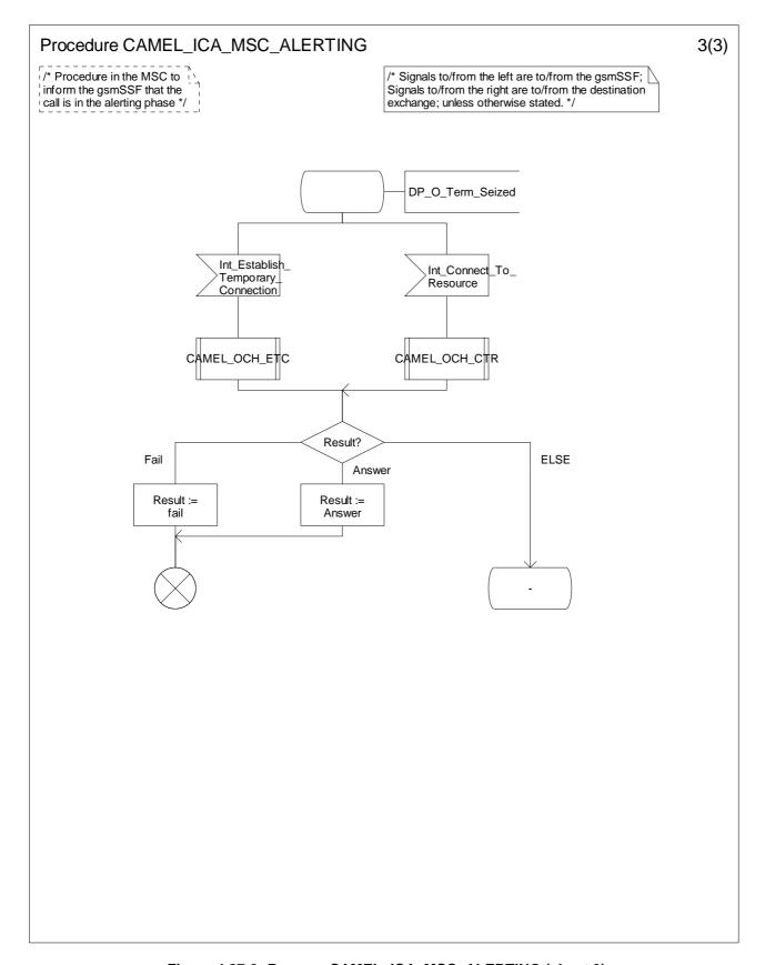
Figure 4.87-3: Process CAMEL\_ICA\_MSC\_ALERTING (sheet 3)
