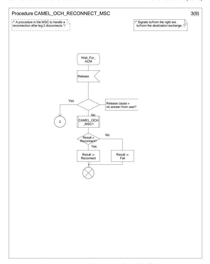
Figure 4.33-3: Procedure CAMEL\_OCH\_RECONNECT\_MSC (sheet 3)
