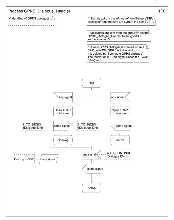
Figure 6.18-1: Process GPRS\_Dialogue\_Handler (sheet 1)
