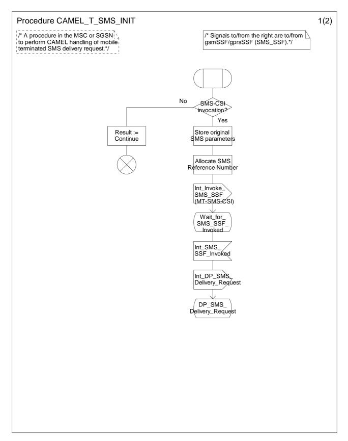
Figure 7.10-1: Procedure CAMEL\_T\_SMS\_INIT (sheet 1)
