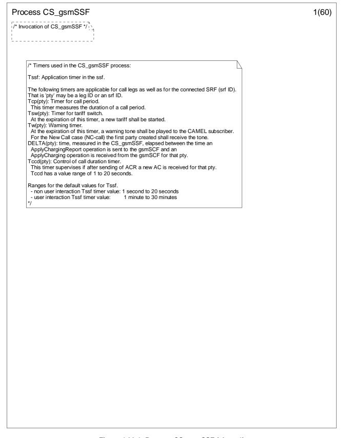
Figure 4.96-1: Process CS\_gsmSSF (sheet 1)
