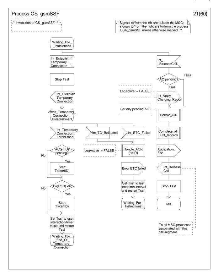
Figure 4.96-21: Process CS\_gsmSSF (sheet 21)
