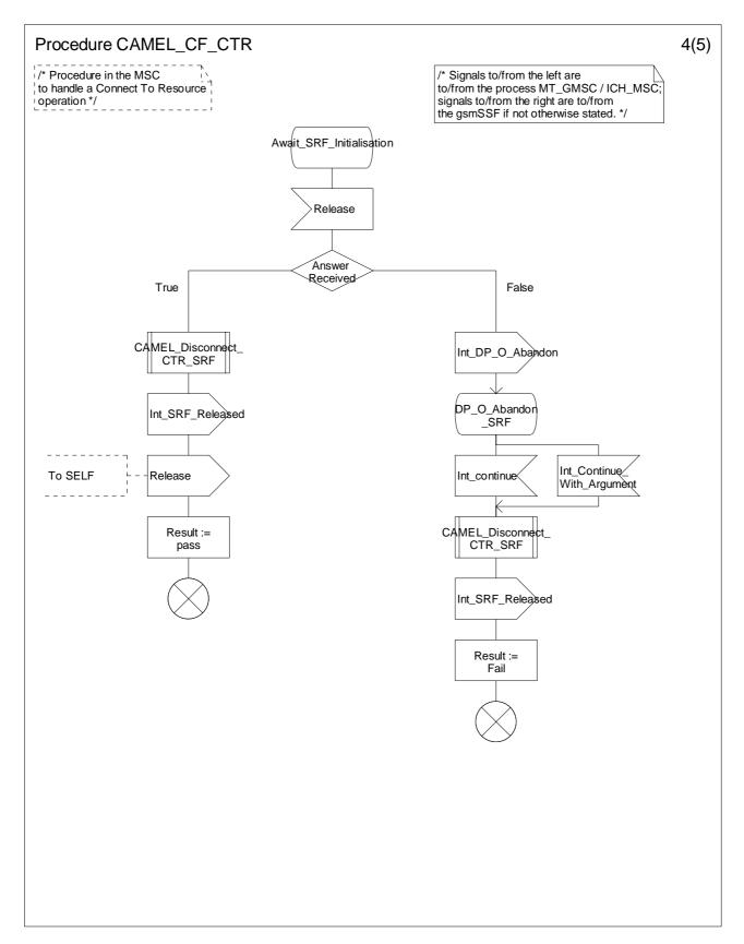
Figure 4.82-4: Procedure CAMEL\_CF\_CTR (sheet 4)
