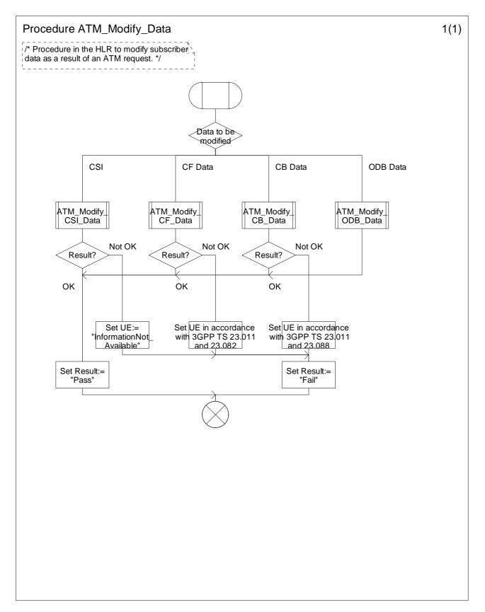
Figure 10.4-1: Procedure ATM\_Modify\_Data (sheet 1)
