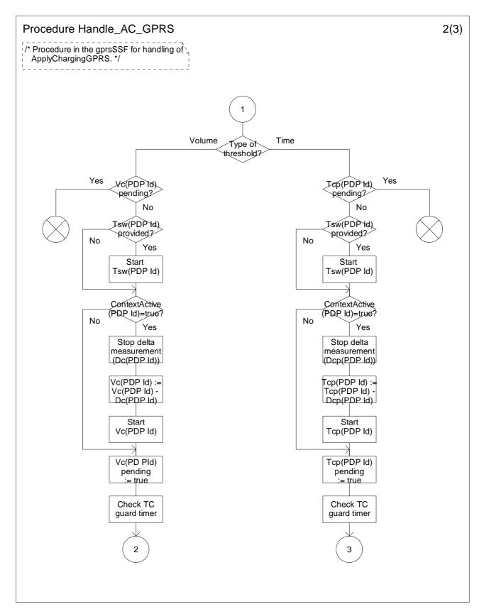
Figure 6.19-2: Procedure Handle\_AC\_GPRS (sheet 2)
