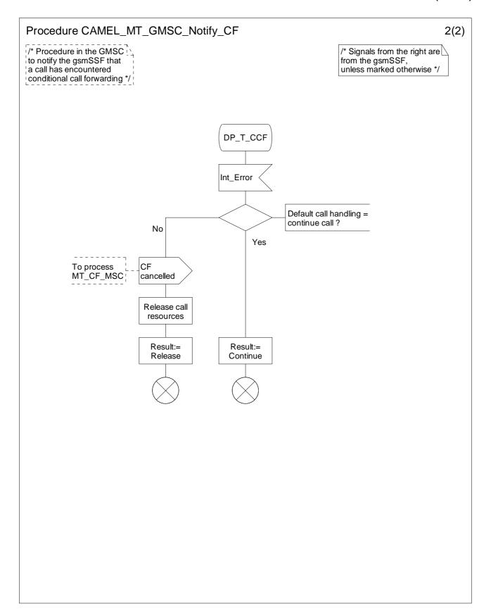
Figure 4.51-2: Procedure CAMEL\_MT\_GMSC\_Notify\_CF (sheet 2)
