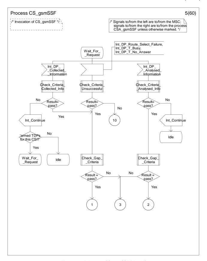
Figure 4.96-5: Process CS\_gsmSSF (sheet 5)
