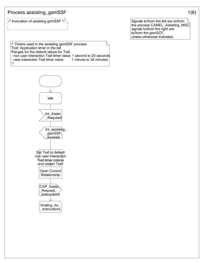
Figure 4.115-1: Process Assisting\_gsmSSF (sheet 1)
