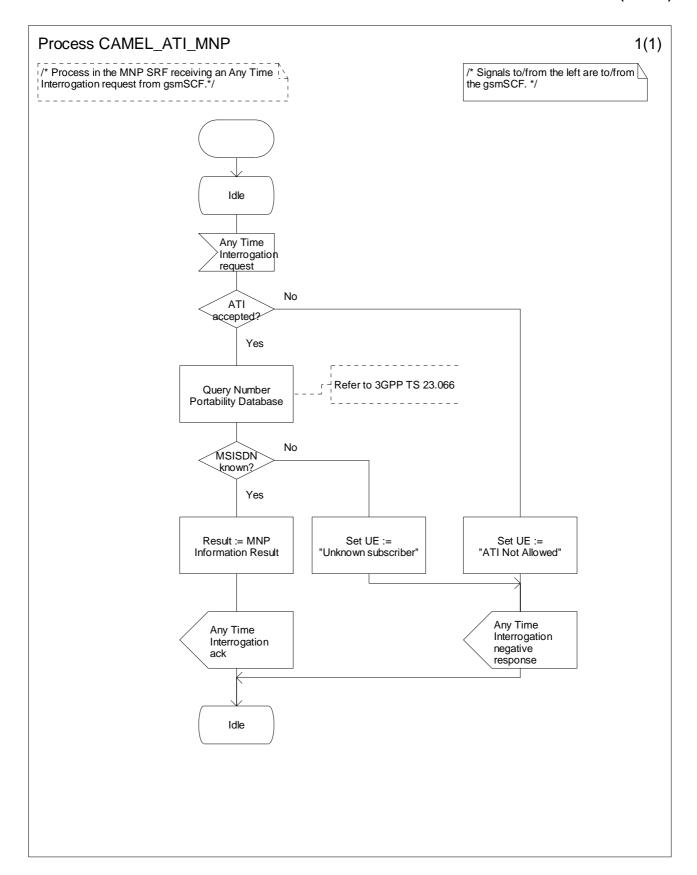
Figure 12.2-1: Process CAMEL\_ATI\_MNP (sheet 1)
