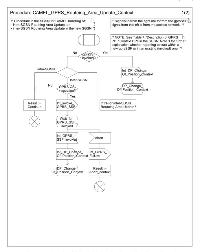
Figure 6.11-1: Procedure CAMEL\_GPRS\_Routeing\_Area\_Update\_Context (sheet 1)
