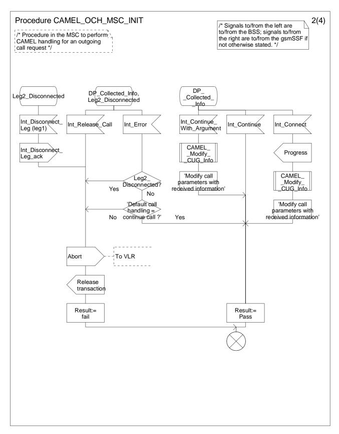
Figure 4.10-2: Procedure CAMEL\_OCH\_MSC\_INIT (sheet 2)
