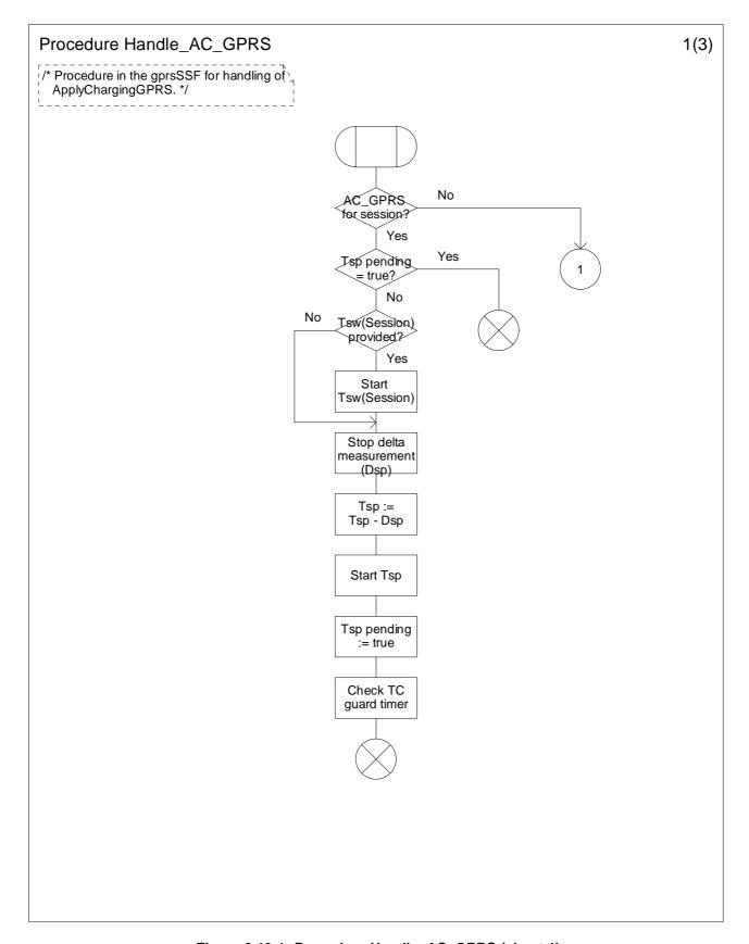
Figure 6.19-1: Procedure Handle\_AC\_GPRS (sheet 1)
