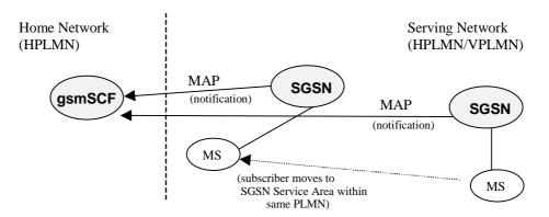
Figure 9.4-2: Routeing Area Update from one SGSN Service Area to another SGSN Service Area
