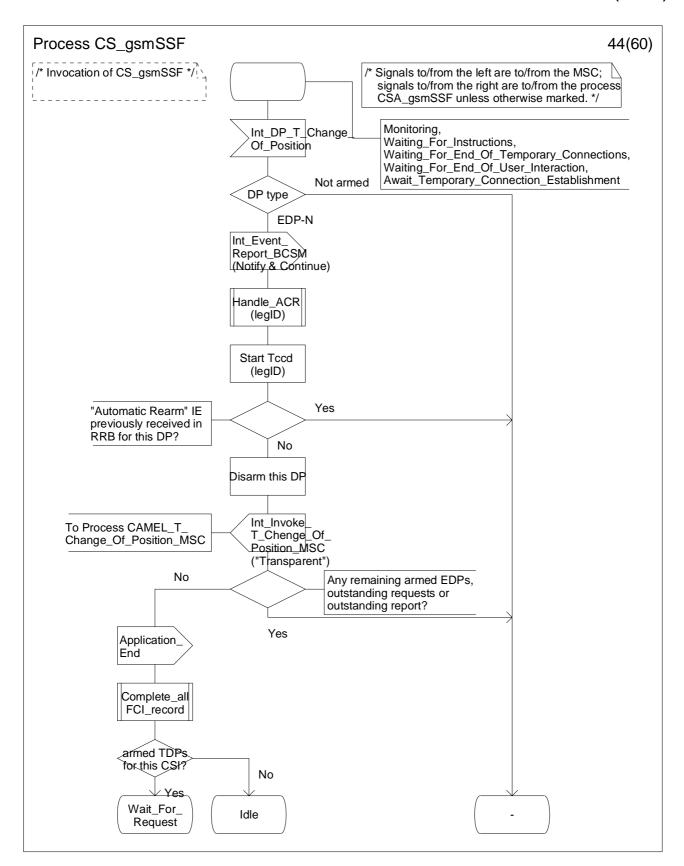
Figure 4.96-44: Process CS\_gsmSSF (sheet 44)
