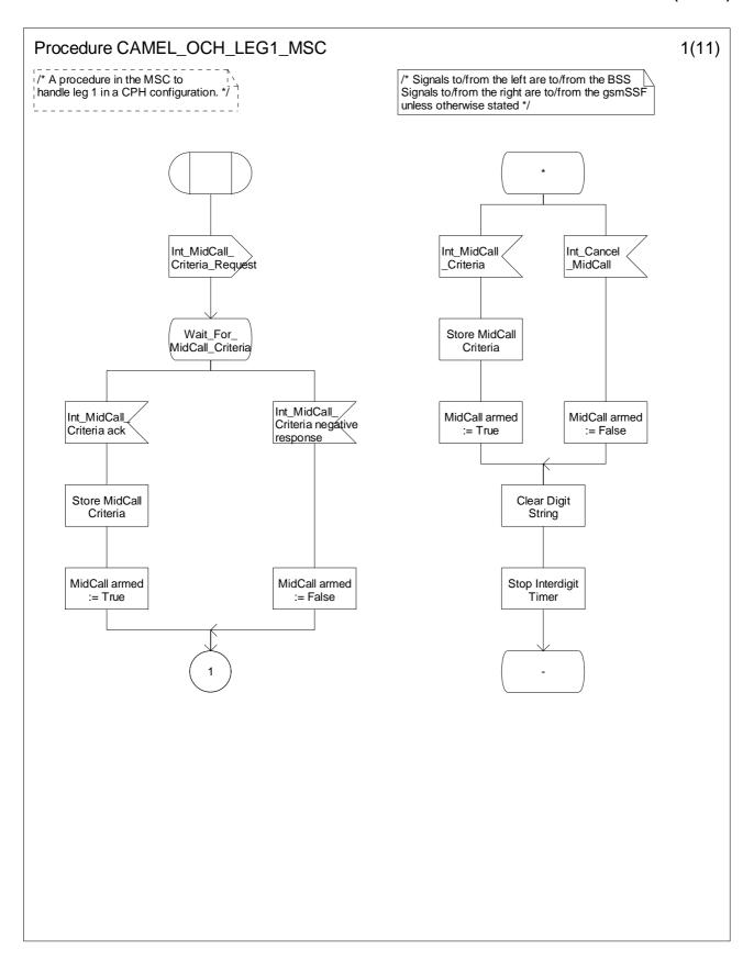
Figure 4.30-1: Procedure CAMEL\_OCH\_LEG1\_MSC (sheet 1)
