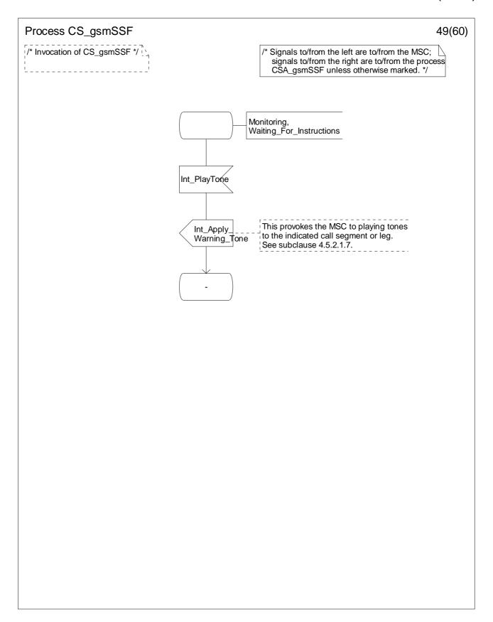
Figure 4.96-49: Process CS\_gsmSSF (sheet 49)
