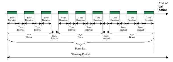
Figure 4.94: Representation of burst list
