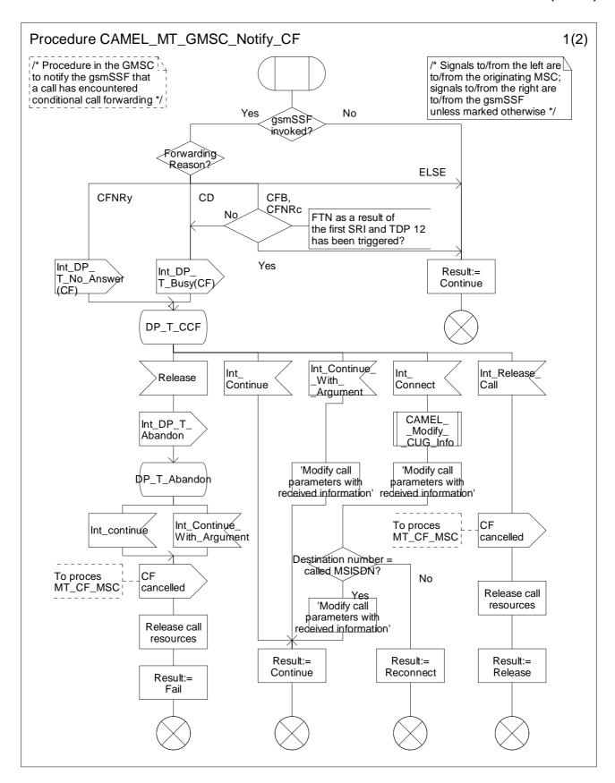
Figure 4.51-1: Procedure CAMEL\_MT\_GMSC\_Notify\_CF (sheet 1)
