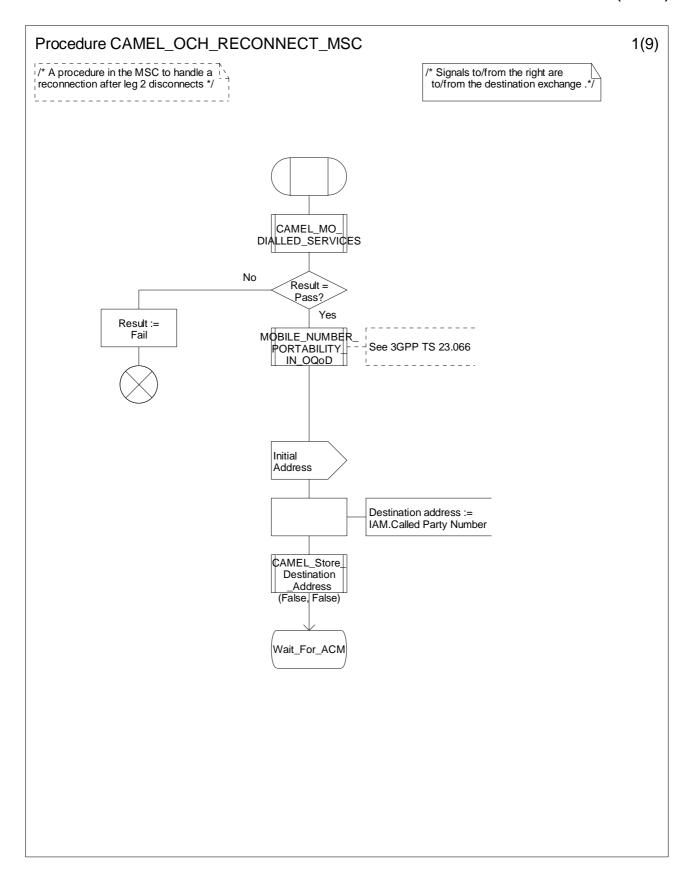
Figure 4.33-1: Procedure CAMEL\_OCH\_RECONNECT\_MSC (sheet 1)
