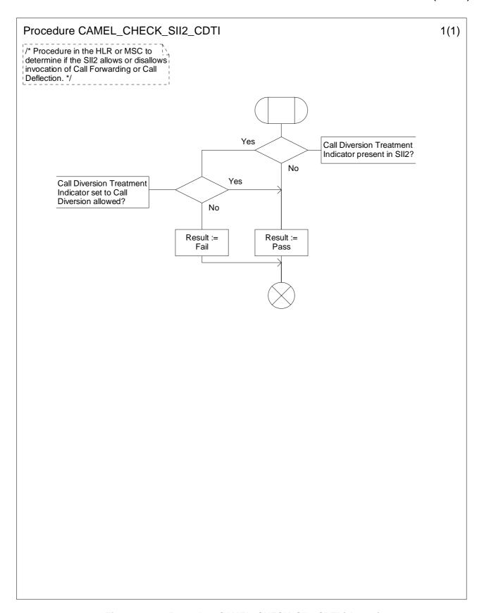
Figure 4.60-1: Procedure CAMEL\_CHECK\_SII2\_CDTI (sheet 1)
