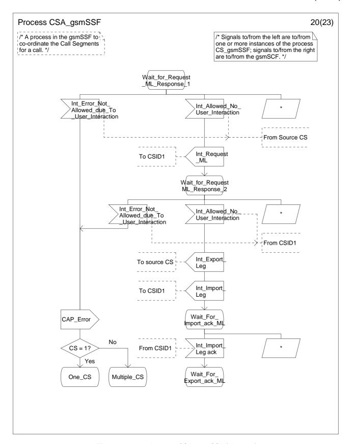
Figure 4.113-20: Process CSA\_gsmSSF (sheet 20)
