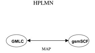
Figure 11.1-1: Functional architecture for CAMEL Support of Location Services
