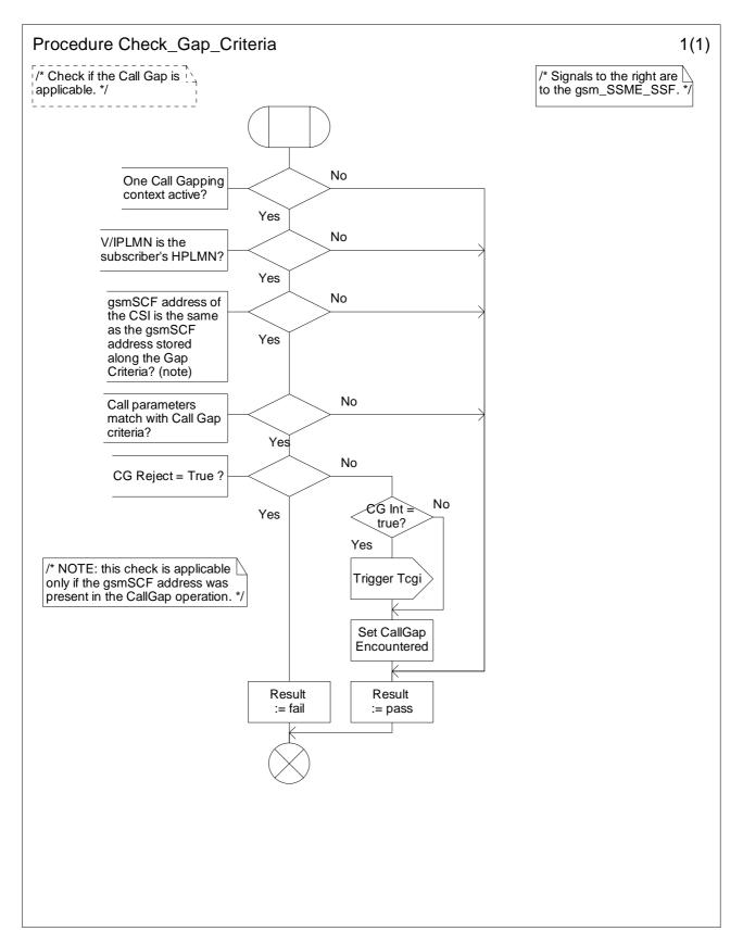
Figure 4.112-1: Procedure Check\_Gap\_Criteria (sheet 1)
