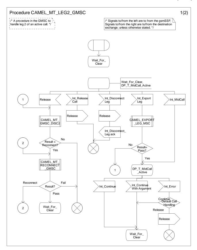
Figure 4.52-1: Procedure CAMEL\_MT\_LEG2\_GMSC (sheet 1)
