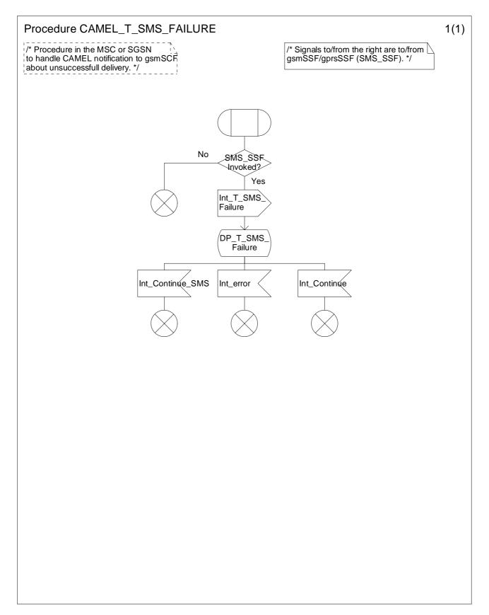
Figure 7.11-1: Procedure CAMEL\_T\_SMS\_FAILURE (sheet 1)
