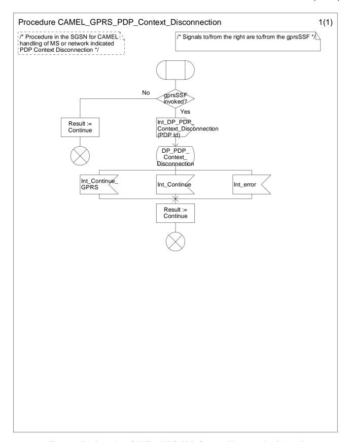
Figure 6.15-1: Procedure CAMEL\_GPRS\_PDP\_Context\_Disconnection (sheet 1)
