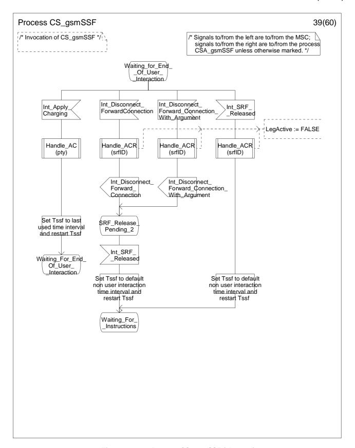
Figure 4.96-39: Process CS\_gsmSSF (sheet 39)
