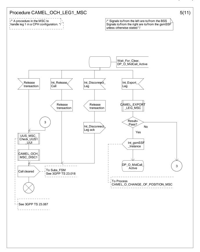
Figure 4.30-5: Procedure CAMEL\_OCH\_LEG1\_MSC (sheet 5)
