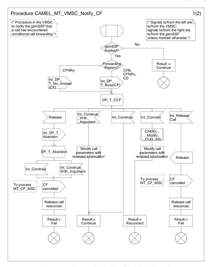
Figure 4.67-1: Procedure CAMEL\_MT\_VMSC\_Notify\_CF (sheet 1)
