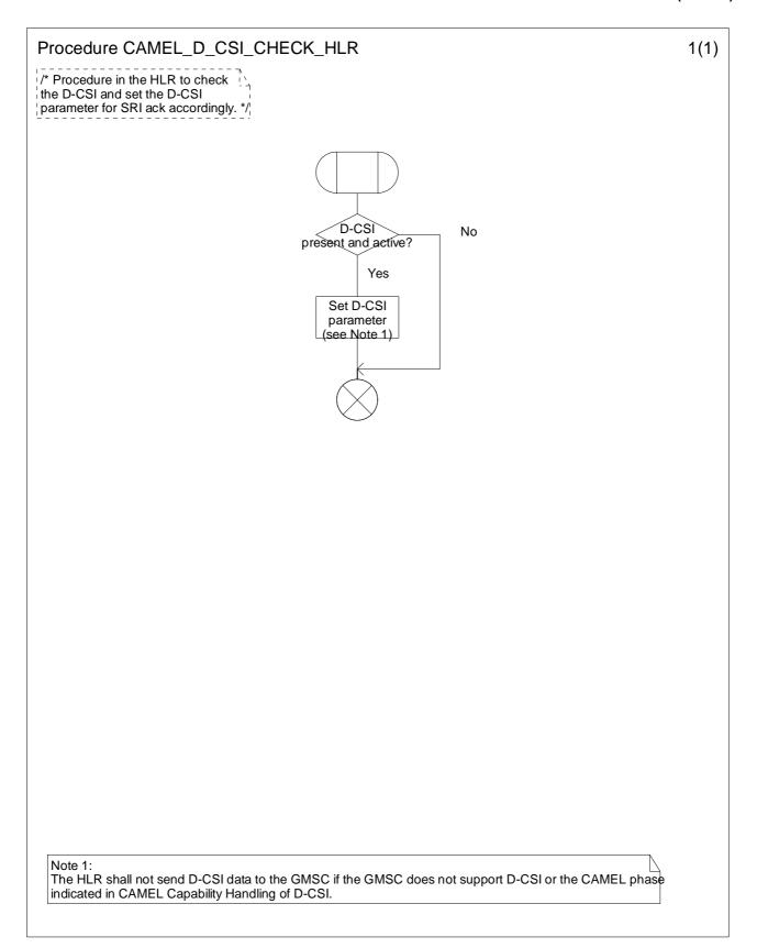
Figure 4.58-1: Procedure CAMEL\_D\_CSI\_CHECK\_HLR (sheet 1)
