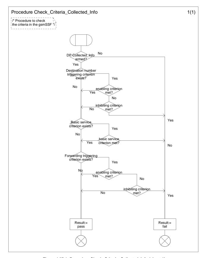
Figure 4.97-1: Procedure Check\_Criteria\_Collected\_Info (sheet 1)
