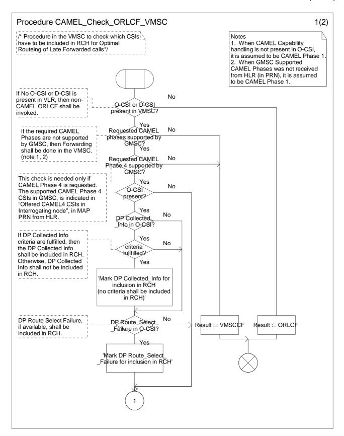
Figure 4.74-1: Procedure CAMEL\_Check\_ORLCF\_VMSC (sheet 1)
