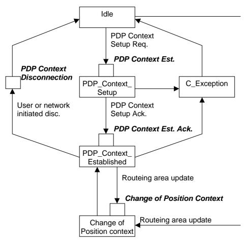
Figure 6.4: GPRS PDP Context State Model
