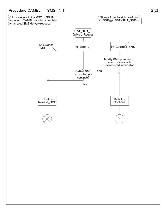
Figure 7.10-2: Procedure CAMEL\_T\_SMS\_INIT (sheet 2)
