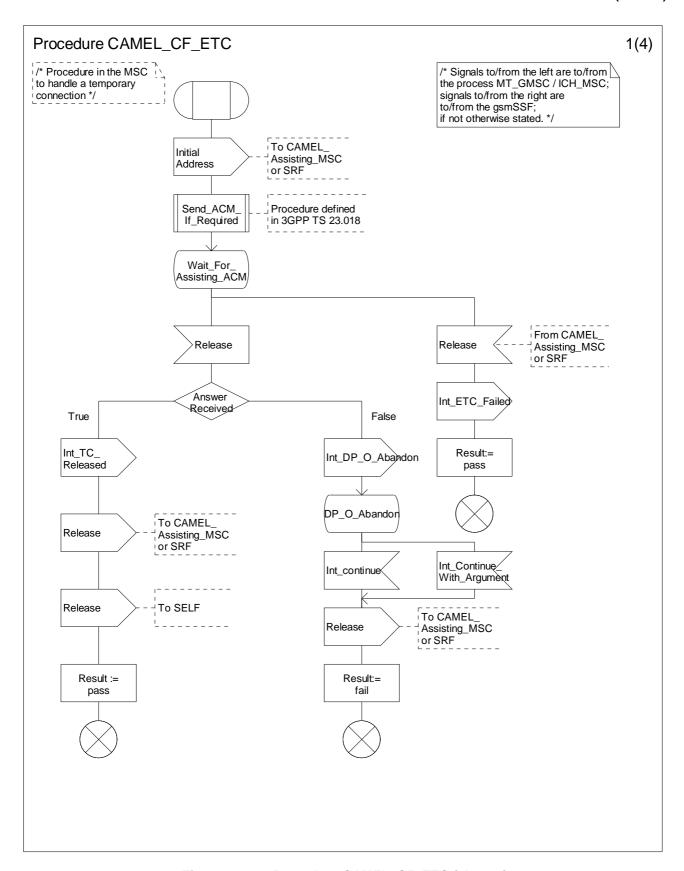
Figure 4.84-1: Procedure CAMEL\_CF\_ETC (sheet 1)
