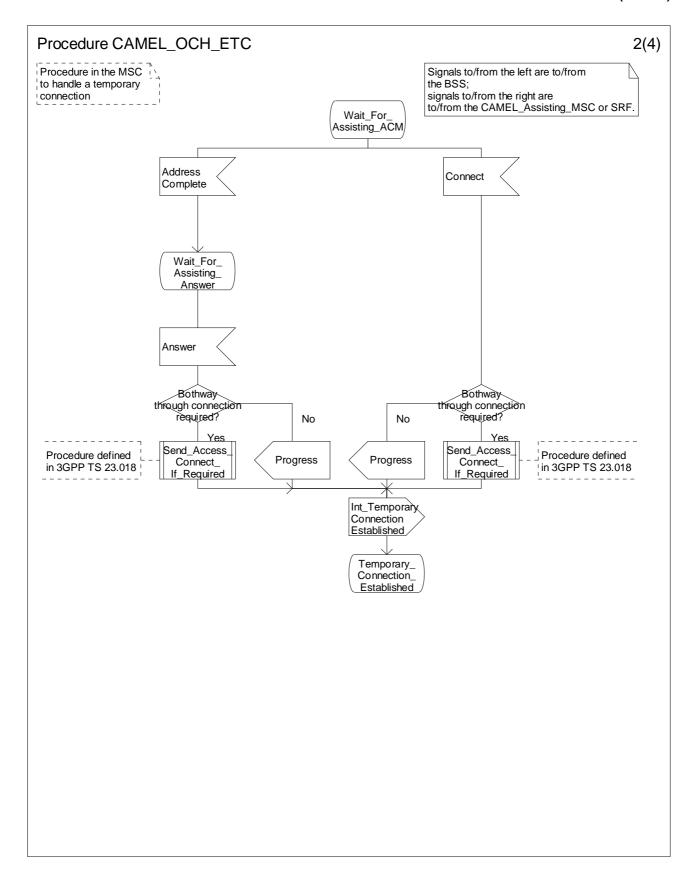
Figure 4.23-2: Procedure CAMEL\_OCH\_ETC (sheet 2)
