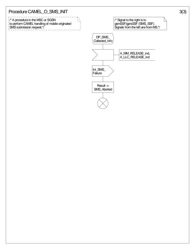
Figure 7.5-3: Procedure CAMEL\_O\_SMS\_INIT (sheet 3)
