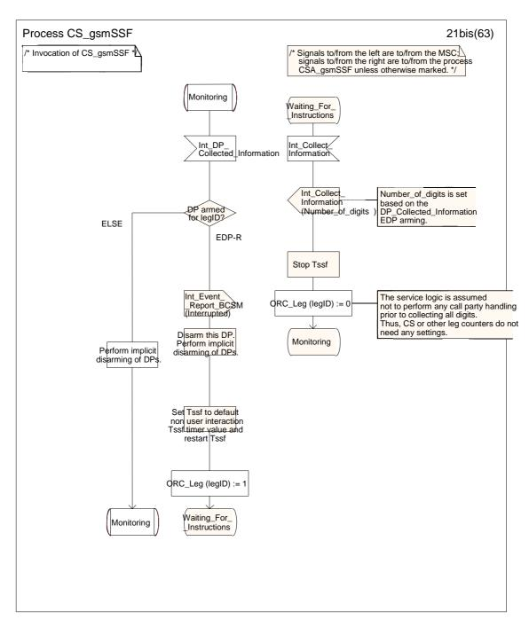
Figure 4.99-21A: Process CS\_gsmSSF (sheet 21A)
