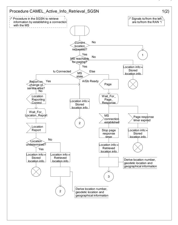
Figure 11.5-1: Procedure CAMEL\_Active\_Info\_Retrieval\_SGSN (sheet 1)
