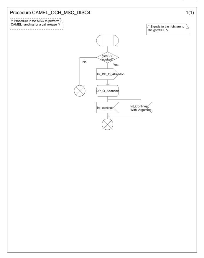
Figure 4.21-1: Procedure CAMEL\_OCH\_MSC\_DISC4 (sheet 1)
