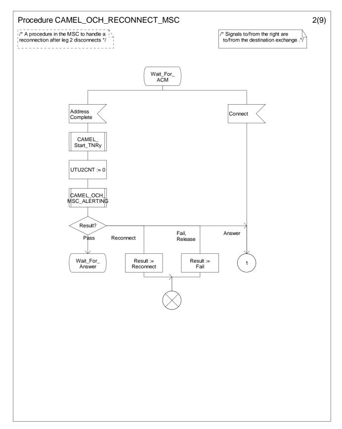
Figure 4.33-2: Procedure CAMEL\_OCH\_RECONNECT\_MSC (sheet 2)
