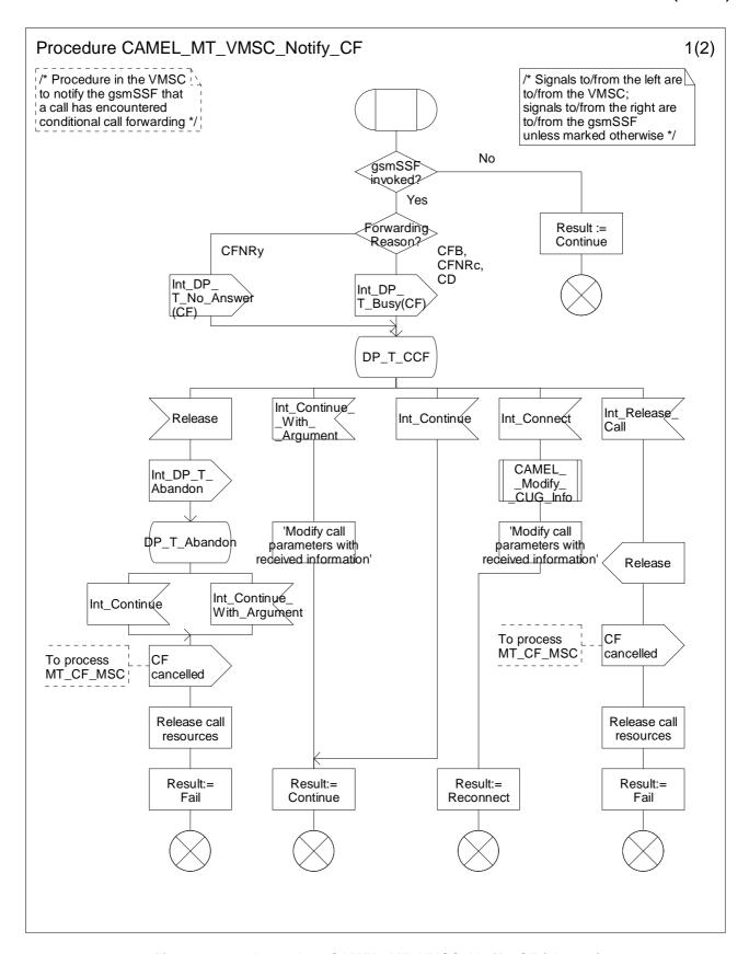
Figure 4.70-1: Procedure CAMEL\_MT\_VMSC\_Notify\_CF (sheet 1)
