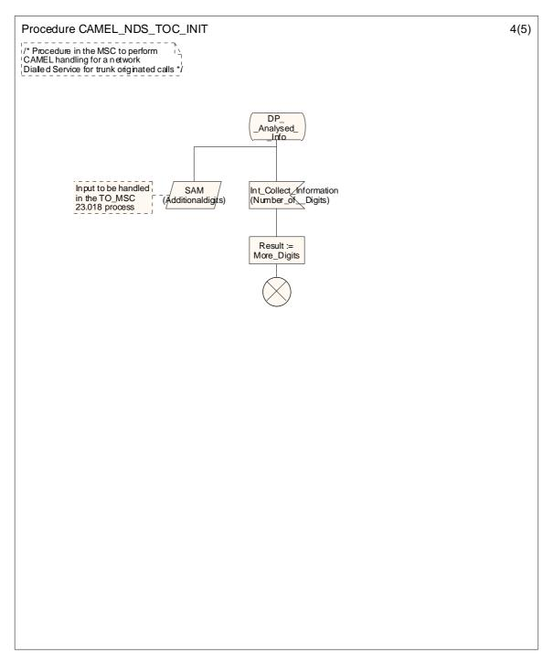
Figure 4.119C-4: Procedure CAMEL\_NDS\_TOC\_INIT (sheet 4)
