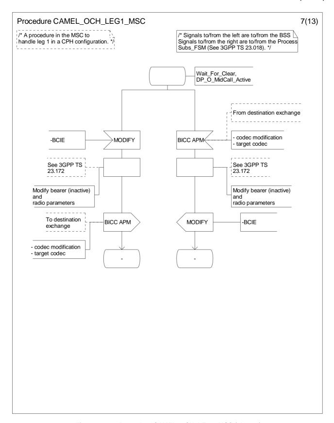
Figure 4.30-7: Procedure CAMEL\_OCH\_LEG1\_MSC (sheet 7)
