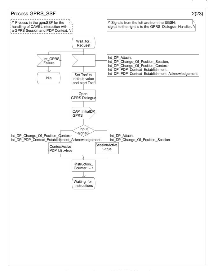
Figure 6.17-2: Process GPRS\_SSF (sheet 2)
