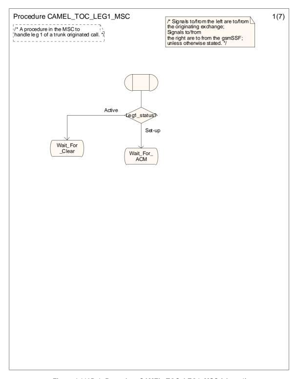
Figure 4.119D-1: Procedure CAMEL\_TOC\_LEG1\_MSC (sheet 1)
