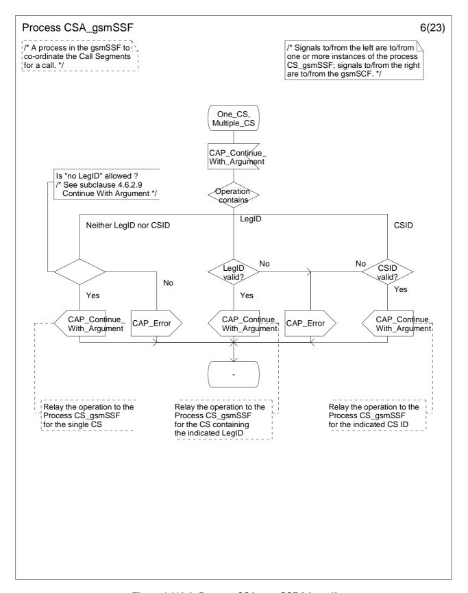
Figure 4.116-6: Process CSA\_gsmSSF (sheet 6)
