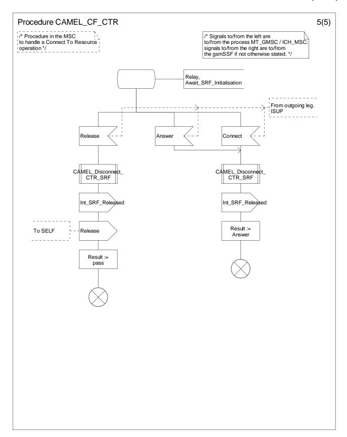
Figure 4.85-5: Procedure CAMEL\_CF\_CTR (sheet 5)
