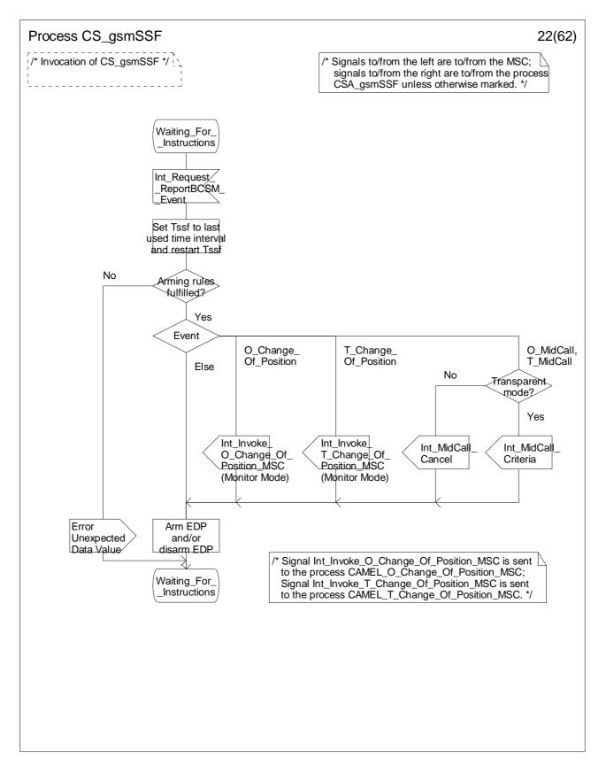
Figure 4.99-22: Process CS\_gsmSSF (sheet 22)
