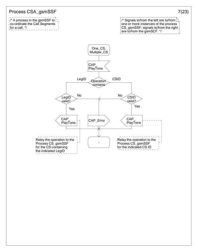
Figure 4.116-7: Process CSA\_gsmSSF (sheet 7)
