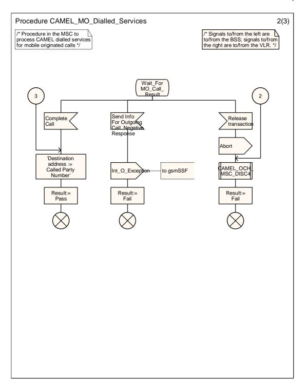
Figure 4.11-2: Procedure CAMEL\_MO\_Dialled\_Services (sheet 2)
