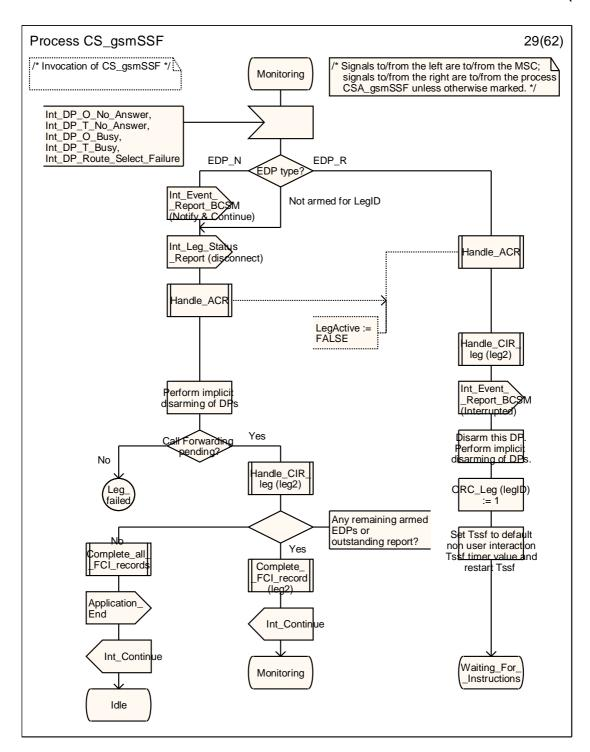
Figure 4.99-29: Process CS\_gsmSSF (sheet 29)
