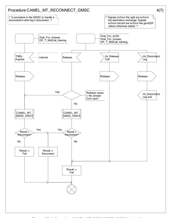
Figure 4.56-4: Procedure CAMEL\_MT\_RECONNECT\_GMSC (sheet 4)
