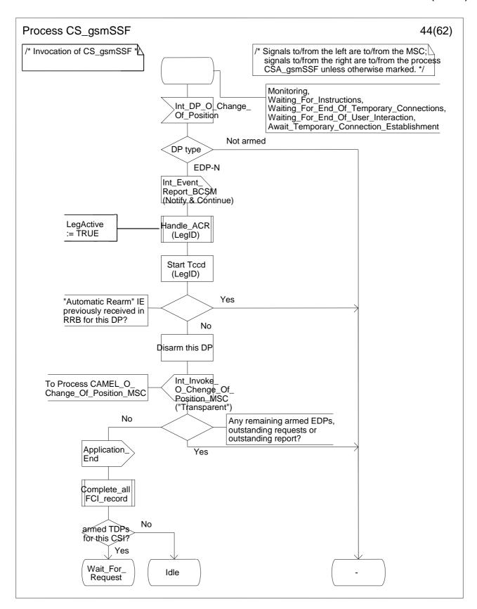
Figure 4.99-44: Process CS\_gsmSSF (sheet 44)
