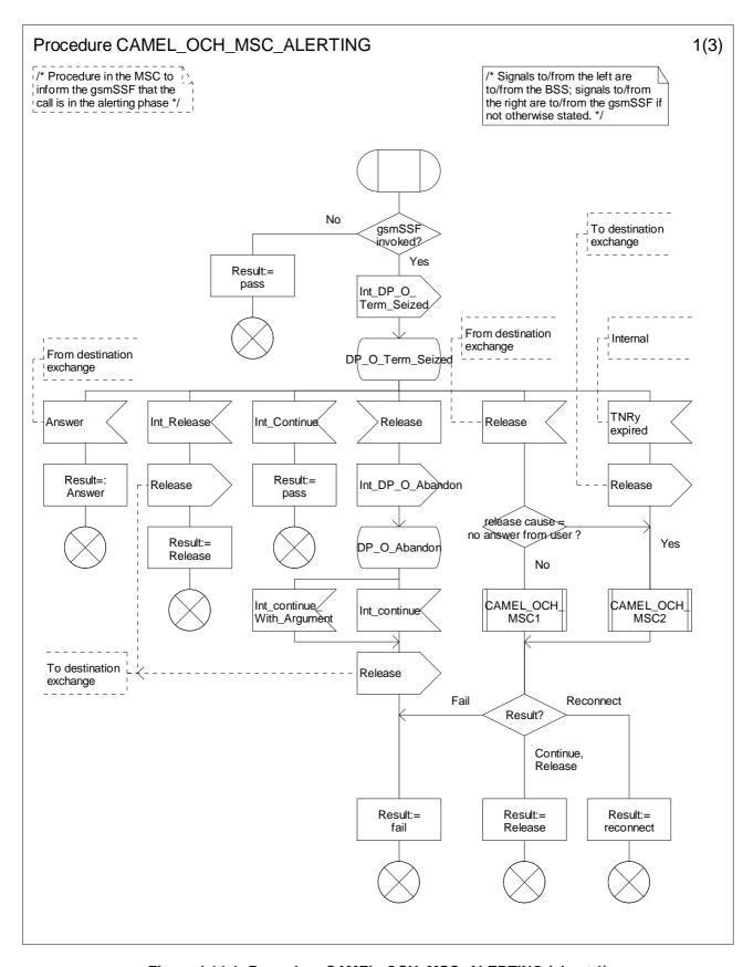
Figure 4.14-1: Procedure CAMEL\_OCH\_MSC\_ALERTING (sheet 1)
