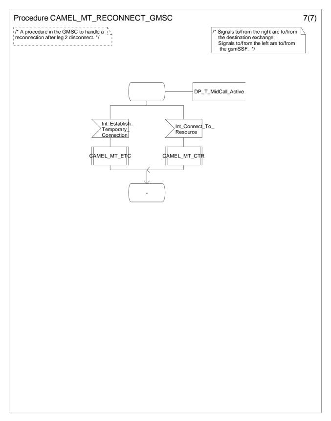
Figure 4.56-7: Procedure CAMEL\_MT\_RECONNECT\_GMSC (sheet 7)
