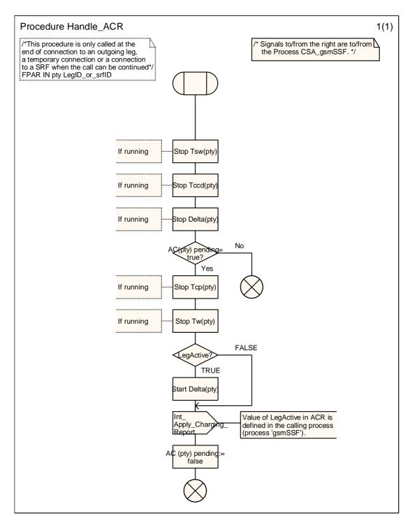
Figure 4.105-1: Procedure Handle\_ACR (sheet 1)
