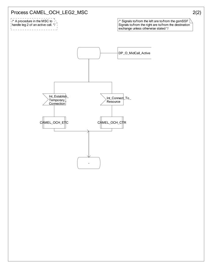
Figure 4.32-2: Process CAMEL\_OCH\_LEG2\_MSC (sheet 2)
