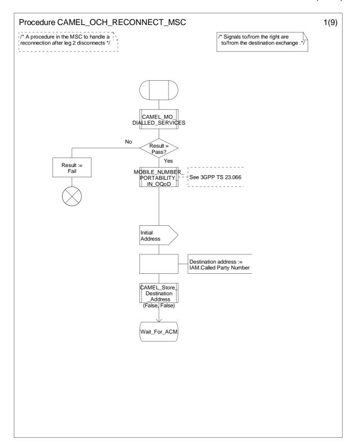
Figure 4.33-1: Procedure CAMEL\_OCH\_RECONNECT\_MSC (sheet 1)
