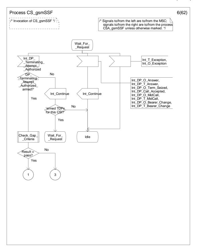
Figure 4.99-6: Process CS\_gsmSSF (sheet 6)
