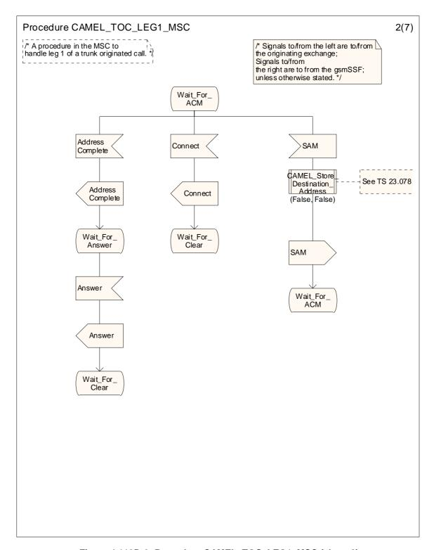
Figure 4.119D-2: Procedure CAMEL\_TOC\_LEG1\_MSC (sheet 2)
