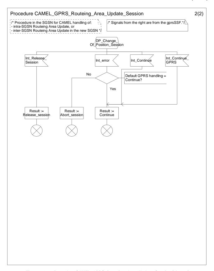
Figure 6.10-2: Procedure CAMEL\_GPRS\_Routeing\_Area\_Update\_Session (sheet 2)
