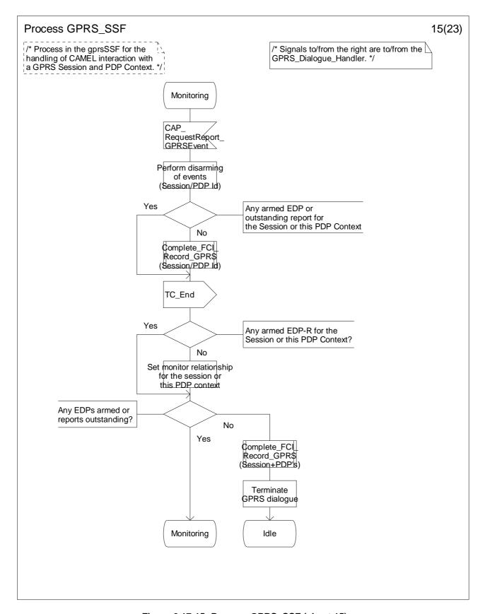
Figure 6.17-15: Process GPRS\_SSF (sheet 15)
