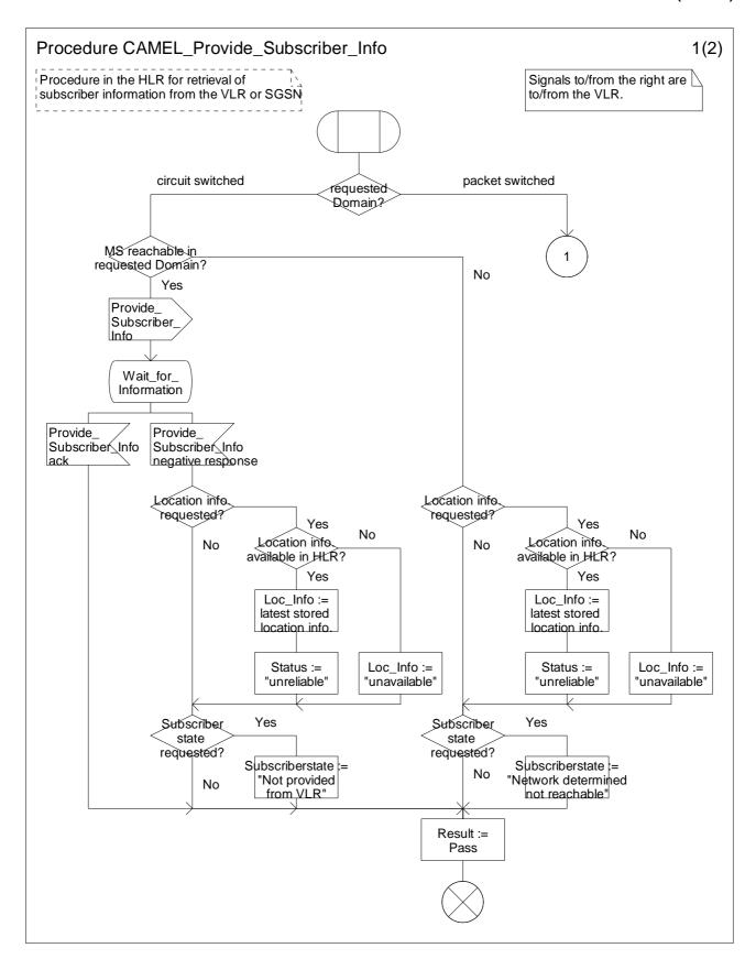
Figure 4.119-1: Procedure CAMEL\_Provide\_Subscriber\_Info (sheet 1)
