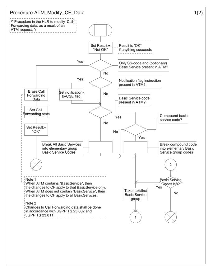
Figure 10.6-1: Procedure ATM\_Modify\_CF\_Data (sheet 1)
