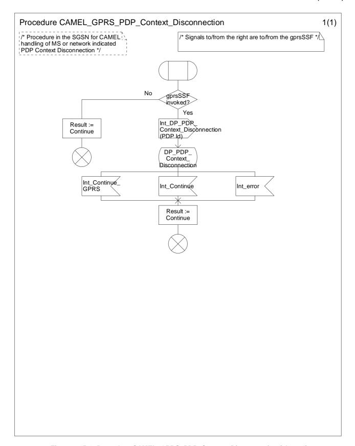
Figure 6.15-1: Procedure CAMEL\_GPRS\_PDP\_Context\_Disconnection (sheet 1)
