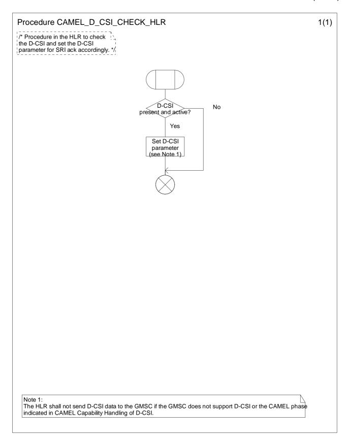
Figure 4.61-1: Procedure CAMEL\_D\_CSI\_CHECK\_HLR (sheet 1)
