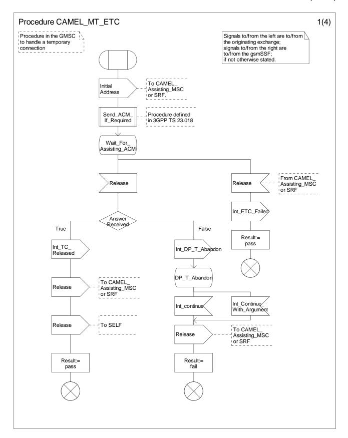
Figure 4.51-1: Procedure CAMEL\_MT\_ETC (sheet 1)
