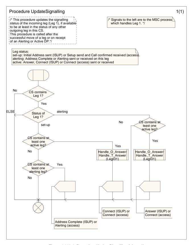
Figure 4.112-1: Procedure UpdateSignalling (sheet 1)
