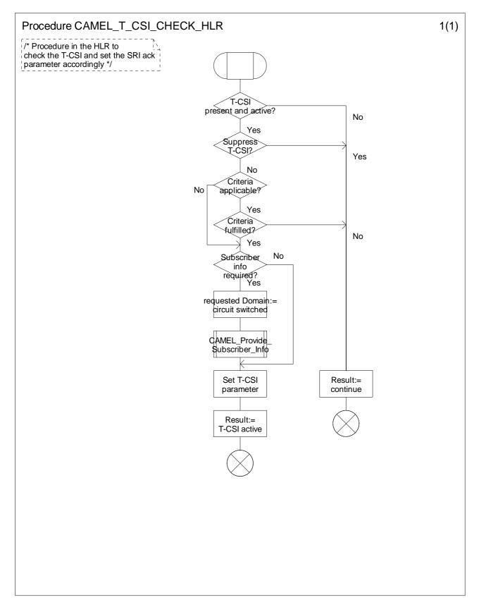
Figure 4.62-1: Procedure CAMEL\_T\_CSI\_CHECK\_HLR (sheet 1)
