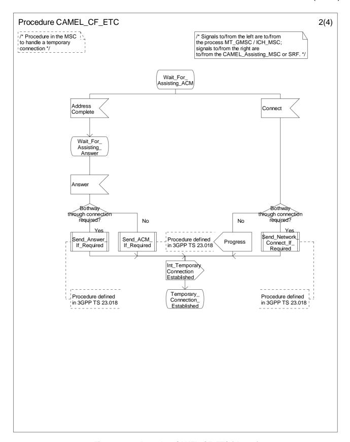
Figure 4.84-2: Procedure CAMEL\_CF\_ETC (sheet 2)
