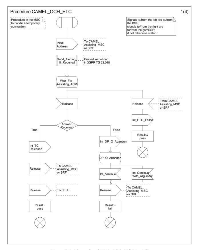
Figure 4.23-1: Procedure CAMEL\_OCH\_ETC (sheet 1)
