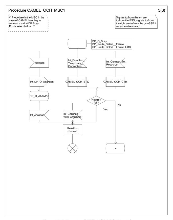
Figure 4.16-3: Procedure CAMEL\_OCH\_MSC1 (sheet 3)
