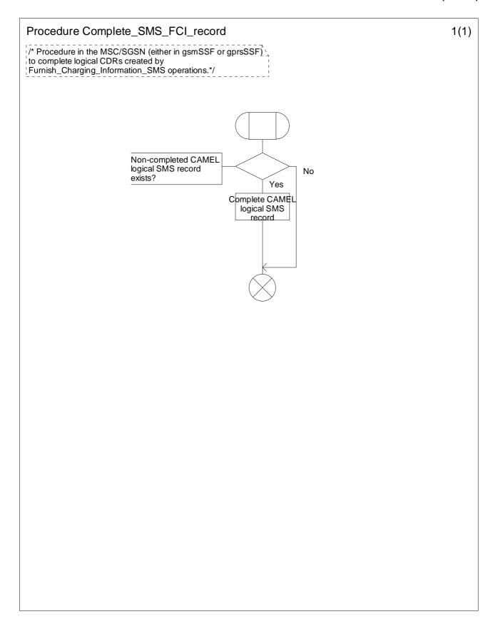
Figure 7.17-1: Procedure Complete\_SMS\_FCI\_record (sheet 1)
