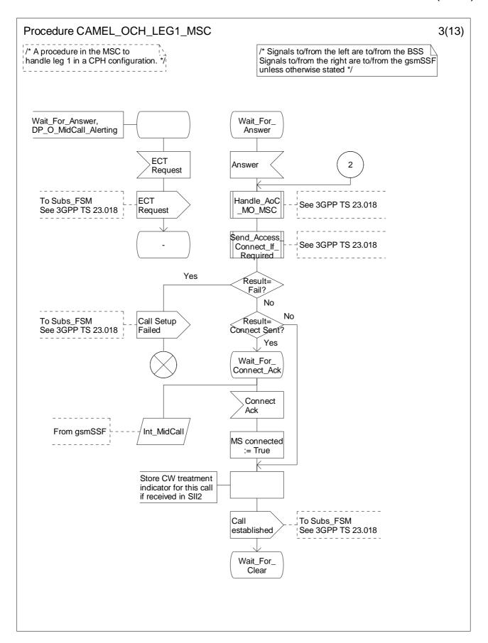
Figure 4.30-3: Procedure CAMEL\_OCH\_LEG1\_MSC (sheet 3)
