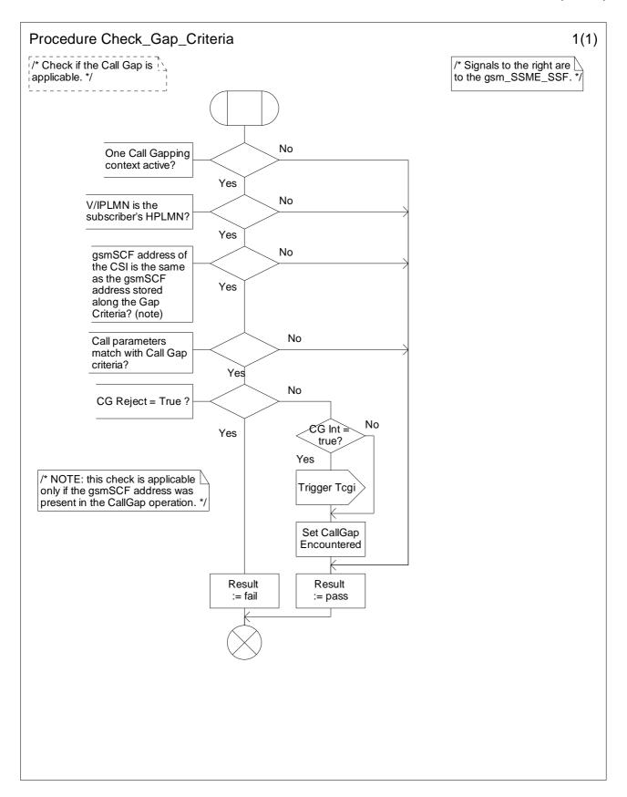
Figure 4.115-1: Procedure Check\_Gap\_Criteria (sheet 1)
