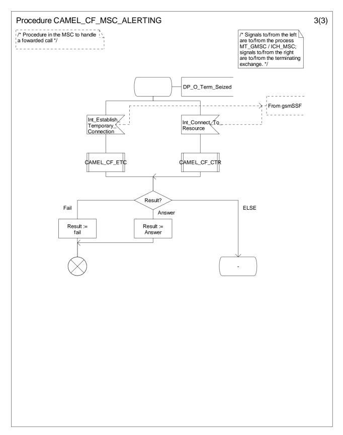
Figure 4.82-3: Procedure CAMEL\_CF\_MSC\_ALERTING (sheet 3)
