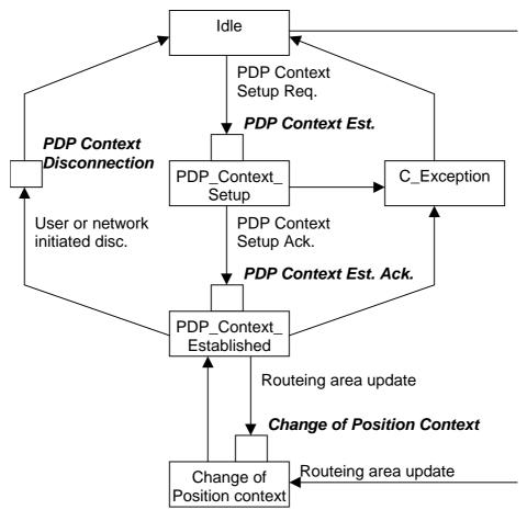
Figure 6.4: GPRS PDP Context State Model
