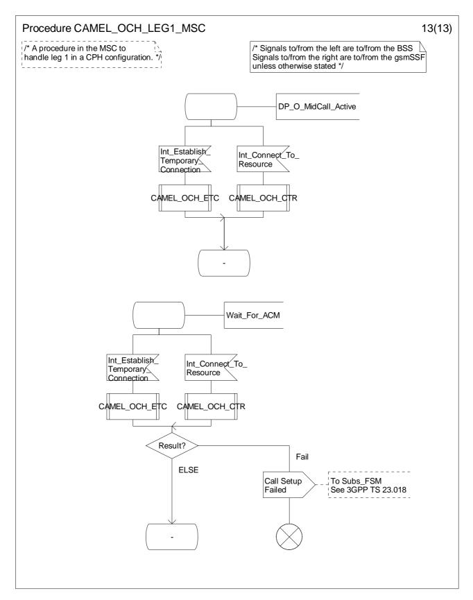
Figure 4.30-13: Procedure CAMEL\_OCH\_LEG1\_MSC (sheet 13)
