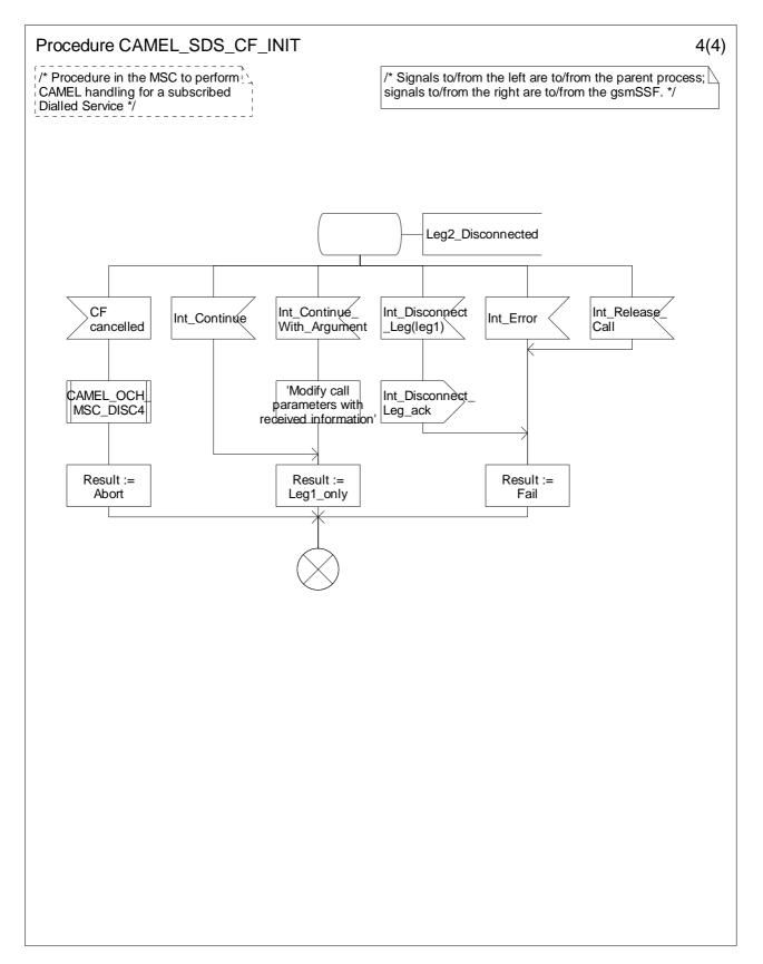
Figure 4.81-4: Procedure CAMEL\_NDS\_CF\_INIT (sheet 4)
