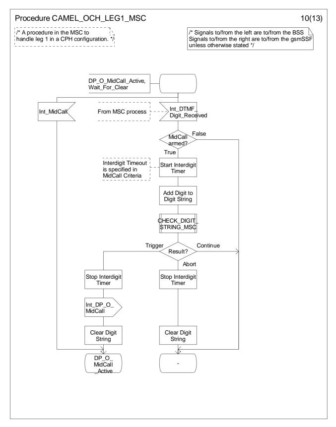
Figure 4.30-10: Procedure CAMEL\_OCH\_LEG1\_MSC (sheet 10)
