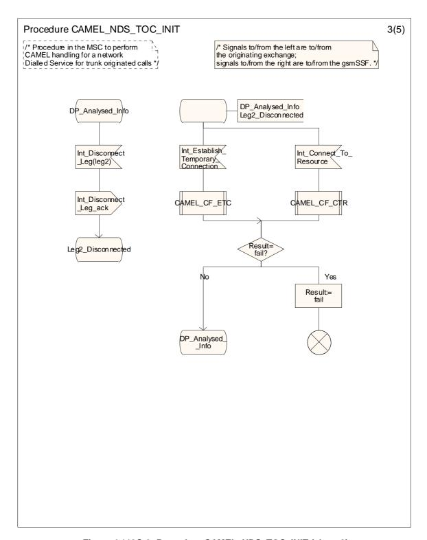
Figure 4.119C-3: Procedure CAMEL\_NDS\_TOC\_INIT (sheet 3)
