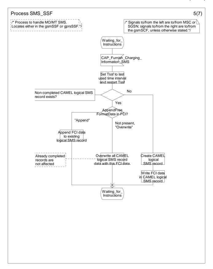
Figure 7.15-5: Process SMS\_SSF (sheet 5)
