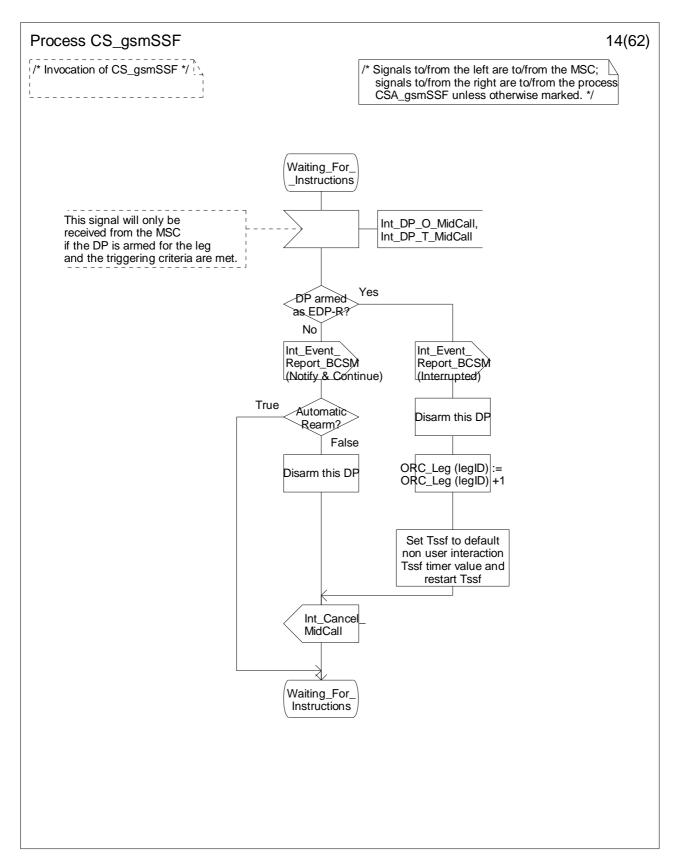
Figure 4.99-14: Process CS\_gsmSSF (sheet 14)
