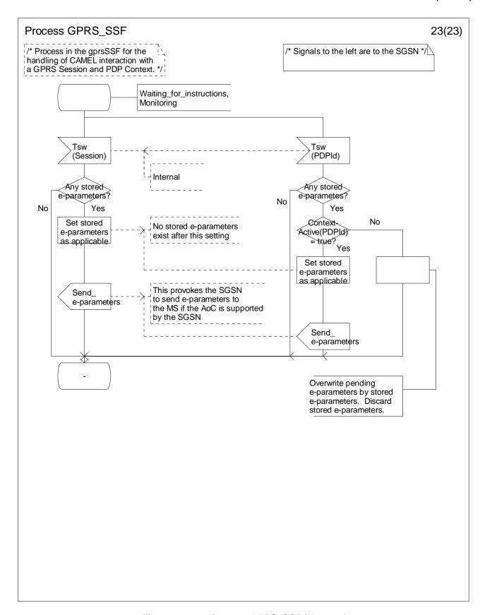
Figure 6.17-23: Process GPRS\_SSF (sheet 23)
