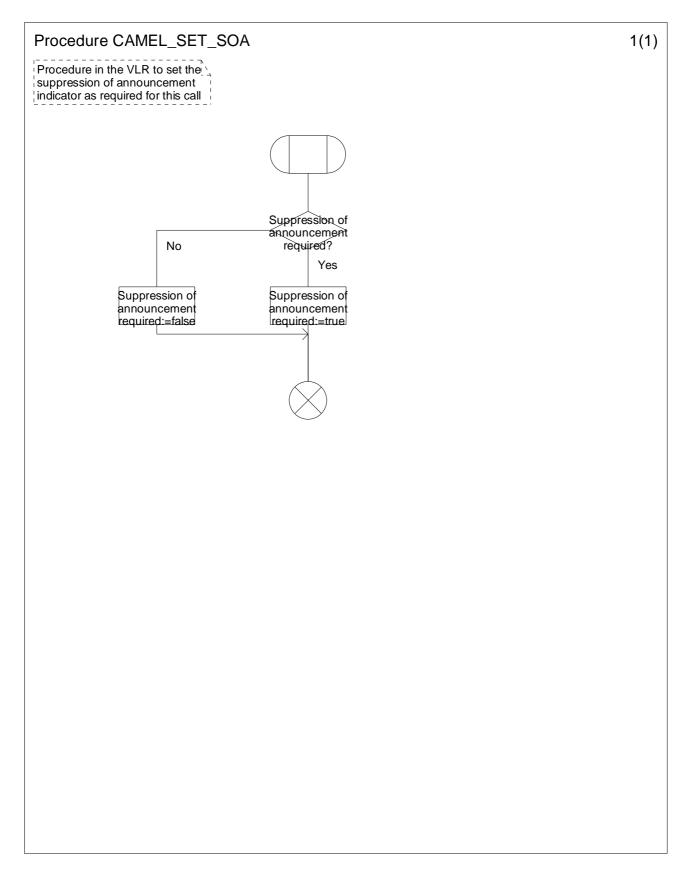
Figure 4.64-1: Procedure CAMEL\_SET\_SOA (sheet 1)
