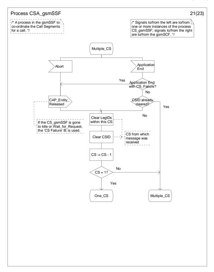
Figure 4.116-21: Process CSA\_gsmSSF (sheet 21)
