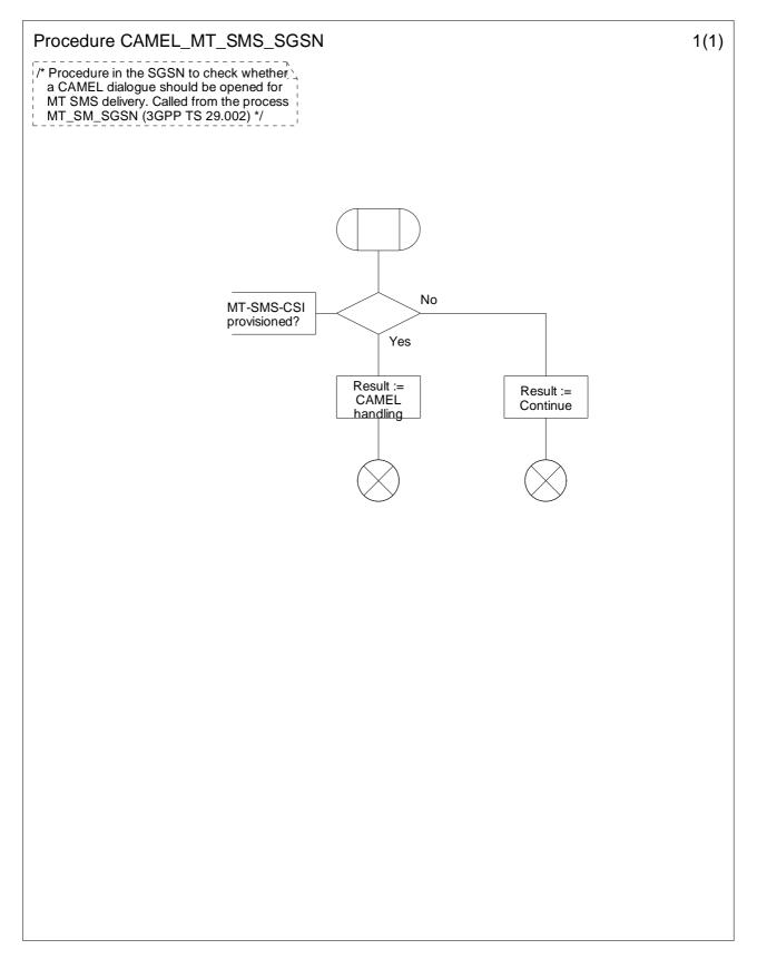
Figure 7.14-1: Procedure CAMEL\_MT\_SMS\_SGSN (sheet 1)
