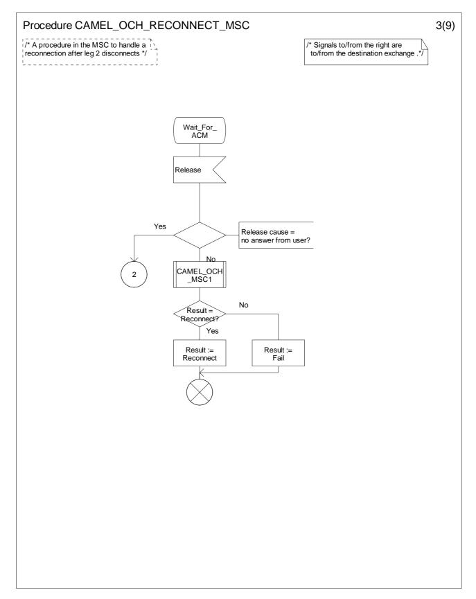
Figure 4.33-3: Procedure CAMEL\_OCH\_RECONNECT\_MSC (sheet 3)
