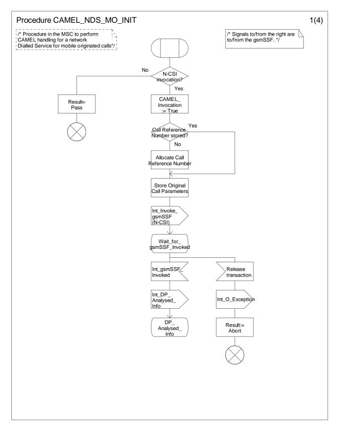
Figure 4.13-1: Procedure CAMEL\_NDS\_MO\_INIT (sheet 1)
