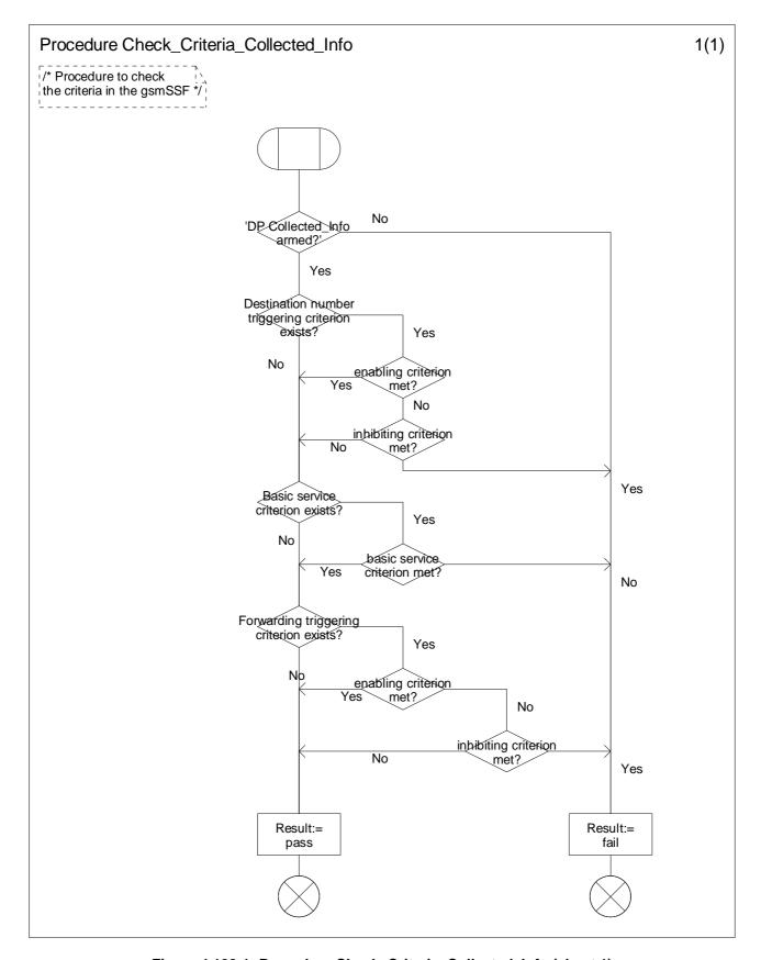
Figure 4.100-1: Procedure Check\_Criteria\_Collected\_Info (sheet 1)
