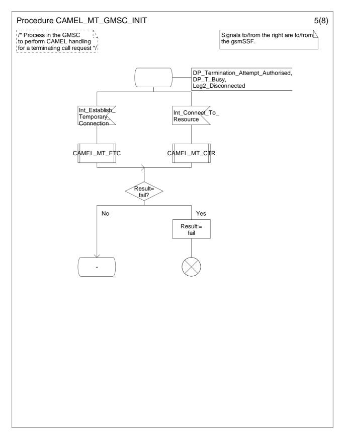
Figure 4.42-5: Procedure CAMEL\_MT\_GMSC\_INIT (sheet 5)
