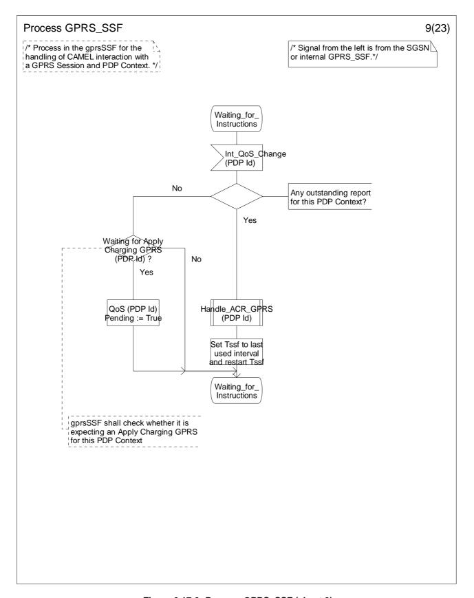
Figure 6.17-9: Process GPRS\_SSF (sheet 9)
