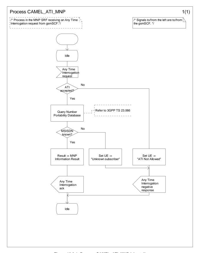
Figure 12.2-1: Process CAMEL\_ATI\_MNP (sheet 1)
