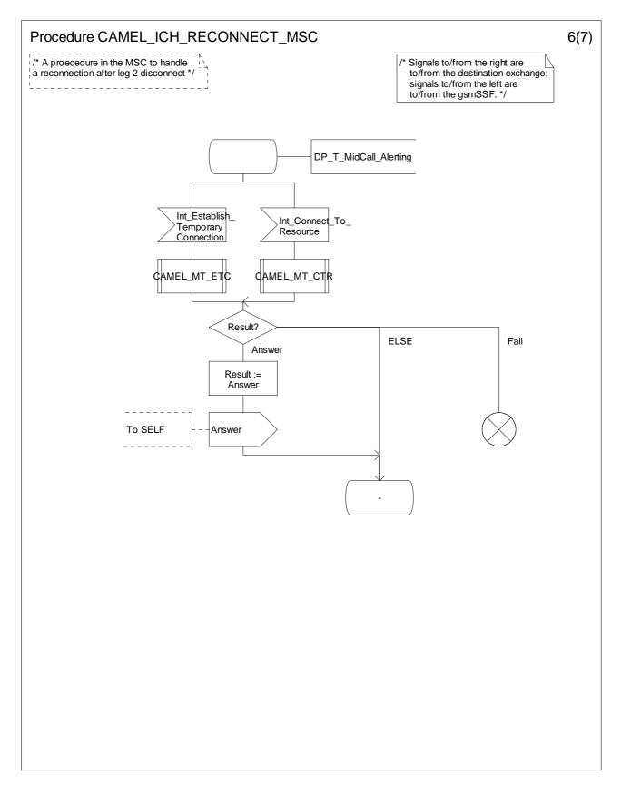
Figure 4.74-6: Procedure CAMEL\_ICH\_RECONNECT\_MSC (sheet 6)
