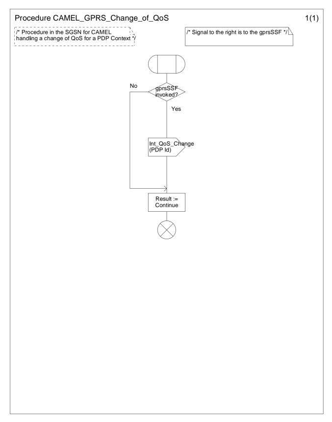
Figure 6.14-1: Procedure CAMEL\_GPRS\_Change\_Of\_QoS (sheet 1)
