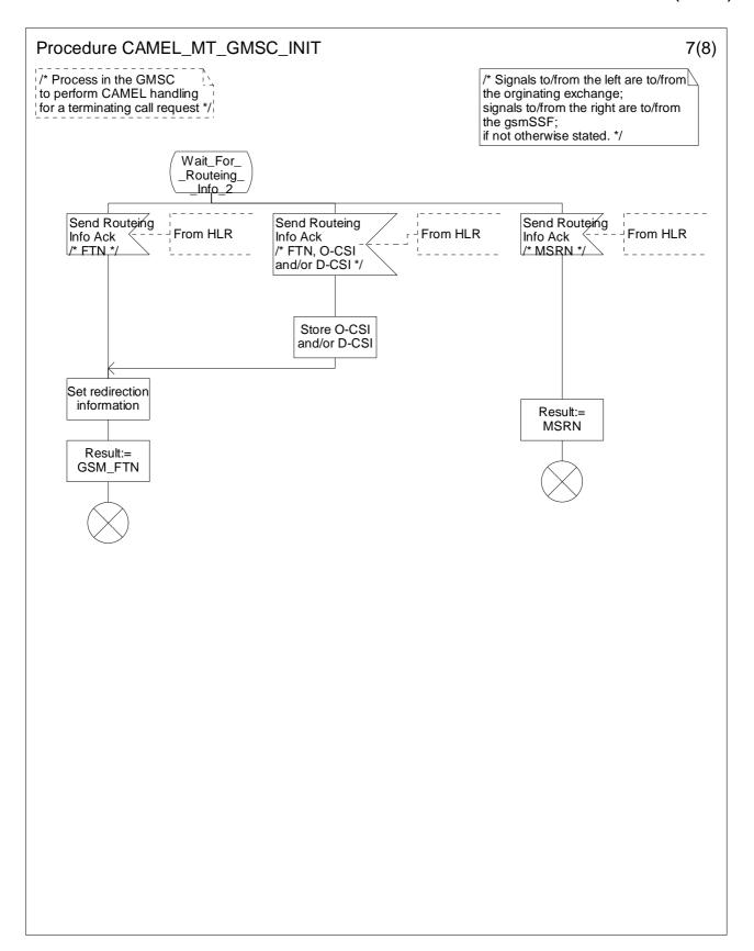
Figure 4.42-7: Procedure CAMEL\_MT\_GMSC\_INIT (sheet 7)
