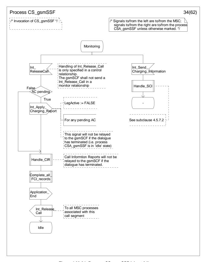
Figure 4.99-34: Process CS\_gsmSSF (sheet 34)
