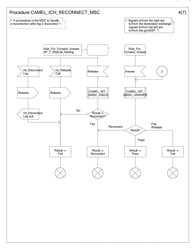
Figure 4.74-4: Procedure CAMEL\_ICH\_RECONNECT\_MSC (sheet 4)
