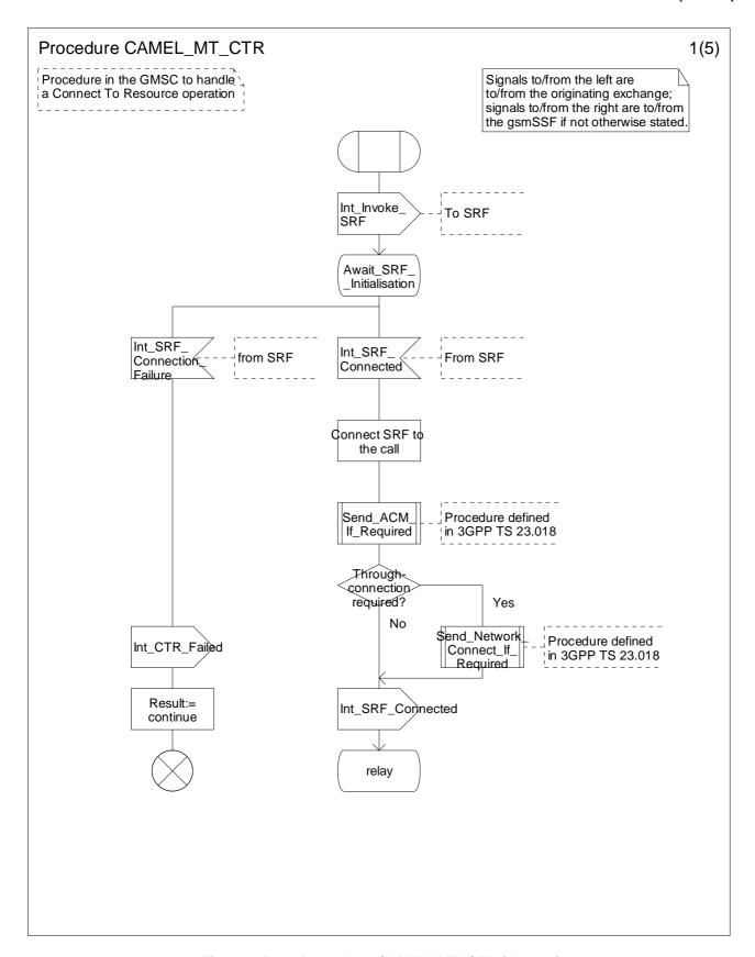
Figure 4.52-1: Procedure CAMEL\_MT\_CTR (sheet 1)
