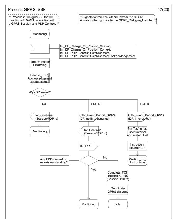
Figure 6.17-17: Process GPRS\_SSF (sheet 17)
