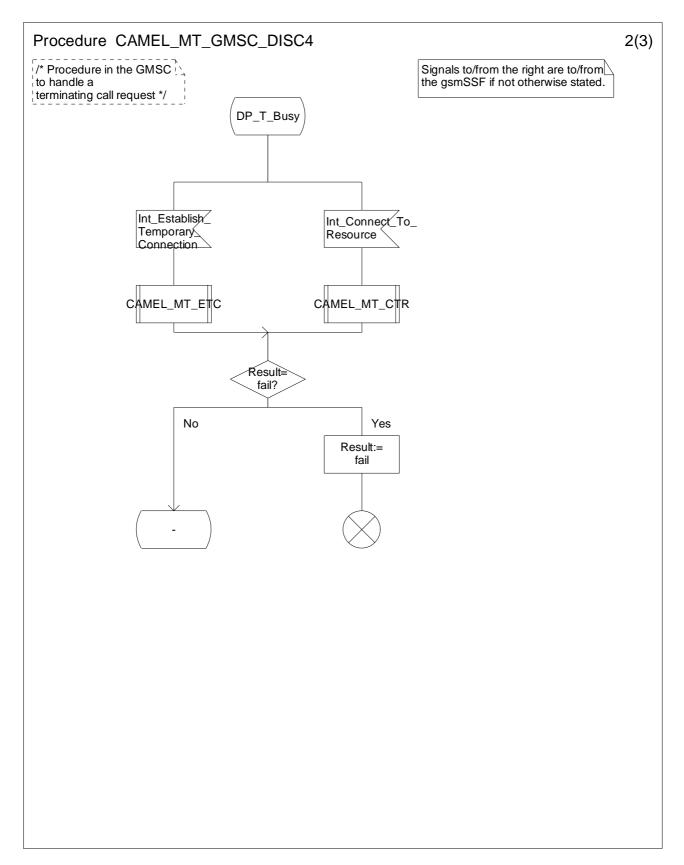
Figure 4.48-2: Procedure CAMEL\_MT\_GMSC\_DISC4 (sheet 2)
