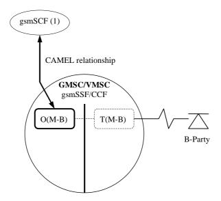
Figure 4.8: BCSM Scenario for gsmSCF Initiated New Call
