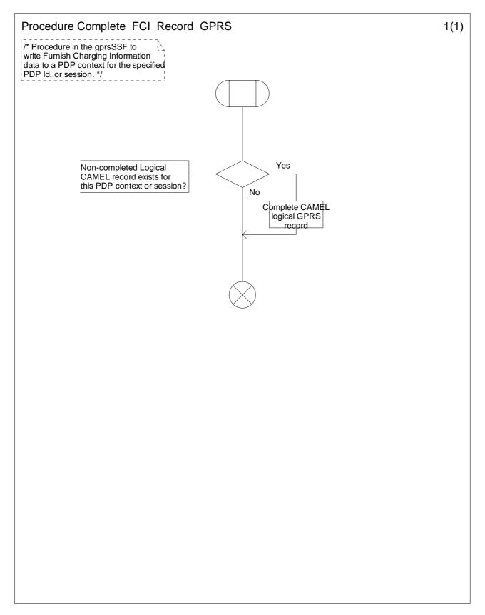
Figure 6.22-1: Procedure Complete\_FCI\_Record\_GPRS (sheet 1)
