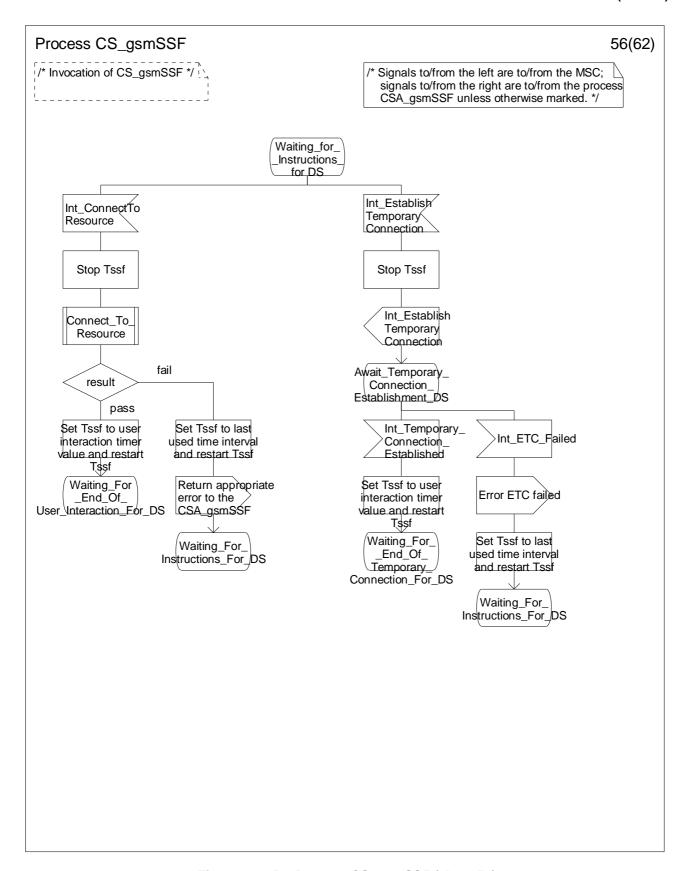
Figure 4.99-56: Process CS\_gsmSSF (sheet 56)
