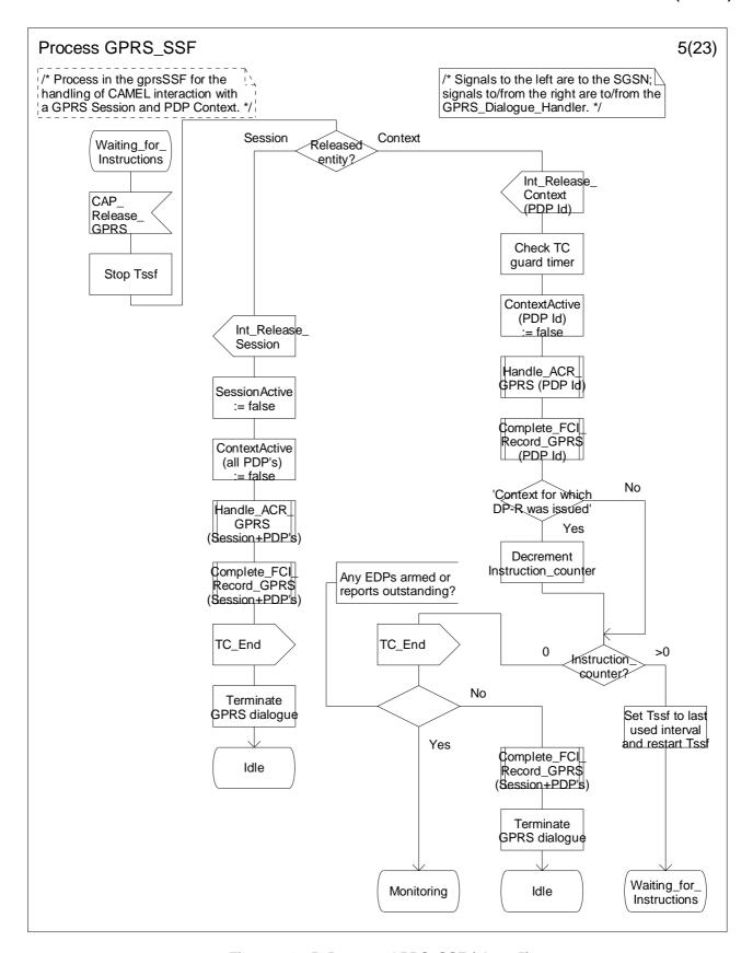
Figure 6.17-5: Process GPRS\_SSF (sheet 5)
