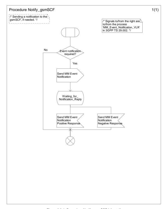
Figure 9.3-1: Procedure Notify\_gsmSCF (sheet 1)
