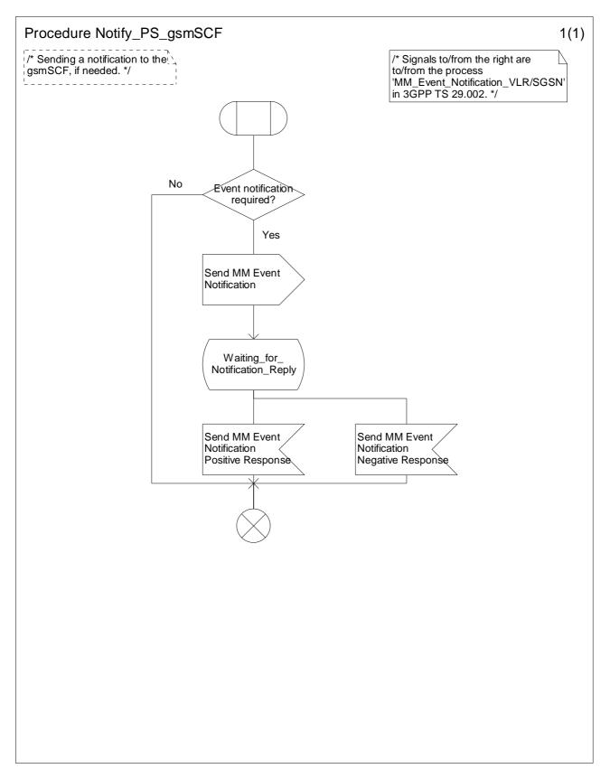
Figure 9.7-1: Procedure Notify\_PS\_gsmSCF (sheet 1)
