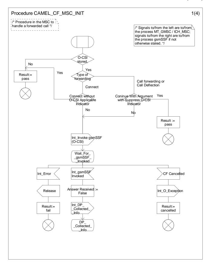
Figure 4.79-1: Procedure CAMEL\_CF\_MSC\_INIT (sheet 1)
