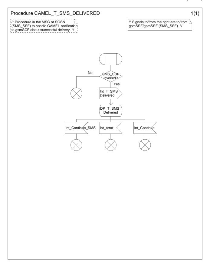
Figure 7.12-1: Procedure CAMEL\_T\_SMS\_DELIVERED (sheet 1)
