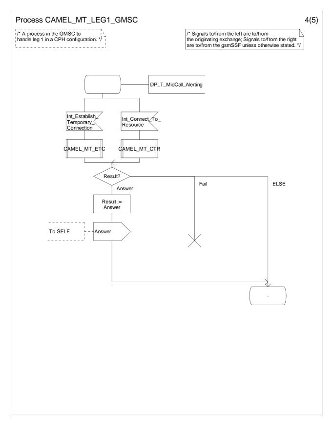
Figure 4.55-4: Process CAMEL\_MT\_LEG1\_GMSC (sheet 4)
