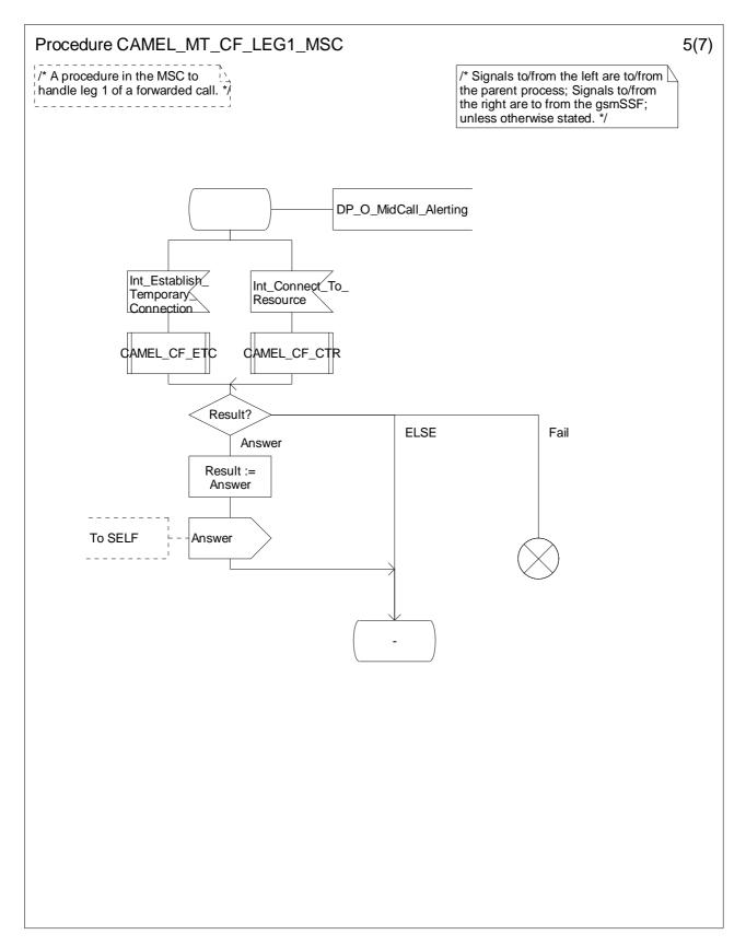
Figure 4.86-5: Procedure CAMEL\_MT\_CF\_LEG1\_MSC (sheet 5)
