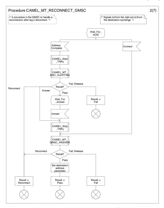
Figure 4.56-2: Procedure CAMEL\_MT\_RECONNECT\_GMSC (sheet 2)
