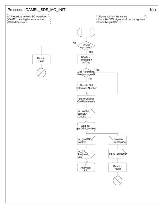
Figure 4.12-1: Procedure CAMEL\_SDS\_MO\_Init (sheet 1)
