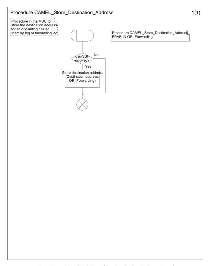
Figure 4.27-1: Procedure CAMEL\_Store\_Destination\_Address (sheet 1)
