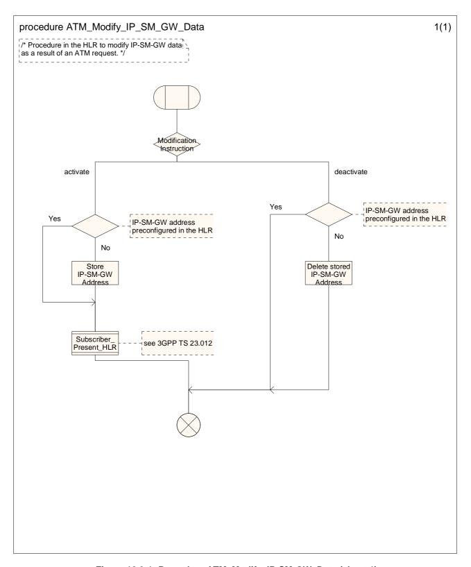
Figure 10.9-1: Procedure ATM\_Modify\_IP-SM-GW\_Data (sheet 1)
