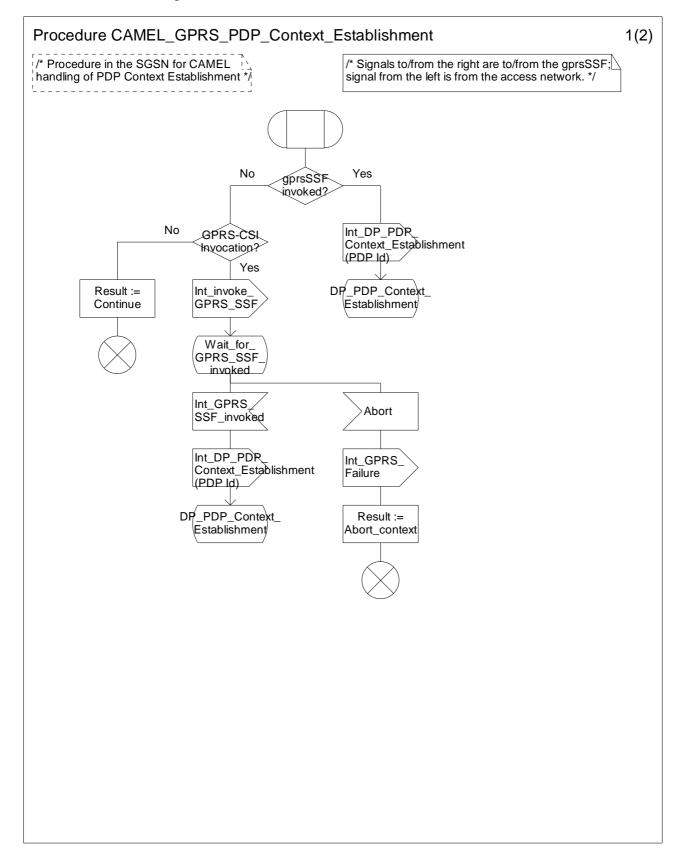
Figure 6.12-1: Procedure CAMEL\_GPRS\_PDP\_Context\_Establishment (sheet 1)
