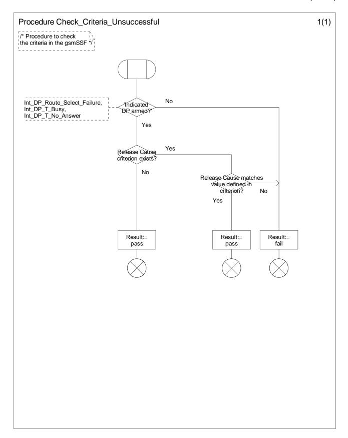
Figure 4.102-1: Procedure Check\_Criteria\_Unsuccessful (sheet 1)
