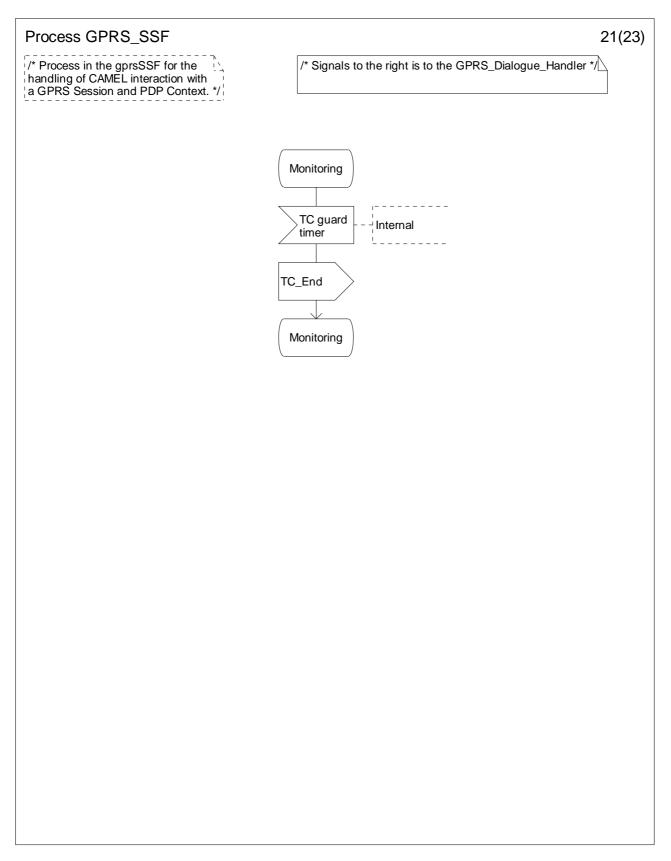
Figure 6.17-21: Process GPRS\_SSF (sheet 21)
