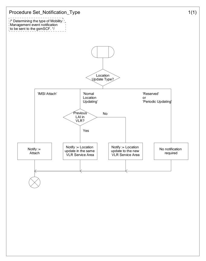
Figure 9.-1a: Procedure Set\_Notification\_Type (sheet 1)
