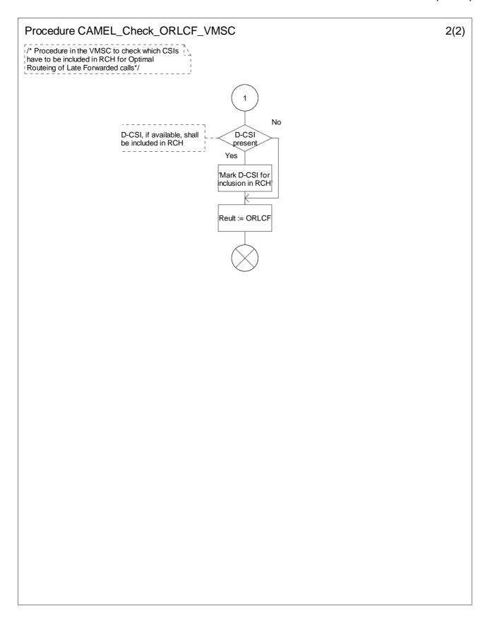
Figure 4.77-2: Procedure CAMEL\_Check\_ORLCF\_VMSC (sheet 2)
