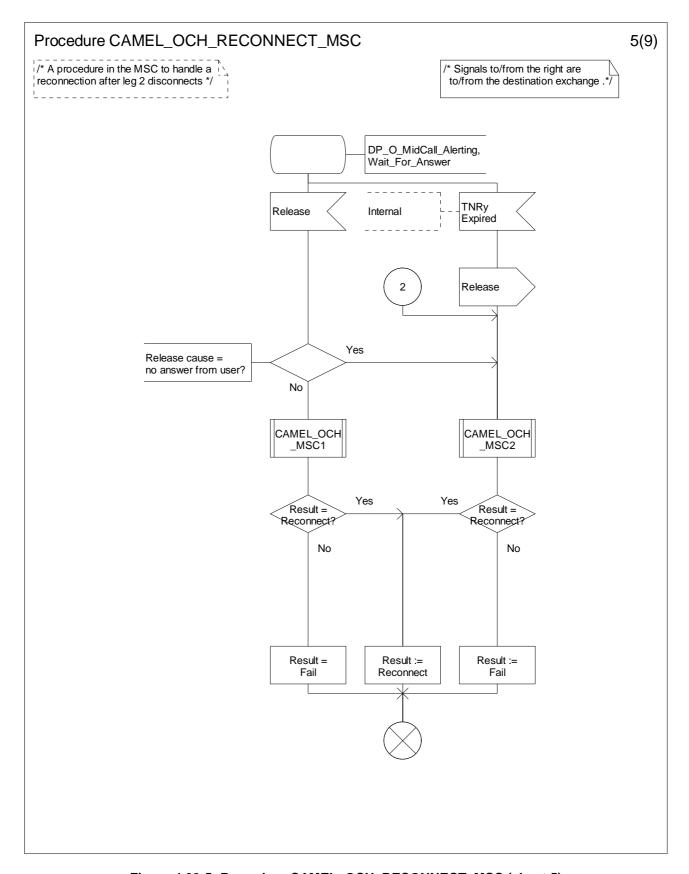
Figure 4.33-5: Procedure CAMEL\_OCH\_RECONNECT\_MSC (sheet 5)
