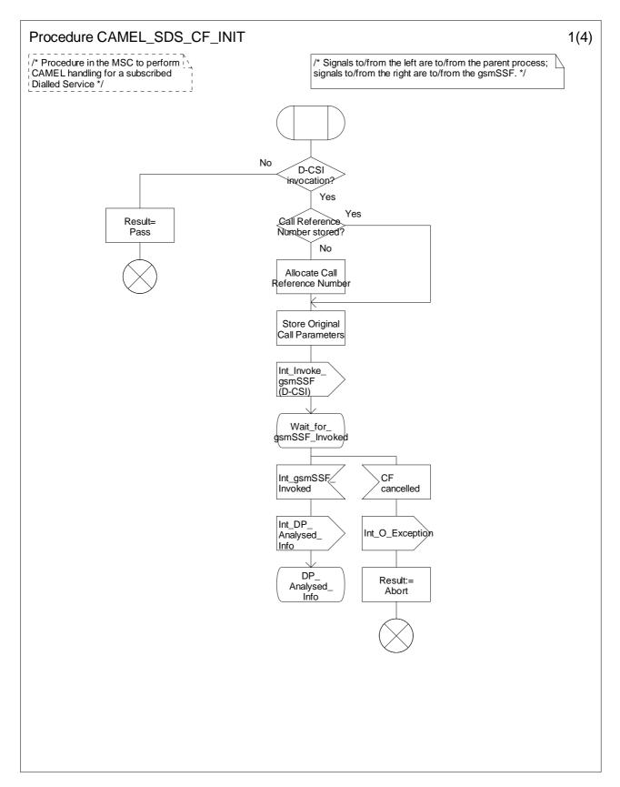
Figure 4.80-1: Procedure CAMEL\_SDS\_CF\_INIT (sheet 1)
