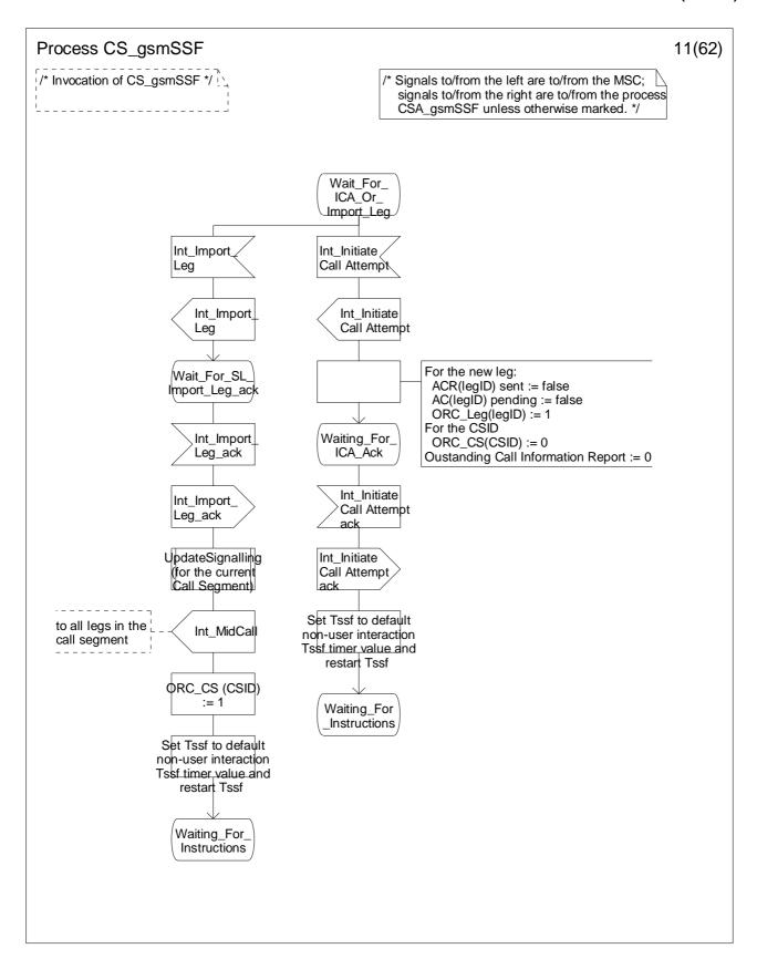
Figure 4.99-11: Process CS\_gsmSSF (sheet 11)
