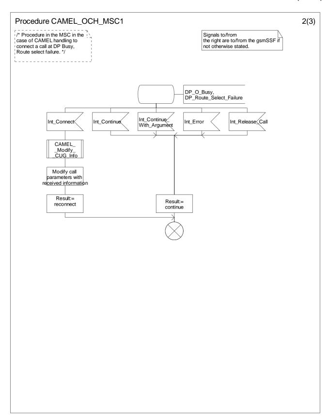
Figure 4.16-2: Procedure CAMEL\_OCH\_MSC1 (sheet 2)
