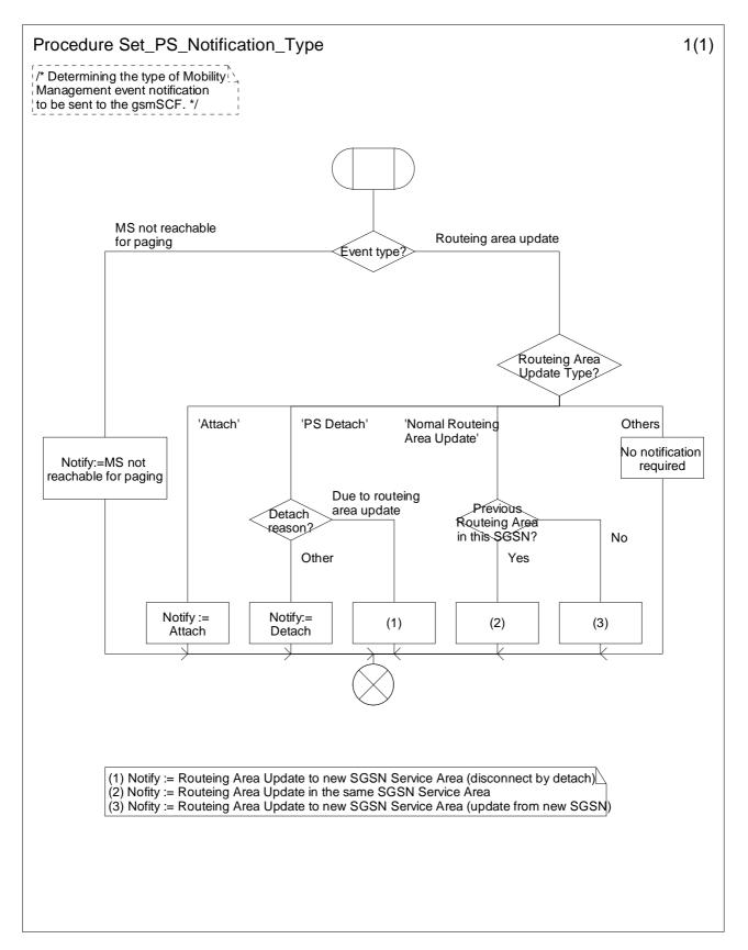
Figure 9.6-1: Procedure Set\_PS\_Notification\_Type (sheet 1)
