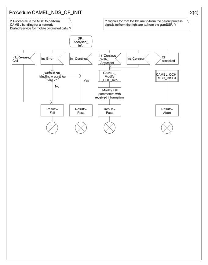
Figure 4.81-2: Procedure CAMEL\_NDS\_CF\_INIT (sheet 2)
