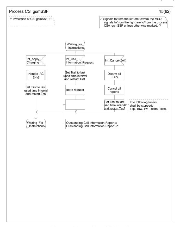
Figure 4.99-15: Process CS\_gsmSSF (sheet 15)
