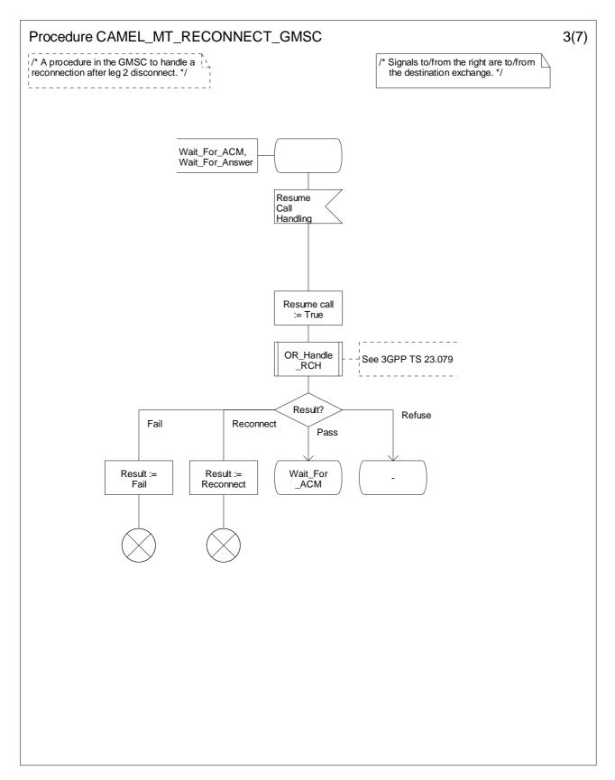
Figure 4.56-3: Procedure CAMEL\_MT\_RECONNECT\_GMSC (sheet 3)
