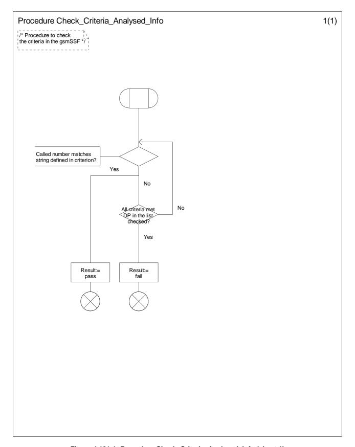
Figure 4.101-1: Procedure Check\_Criteria\_Analysed\_Info (sheet 1)
