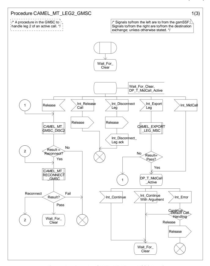
Figure 4.54-1: Procedure CAMEL\_MT\_LEG2\_GMSC (sheet 1)
