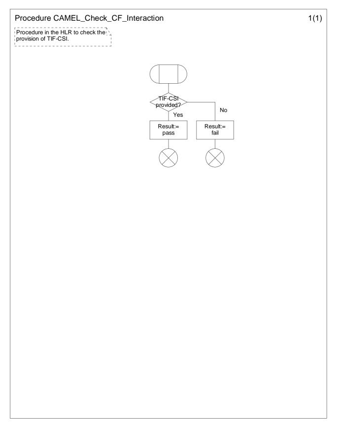
Figure 4.120-1: Procedure CAMEL\_Check\_CF\_Interaction (sheet 1)
