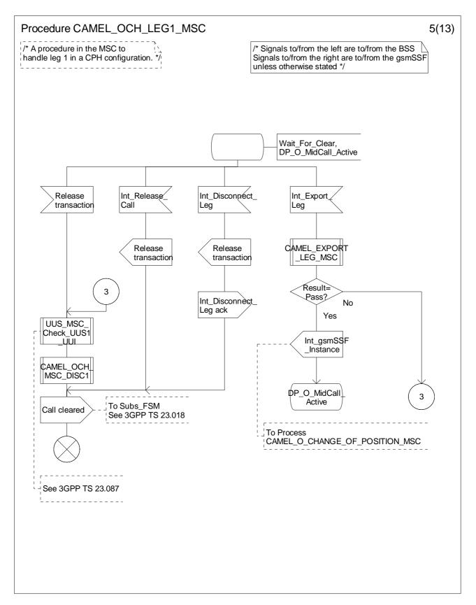
Figure 4.30-5: Procedure CAMEL\_OCH\_LEG1\_MSC (sheet 5)
