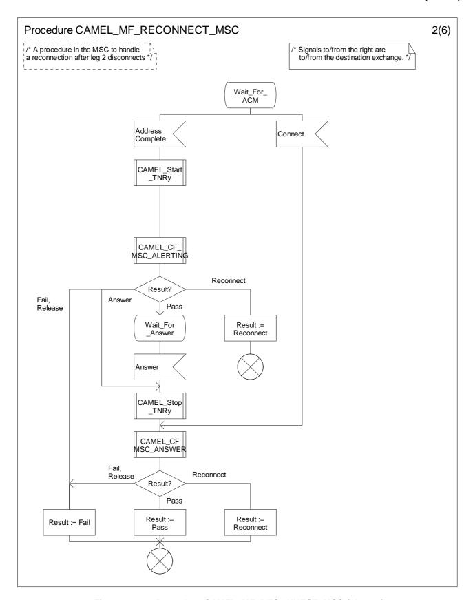
Figure 4.88-2: Procedure CAMEL\_MF\_RECONNECT\_MSC (sheet 2)
