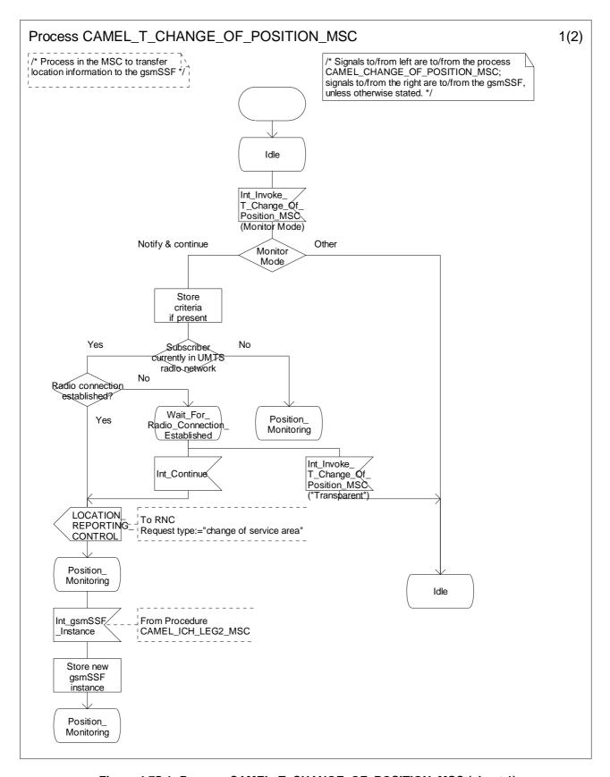
Figure 4.75-1: Process CAMEL\_T\_CHANGE\_OF\_POSITION\_MSC (sheet 1)
