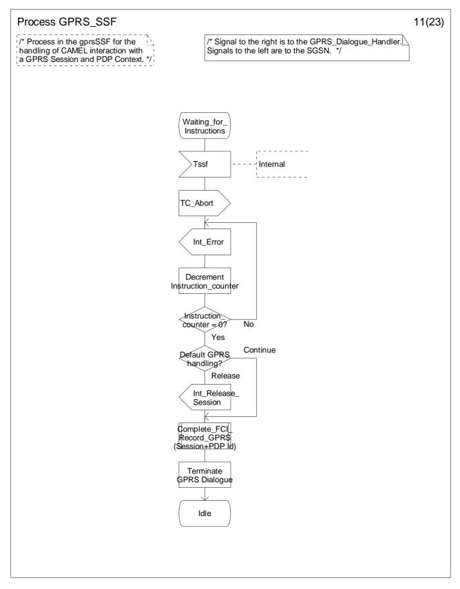
Figure 6.17-11: Process GPRS\_SSF (sheet 11)
