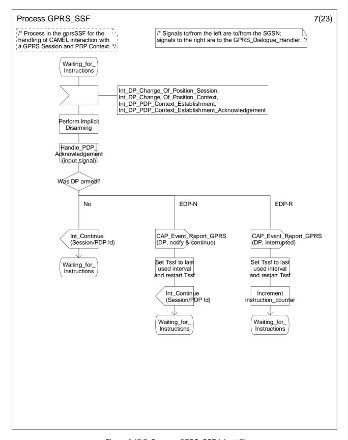
Figure 6.17-7: Process GPRS\_SSF (sheet 7)
