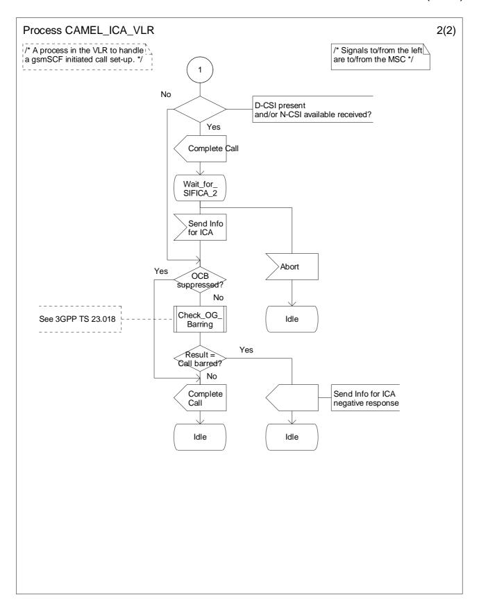
Figure 4.95-2: Process CAMEL\_ICA\_VLR (sheet 2)
