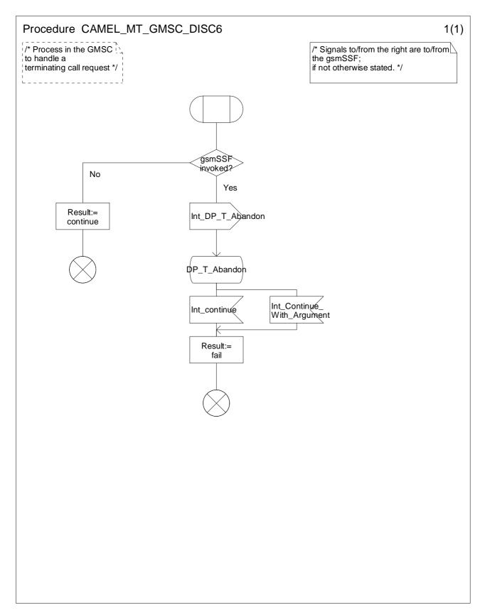
Figure 4.50-1: Procedure CAMEL\_MT\_GMSC\_DISC6 (sheet 1)
