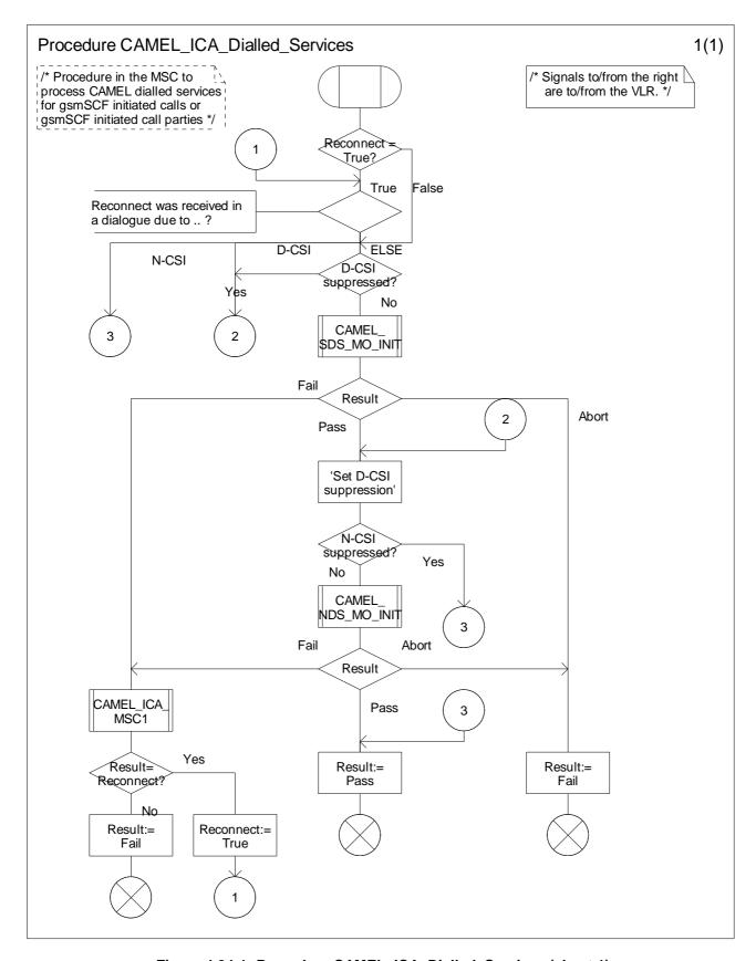
Figure 4.94-1: Procedure CAMEL\_ICA\_Dialled\_Services (sheet 1)
