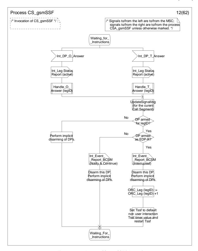
Figure 4.99-12: Process CS\_gsmSSF (sheet 12)
