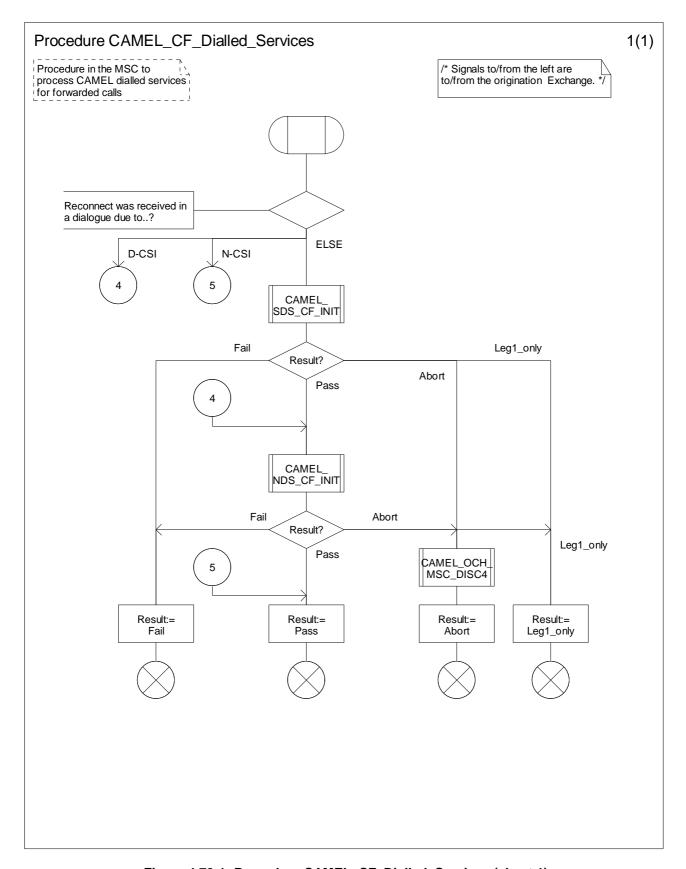
Figure 4.78-1: Procedure CAMEL\_CF\_Dialled\_Services (sheet 1)
