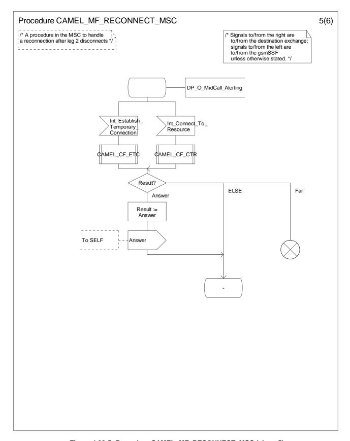
Figure 4.88-5: Procedure CAMEL\_MF\_RECONNECT\_MSC (sheet 5)
