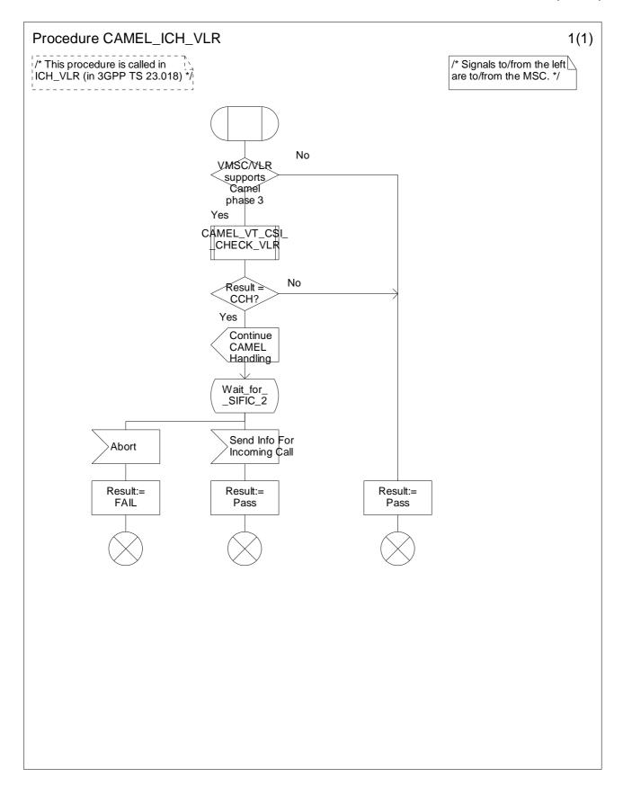
Figure 4.65-1: Procedure CAMEL\_ICH\_VLR (sheet 1)
