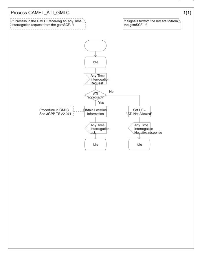
Figure 11.2-1: Process CAMEL\_ATI\_GMLC (sheet 1)
