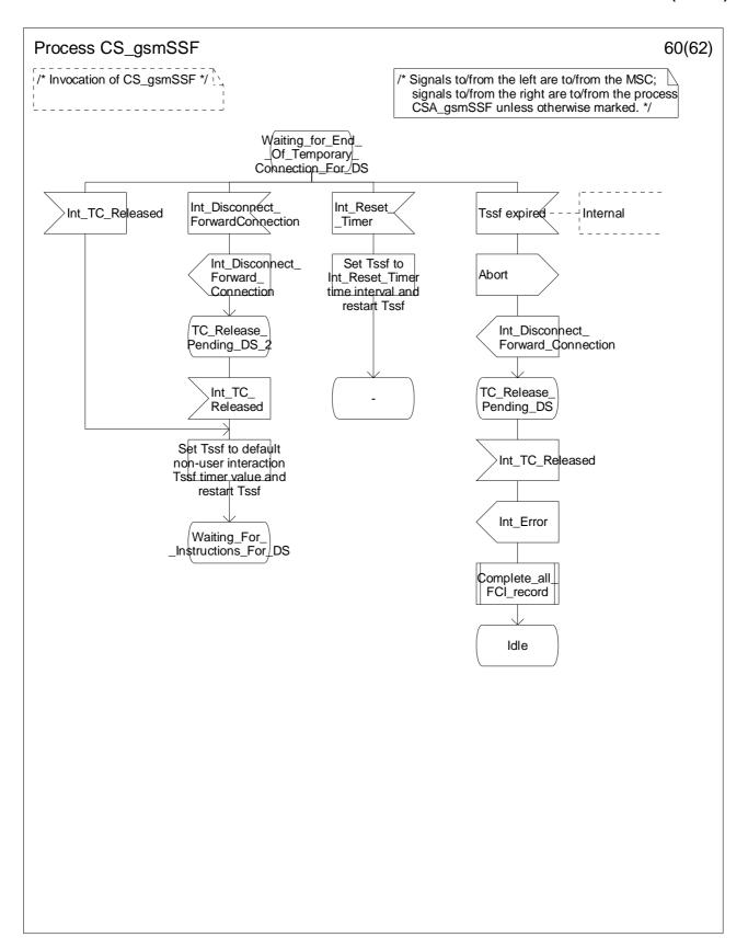
Figure 4.99-60: Process CS\_gsmSSF (sheet 60)
