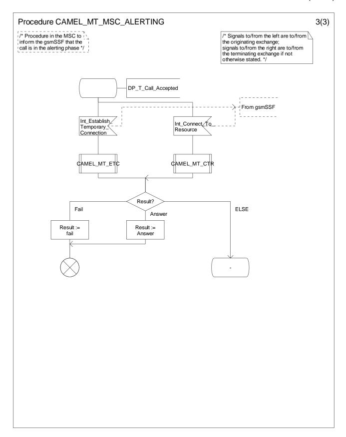
Figure 4.43-3: Procedure CAMEL\_MT\_MSC\_ALERTING (sheet 3)
