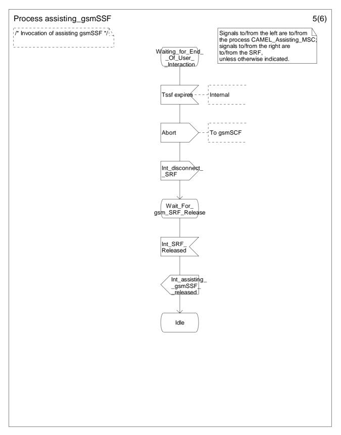
Figure 4.118-5: Process Assisting\_gsmSSF (sheet 5)
