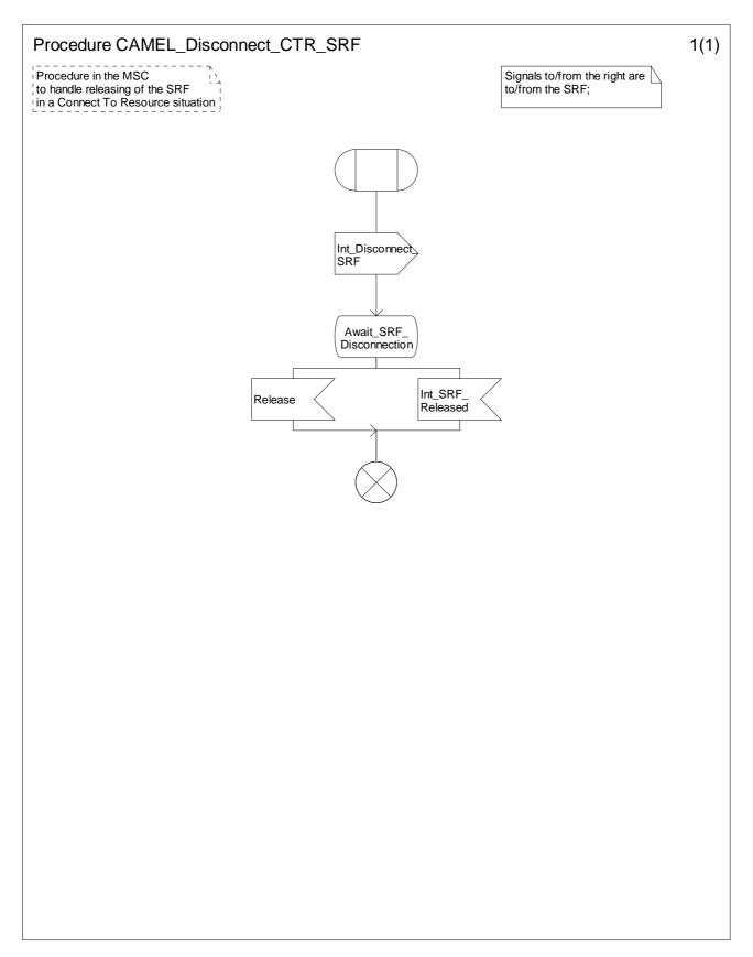
Figure 4.22-1: Procedure CAMEL\_Disconnect\_CTR\_SRF (sheet 1)
