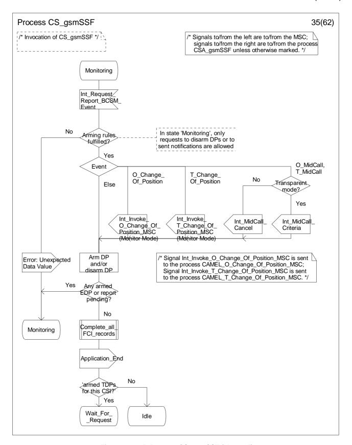
Figure 4.99-35: Process CS\_gsmSSF (sheet 35)
