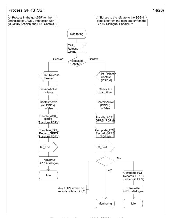
Figure 6.17-14: Process GPRS\_SSF (sheet 14)
