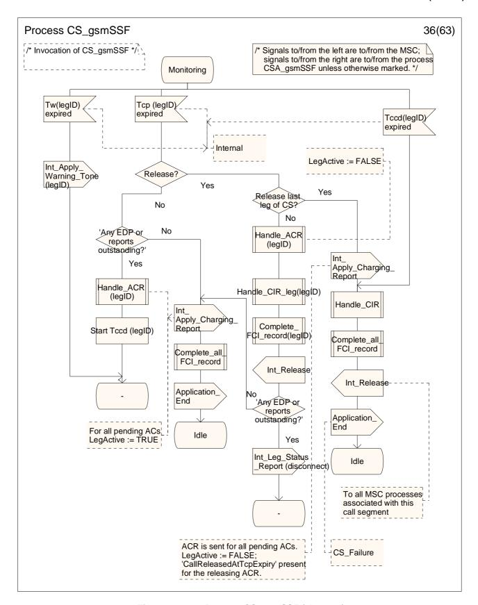
Figure 4.99-36: Process CS\_gsmSSF (sheet 36)
