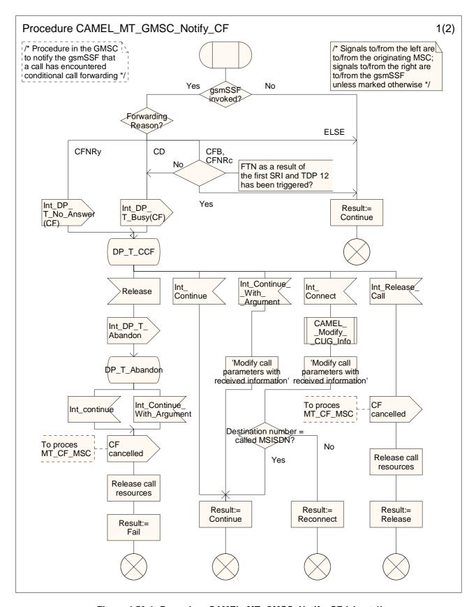
Figure 4.53-1: Procedure CAMEL\_MT\_GMSC\_Notify\_CF (sheet 1)
