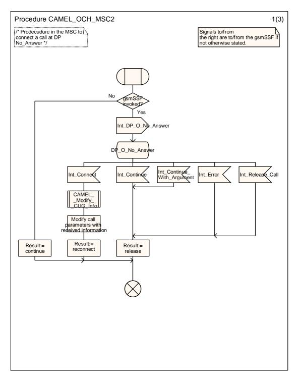
Figure 4.17-1: Procedure CAMEL\_OCH\_MSC2 (sheet 1)
