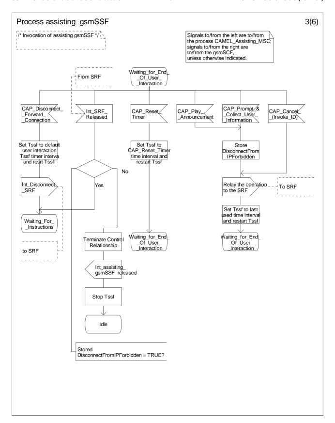
Figure 4.118-3: Process Assisting\_gsmSSF (sheet 3)
