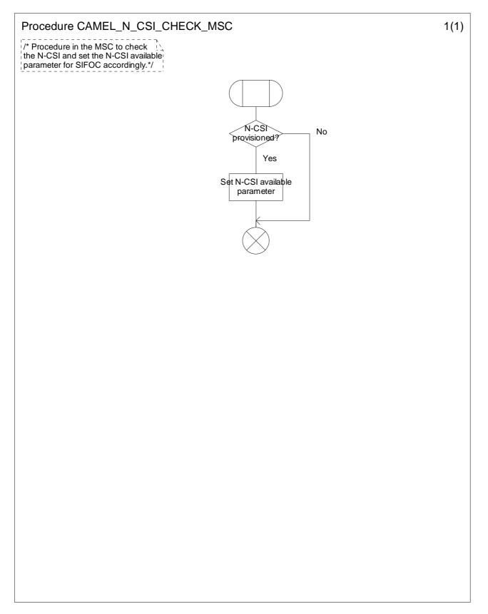
Figure 4.29-1: Procedure CAMEL\_N\_CSI\_CHECK\_MSC (sheet 1)
