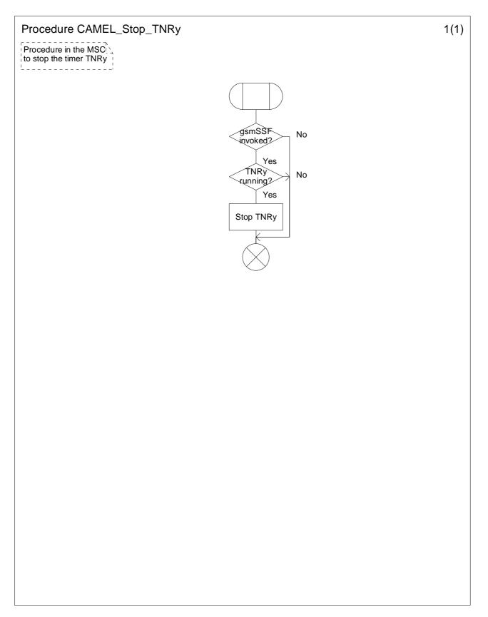
Figure 4.26-1: Procedure CAMEL\_Stop\_TNRy (sheet 1)
