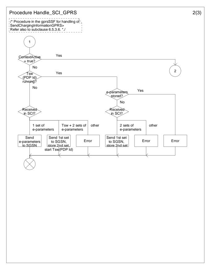
Figure 6.23-2: Procedure Handle\_SCI\_GPRS (sheet 2)
