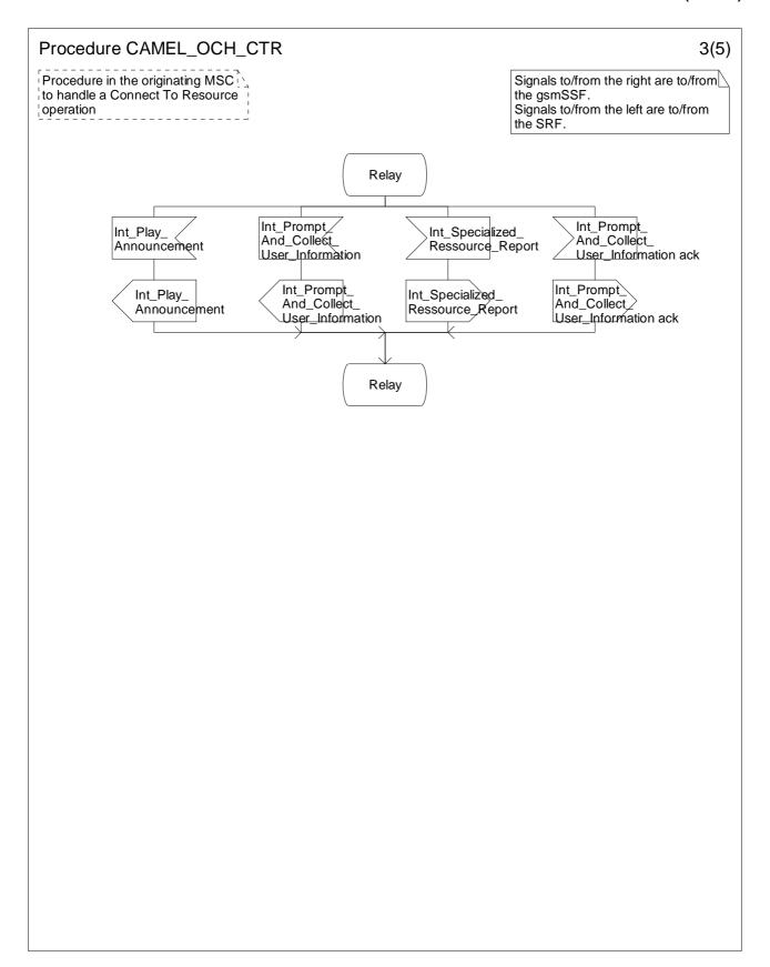
Figure 4.24-3: Procedure CAMEL\_OCH\_CTR (sheet 3)
