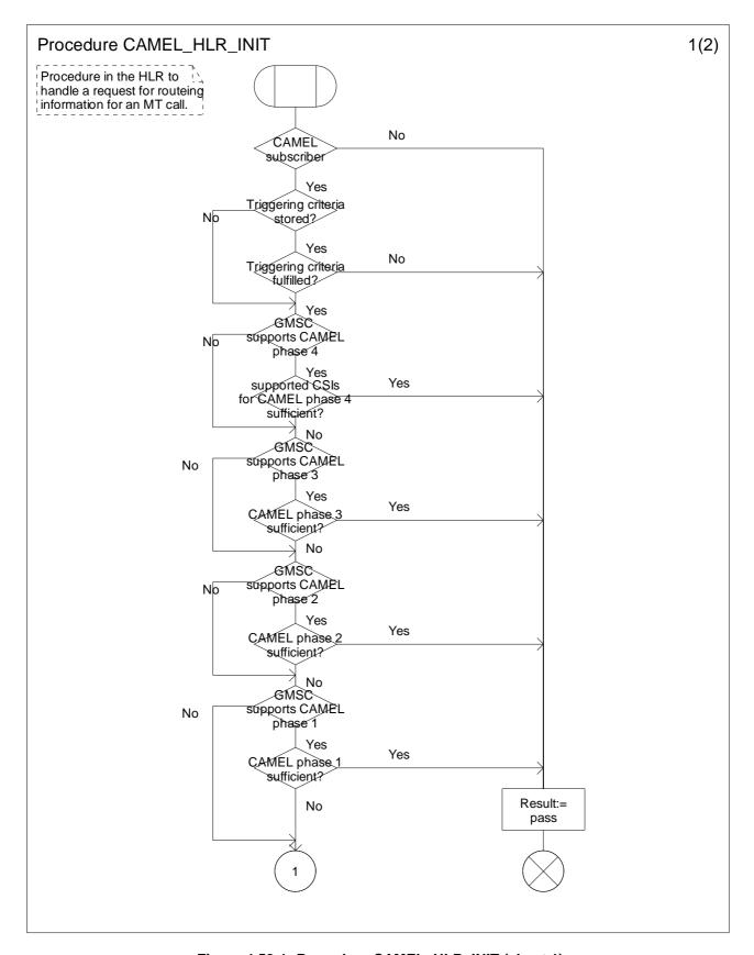
Figure 4.58-1: Procedure CAMEL\_HLR\_INIT (sheet 1)
