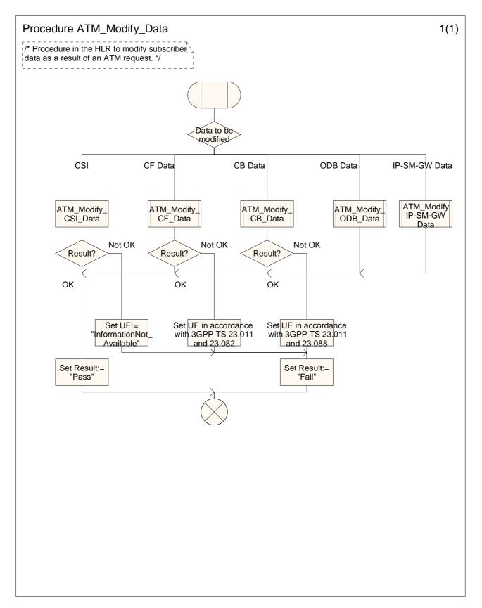
Figure 10.4-1: Procedure ATM\_Modify\_Data (sheet 1)
