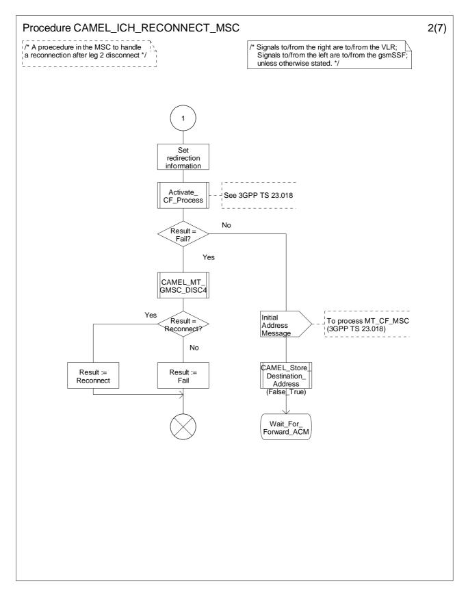
Figure 4.74-2: Procedure CAMEL\_ICH\_RECONNECT\_MSC (sheet 2)
