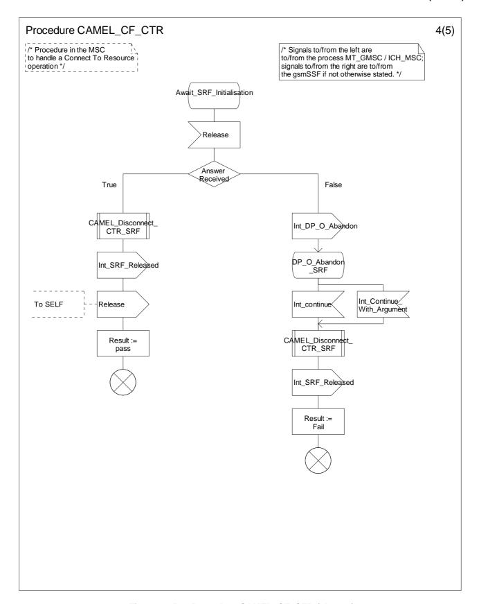
Figure 4.85-4: Procedure CAMEL\_CF\_CTR (sheet 4)
