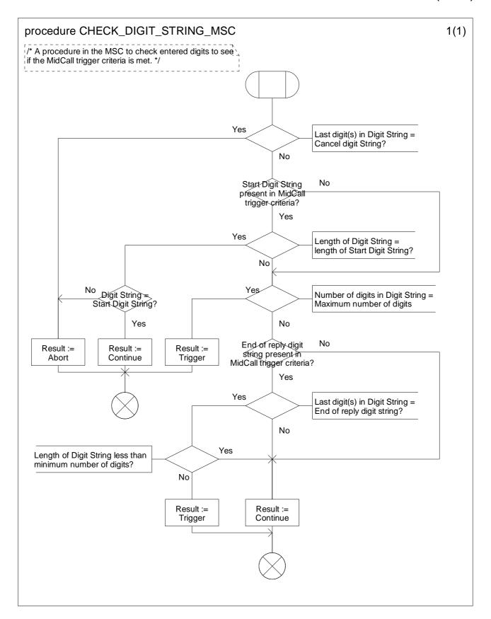
Figure 4.31-1: Procedure CHECK\_DIGIT\_STRING\_MSC (sheet 1)
