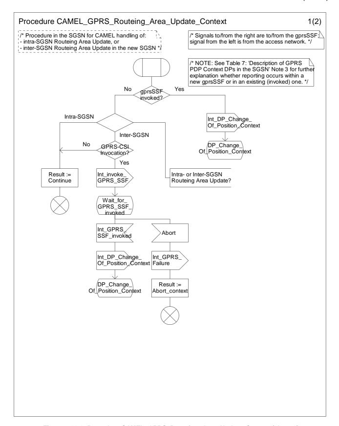
Figure 6.11-1: Procedure CAMEL\_GPRS\_Routeing\_Area\_Update\_Context (sheet 1)
