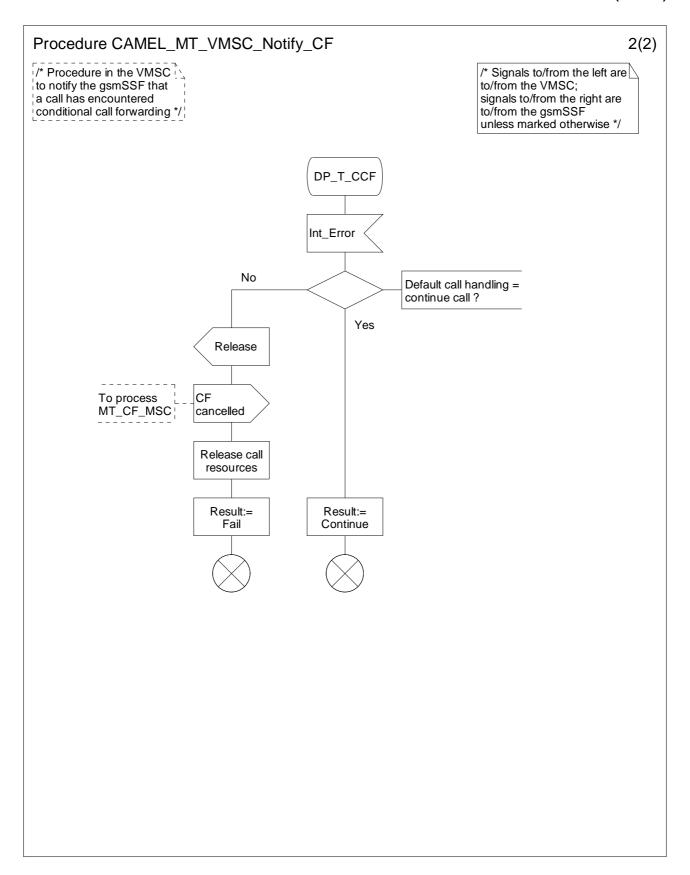
Figure 4.70-2: Procedure CAMEL\_MT\_VMSC\_Notify\_CF (sheet 2)
