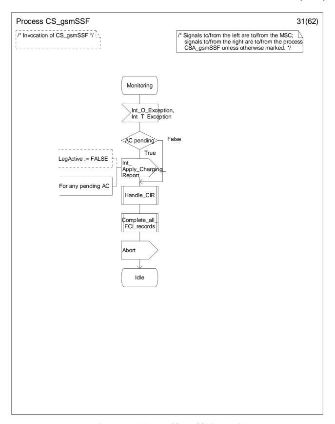
Figure 4.99-31: Process CS\_gsmSSF (sheet 31)
