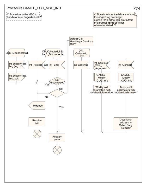
Figure 4.119B-2: Procedure CAMEL\_TOC\_MSC\_INIT (sheet 2)
