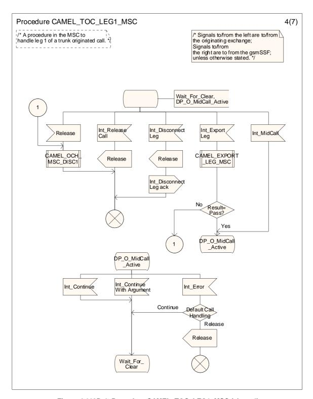
Figure 4.119D-4: Procedure CAMEL\_TOC\_LEG1\_MSC (sheet 4)
