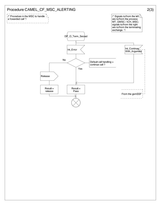
Figure 4.82-2: Procedure CAMEL\_CF\_MSC\_ALERTING (sheet 2)
