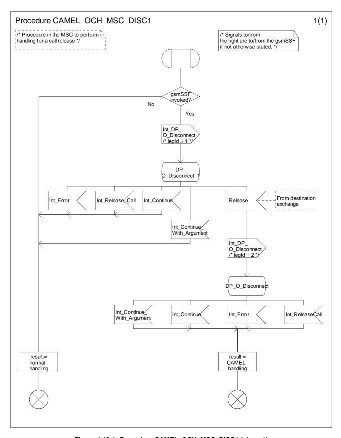
Figure 4.18-1: Procedure CAMEL\_OCH\_MSC\_DISC1 (sheet 1)
