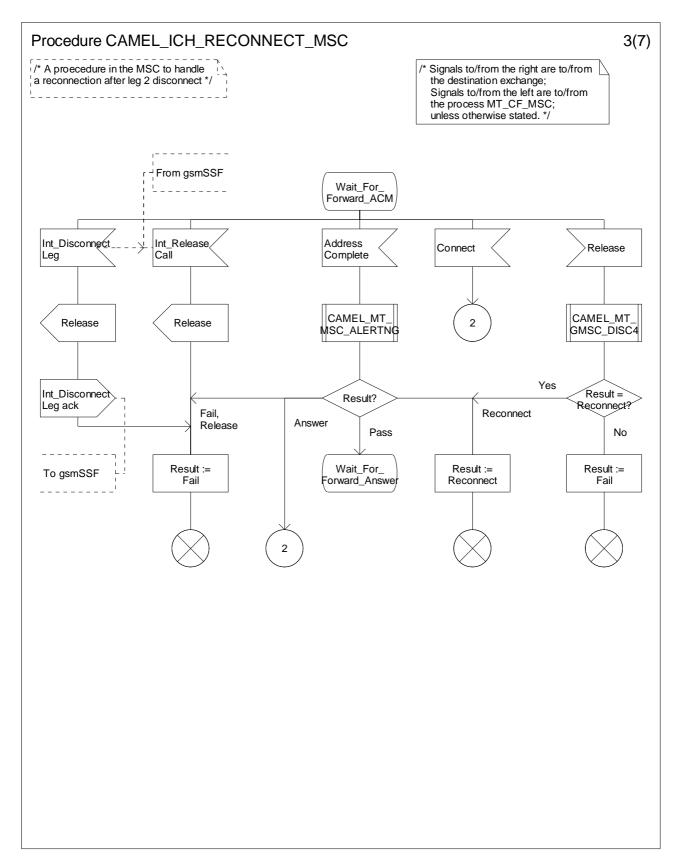
Figure 4.74-3: Procedure CAMEL\_ICH\_RECONNECT\_MSC (sheet 3)
