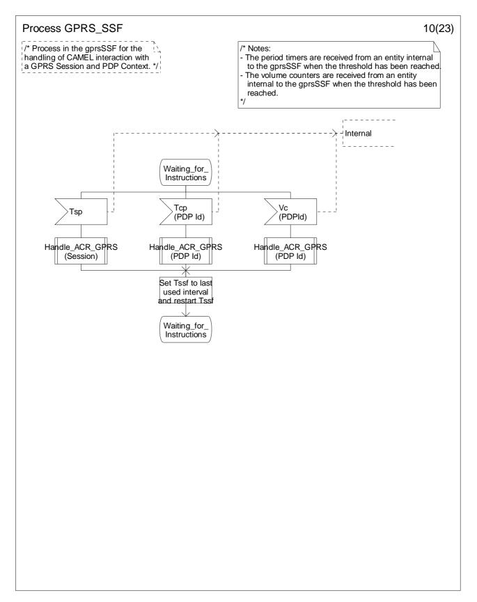
Figure 6.17-10: Process GPRS\_SSF (sheet 10)
