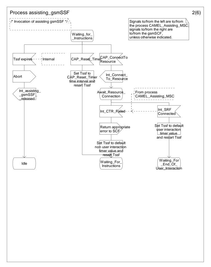
Figure 4.118-2: Process Assisting\_gsmSSF (sheet 2)
