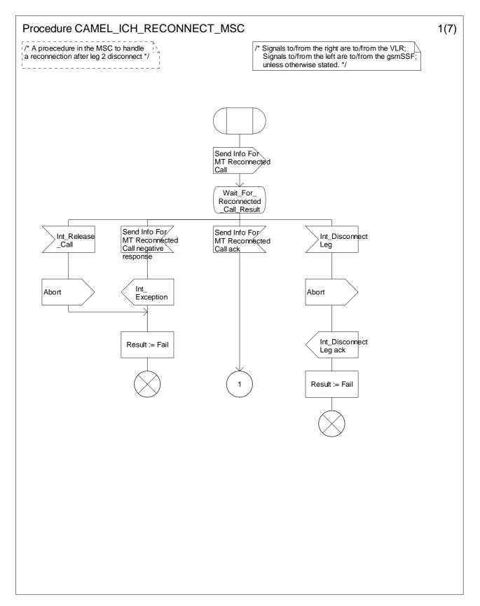
Figure 4.74-1: Procedure CAMEL\_ICH\_RECONNECT\_MSC (sheet 1)
