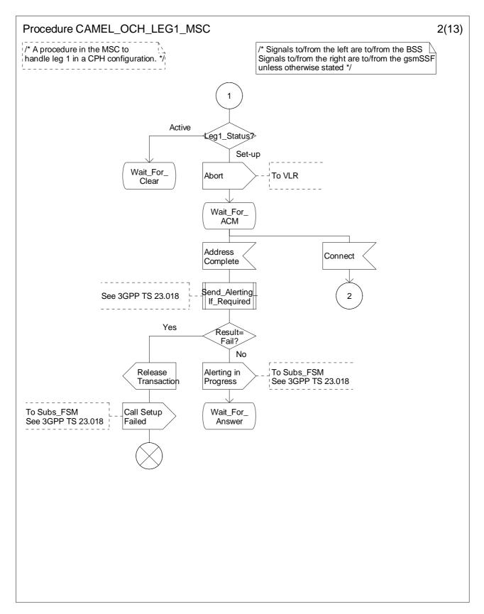
Figure 4.30-2: Procedure CAMEL\_OCH\_LEG1\_MSC (sheet 2)
