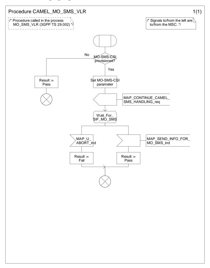
Figure 7.8-1: Procedure CAMEL\_MO\_SMS\_VLR (sheet 1)
