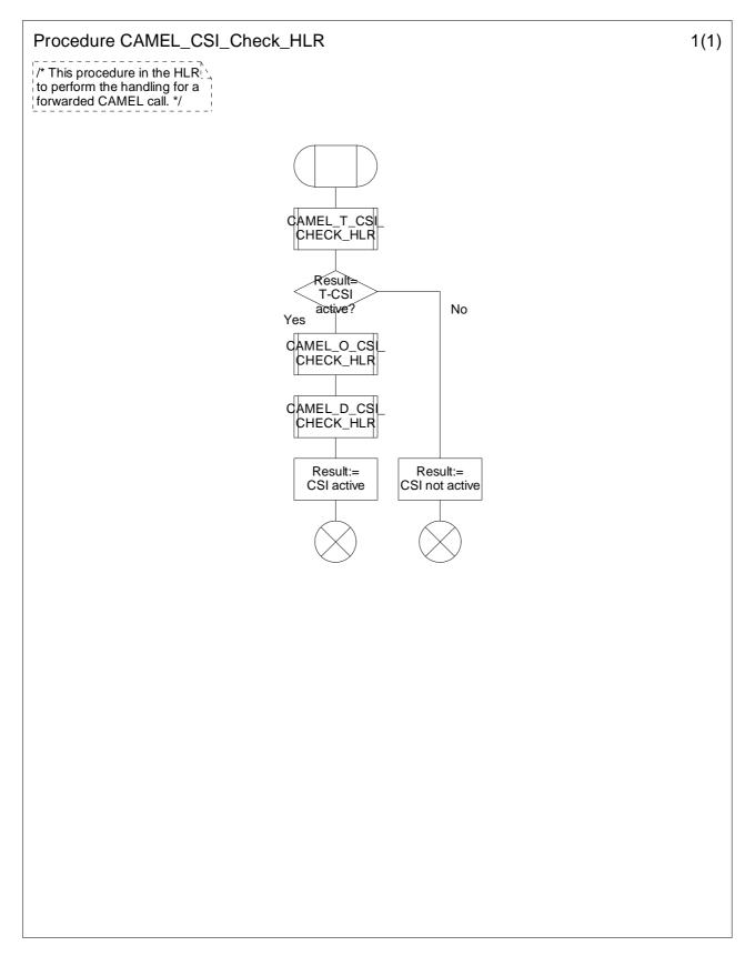
Figure 4.59-1: Procedure CAMEL\_CSI\_Check\_HLR (sheet 1)
