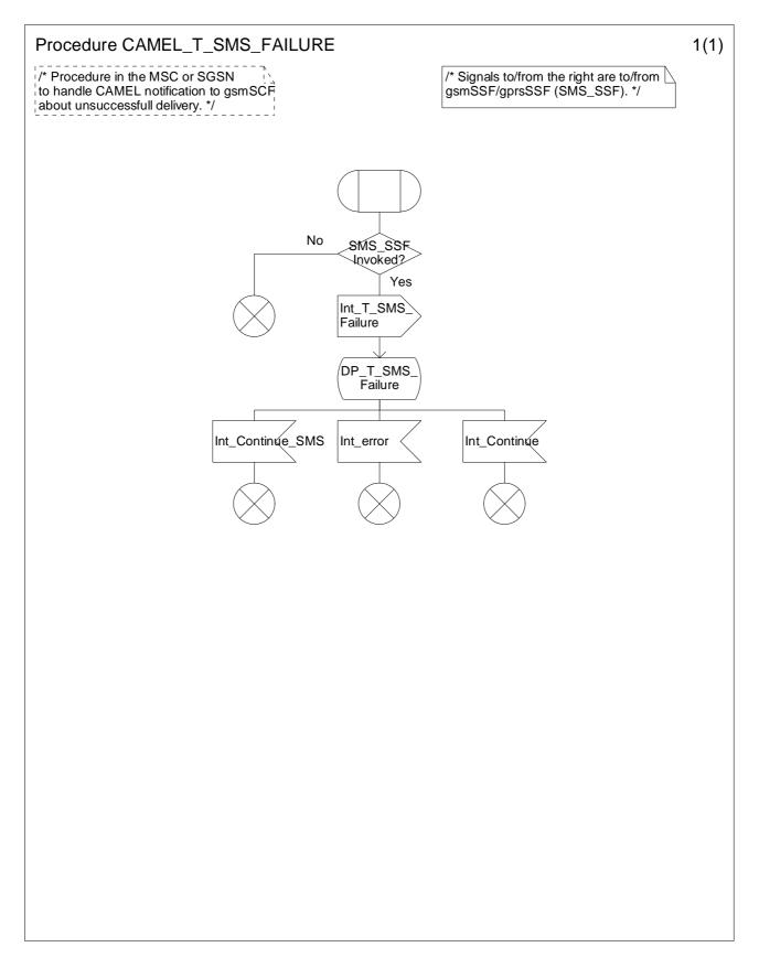
Figure 7.11-1: Procedure CAMEL\_T\_SMS\_FAILURE (sheet 1)
