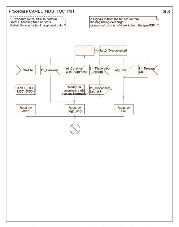
Figure 4.119C-5: Procedure CAMEL\_NDS\_TOC\_INIT (sheet 5)
