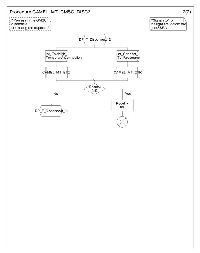
Figure 4.46-2: Procedure CAMEL\_MT\_GMSC\_DISC2 (sheet 2)
