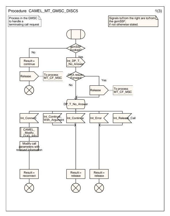
Figure 4.49-1: Procedure CAMEL\_MT\_GMSC\_DISC5 (sheet 1)
