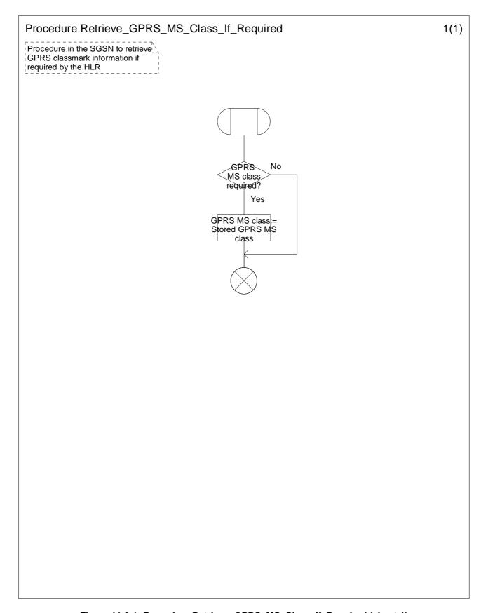
Figure 11.6-1: Procedure Retrieve\_GPRS\_MS\_Class\_If\_Required (sheet 1)
