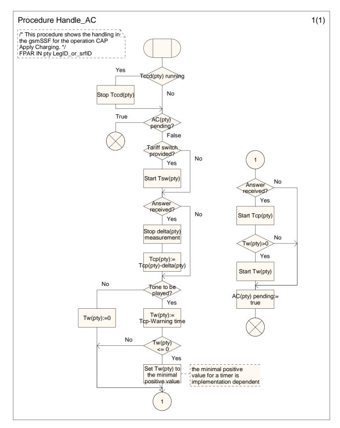
Figure 4.104-1: Procedure Handle\_AC (sheet 1)
