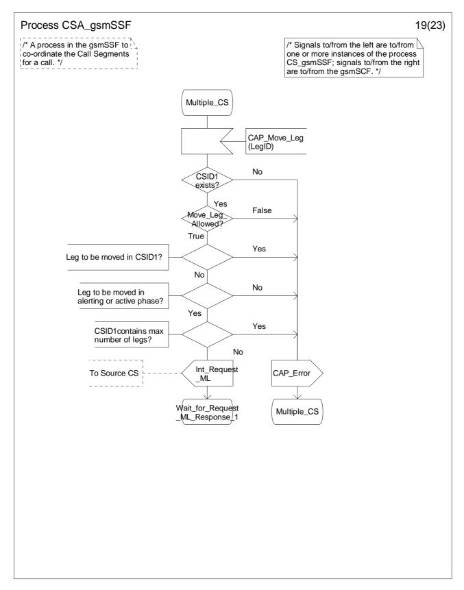
Figure 4.116-19: Process CSA\_gsmSSF (sheet 19)
