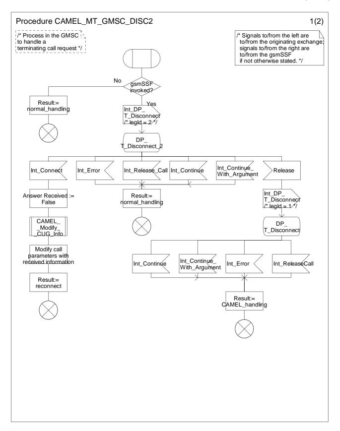
Figure 4.46-1: Procedure CAMEL\_MT\_GMSC\_DISC2 (sheet 1)
