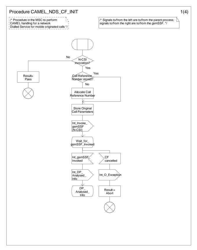
Figure 4.81-1: Procedure CAMEL\_NDS\_CF\_INIT (sheet 1)
