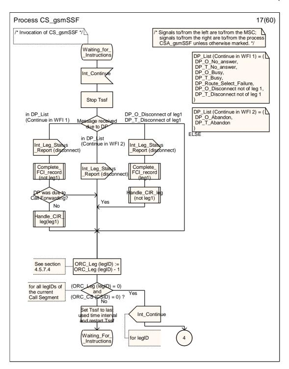
Figure 4.99-17: Process CS\_gsmSSF (sheet 17)
