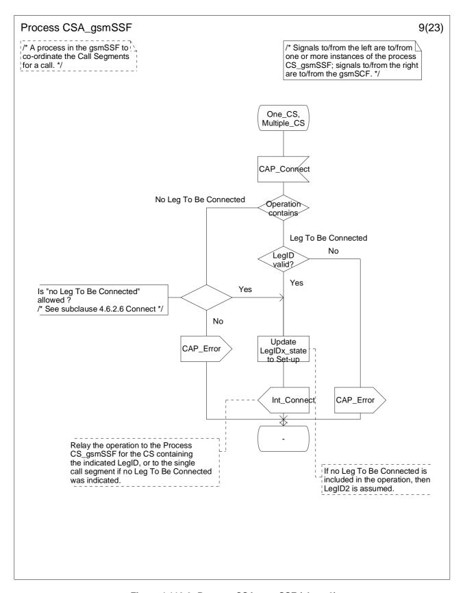
Figure 4.116-9: Process CSA\_gsmSSF (sheet 9)
