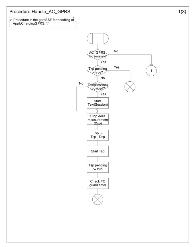
Figure 6.19-1: Procedure Handle\_AC\_GPRS (sheet 1)
