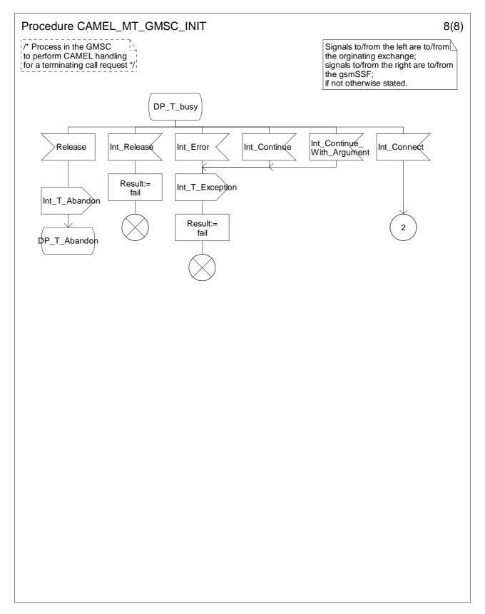
Figure 4.42-8: Procedure CAMEL\_MT\_GMSC\_INIT (sheet 8)
