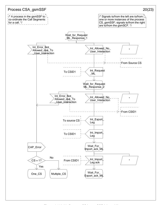
Figure 4.116-20: Process CSA\_gsmSSF (sheet 20)
