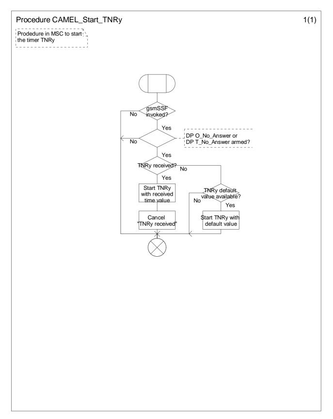
Figure 4.25-1: Procedure CAMEL\_Start\_TNRy (sheet 1)
