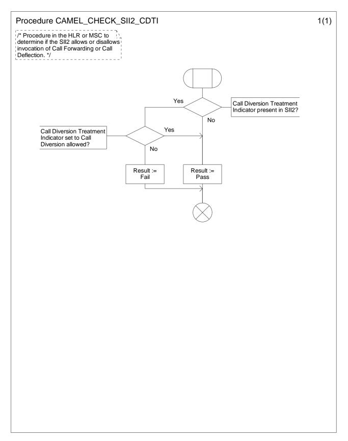
Figure 4.63-1: Procedure CAMEL\_CHECK\_SII2\_CDTI (sheet 1)
