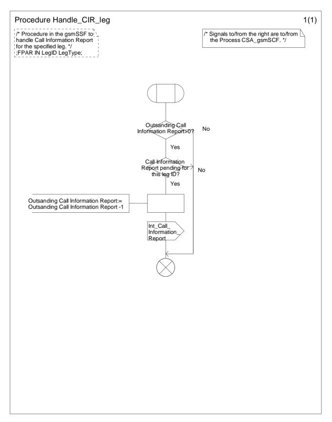
Figure 4.107-1: Procedure Handle\_CIR\_leg (sheet 1)
