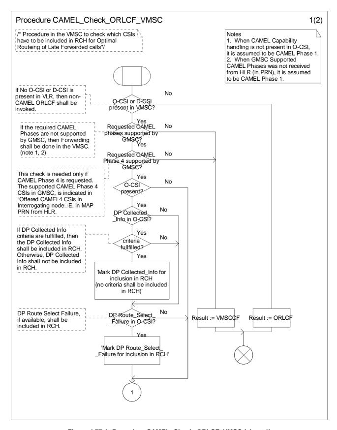
Figure 4.77-1: Procedure CAMEL\_Check\_ORLCF\_VMSC (sheet 1)
