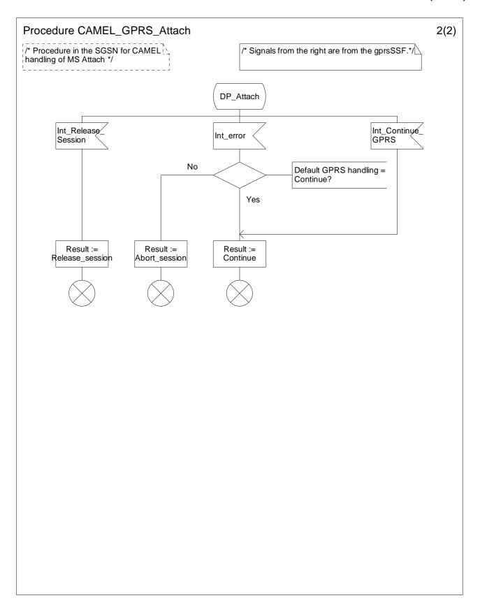
Figure 6.8-2: Procedure CAMEL\_GPRS\_Attach (sheet 2)
