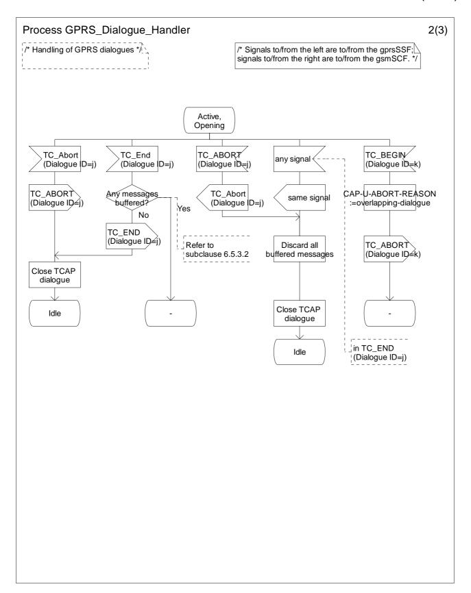
Figure 6.18-2: Process GPRS\_Dialogue\_Handler (sheet 2)
