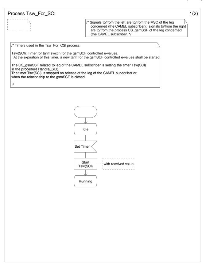
Figure 4.98-1: Process Tsw\_For\_SCI (sheet 1)
