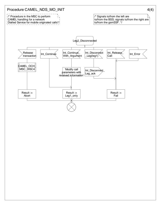
Figure 4.13-4: Procedure CAMEL\_NDS\_MO\_INIT (sheet 4)
