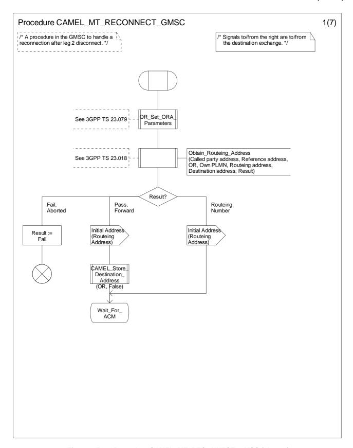
Figure 4.56-1: Procedure CAMEL\_MT\_RECONNECT\_GMSC (sheet 1)
