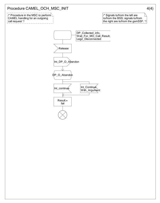
Figure 4.10-4: Procedure CAMEL\_OCH\_MSC\_INIT (sheet 4)
