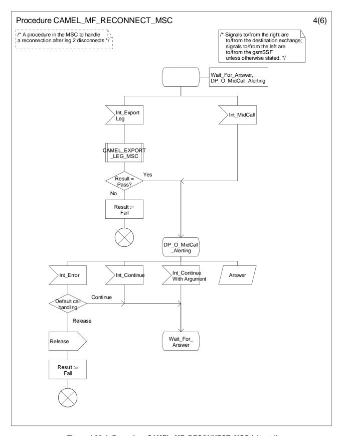
Figure 4.88-4: Procedure CAMEL\_MF\_RECONNECT\_MSC (sheet 4)
