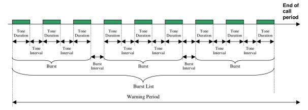
Figure 4.97: Representation of burst list
