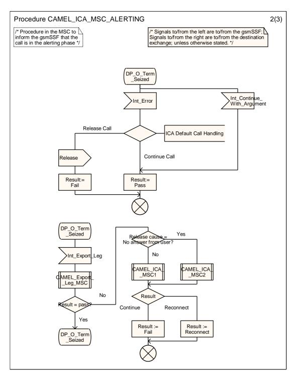
Figure 4.90-2: Process CAMEL\_ICA\_MSC\_ALERTING (sheet 2)
