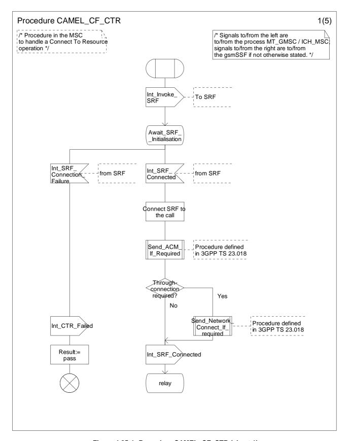
Figure 4.85-1: Procedure CAMEL\_CF\_CTR (sheet 1)
