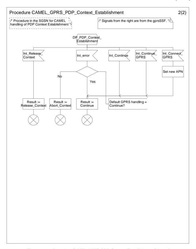
Figure 6.12-2: Procedure CAMEL\_GPRS\_PDP\_Context\_Establishment (sheet 2)
