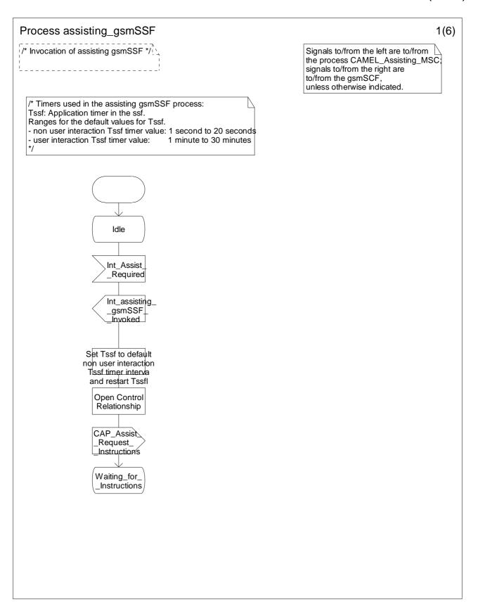
Figure 4.118-1: Process Assisting\_gsmSSF (sheet 1)
