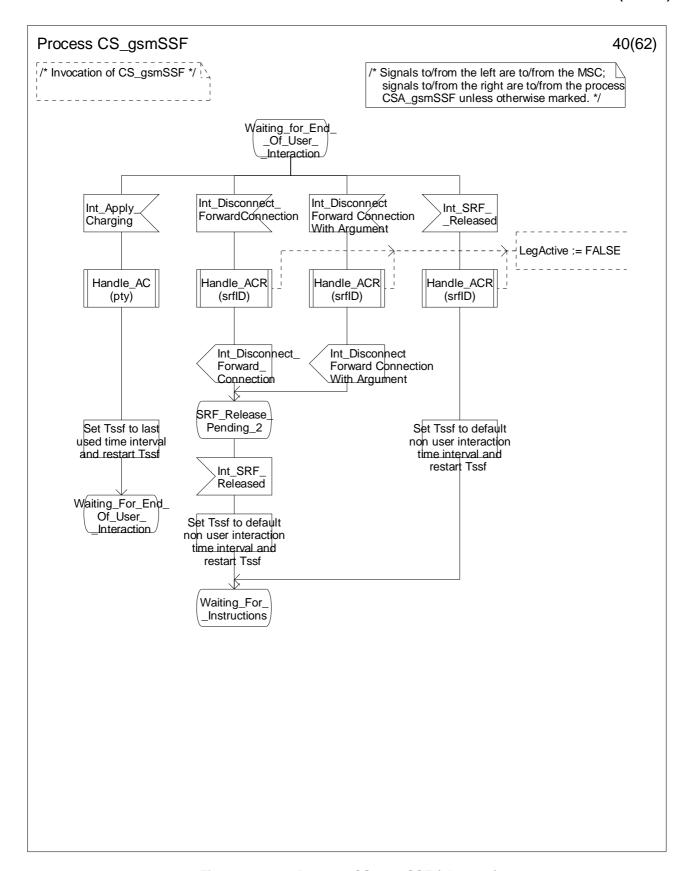
Figure 4.99-40: Process CS\_gsmSSF (sheet 40)
