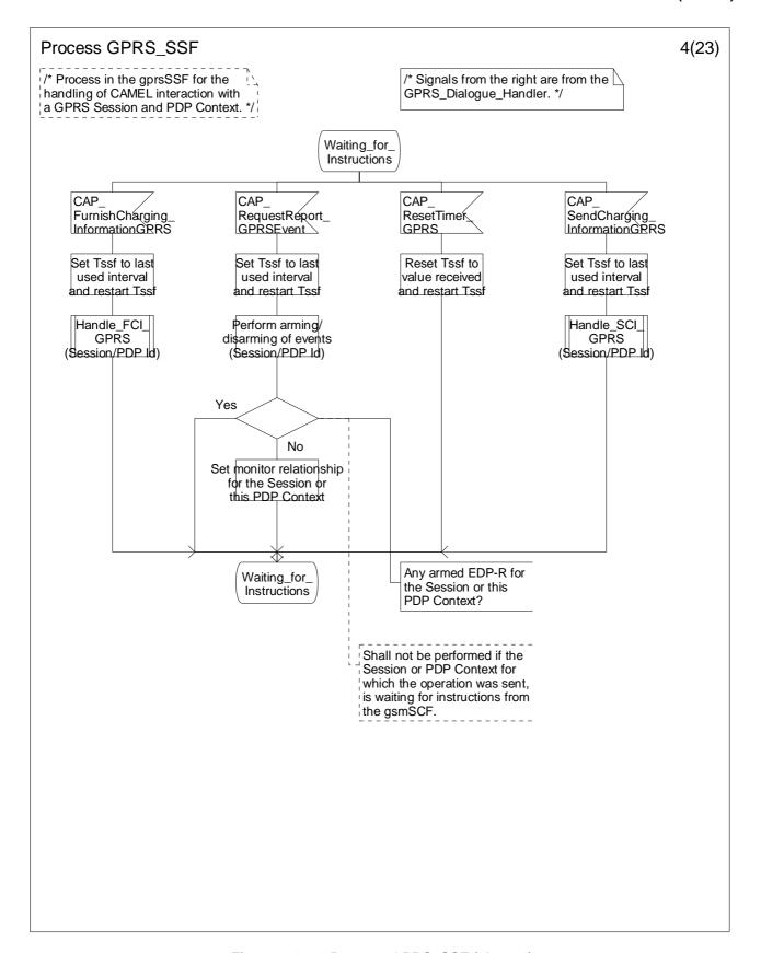
Figure 6.17-4: Process GPRS\_SSF (sheet 4)
