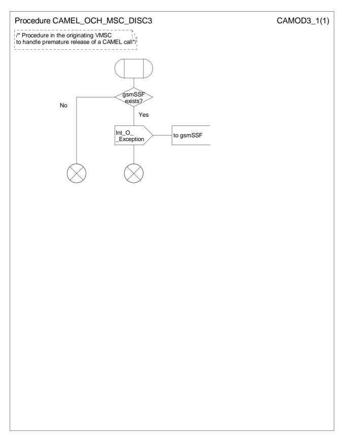
Figure 4.20-1: Procedure CAMEL\_OCH\_MSC\_DISC3 (sheet 1)
