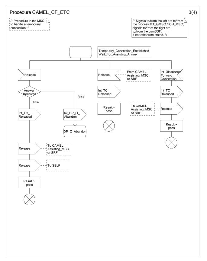
Figure 4.84-3: Procedure CAMEL\_CF\_ETC (sheet 3)
