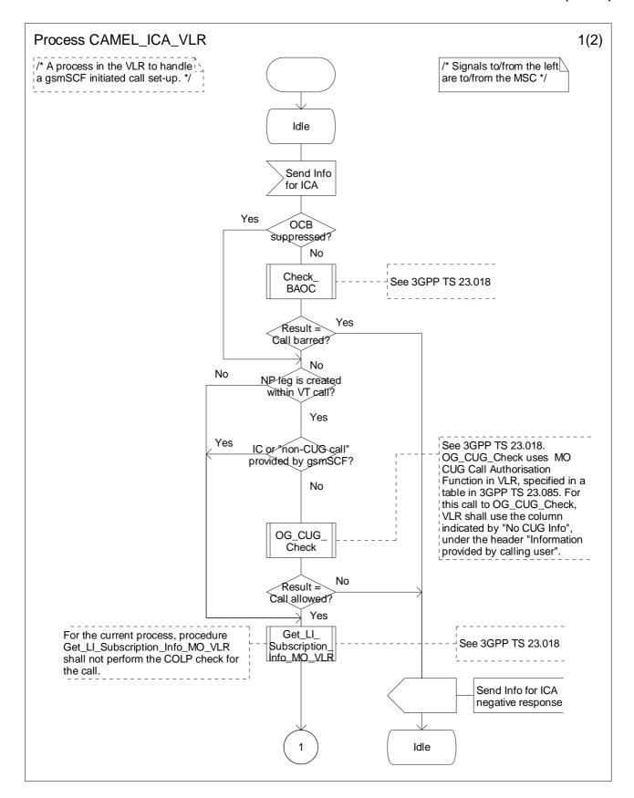
Figure 4.95-1: Process CAMEL\_ICA\_VLR (sheet 1)
