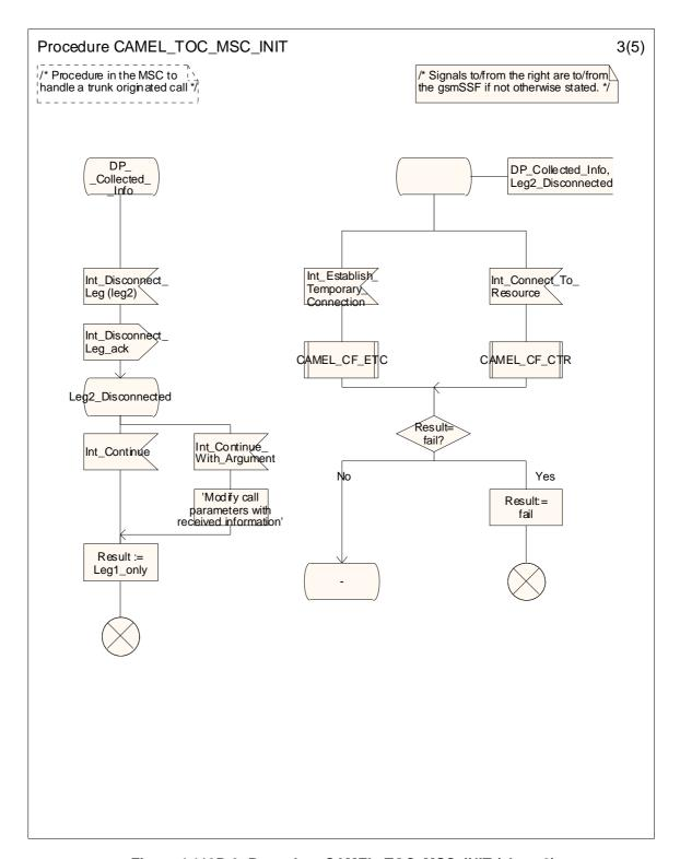
Figure 4.119B-3: Procedure CAMEL\_TOC\_MSC\_INIT (sheet 3)
