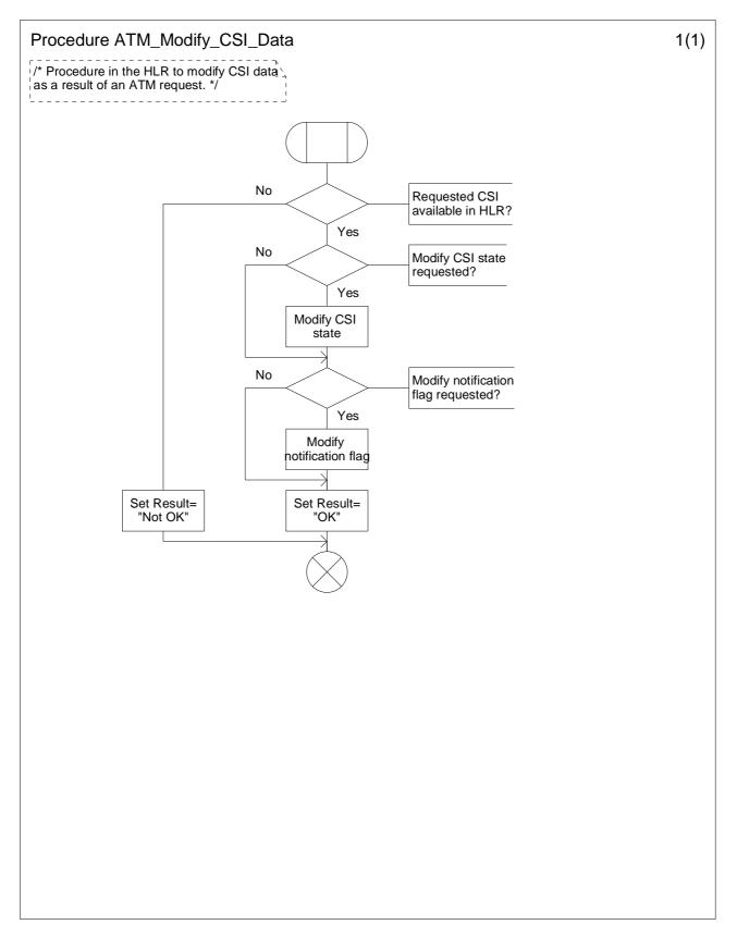
Figure 10.5-1: Procedure ATM\_Modify\_CSI\_Data (sheet 1)
