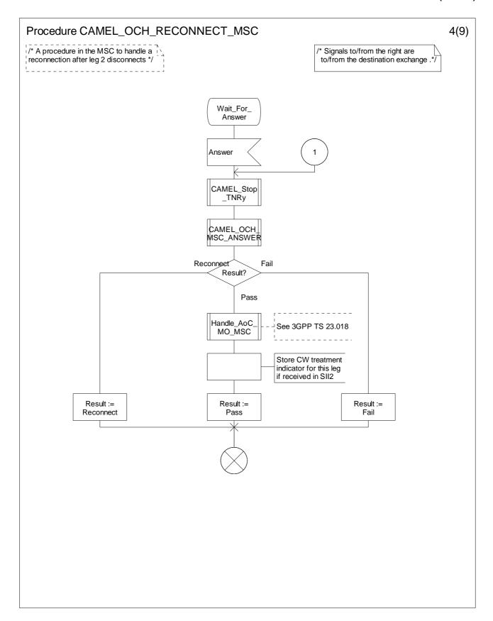
Figure 4.33-4: Procedure CAMEL\_OCH\_RECONNECT\_MSC (sheet 4)
