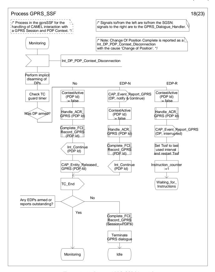
Figure 6.17-18: Process GPRS\_SSF (sheet 18)
