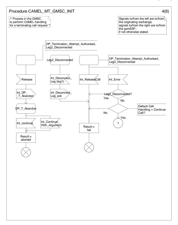
Figure 4.42-4: Procedure CAMEL\_MT\_GMSC\_INIT (sheet 4)
