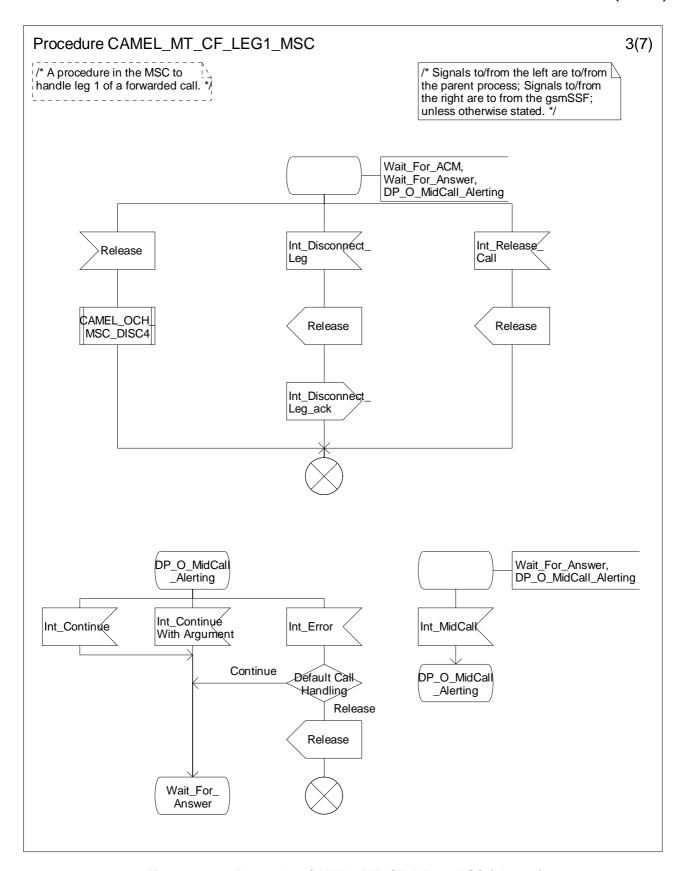
Figure 4.86-3: Procedure CAMEL\_MT\_CF\_LEG1\_MSC (sheet 3)
