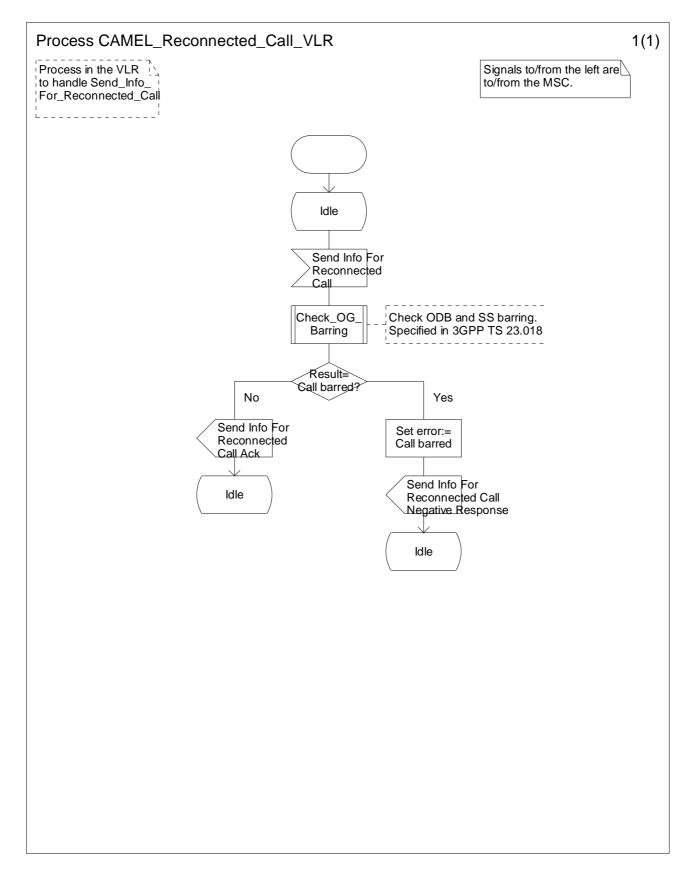
Figure 4.40-1: Process CAMEL\_Reconnected\_Call\_VLR (sheet 1)
