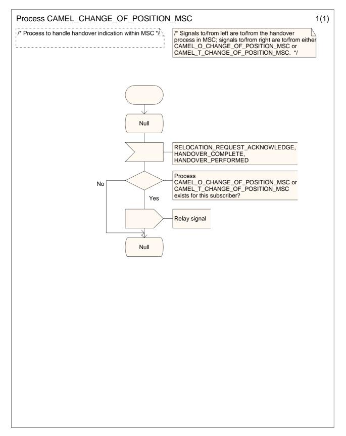
Figure 4.35-1: Process CAMEL\_CHANGE\_OF\_POSITION\_MSC (sheet 1)
