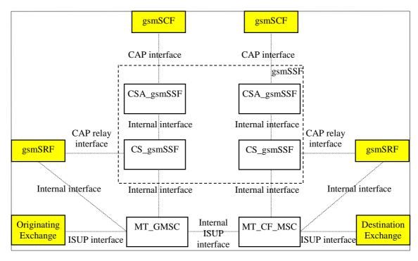
Figure 4.9-3: Terminating GMSC case (gsmSSF relay)
