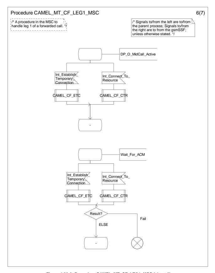
Figure 4.86-6: Procedure CAMEL\_MT\_CF\_LEG1\_MSC (sheet 6)
