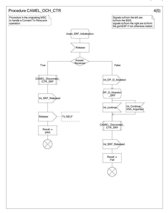
Figure 4.24-4: Procedure CAMEL\_OCH\_CTR (sheet 4)
