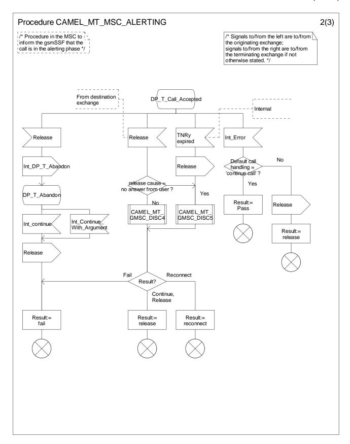
Figure 4.43-2: Procedure CAMEL\_MT\_MSC\_ALERTING (sheet 2)
