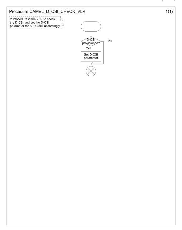
Figure 4.67-1: Procedure CAMEL\_D\_CSI\_Check\_VLR (sheet 1)
