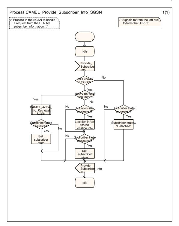
Figure 11.4-1: Process CAMEL\_Provide\_Subscriber\_Info\_SGSN (sheet 1)
