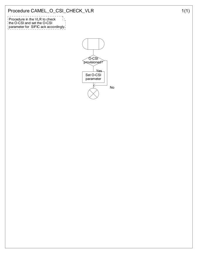
Figure 4.66-1: Procedure CAMEL\_O\_CSI\_Check\_VLR (sheet 1)
