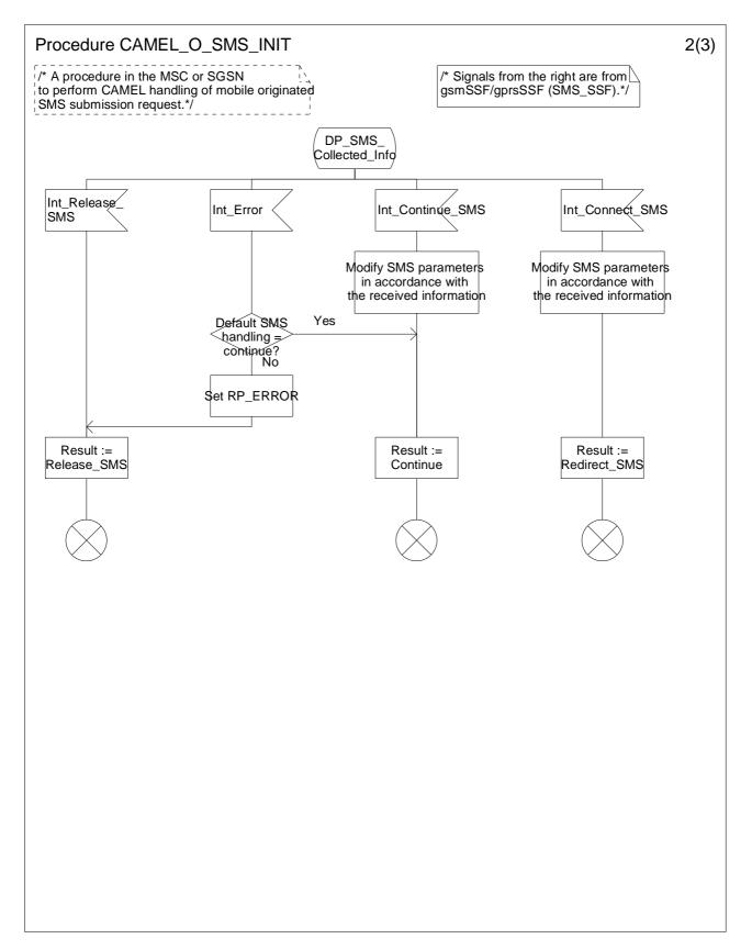
Figure 7.5-2: Procedure CAMEL\_O\_SMS\_INIT (sheet 2)
