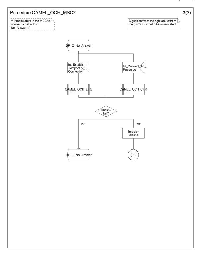
Figure 4.17-3: Procedure CAMEL\_OCH\_MSC2 (sheet 3)
