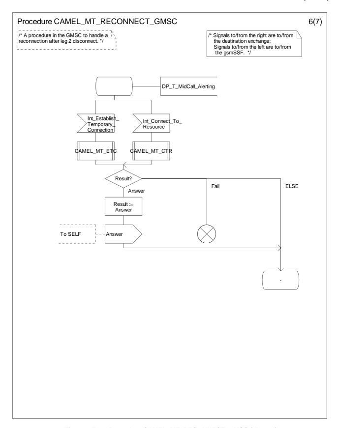
Figure 4.56-6: Procedure CAMEL\_MT\_RECONNECT\_GMSC (sheet 6)
