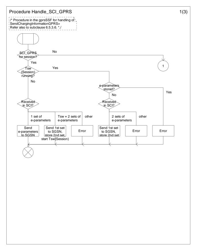
Figure 6.23-1: Procedure Handle\_SCI\_GPRS (sheet 1)
