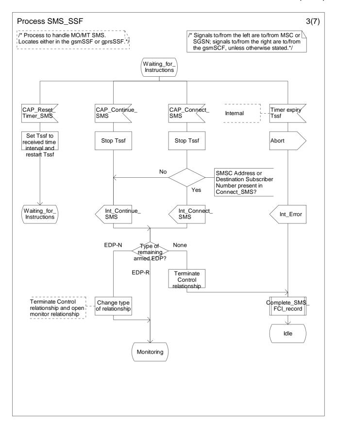
Figure 7.15-3: Process SMS\_SSF (sheet 3)
