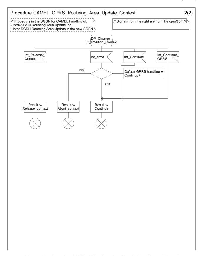
Figure 6.11-2: Procedure CAMEL\_GPRS\_Routeing\_Area\_Update\_Context (sheet 2)
