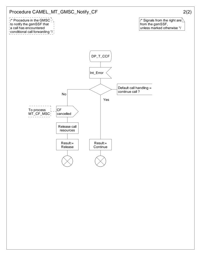
Figure 4.53-2: Procedure CAMEL\_MT\_GMSC\_Notify\_CF (sheet 2)
