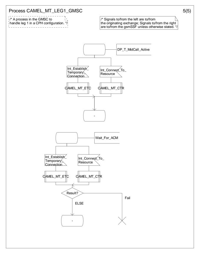
Figure 4.55-5: Process CAMEL\_MT\_LEG1\_GMSC (sheet 5)
