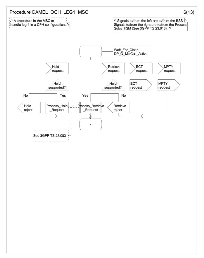
Figure 4.30-6: Procedure CAMEL\_OCH\_LEG1\_MSC (sheet 6)
