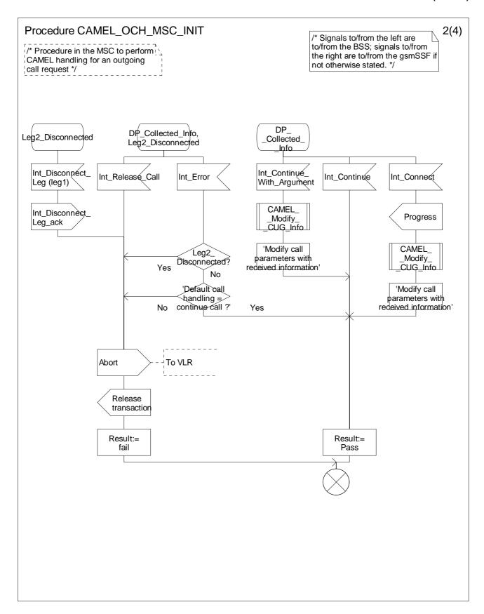
Figure 4.10-2: Procedure CAMEL\_OCH\_MSC\_INIT (sheet 2)
