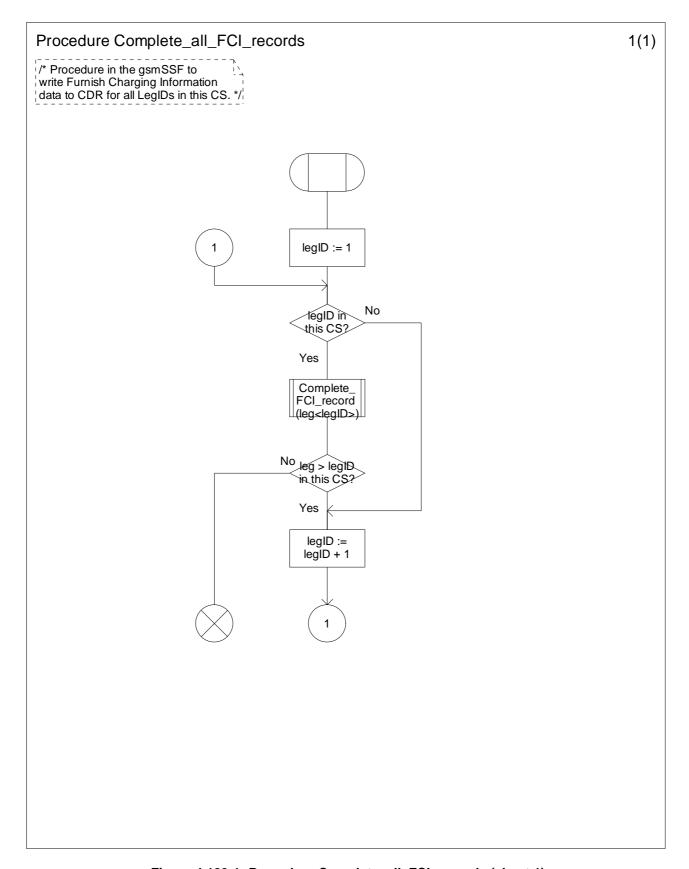
Figure 4.109-1: Procedure Complete\_all\_FCI\_records (sheet 1)
