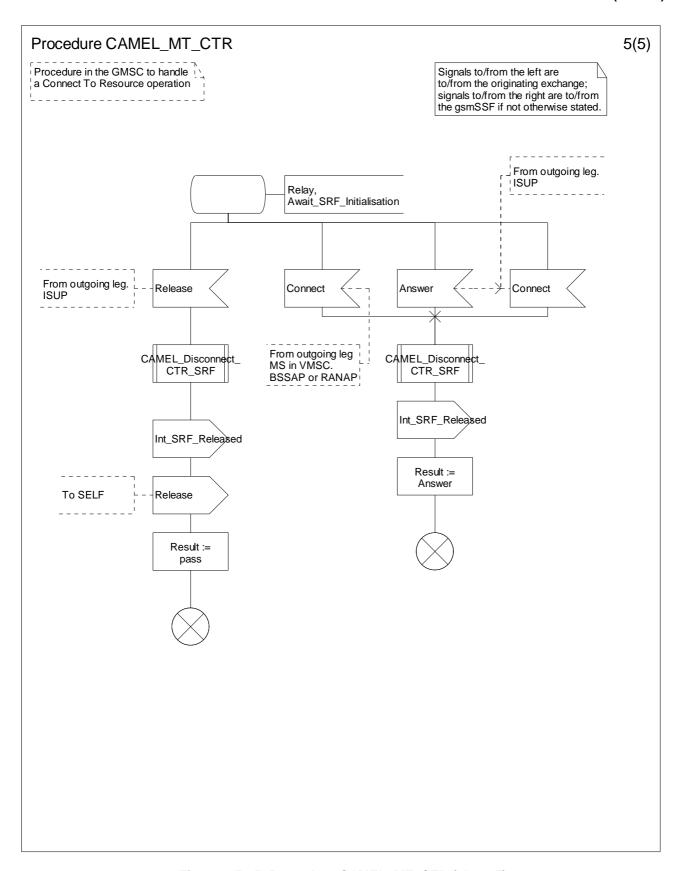
Figure 4.52-5: Procedure CAMEL\_MT\_CTR (sheet 5)
