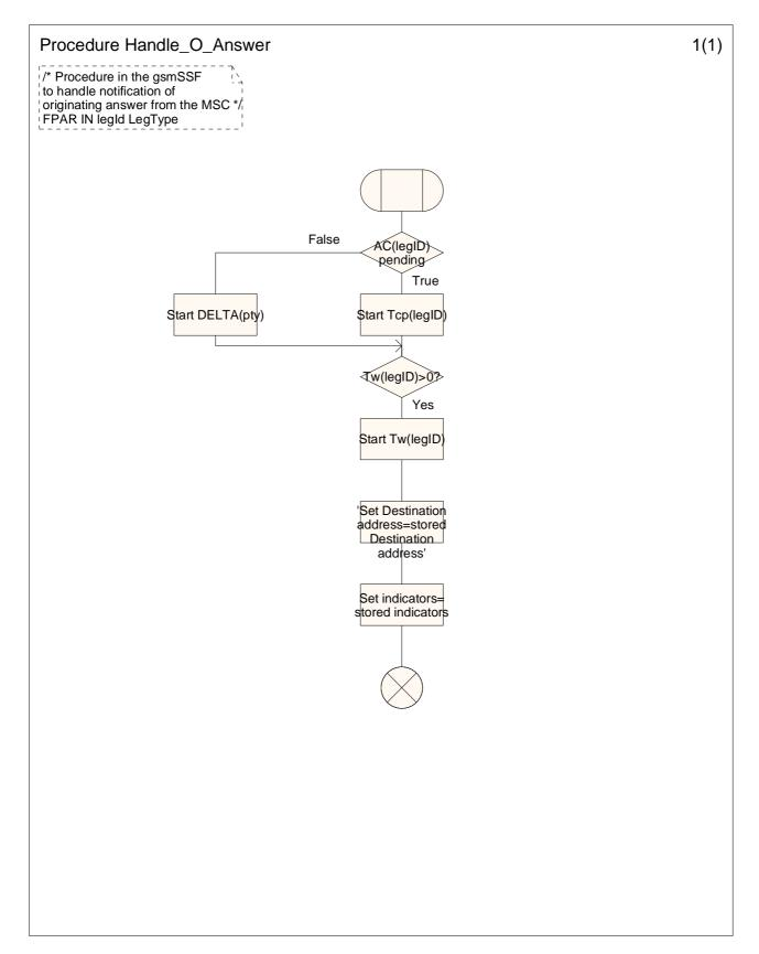
Figure 4.110-1: Procedure Handle\_O\_Answer (sheet 1)
