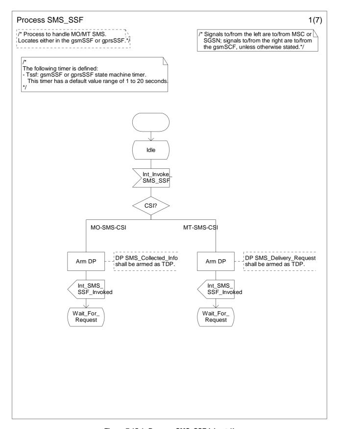
Figure 7.15-1: Process SMS\_SSF (sheet 1)
