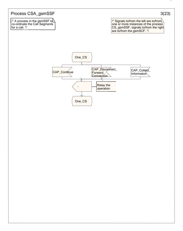
Figure 4.116-3: Process CSA\_gsmSSF (sheet 3)
