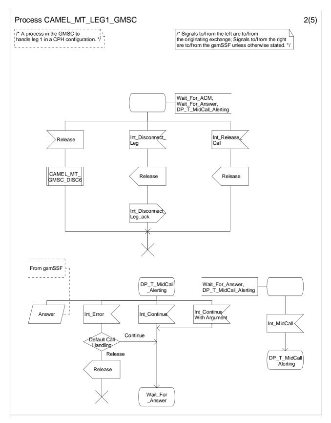
Figure 4.55-2: Process CAMEL\_MT\_LEG1\_GMSC (sheet 2)
