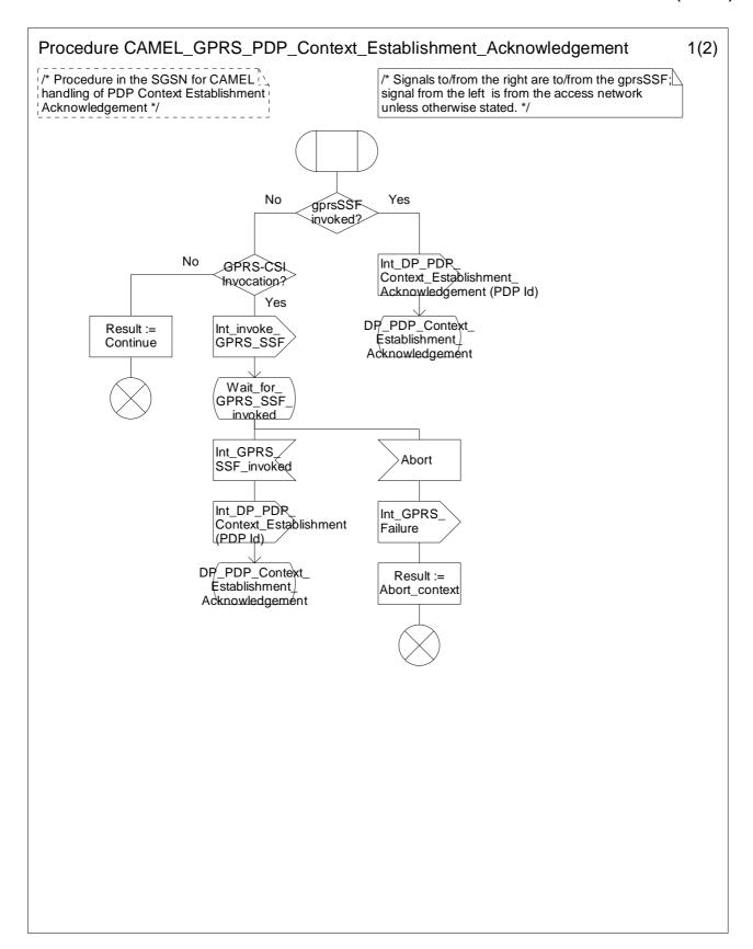
Figure 6.13-1: Procedure CAMEL\_GPRS\_PDP\_Context\_Establishment\_Acknowledgement (sheet 1)
