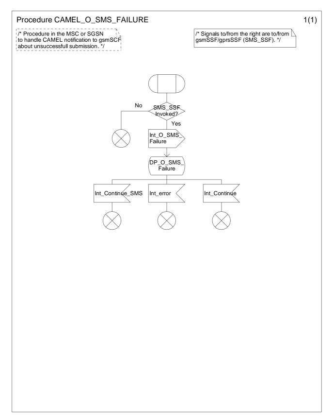
Figure 7.7-1: Procedure CAMEL\_O\_SMS\_FAILURE (sheet 1)
