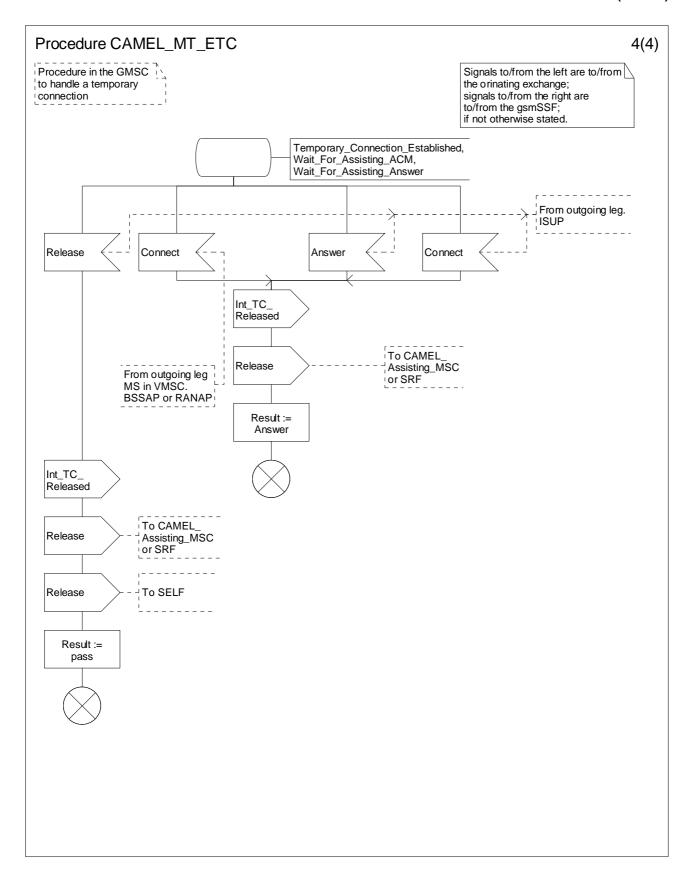
Figure 4.51-4: Procedure CAMEL\_MT\_ETC (sheet 4)
