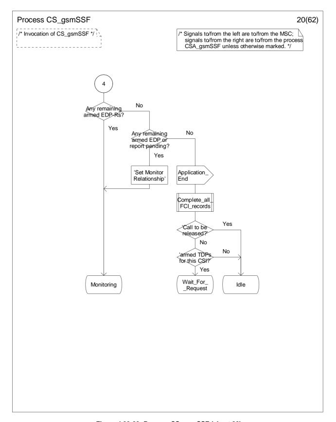
Figure 4.99-20: Process CS\_gsmSSF (sheet 20)
