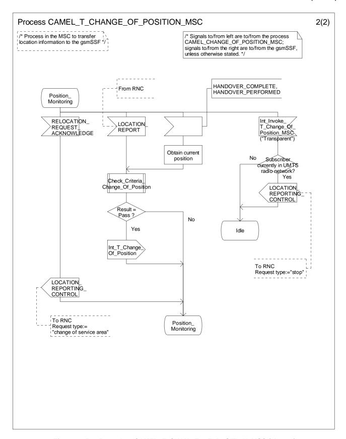
Figure 4.75-2: Procedure CAMEL\_T\_CHANGE\_OF\_POSITION\_MSC (sheet 2)
