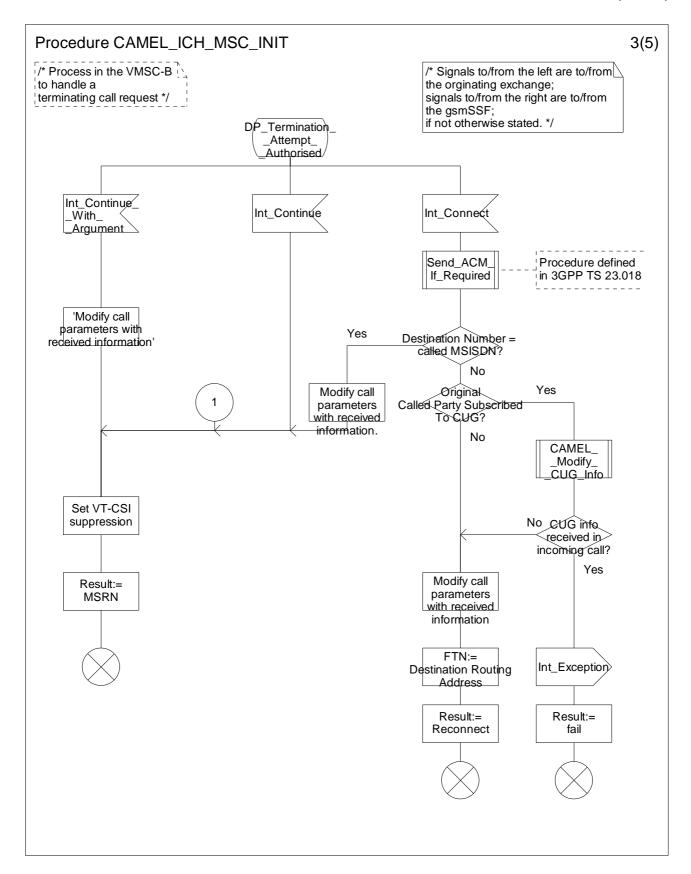
Figure 4.69-3: Procedure CAMEL\_ICH\_MSC\_INIT (sheet 3)
