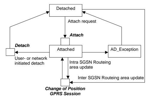
Figure 6.3: GPRS Attach/Detach State Model
