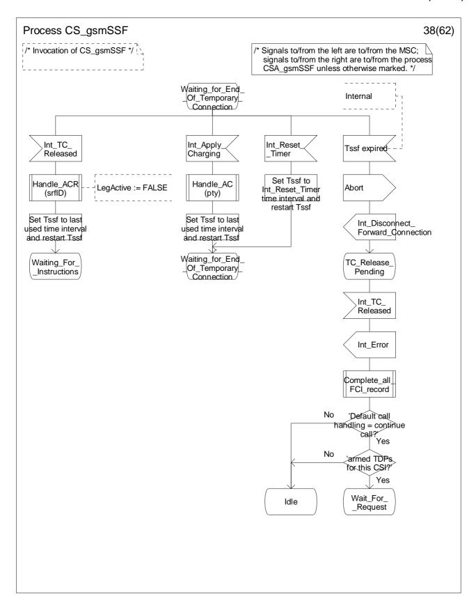
Figure 4.99-38: Process CS\_gsmSSF (sheet 38)
