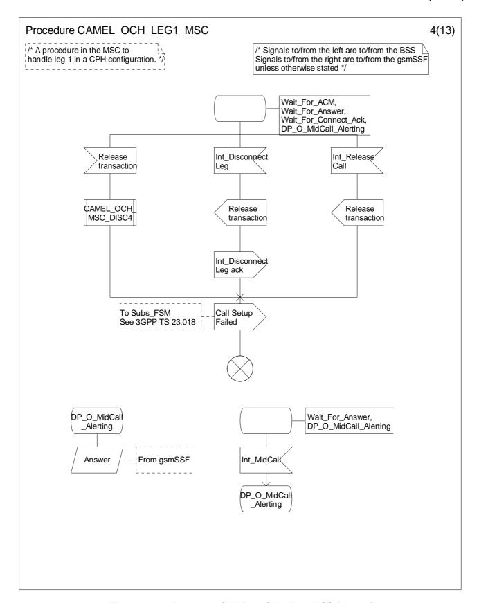
Figure 4.30-4: Procedure CAMEL\_OCH\_LEG1\_MSC (sheet 4)
