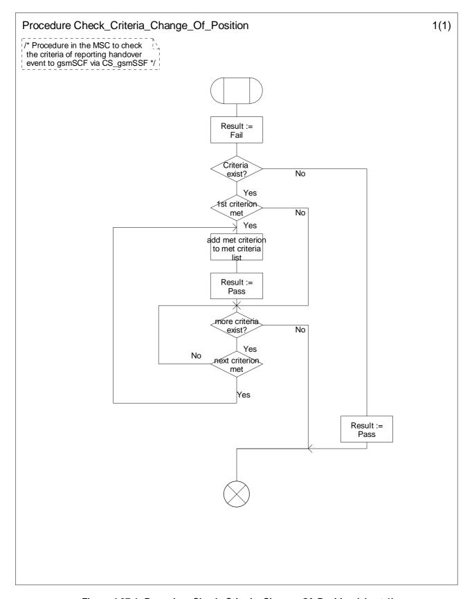
Figure 4.37-1: Procedure Check\_Criteria\_Change\_Of\_Position (sheet 1)
