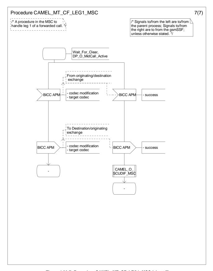
Figure 4.86-7: Procedure CAMEL\_MT\_CF\_LEG1\_MSC (sheet 7)
