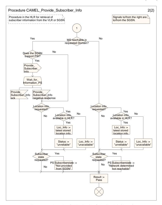
Figure 4.119-2: Procedure CAMEL\_Provide\_Subscriber\_Info (sheet 2)
