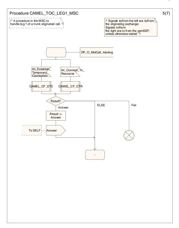
Figure 4.119D-5: Procedure CAMEL\_TOC\_LEG1\_MSC (sheet 5)
