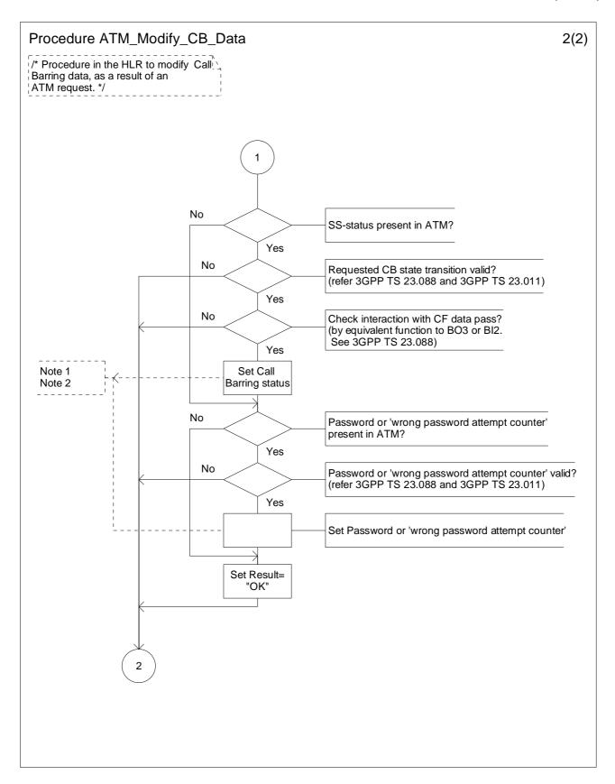
Figure 10.7-2: Procedure ATM\_Modify\_CB\_Data (sheet 2)
