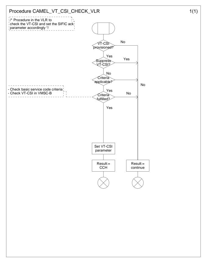
Figure 4.68-1: Procedure CAMEL\_VT\_CSI\_Check\_VLR (sheet 1)
