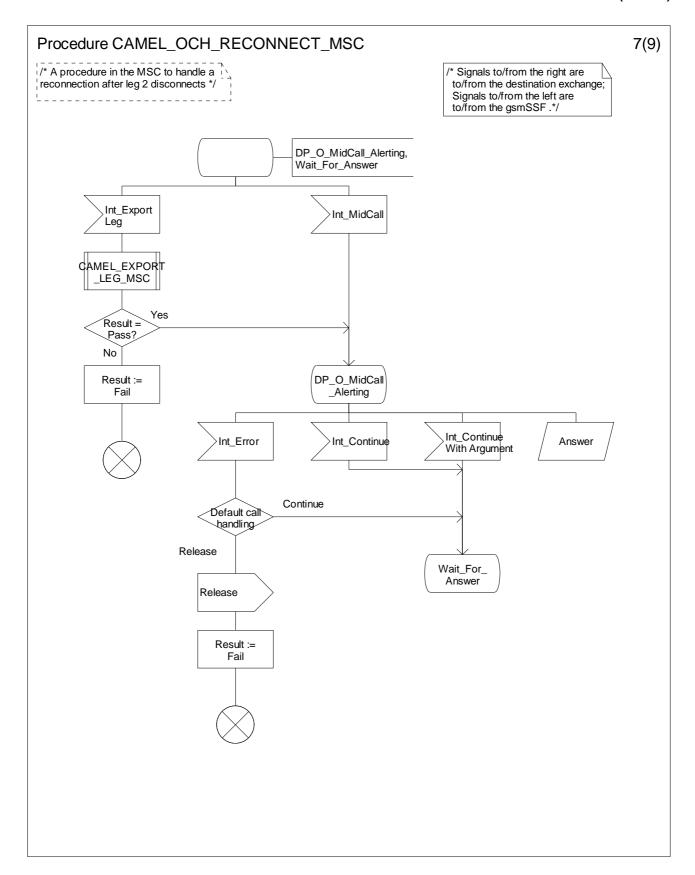
Figure 4.33-7: Procedure CAMEL\_OCH\_RECONNECT\_MSC (sheet 7)
