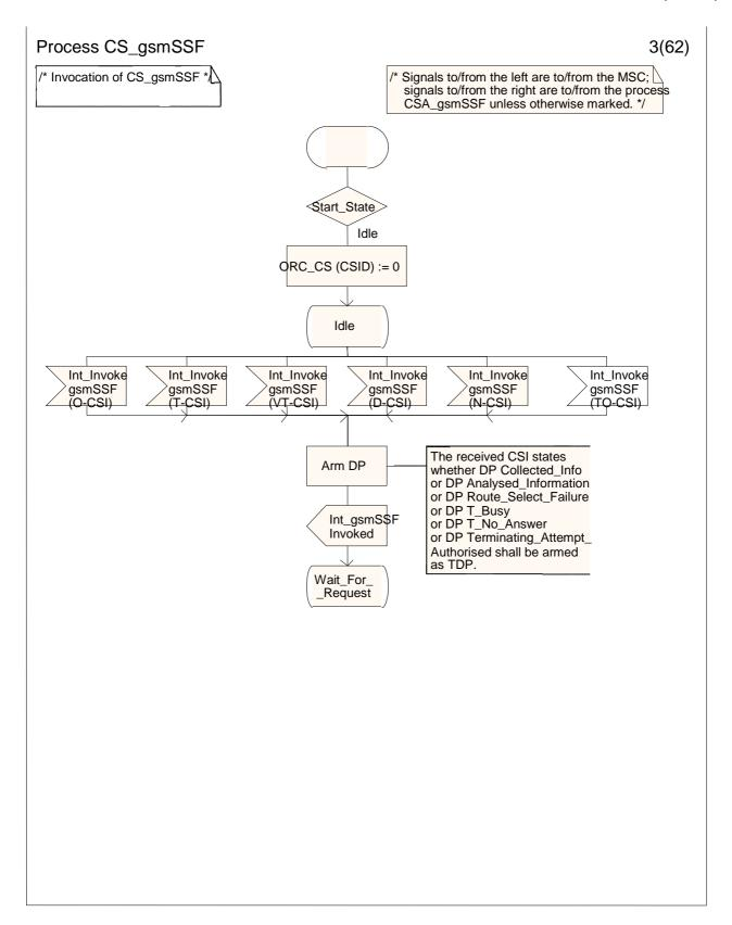
Figure 4.99-3: Process CS\_gsmSSF (sheet 3)
