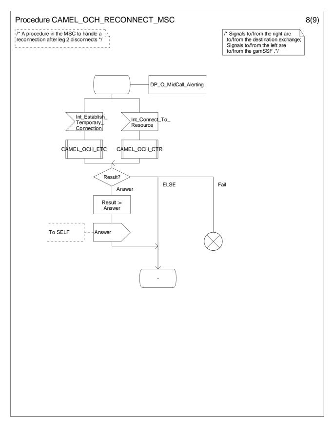
Figure 4.33-8: Procedure CAMEL\_OCH\_RECONNECT\_MSC (sheet 8)
