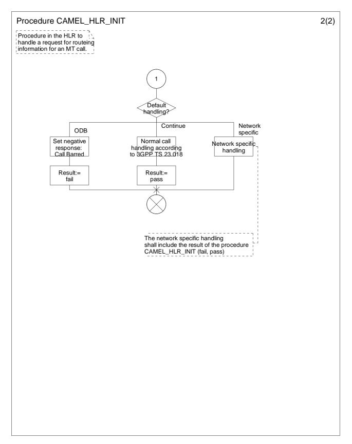
Figure 4.58-2: Procedure CAMEL\_HLR\_INIT (sheet 2)
