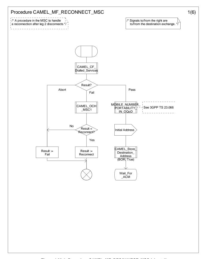
Figure 4.88-1: Procedure CAMEL\_MF\_RECONNECT\_MSC (sheet 1)
