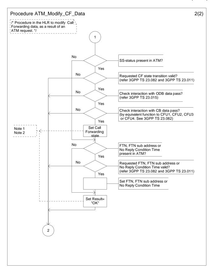
Figure 10.6-2: Procedure ATM\_Modify\_CF\_Data (sheet 2)
