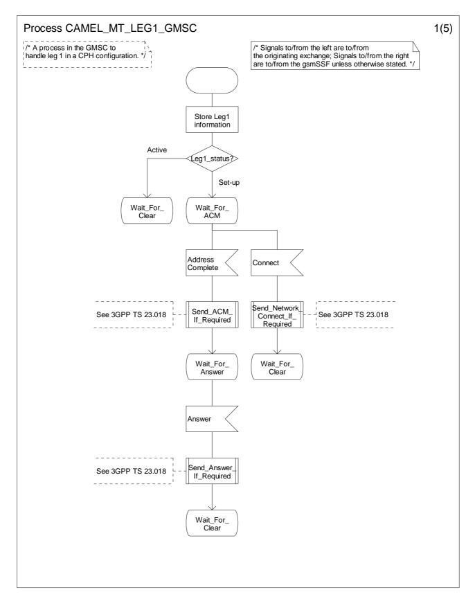
Figure 4.55-1: Process CAMEL\_MT\_LEG1\_GMSC (sheet 1)
