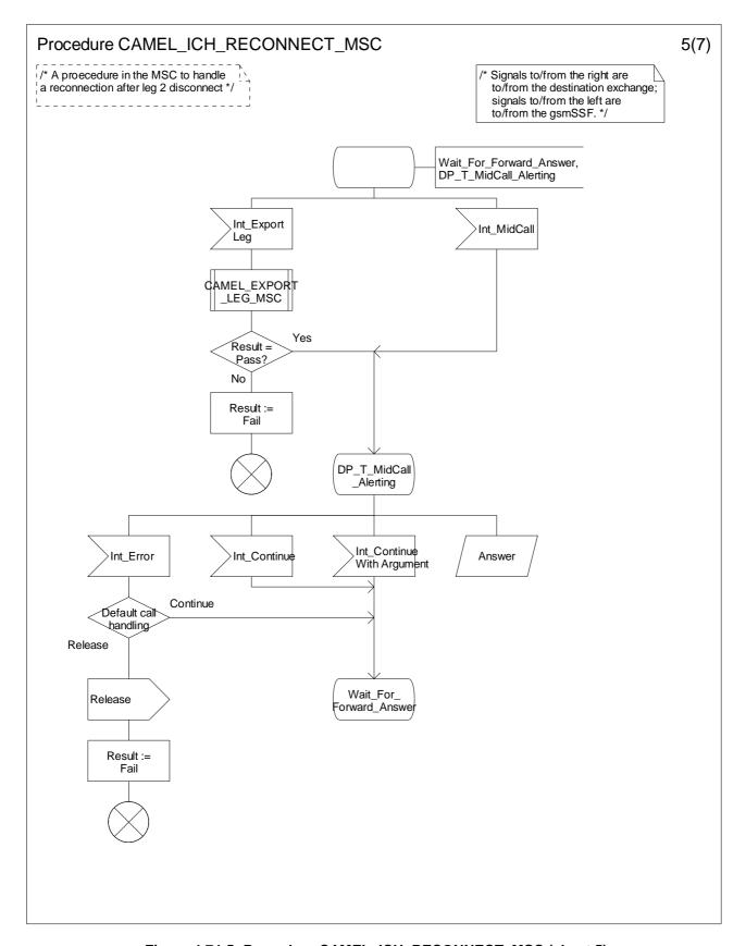
Figure 4.74-5: Procedure CAMEL\_ICH\_RECONNECT\_MSC (sheet 5)
