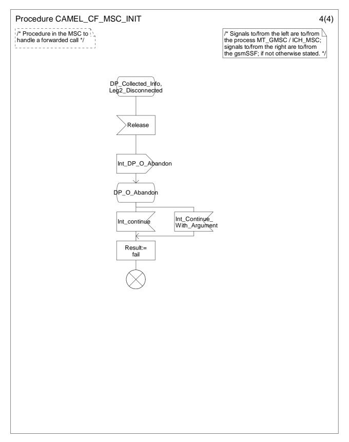
Figure 4.79-4: Procedure CAMEL\_CF\_MSC\_INIT (sheet 4)
