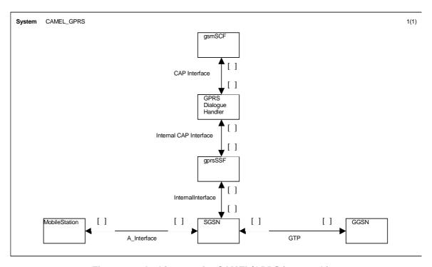
Figure 6.7: Architecture for CAMEL/GPRS interworking
