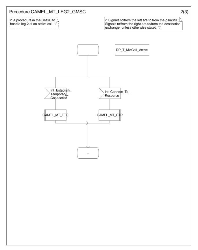
Figure 4.54-2: Procedure CAMEL\_MT\_LEG2\_GMSC (sheet 2)
