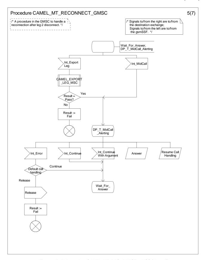
Figure 4.56-5: Procedure CAMEL\_MT\_RECONNECT\_GMSC (sheet 5)
