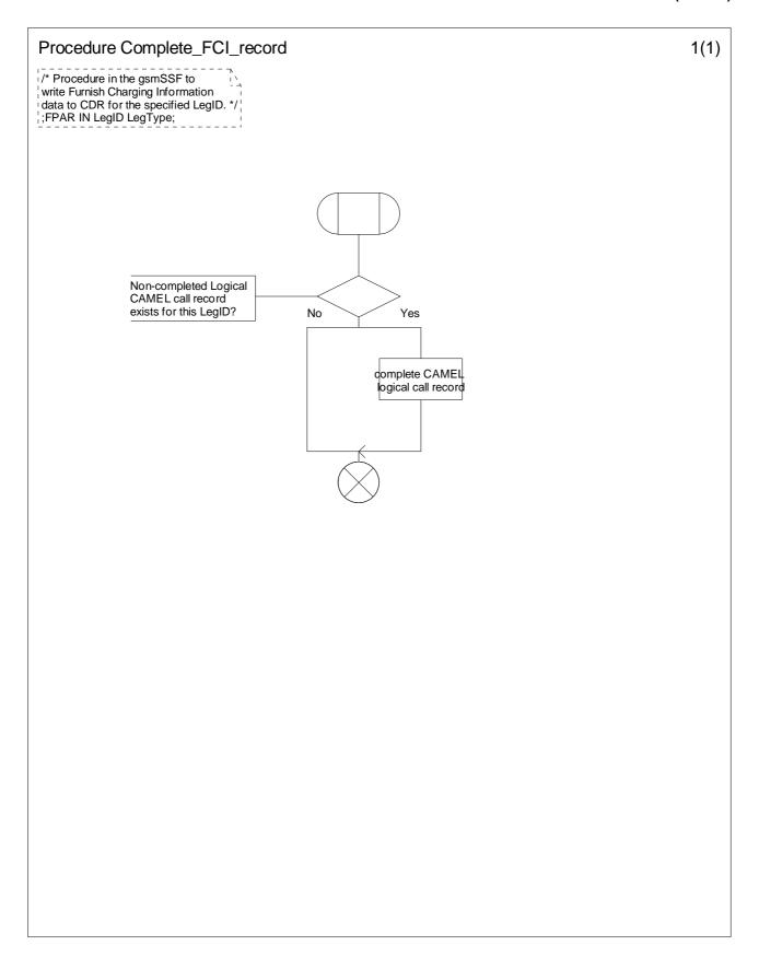
Figure 4.108-1: Procedure Complete\_FCI\_record (sheet 1)
