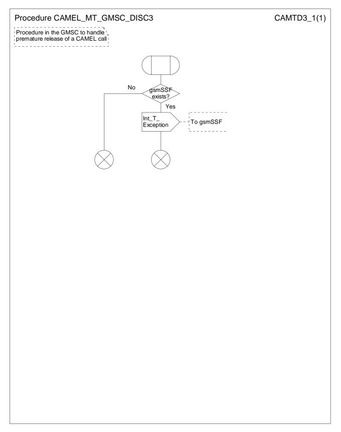
Figure 4.47-1: Procedure CAMEL\_MT\_GMSC\_DISC3 (sheet 1)
