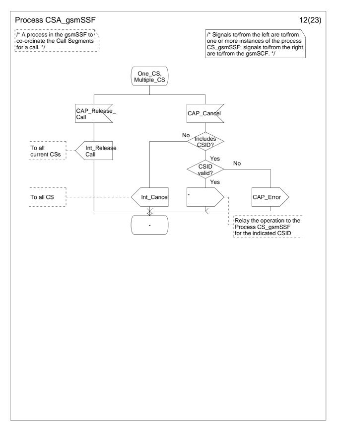
Figure 4.116-12: Process CSA\_gsmSSF (sheet 12)
