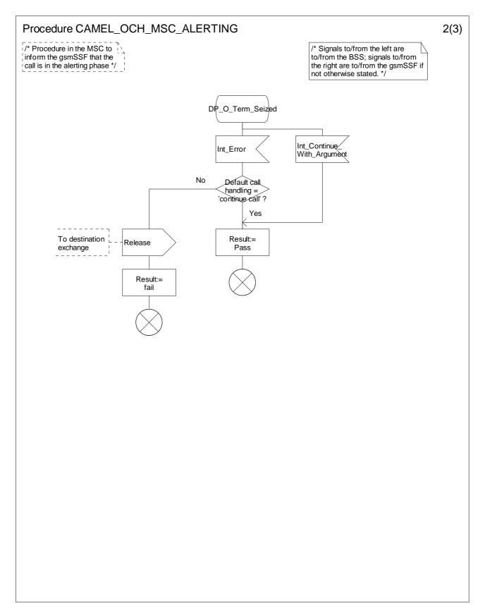
Figure 4.14-2: Procedure CAMEL\_OCH\_MSC\_ALERTING (sheet 2)
