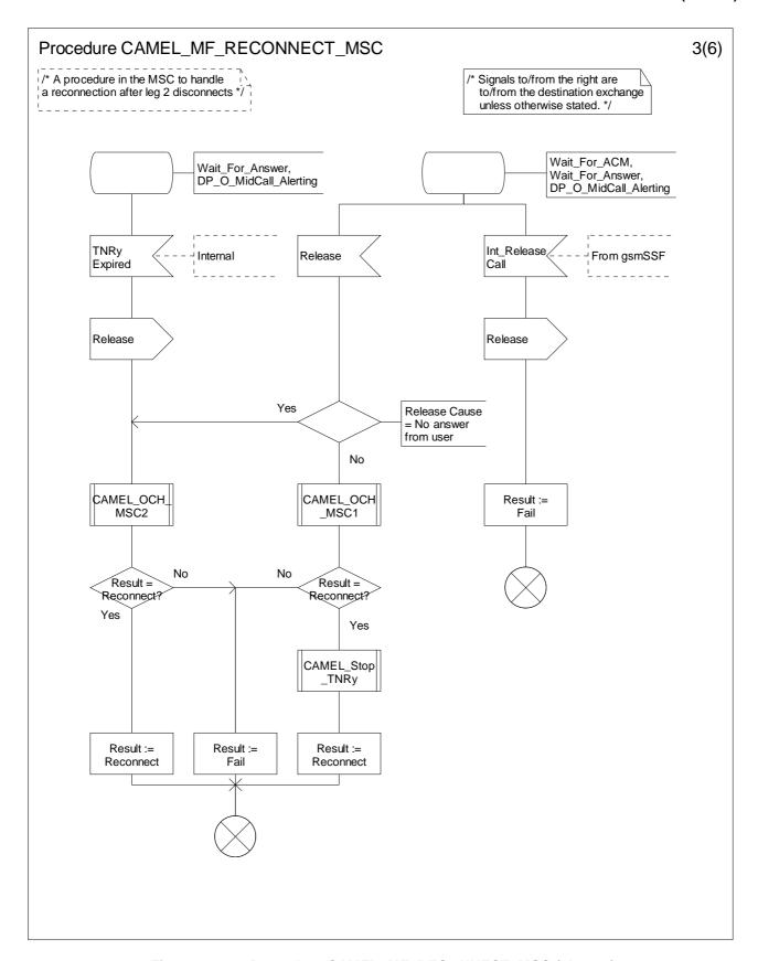
Figure 4.88-3: Procedure CAMEL\_MF\_RECONNECT\_MSC (sheet 3)
