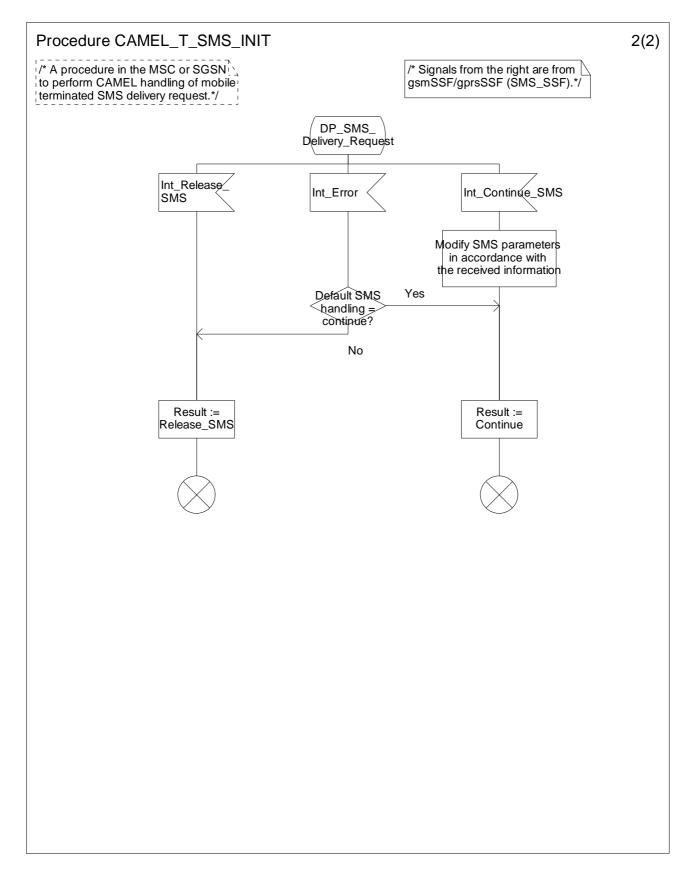
Figure 7.10-2: Procedure CAMEL\_T\_SMS\_INIT (sheet 2)
