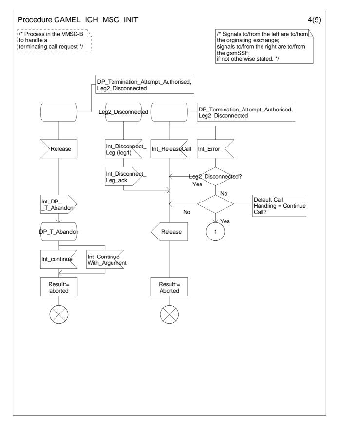
Figure 4.69-4: Procedure CAMEL\_ICH\_MSC\_INIT (sheet 4)
