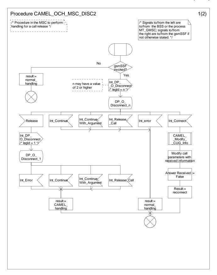
Figure 4.19-1: Procedure CAMEL\_OCH\_MSC\_DISC2 (sheet 1)
