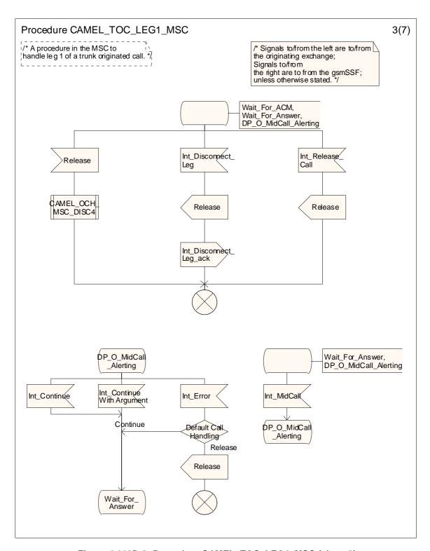
Figure 4.119D-3: Procedure CAMEL\_TOC\_LEG1\_MSC (sheet 3)
