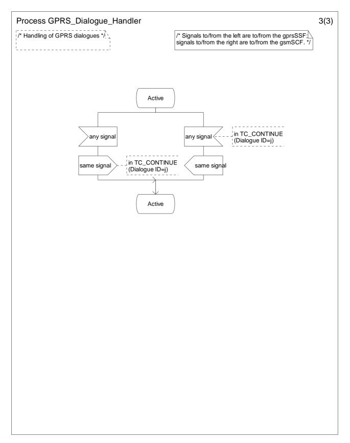
Figure 6.18-3: Process GPRS\_Dialogue\_Handler (sheet 3)
