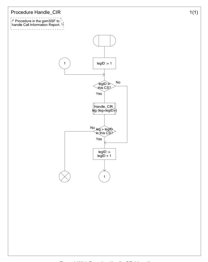
Figure 4.106-1: Procedure Handle\_CIR (sheet 1)
