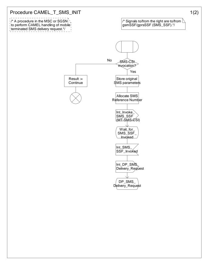
Figure 7.10-1: Procedure CAMEL\_T\_SMS\_INIT (sheet 1)
