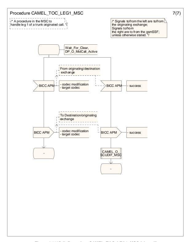
Figure 4.119D-7: Procedure CAMEL\_TOC\_LEG1\_MSC (sheet 7)
