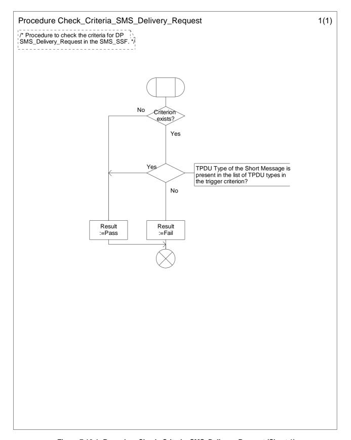
Figure 7.16-1: Procedure Check\_Criteria\_SMS\_Delivery\_Request (Sheet 1)
