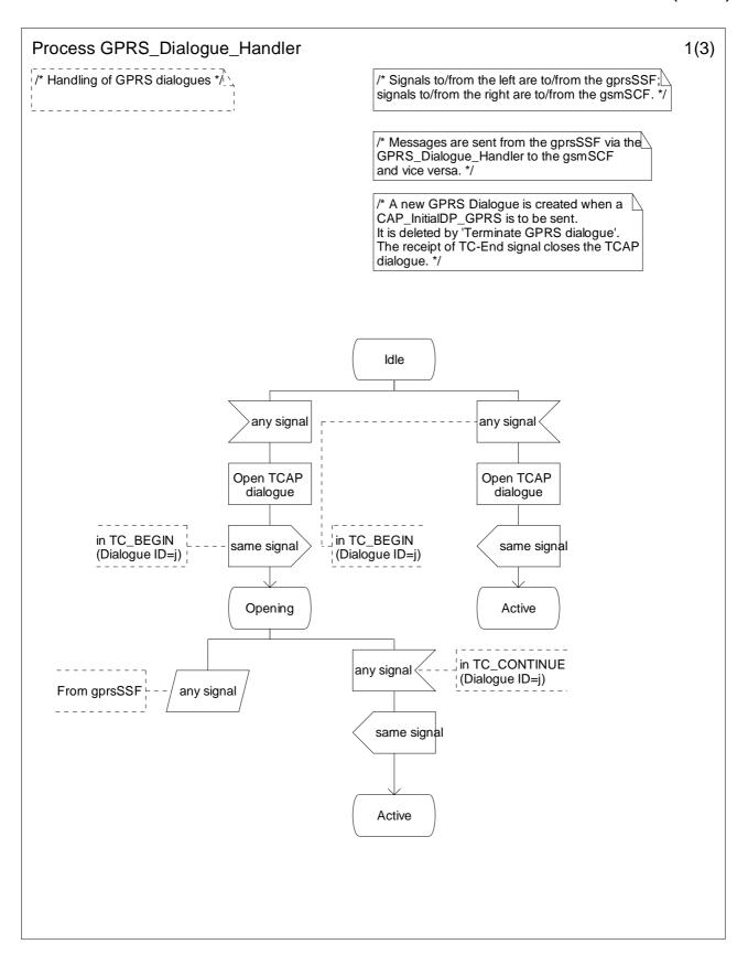
Figure 6.18-1: Process GPRS\_Dialogue\_Handler (sheet 1)
