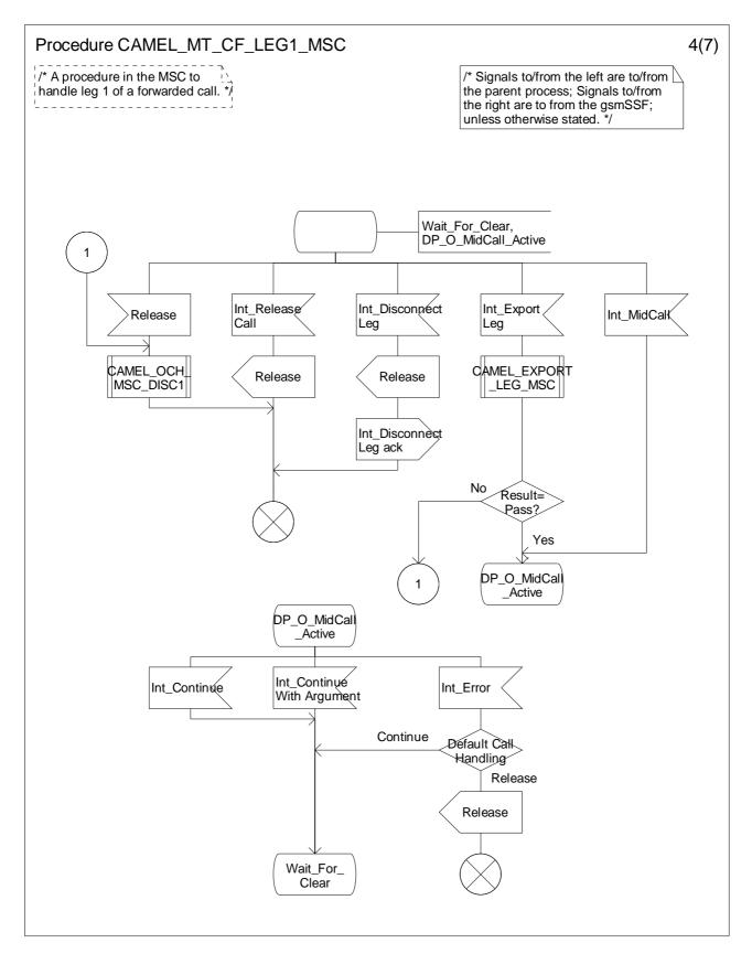
Figure 4.86-4: Procedure CAMEL\_MT\_CF\_LEG1\_MSC (sheet 4)
