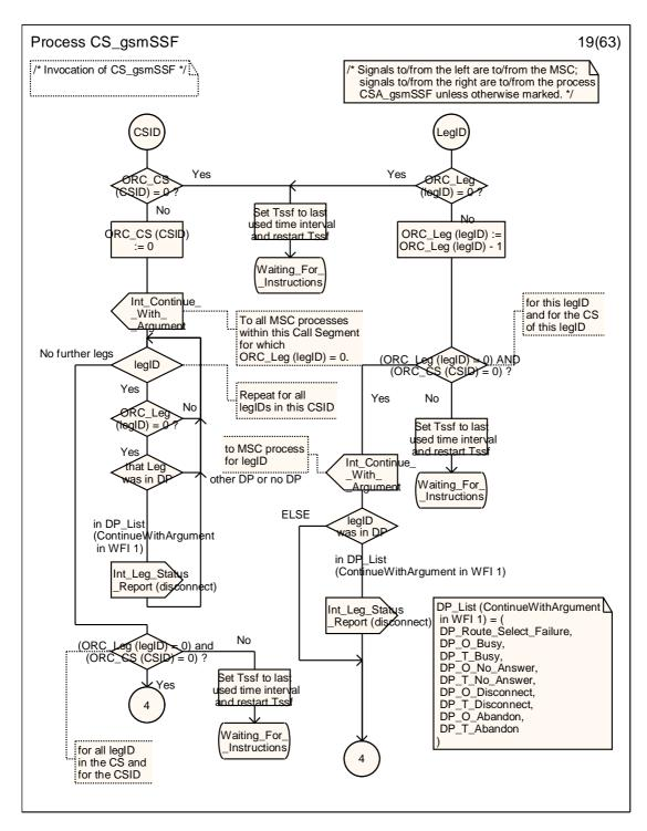
Figure 4.99-19: Process CS\_gsmSSF (sheet 19)
