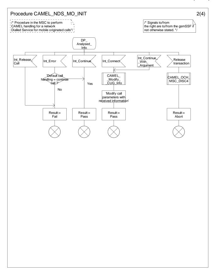
Figure 4.13-2: Procedure CAMEL\_NDS\_MO\_INIT (sheet 2)
