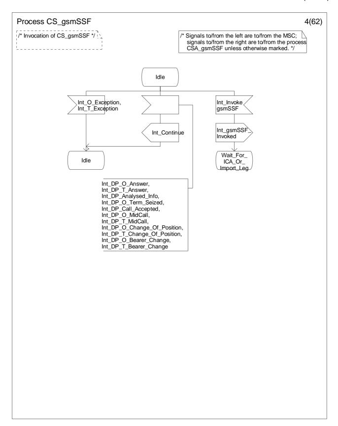
Figure 4.99-4: Process CS\_gsmSSF (sheet 4)
