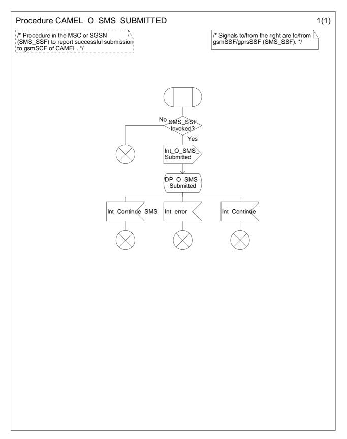
Figure 7.6-1: Procedure CAMEL\_O\_SMS\_SUBMITTED (sheet 1)
