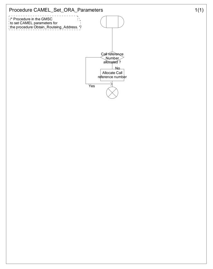
Figure 4.41-1: Procedure CAMEL\_Set\_ORA\_Parameters (sheet 1)
