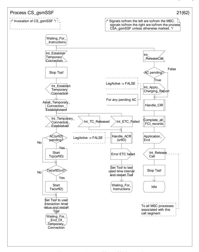
Figure 4.99-21: Process CS\_gsmSSF (sheet 21)
