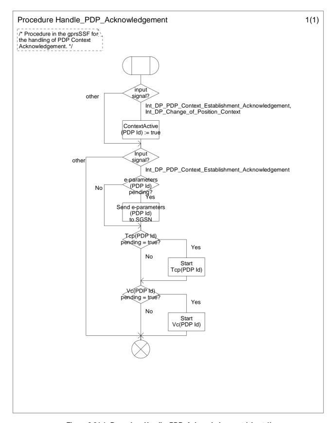
Figure 6.24-1: Procedure Handle\_PDP\_Acknowledgement (sheet 1)
