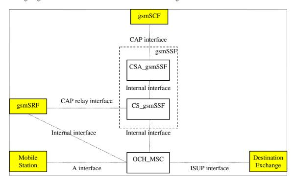
Figure 4.9-1: Outgoing case (gsmSSF relay)
