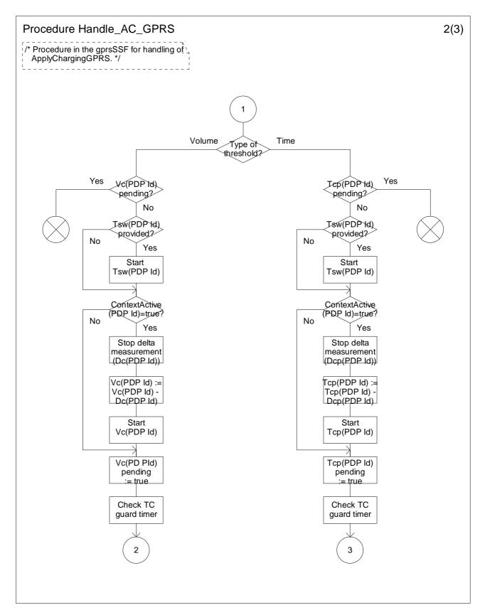
Figure 6.19-2: Procedure Handle\_AC\_GPRS (sheet 2)
