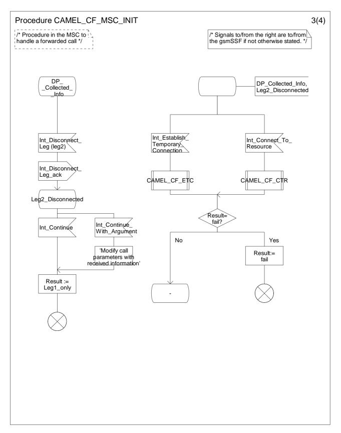
Figure 4.79-3: Procedure CAMEL\_CF\_MSC\_INIT (sheet 3)
