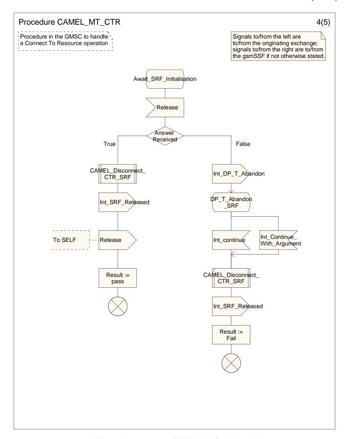
Figure 4.52-4: Procedure CAMEL\_MT\_CTR (sheet 4)
