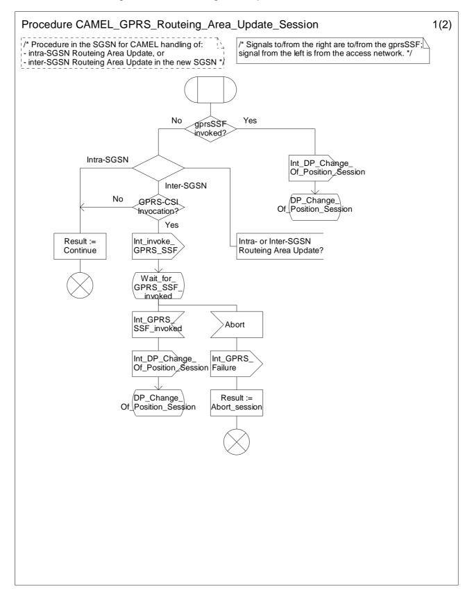
Figure 6.10-1: Procedure CAMEL\_GPRS\_Routeing\_Area\_Update\_Session (sheet 1)
