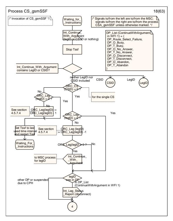
Figure 4.99-18: Process CS\_gsmSSF (sheet 18)
