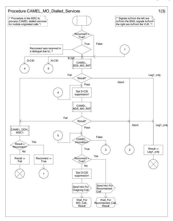
Figure 4.11-1: Procedure CAMEL\_MO\_Dialled\_Services (sheet 1)
