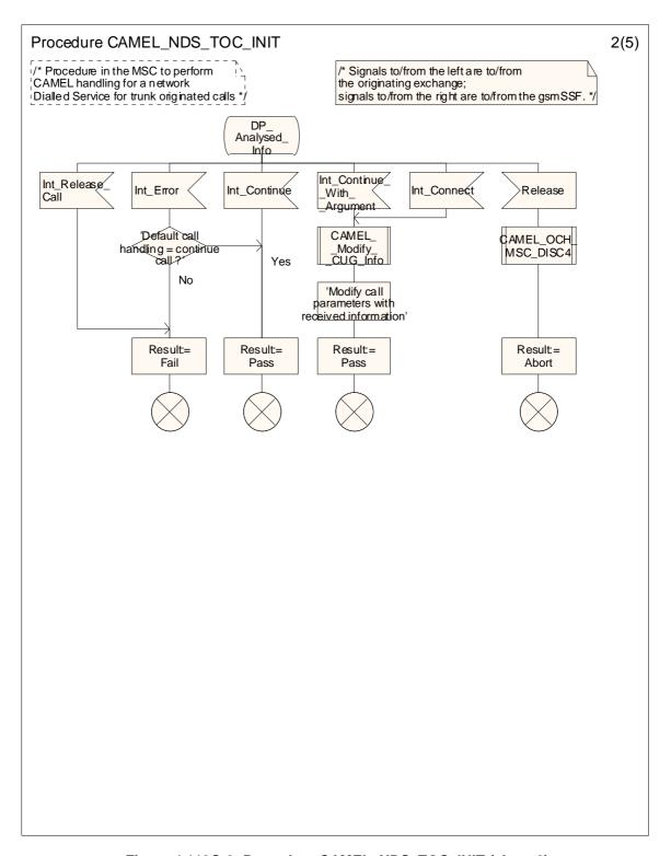
Figure 4.119C-2: Procedure CAMEL\_NDS\_TOC\_INIT (sheet 2)
