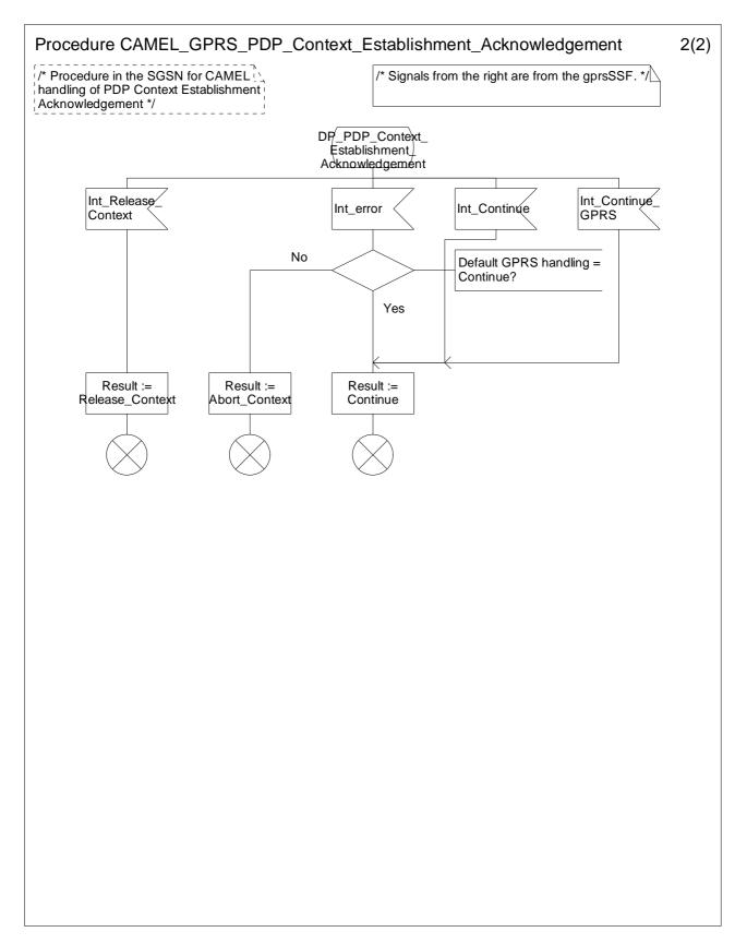
Figure 6.13-2: Procedure CAMEL\_GPRS\_PDP\_Context\_Establishment\_Acknowledgement (sheet 2)
