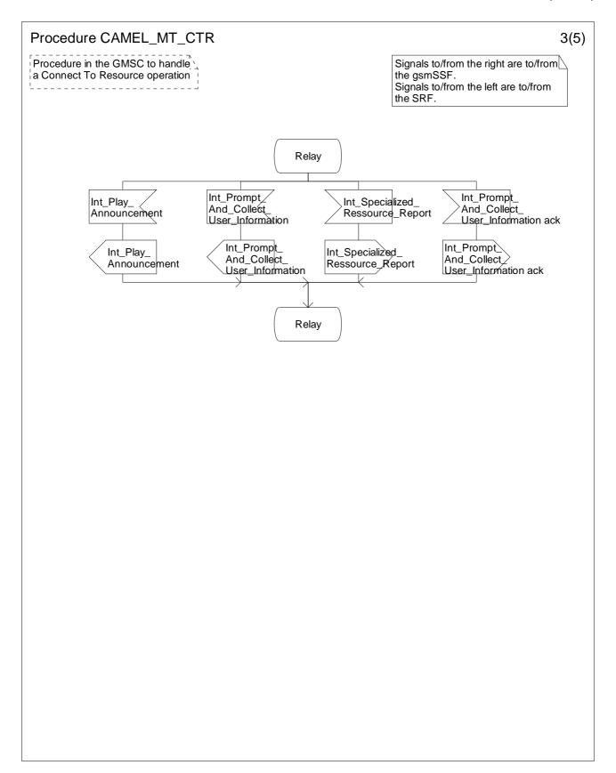
Figure 4.52-3: Procedure CAMEL\_MT\_CTR (sheet 3)
