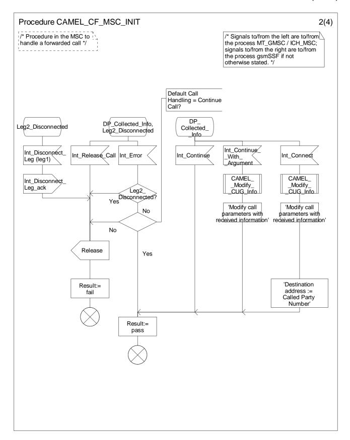
Figure 4.79-2: Procedure CAMEL\_CF\_MSC\_INIT (sheet 2)
