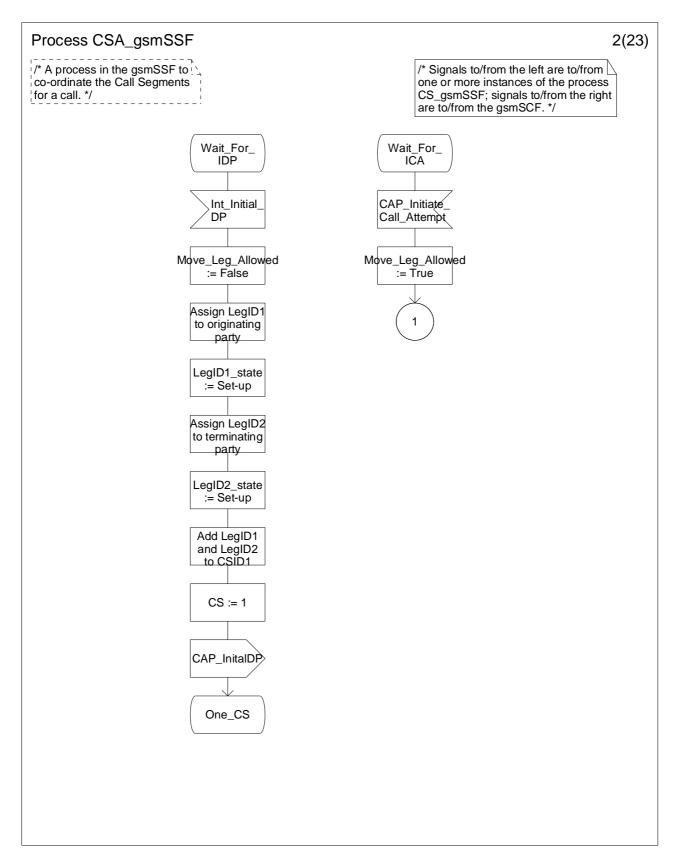
Figure 4.116-2: Process CSA\_gsmSSF (sheet 2)
