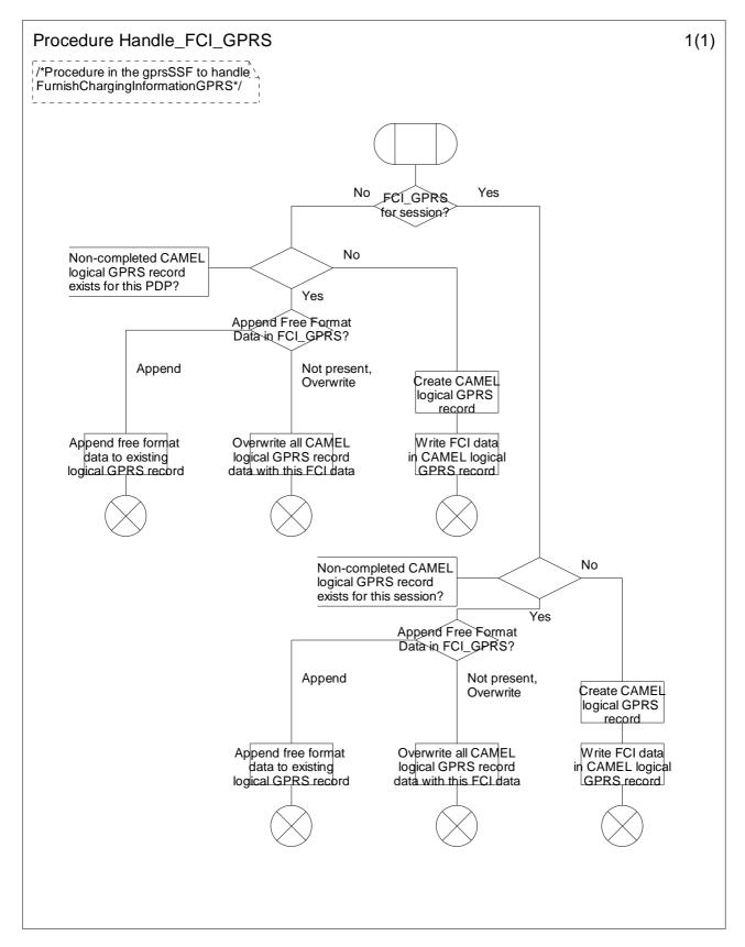
Figure 6.21-1: Procedure Handle\_FCI\_GPRS (sheet 1)
