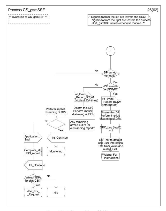
Figure 4.99-26: Process CS\_gsmSSF (sheet 26)
