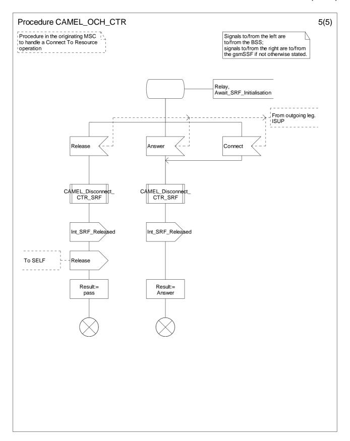
Figure 4.24-5: Procedure CAMEL\_OCH\_CTR (sheet 5)
