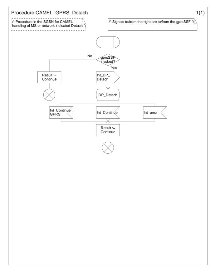
Figure 6.9-1: Procedure CAMEL\_GPRS\_Detach (sheet 1)
