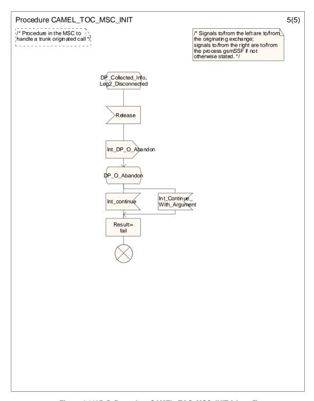
Figure 4.119B-5: Procedure CAMEL\_TOC\_MSC\_INIT (sheet 5)
