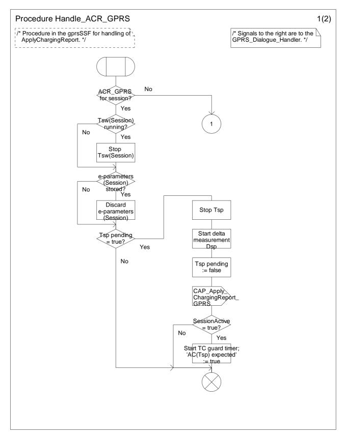
Figure 6.20-1: Procedure Handle\_ACR\_GPRS (sheet 1)
