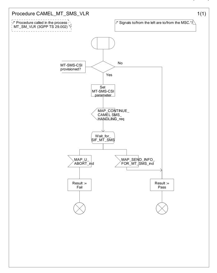
Figure 7.13-1: Procedure CAMEL\_MT\_SMS\_VLR (sheet 1)
