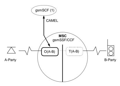
Figure 4.4.5.5.1: BCSM Scenario for Trunk Originated Call
