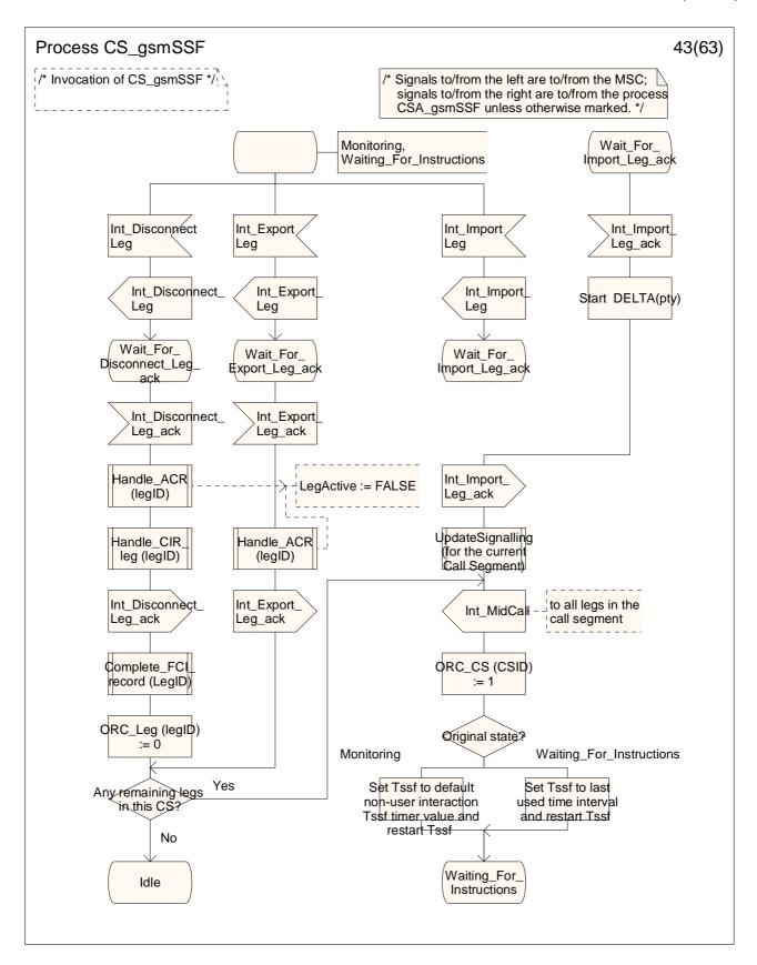
Figure 4.99-43: Process CS\_gsmSSF (sheet 43)
