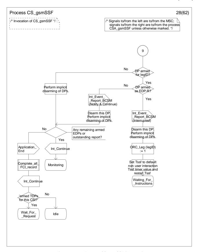
Figure 4.99-28: Process CS\_gsmSSF (sheet 28)
