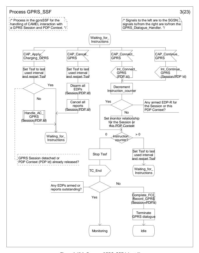
Figure 6.17-3: Process GPRS\_SSF (sheet 3)
