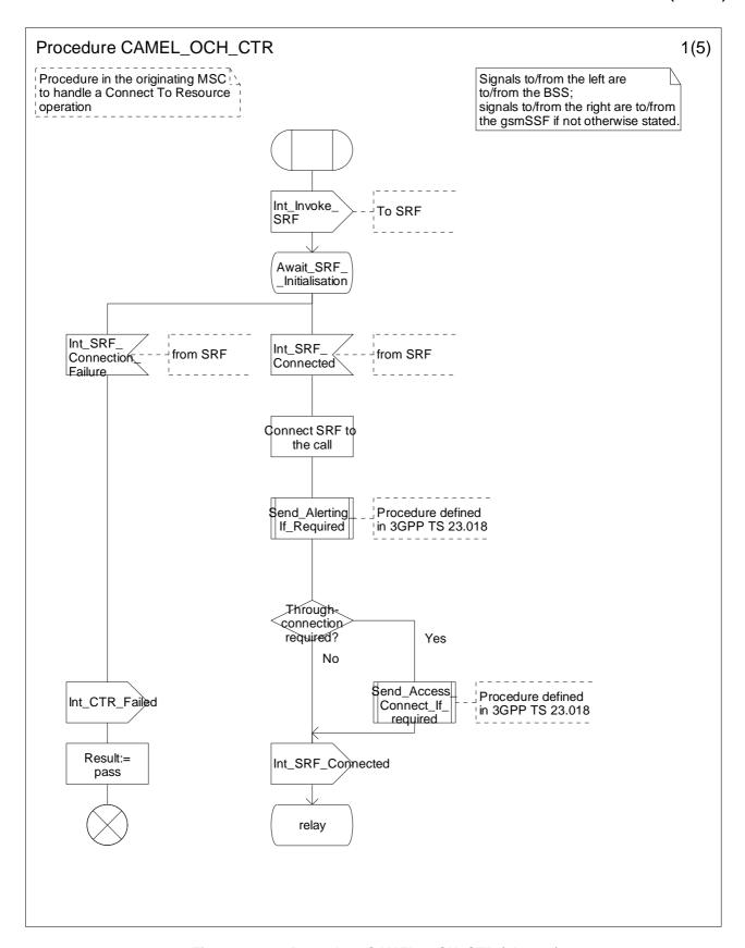
Figure 4.24-1: Procedure CAMEL\_OCH\_CTR (sheet 1)
