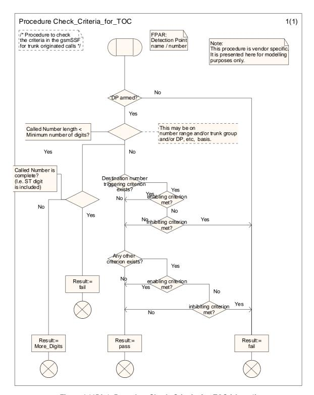
Figure 4.115A-1: Procedure Check\_Criteria\_for\_TOC (sheet 1)
