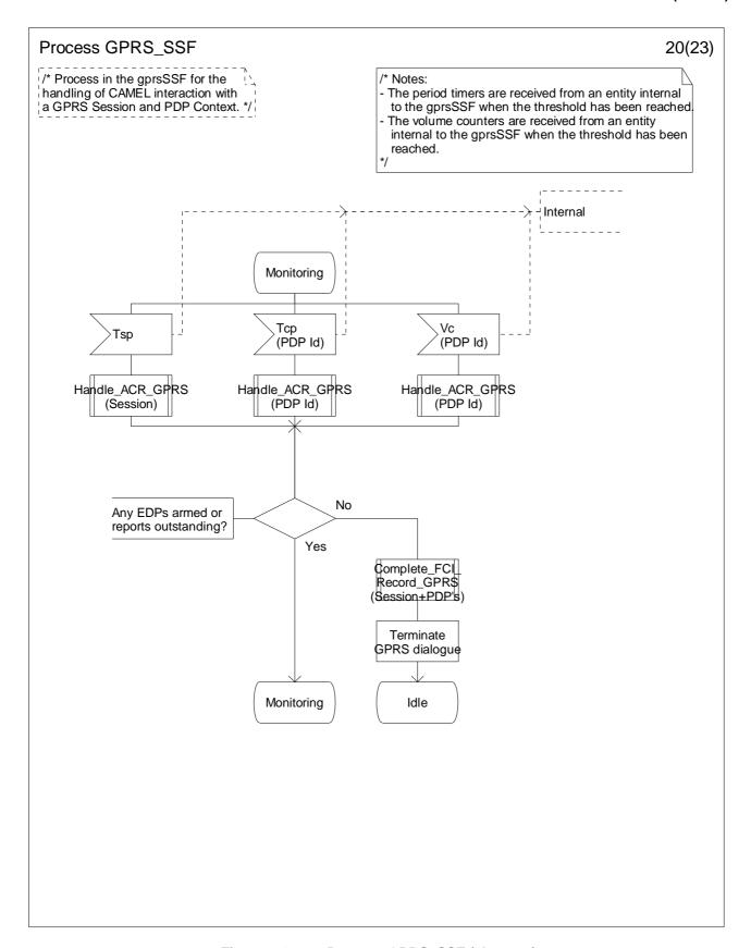
Figure 6.17-20: Process GPRS\_SSF (sheet 20)
