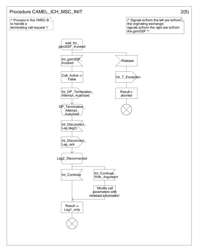
Figure 4.69-2: Procedure CAMEL\_ICH\_MSC\_INIT (sheet 2)
