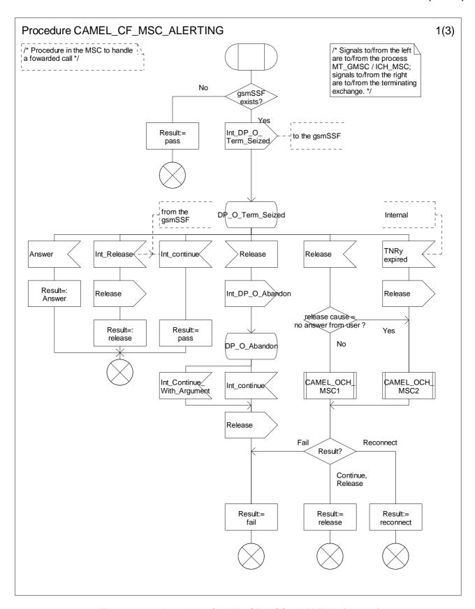
Figure 4.82-1: Procedure CAMEL\_CF\_MSC\_ALERTING (sheet 1)
