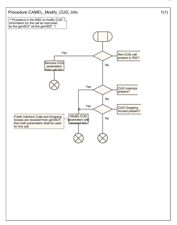
Figure 4.28-1: Procedure CAMEL\_Modify\_CUG\_Info (sheet 1)
