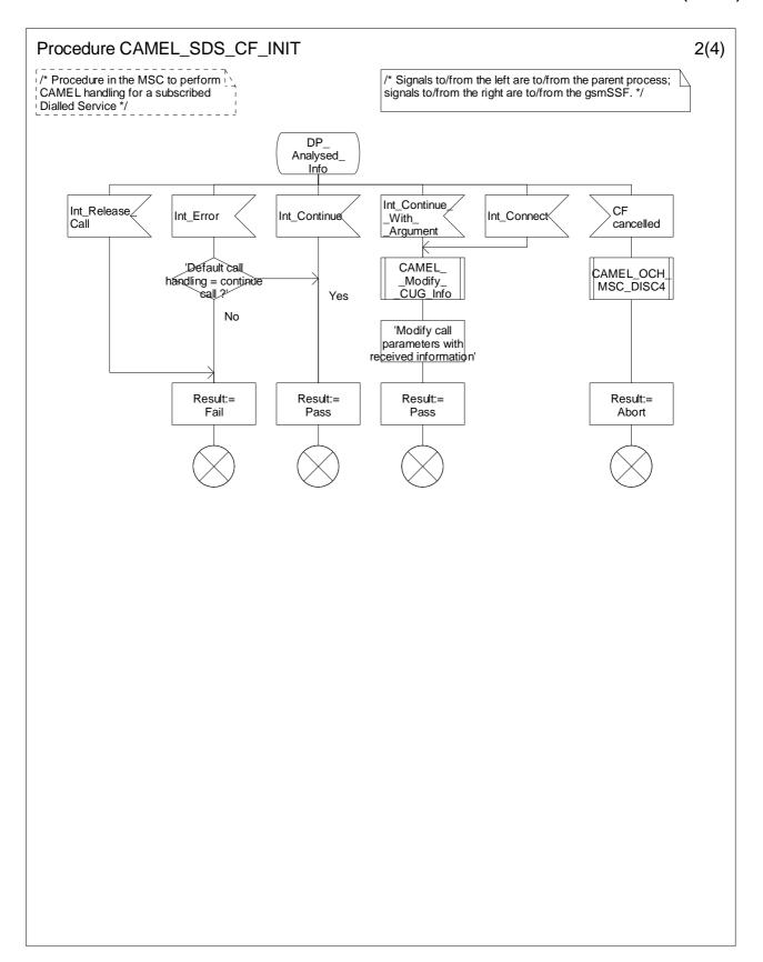
Figure 4.80-2: Procedure CAMEL\_SDS\_CF\_INIT (sheet 2)
