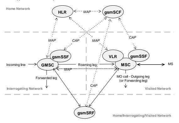
Figure 4.1: Functional architecture for support of CAMEL
