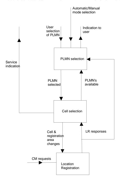
Figure 1: Overall Idle Mode process
