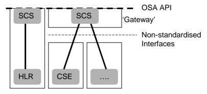
Figure 5: Hybrid implementation (combination of option 1 and 2)
