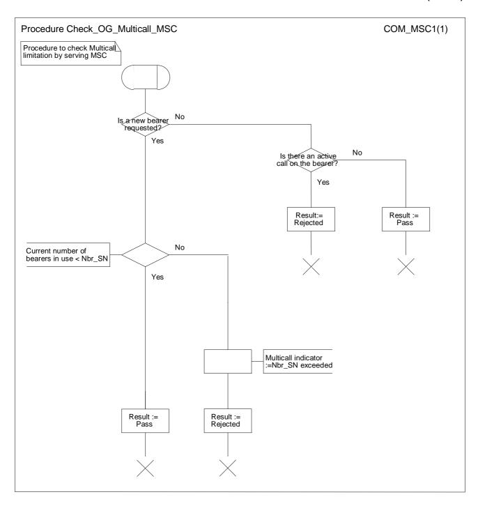
Figure 8: Procedure Check\_OG\_Multicall\_MSC
