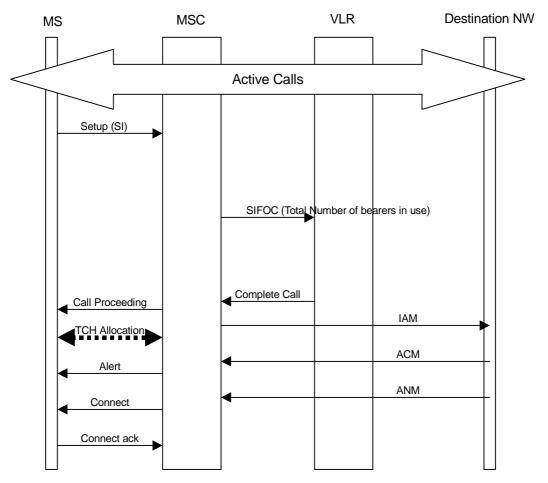
Figure 5: Information flow for mobile originating call
