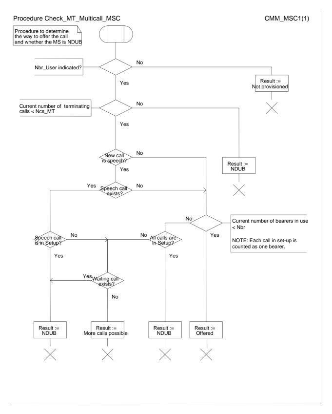
Figure 10: Procedure Check\_MT\_Multicall\_MSC
