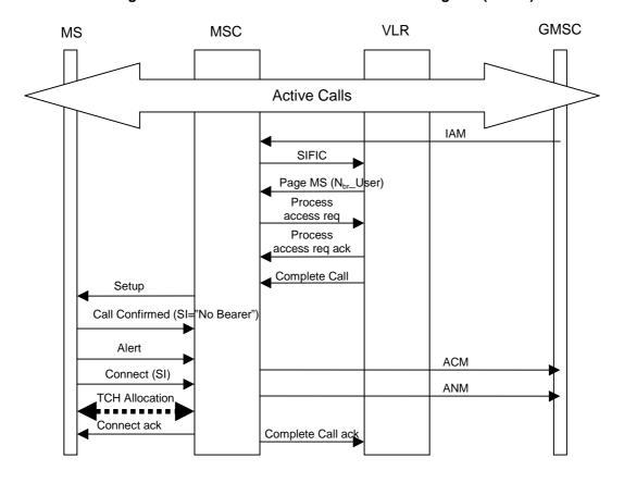
Figure 7: Information flow for mobile terminating call (Case2)
