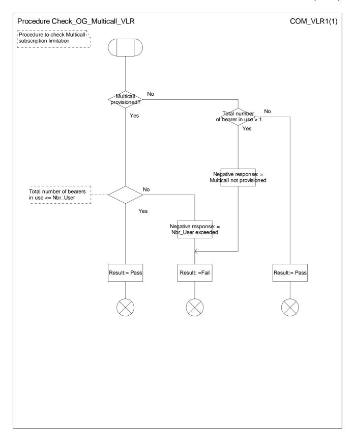
Figure 9: Procedure Check\_OG\_Multicall\_VLR
