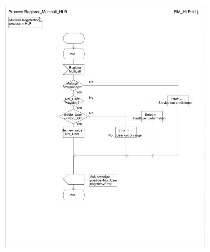
Figure 2: Process Register\_Multicall\_HLR
