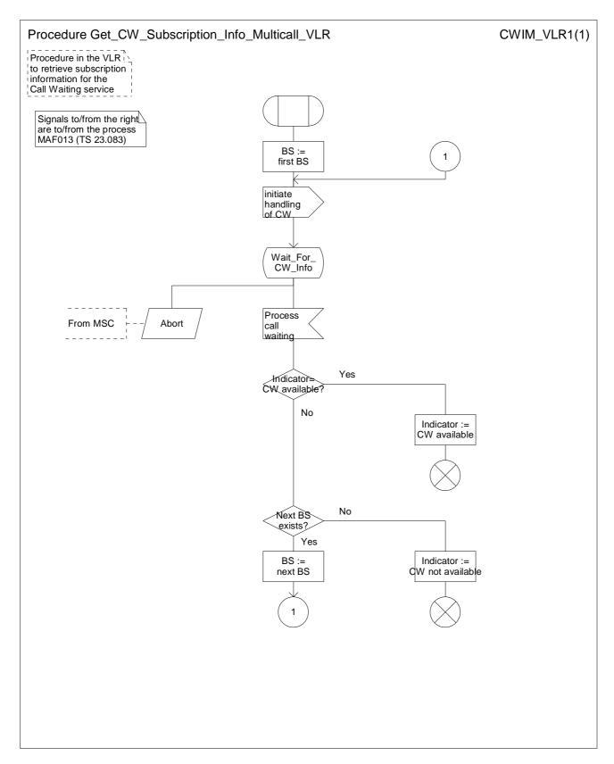
Figure 13: Procedure Get\_CW\_Subscription\_Info\_Multicall\_VLR
