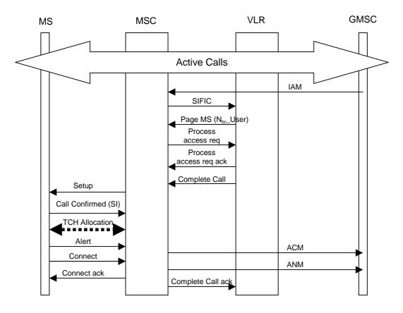
Figure 6: Information flow for mobile terminating call (Case1)
