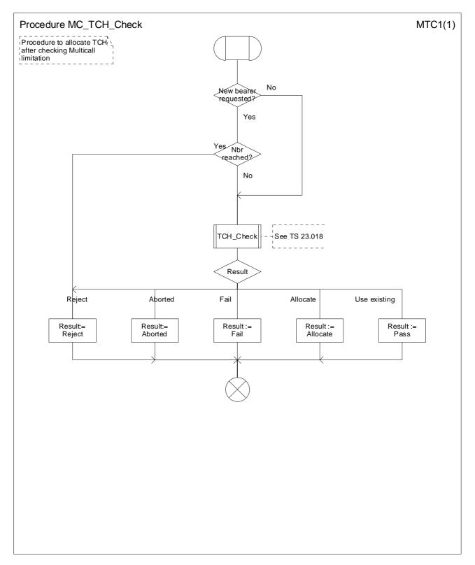
Figure 12: Procedure MC\_TCH\_Check
