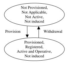
Figure 14: State transition model for Multicall
