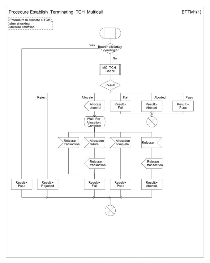
Figure 11: Procedure Establish\_Terminating\_TCH\_Multicall
