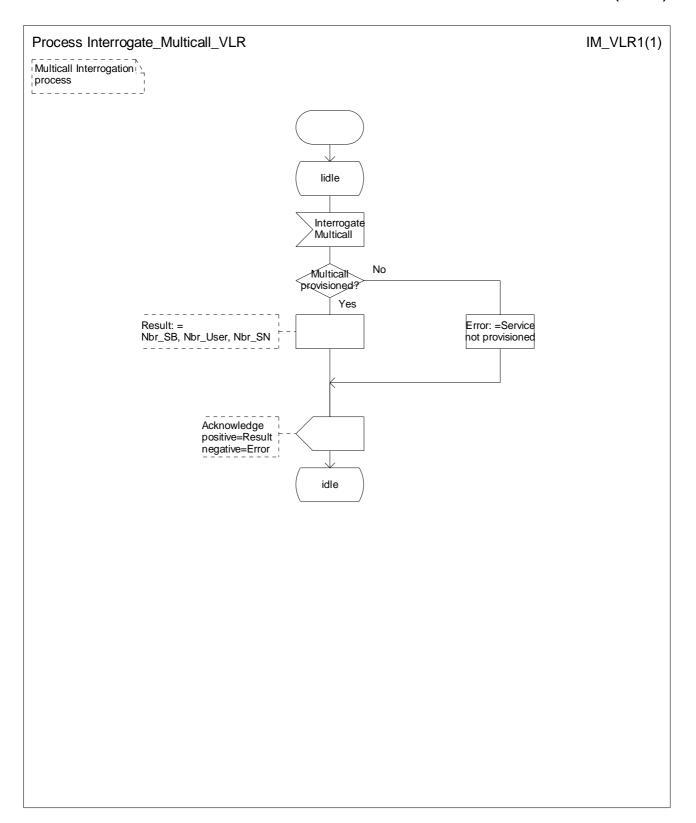
Figure 4: Process Interrogate\_Multicall\_VLR
