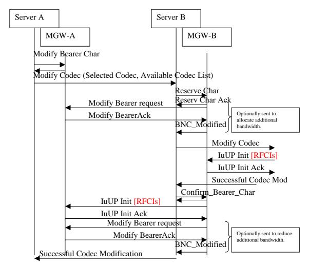
Figure 5.8.3.4/1: Successful Codec Modification including luFP
