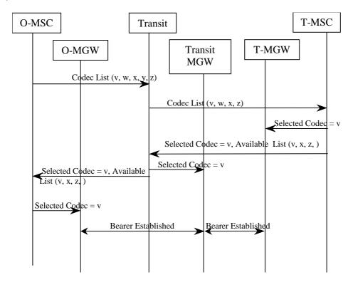
Figure 5.2/1. Basic Codec Negotiation Sequence
