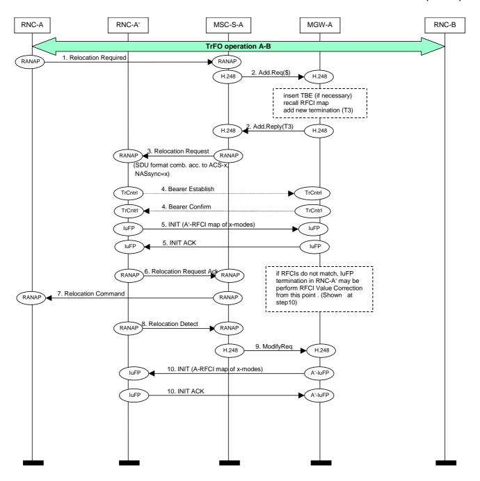
Figure 6.2/2:SRNS Relocation and TrFO. Flow chart part 1
