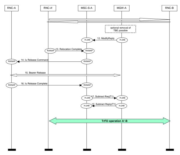
Figure 6.2/3 SRNS Relocation and TrFO. Flow chart part 2
