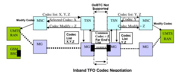
Figure 5.5/3: TFO support by OoBTC signalling
