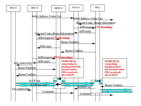
Figure 5.4.1/1: lu Framing Protocol Establishment, Forward Bearer
