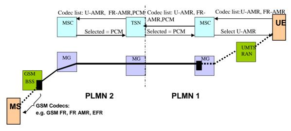
Figure 5.5/2: UMTS to GSM interworking
