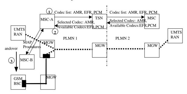
Figure 6.5/2: Inter-MSC, UMTS to GSM handover
