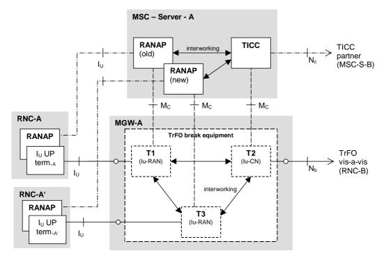
Figure 6.2/1: Configuration during SRNS Relocation
