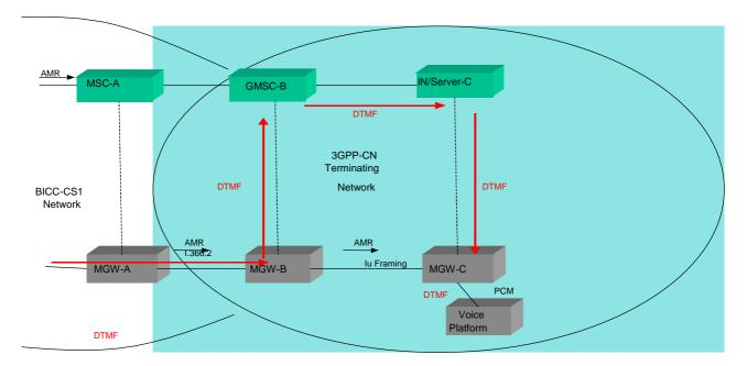
Figure 5.9/1:DTMF received inband from external network
