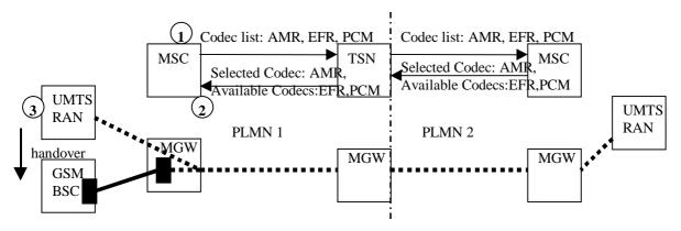
Figure 6.5/1: UMTS to GSM Inter-System Handover
