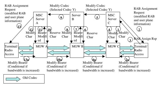
Figure 5.8.1/1: Codec Modification Control Procedures
