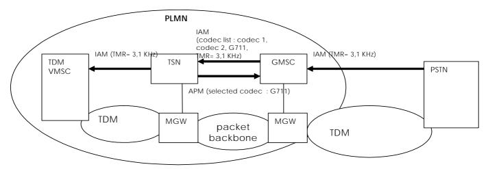
Figure 6.12.2/1. Handling of possible data call at transit exchange between TDM and packet backbone
