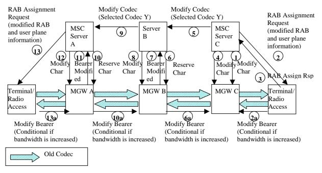
Figure 5.8.1/1: Codec Modification Control Procedures
