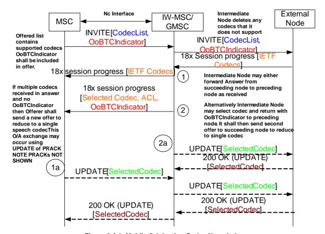
Figure 9.6.1: Mobile Originating Codec Negotiation
