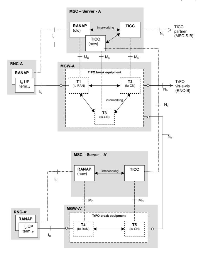
Figure 6.2/4: Configuration during inter-MSC SRNS Relocation
