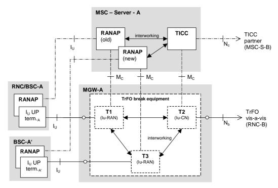
Figure 6.10/1: Configuration during intra-MSC SRNS Relocation towards GERAN lu-mode
