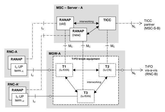
Figure 6.2/1: Configuration during intra-MSC SRNS Relocation
