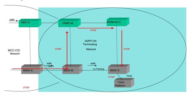
Figure 5.9/1:DTMF received inband from external network
