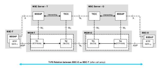
Figure 6.13/1: Configuration during Call Setup of a Mobile to Mobile Call in GERAN AoIP mode
