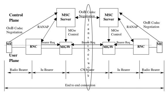
Figure 5.1/1. Basic Architecture for UMTS to UMTS TrFO Connection
