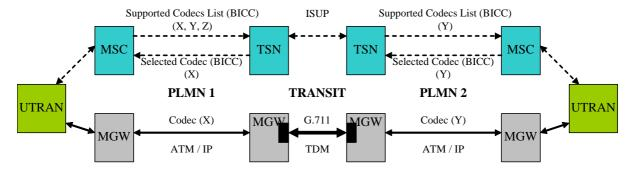
Figure 5.5/1: Cascaded TrFO & Transcoding
