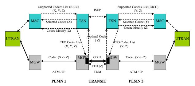
Figure 5.5/3: TFO support by OoBTC signalling
