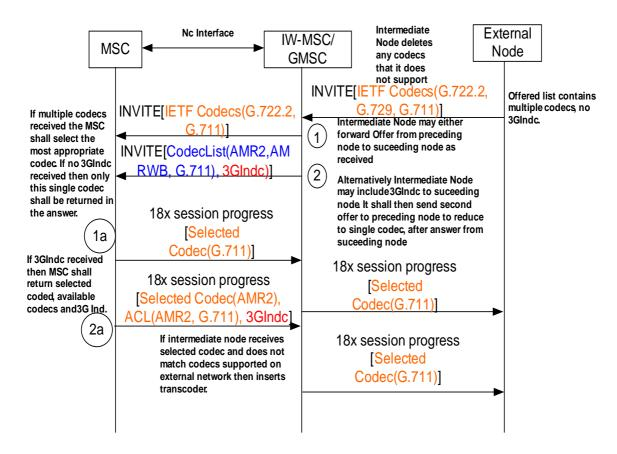
Figure 9.6.7: Mobile Terminating Codec Negotiation with specific codec examples
