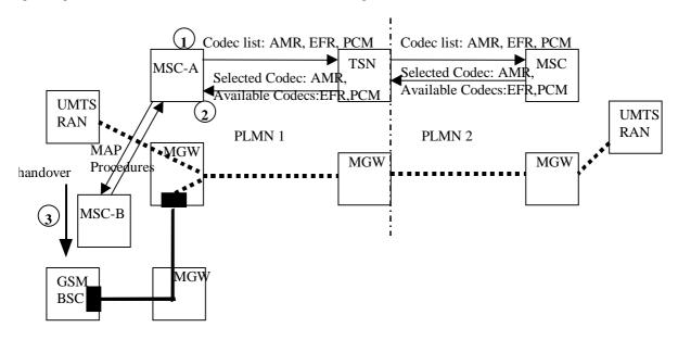
Figure 6.5/2: Inter-MSC, UMTS to GSM handover
