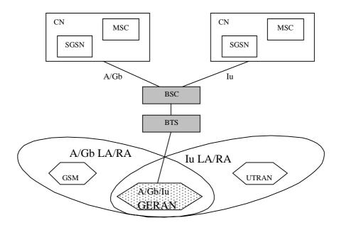
Figure 6.2b: Combined A/Gb/lu Cell with Separate CN
