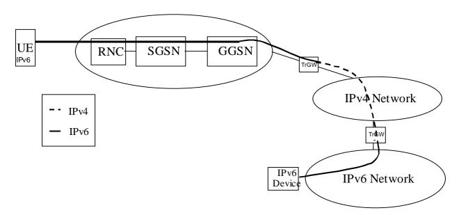
Figure 5-3 IPv6 mobile connected to an IPv6 device via an IPv4 network
