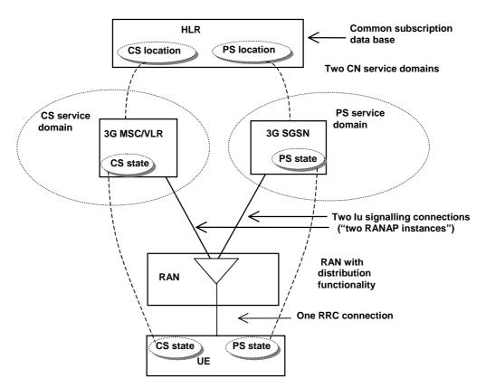
Figure 6.1: Overview of the UE registration and connection principles for the separate CN architecture case
