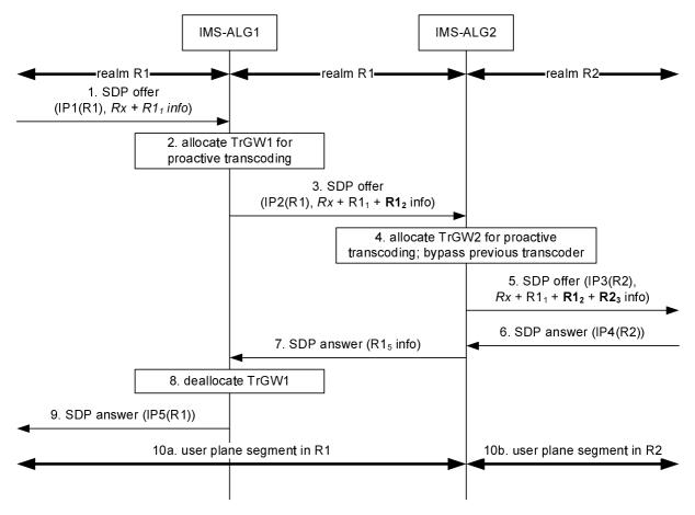
Figure Q.8: IMS-ALG replaces prior proactive transcoder
