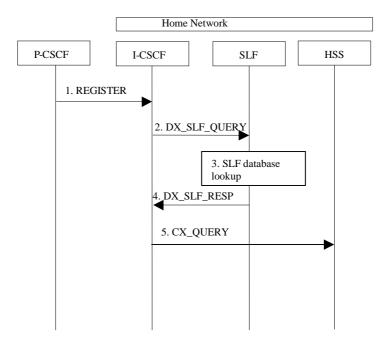
Figure 5.20: SLF on register (1st case)
