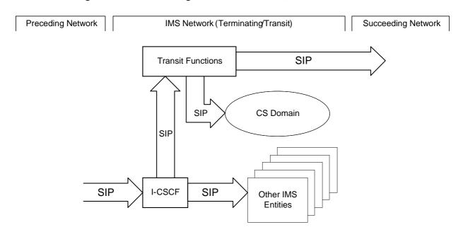
Figure 5.50b: Terminating/Transit IMS network, I-CSCF first
