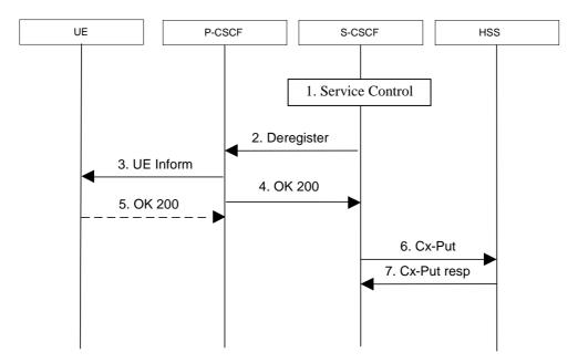
Figure 5.5a: Network initiated application de-registration, service platform
