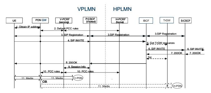
Figure M.1.1.2: Example scenario with P-CSCF located in visited network
