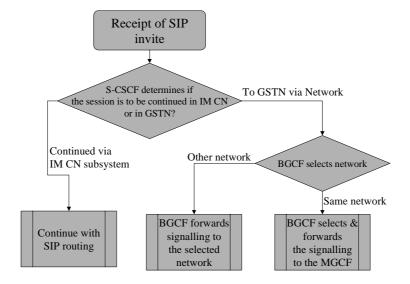
Figure 5.6: Network based PSTN interworking breakout process
