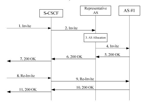
Figure J.2.2: Bypassing Representative AS procedure
