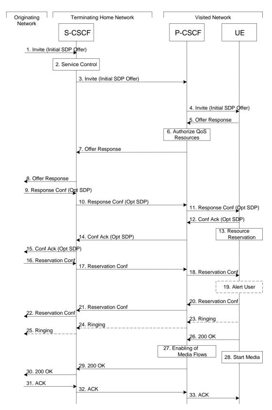
Figure 5.17: Mobile termination procedure - roaming
