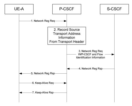
Figure G.7: Flow Establishment Procedures for Outbound
