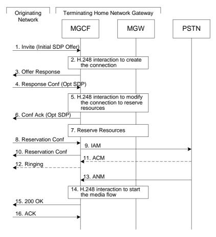
Figure 5.19: PSTN termination procedure
