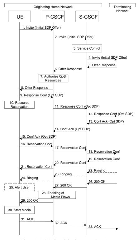
Figure 5.15: Mobile origination procedure - home
