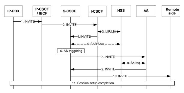
Figure S.2-1: Originating procedures for IP-PBXs using static mode business trunking and served by the S-CSCF
