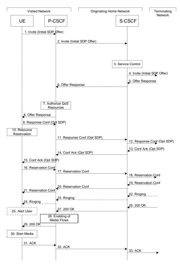
Figure 5.14: Mobile origination procedure - roaming
