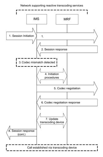
Figure P.1.3.3-1: Reactive transcoding triggering logic
