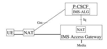
Figure G.1: Reference model for IMS access when both the signalling and media traverses NAT
