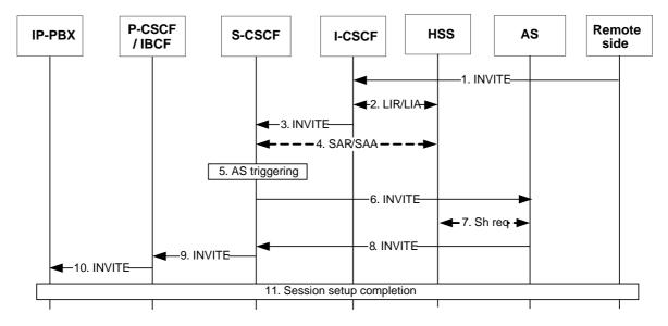
Figure S.2-3: Terminating procedures for IP-PBXs using static mode business trunking and served by the S-CSCF
