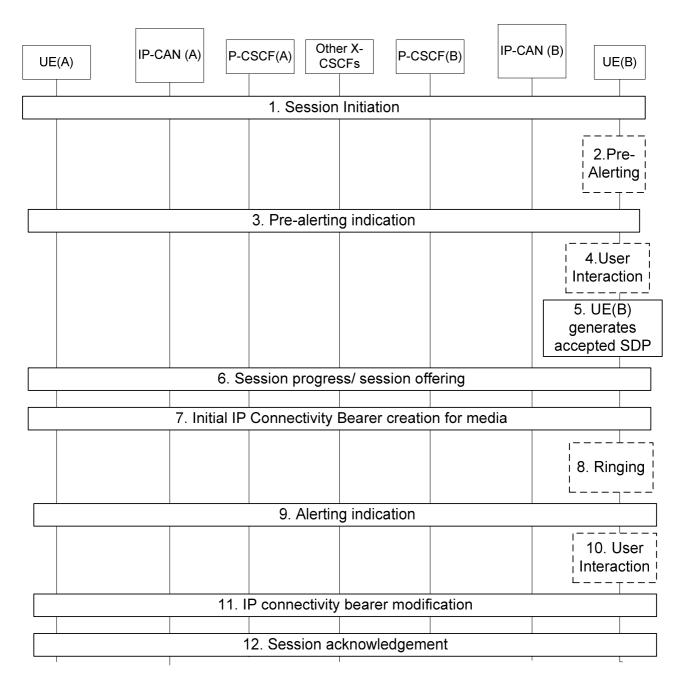
Figure 5.7: Bearer establishment showing optional pre-alerting
