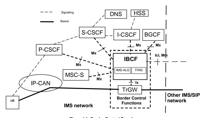
Figure I.1: Border Control Functions
