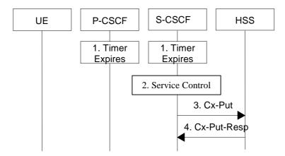
Figure 5.4: Network initiated application de-registration, registration timeout
