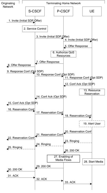
Figure 5.18: Mobile termination procedure - home
