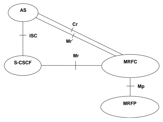
Figure 4.7: Architecture of MRF
