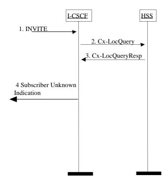
Figure 5.45: HSS determination of unknown user
