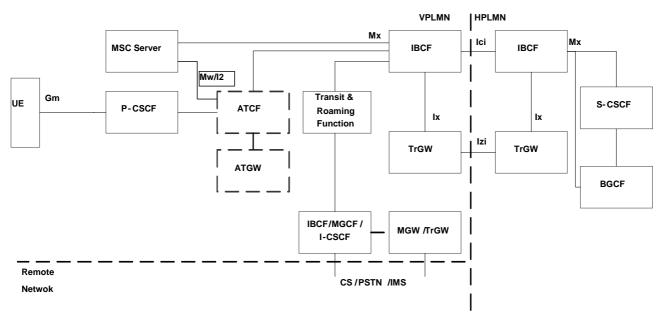
Figure M.3.1.2: Overall architecture for IMS Local Breakout with P-CSCF located in visited network and with VPLMN loopback possibility
