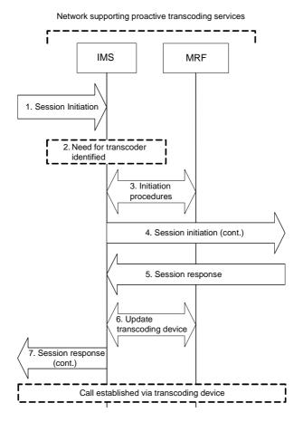
Figure P.1.3.2-1: Proactive transcoding triggering logic
