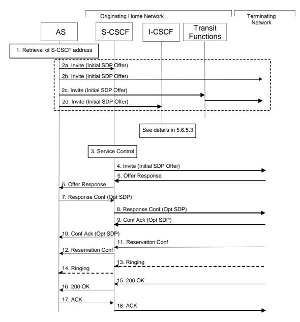
Figure 5.16b: Application Server origination procedure
