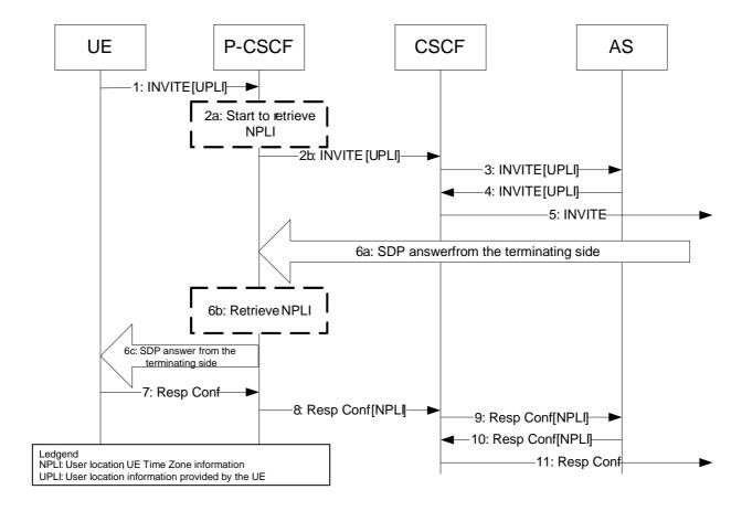
Figure R.3-1: Mobile origination (user location and/or UE Time Zone information included within Response Confirmation)
