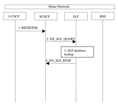
Figure 5.20a: SLF on register (2<sup>nd</sup> case)
