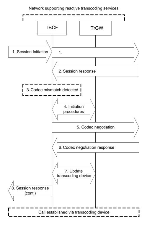
Figure I.5: Reactive transcoding invocation
