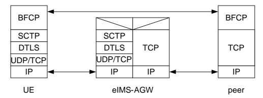
Figure U.1.5.2-1: Protocol architecture for BFCP
