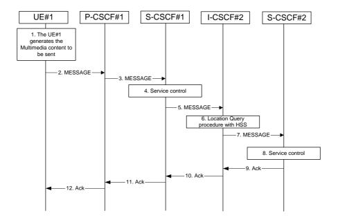
Figure 5.48: Immediate messaging to unregistered Public User Identity, service control invoked
