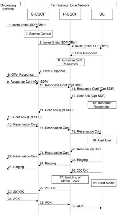
Figure 5.18: Mobile termination procedure - home
