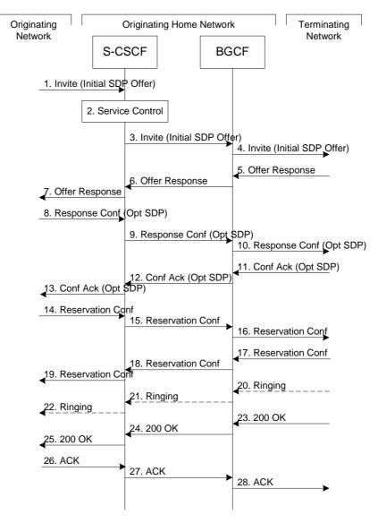
Figure 5.12: Serving to PSTN procedure - same operator
