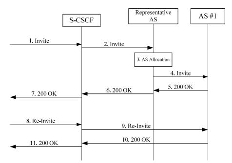
Figure J.2.2: Bypassing Representative AS procedure
