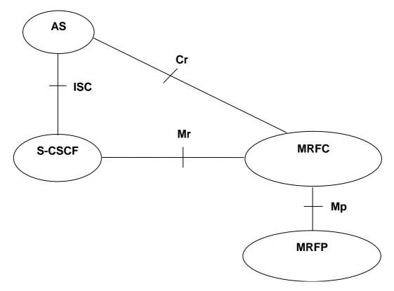
Figure 4.7: Architecture of MRF
