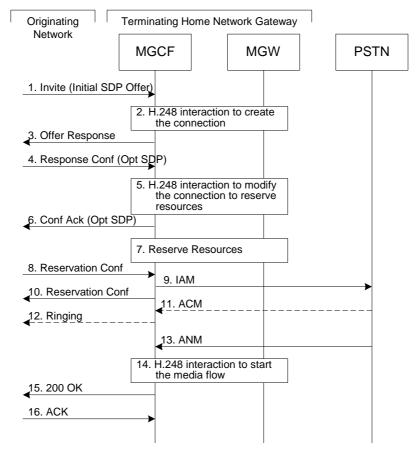
Figure 5.19: PSTN termination procedure
