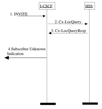
Figure 5.45: HSS determination of unknown user
