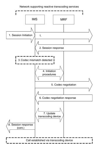
Figure P.1.3.3-1: Reactive transcoding triggering logic
