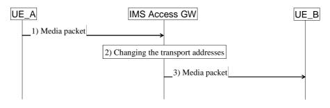
Figure G.5: Packet forwarding in the IMS Access Gateway
