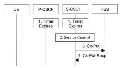
Figure 5.4: Network initiated application de-registration, registration timeout
