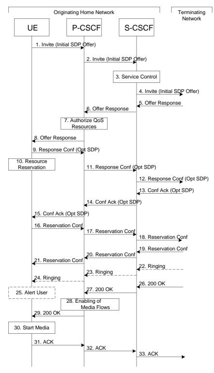
Figure 5.15: Mobile origination procedure - home
