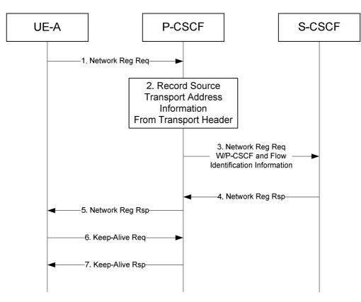
Figure G.7: Flow Establishment Procedures for Outbound
