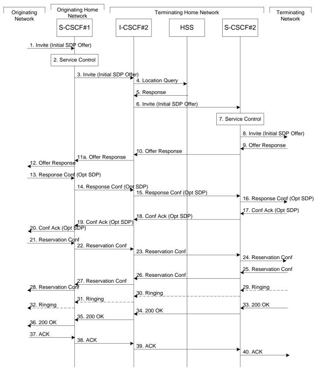
Figure 5.11: Serving to serving procedure - same operator
