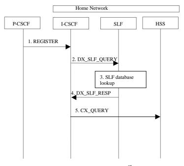
Figure 5.20: SLF on register (1<sup>st</sup> case)
