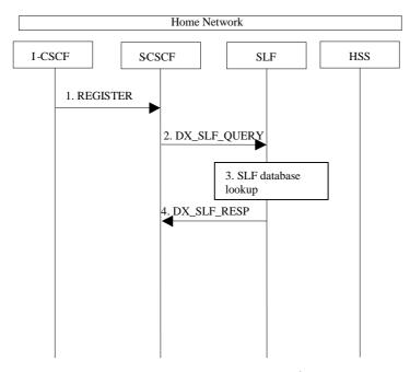
Figure 5.20a: SLF on register (2<sup>nd</sup> case)
