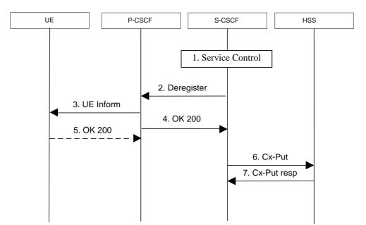
Figure 5.5a: Network initiated application de-registration, service platform
