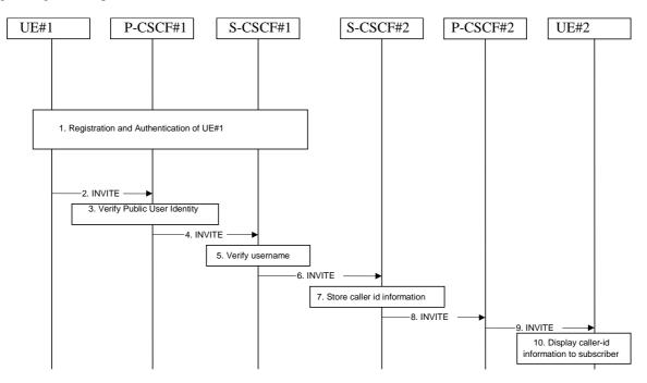
Figure 5.34: Providing the authenticated Identity of the originating party
