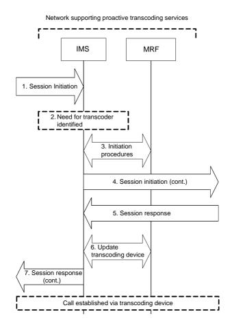
Figure P.1.3.2-1: Proactive transcoding triggering logic
