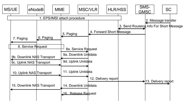
Figure 8.2.4-1: Mobile terminating SMS in idle mode
