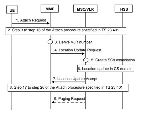
Figure 5.2-1: Attach Procedure
