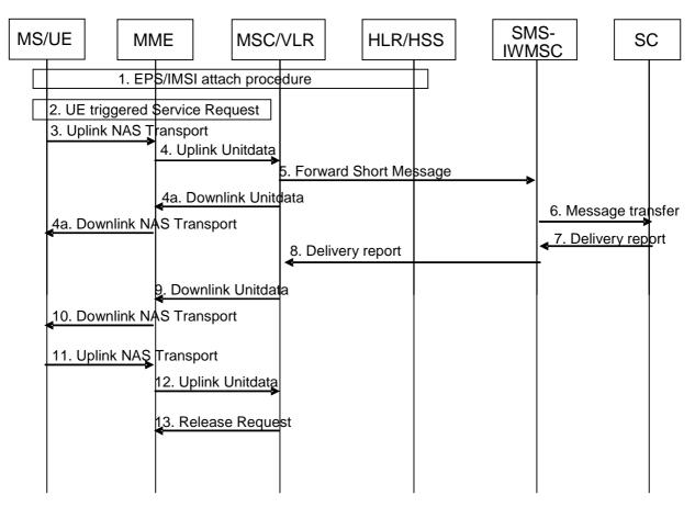
Figure 8.2.2-1: Mobile originating SMS in idle mode
