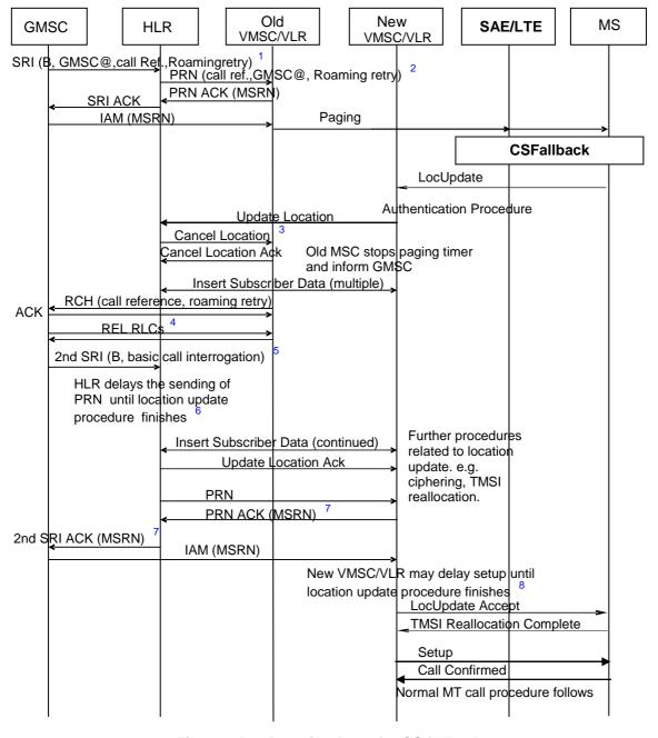
Figure 7.5-1: Roaming Retry for CS fallback
