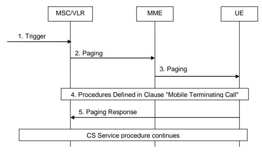
Figure 8.4.2-1: NW-Initiated CS Service procedure
