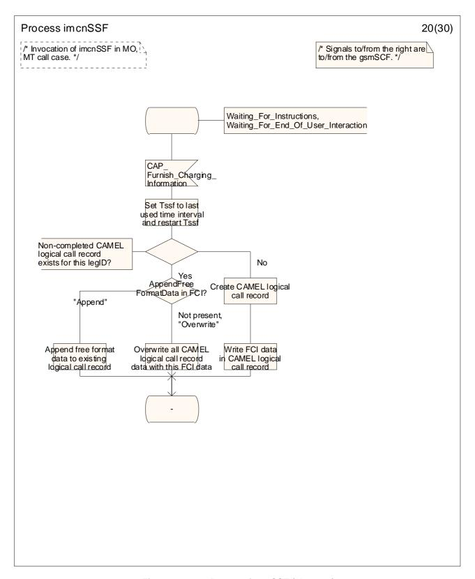
Figure 4.34-20: Process imcnSSF (sheet 20)
