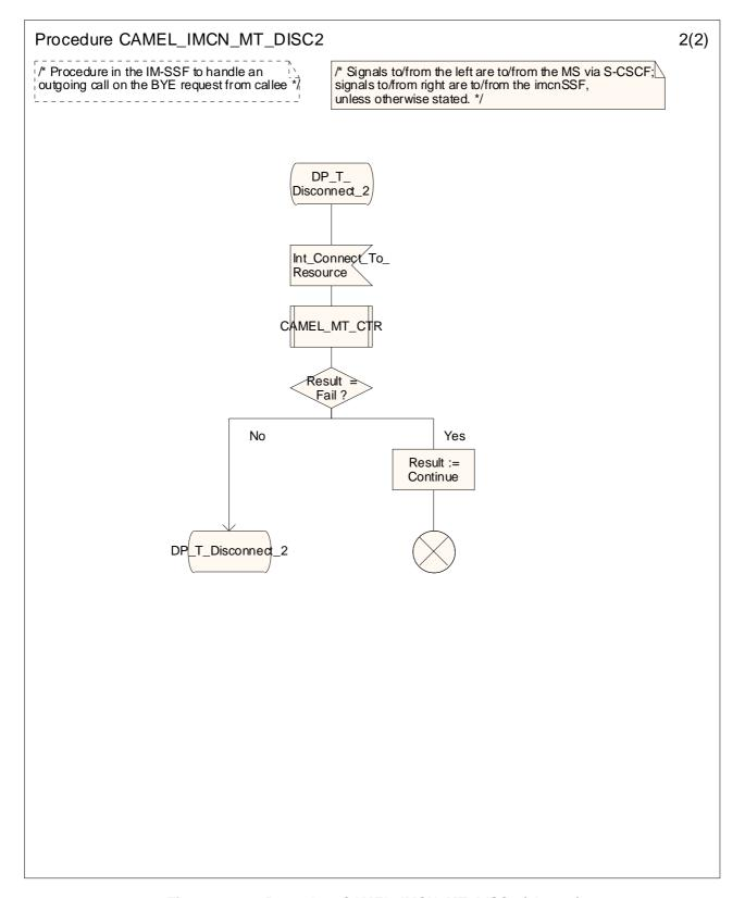
Figure 4.30-2: Procedure CAMEL\_IMCN\_MT\_DISC2 (sheet 2)
