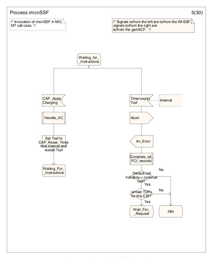
Figure 4.34-5: Process imcnSSF (sheet 5)
