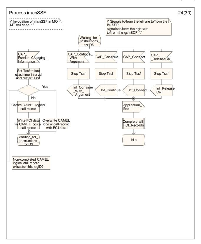
Figure 4.34-24: Process imcnSSF (sheet 24)
