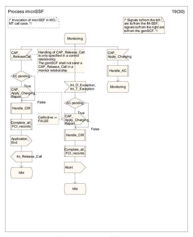
Figure 4.34-19: Process imcnSSF (sheet 19)
