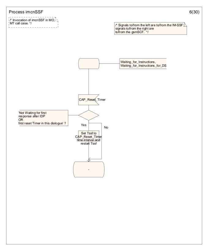
Figure 4.34-6: Process imcnSSF (sheet 6)
