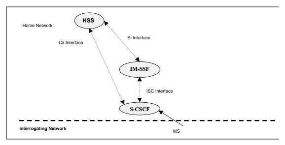
Figure 4.1: Functional architecture for support of CAMEL when mobile registers for IP Multimedia session
