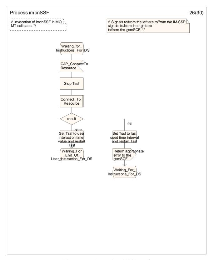
Figure 4.34-26: Process imcnSSF (sheet 26)
