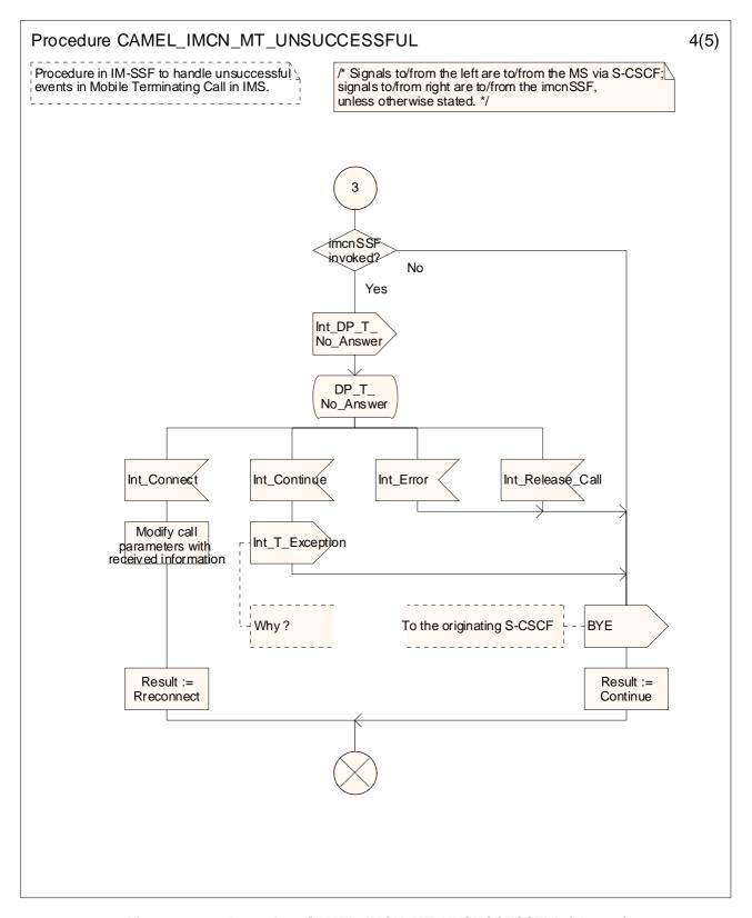
Figure 4.28-4: Procedure CAMEL\_IMCN\_MT\_UNSUCCESSFUL (sheet 4)
