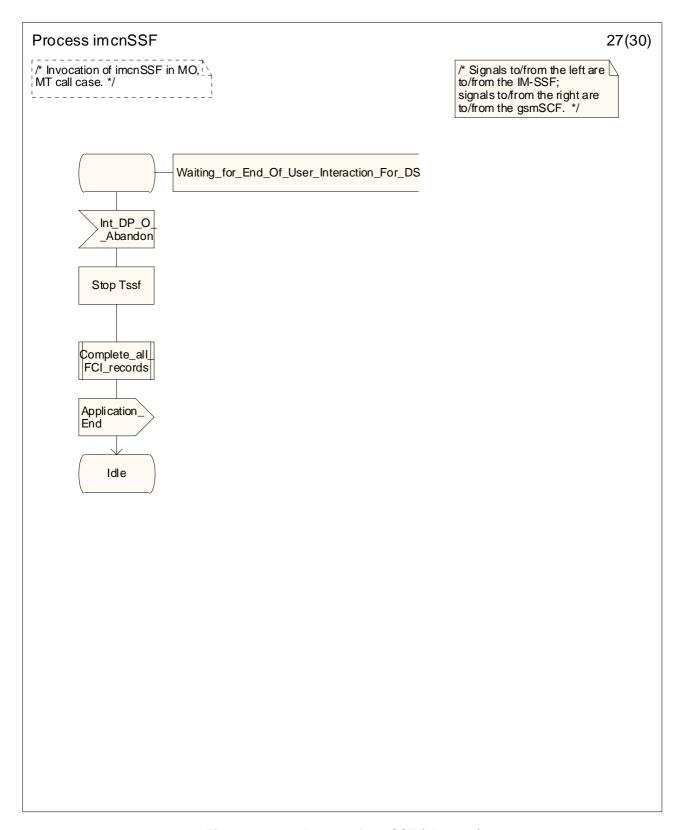
Figure 4.34-27: Process imcnSSF (sheet 27)
