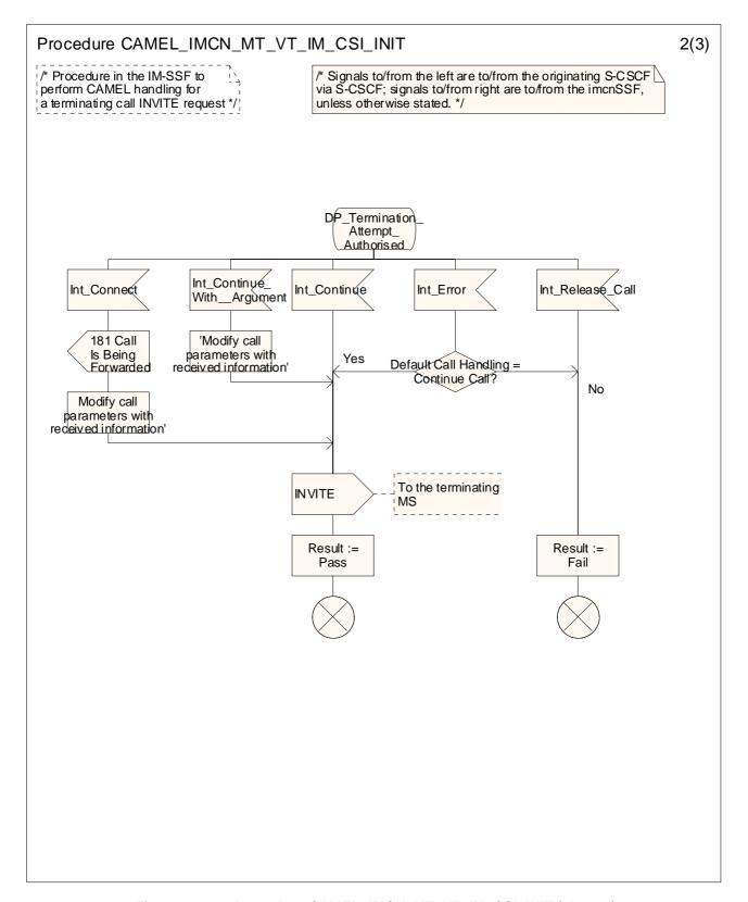
Figure 4.24-2: Procedure CAMEL\_IMCN\_MT\_VT\_IM\_CSI\_INIT (sheet 2)
