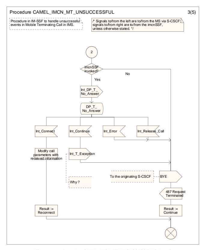
Figure 4.28-3: Procedure CAMEL\_IMCN\_MT\_UNSUCCESSFUL (sheet 3)
