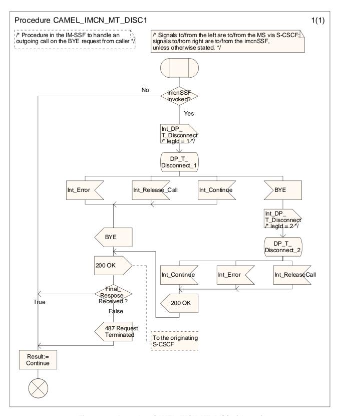
Figure 4.29: Procedure CAMEL\_IMCN\_MT\_DISC1 (sheet 1)
