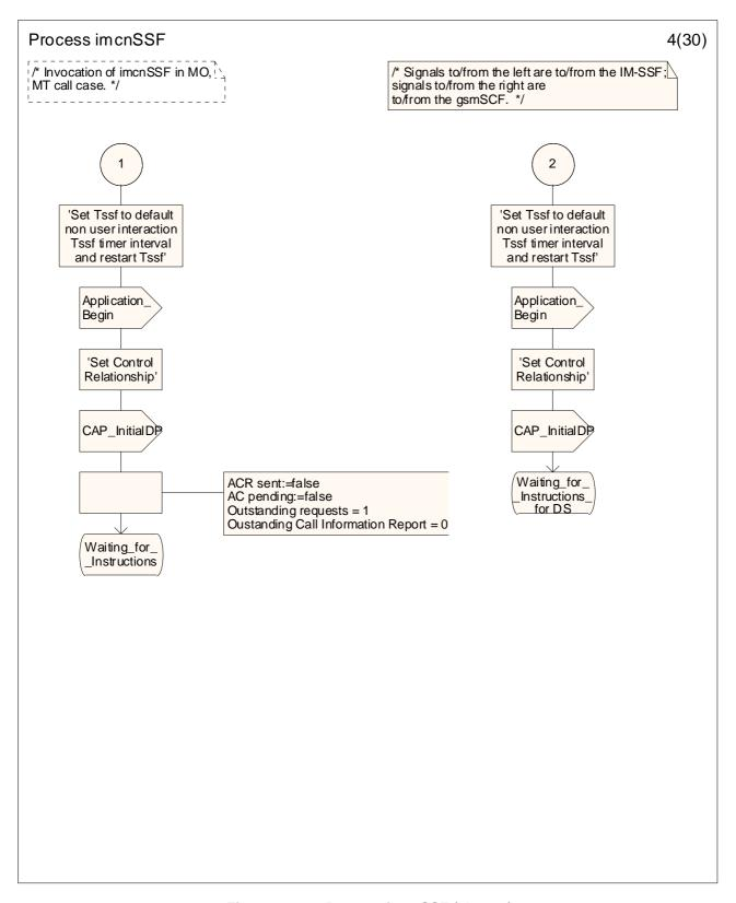
Figure 4.34-4: Process imcnSSF (sheet 4)
