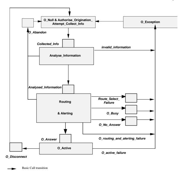
Figure 4.4: Originating CAMEL Basic Call State Model (O-IM-BCSM)
