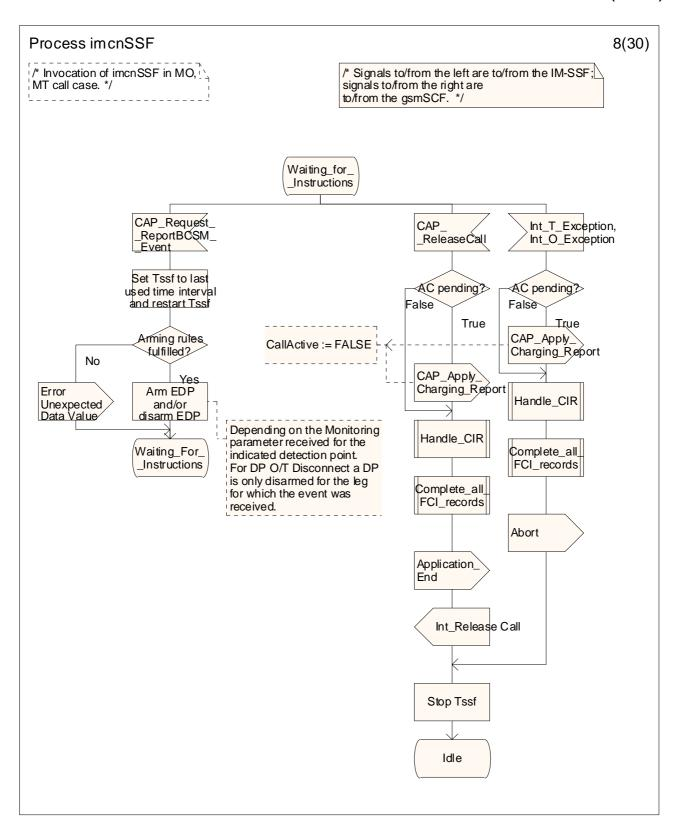
Figure 4.34-8: Process imcnSSF (sheet 8)
