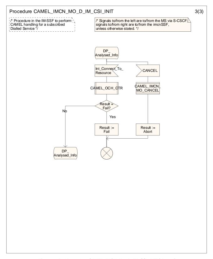
Figure 4.15-3: Procedure CAMEL\_IMCN\_MO\_D\_IM\_CSI\_INIT (sheet 3)
