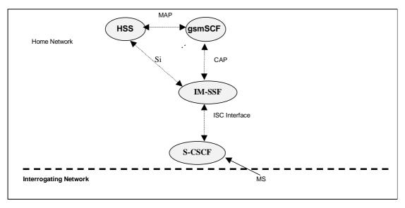
Figure 4.2: Functional architecture for support of CAMEL control of a MO IP Multimedia session
