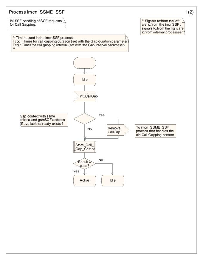
Figure 4.35-1: Process imcn\_SSME\_SSF (sheet 1)
