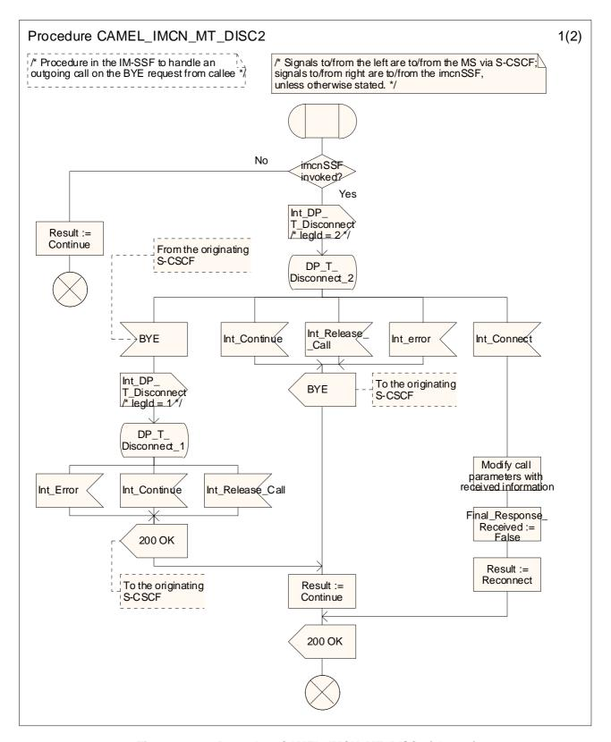
Figure 4.30-1: Procedure CAMEL\_IMCN\_MT\_DISC2 (sheet 1)
