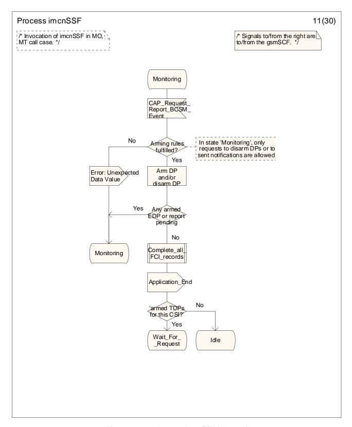
Figure 4.34-11: Process imcnSSF (sheet 11)
