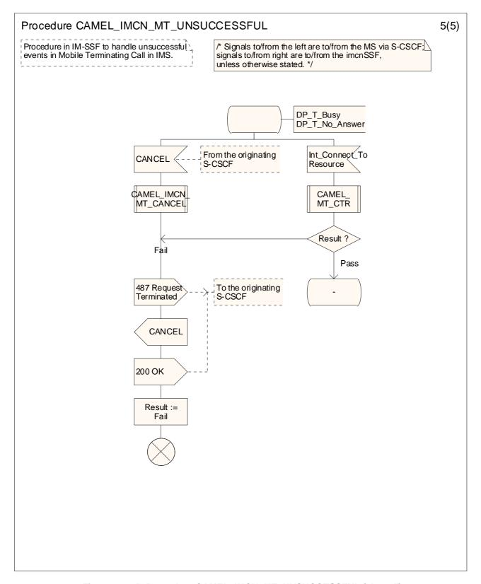
Figure 4.28-5: Procedure CAMEL\_IMCN\_MT\_UNSUCCESSFUL (sheet 5)
