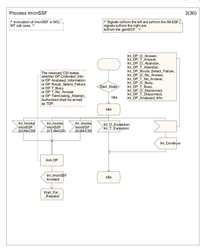
Figure 4.34-2: Process imcnSSF (sheet 2)
