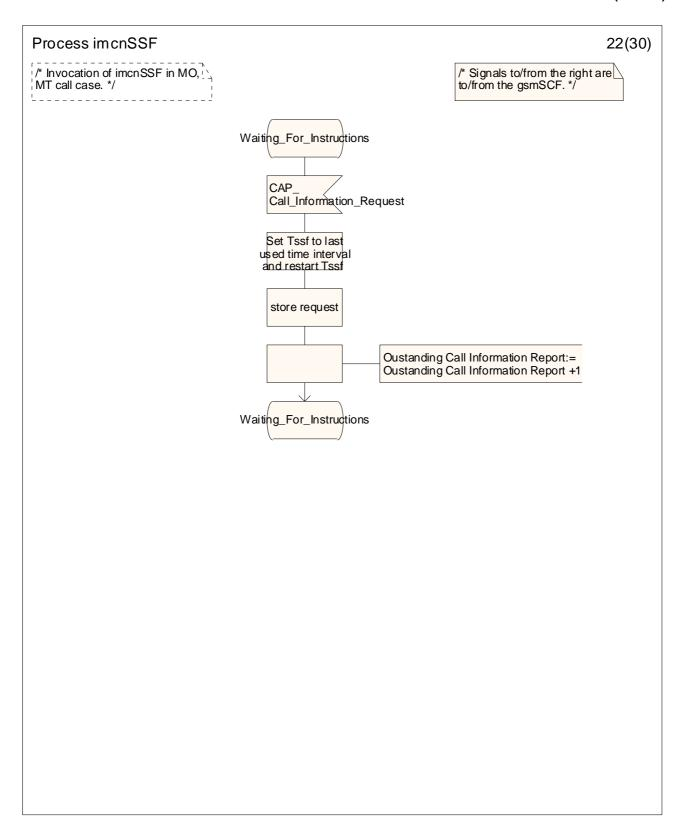
Figure 4.34-22: Process imcnSSF (sheet 22)
