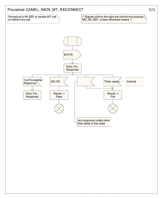
Figure 4.25: Procedure CAMEL\_IMCN\_MT\_RECONNECT (sheet 1)
