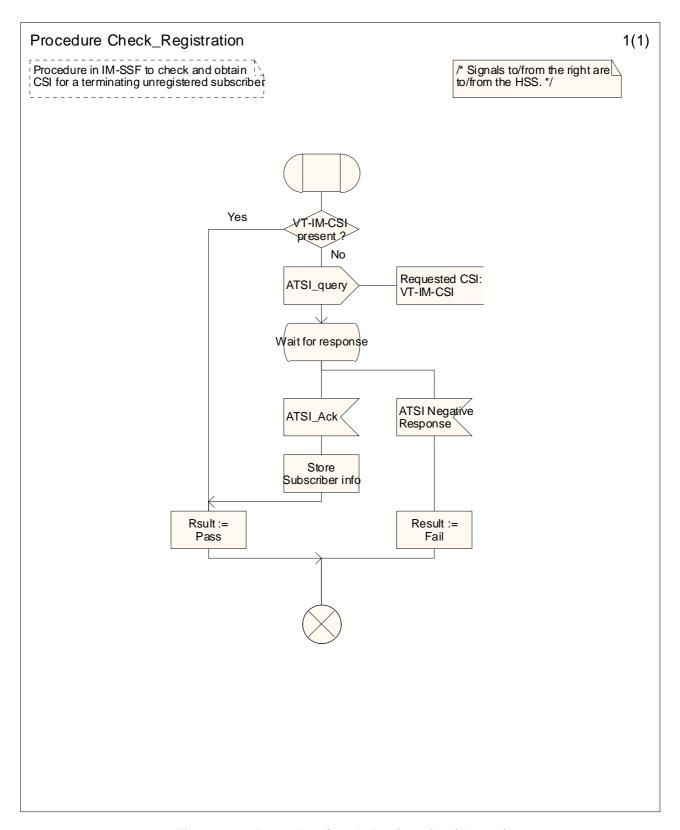
Figure 4.23: Procedure Check\_Registration (sheet 1)
