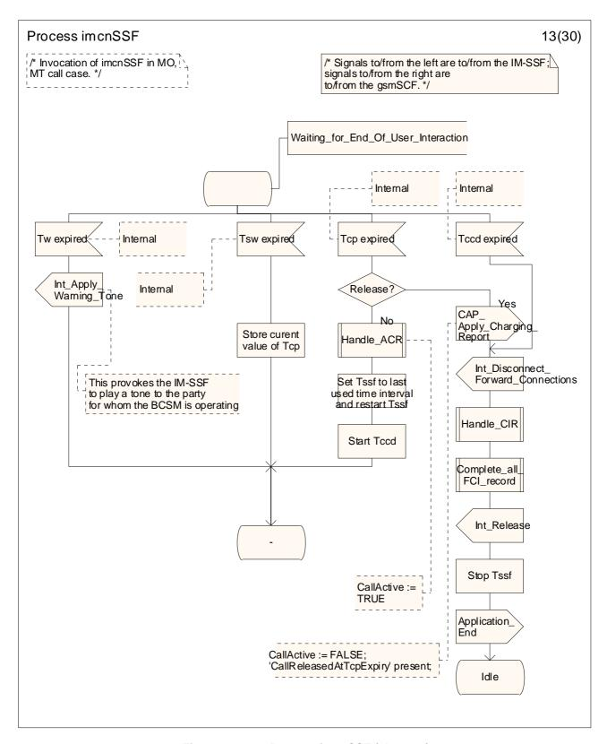
Figure 4.34-13: Process imcnSSF (sheet 13)
