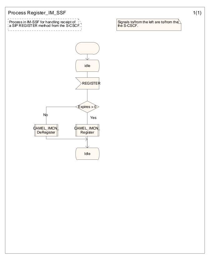
Figure 4.9: Process Register\_IM\_SSF (sheet 1)
