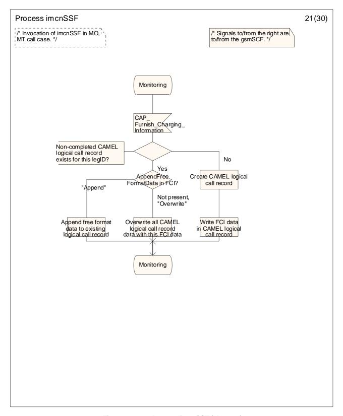
Figure 4.34-21: Process imcnSSF (sheet 21)
