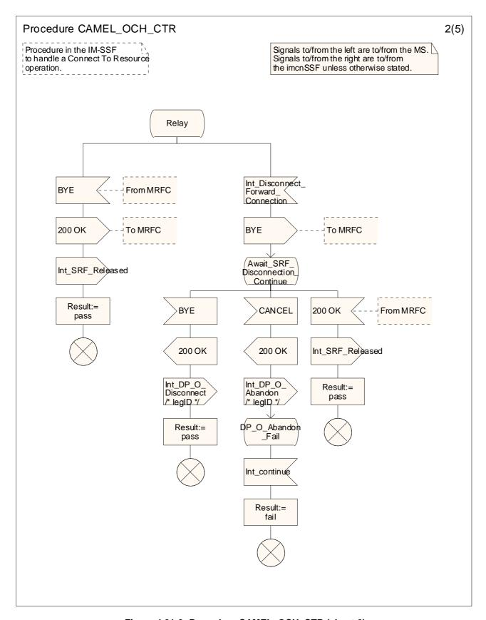
Figure 4.21-2: Procedure CAMEL\_OCH\_CTR (sheet 2)
