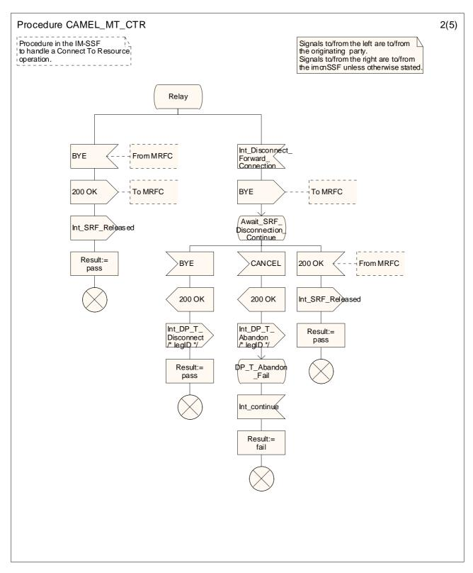
Figure 4.33-2: Procedure CAMEL\_MT\_CTR (sheet 2)
