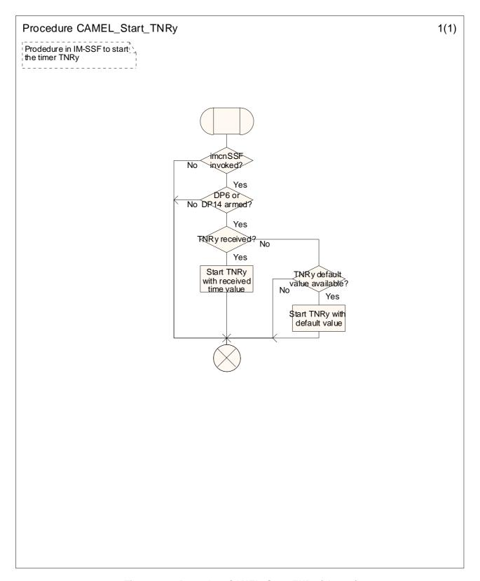
Figure 4.31: Procedure CAMEL\_Start\_TNRy (sheet 1)
