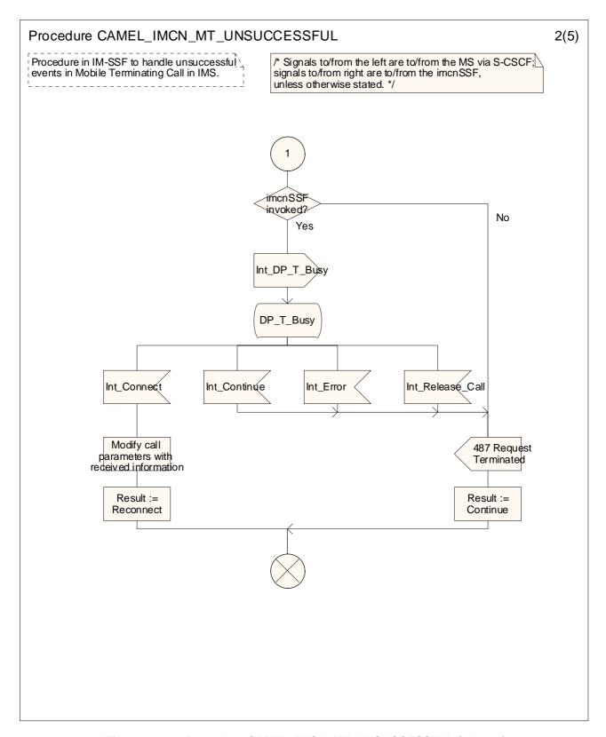
Figure 4.28-2: Procedure CAMEL\_IMCN\_MT\_UNSUCCESSFUL (sheet 2)
