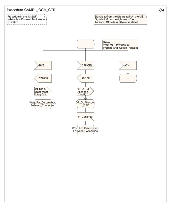
Figure 4.21-3: Procedure CAMEL\_OCH\_CTR (sheet 3)
