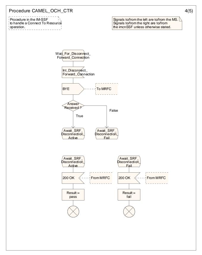
Figure 4.21-4: Procedure CAMEL\_OCH\_CTR (sheet 4)
