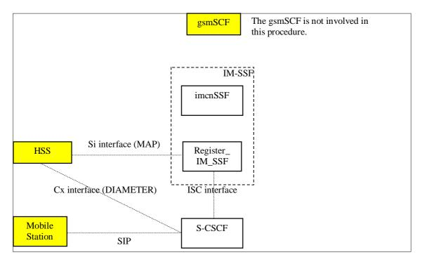
Figure 4.6: SIP Registration into IM-SSF
