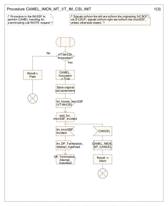
Figure 4.24-1: Procedure CAMEL\_IMCN\_MT\_VT\_IM\_CSI\_INIT (sheet 1)
