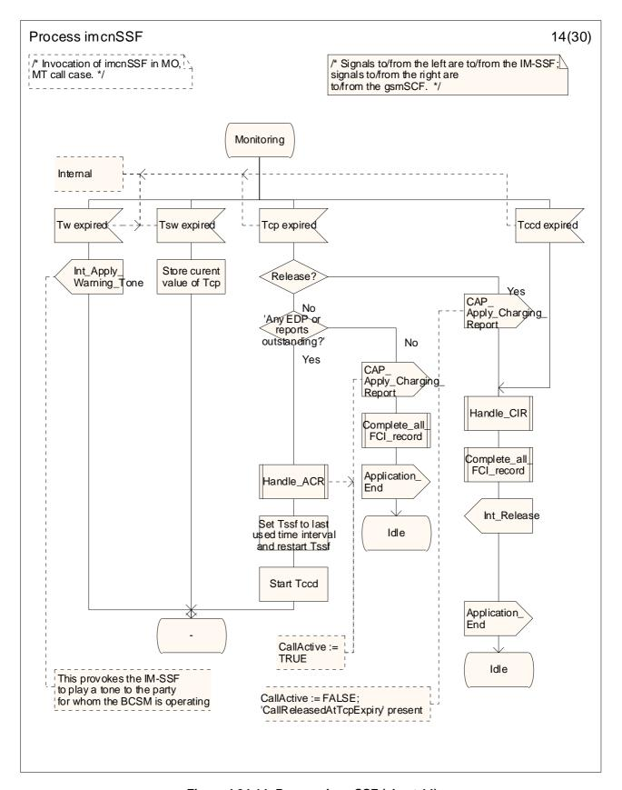
Figure 4.34-14: Process imcnSSF (sheet 14)
