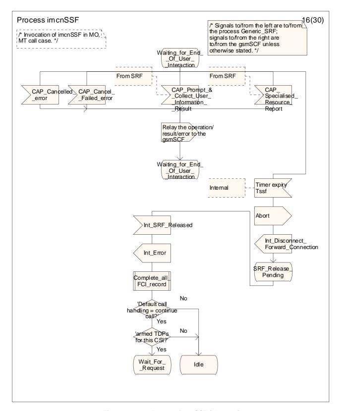
Figure 4.34-16: Process imcnSSF (sheet 16)
