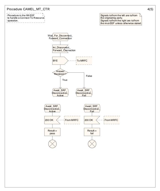
Figure 4.33-4: Procedure CAMEL\_MT\_CTR (sheet 4)
