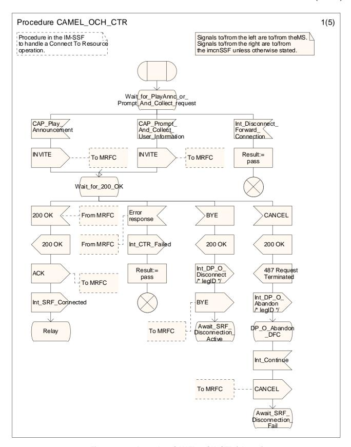
Figure 4.21-1: Procedure CAMEL\_OCH\_CTR (sheet 1)
