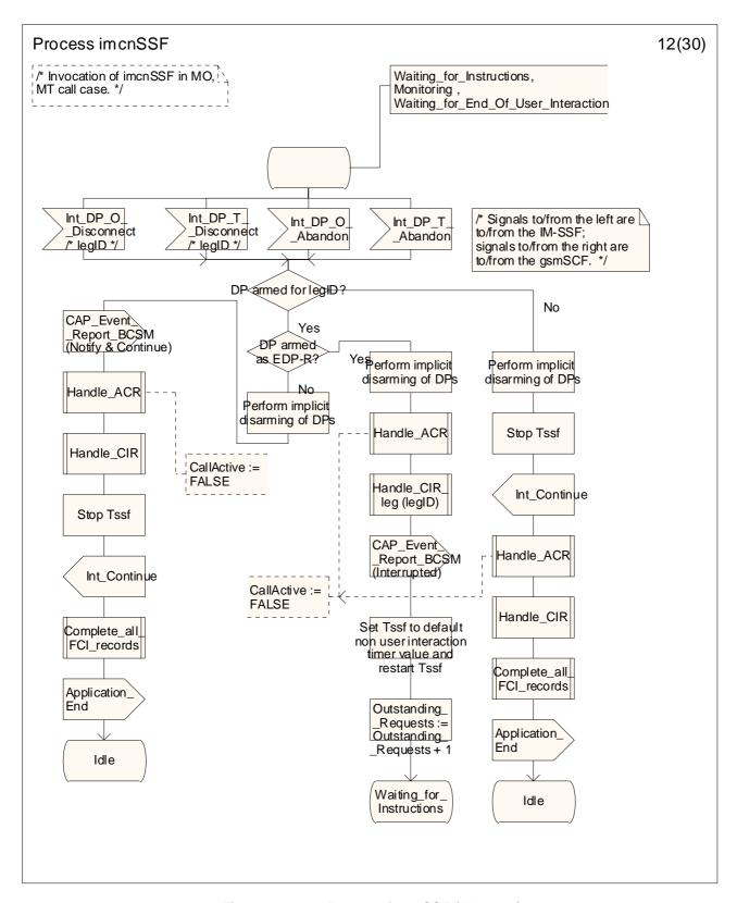
Figure 4.34-12: Process imcnSSF (sheet 12)
