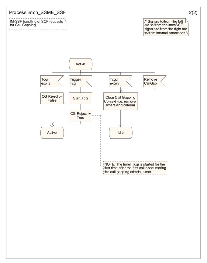
Figure 4.35-2: Process imcn\_SSME\_SSF (sheet 2)
