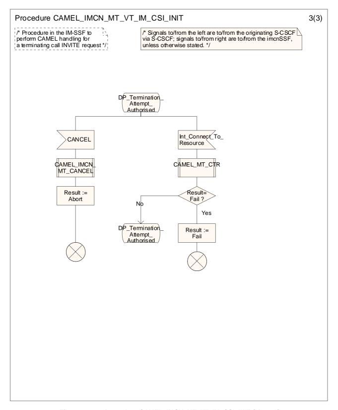
Figure 4.24-3: Procedure CAMEL\_IMCN\_MT\_VT\_IM\_CSI\_INIT (sheet 3)
