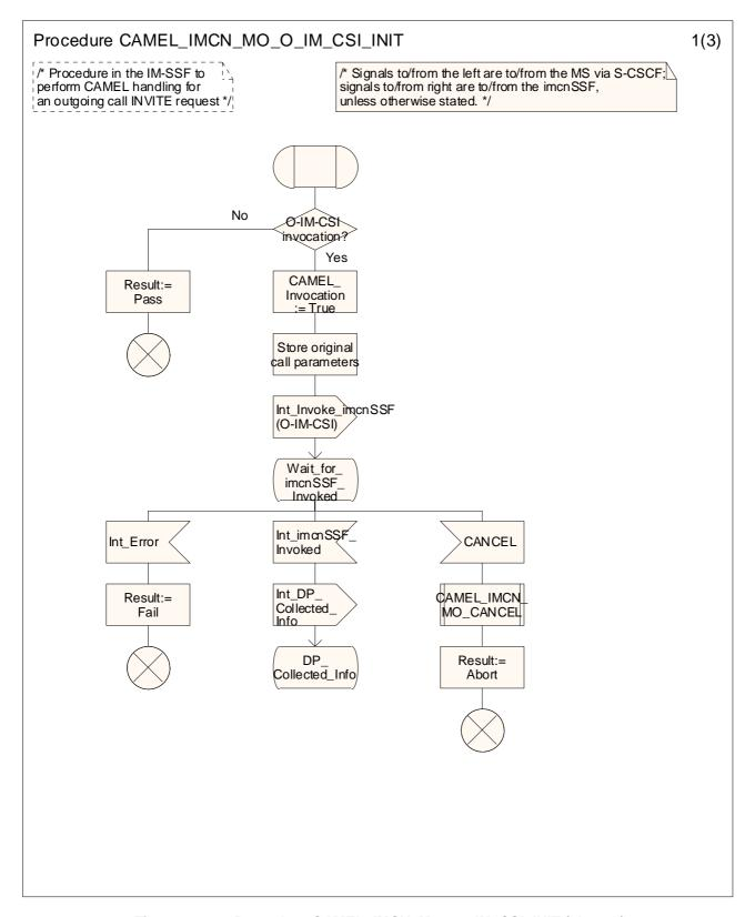
Figure 4.14-1: Procedure CAMEL\_IMCN\_MO\_ O\_IM\_CSI\_INIT (sheet 1)
