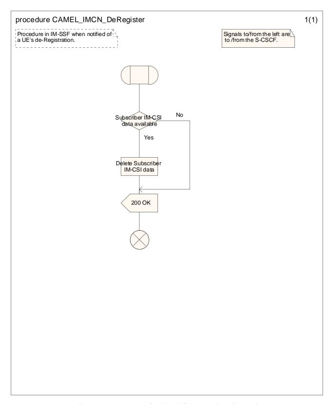
Figure 4.11: Procedure CAMEL\_IMCN\_DeRegister (sheet 1)
