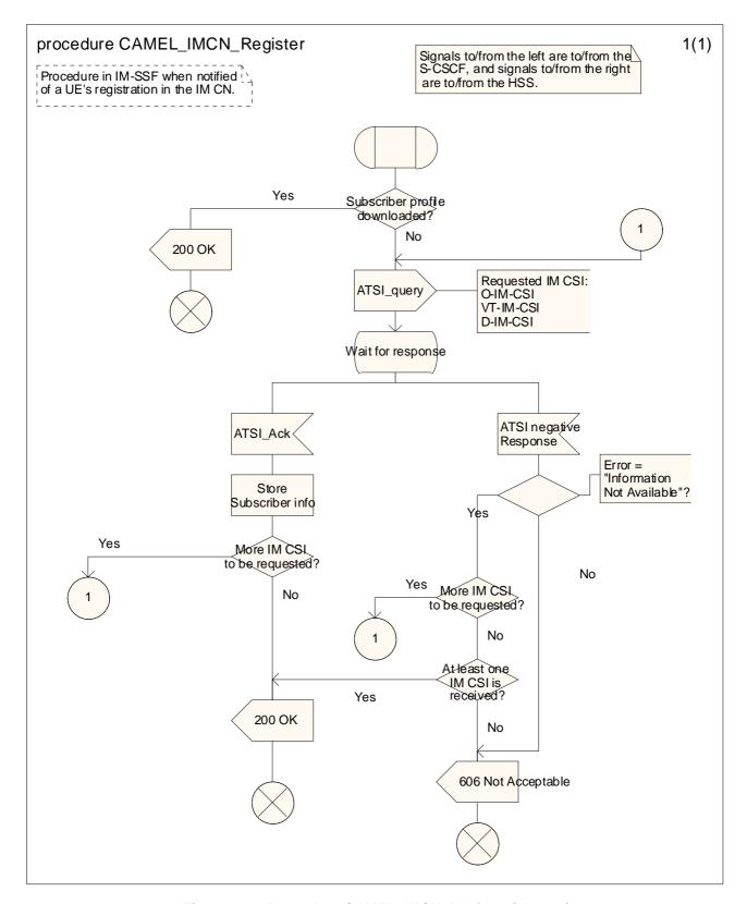
Figure 4.10: Procedure CAMEL\_IMCN\_Register (sheet 1)
