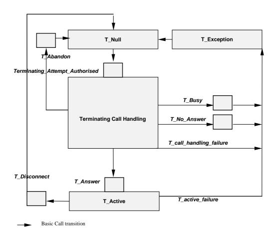
Figure 4.5: Terminating CAMEL Basic Call State Model (T-IM-BCSM)
