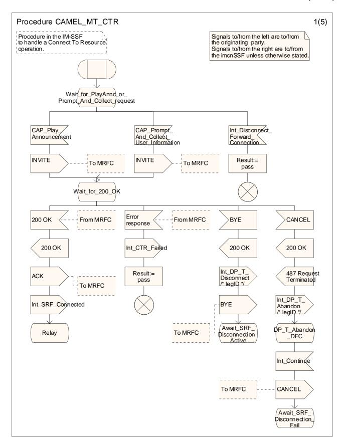
Figure 4.33-1: Procedure CAMEL\_MT\_CTR (sheet 1)
