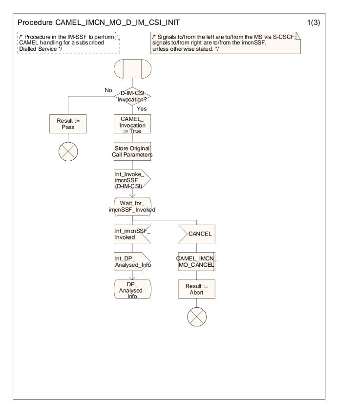
Figure 4.15-1: Procedure CAMEL\_IMCN\_MO\_D\_IM\_CSI\_INIT (sheet 1)
