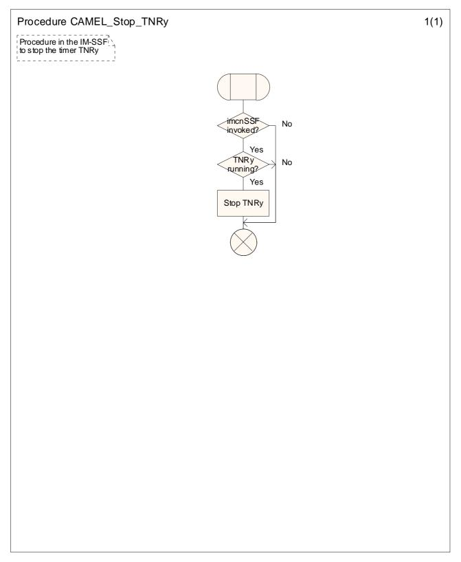
Figure 4.32: Procedure CAMEL\_Stop\_TNRy (sheet 1)
