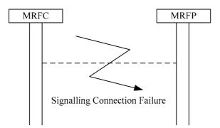
Figure 6.1.2.1: Signalling connection failure
