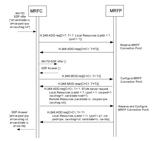
Figure 6.2.18.1: Procedure for interactive connectivity establishment using ICE lite towards the offerer
