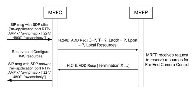
Figure 6.2.2.1.1: Procedure to indicate Video ROI using FECC
