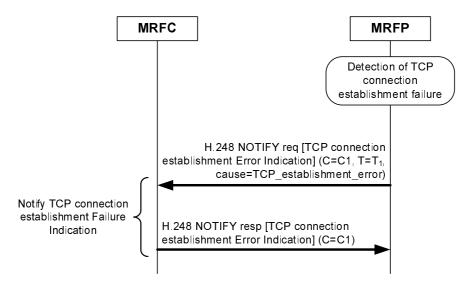
Figure 6.2.20.2.1: TCP connection establishment Failure Indication
