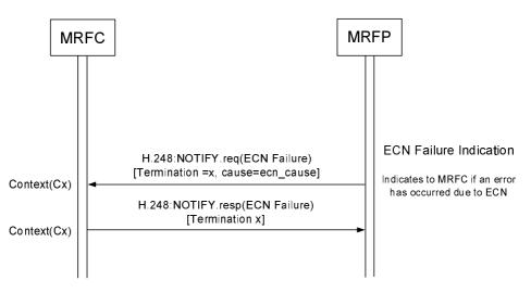
Figure 6.2.14.3.1: Procedure to Report ECN Failure
