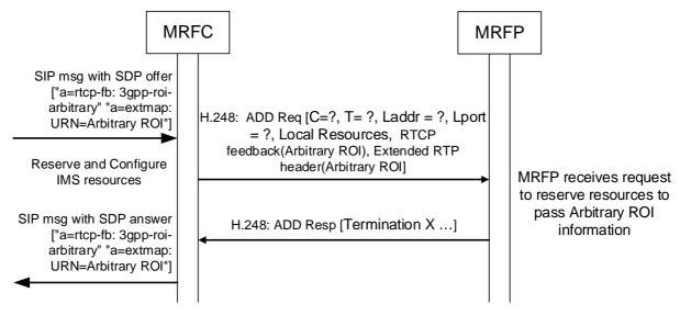
Figure 6.2.22.3.1: Procedure to indicate Arbitrary ROI mode
