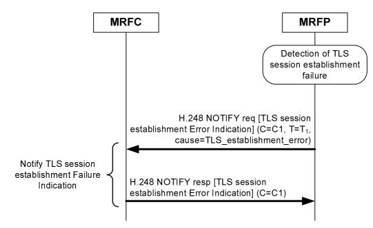
Figure 6.2.19.4.1: TLS session establishment Failure Indication
