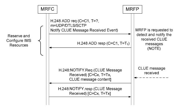
NOTE: Other IEs for Telepresence are shown in CLUE data channel establishment procedure. Figure 6.2.21.2.1: Procedure for detection and notification of CLUE message received
