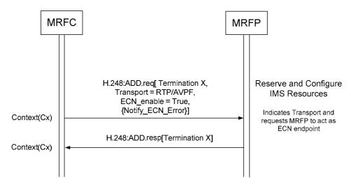
Figure 6.2.14.2.1: Procedure to Request ECN
