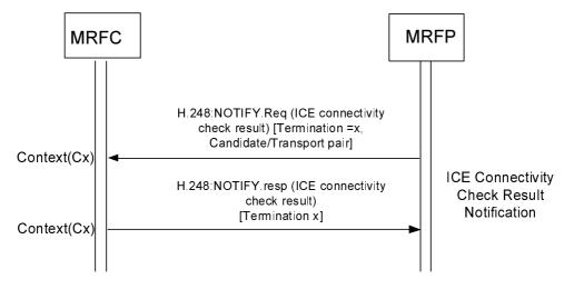
Figure 6.2.18.3.1: Procedure to report ICE connectivity check result
