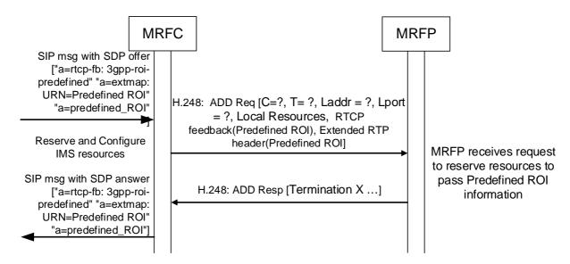
Figure 6.2.22.2.1: Procedure to indicate Predefined ROI mode
