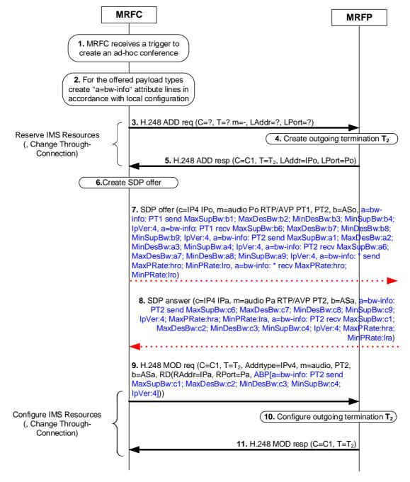
Figure 6.2.23.2: Multimedia conference establishment ("dial-out" procedure) with support of the enhanced bandwidth negotiation mechanism
