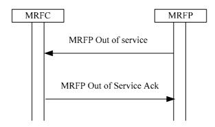
Figure 6.1.2.2: MRFP indicates the Failure/Maintenance locking
