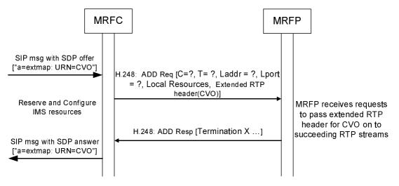
Figure 6.2.16.1: Procedure to indicate RTP extension header for CVO
