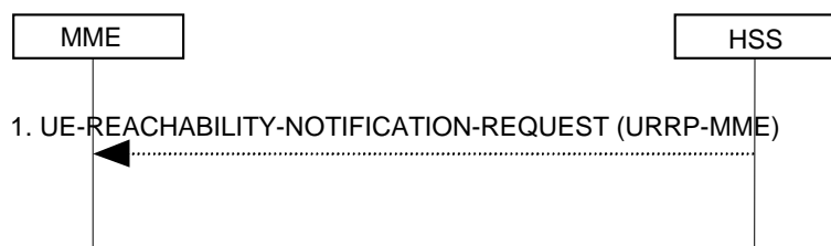
Figure 5.3.11.2-1: UE Reachability Notification Request Procedure
