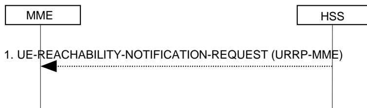
Figure 5.3.11.2-1: UE Reachability Notification Request Procedure
