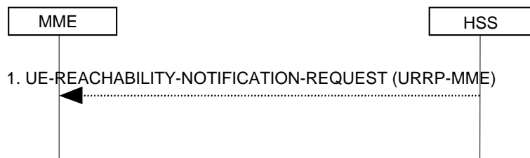
Figure 5.3.11.2-1: UE Reachability Notification Request Procedure
