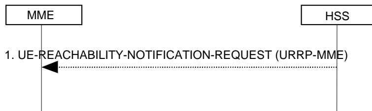
Figure 5.3.11.2-1: UE Reachability Notification Request Procedure
