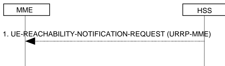
Figure 5.3.11.2-1: UE Reachability Notification Request Procedure
