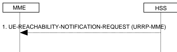
Figure 5.3.11.2-1: UE Reachability Notification Request Procedure
