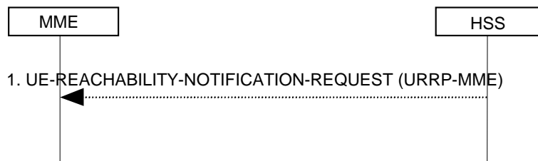
Figure 5.3.11.2-1: UE Reachability Notification Request Procedure
