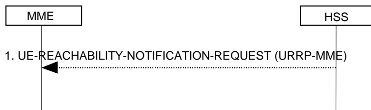
Figure 5.3.11.2-1: UE Reachability Notification Request Procedure
